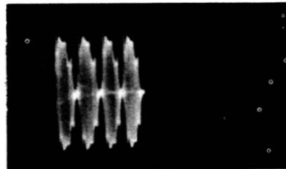
Fig. 11-6. Envelope changes with receiver tuning due to incidental f-m.
