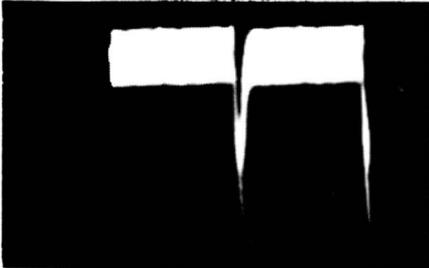
Fig. 5-17. Excessive video in the stripped-sync waveform.
