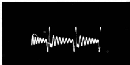
(B) *Breakdown in high-voltage winding.*
