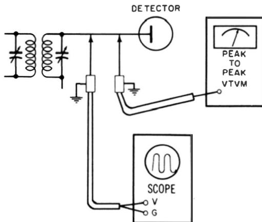
Fig. 11-2. Calibrating the probe and the scope.
