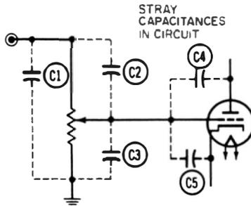
Fig. 2-18. Potentiometer gain control.
