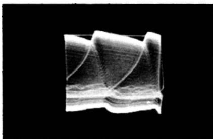
Fig. 6-10. Waveform at point B when C5 is open.
