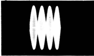
(A) Output waveform from a-m generator.
