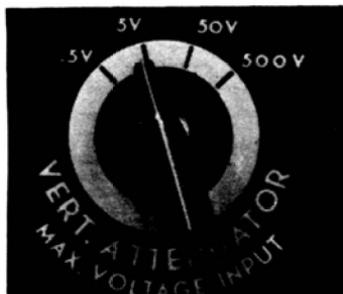
Fig. 2-21. Step attenuator with maximum input voltages marked.
