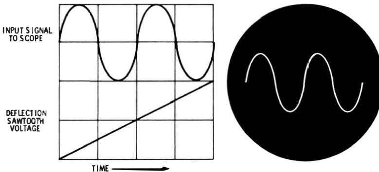
**Fig. 2-16. Display of sine wave when the sweep frequency is one-half the signal frequency.**
