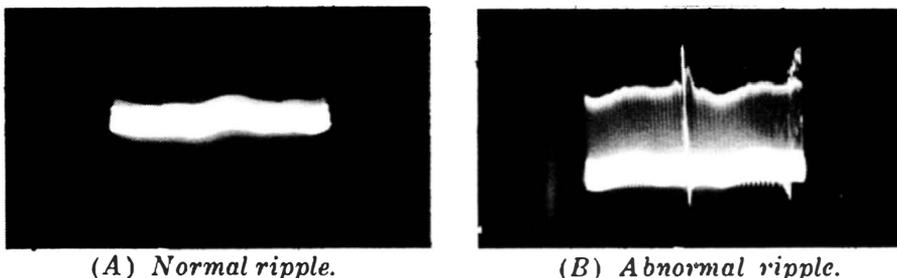
Fig. 10-2. Ripple wave at cathode of audio-output tube when 200-mfd bypass capacitor is defective.
