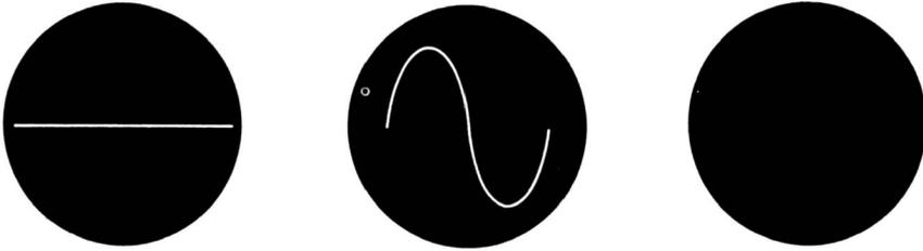
(A) *Horizontal trace.* (B) *Desired pattern.* (C) *Blank screen.*
