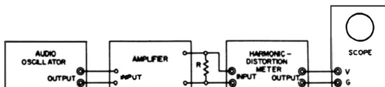
Fig. 12-7. Scope identifies the nature of distortion.
