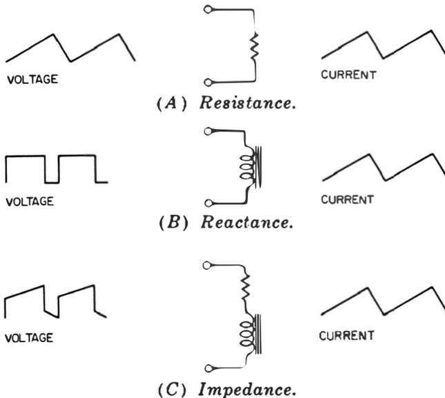
**Fig. 7-3. Voltage waveforms needed for a sawtooth current.**
