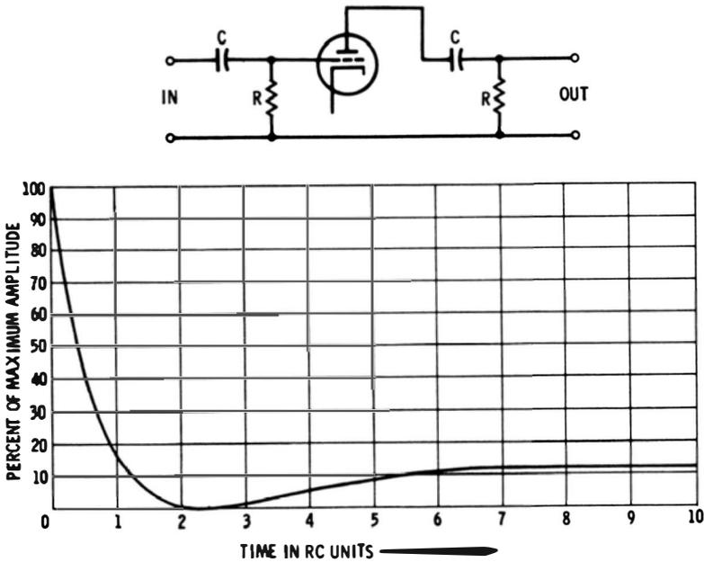
Fig. 1-10. Universal time-constant chart for r-c coupled amplifier with two r-c sections.
