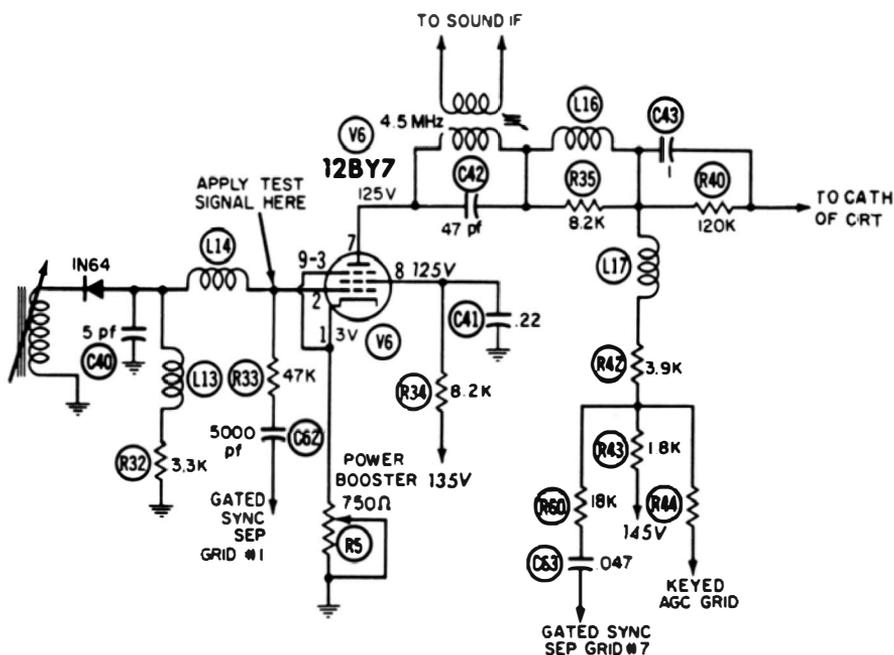
Fig. 9-9. Apply test signal at grid—not at plate.
