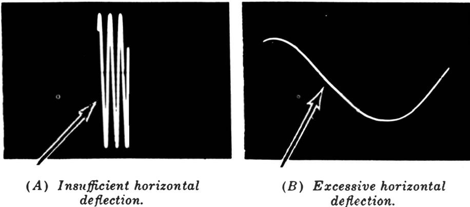
**Fig. 2-23. Horizontal-gain control effect.**
