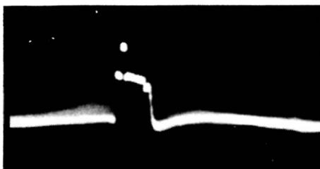
**Fig. 4-25. Video signal with white portions compressed.**
