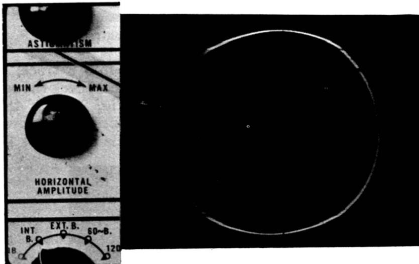
Fig. 2-6. Astigmatism control completes the edge focus.
