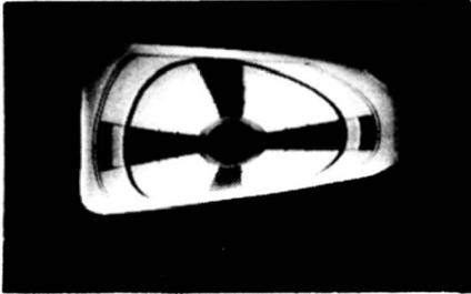
**Fig. 7-13. Keystoning is not always caused by yoke trouble.**
