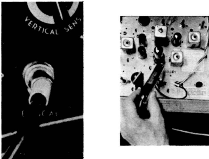
**Fig. 3-1.** Coaxial cable prevents pickup of stray fields.
