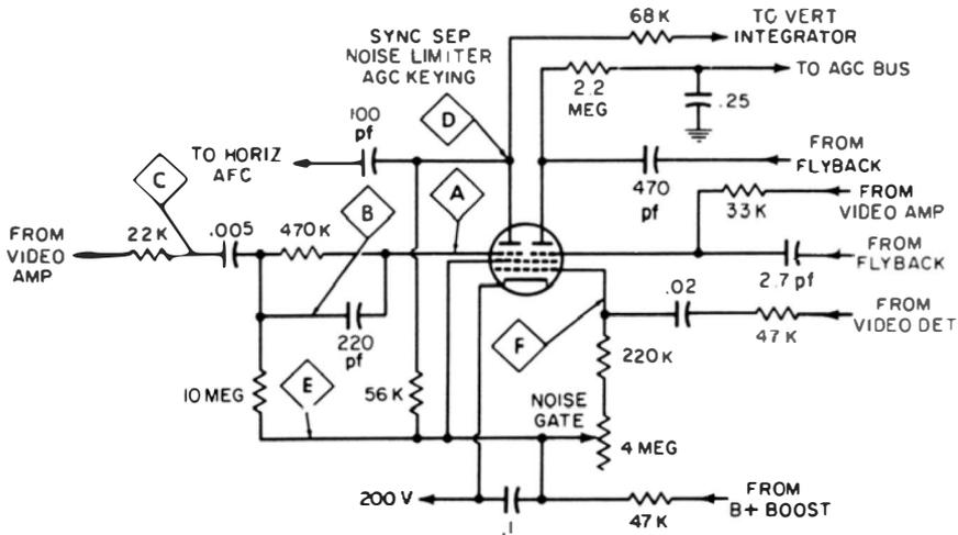
Fig. 5-1. Typical sync-separator configuration.
