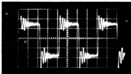
**Fig. 3-5. Square-wave test showing the effect of using a service-type low-capacitance probe with a lab-type scope.**
