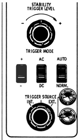
Fig. 2-43. Trigger controls of a triggered-sweep scope.
