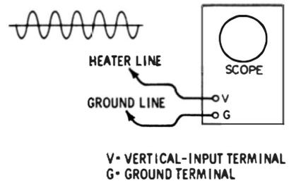
(B) Using external 60-Hz voltage.
