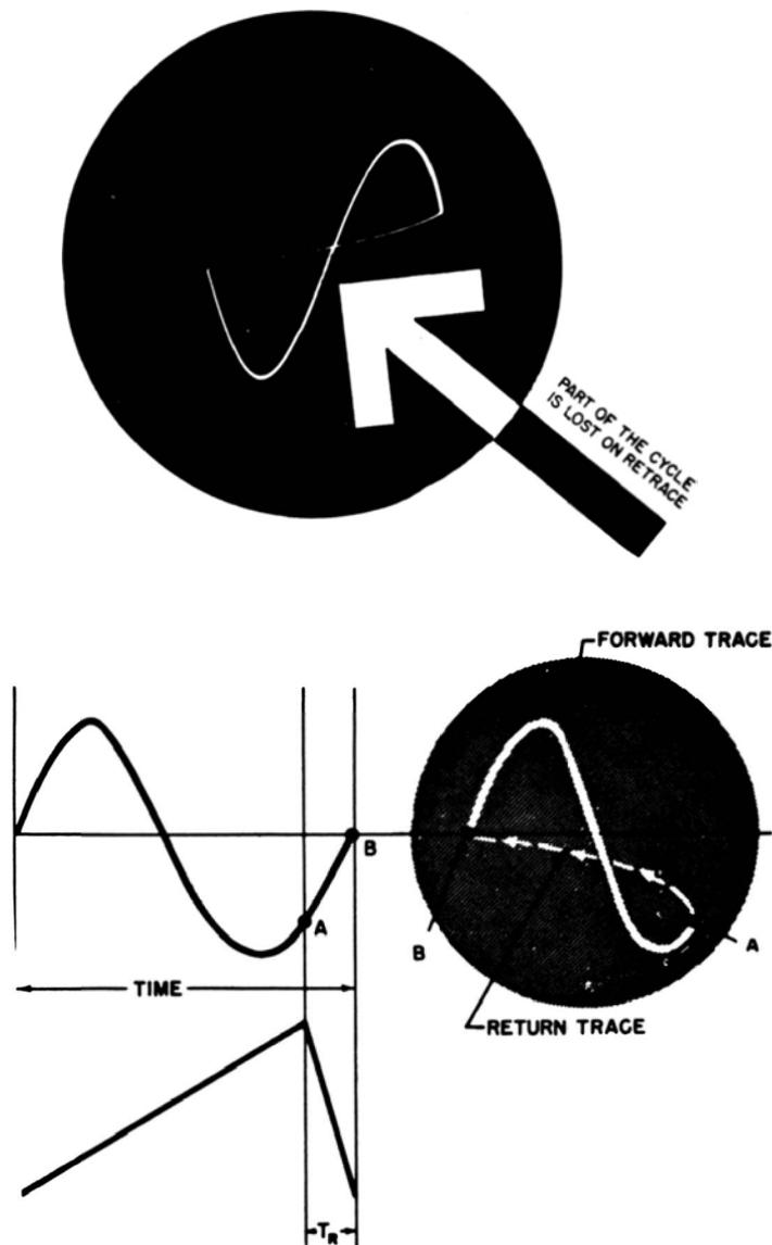
Fig. 2-13. Detail of a single-cycle display.
