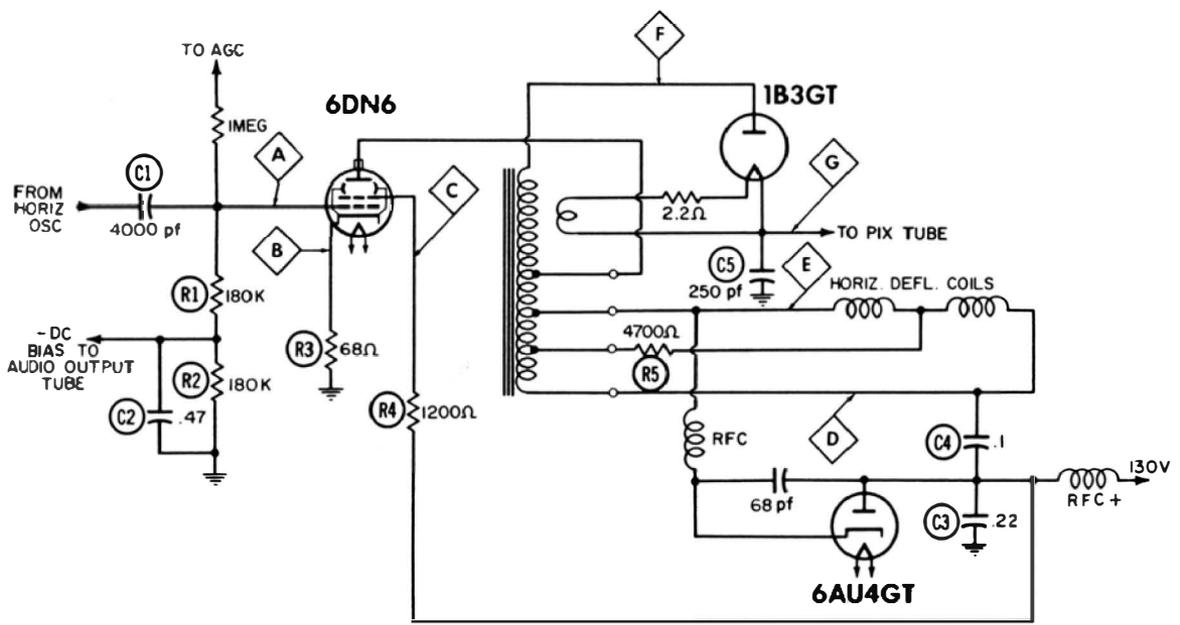
Fig. 7-2. Typical horizontal-sweep configuration.
