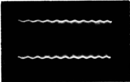
Fig. 9-2. Apparent a-m limiter output, due to incidental f-m.
