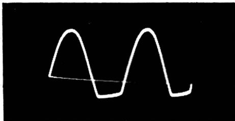
Fig. 2-22. Sine wave clipped by overloading.
