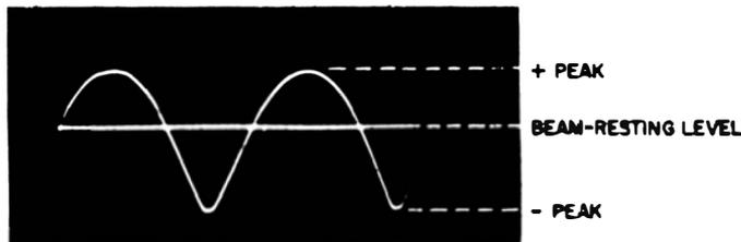
Fig. 2-35. The beam-resting level of a scope shows the positive and negative portions of a waveform.
