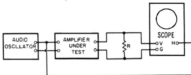
**Fig. 12-3. Amplifier linearity check.**
