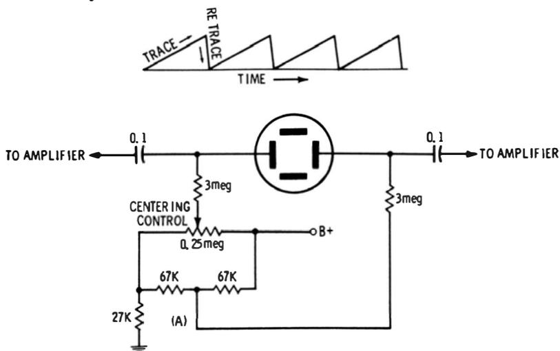
**Fig. 2-9. A sawtooth voltage deflects the beam back and forth linearly.**
