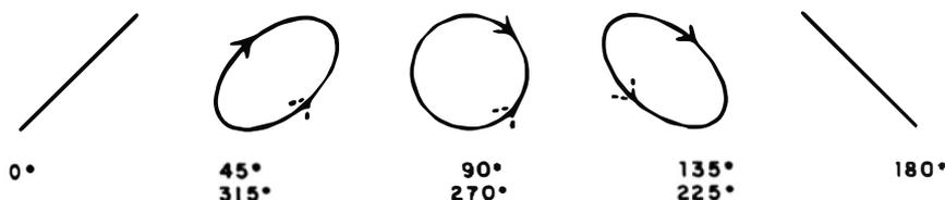
Fig. 12-4. Typical phase-shift patterns.
