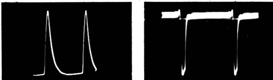
Fig. 5-16. Sync-separator outputs from two different receivers.
