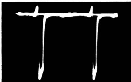
Fig. 5-4. Normal separated sync signal.
