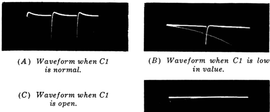
Fig. 8-15. Waveforms at point A of Fig. 8-14.
