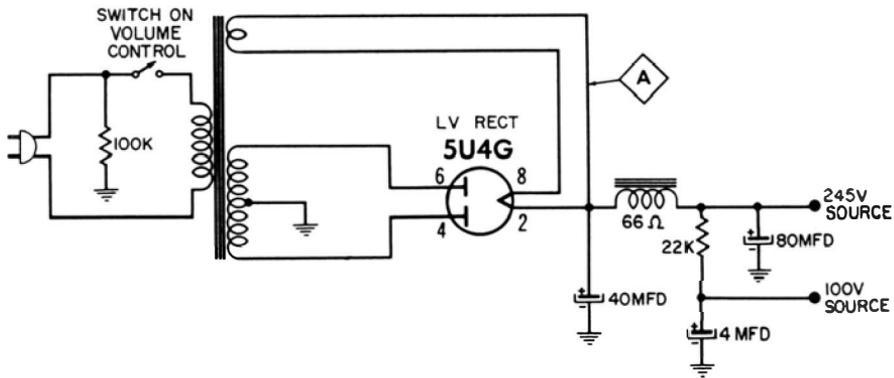
Fig. 10-3. A transformer-type power supply.
