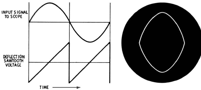
**Fig. 2-15. Display of sine wave when the sweep frequency is double the signal frequency.**
