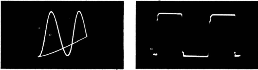
Fig. 2-34. These waveforms have the same peak-to-peak voltages, but their rms values are different.
