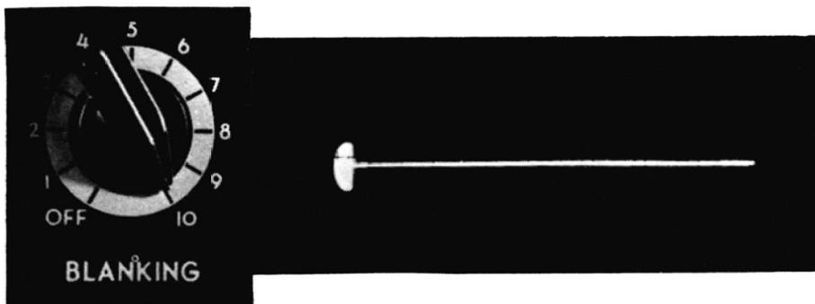
Fig. 2-26. Retrace blanking control, and pattern resulting from misadjustment.
