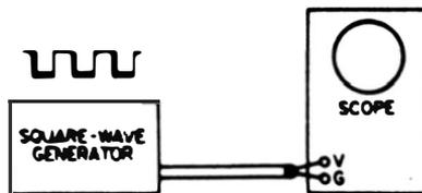
Fig. 12-10. Checking the transient response of a scope.
