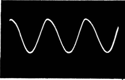
Fig. 12-5. Distorted sine wave.
