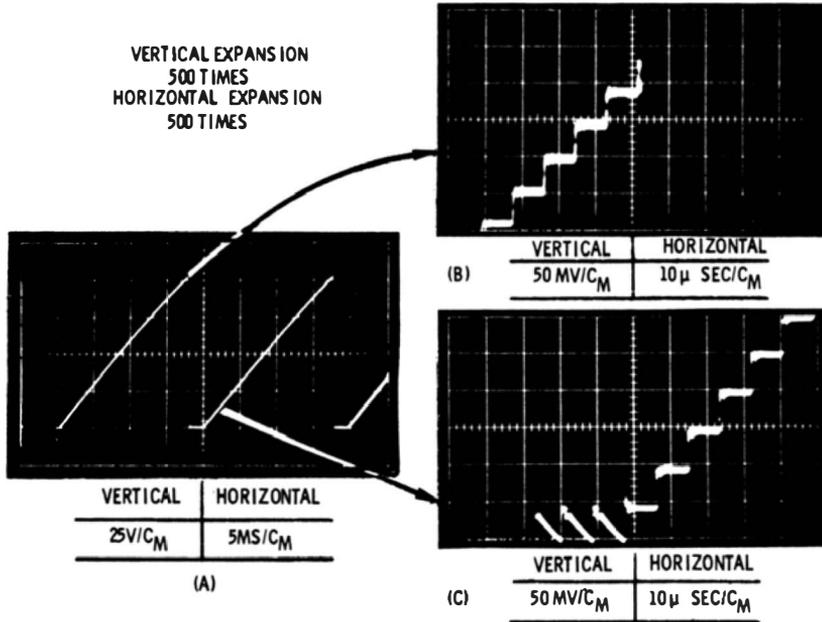
Fig. 2-42. “Stairstep” voltage waveform expanded 500 times.
