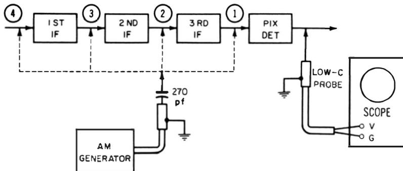
Fig. 4-18. Stage-gain test setup.
