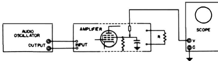
Fig. 12-6. Checking a screen bypass capacitor.
