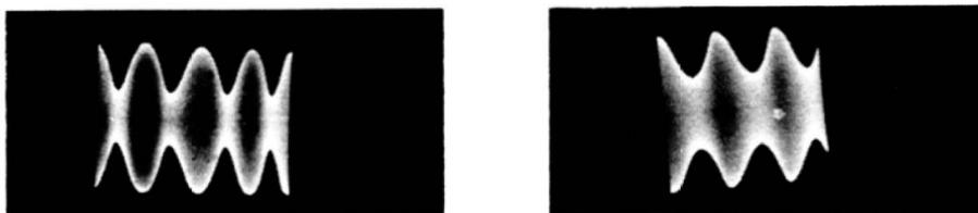
Fig. 11-7. Envelope variation at lower-percentage modulation.
