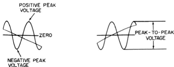
Fig. 2-30. Meaning of positive-peak, negative-peak, and peak-to-peak voltages.
