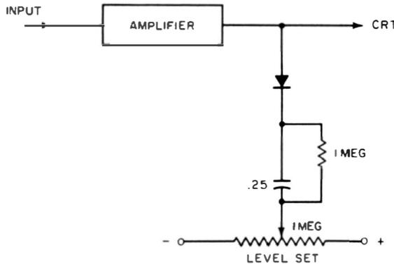
Fig. 5-10. Circuit for automatic centering.
