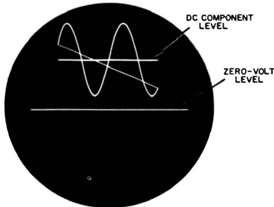
Fig. 2-37. Response of a d-c scope to a-c voltage with a d-c component.
