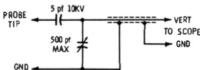
Fig. 3-13. Typical high-voltage capacitance-divider probe.
