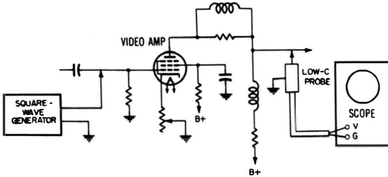
Fig. 3-20. Video amplifier serves as utility wide-band amplifier.
