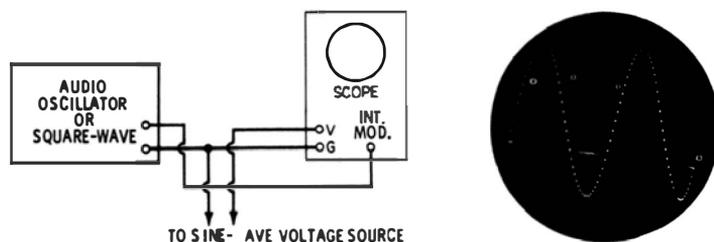
Fig. 2-29. Instantaneous voltages "marked" and timed by intensity modulation of the scope.
