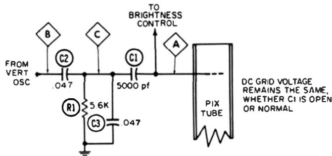
Fig. 8-14. Vertical-retrace blanking circuit.
