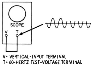
(A) Using internal 60-Hz voltage.
