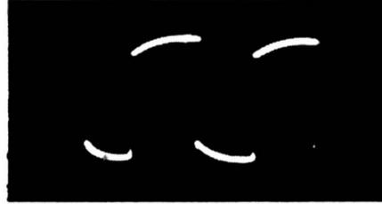
**Fig. 12-12.** Low-frequency overcompensation causes top of square wave to slope uphill.
