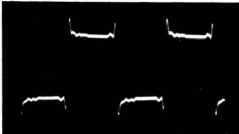
**Fig. 4-32. Normal 100-kHz square-wave response of a high-performance video amplifier.**
