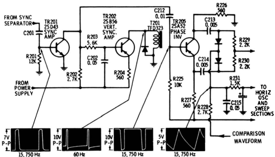
Fig. 5-15. A typical transistor sync amplifier and afc section, with separate vertical-sync amplifier.
