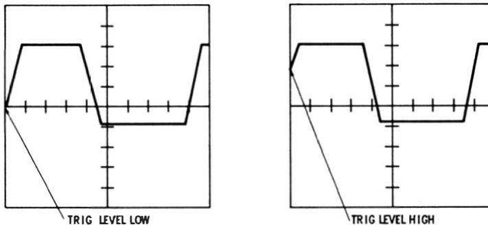
**Fig. 2-45. This waveform is being triggered along its positive slope (rising interval).**
