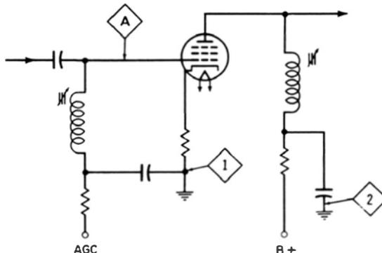
Fig. 4-19. Grounds (1) and (2) are at different 40-MHz potential.
