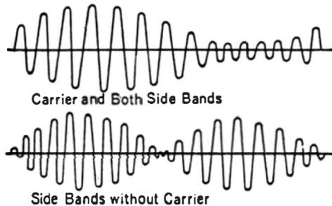
**Fig. 11-14. Suppression of the carrier results in a double-frequency modulation envelope.**
