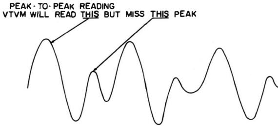
**Fig. 5-27. Waveshape having two different values of peak voltage.**
