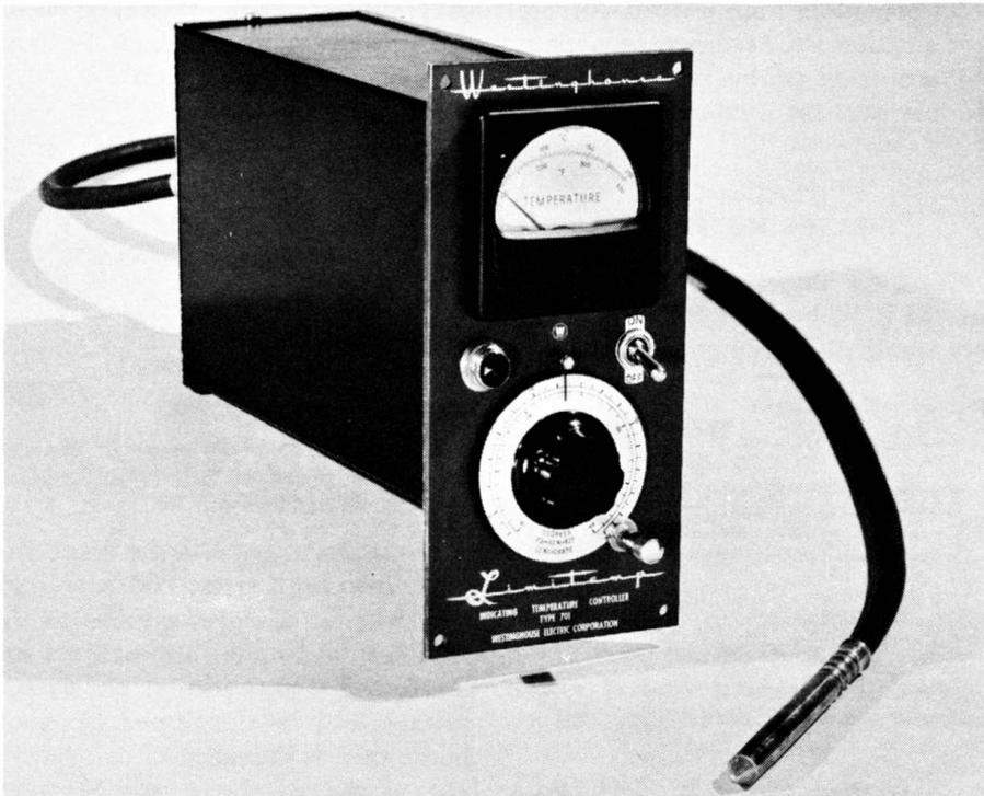
**Fig. 7-42. Temperature-controlling and -indicating instrument.**
