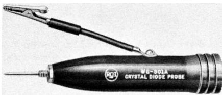
**Fig. 4-28.** This crystal diode-detector probe is slipped over the regular DC isolation probe for which it was designed. (Courtesy of Radio Corporation of America.)
