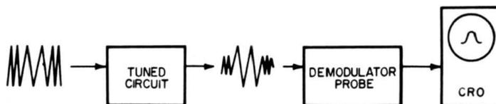
**Fig. 5-1. Tuned circuit changes FM signal to AM signal; demodulator probe extracts information from AM signal; oscilloscope displays information.**
