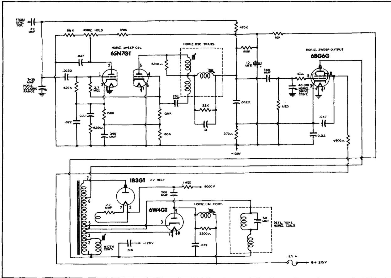
Figure 1. Horizontal Sweep System.
