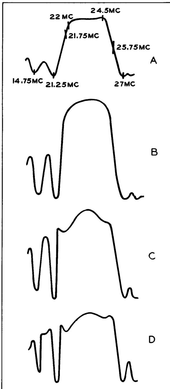
Figure 25. (A) Ideal Response Curve. (B) Bias at -2.5 Volts. (C) Bias at -2.0 Volts. (D) Bias at -1.5 Volts.
