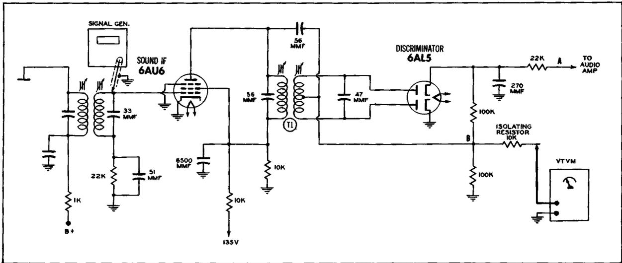
Figure 16. How to Connect a VTVM and Signal Generator for Discriminator Alignment.
