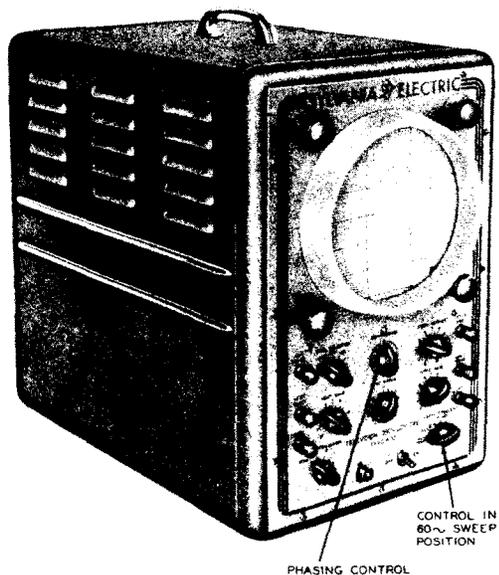
Figure 15. An Oscilloscope which can Provide its own 60 Cycle Sweep and Phasing Control. Courtesy Sylvania Electric Products Company.
