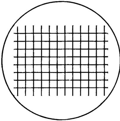
Figure 22. A Cross-Hatch Pattern Possessing the Proper 4:3 Aspect Ratio.
