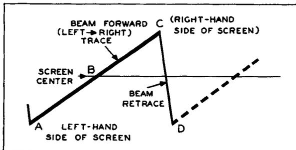
Figure 5. The most Common Type of Voltage which Is Applied to the Horizontal Deflection Plates in a CRT Is the Saw-Tooth Wave.
