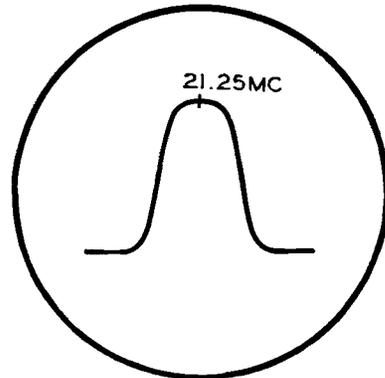
Figure 19. The Sound IF Response Curve of the Circuit in Figure 18 as Given by the Manufacturer.
