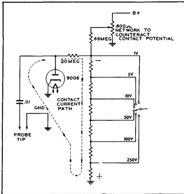
Figure 8. To Counteract the Negative Potential developed by the Contact Potential, a Small Positive Voltage is Fed Into the Circuit.
