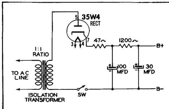
Figure 33. By Using an Isolation Transformer, There Is no Direct Connection Between the Power Line and the Receiver.
