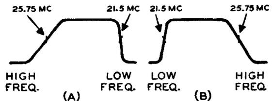
Figure 29. (A) A Video IF Response Curve That May be Obtained on the Scope Screen. Note That the High IF Frequencies Are at the Left and Low IF Values at the Right. (B) By Flipping the Phase Reversal on the Jackson Generator, the Curve in (A) Is Reversed to the Form Shown in (B).
