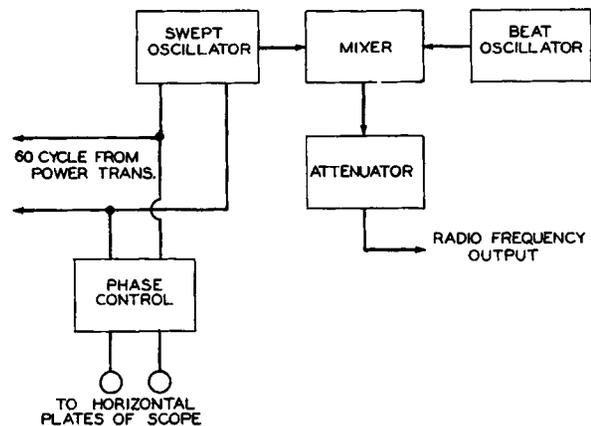
Figure 36. A Block Diagram (Simplified) of the G.E. Sweep Generator.
