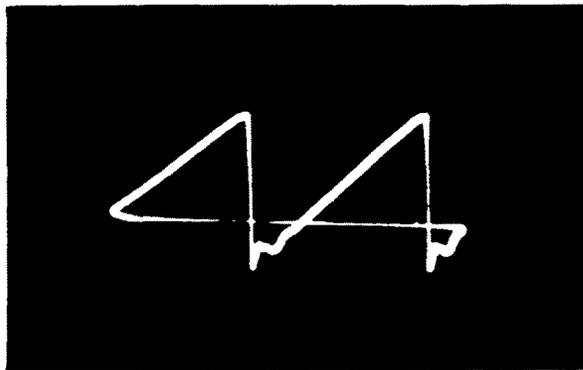
Figure 2. The Waveform Normally Present at the Grid of the Horizontal Output Amplifier in Figure 1.
