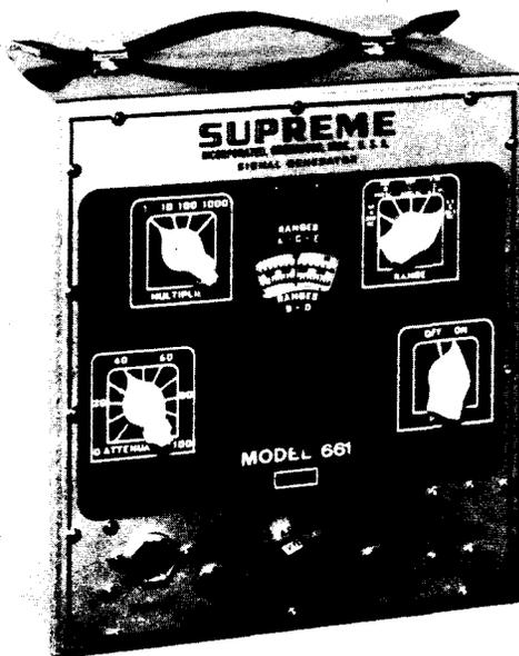
Figure 7. A Supreme Model 661 AM Signal Generator.
