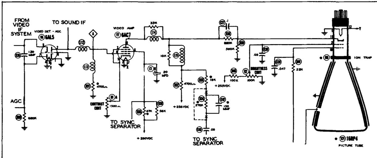
Figure 48. A One-Stage Video Amplifier System.
