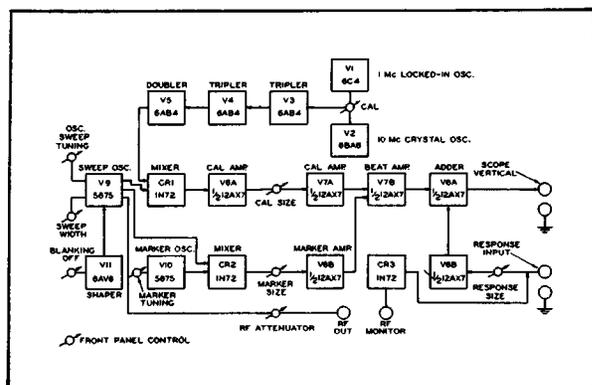
Figure 14. Block Diagram of the RCA UHF Sweep-Marker Generator.
