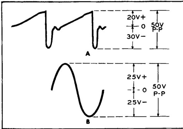
Figures 12A and B. The VTVM Must Contain a Special Circuit to Indicate Correctly the Peak-to-peak Value of Waves Other Than Sine Waves. See Text.
