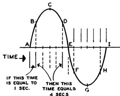
Figure 10. The Rate of Change Varies at Different Points on a Sine Wave.
