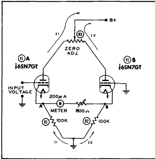
Figure 1. The Basic Circuit of a Modern VTVM.
