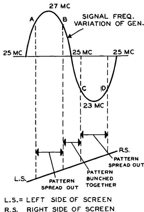
Figure 14. A Sinusoidal Frequency Variation, Coupled With a Linear Saw-tooth Beam Motion, Will Produce a Pattern Bunched in the Middle and Stretched Out at the Ends.
