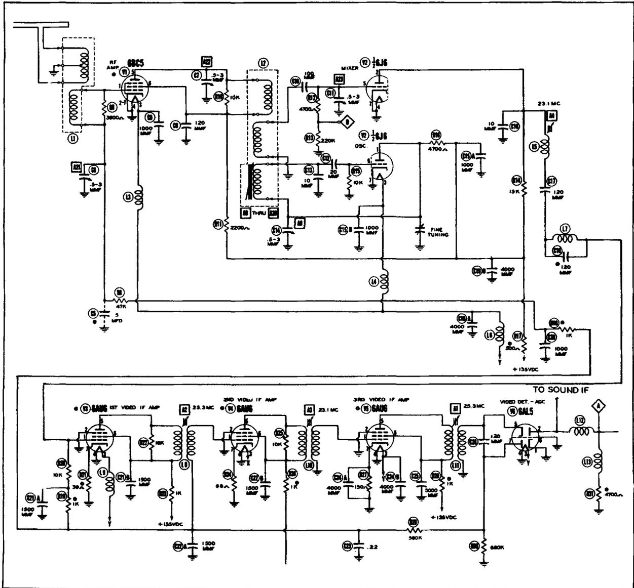
Figure 38. The RF and IF Stages of an Intercarrier Receiver.
