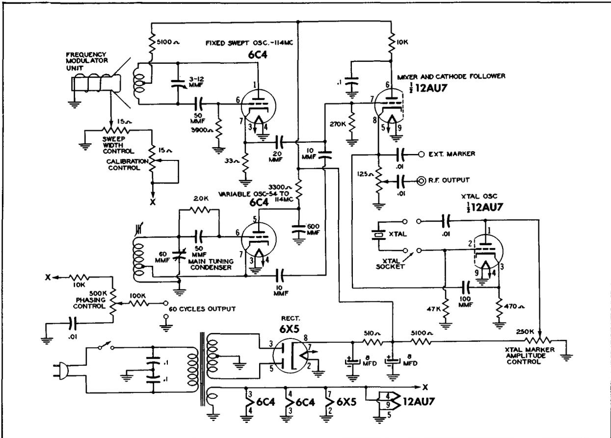
Figure 21. A Schematic Diagram of the Eico Sweep Generator.
