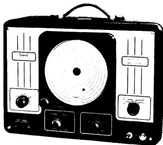
Figure 8A. A Signal Generator Which Will Generate Frequencies up to 120 mc. The Range Selector Markings Extend Only to 40 mc, but by Means of Harmonics, 120 mc can be Obtained. Courtesy of Triplet Electrical Instrument Co.
