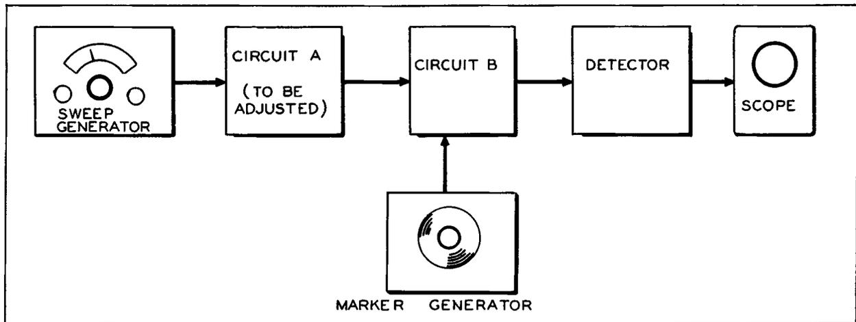
Figure 7. The Marker Signal Need Not Necessarily Pass Through the Circuit Being Aligned in Order to Serve its Purpose.
