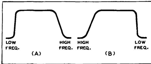
Figure 21. (A) Video IF Response Curve with the Low Frequencies at the Left and the High Frequencies at the Right. (B) Same Curve in Reversed Position.
