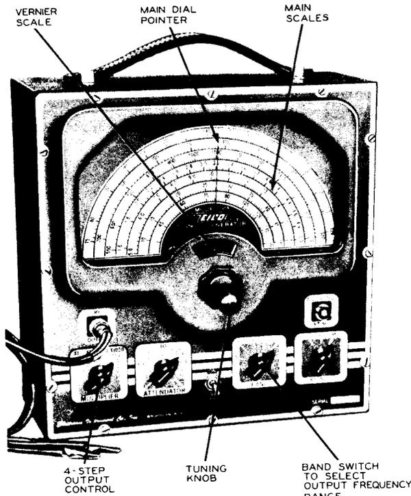
Figure 2. An AM Generator Available in Kit Form. Courtesy of Eico.
