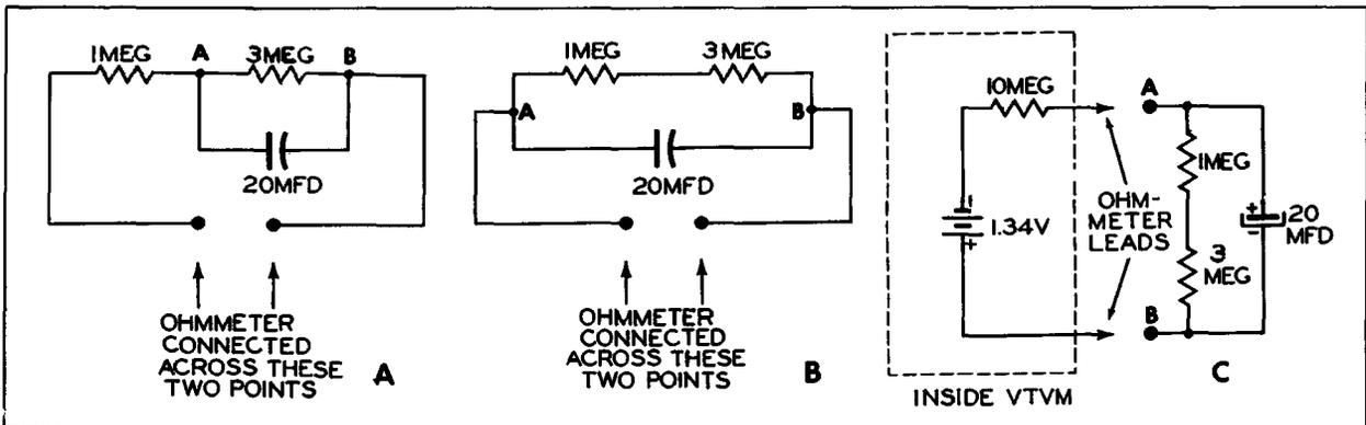
Figures 18 A, B and C. Circuits to Illustrate Why Meter Needle Will Rise Slowly on Some Resistance Measurements.
