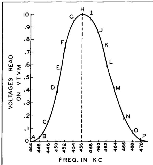
Figure 6. The Response Curve of LC in Figure 5 Obtained Point by Point. (For the Sake of Simplicity, it is Being Assumed That the Amplification of the Pentode Stage in Figure 5 is 1.)
