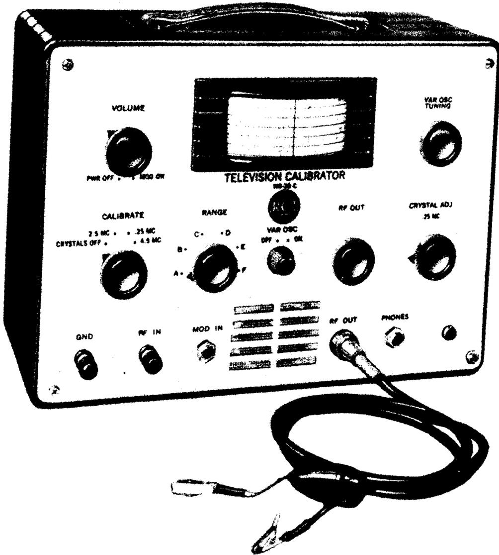
Figure 4. A Versatile Marker Generator. Included Is a Crystal-Calibrated Variable Frequency Oscillator, Two Crystal-Controlled Oscillators, a Modulator Stage for Internally Modulating the Output at Audio and RF Frequencies, and an Audio Amplifier with Internal Speaker. (Model WR-39C, Courtesy RCA.)
