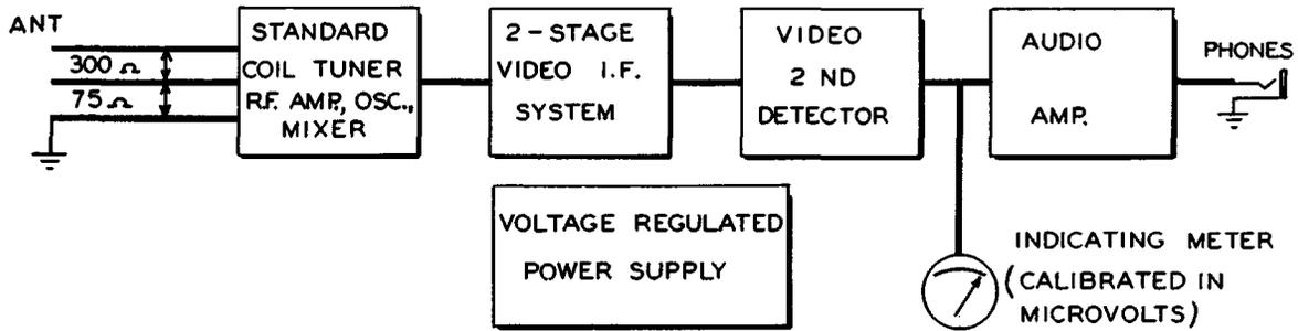
**Figure 32. Block Diagram of the Simpson Field Strength Meter.**
