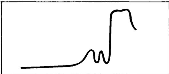
Figure 31. Improper Centering of Sweep Range (Too Low).
