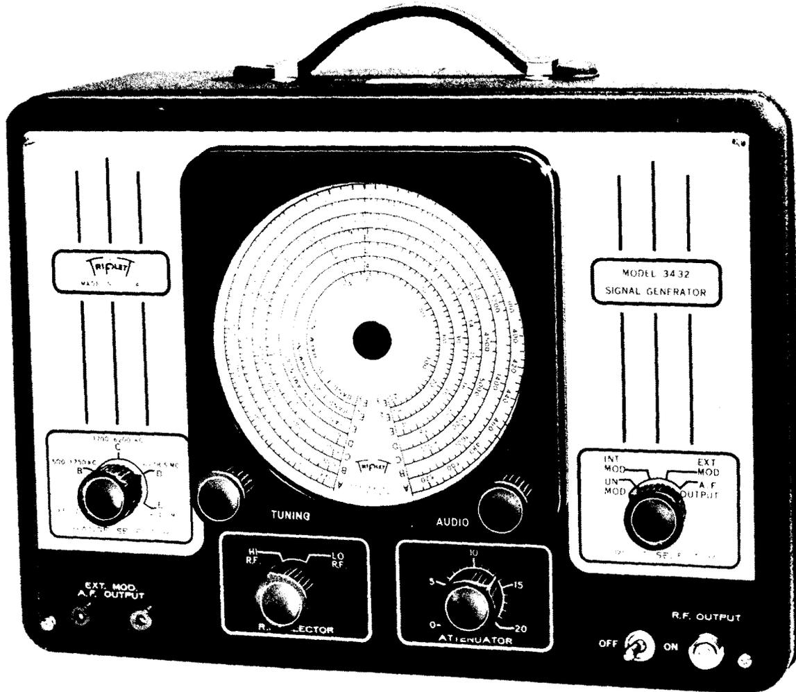
Figure 8A. A Signal Generator Which Will Generate Frequencies up to 120 mc. The Range Selector Markings Extend only to 40 mc. But by Means of Harmonics 120 mc Can Be Obtained. (Model 3432, Courtesy of Triplet Electrical Instrument Co.)
