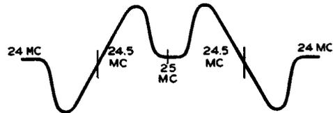
Figure 12. When a 60 Cycle Saw-Tooth Deflection Voltage is Used in the Oscilloscope, The Screen Presentation Will Appear as Shown.
