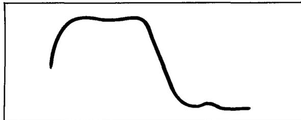
Figure 32. Improper Centering of Sweep Range (Too High).
