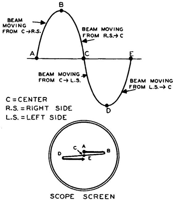
Figure 15. The Motion of the Electron Beam in the Oscilloscope When it is Being Driven by a Sine Voltage.
