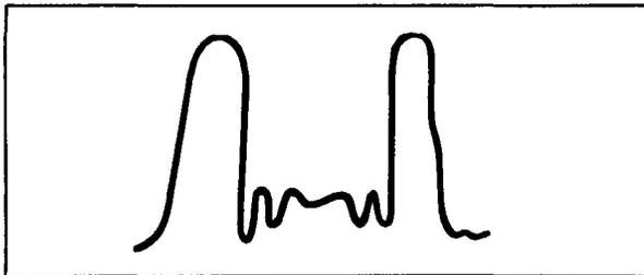
Figure 33. Curve with Incorrect Scope Deflection.
