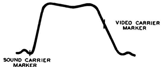
Figure 47. Overall RF and IF Response Curve of a Television Receiver Such as the One Shown in Figure 24.
