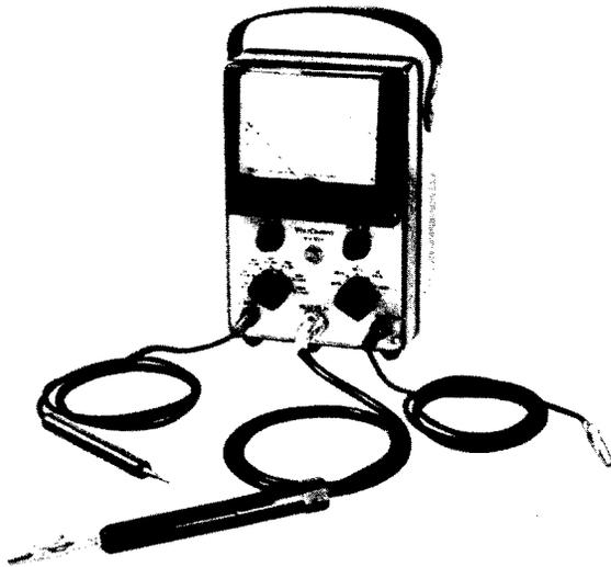
Figure 10A. A VTVM in Which AC and DC Voltages are Fed to the Same Terminal. Courtesy of RCA.
