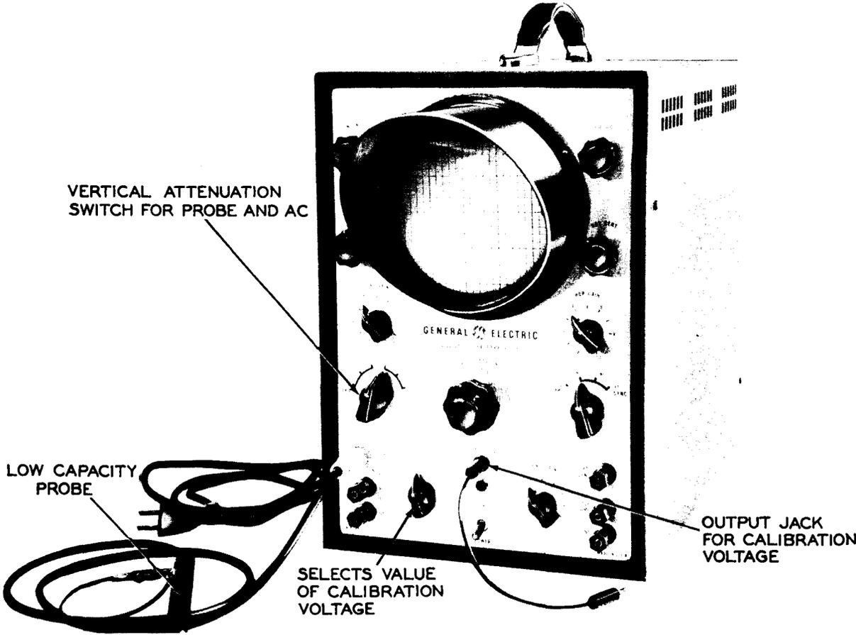
Figure 26. Oscilloscope Containing a Built-In Low Capacity Probe. Provision Is Also Available for Measuring Peak-to-Peak Value of any Waves Depicted on the Screen. (Model ST-2C, Courtesy General Electric Company.)
