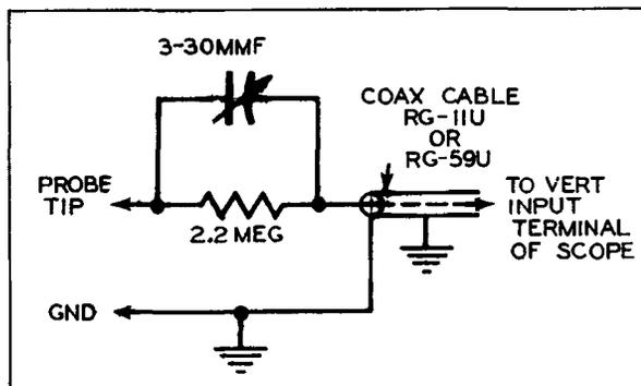
Figure 23A. Low-Capacity Probe Circuit.
