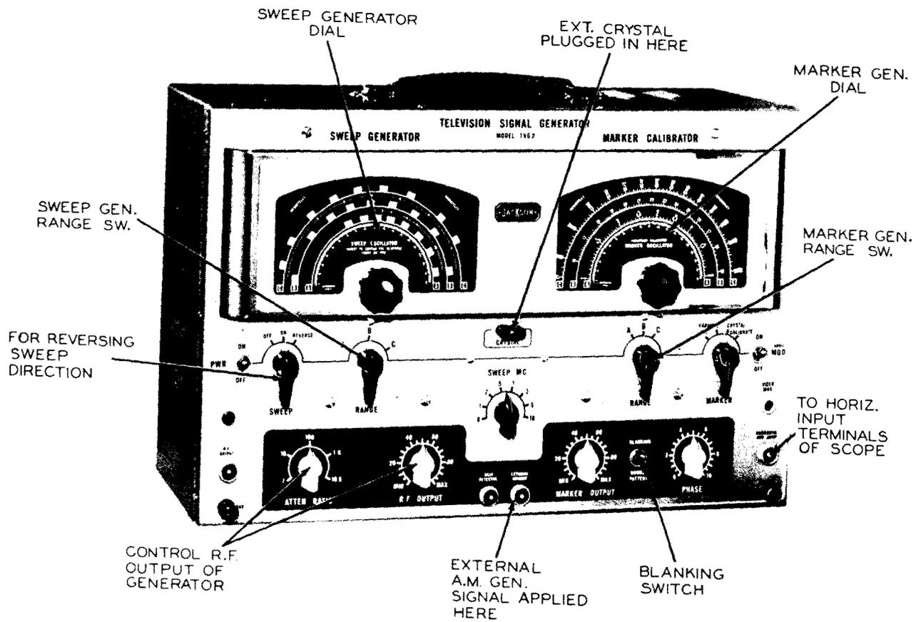
Figure 26. A Sweep and Marker Generator with Blanking and Reverse Sweep Features. (Model TVG2, Courtesy of Jackson Electrical Instrument Co.)
