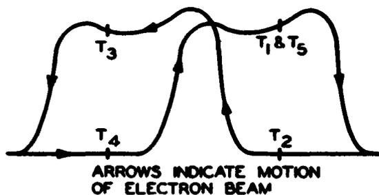
Figure 18. The Arrows Indicate the Path of the Electron Beam. T1 Through T5 are Keyed to Figure 17.
