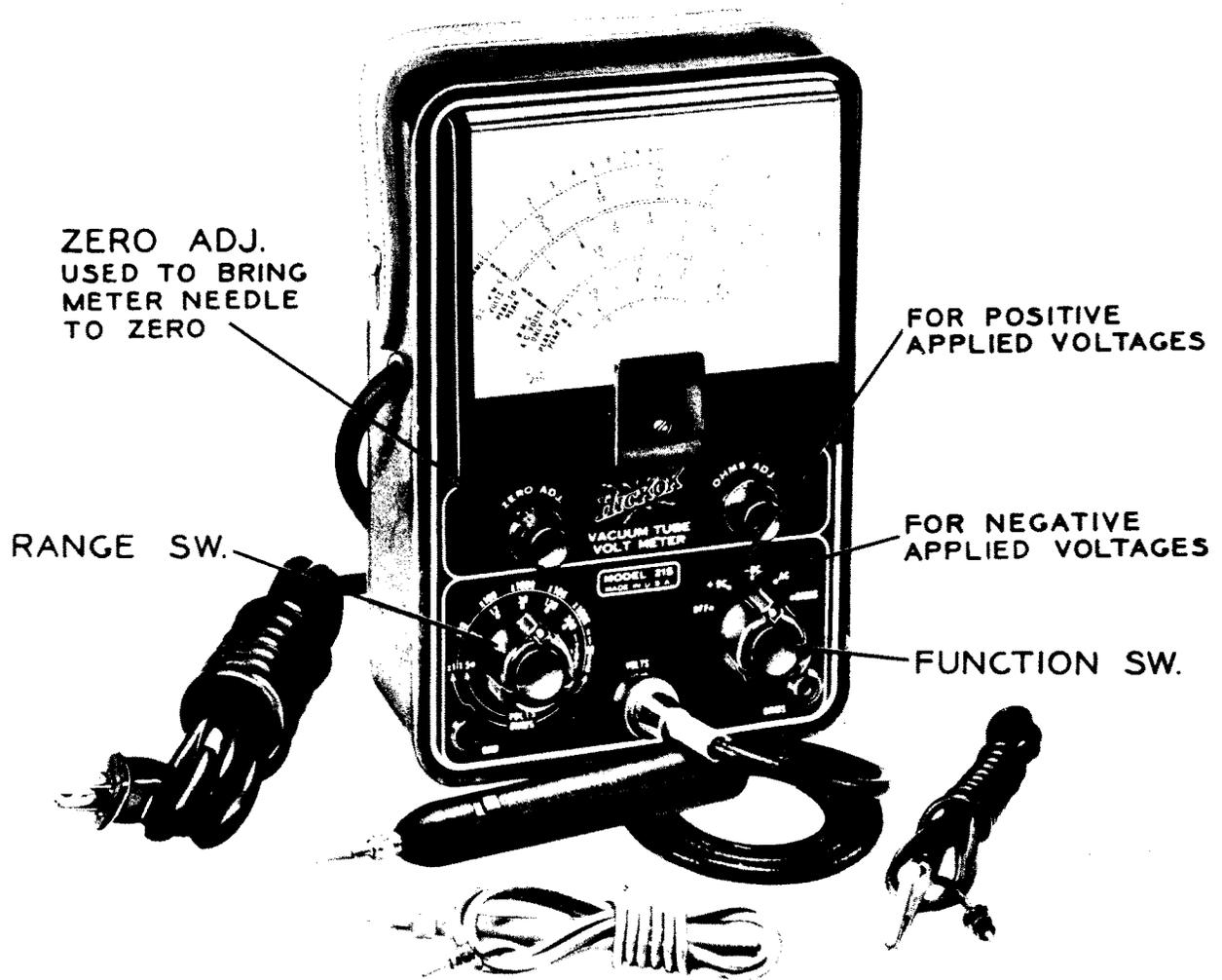
Figure 2. The Front Panel Controls on a Typical VTVM. (Model 215, Courtesy of Hickok Electrical Instrument Co.)
