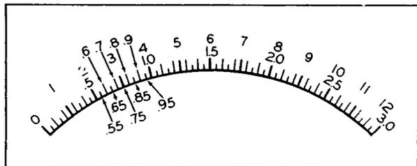
Figure 30. The Value of the Sub-divisions on the 0-3 Scale.
