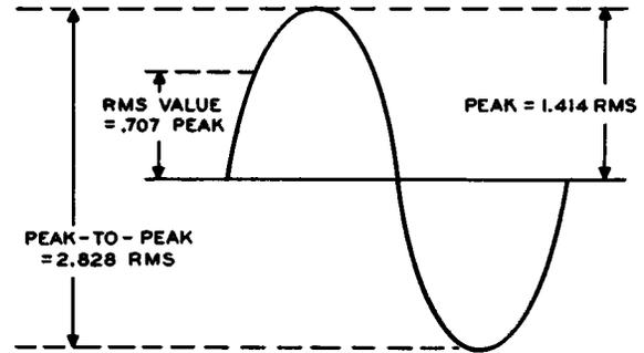
Figure 30. Relationship Between RMS, Peak, and Peak-To-Peak Values of a Sine Wave.
