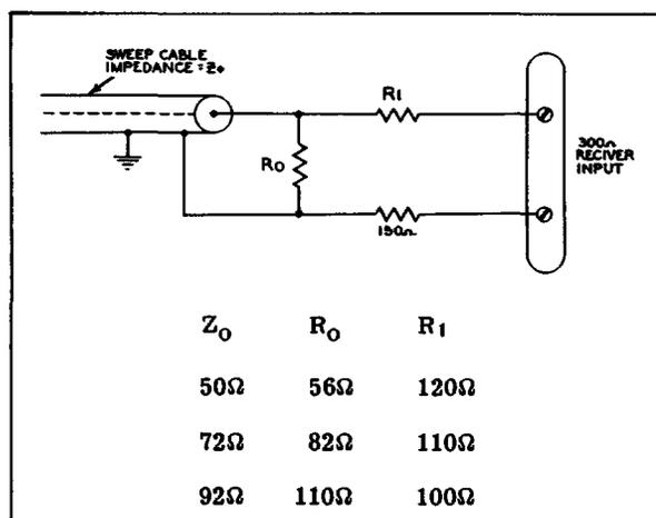
Figure 44. Resistive Network to Match Sweep Cable Impedance to Receiver Input.
