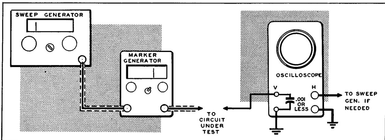
Figure 2. Connecting Sweep Generator to Marker Generator.
