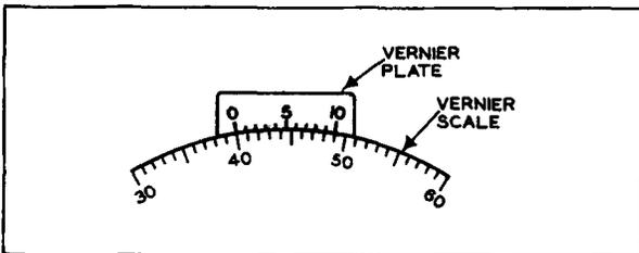
Figure 10. The Reading on the Vernier Scale in its Present Position is 40. This Is True Because the Zero on the Vernier Plate Is Directly Over the 40 on the Vernier Scale.
