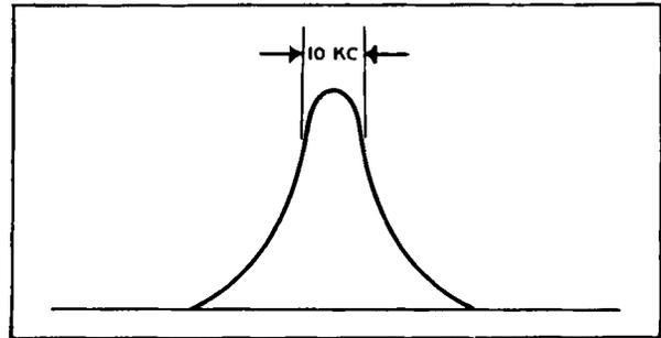
Figure 2. A Typical Response Curve of AM Radio Receiver.
