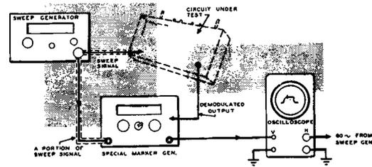
Figure 8. Marker Pip Amplitudes Can be Kept Constant Across the Entire Response Curve by not Passing Marker Signal Through the Test Circuit. See Text.
