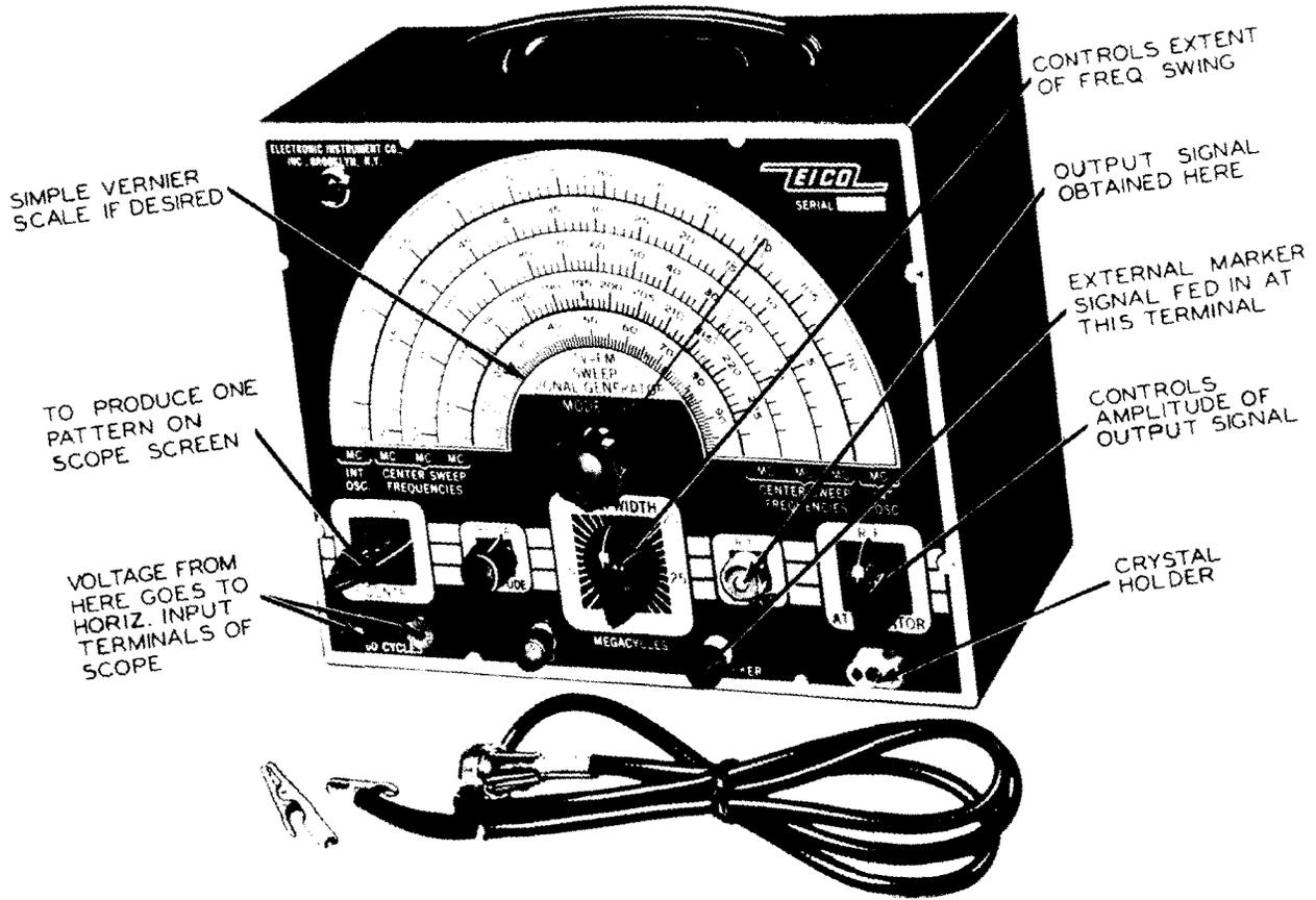
Figure 19. A Commercial Sweep Generator Which Is Available in Kit Form. (Model 360, Courtesy of Eico.)
