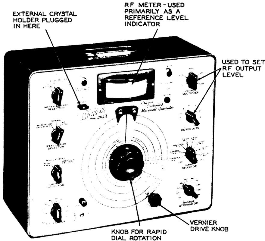
Figure 13. A Crystal-Controlled AM Generator. (Model 292X, Courtesy of Hickok Electrical Instrument Co.)
