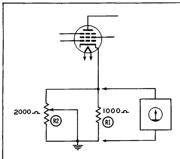
Figure 17. The Measured Value of R1 (Without Removing From Circuit) Is Dependent Upon a Center Arm Setting of R2.
