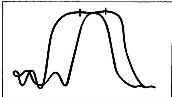
Figure 28. Sweep Generator Phasing Control not Properly Adjusted.
