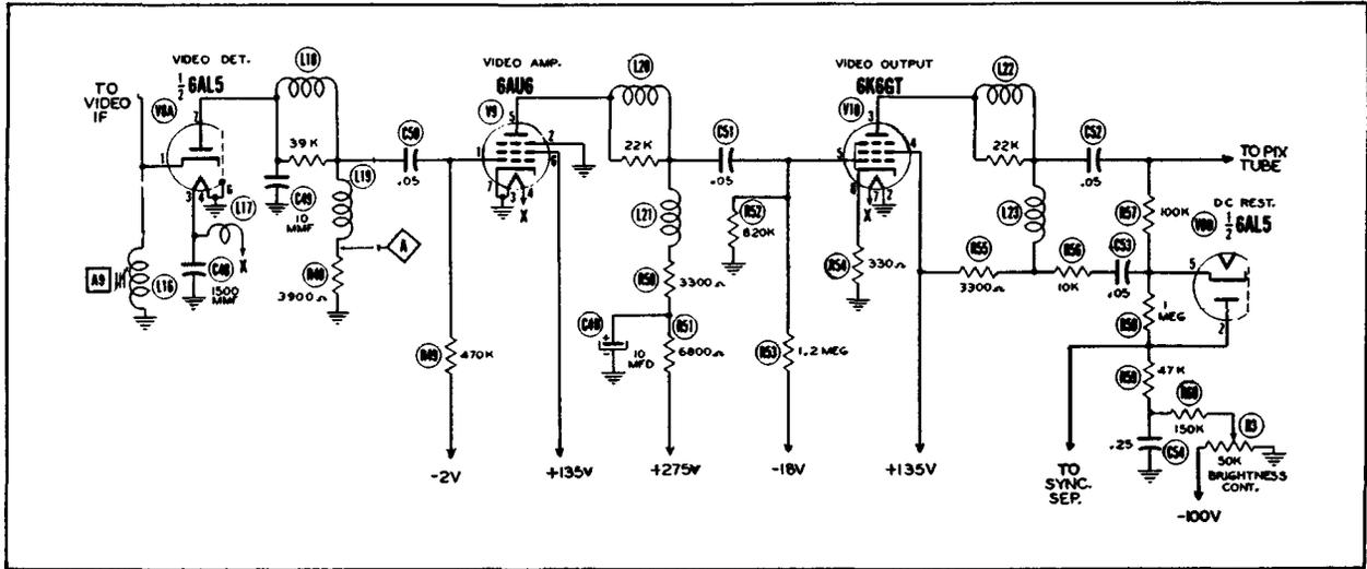
Figure 49. A Two-Stage Video Amplifier System.
