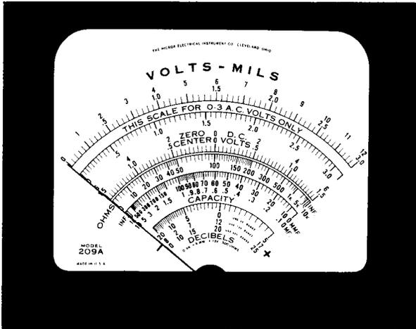
Figure 28. The Scale Used on the Hickok Model 209A VTVM. Courtesy of Hickok Electrical Instrument Co.
