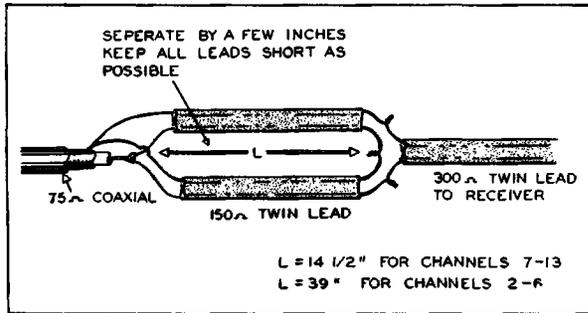
Figure 45. How to Match an Unbalanced 75 Ohm Coaxial Cable to a Balanced 300 Ohm Impedance. Courtesy of Sylvania Electric.
