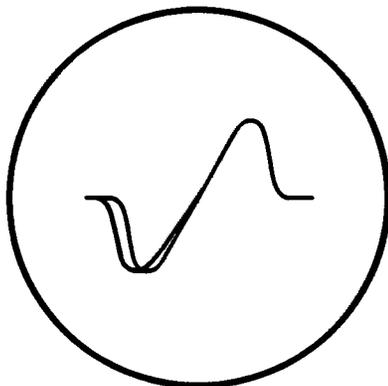
Figure 13. Sweep Generator Unbalance May Prevent Perfect Blending at all Points.
