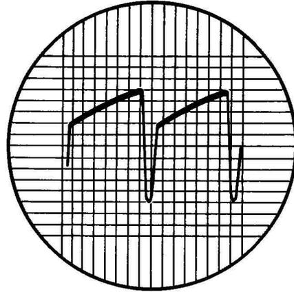
Figure 27. The Wave Shown Above Covers a Height of Ten Squares on the Ruled Mask.
