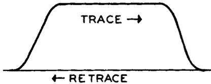
Figure 27. The Appearance of a Response Curve and its Zero Reference Retrace Line When Blanking is Employed in Sweep Generator.
