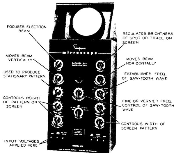
Figure 2. The Front Panel Controls of an Oscilloscope. Courtesy Simpson Electric Company.
