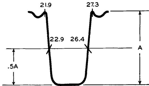
Figure 34. Overall Video IF Response Curve Recommended by a Large Manufacturer for his Sets.
