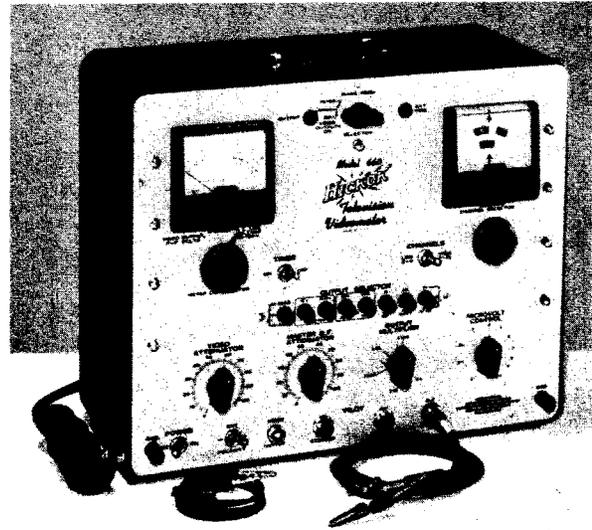
Figure 24. An Elaborate Servicing Instrument Designed to Enable the Serviceman to Carry out a Series of Tests on a Television Receiver. Some of its Features are Discussed in the Text. Courtesy Hickok Electrical Instrument Company.
