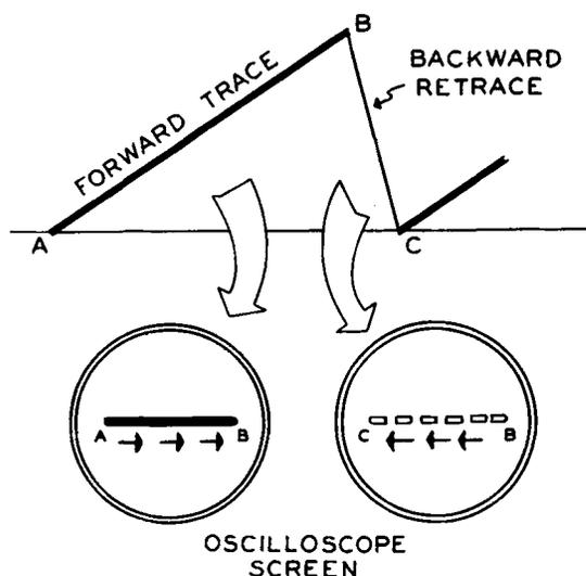
Figure 13. The Manner in Which the Beam on an Oscilloscope Screen Traces and Retraces.
