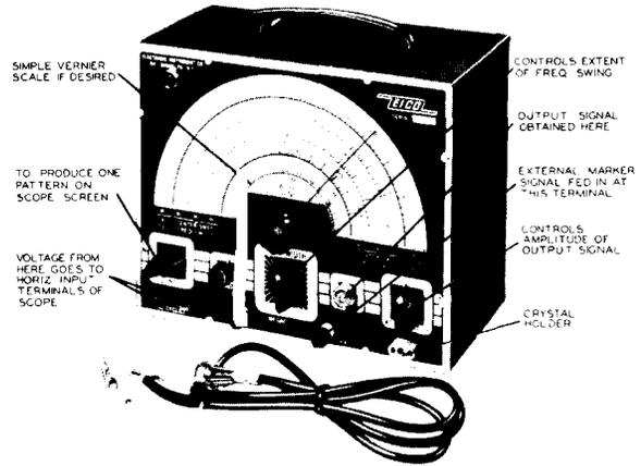
Figure 19. A Commercial Sweep Generator Which is Available in Kit Form. Courtesy of Eico.
