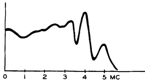
Figure 52. The Video Amplifier Response Patterns of Several Commercial Receivers.
