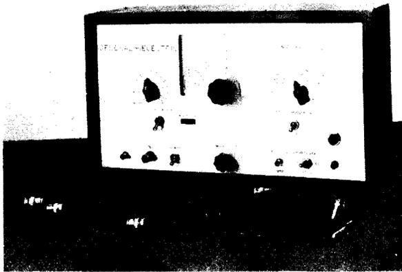
Figure 9A. A Special Marker Generator Designed to Develop Marker Pips Independently of the Test Circuit. Courtesy of General Electric Company.
