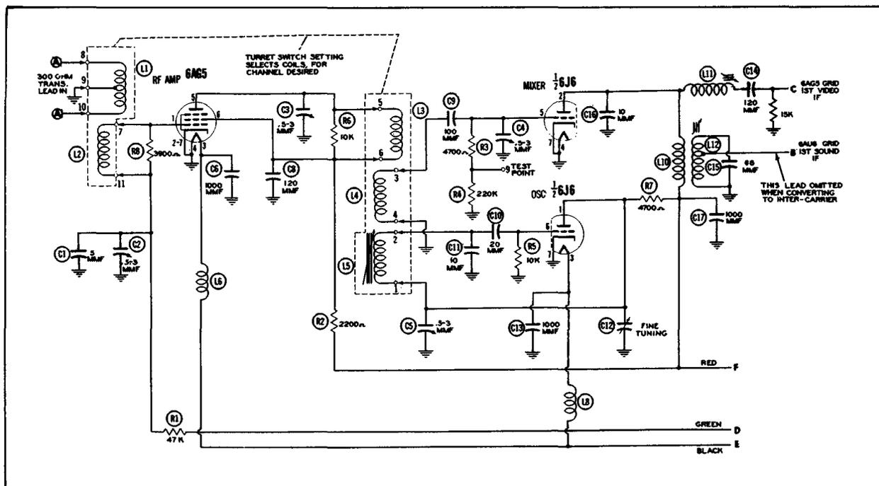
Figure 43. Circuit Diagram of the Standard Coil Tuner.
