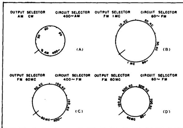
Figure 39. Modulation Dial Detail of Sylvania AM-FM Generator.
