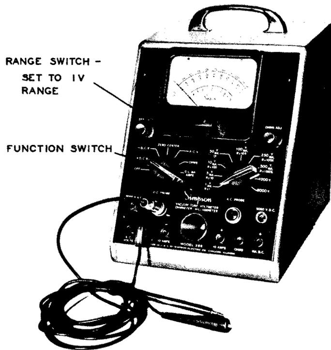
Figure 4. The Simpson Model 266 VTVM Set up to Measure Positive DC Voltages of 1 Volt or Less. Pay Particular Attention to the Range and Function Switches. (Courtesy of Simpson Electric Co.)
