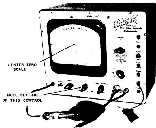
Figure 6. A VTVM With a Special Zero Center Scale. Courtesy of Hickok Electrical Instrument Co.
