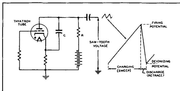
Figure 8. Thyratron Tube Method of Developing Saw-Tooth Waves.
