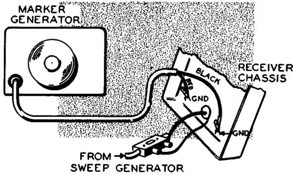
Figure 9. The "Chassis" Method of Injecting a Marker Signal. Courtesy Precision Apparatus Co., Inc.
