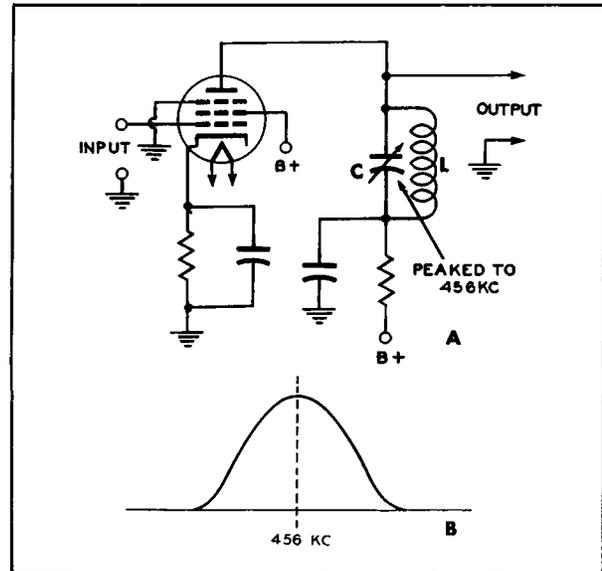
Figure 4. (A) A Simple Tuned Circuit LC, and (B) Its Response Curve.
