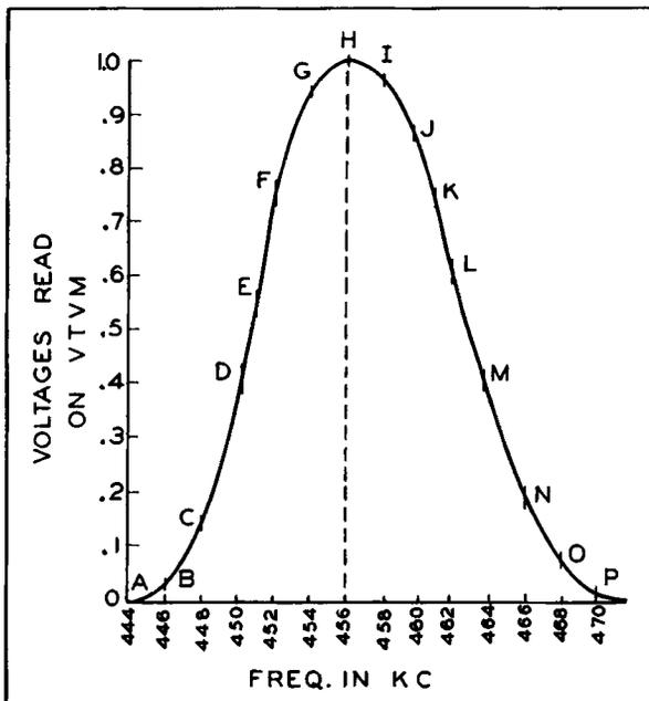
Figure 6. The Response Curve of LC in Figure 5 Obtained Point by Point. (For the Sake of Simplicity, it is Being Assumed That the Amplification of the Pentode Stage in Figure 5 is 1.)
