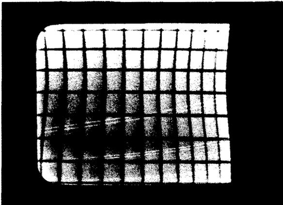
Figure 23. A Cross-Hatch Pattern is a very Sensitive Indicator of Hum in a Television Receiver.
