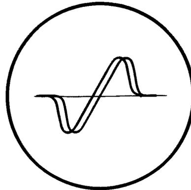
Figure 3. When You First Obtain a Response Pattern on the Screen, You Will Most Probably Have a Dual Trace.
