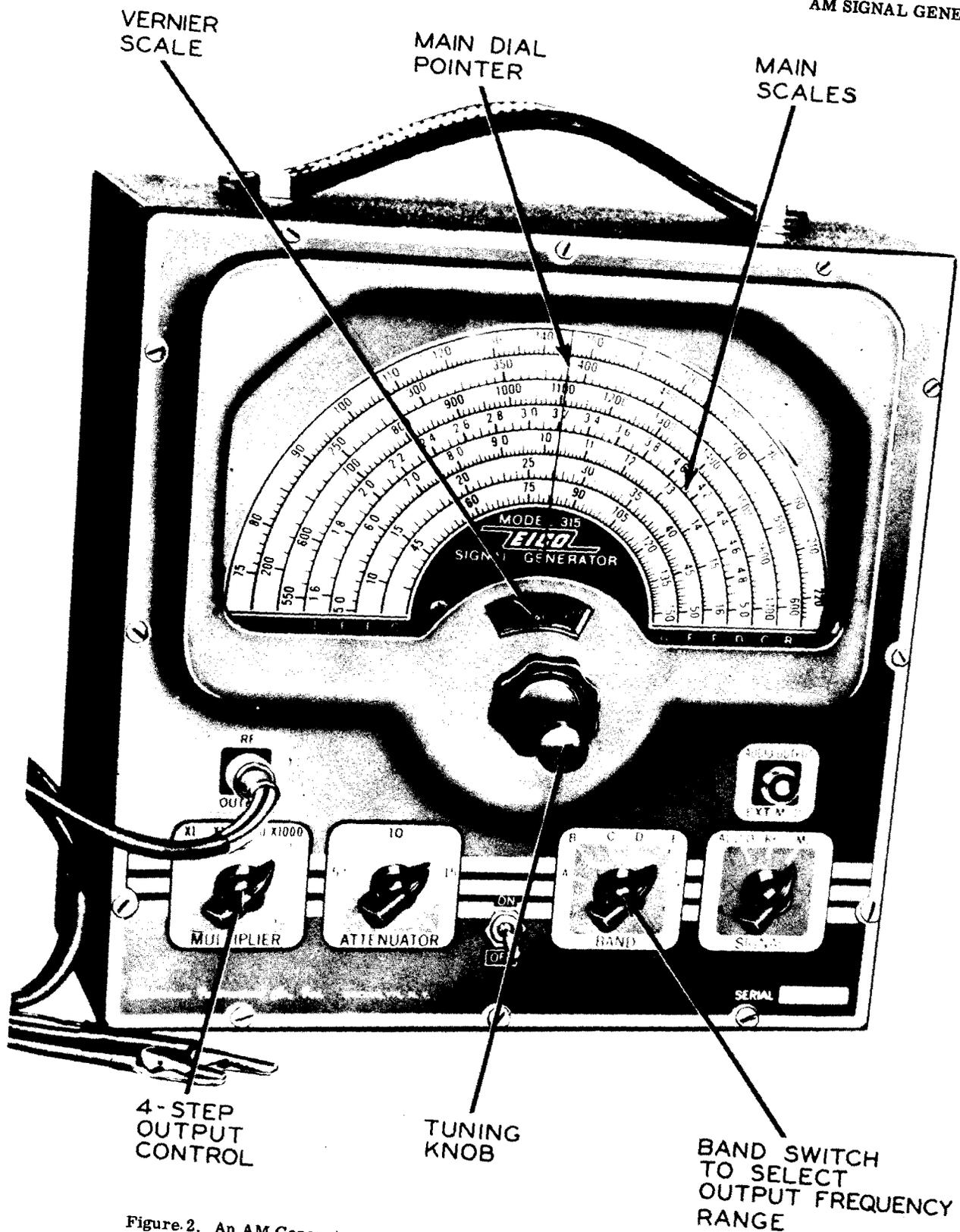
Figure 2. An AM Generator Available in Kit Form. (Model 315, Courtesy of Eico.)
