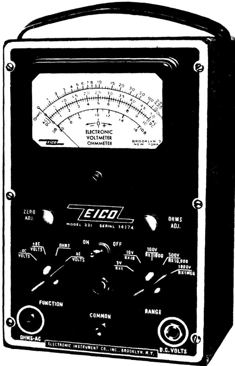
Figure 10B. An Eico VTVM Instrument Is Set up to Measure AC Volts. Note Function Switch Is Set to AC Volts Position; Setting of Range Switch Is Dependent on Voltage to Be Measured. (Model 221, Courtesy of Eico.)
