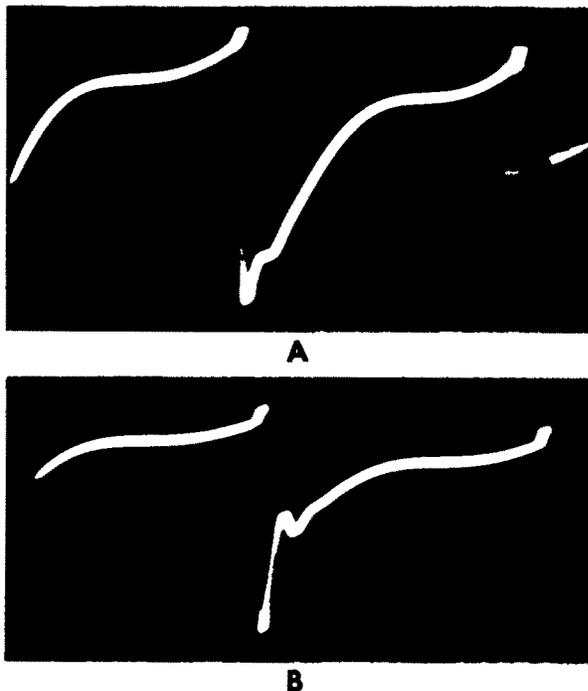
Figure 24. Wave Shown at (A) Was Obtained Without use of Low-Capacity Probe; Wave at (B) Did have Probe. Note the Difference Between the Two.
