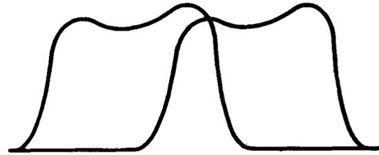
Figure 16. A Double Pattern On Figure 10 Due to Improper Phase Control Setting.
