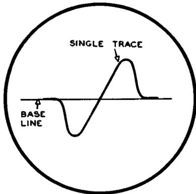
Figure 10. With a Blanking Control in the Sweep Generator, One of the Two Traces can be Converted into a Base or Reference Line.
