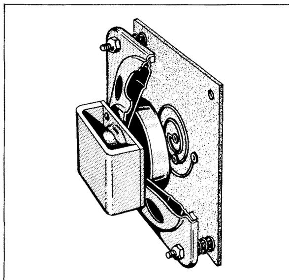
Figure 7. The Speaker-mounted Movable Membrane and Flat Oscillator Coil by Means of Which Frequency Sweeping Is Achieved.
