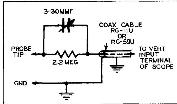
Figure 23A. Low-Capacity Probe Circuit.
