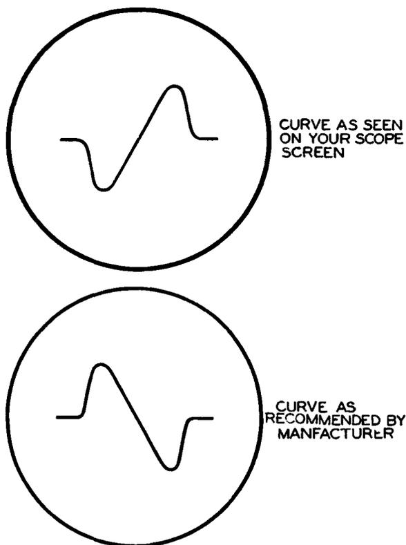
Figure 15. Two Curves 180° Out of Phase With Each Other. This is Generally Caused by Number of Vertical System Amplifiers in Oscilloscope.
