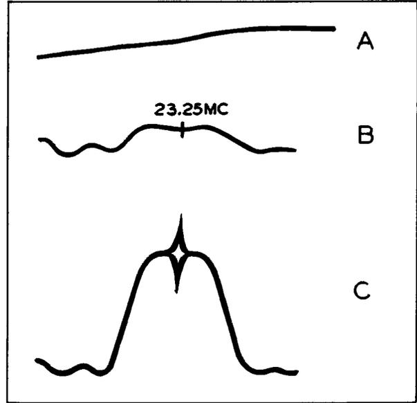
Figure 27. (A) Marker Generator Connected Directly to Grid of the First Video IF Amplifier. Strong Signal Output. (B) Marker Generator Connected Same as "A" but With Weak Signal Output. (C) Marker Generator Coupled to Grid of First Video IF Amplifier Through 75,000 Ohm Isolating Resistor. Strong Signal Output.
