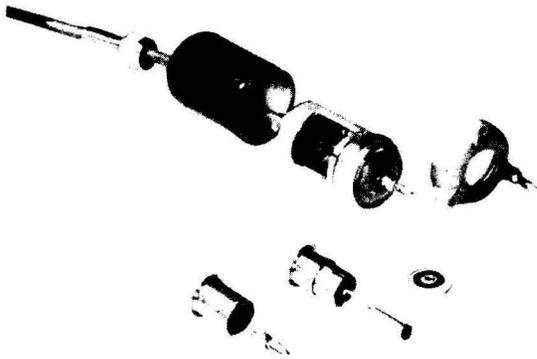
Figure 14A. Exploded View of Diode High-frequency Probe. Courtesy of General Radio.
