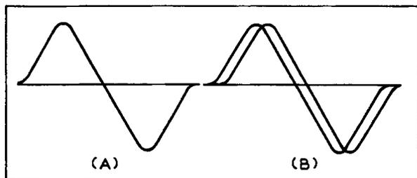
Figure 18. FM Detector Response Obtained on an Oscilloscope with Blanking Control in Sweep Generator. (B) Usual Dual Pattern with no Blanking.
