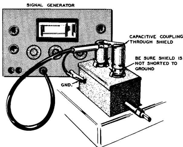
Figure 8. Signal Injection by Clipping "Hot" Lead From Generator Onto Tube Shield. Make Certain Tube is not Touching Chassis or Other Ground Points.
