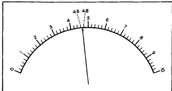
Figure 25. The Pointer Being Between 4.6 and 4.8 Would be Read as Indicating a Value of 4.7.
