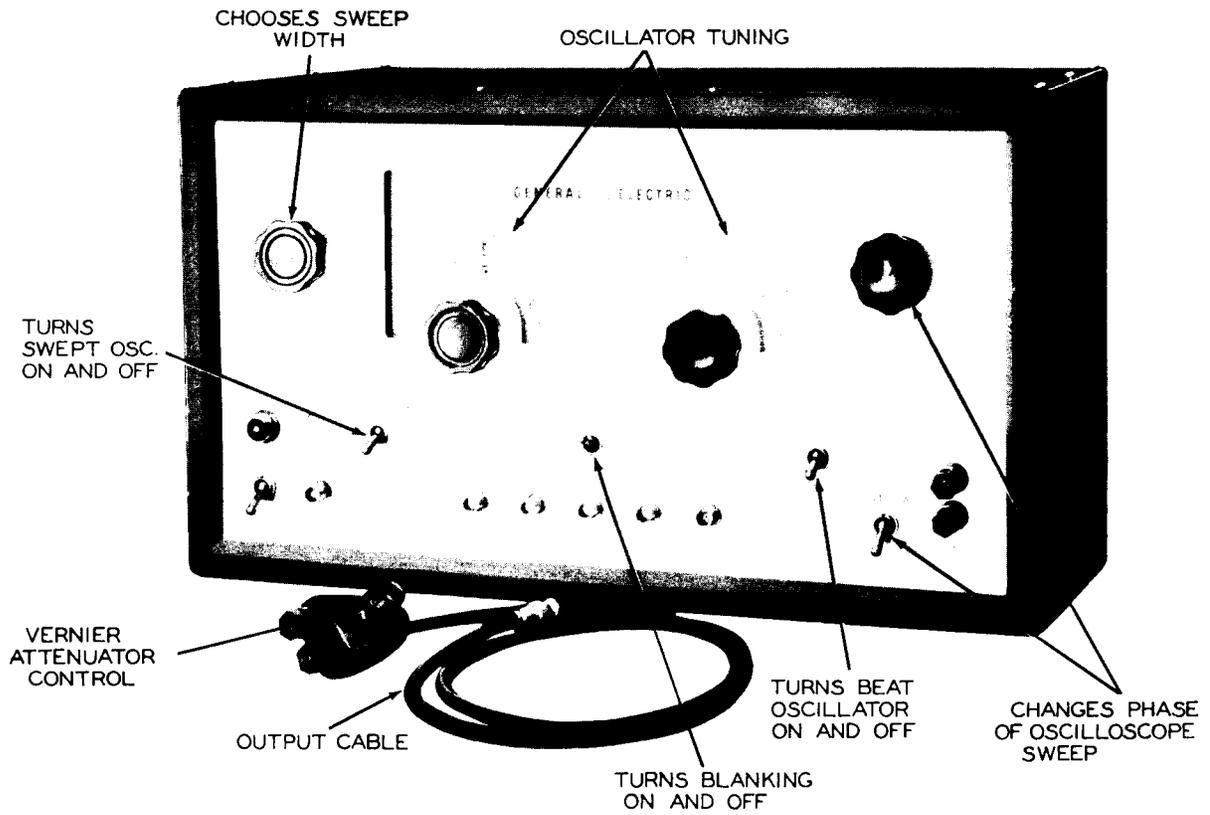
Figure 34. A Variable Permeability Sweep Generator. (Model ST-4A, Courtesy of General Electric Co.)
