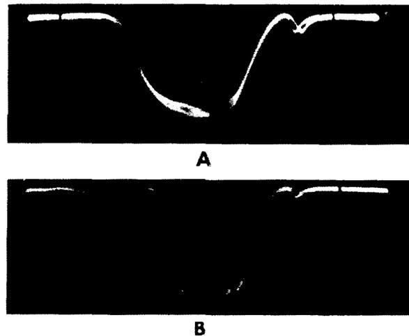
Figure 25. A Comparison Between the Appearance of a Conventional Pip Produced by the Beat Method (A), and a Pip (or Dip, Actually) Produced by the Absorption Method (B).
