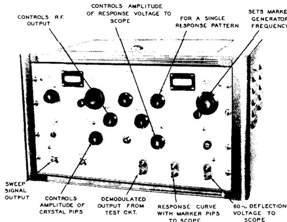
Figure 13. A UHF Sweep-Marker Generator. Courtesy RCA.
