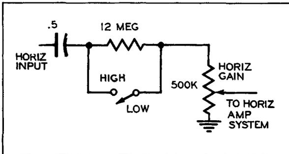
Figure 9. The Horizontal Input Circuit of the Instrument Shown in Figure 2.
