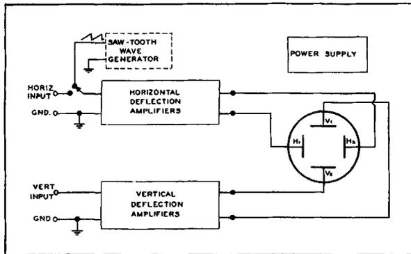
Figure 7. A Simplified Block Diagram of an Oscilloscope.
