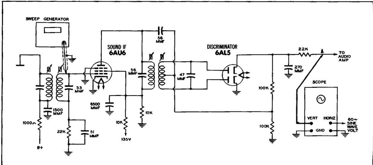
Figure 1. The Manner In Which the Response Pattern of a Foster-Seeley Discriminator Would be Obtained.
