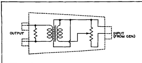
Figure 37B. Schematic Diagram of the Output Adaptor.
