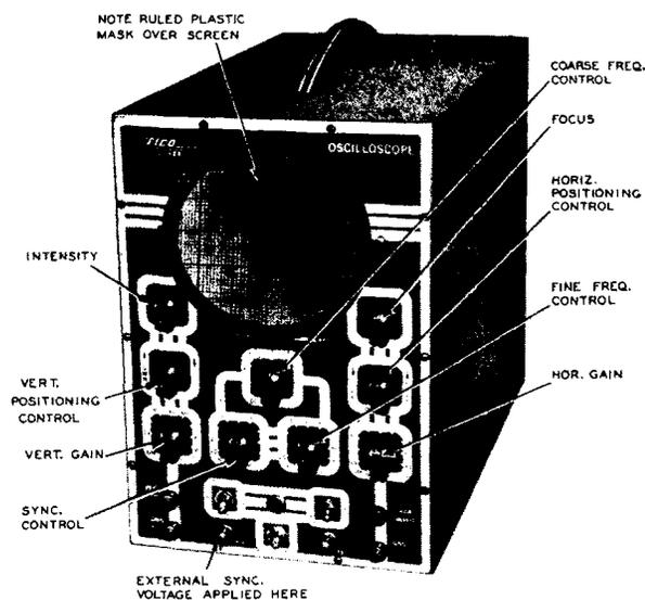
Figure 12. An Oscilloscope which is Available in Kit Form. Courtesy Eico.
