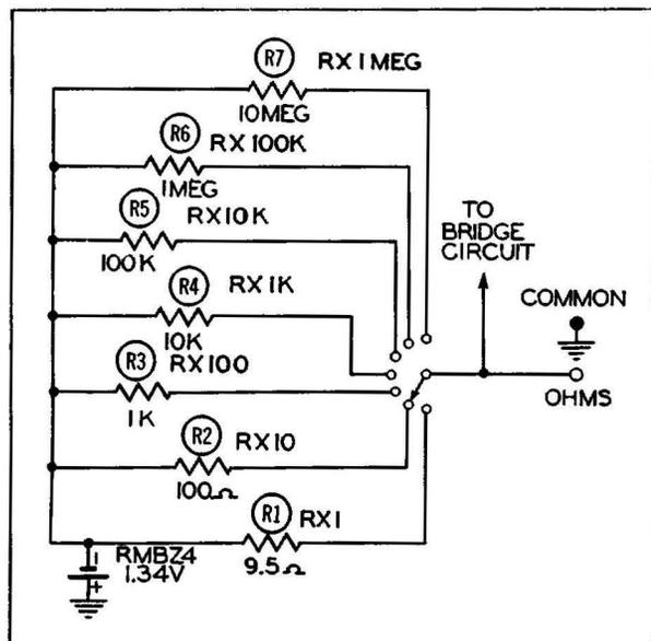
Figure 15. The Ohmmeter Section of a VTVM.
