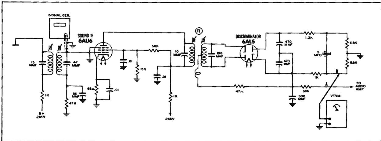
Figure 17. How to Connect a VTVM and Signal Generator for Ratio Detector Alignment.
