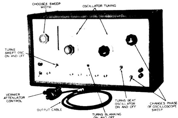
Figure 34. A Variable Permeability Sweep Generator. Courtesy of General Electric.
