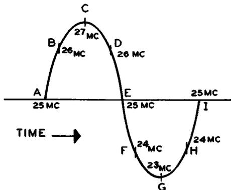
Figure 9. The Sinusoidal Change in Output Frequency of a Sweep Generator in Which the Modulator Is Driven by a 60-cycle Voltage. (Whether the Output Frequencies Increase on the Positive 1/2 Cycle, as Shown, Depends on the AC Connections to the Voice Coil of the Speaker-driving Unit.)
