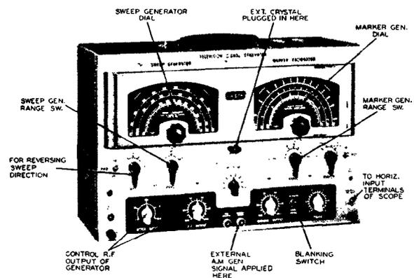
Figure 26. A Sweep and Marker Generator With Blanking and Reverse Sweep Features. Courtesy of Jackson Electrical Instrument Company.
