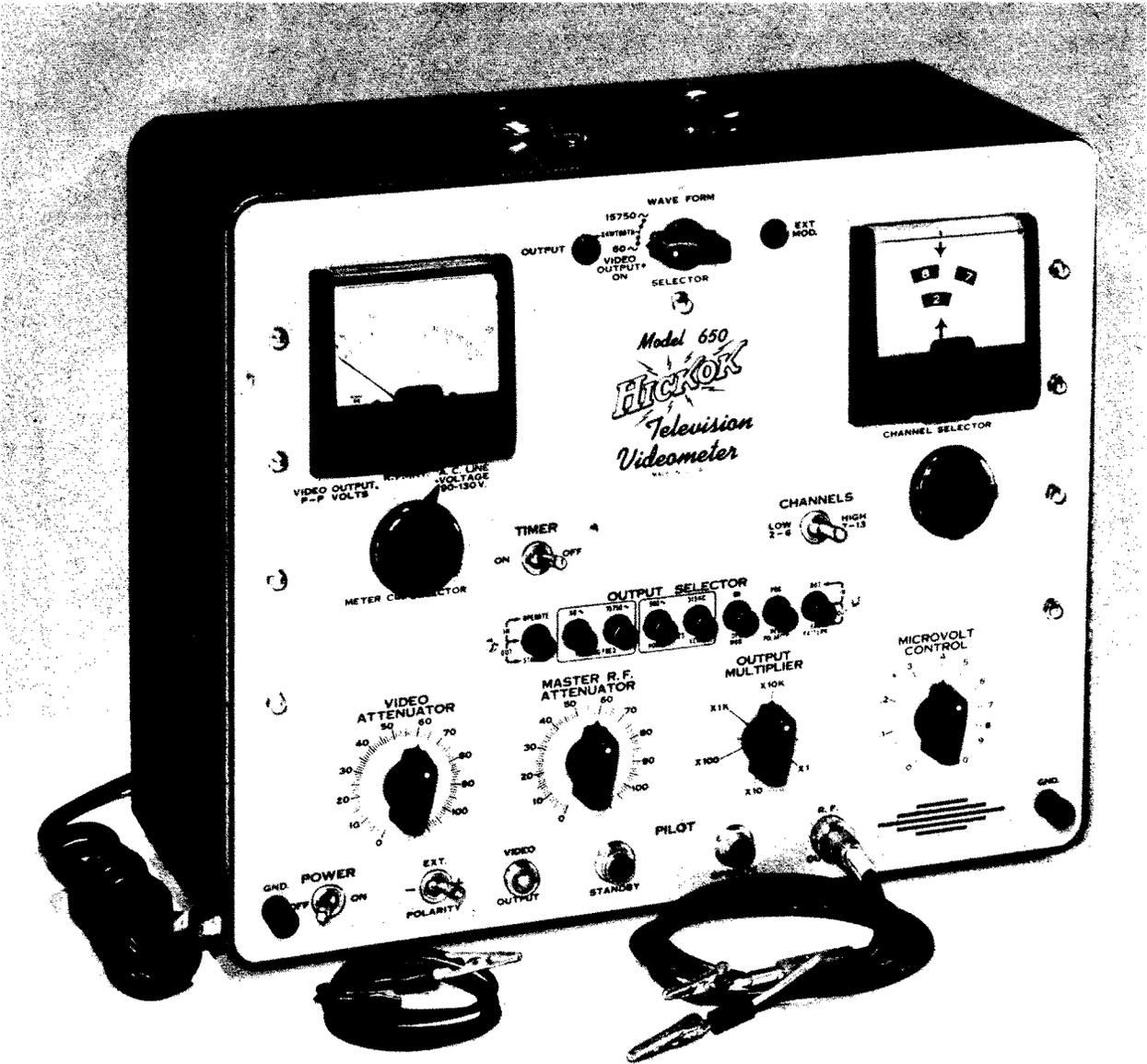
Figure 24. An Elaborate Servicing Instrument Designed to Enable the Serviceman to Carry out a Series of Tests on a Television Receiver. Some of its Features Are Discussed in the Text. (Model 650, Courtesy Hickok Electrical Instrument Co.)
