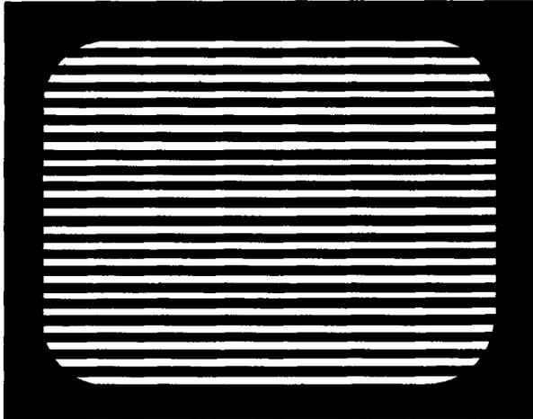
Figure 6. Horizontal Bars Designed to Check Vertical Linearity.
