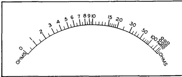
Figure 31. A Typical Ohms Scale.
