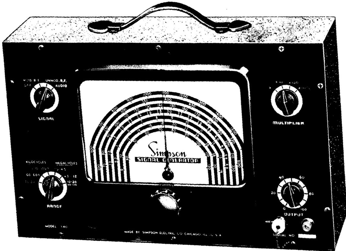
Figure 8B. A Simpson Model 340 Signal Generator. (Courtesy of Simpson Electrical Instrument Co.)
