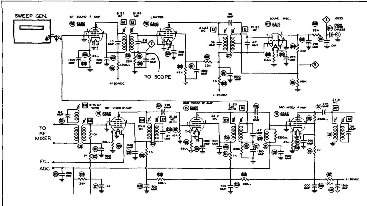
Figure 18. The Sound System in a Television Receiver Employing a Foster-Seeley Discriminator.
