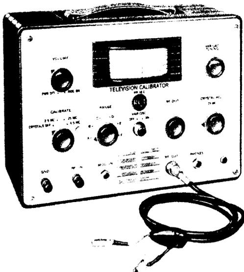
Figure 4. A Versatile Marker Generator. Included is a Crystal-Calibrated Variable Frequency Oscillator, Two Crystal-Controlled Oscillators, a Modulator Stage for Internally Modulating the Output at Audio and RF Frequencies, and an Audio Amplifier with Internal Speaker. Courtesy RCA.
