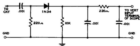
Figure 40. A Probe Detector Recommended by Du-Mont for Use in Their Video Circuits. There are Many Variations of This Circuit.
