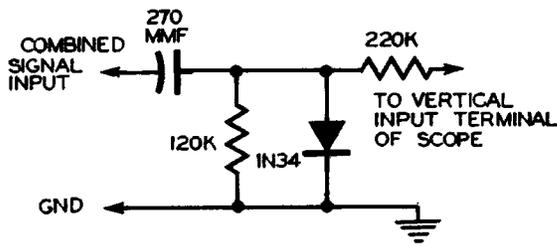
Figure 3. A Crystal Detector which can be Used for Zero Beating Two Signals, as Described in Text.
