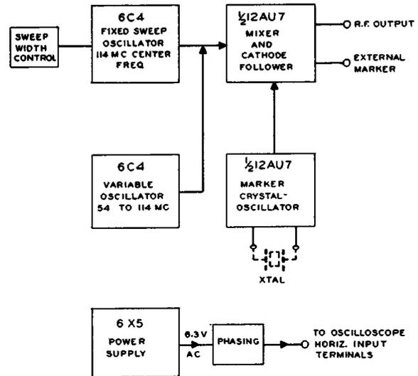
Figure 20. A Block Diagram of the Sweep Generator Shown in Figure 19.
