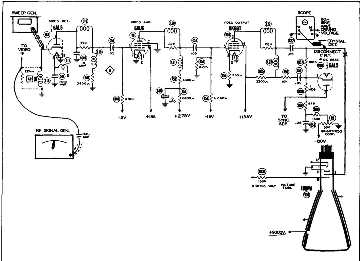
Figure 50. How the Equipment is Set Up to Obtain Video Amplifier Response Curve.
