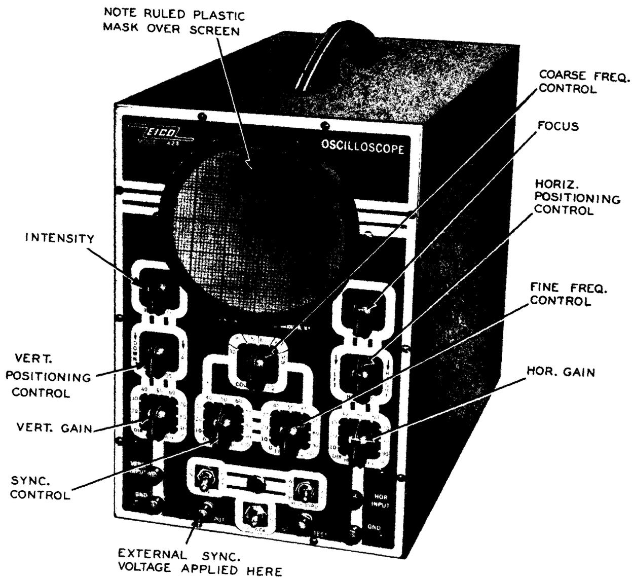
Figure 12. An Oscilloscope Which Is Available in Kit Form. (Model 425, Courtesy Eico.)
