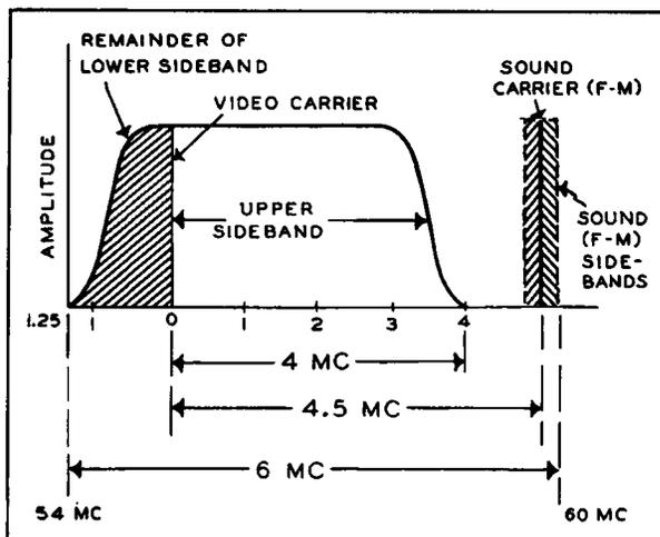
Figure 3. The Video and Sound Signals Broadcast by a Television Station. The 54-60 mc Range Is That Allotted to Channel 2.
