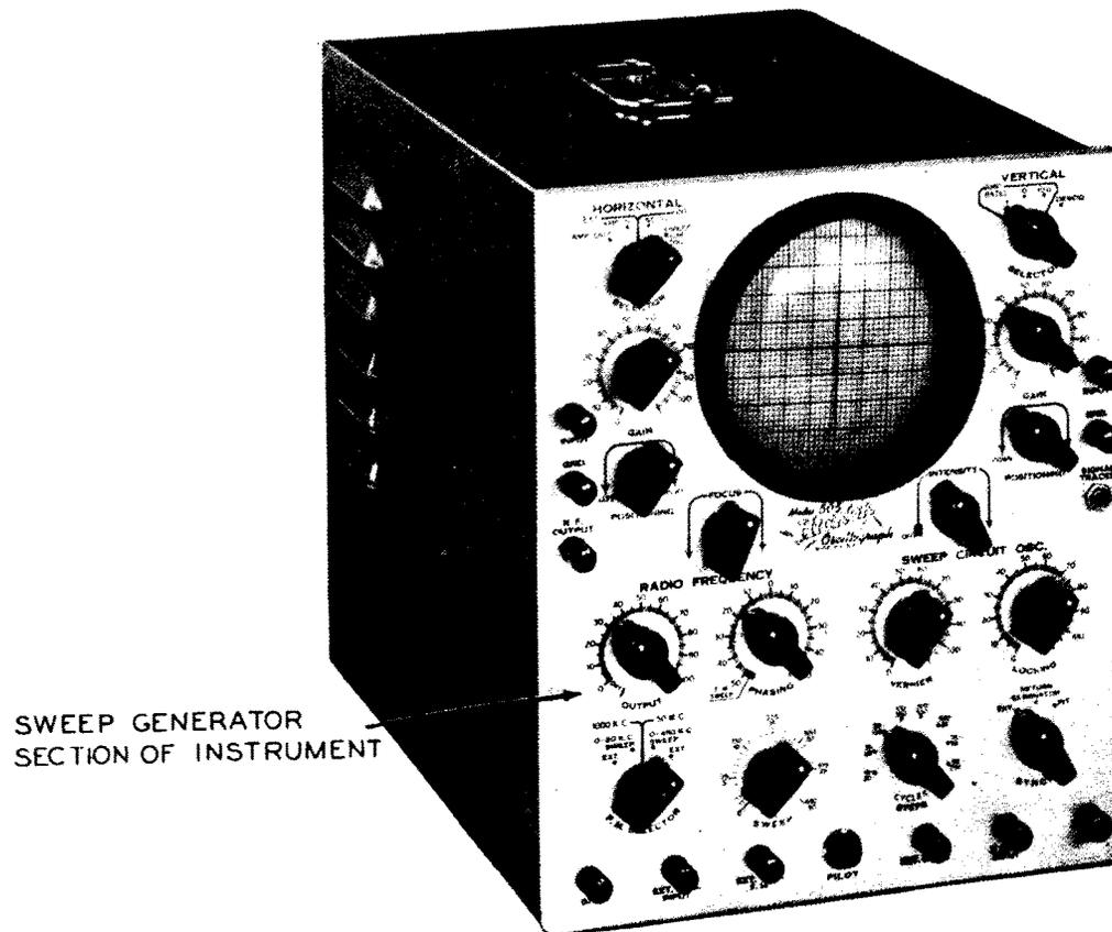
Figure 39. An Oscilloscope Containing a Modified Sweep Generator. (Model 505, Courtesy of Hickok Electrical Instrument Co.)
