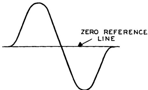
Figure 28. The "S" Response Curve of an FM Detector With Zero Reference Line Produced by Blanking Circuit in the Sweep Generator.
