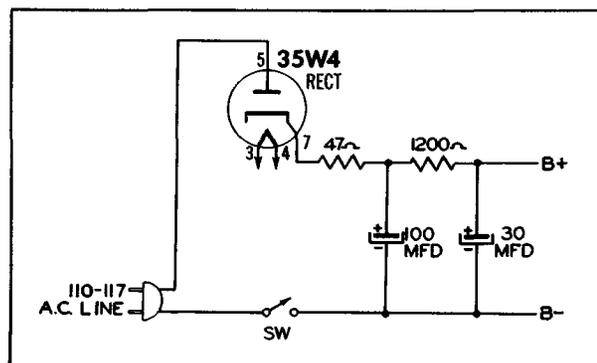
Figure 32. A Power Supply Circuit Common to Transformerless Receivers.
