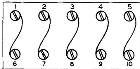
Figure 10. The Terminal Board Located Behind the Front Panel Cover Plate of the Oscilloscope Shown in Figure 2.
