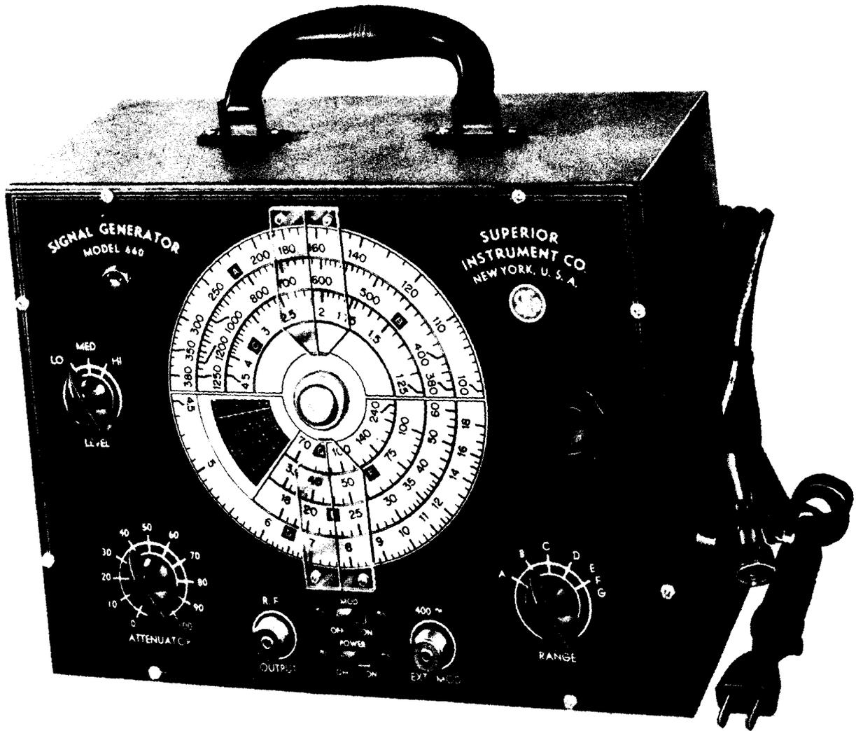
Figure 5. A Signal Generator with a Range from 100 kc to 240 mc. (Model 660, Courtesy of Superior Instrument Co.)
