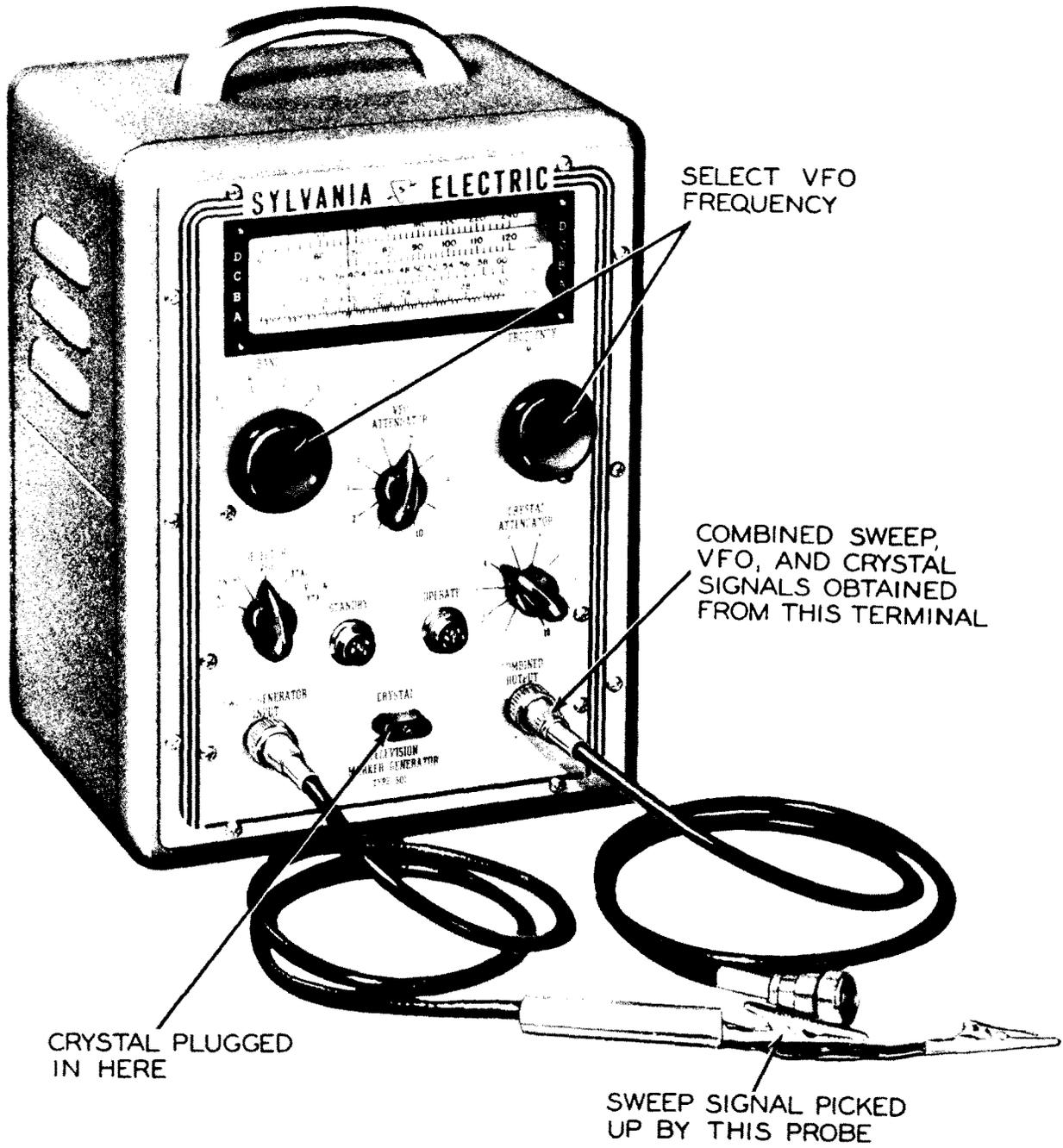
Figure 1. Sylvania Television Marker Generator. (Model 501, Courtesy of Sylvania Electric Products Inc.)
