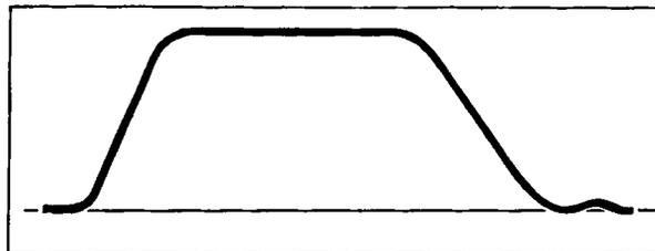
Figure 6. To Reproduce this Curve on a Scope Screen, then as the Beam Travels from Left to Right, it Must also be Made to Move Vertically.
