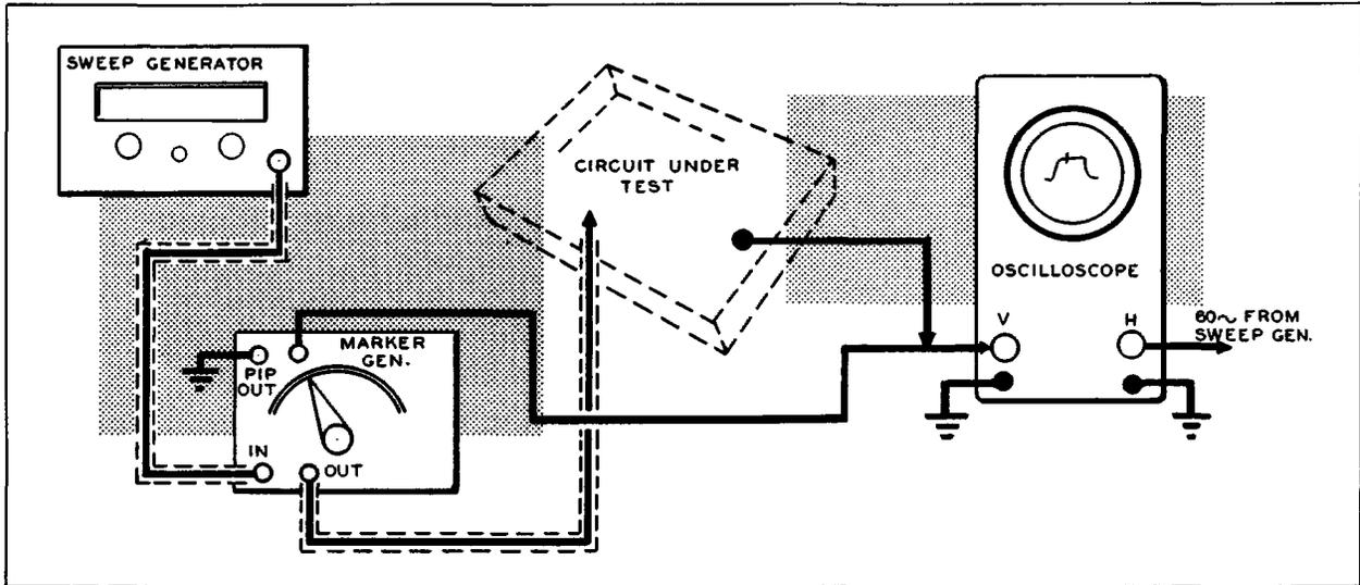
Figure 12. Instrument Set-Up Using the Marker Generator Shown in Figure 11.
