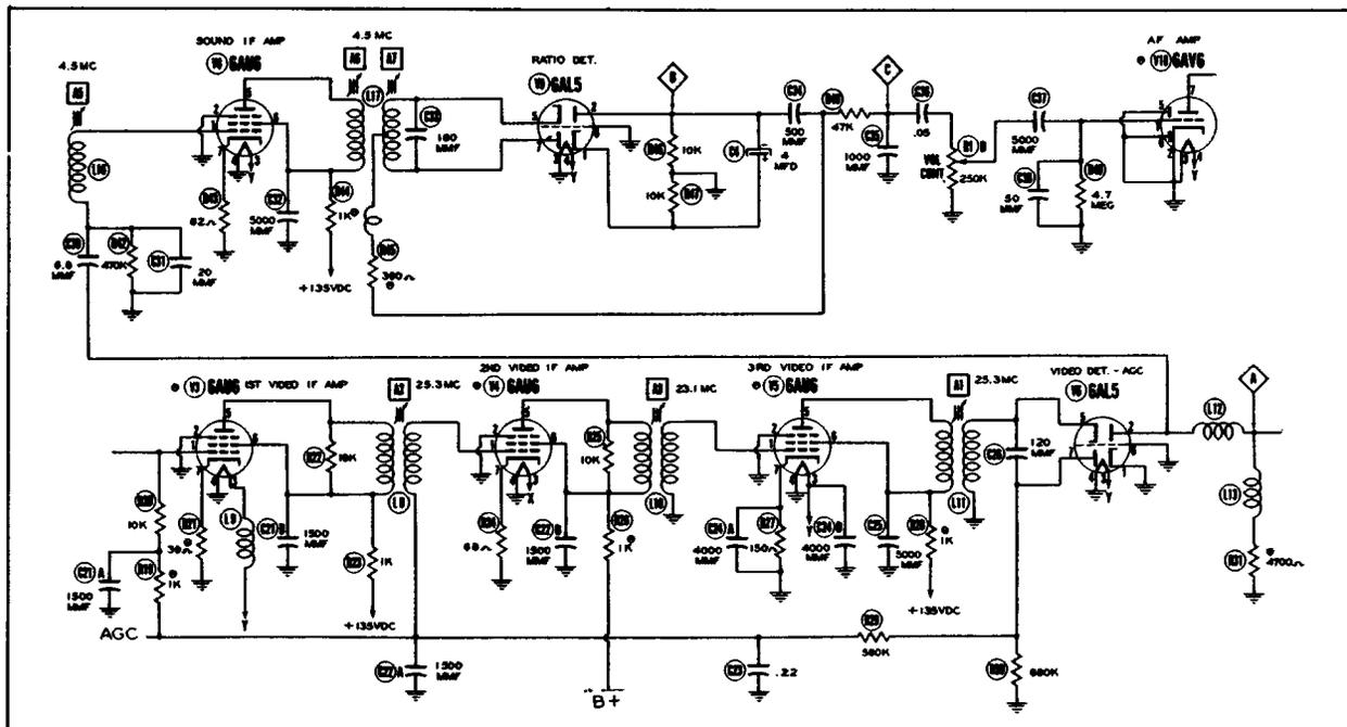
Figure 22. A Sound System of a Television Receiver Employing a Ratio Detector.
