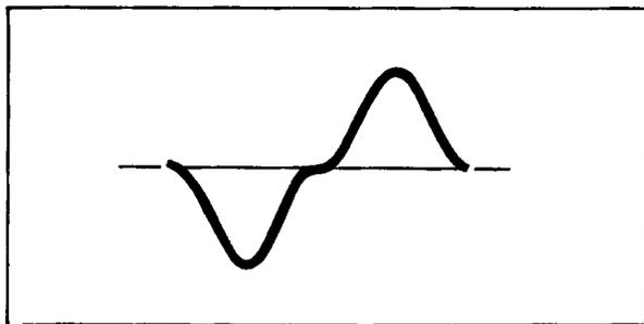
Figure 6. Response Distortion when the Secondary Slug is Misadjusted.
