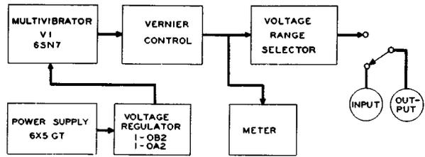
Figure 32. Block Diagram of the Hickok Model 630 Television Voltage Calibrator.
