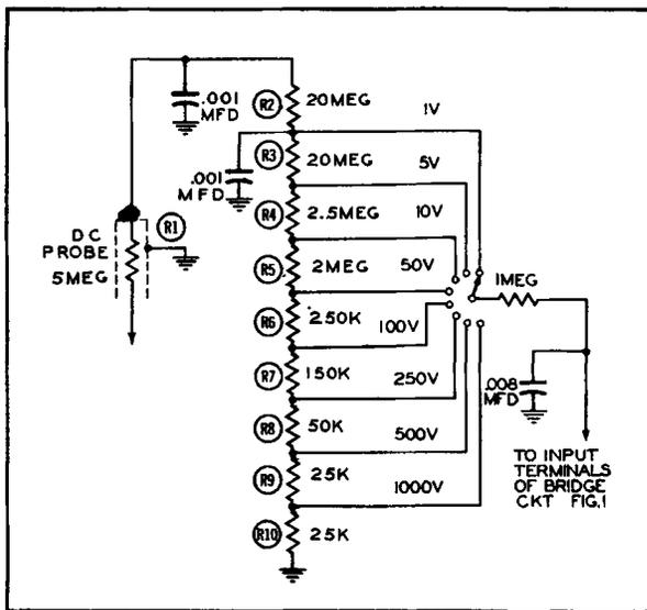
Figure 3. A Voltage Divider Network Across VTVM Input.
