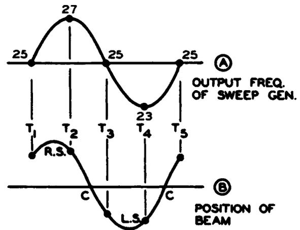
Figure 17. To Illustrate Why Double Patterns are Obtained on the Screen.
