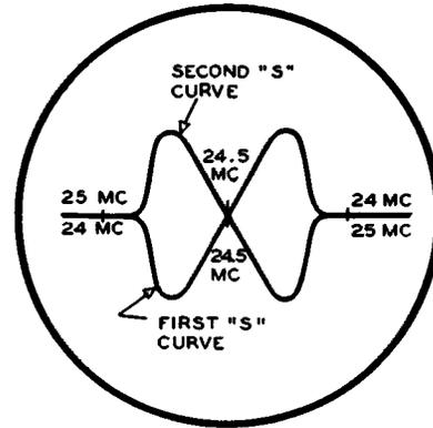
Figure 11. A Double "S" Curve Produced When the Scope Beam is Deflected by a 120 Cycle Saw-Tooth Voltage.
