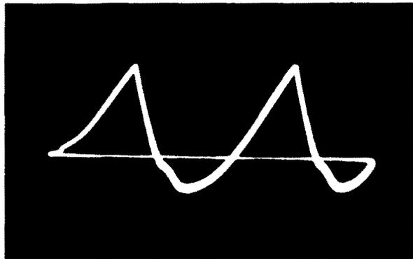
Figure 3. The Cathode Waveform of the Horizontal Output Amplifier in Figure 1.
