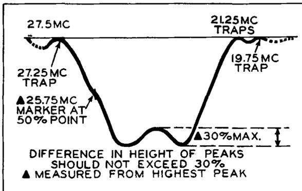
Figure 35. The Overall Video IF Response Curve Recommended by Another Manufacturer. Note Dip in Center of Curve.
