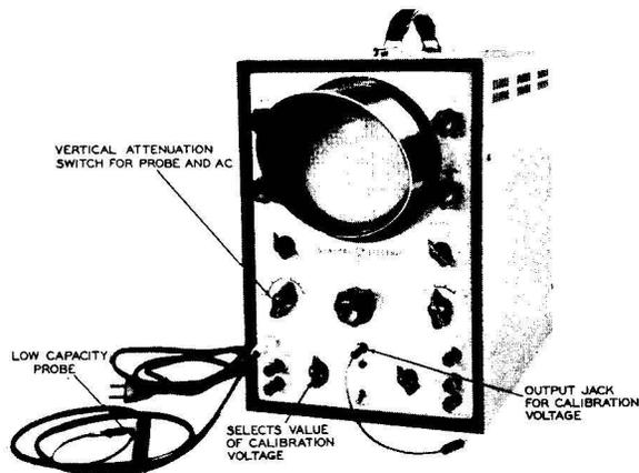
Figure 26. Oscilloscope Containing a Built-In Low-Capacity Probe. Provision is Also Available for Measuring Peak-To-Peak Values of Any Waves Depicted on Screen. Courtesy General Electric Company.
