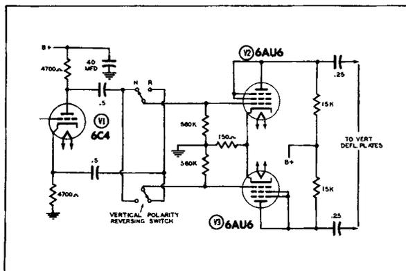
Figure 20. Simplified Diagram of the Vertical Reversing Switch Circuit in the Precision Oscilloscope.
