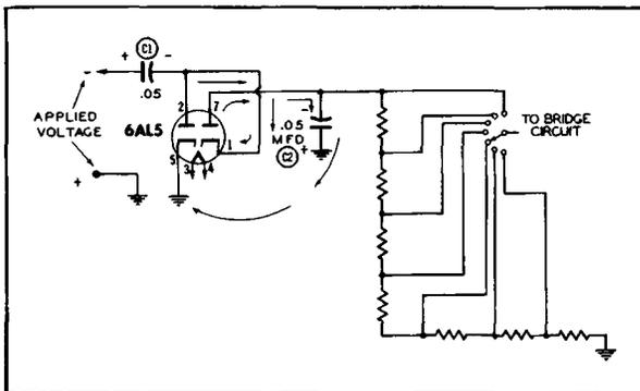
Figure 11B. The Full Peak-to-peak Voltage Is Developed Across C2. See Text.
