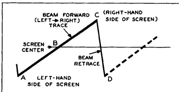
Figure 5. The most Common Type of Voltage which Is Applied to the Horizontal Deflection Plates in a CRT Is the Saw-Tooth Wave.
