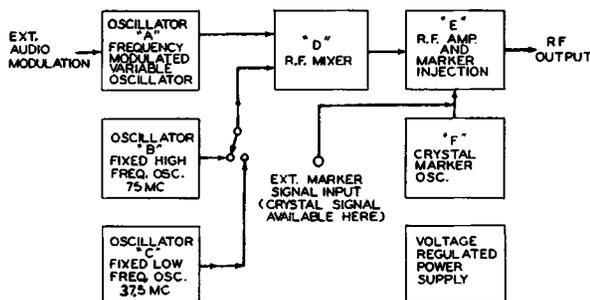
Figure 23. A Simplified Block Diagram of the Sweep Generator Shown in Figure 22.
