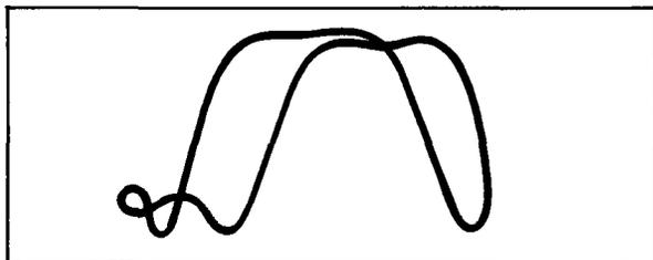
Figure 29. Insufficient Sweep Width for Phasing.
