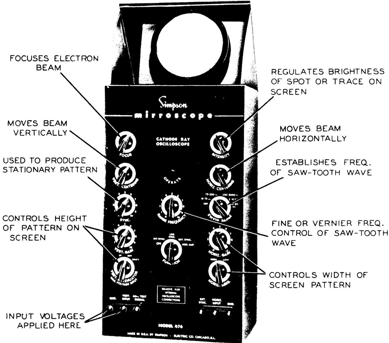
Figure 2. The Front Panel Controls of an Oscilloscope. (Model 476, Courtesy of Simpson Electrical Co.)
