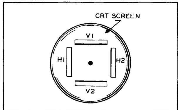
Figure 3. The Horizontal Deflection Plates (P1 and P2), the Vertical Deflection Plates (V1 and V2), and the Fluorescent Screen of a CRT as Seen Head-On. With no Deflection Voltages Applied to any of the Plates, the Electron Beam Will Strike the Screen at the Center.
