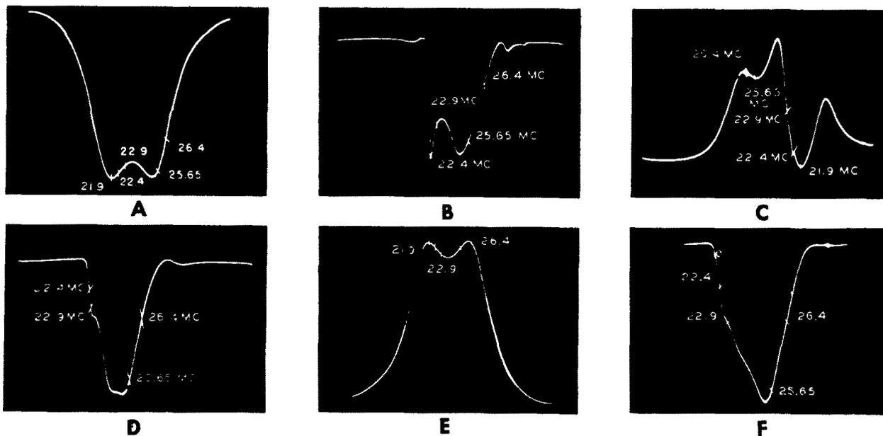
Figure 42. The Response Characteristics of the Tuned Circuits in the IF System of Figure 41.
