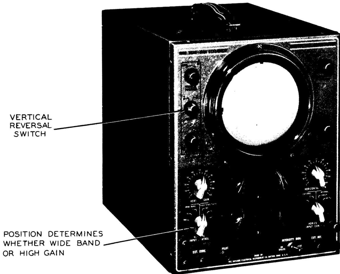
Figure 38. An Oscilloscope Capable of Providing Either Wide-Bandpass (4 mc) or High Gain. (Model CRO-2, Courtesy of Jackson Electrical Instrument Co.)
