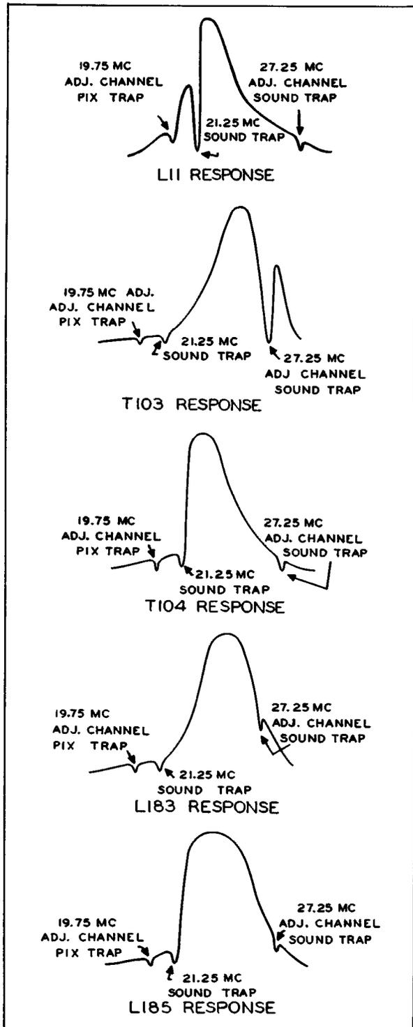
Figure 39. Representative Response Curves for Each of the Tuned Circuits (Except Traps) in Figure 24.
