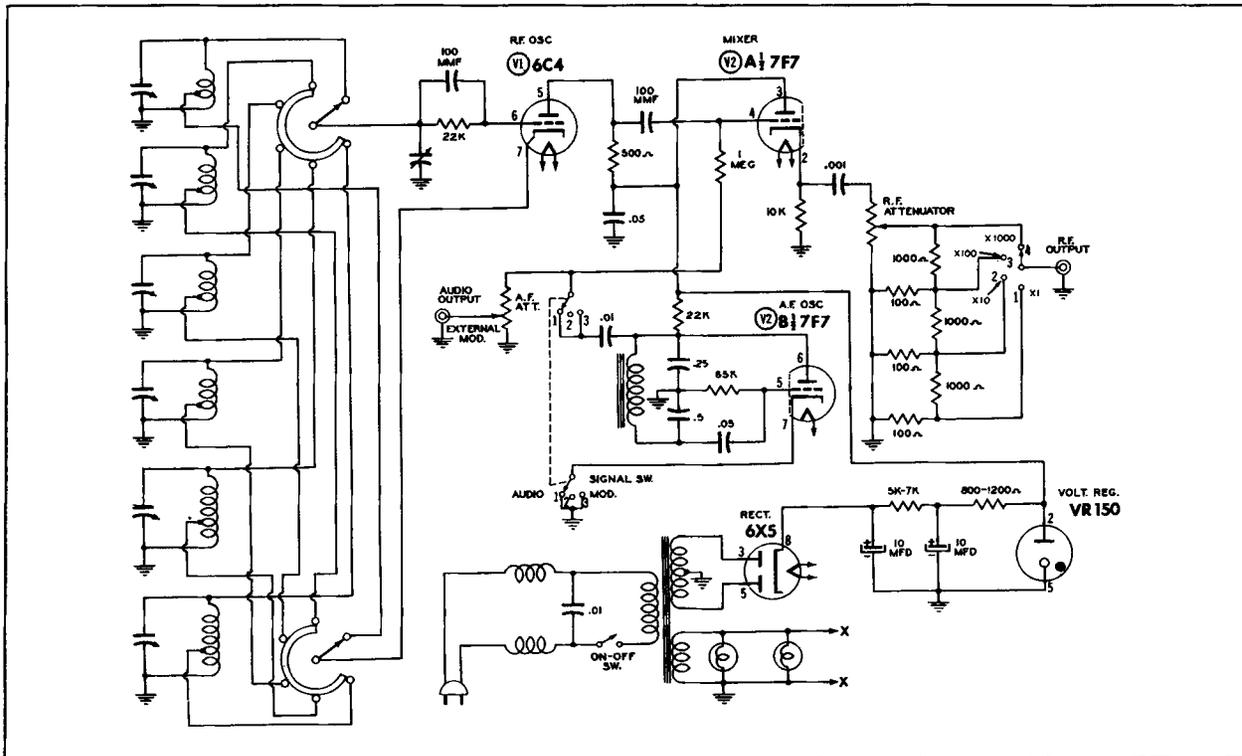
Figure 1. The Circuit Diagram of a Simple AM Generator.
