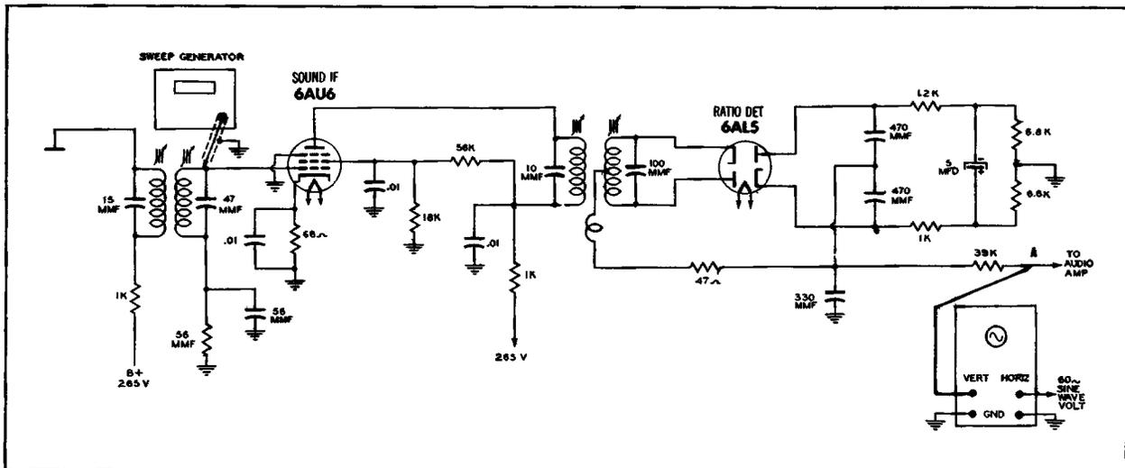
Figure 2. The Manner in Which the Response Pattern of a Ratio Detector Would be Obtained.
