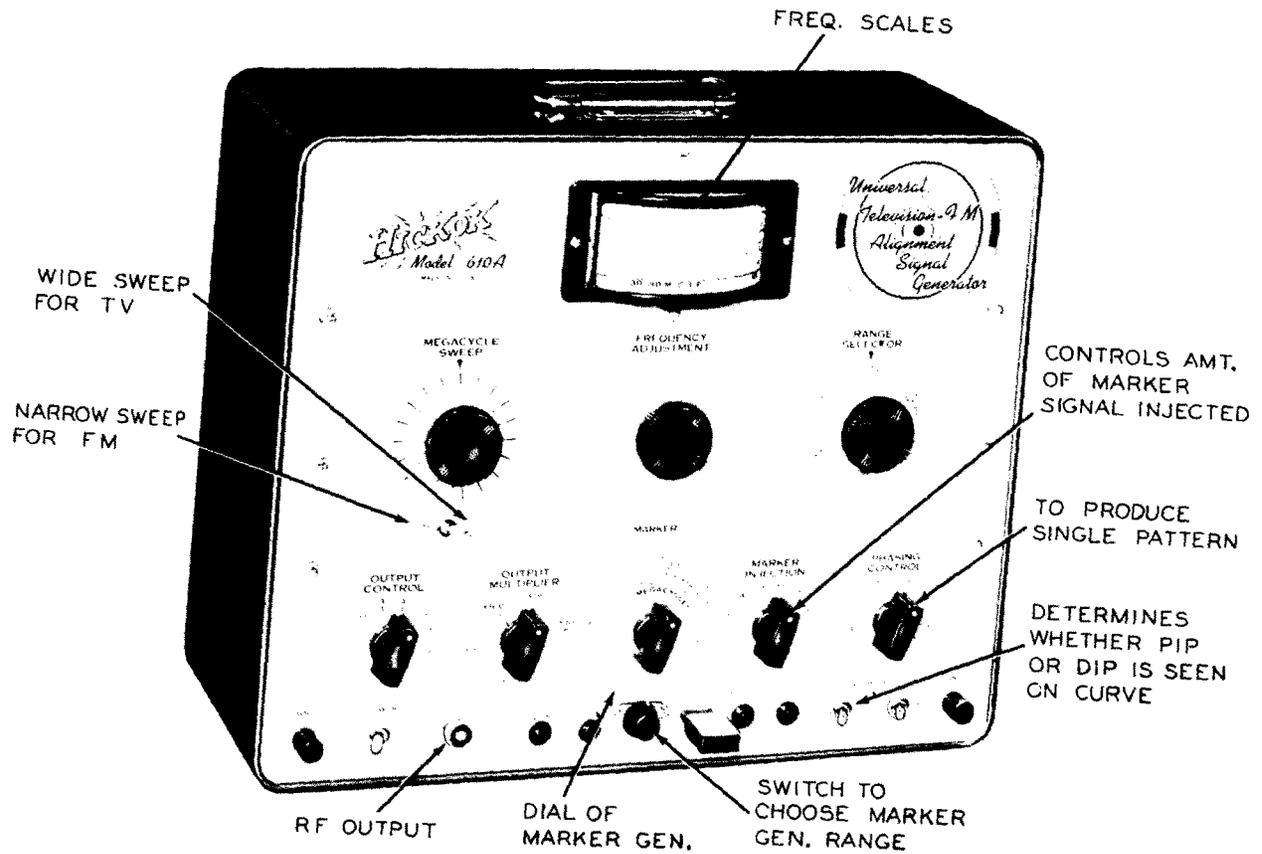
Figure 24. A Sweep Generator Possessing its Own Marker Generator. (Model 610-A, Courtesy Hickok Electrical Instrument Co.)
