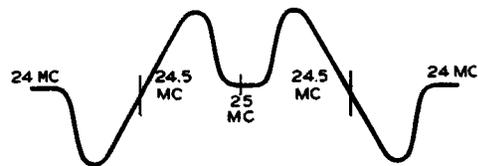
Figure 12. When a 60 Cycle Saw-Tooth Deflection Voltage is Used in the Oscilloscope, The Screen Presentation Will Appear as Shown.
