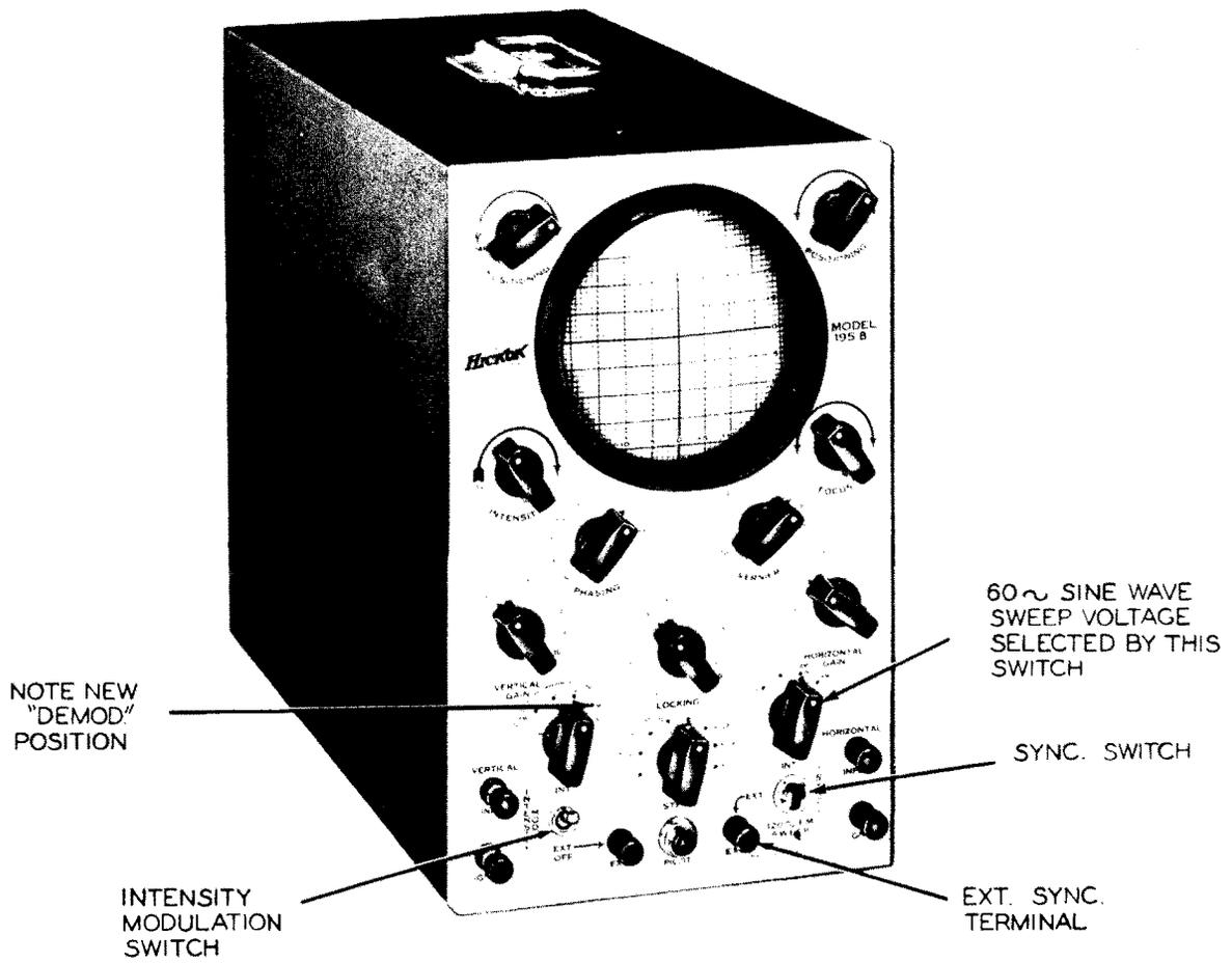
Figure 22. Hickok Model 195-B Oscilloscope. (Courtesy Hickok Electrical Instrument Company.)
