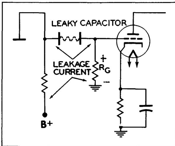
Figure 20. A Leaky Coupling Capacitor Will Place a Positive Potential at the Grid of the Following Tube.
