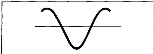
Figure 5. Response Distortion When the Discriminator Primary is Misadjusted.
