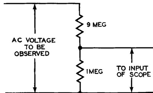
Figure 14. A resistive Voltage Divider Network Suggested by Supreme, Inc. for use with their Oscilloscope of Figure 13.
