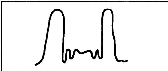
Figure 33. Curve with Incorrect Scope Deflection.
