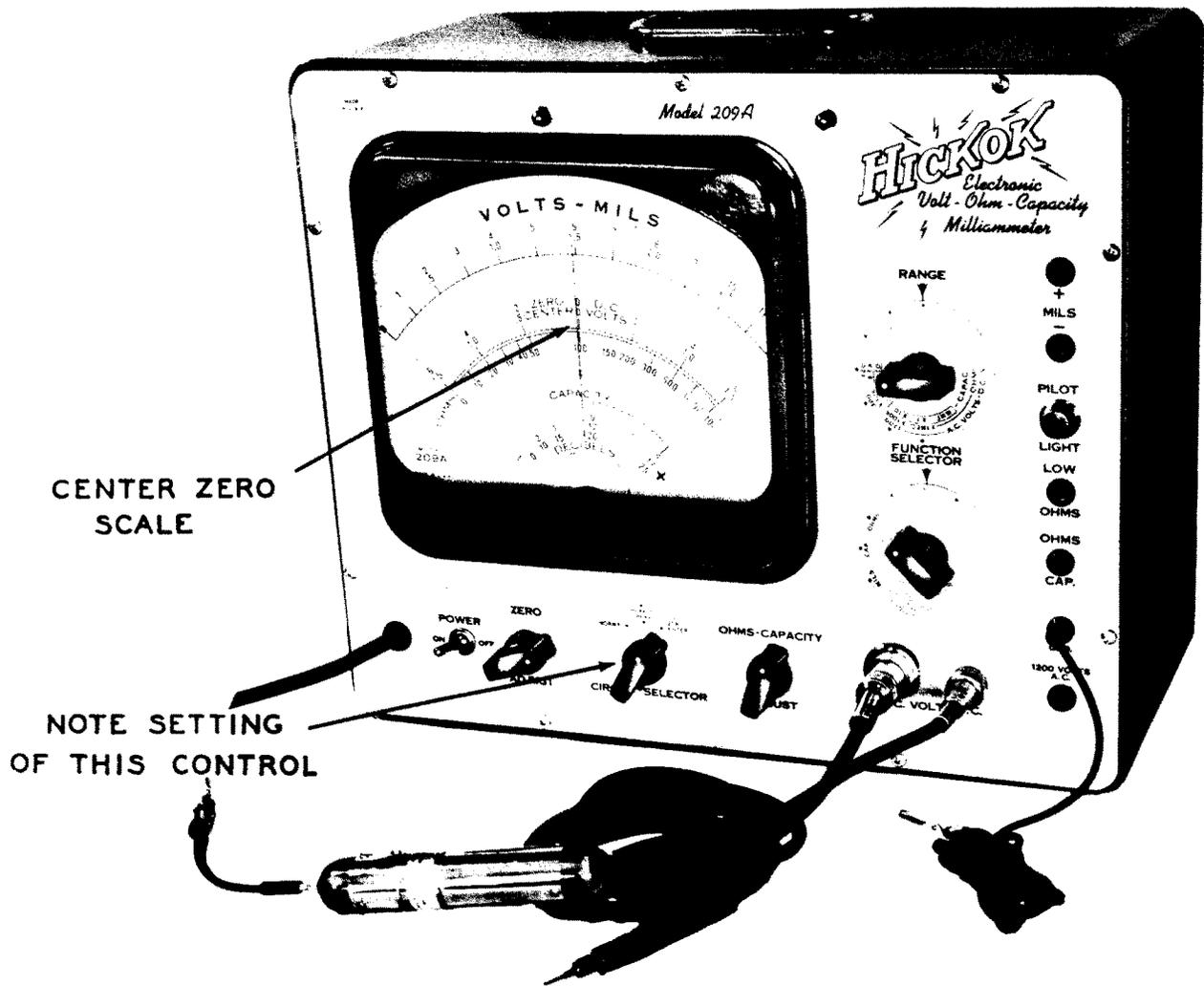
Figure 6. A VTVM with a Special Zero Center Scale. (Model 209A, Courtesy of Hickok Electrical Instrument Co.)
