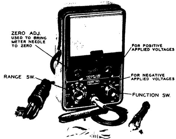
Figure 2. The Front Panel Controls on a Typical VTVM. Courtesy of Hickok Electrical Instrument Co.
