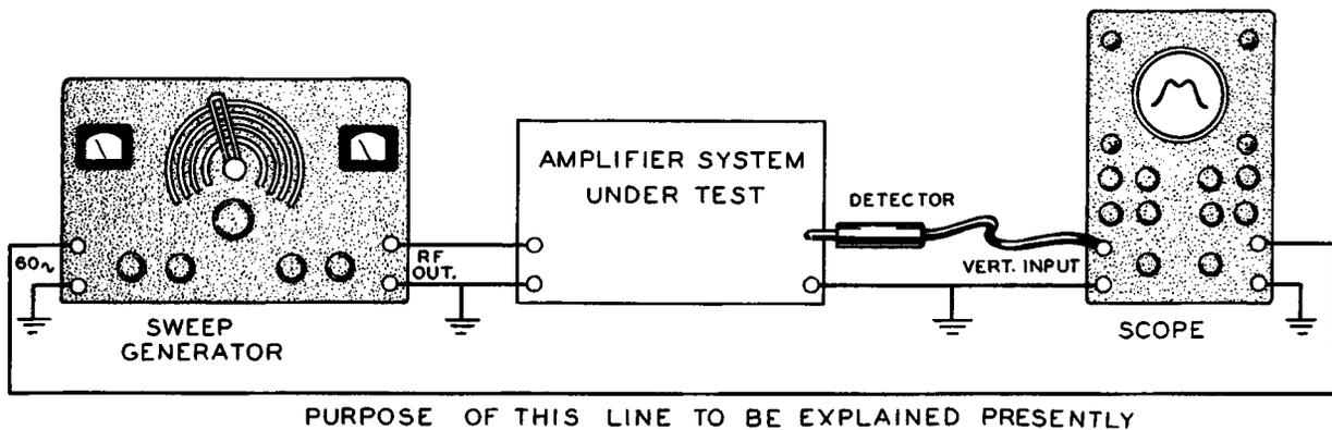
Figure 12. How to Connect Sweep Generators and Oscilloscopes to an Amplifier System to Obtain Its Response Curve. See Text.
