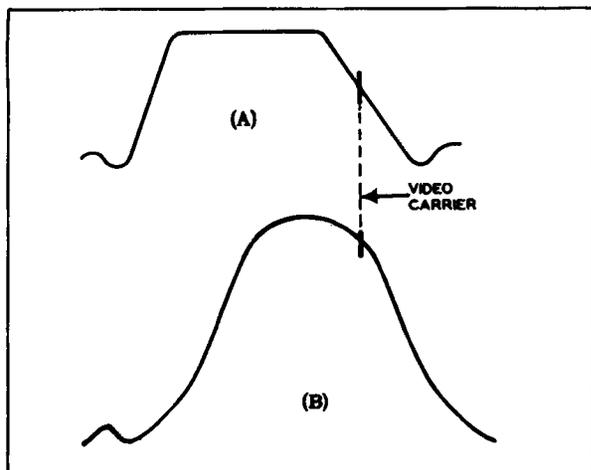
Figure 36. (A) Normal Video IF Response Curve. (B) Modified Response for Fringe Operation.
