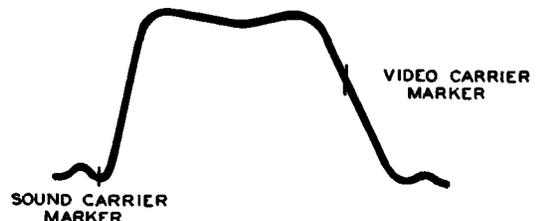
Figure 47. Overall RF and IF Response Curve of a Television Receiver Such as the One Shown in Figure 24.
