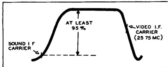
Figure 37. In an Intercarrier Receiver, The Sound Carrier Should Receive no More Than 5% of the Total Amplification Available in the Video IF System.
