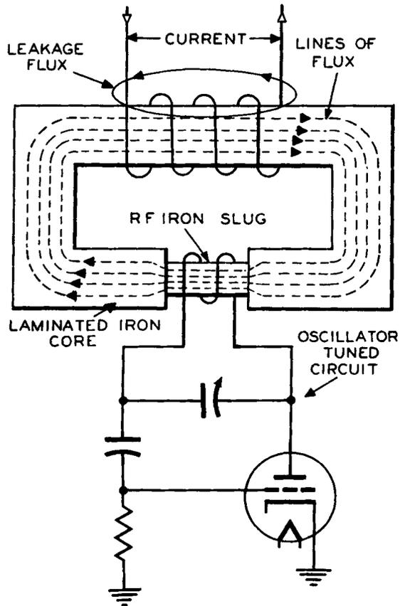
Figure 35. The Basic Modulator and Oscillator Circuit Used in the G.E. Variable Reluctance Generator.
