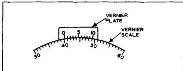
Figure 12. The Vernier Scale Reading Is 40.2 Because Only the Two (2) Mark on the Vernier Plate Is Directly Over a Vernier Scale Division.
