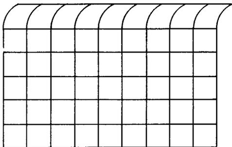
Figure 10. Horizontal Pull at Top of Picture.
