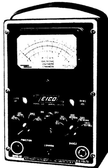
Figure 10B. An Eico VTVM Instrument is Set up to Measure AC Voltages. Note: Function Switch is Set to AC Volts Position; Setting of Range Switch is dependent on Voltage to be Measured. Courtesy of Eico.
