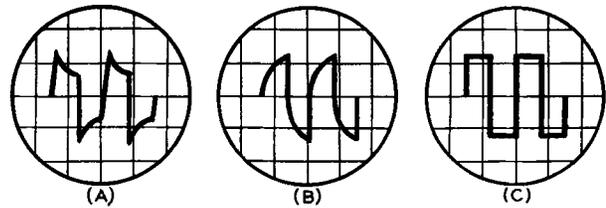
Figure 25. (A) Padder Capacitor Value too High. (B) Padder Capacitor Value too Low. (C) Padder Properly Adjusted.
