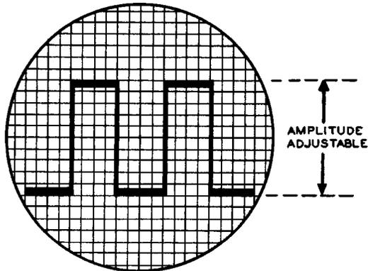
Figure 34. The Screen Presentation Produced by the Hickok Calibrator.
