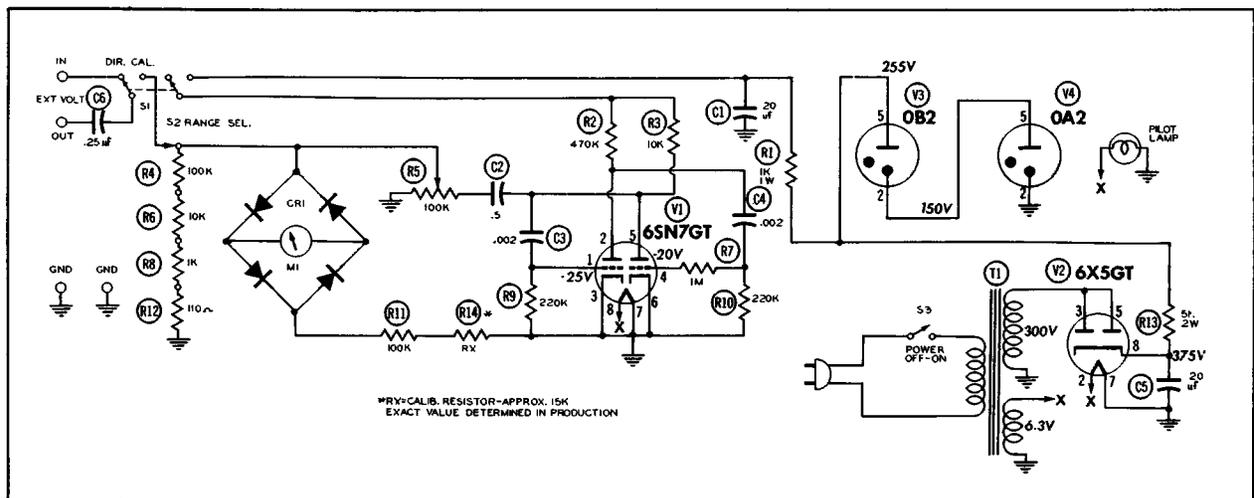
Figure 33. The Schematic Diagram of the Hickok Model 630 Television Voltage Calibrator.
