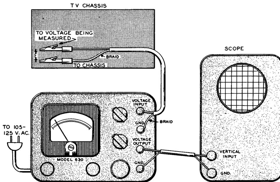
Figure 35. How the Hickok Calibrator is Connected for Use.
