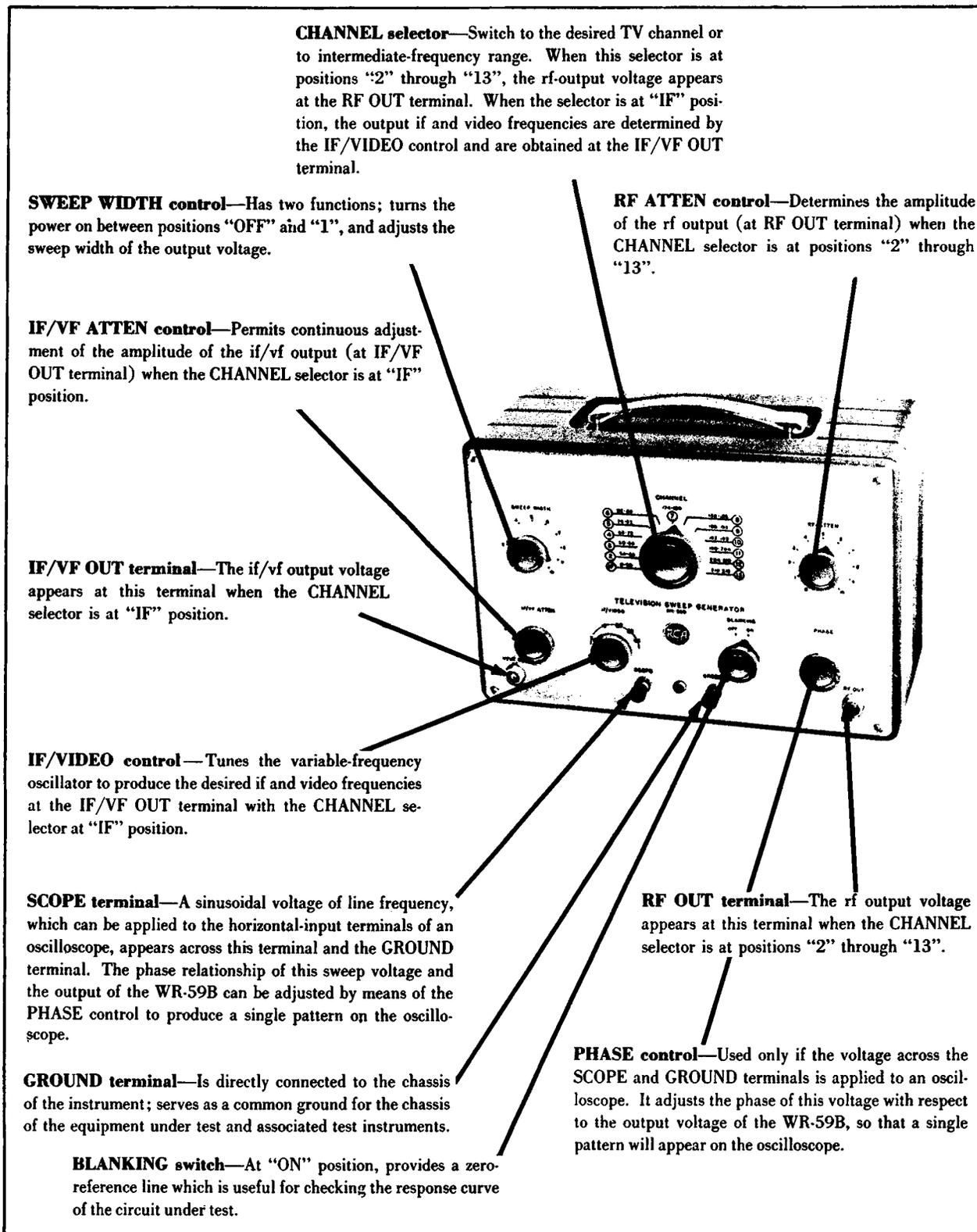
Figure 33. Another Sweep Generator in Which the Various Frequencies are Selected by Means of a Switch. Courtesy of RCA.
