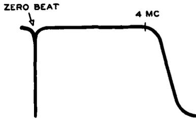
Figure 51. An Ideal 4 mc Video Amplifier Response Pattern.
