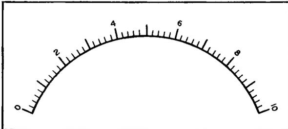
Figure 26A. A Scale Which Is Similar to the One Shown in Figure 24. Note That Only Alternate Major Lines are Numbered.
