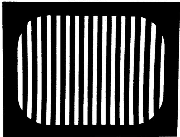
Figure 5. Vertical Bars to Check Horizontal Linearity.
