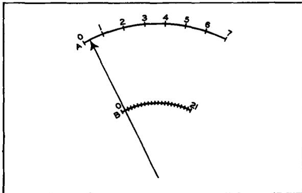
Figure 4. The Vernier Scale "B" Helps to Set the Pointer to a Desired Point on Scale "A".
