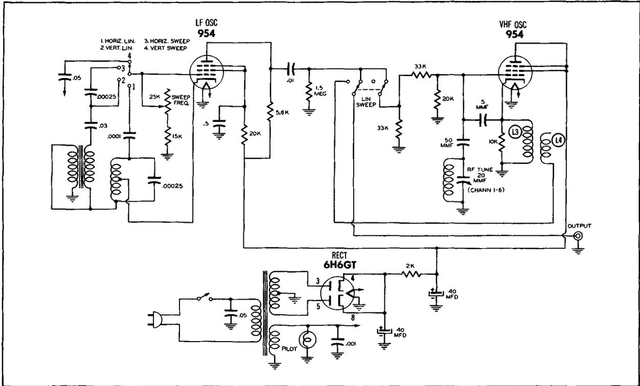
Figure 20. The Schematic Diagram of the Superior Cross-Bar Generator.
