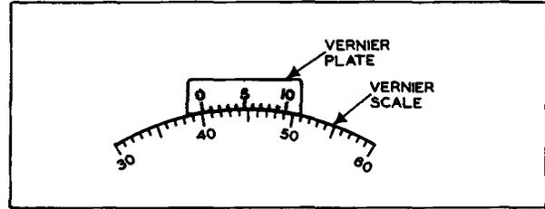
Figure 11. The Vernier Scale Reading Is 40.1.
