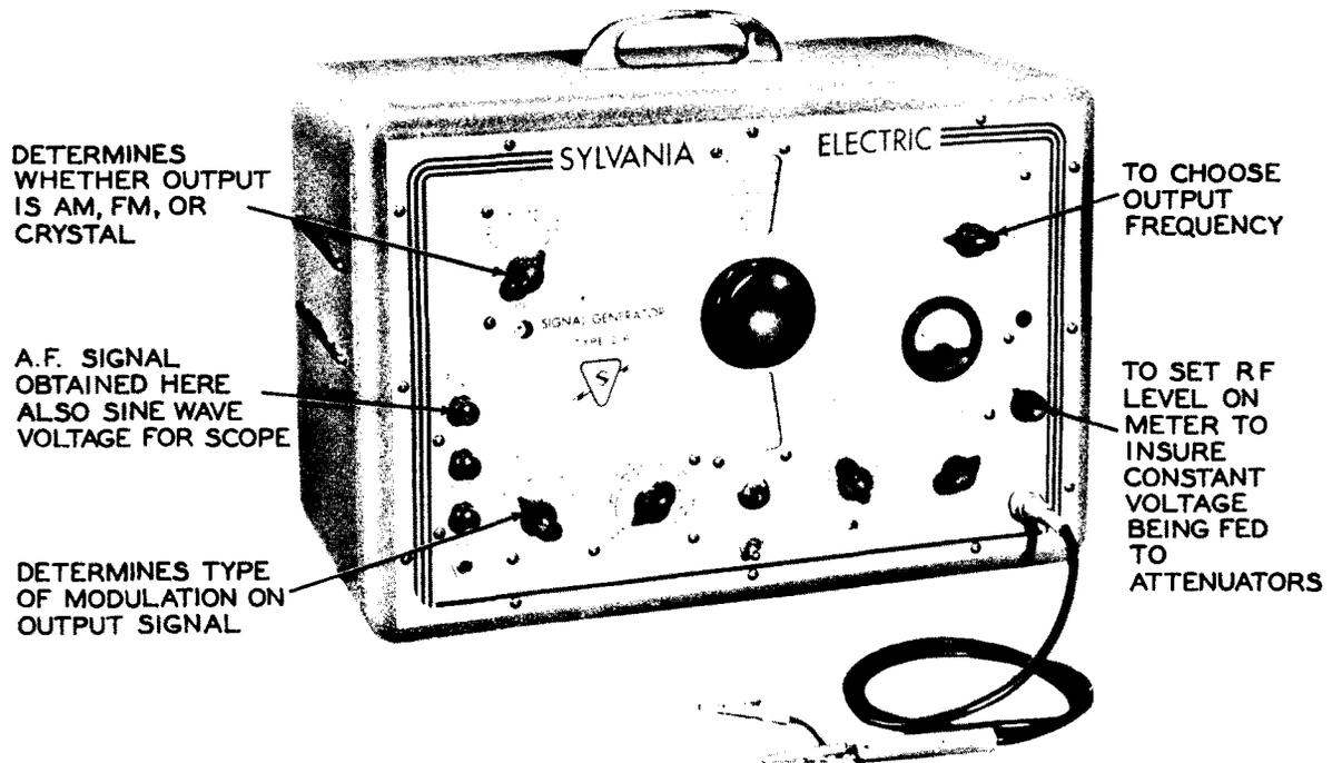
Figure 38. A Sweep Generator Designed Primarily for AM-FM Application, Although it Can Be Employed for Peaking of TV Circuits. (Model 216, Courtesy of Sylvania Electric Products Inc.)
