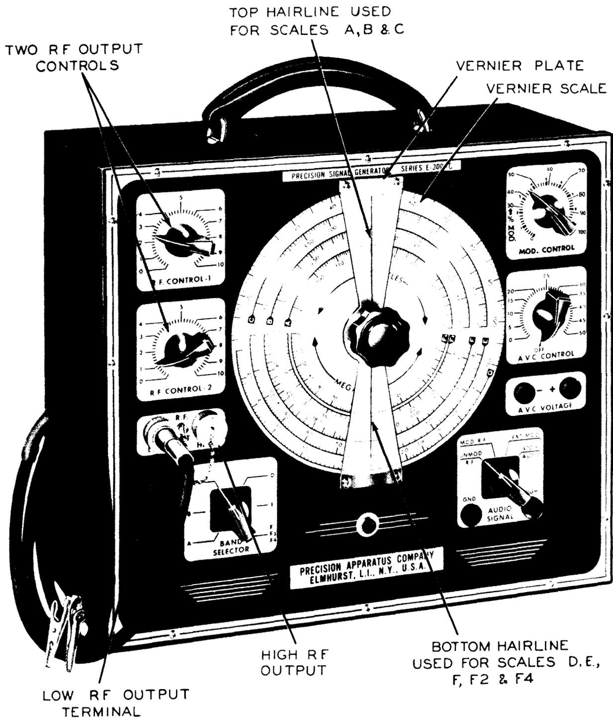
Figure 9. The Precision Model E-200C Signal Generator. The RF Attenuator Controls Are Both Continuously Variable. This Is a Departure from the Previous Instrument. (Courtesy of Precision Apparatus Company, Inc.)
