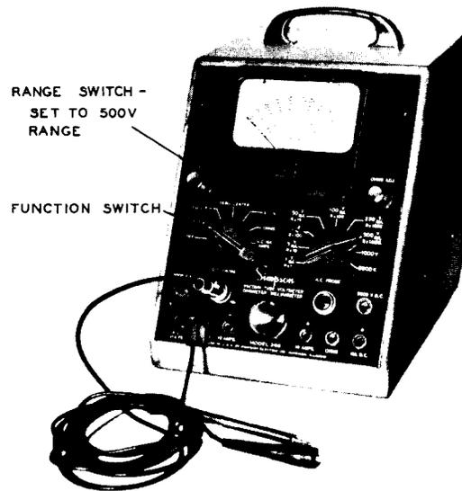
Figure 5. VTVM of Figure 4 Set up to Measure Voltages up to 500 Volts DC. Nothing has Changed Except Setting of Range Control. Courtesy of Simpson Electric Co.
