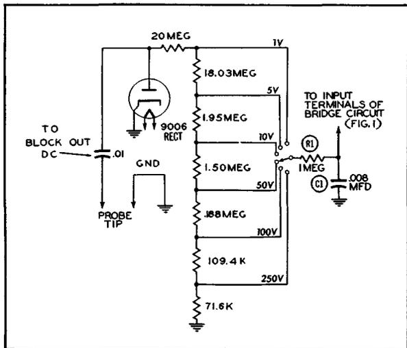
Figure 7. A Simplified Schematic of the AC Voltmeter Circuit of a VTVM.
