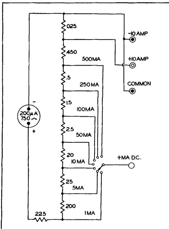
Figure 19. A Simplified Milliammeter and Ammeter Circuit Used in a VTVM.
