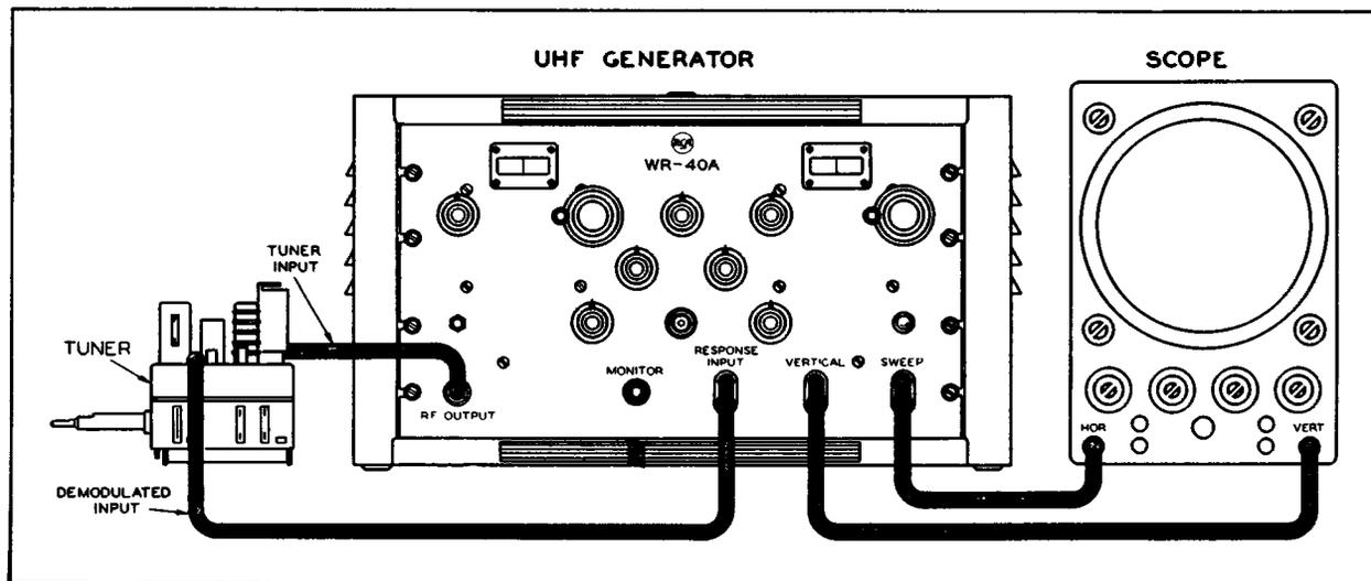
Figure 15. The Manner in Which the UHF Generator is Employed to Align a UHF Tuner. Courtesy RCA.
