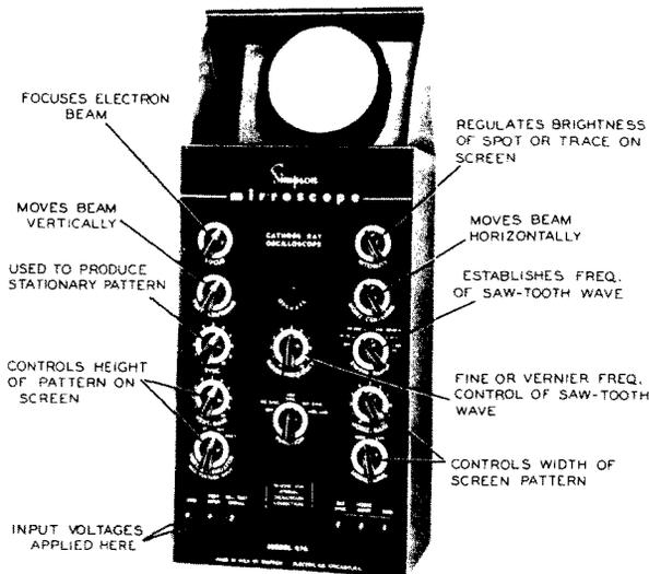
Figure 2. The Front Panel Controls of an Oscilloscope. Courtesy Simpson Electric Company.
