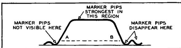
Figure 7. When the Marker Signal Passes Through the Circuit Under Test, it is Frequently Difficult to Discern the Marker Pips Below Level A-B.
