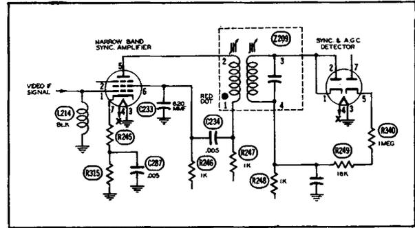
Figure 5. The Narrow-Band Sync Amplifier Used in many DuMont Receivers.
