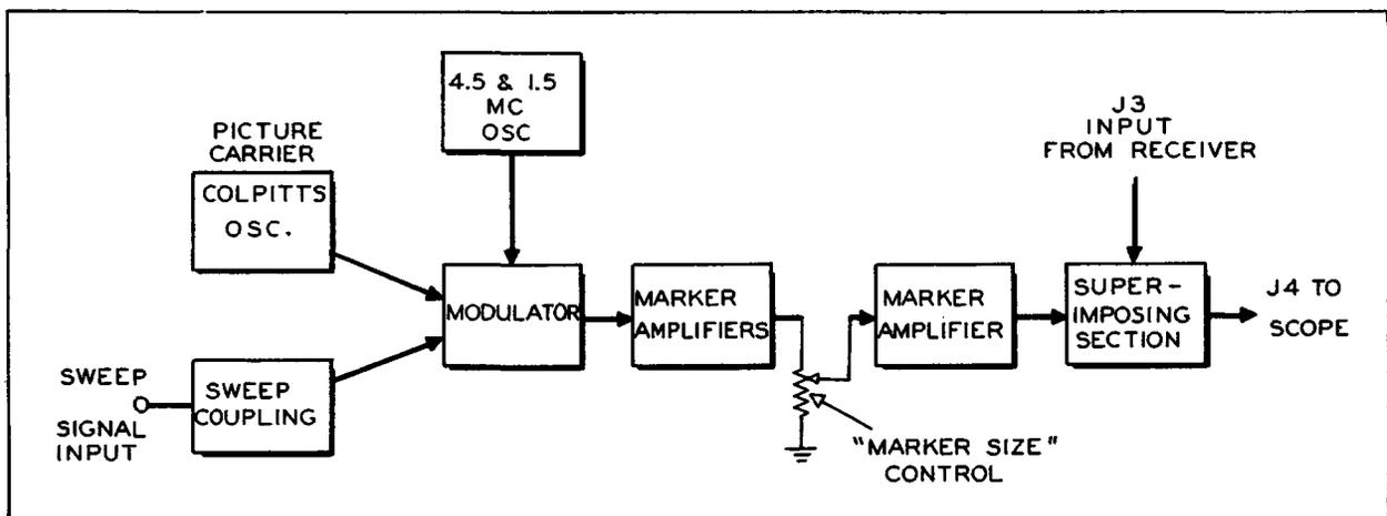
Figure 9B. Block Diagram of The G. E. Marker Generator.
