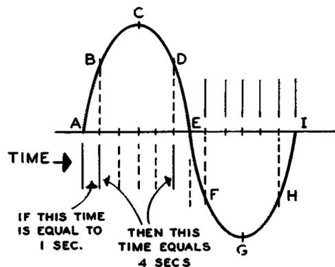
Figure 10. The Rate of Change Varies at Different Points on a Sine Wave.
