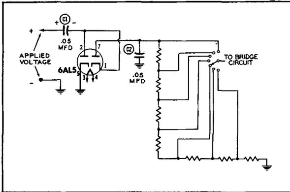
Figure 11A. A Voltage Doubler Circuit for Peak-to-peak Measurements. The Positive Peak Voltage Appears Across C1. See Text.
