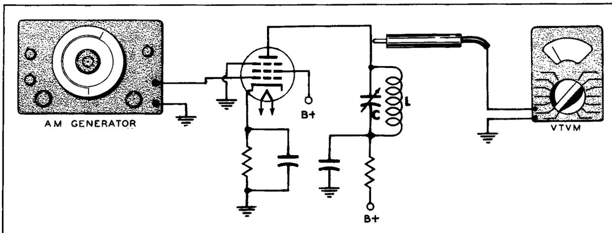
Figure 5. The Equipment Set Up to Obtain the Response Curve of LC.
