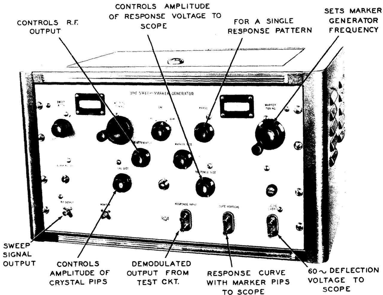
Figure 13. A UHF Sweep-Marker Generator. (Courtesy of RCA.)
