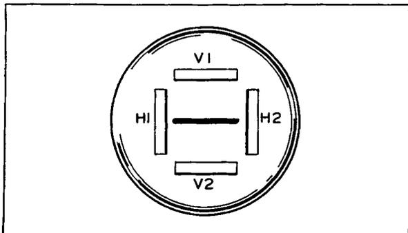
Figure 4. An Alternating Voltage Applied to the Horizontal Deflection Plates H1 and H2 Will Produce a Line on the Screen.
