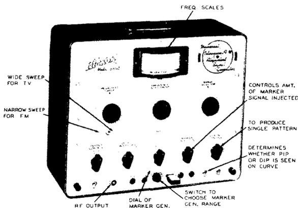
Figure 24. A Sweep Generator Possessing its Own Marker Generator. Courtesy of Hickok Electrical Instrument Co.
