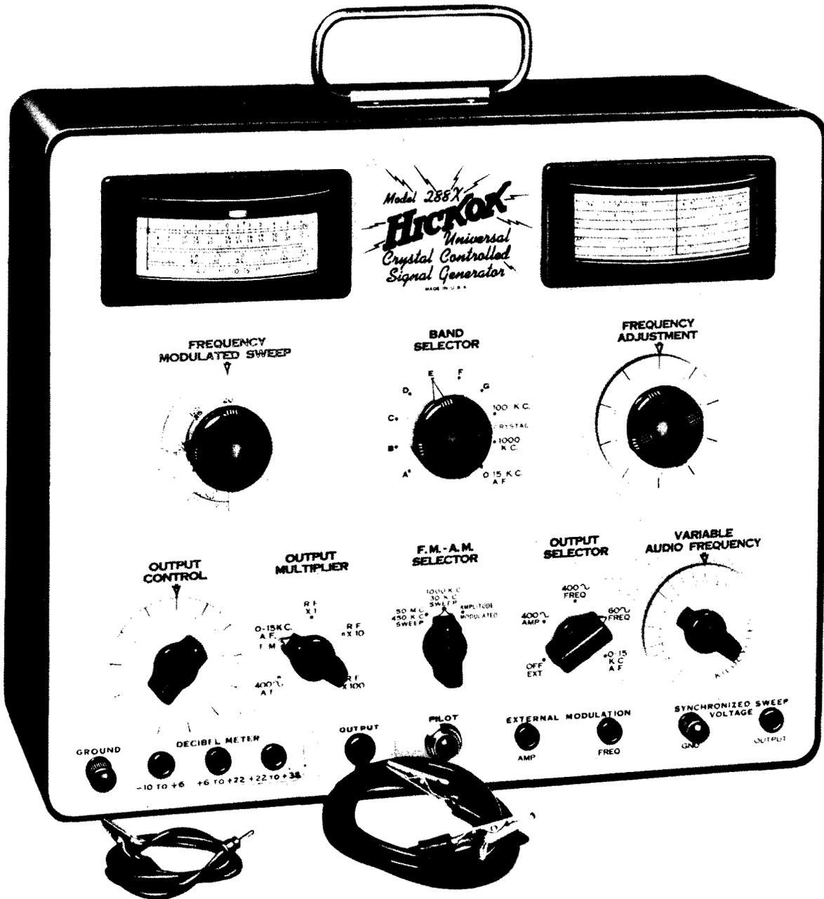
Figure 40. Another Sweep Generator Designed Principally for AM-FM Application. (Model 288, Courtesy of Hickok Electrical Instrument Co.)
