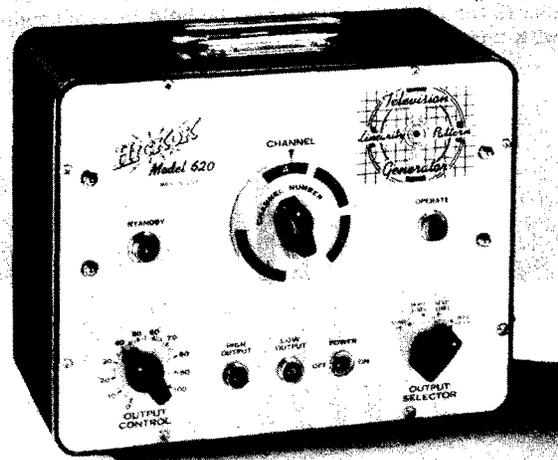
Figure 21. The Hickok Linearity Generator.
