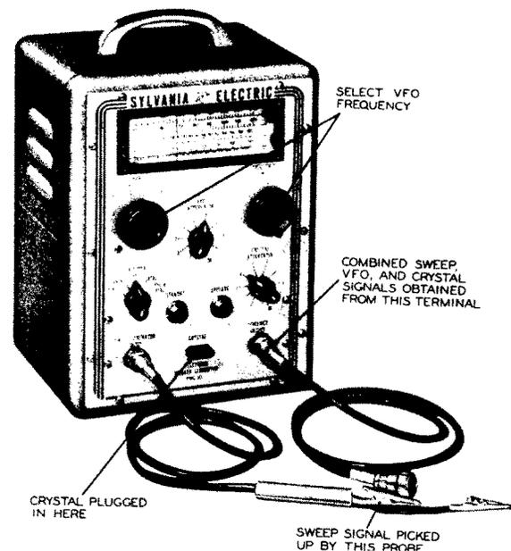
Figure 1. Sylvania Television Marker Generator. Courtesy Sylvania Electric Products, Inc.
