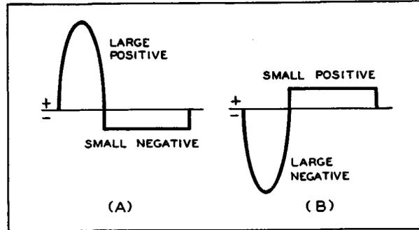
Figure 17. Non-Symmetrical Waveforms which Could Make it Difficult to Obtain Suitable Synchronization in an Oscilloscope. See text.
