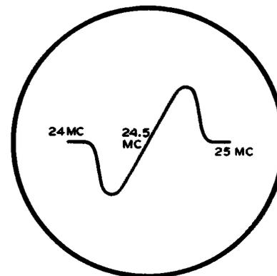
Figure 4. When the Phase Control has Been Properly Adjusted, the Two Patterns of Figure 3 Will Blend Together, as Shown.
