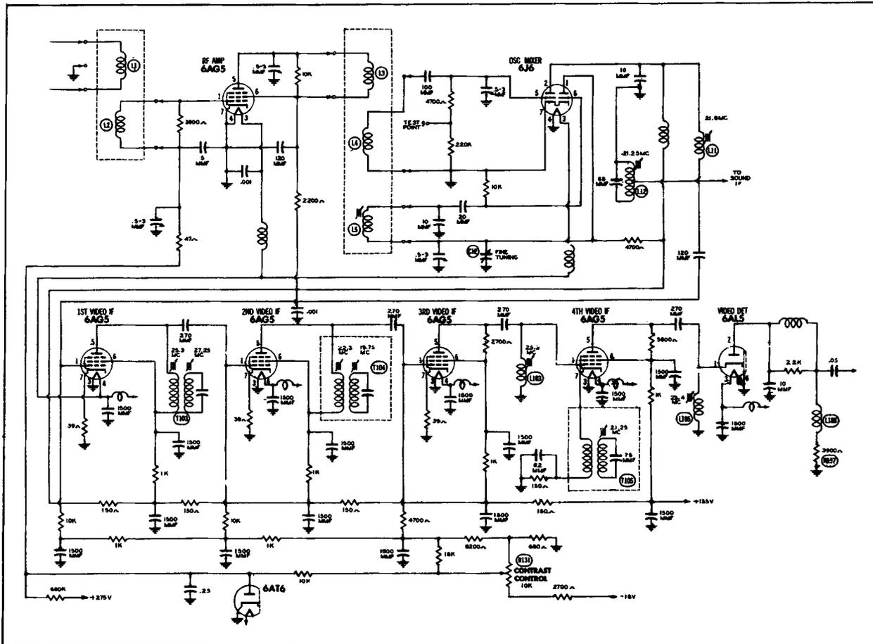
Figure 24. The RF and IF Sections of the Popular Model 630 Receiver. These Circuits are Widely Copied.
