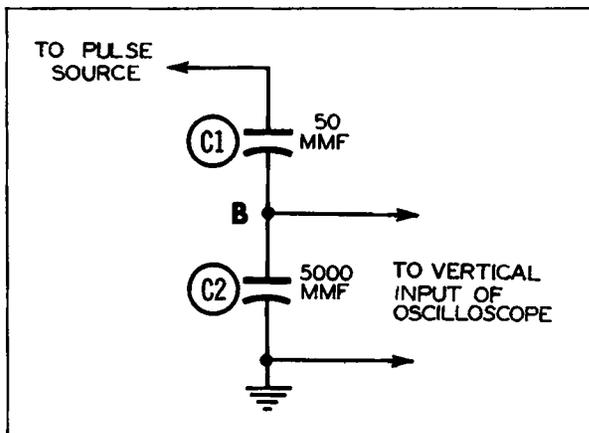
Figure 4. A Capacity Voltage Divider which Can Be Used to Observe the Pulse Voltages at the Plate of the Horizontal Output Amplifier.
