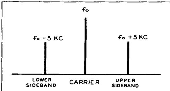
Figure 1. A Signal Which Is Broadcast by an AM Radio Station can Occupy a Maximum Band Width of 10 kc.
