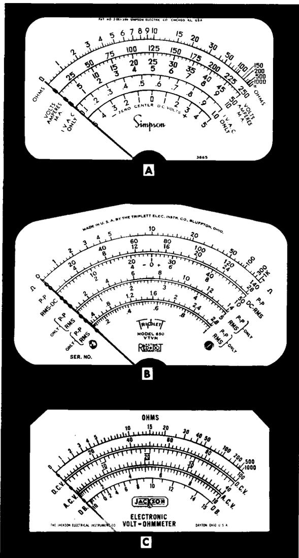
Figure 22. The Meter Scales of Several Vacuum-Tube Volt-Meters. (A) Courtesy of Simpson Electric Company. (B) Courtesy of Triplet Electrical Instrument Company. (C) Courtesy of Jackson Electrical Instrument Company.
