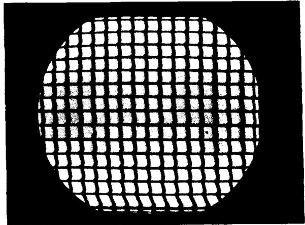
Figure 29. Poor Isolation Between Horizontal and Vertical Deflection Circuits.
