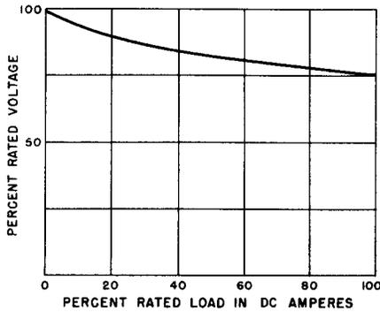
**Fig. 4-13. Voltage Regulation Curve of a Typical Copper-Oxide Rectifier Cell.**
