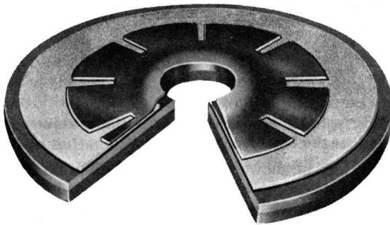
**Fig. 5-2. Cut-Away View of a Selenium Rectifier Cell. (Courtesy of General Electric Co.)**
