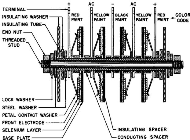
**Fig. 5-5. Selenium Rectifier Stack Construction. Full-Wave Bridge, Using Contact Type Cell.**
