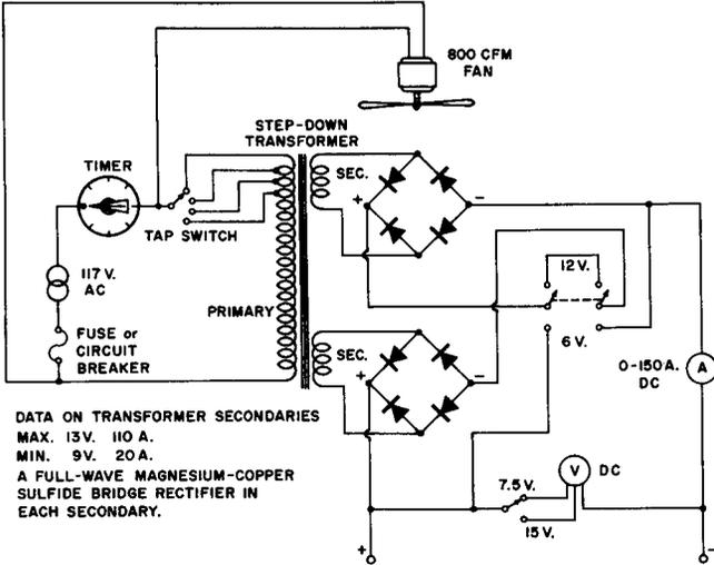
**Fig. 10-8. A More Elaborate Battery Charging Circuit.**
