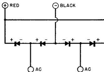
(A) A Single-Phase, Full-Wave, Rectifier Bridge Using Four Cells in a Stack Assembly With the Outer Cells Positive and Strapped Together.
