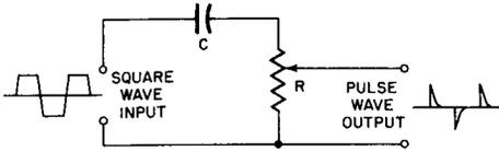
**Fig. 13-9. Circuit for Obtaining a Pulse Waveform from a Square Wave Input.**
