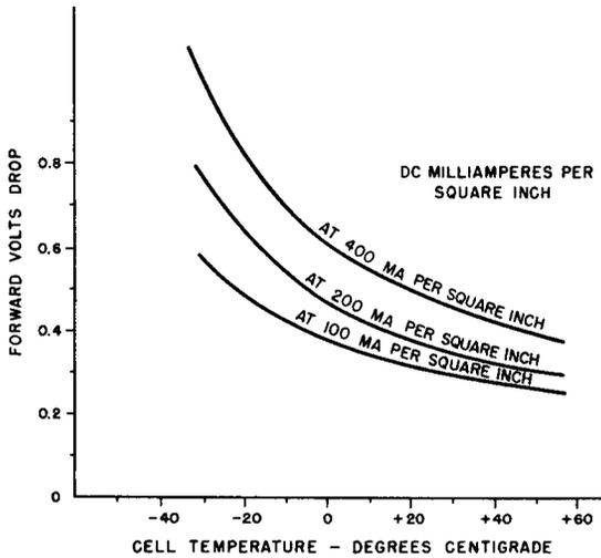
**Fig. 4-10. Temperature Characteristics of Copper-Oxide in Forward Direction.**
