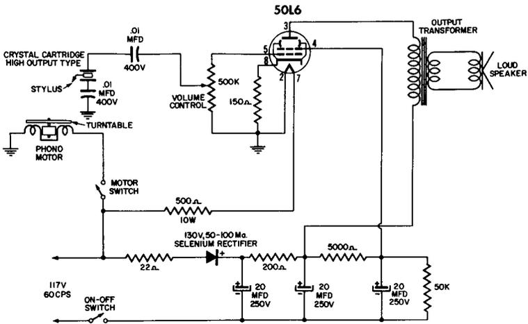
**Fig. 11-3. A Phono Amplifier Using a Selenium Rectifier Power Supply.**
