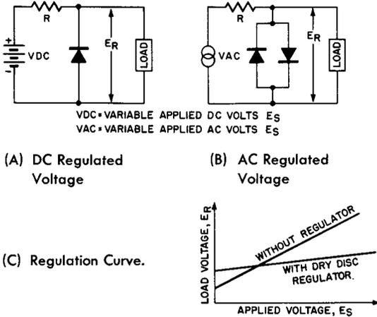
**Fig. 14-10. Voltage Regulator Circuits.**
