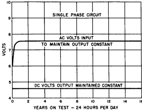
**Fig. 4-16. Aging of Copper-Oxide Rectifiers—Continuous Life Test.**
