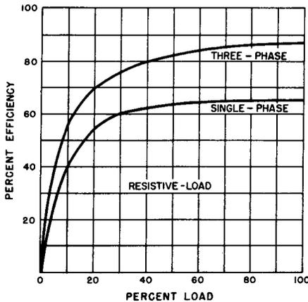
**Fig. 4-15. Efficiency of Single- and Three-Phase, Full-Wave Bridge, Copper-Oxide Rectifier Supplying a Resistive Load.**
