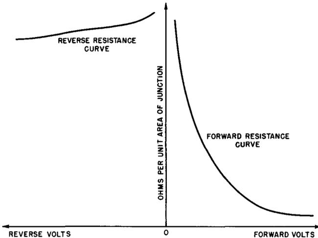
**Fig. 2-8. Static Voltage-Resistance Properties of a Generalized Rectifier Junction of Unit Area Operated Within its Voltage Limits.**
