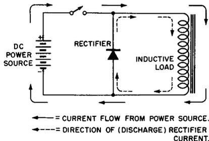
**Fig. 13-1. Metallic Rectifier as an Arc Suppressor.**
