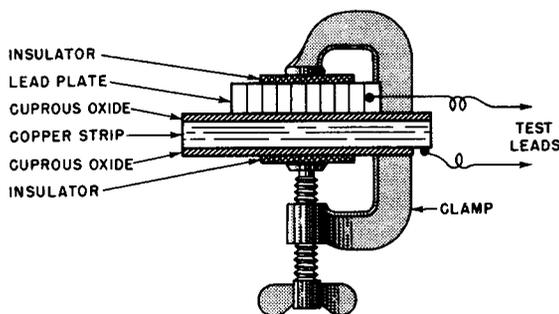
**Fig. 1-6. Exaggerated Cross-Sectional View of Original Copper-Oxide Type, Half-Wave, Metallic Rectifier.**
