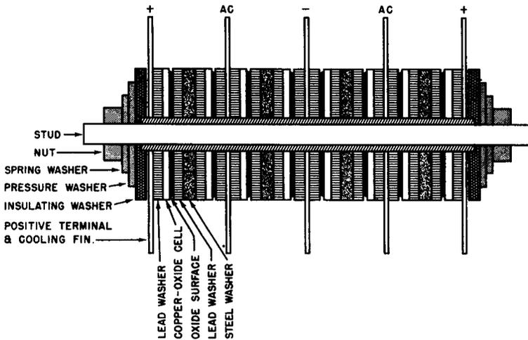
**Fig. 4-4. Cutaway View of a Full-Wave, Copper-Oxide Rectifier Stack Assembly.**
