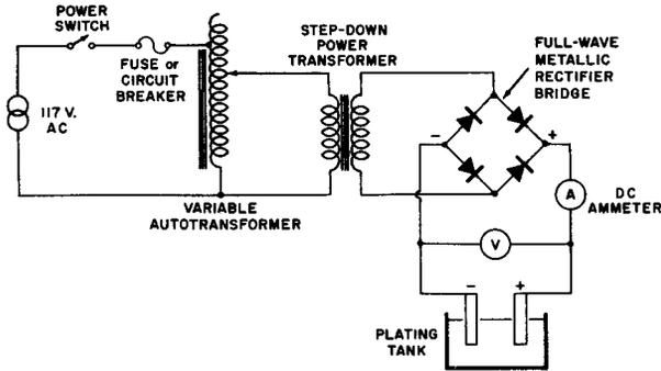
**Fig. 10-10. A Single-Phase, Full-Wave Electroplating Circuit.**
