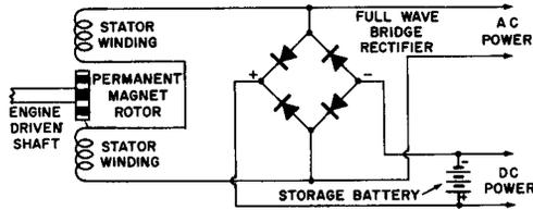
**Fig. 10-15. Metallic Rectifier Application in Automotive Vehicles.**
