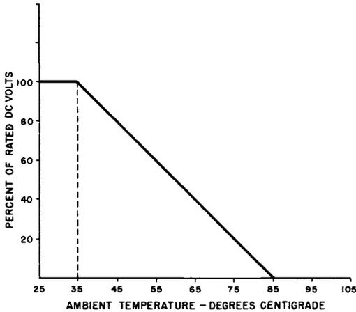
**Fig. 4-17. Voltage Derating for High Ambient Temperatures. No Derating of Output Current.**
