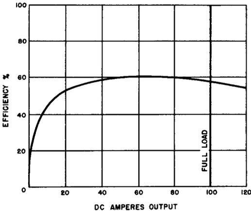
**Fig. 6-16. Efficiency Characteristics of a Magnesium-Copper Sulfide Rectifier Employed in a Three-Phase, Full-Wave Bridge Circuit.**
