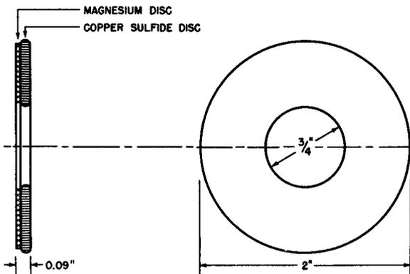
**Fig. 6-4. Cross-Sectional and Front View of a Typical Magnesium-Copper Sulfide Rectifier Cell Without Non-Polarizing Disc.**
