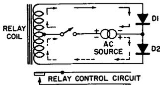
**Fig. 14-11. Full-Wave Rectification Without a Transformer.**
