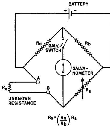
**Fig. 1-7. A DC Wheatstone Bridge for Measuring Unknown Resistances.**
