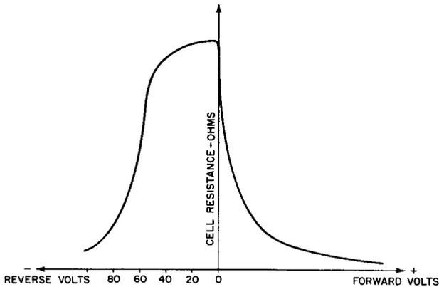
**Fig. 13-3. Reverse Voltage Versus Rectifier Cell Resistance for Selenium Type Cell.**
