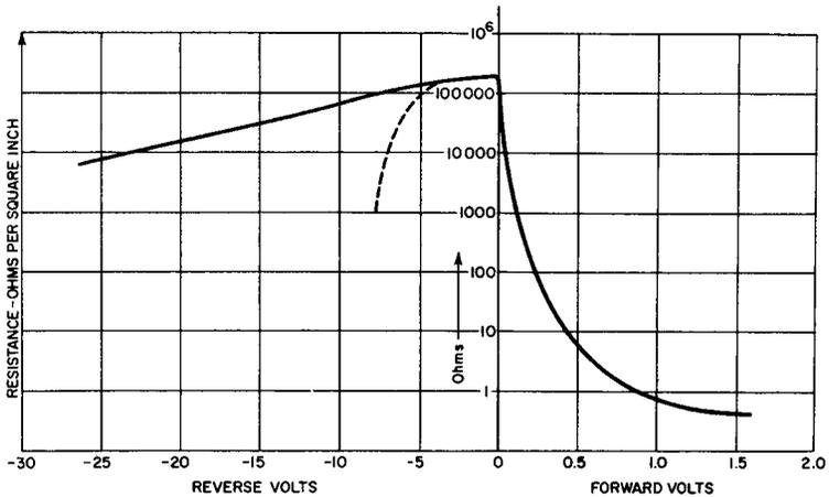
**Fig. 5-16. Static Resistance Curve for Selenium Rectifier Cell.**
