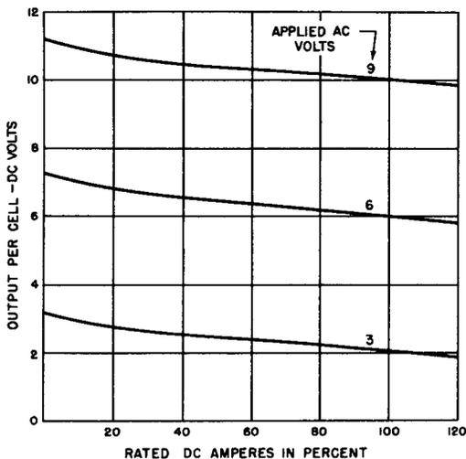
**Fig. 5-21. Voltage Regulation of Three-Phase, Selenium, Bridge-Rectifier on Resistive Load.**
