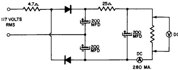
**Fig. 15-11. A Typical Full-Wave, Voltage-Doubler Circuit.**
