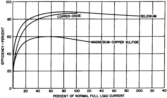
**Fig. 7-5. Efficiency Curves for the Three Types of Rectifiers—Three-Phase Circuit, Resistive Load.**
