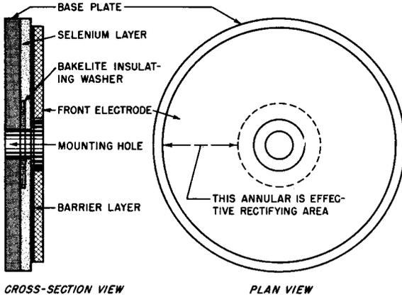
**Fig. 5-3. Cross-Sectional and Plan View of Selenium Rectifier Cell Using Insulating Washer Principle.**
