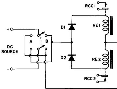
**Fig. 13-5. Duplex Operation from a DC Source.**
