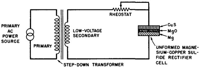
**Fig. 6-2. Electrical Circuit Suitable for Electroforming the Magnesium-Copper Sulfide Discs into a Magnesium-Copper Sulfide Cell.**
