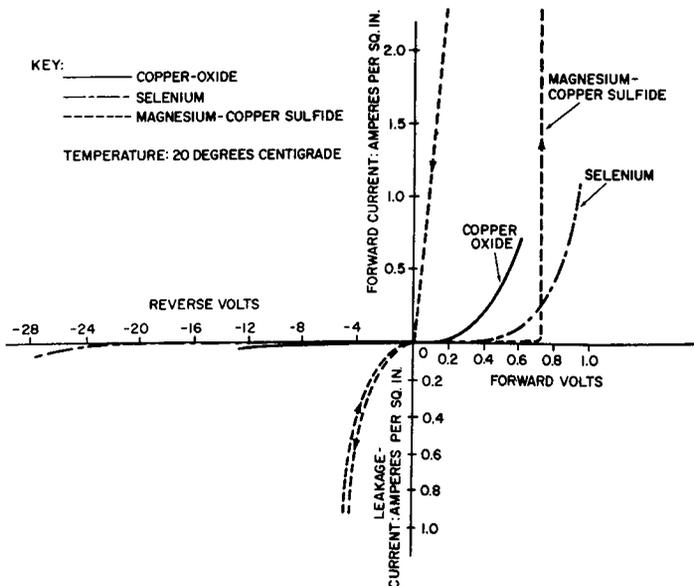
**Fig. 7-1. A Comparison of the Volt-Ampere Characteristics of the Three Types of Rectifiers.**
