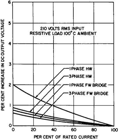
**Fig. 15-3. Typical Regulation Curves for Various Circuits.**
