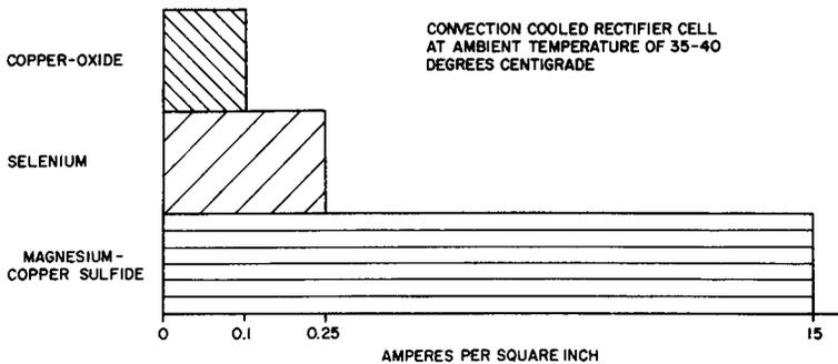
**Fig. 7-4. Comparison of Rectifier Types on Basis of Ampere Per Square Inch Current Flow Permissible.**
