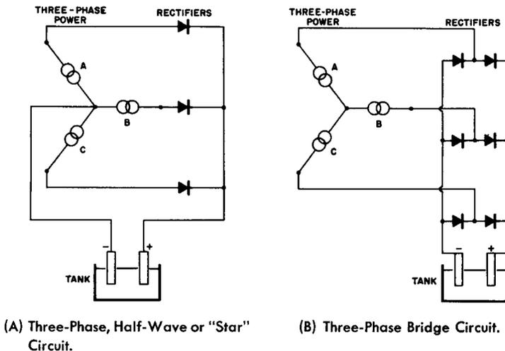
**Fig. 10-11. Three-Phase Electrofinishing Circuits.**
