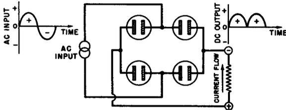
(B) Using Four Cells in a Bridge Circuit.
