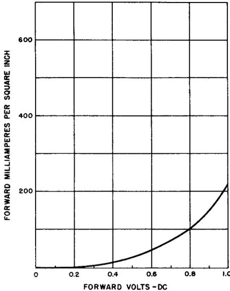
**Fig. 5-25. Static Forward Characteristic of a 26 Volt Selenium Rectifier Cell.**
