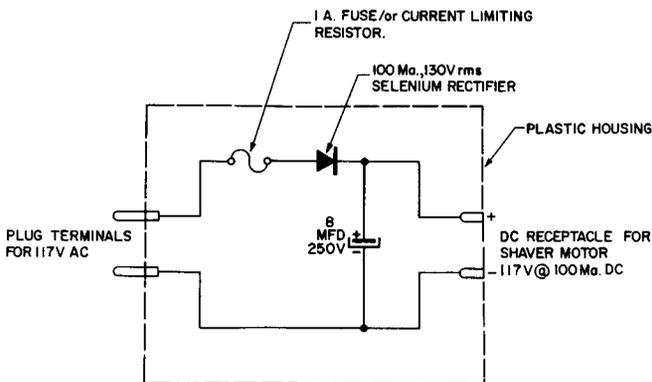
**Fig. 11-2. A Selenium Rectifier Power Converter for Electric Shavers.**
