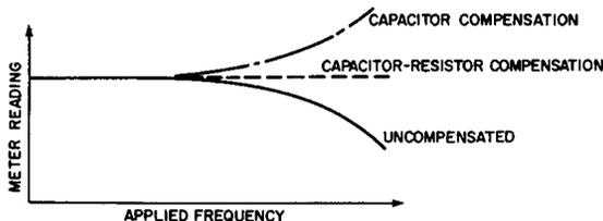
(B) Rectifier-Type Meter Reading Versus Applied Frequency.
