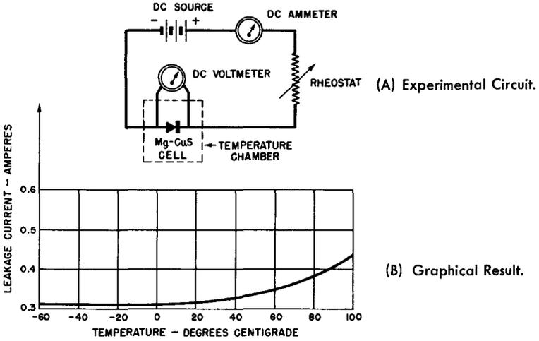
**Fig. 6-12. Reverse Current-Temperature Characteristics of a Magnesium-Copper Sulfide Cell.**
