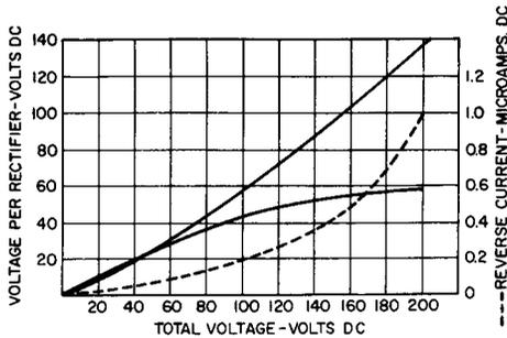
**Fig. 15-6. Inverse Voltage Per Rectifier with Two Sarkes Tarzian "P" Type Silicon Rectifiers Connected in Series.**
