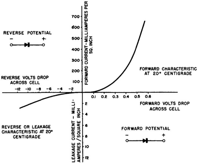
**Fig. 4-8. Volt-Ampere Characteristics of Copper-Oxide Cell at 20° C.**
