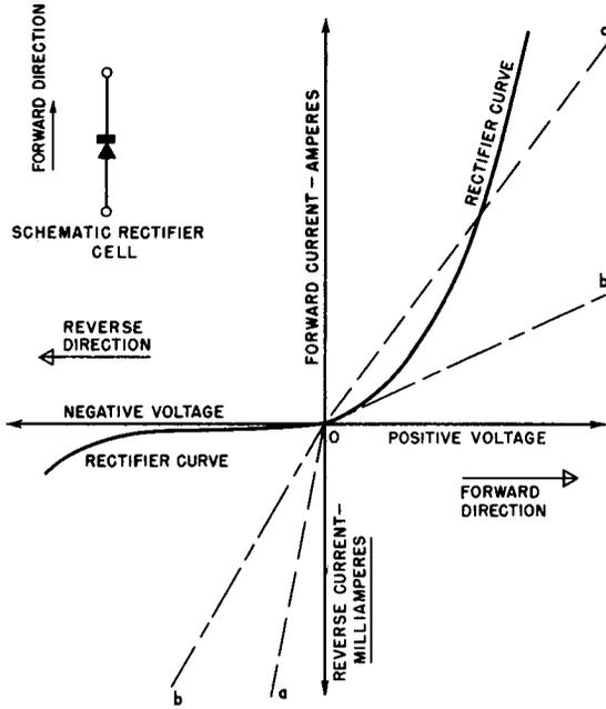
**Fig. 2-6. Volt-Ampere Curve for Generalized Metallic Rectifier Junction.**
