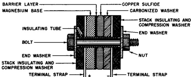
(C) Exaggerated Cutaway View of Half-Wave Rectifier With Rectification Polarity Identified.
