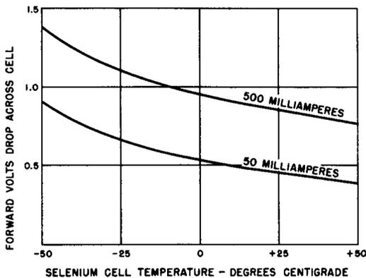
**Fig. 5-14. Temperature Characteristics of the Selenium Rectifier Cell.**
