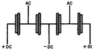
(B) Single-Phase, Full-Wave Bridge Rectifier Without Positive Terminals Strapped Together.
