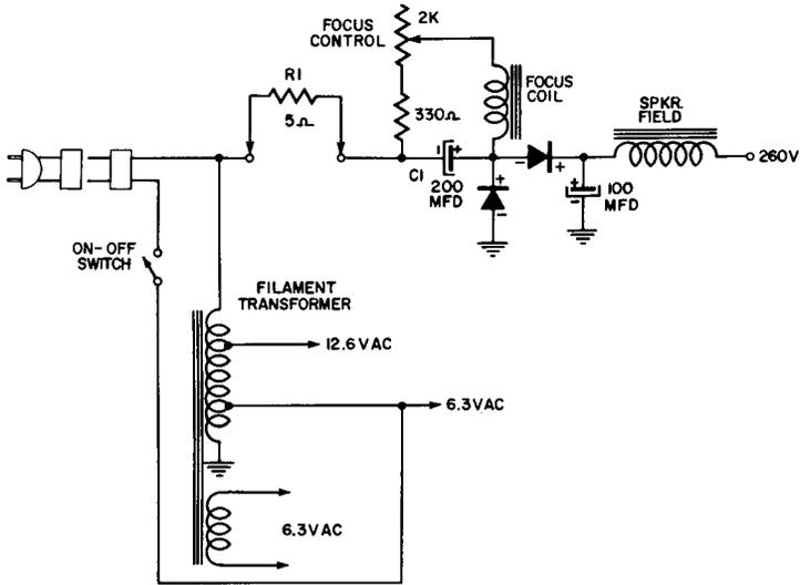
**Fig. 11-7. Half-Wave, Voltage-Doubler Circuit Employing Selenium Rectifiers, Used in Television Power Supplies.**
