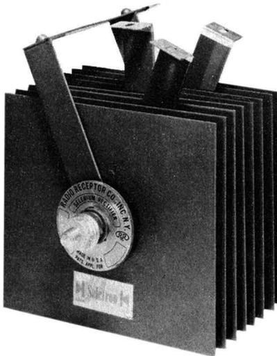
**Fig. 3-4. A Single-Phase Full-Wave Bridge Rectifier. Maximum Input 52 Volts rms. Output 37.8 Volts, 7.5 Amperes, DC. (Courtesy of Seletron Division of Radio Receptor Co., Inc.)**
