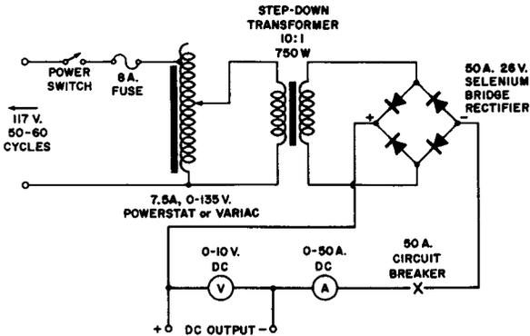
**Fig. 10-6. A Battery Eliminator Circuit With a Variable DC Output Voltage of 0 to 10 Volts, Current Capacity, 50 Amperes.**
