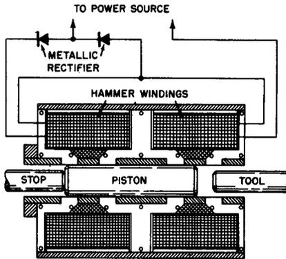
**Fig. 14-8. Cutaway Section of an Electric Hammer Designed for Operation With Metallic Rectifiers.**
