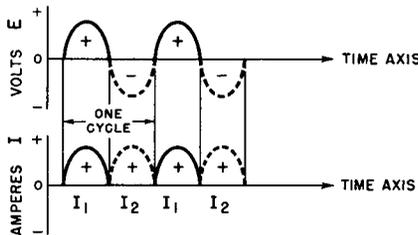
(B) Voltage and Current Waveforms.
