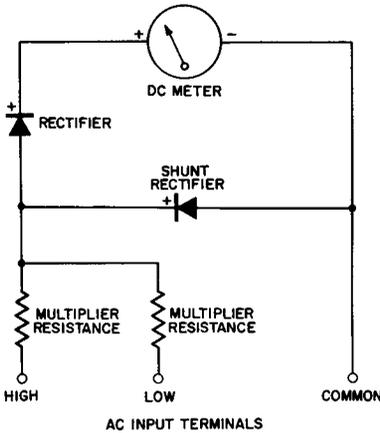
**Fig. 12-8. Half-Wave Rectifier-Type AC Voltmeter with Rectifier Shunt.**
