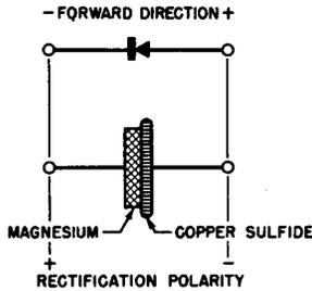
(A) Magnesium-Copper Sulfide Rectifier Cell.
