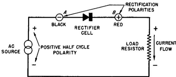
**Fig. 3-8. Current Flow and Rectification Polarity Markings.**
