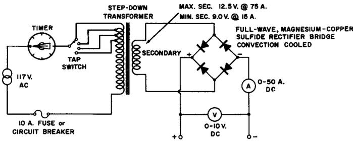
**Fig. 10-7. The Basic Battery Charging Circuit, Low Amperage, Convection Cooling.**
