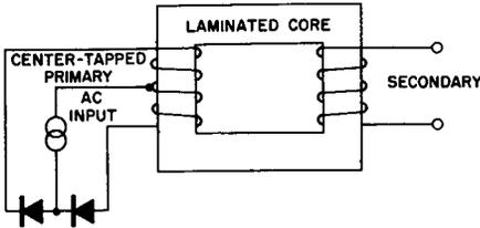
**Fig. 14-5. Frequency Doubler Circuit Using Two Rectifiers and a Center-Tapped Primary.**
