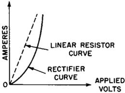
(A) Rectifier and Linear Resistor Curves.
