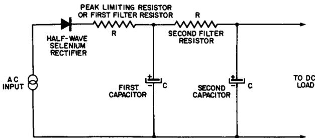
**Fig. 9-6. Adding a Second Stage of R-C Filtering to the Half-Wave Rectifier Circuit.**
