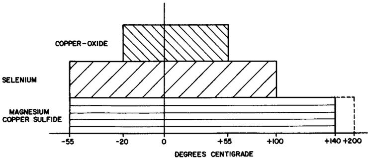
**Fig. 7-6. Operating Temperature Range for the Three Rectifier Types.**
