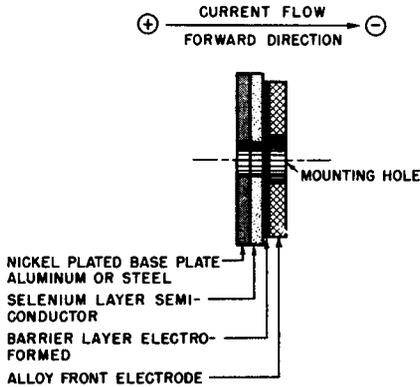
(A) Exaggerated Cross-Sectional View of Selenium Rectifier Cell.
