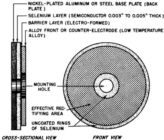
**Fig. 5-1. Front and Cross-Sectional View of the Selenium Rectifier Cell.**
