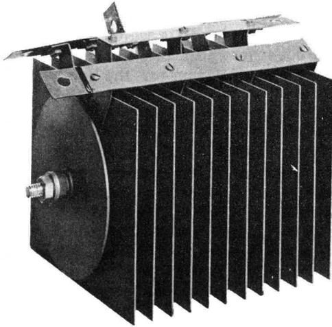
**Fig. 5-10. A Three-Phase Bridge Selenium Rectifier. Fan Cooling, 24 Volts AC Input, 60 Amperes DC Output. (Courtesy of Seletron Division of Radio Receptor Co., Inc.)**
