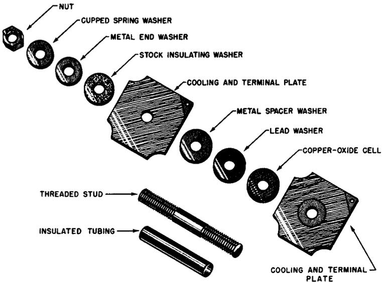
**Fig. 3-2. Elements of a Copper-Oxide Rectifier Stack Assembly.**
