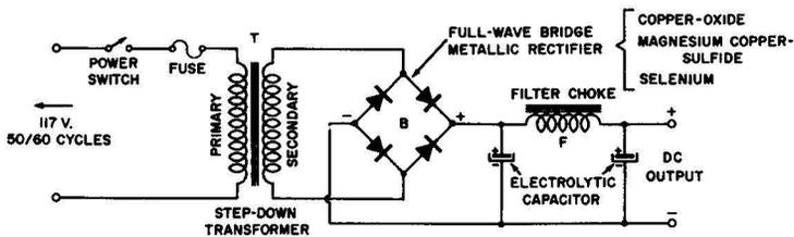
**Fig. 10-5. A Storage Battery Eliminator Circuit.**
