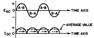
(B) Voltage and Current Waveforms
