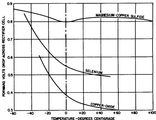
**Fig. 7-2. Forward Voltage-Temperature Characteristics of Rectifier Types.**
