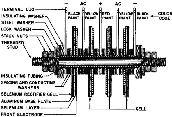
**Fig. 5-7. Selenium Rectifier Stack Construction. Full-Wave Bridge, One Cell per Arm. Cells are of the Insulating Washer Type.**
