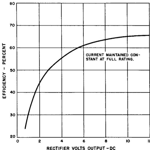
**Fig. 5-23. The Efficiency of a Single-Phase Selenium Rectifier is a function of Output Voltage and Current.**
