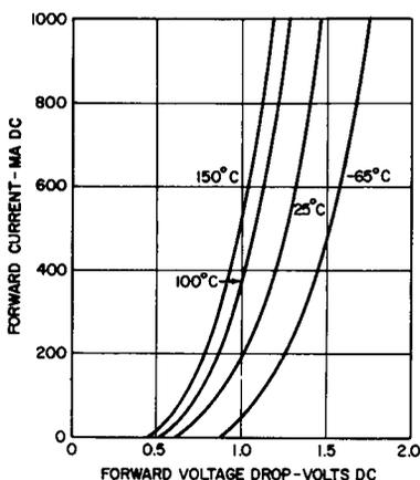
Fig. 15-2. Static Forward Current Vs. Applied Voltage.
