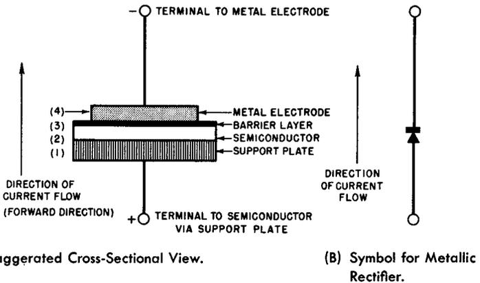
**Fig. 2-1. The Generalized Metallic Rectifier Element.**
