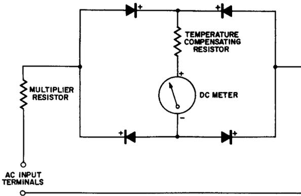
**Fig. 12-17. Compensating Resistor in Series With Meter for Temperature Effects.**
