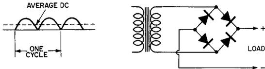
**Fig. 15-8. Single-Phase, Full-Wave Bridge Type Circuit.**
