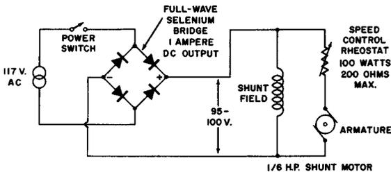
**Fig. 10-14. A Simple Variable-Speed Drive Circuit.**
