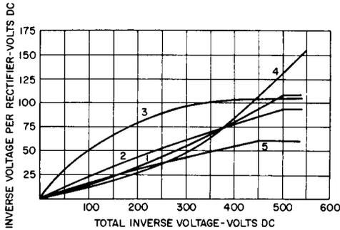
**Fig. 15-5. Inverse Voltage Per Rectifier with Five Sarkes Tarzian "P" Type Silicon Rectifiers Connected in Series.**
