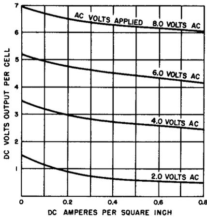
**Fig. 4-14. Voltage Regulation for a Single-Phase, Full-Wave Bridge, Copper-Oxide Rectifier Supplying a Resistive Load.**
