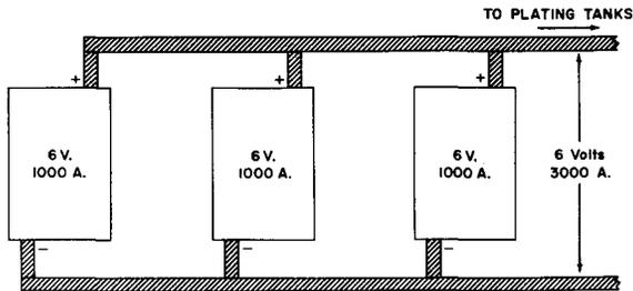
**Fig. 10-12. Method of Paralleling Rectifiers for Greater Current Capacity.**
