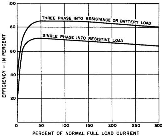
**Fig. 5-22. Typical Efficiency Curves of a 26 Volt Selenium Rectifier Cell Operating at Full Voltage.**
