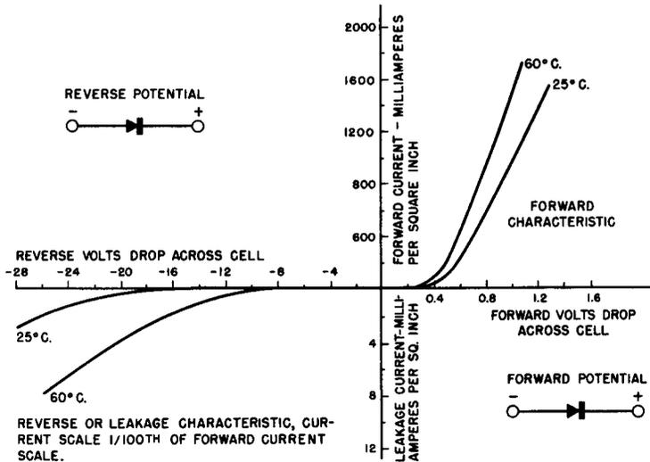
**Fig. 5-13. Effect of Temperature on the Volt-Ampere Characteristic of a Selenium Rectifier Cell.**
