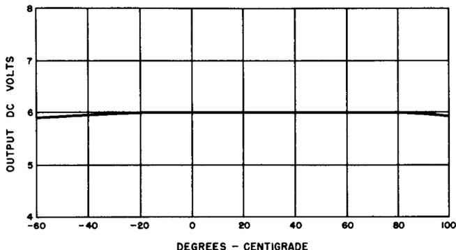
**Fig. 6-14. DC Output Voltage of Single-Phase, Full-Wave, Magnesium-Copper Sulfide Bridge Rectifier Versus Temperature.**
