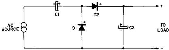
(A) Half-Wave Voltage-Doubler Circuit
