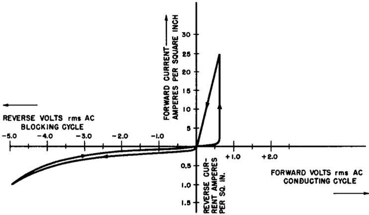
**Fig. 6-9. Dynamic Volt-Ampere Characteristics of a Typical Magnesium-Copper Sulfide Rectifier Cell.**
