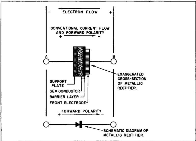
**Fig. 3-6. Nomenclature and Forward Polarity of a Half-Wave Rectifier.**
