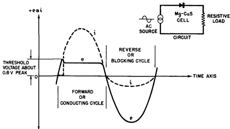
**Fig. 6-10. Applied Voltage and Resulting Current Versus Time as Seen on an Oscilloscope for a Magnesium-Copper Sulfide Rectifier Cell.**
