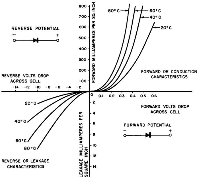
**Fig. 4-9. Volt-Ampere Characteristics of Copper-Oxide Cell Versus Temperature.**
