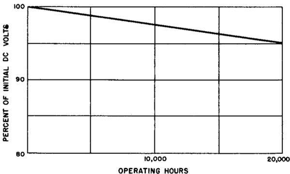
**Fig. 5-24. Aging Characteristics of Selenium Rectifiers.**
