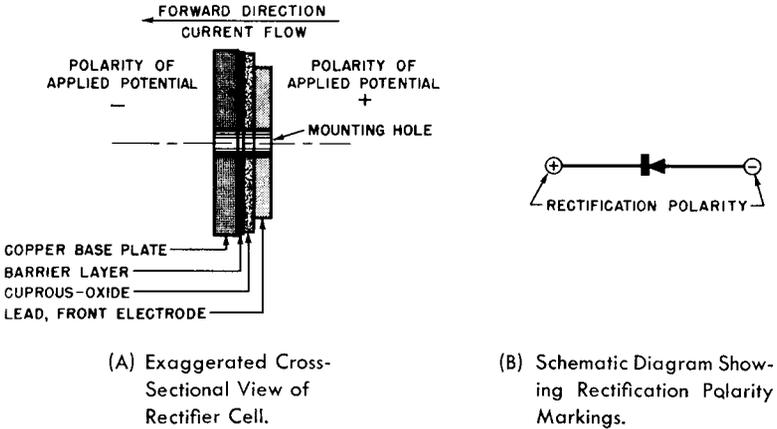
(A) Exaggerated Cross-Sectional View of Rectifier Cell.
