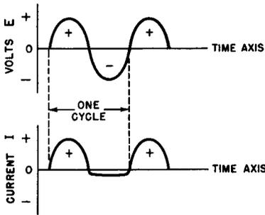
(B) Voltage and Current Waveforms.
