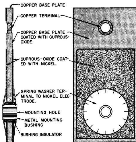
**Fig. 4-3. Plan and Exaggerated Cross-Sectional View of Plate Type Copper-Oxide Rectifier Cell With the Oxide Coating on Both Sides.**
