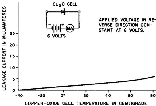
**Fig. 4-11. Temperature Characteristics of Copper-Oxide Cell in Blocking Direction.**
