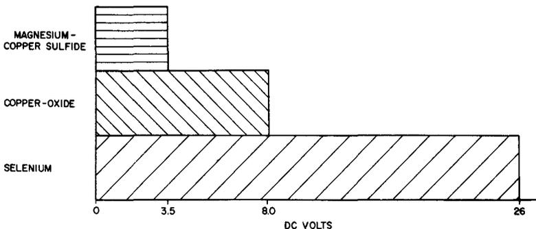
**Fig. 7-3. Selection Chart on Basis of Expected DC Volts Required.**
