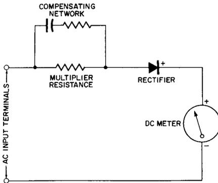
(B) Capacitor-Resistor Compensation.
