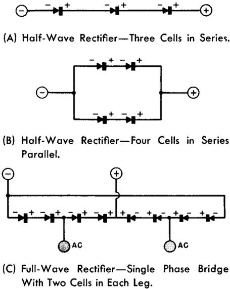
**Fig. 3-14. Series Parallel Arrangements of Rectifier Cells.**
