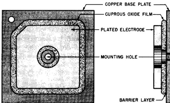
**Fig. 4-2. Plan and Exaggerated Cross-Sectional View of Plate Type Copper-Oxide Rectifier Cell.**
