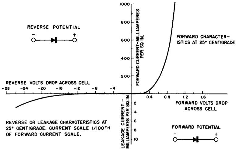
**Fig. 5-12. Volt-Ampere Characteristic of a Selenium Rectifier Cell at 25 degrees Centigrade.**
