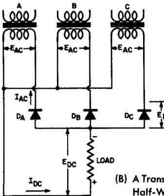
(B) A Transformer-Coupled, Three-Phase, Half-Wave Rectifier Circuit.
