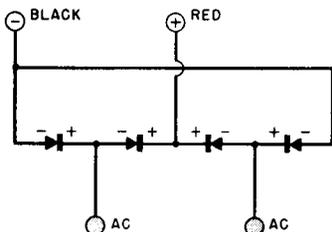
(B) A Single-Phase, Full-Wave, Rectifier Bridge Using Four Cells in a Stack Assembly With the Outer Cells Negative and Strapped Together.
