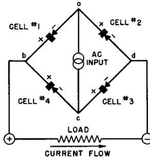
(A) Correct Method of Wiring Four Rectifier Cells for Single-Phase, Full-Wave, Bridge Rectification.
