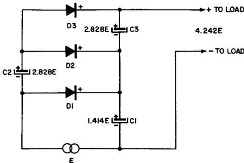
**Fig. 9-20. The Ladder Voltage Multiplier Circuit.**
