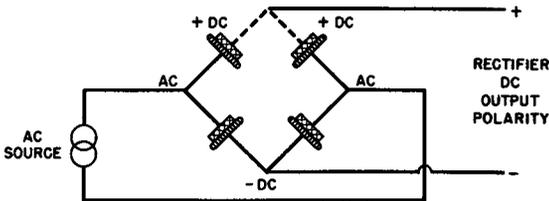
(C) Single-Phase, Full-Wave, Bridge Rectifier With Positive Terminals Strapped Together by Dotted Line.
