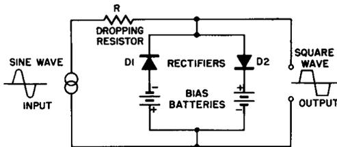
**Fig. 13-8. Square Wave or Clipping Circuit Using Metallic Rectifiers.**
