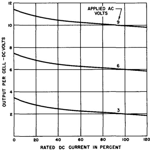
**Fig. 5-20. Voltage Regulation of Single-Phase, Selenium, Bridge-Rectifier on Battery Load.**
