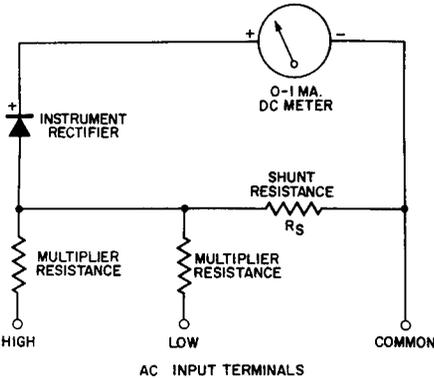
**Fig. 12-7. Rectifier-Type AC Voltmeter Using Resistive Shunt.**
