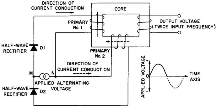
**Fig. 14-3. A Frequency Doubler Circuit Using Two Primaries and Two Rectifiers.**
