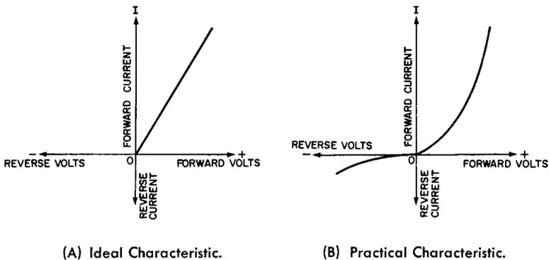
**Fig. 12-3. Characteristics of Theoretical and Practical Instrument Rectifiers.**
