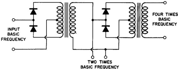
**Fig. 14-6. A Frequency Quadrupler Circuit.**
