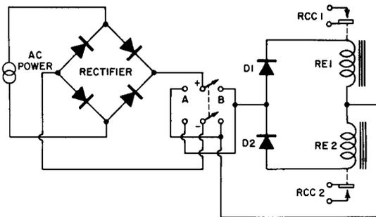
**Fig. 13-6. Duplex Operation from an AC Source.**
