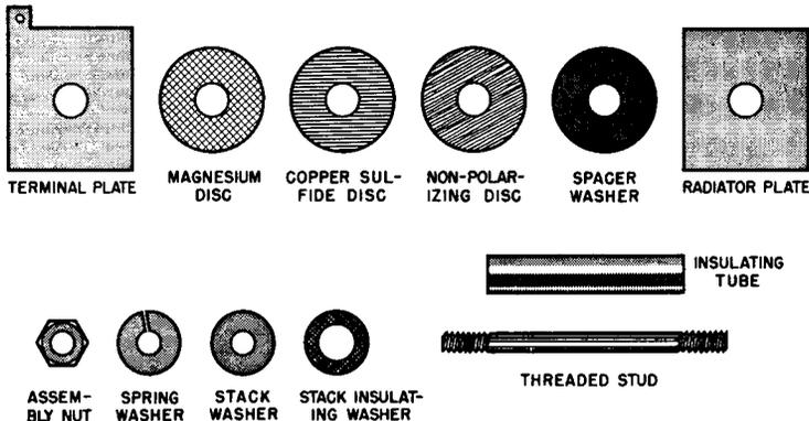
**Fig. 6-5. Elements of the Magnesium-Copper Sulfide Rectifier Stack.**
