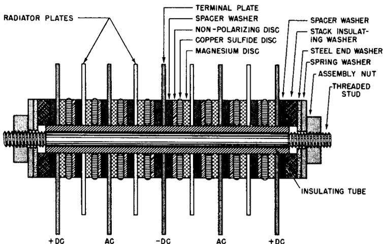
**Fig. 6-6. Cutaway View of a Magnesium-Copper Sulfide Bridge Rectifier, Single-Phase, Full-Wave.**
