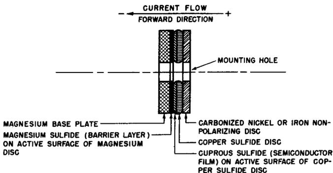
(A) Exaggerated Cross-Sectional View of Rectifier Cell.
