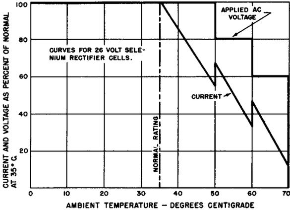
**Fig. 5-26. Current and Voltage Derating Curves to Maintain Constant Operating Temperature for Ambients above 35 Degrees Centigrade.**
