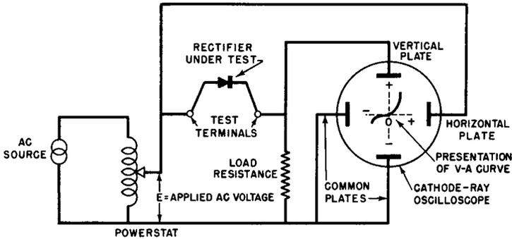
**Fig. 2-7. Circuit for Testing Dynamic Volt-Ampere Properties of Metallic Rectifier Cells.**
