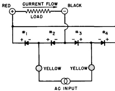
(B) Schematic of the Same Full-Wave Bridge Rectifier as Arranged in a Commercial Stack.
