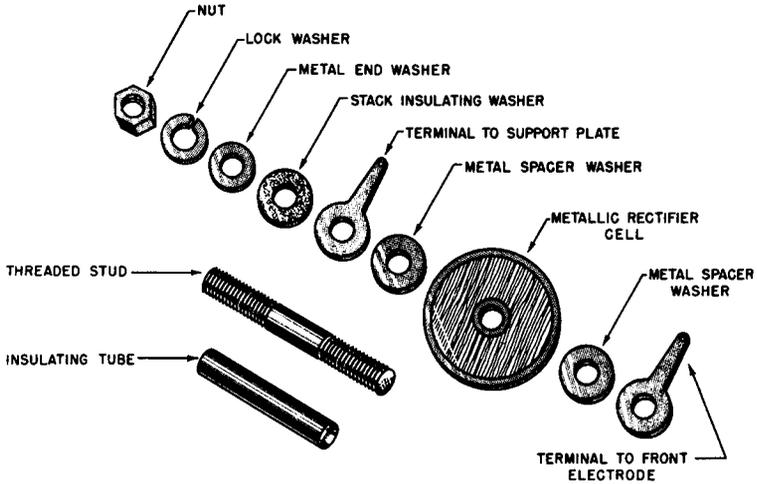
**Fig. 3-1. Elements of a Selenium Rectifier Stack Assembly.**
