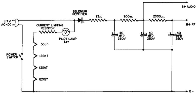
**Fig. 11-6. An AC-DC Radio Power Supply Using Selenium Rectifiers.**
