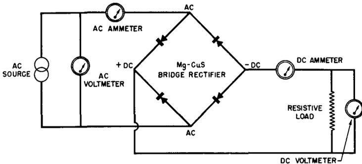
**Fig. 6-13. Experimental Setup for Single-Phase, Full-Wave, Magnesium-Copper Sulfide Bridge Rectifier.**
