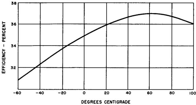
**Fig. 6-15. Efficiency Versus Temperature for a Single-Phase, Full-Wave, Magnesium-Copper Sulfide Bridge Rectifier Feeding A Resistive Load.**
