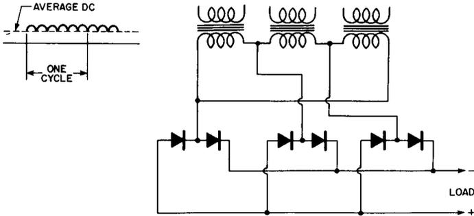
**Fig. 15-10. Three-Phase, Full-Wave Bridge Type Circuit.**
