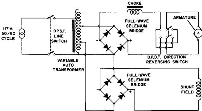
**Fig. 10-13. A Speed Control Circuit for a DC Motor Fed From an AC Source.**
