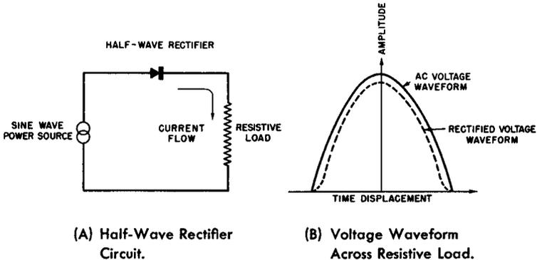
**Fig. 5-17. Waveform Distortion Due to Resistance Change of Selenium Rectifier Cell.**
