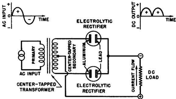
(A) Using Two Cells and a Center-Tapped Transformer.
