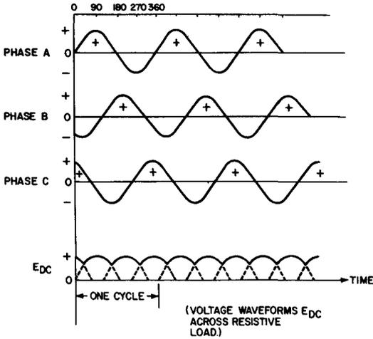
**Fig. 9-22. Waveform Graphs for Three-Phase, Half-Wave, Rectifier Circuit.**
