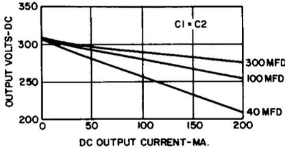
(B) Voltage Regulation Curves for Different Values of Capacitors.
