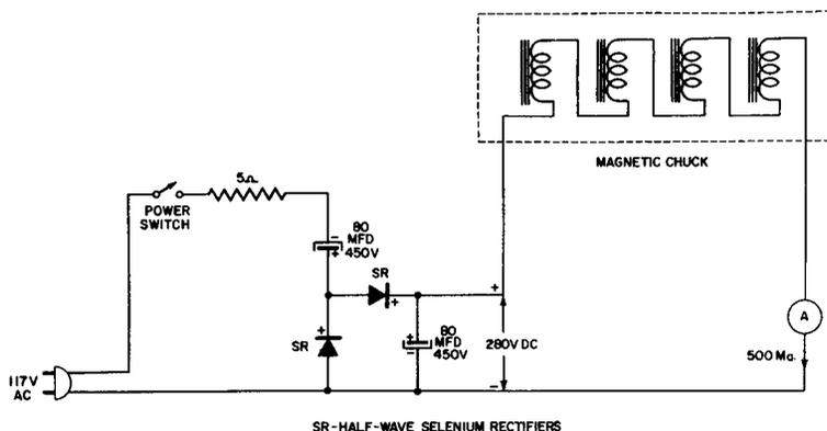
**Fig. 11-5. Selenium Rectifier Power Supply for a Magnetic Chuck.**
