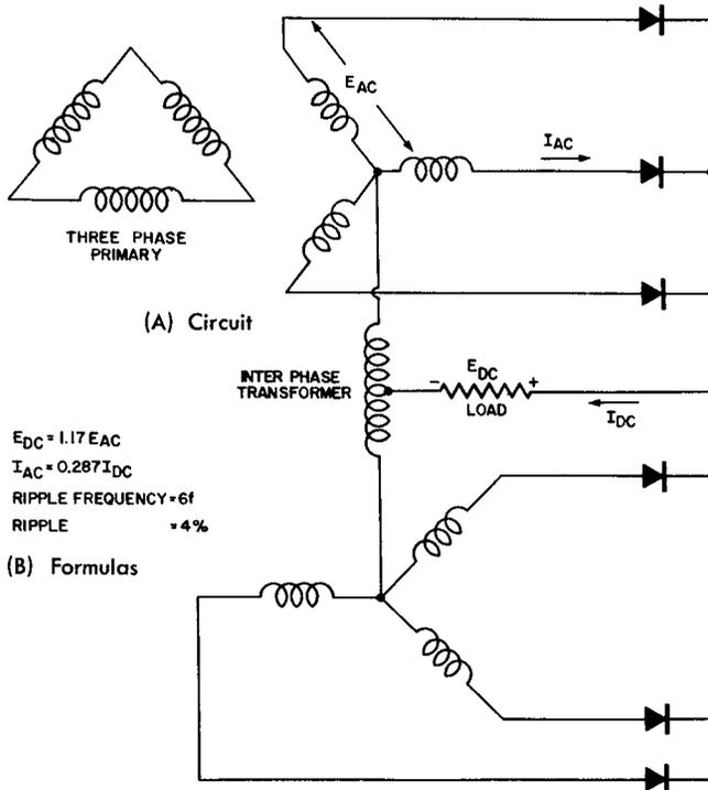
**Fig. 9-25. A Three-Phase, Full-Wave, Rectifier Circuit With Inter-Phase Transformer.**
