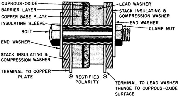
(C) Exaggerated Cross-Sectional View of Stack Assembly of Half-Wave Rectifier.
