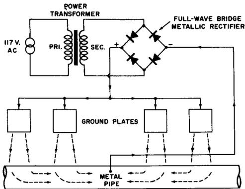
**Fig. 10-16. Cathodic Protection of Buried Metal Pipe.**
