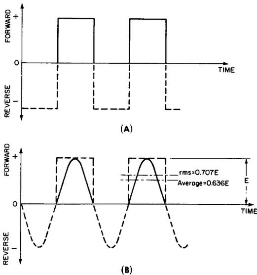
**Fig. 12-6. Rectangular and Sine Waveforms.**
