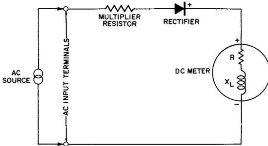
**Fig. 12-15. Simplified Equivalent of DC Meter Coil at High Frequencies.**
