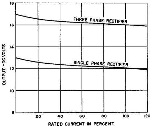
**Fig. 5-18. Voltage Regulation Curves for Selenium Rectifier Cell for Single- and Three-Phase Circuit Feeding Resistive Load.**
