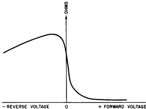
**Fig. 4-12. Voltage-Resistance Graph for Copper-Oxide Rectifier Cell.**
