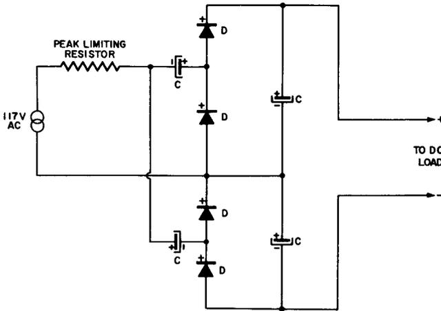
**Fig. 9-19. Another Voltage-Quadrupling Scheme.**
