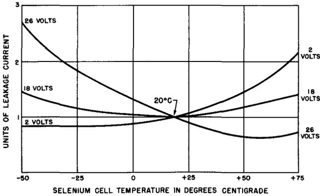
**Fig. 5-15. Leakage Current versus Cell Temperature for Rated and Reduced Applied Voltages.**
