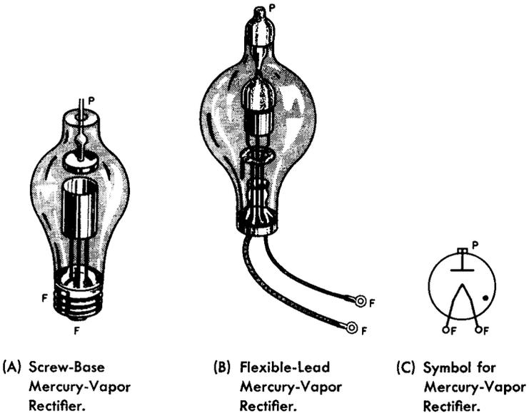
**Fig. 1-5. Small Mercury-Vapor Rectifiers Rated at 10 to 15 Amperes.**
