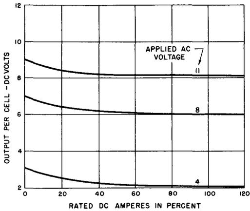
**Fig. 5-19. Voltage Regulation of Single-Phase, Selenium, Bridge-Rectifier on Resistive Load.**
