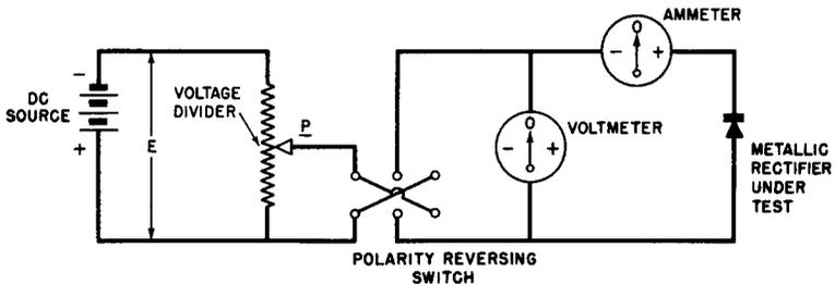
**Fig. 2-5. Test Circuit for Rectifier Junction.**
