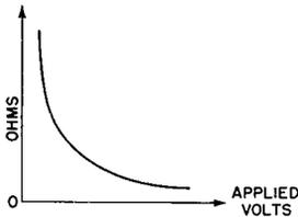
(B) Forward Resistance of a Rectifier.
