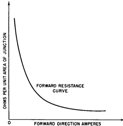
**Fig. 2-9. Forward Resistance Versus Forward Current for Generalized Rectifier.**
