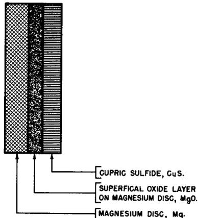
To electroform the magnesium-copper sulfide cell, the magnesium and the cupric sulfide electrodes are placed together, either as cells in special forming fixtures or in the ultimate rectifier stack. Fig. 6-1 shows in cross-sectional
