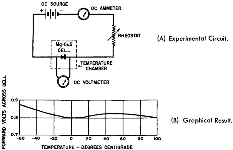
**Fig. 6-11. Voltage-Temperature Characteristics of a Magnesium-Copper Sulfide Cell.**
