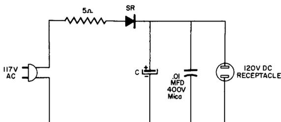
SELECT SELENIUM RECTIFIER SR WITH ADEQUATE CURRENT RATING FOR DESIRED CURRENT OUTPUT.
