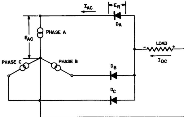
(A) A Three-Phase, Half-Wave, Rectifier Circuit Connected Direct to Y Connected Source.
