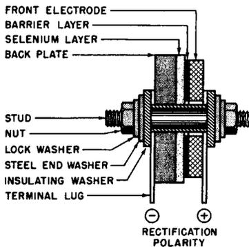
(C) Exaggerated Cross-Sectional View of Half-Wave Selenium Rectifier.
