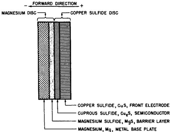
**Fig. 6-3. Exaggerated Cross-Sectional View of Magnesium-Copper Sulfide Cell After Electroforming Operation.**
