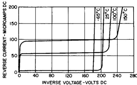
**Fig. 15-4. Static Reverse Isothermal Curves for Sarkes Tarzian Type 15N1 Silicon Rectifier.**
