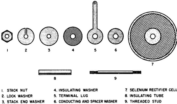
**Fig. 5-6. The Elements of a Selenium Rectifier Stack Using the Insulating Washer Type Cell.**
