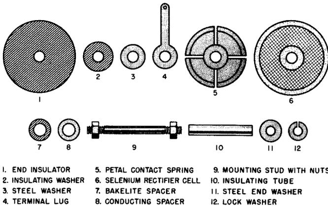
**Fig. 5-4. The Elements of a Selenium Rectifier Stack Using the Contact Type Cell.**
