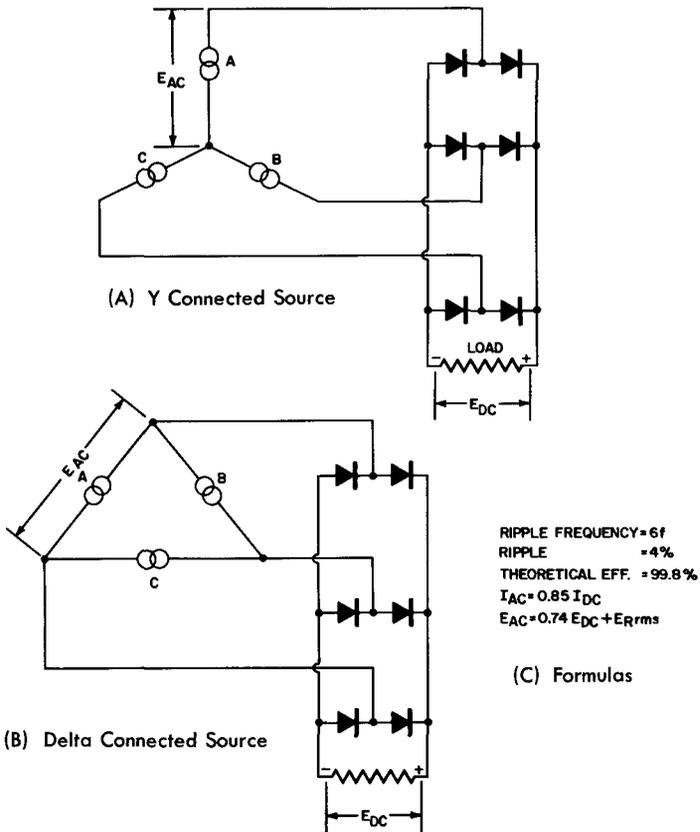
**Fig. 9-24. The Three-Phase, Full-Wave Bridge Rectifier.**
