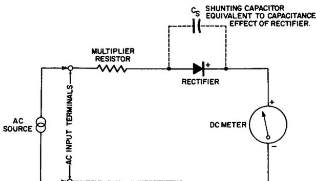
**Fig. 12-14. Equivalent Circuit Illustrating Capacitance of Rectifier at Higher Frequencies.**
