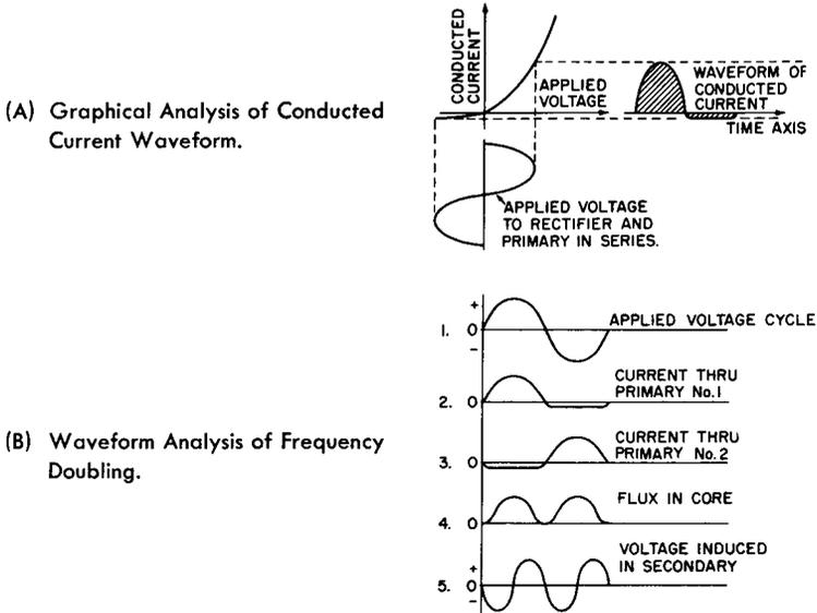
**Fig. 14-4. Analysis of Frequency Doubler Circuit.**
