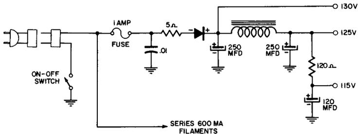
**Fig. 11-8. Conventional Half-Wave Rectifier System Using Selenium Rectifiers.**
