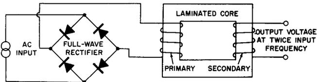
**Fig. 14-7. A Frequency Doubler Circuit Using Full-Wave Rectifiers.**
