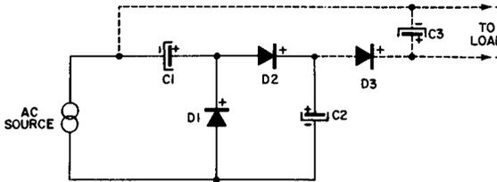
(B) Voltage-Tripler Circuit
