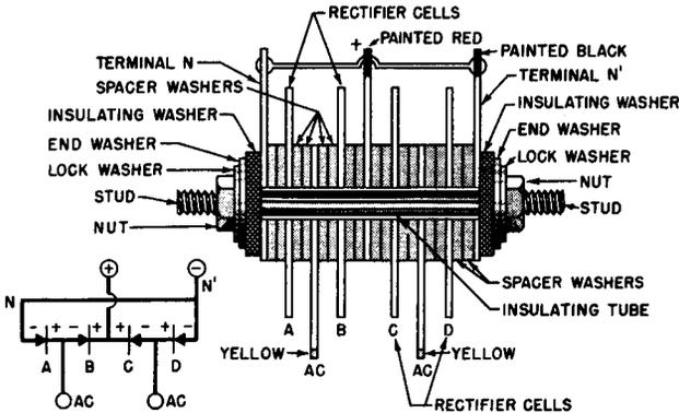
schematic diagram of the rectifier stack shown in the photograph of Fig. 3-4.
