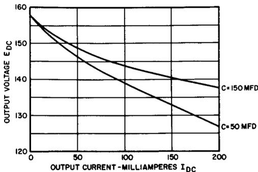
**Fig. 9-5. Circuit and Voltage Regulation Curves for Half-Wave Rectifier Circuit, With Capacitor.**
