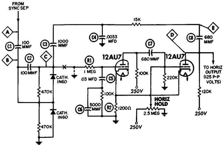
Fig. 4-4. Freewheeling test is made in this circuit by breaking the lead at X and grounding the 1-meg resistor.
