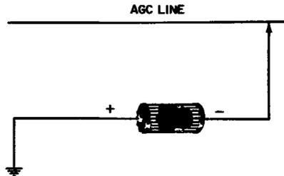
Fig. 10-1. Battery bias clamps the AGC line.
