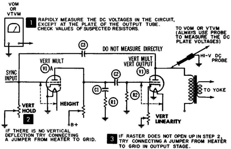
(A) Preliminary tests in the vertical circuitry.
