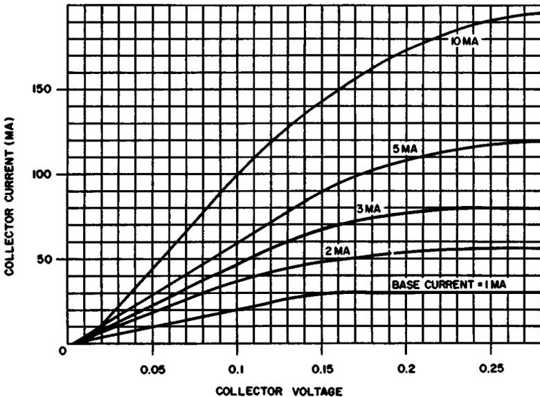
Fig. 10-8. Typical collector saturation characteristics.
