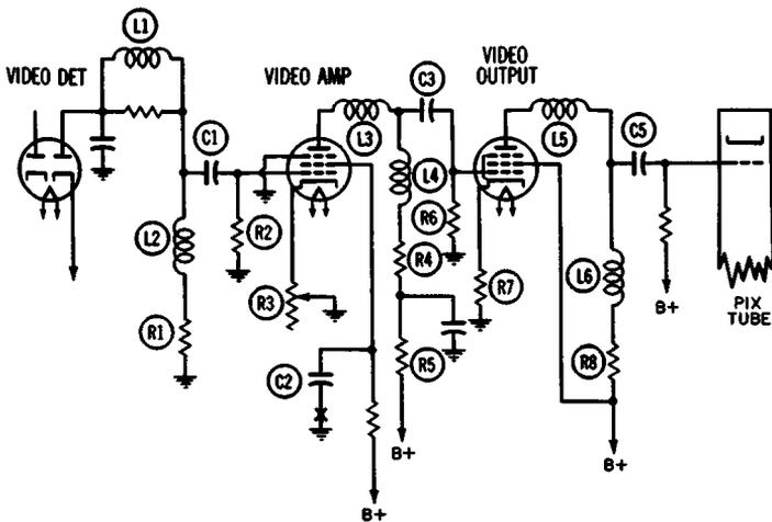
Fig. 2-21. Video-amplifier circuit.
