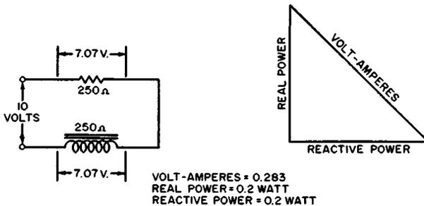
Fig. 1-13. Relationship of real and reactive power to volt-amperes.
