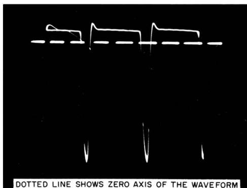
Fig. 3-5. The positive- and negative-peak voltages of stripped sync are widely different.
