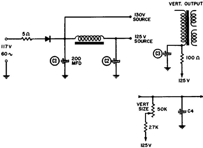
Fig. 8-6. Capacitors C2 and C4 are part of the filter system.
