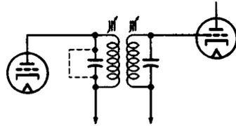
it for a short circuit. Other IF strips also utilize damping resistors in shunt with IF-coil windings, as depicted in Fig. 2-11. In case the coil is open, the DC voltage measures correctly at the grid terminal, but the signal is stopped. Since a typical value for a damping resistor is 82 K, an ohmmeter check will disclose the defect without any circuit disconnections.
