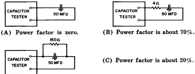
Fig. 8-3. Effect of series and shunt resistance on the power factor of a capacitor.
