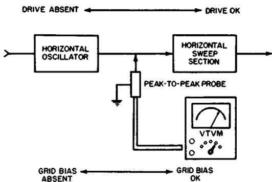
(A) Measurement of peak-to-peak voltage.
