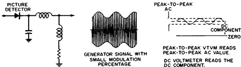
Fig. 2-18. Detector-output-envelope voltage is less than the DC component.
