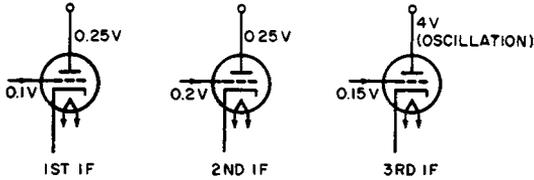
Fig. 2-8. Typical series of IF-voltage measurements.
