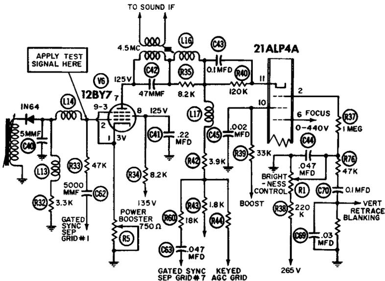
Fig. 7-2. Applying the intercarrier-test signal at the grid—not at the plate.
