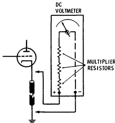
Fig. 10-6. Open cathode resistor causes B+ to appear on cathode.
