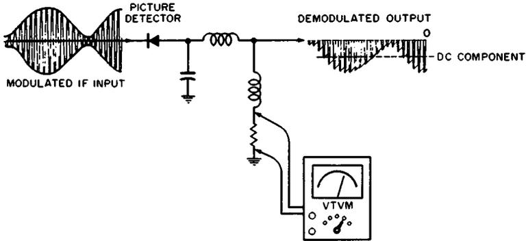
Fig. 2-17. Metering the DC component at the picture-detector output.
