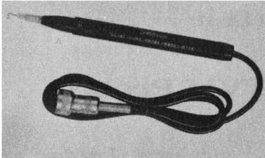
Fig. 11-2. Typical AC-DC probe for a VTVM.
