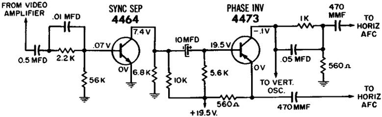
Fig. 3-12. Typical transistorized sync-section of a TV receiver.
