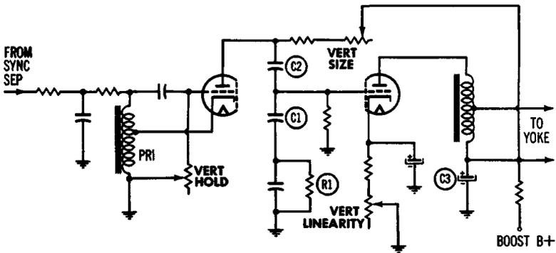
Fig. 6-4. Vertical oscillator and output configuration.
