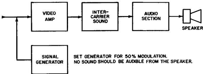
Fig. 7-4. AM rejection test.
