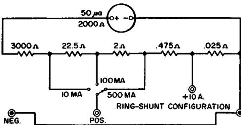
(C) The 10-amp input is brought out to a separate jack to avoid switch-contact resistance.
