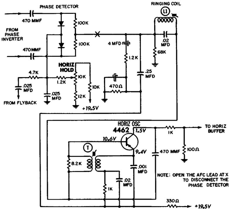
Fig. 4-9. Typical semiconductor AFC and horizontal-oscillator circuit.
