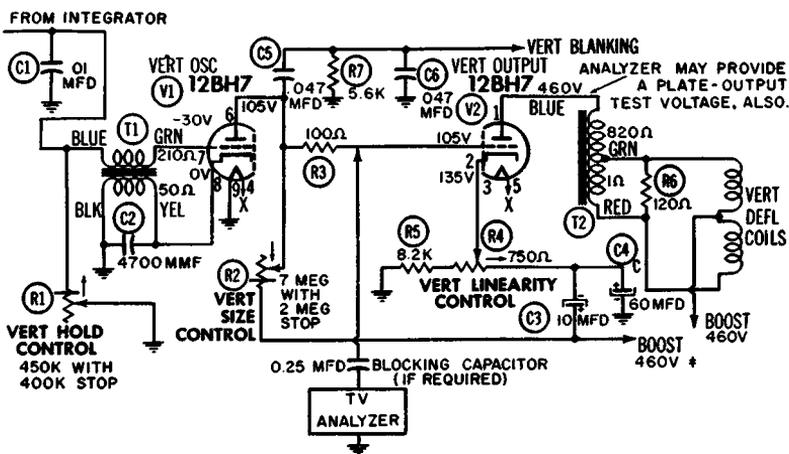
Fig. 6-5. Vertical-drive voltage can be applied from a TV analyzer.
