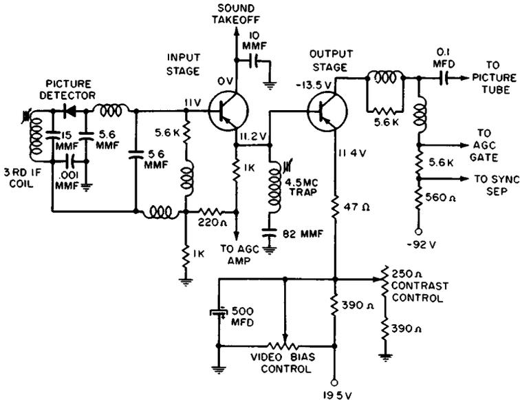
Fig. 2-23. Typical transistorized-video amplifier.
