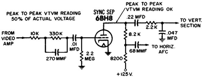
Fig. 3-6. Grid circuit is heavily loaded by peak-to-peak probe—plate circuit is not.
