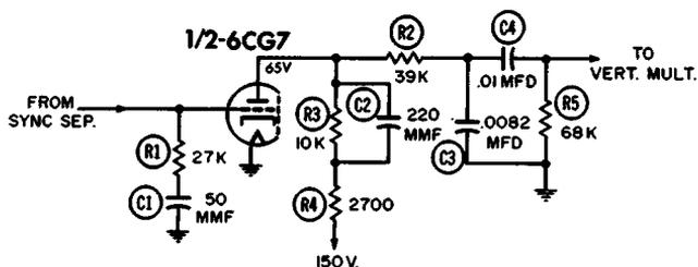
Fig. 3-7. Leakage in C3 or C4 can cause poor vertical-sync locking.
