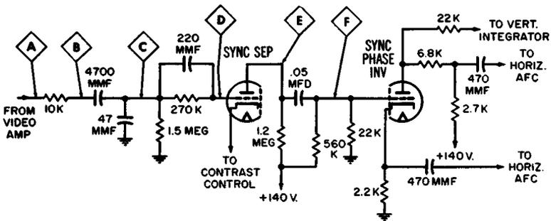
Fig. 3-11. Sync-separator and phase-inverter circuit.
