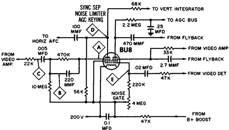
Fig. 3-9. Noise limiter and sync separator are in left-hand section of the tube; keyed AGC is in right.
