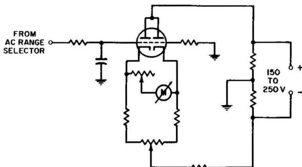
Fig. 11-5. Typical metering measuring circuit.
