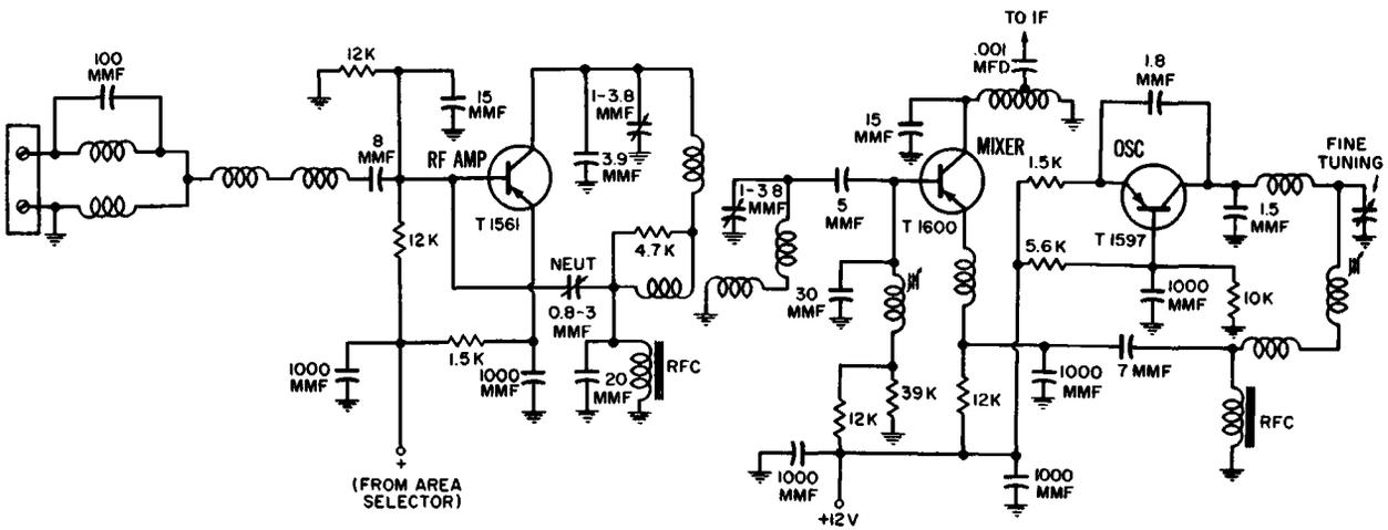
Fig. 2-7. Typical transistorized front-end.
