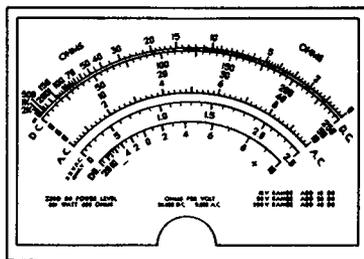
The decibel scale is also highly nonlinear. This is not the consequence of instrument circuitry, but is due to the logarithmic nature of the decibel value. This consideration, as well as the meaning and use of positive and negative db values, are explained in detail. The low AC-voltage scale is appreciably nonlinear toward the zero region, while the high AC scale is less nonlinear. The nonlinearity is a result of the instrument-rectifier characteristics.
