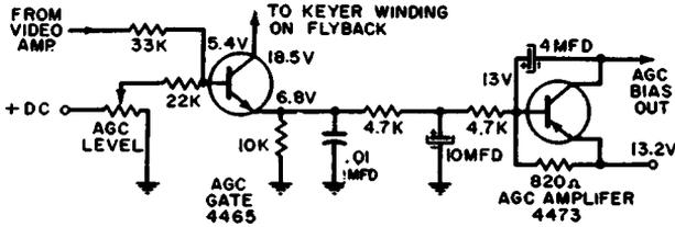
Fig. 10-7. Transistorized gated-AGC circuit.
