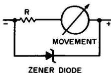
Fig. 1-7. A zener diode protects the meter movement from overload damage.
