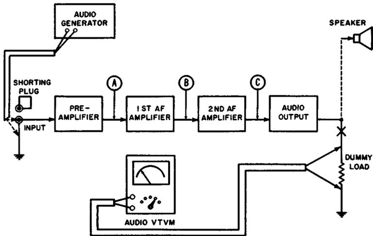
Fig. 9-4. Localizing a noisy amplifier stage.
