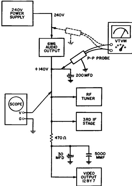
Fig. 8-4. Checking ripple voltage at both plate and cathode of the audio-output tube.
