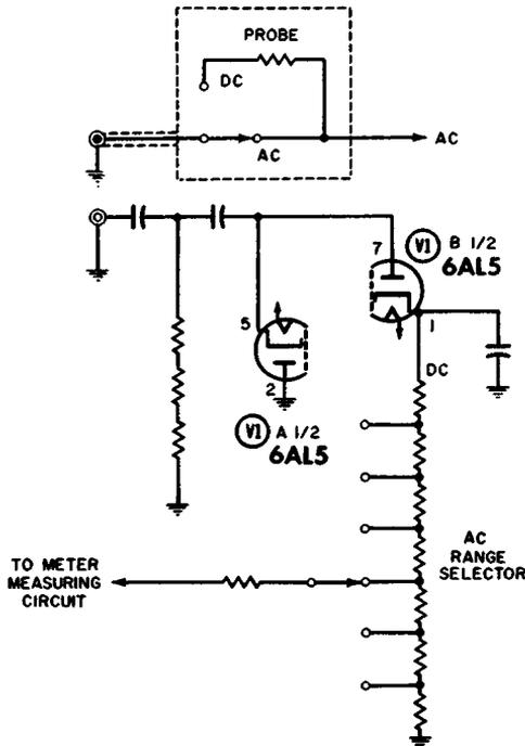
Fig. 11-4. Conversion circuit of AC-DC probe.
