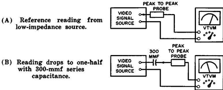
Fig. 3-4. Source reactance reduces voltage indication.
