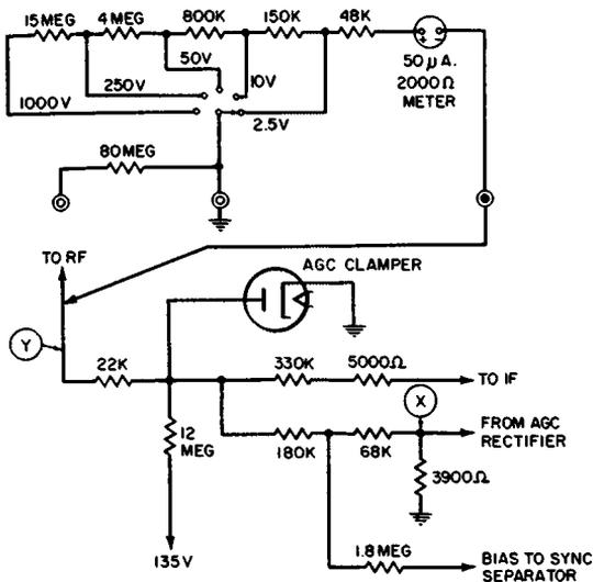
Fig. 10-2. Measuring AGC voltage.
