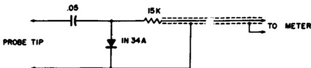
Fig. 5-8. Half-wave signal-tracing probe for VOM.
