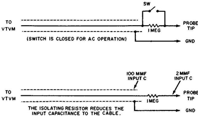
Fig. 11-3. Circuit of AC-DC probe for VTVM.
