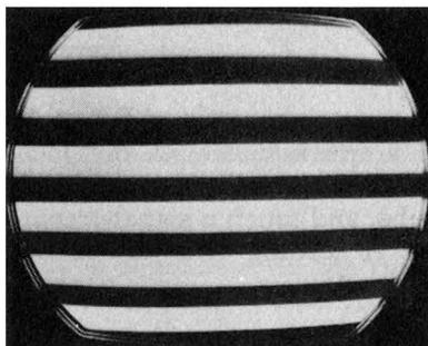
Fig. 2-4. Bar display produced by an AM generator.
