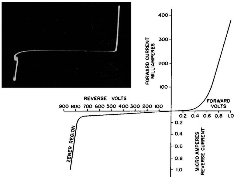
Fig. 1-6. Characteristic of a typical silicon-junction diode.
