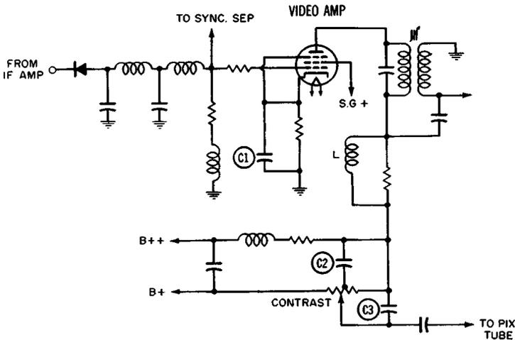
Fig. 2-22. Frequency response being partially controlled by C1, C2, and C3.
