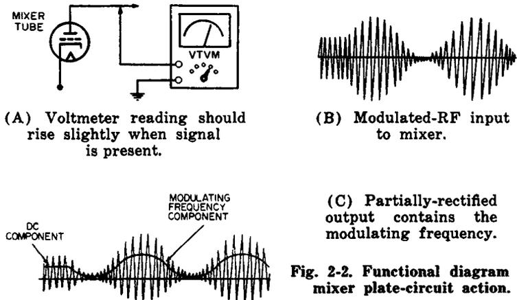
Fig. 2-2. Functional diagram of mixer plate-circuit action.
