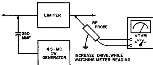
Fig. 7-3. Limiter saturation test.
