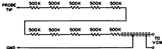
Fig. 5-11. A high-voltage DC probe for use with a VOM.
