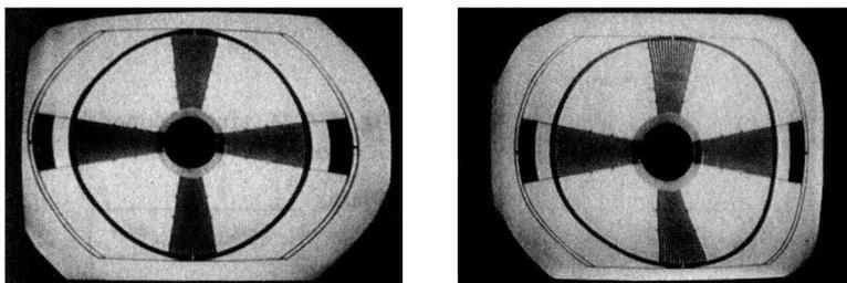
Fig. 5-3. Examples of horizontal nonlinearity.
