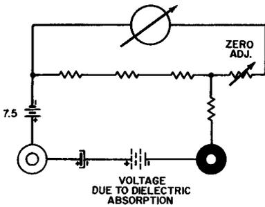
Fig. 8-2. Dielectric-absorption voltage adding to the ohmmeter battery voltage.
