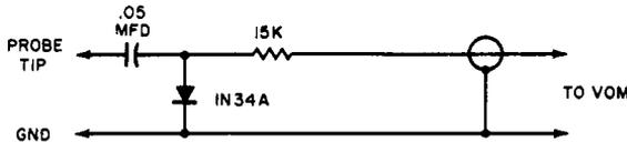
Fig. 11-8. Signal-tracing probe for a VOM.
