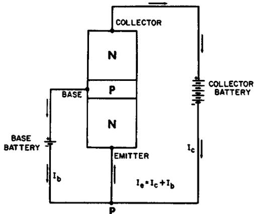
Fig. 2-25. Current in the emitter is the sum of the currents in the base and collector.
