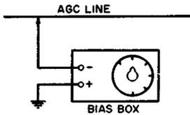
Fig. 3-2. Applying over-ride bias to the AGC line.
