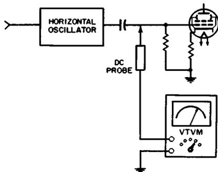
(B) Measurement of signal-developed bias.
