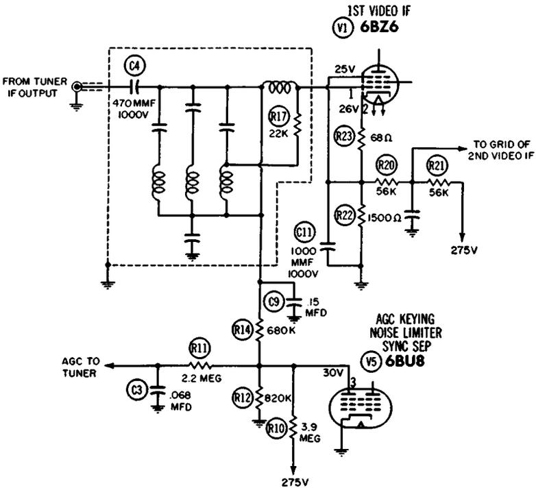
Fig. 10-5. AGC and 1st-IF amplifier circuitry.
