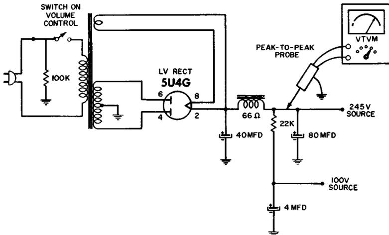
Fig. 8-1. Measurement of ripple voltage.
