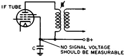
Fig. 2-13. Decoupling capacitor can cause stage oscillation if open.
