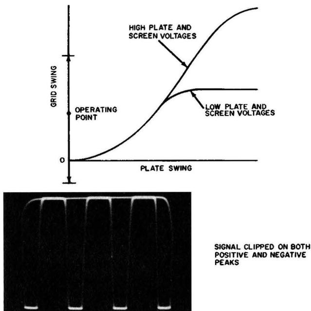
Fig. 7-5. Principle of limiter operation.
