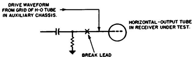
Fig. 5-9. Substitution of drive signal from auxiliary chassis.
