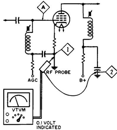
Fig. 2-16. Grounds 1 and 2 are at different 40-mc potentials.
