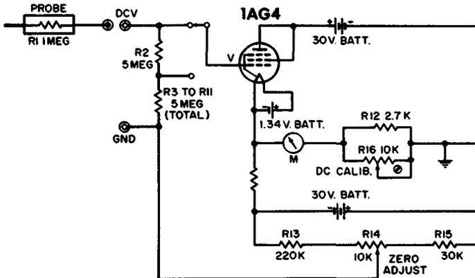
Fig. 1-17. VTVM-adapter configuration.
