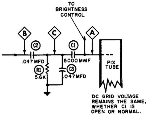
Fig. 6-7 Vertical-retrace blanking circuit.
