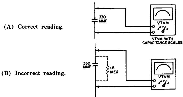
Fig. 4-5. Shunt resistance causes incorrect indication of capacitance value.
