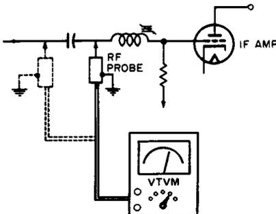
Fig. 2-9. Checking signal voltage at both sides of suspected open capacitor.
