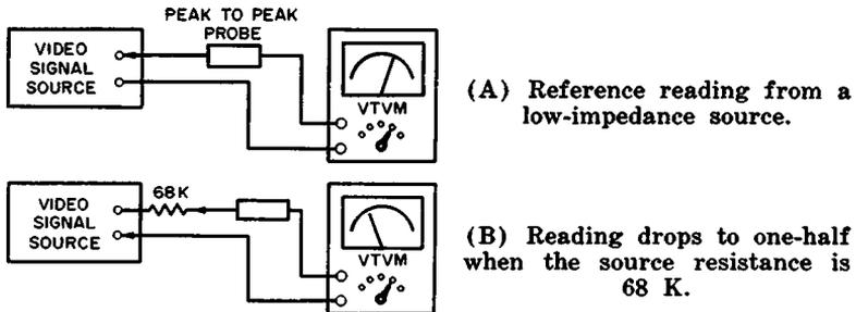
Fig. 3-3. Difference reading with a source resistance.
