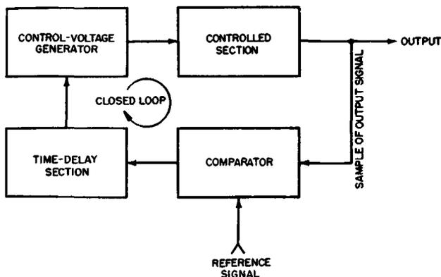
Fig. 4-3. Functional plan of a servo system.
