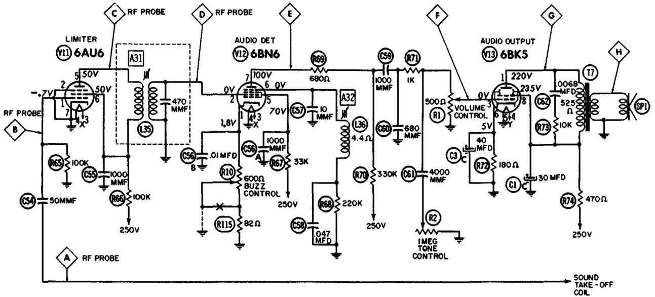
kill the circuit response. If a peak-to-peak probe and a VTVM are used to trace the intercarrier sound signal, it is inevitable that false conclusions will be made regarding dead grid circuits. On the other hand, an RF probe does not load the grid circuits objectionably, and thus will give fairly accurate readings.
