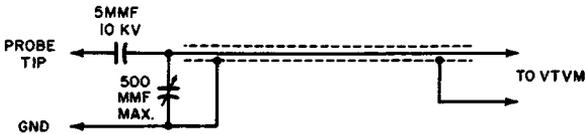
Fig. 11-7. An AC high-voltage capacitance-divider probe.
