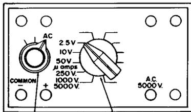
(A) Settings for measurement of AC voltage.
