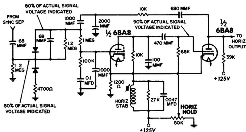
Fig. 4-8. Examples of circuit-loading errors in signal-voltage readings.
