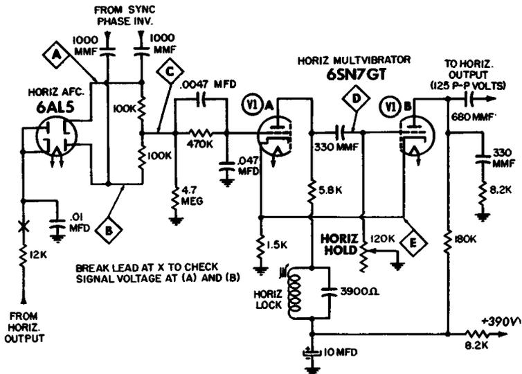
Fig. 4-7. Multivibrator with ringing-coil stabilization.
