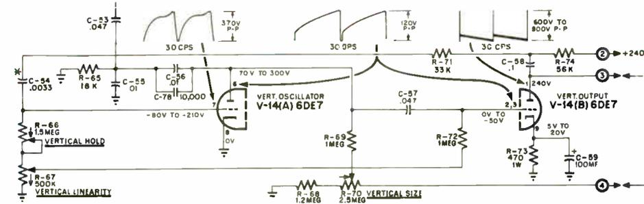
\* C-54, A.0033 MFD CONDENSER, HAS BEEN RELOCATED (TO PREVENT POSSIBILITY OF VERTICAL DRIFT DURING WARM-UP) AND IS HORIZONTALLY MOUNTED ON ETCHED CIRCUIT BOARD. (SEE FIG. #4, PG. 4)
