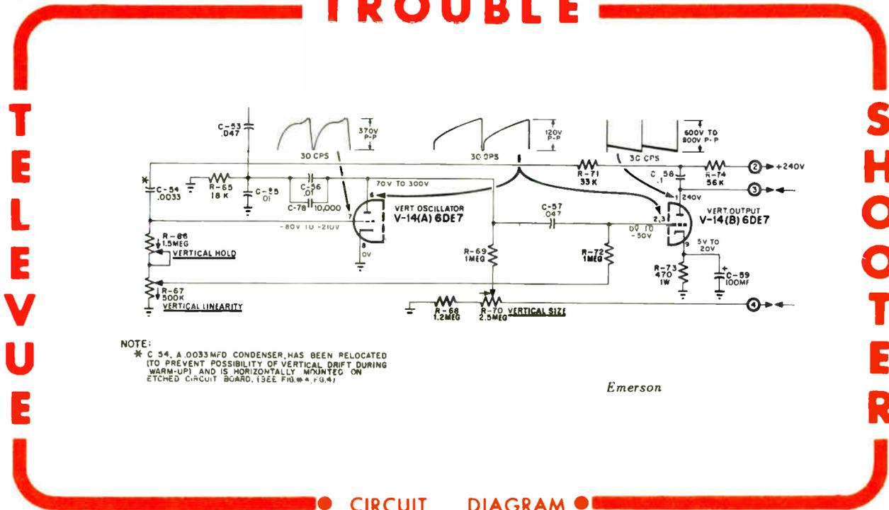
NOTE: \* C-54, A .0033 MFD CONDENSER, HAS BEEN RELOCATED (TO PREVENT POSSIBILITY OF VERTICAL DRIFT DURING WARM-UP) AND IS HORIZONTALLY MOUNTED ON ETCHED CIRCUIT BOARD, 13EE FIG. #4, P. G. 47.
