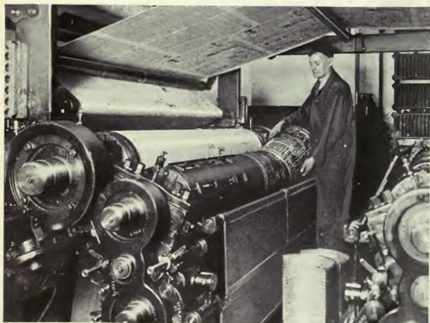
*PLACING stereotype plates on the printing cylinders of a Tribune press.*
