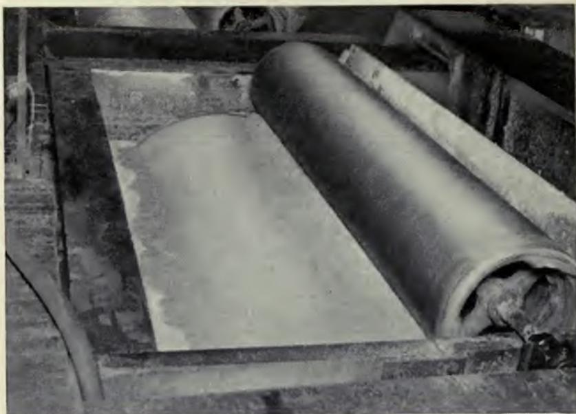
*AFTER splinters have been screened from the wood pulp it is forced between these two rolls. Water carrying away all soluble impurities flows through the lower, which is made of fine copper screen.*
