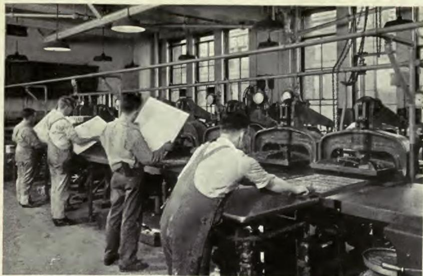
*Row of steam tables for making matrices. Stereotyper is examining mat of type page which his companion is removing.*
