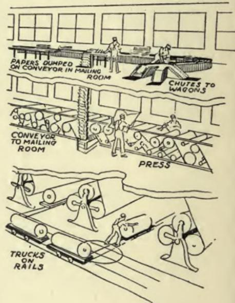
One of the principal features of The Tribune presses is their flexibility. Each press will print any size paper from eight to forty pages, and they can be tied up in such a way that no unit need be idle. The arrangement of the presses may be so adapted that no matter what the size of the paper, all the units are kept going.
