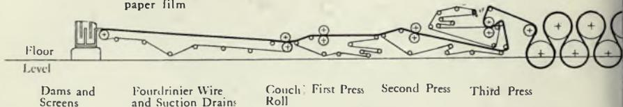
DIAGRAM of Paper Machine showing
