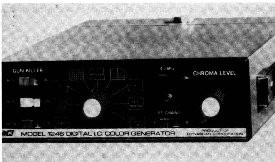
B & K Model 1246 digital IC color generator used for convergence adjustment.
