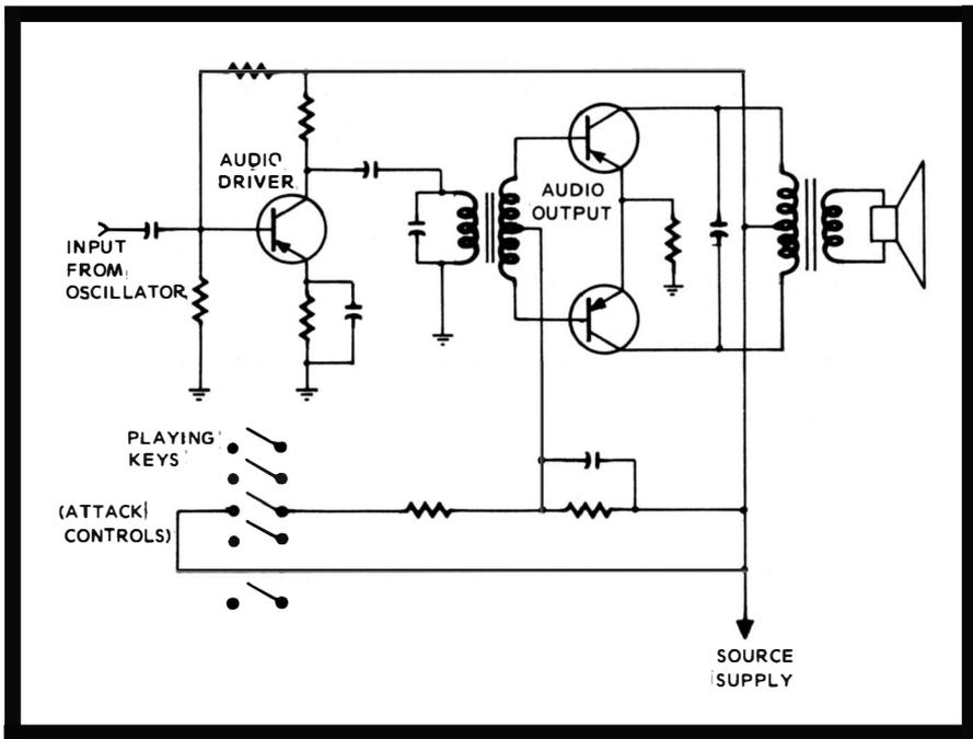
Fig. 97. Attack controls are attached to the playing keys and control a simple pushpull amplifier.
