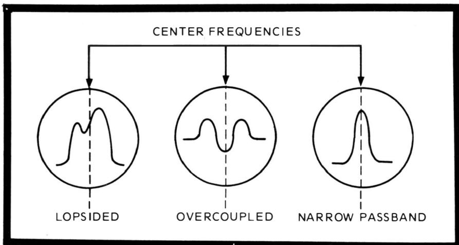
Fig. 3C. All kinds of incorrect response curves appear as the IF transformers are misaligned.
