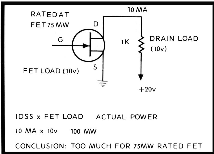
Fig. 72. FET power dissipation is obtained by multiplying  $IDSS$  times the FET load.
