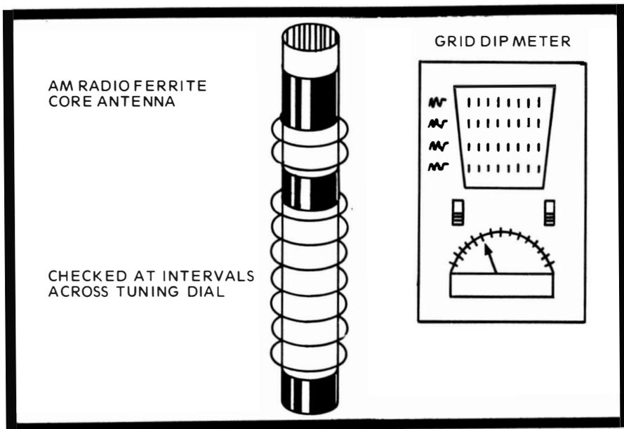
Fig. 7. A grid-dip meter is used to check the tuning of an antenna. At the tuned frequency the needle dips deep.
