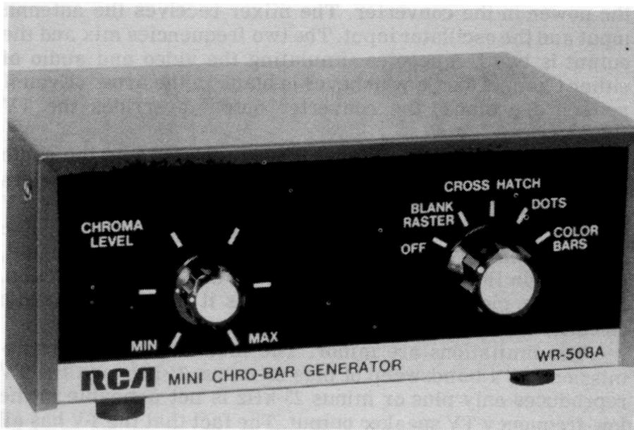
RCA WR-508A Mini Chro-Bar generator designed for color signal production.
