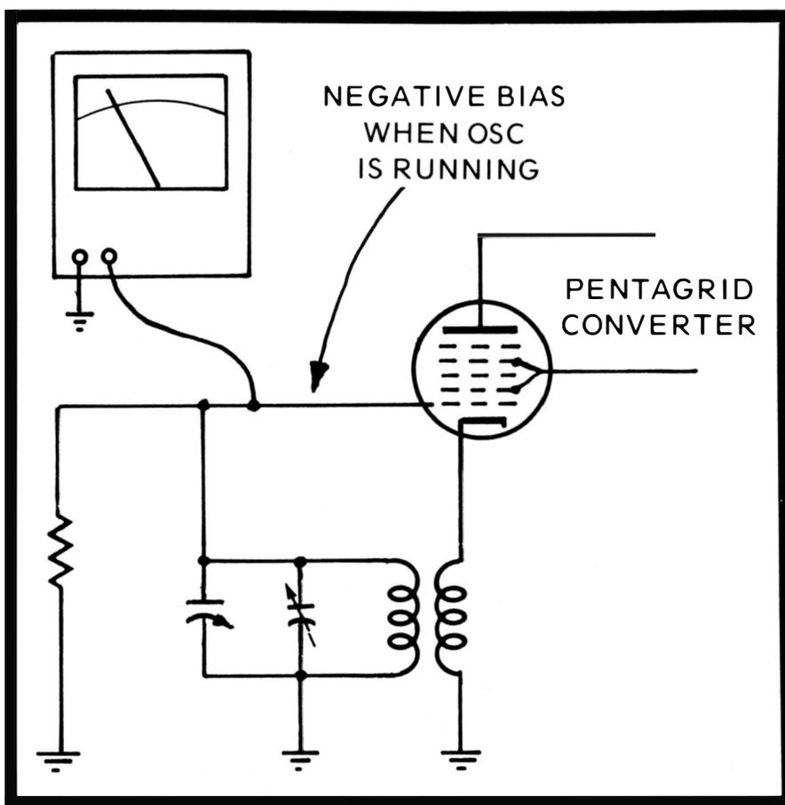
Fig. 9. A tube oscillator circuit is running when there is a good negative bias on the control grid.
