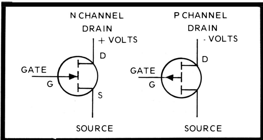
Fig. 66. An enhancement-type FET has a broken channel line, but has the arrows point like a depletion type.
