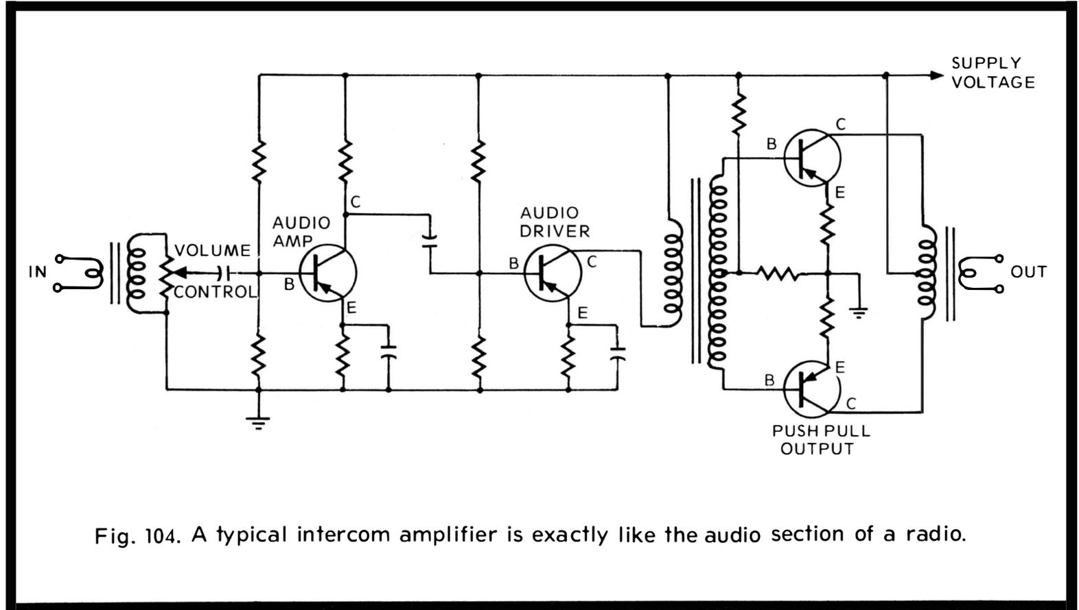
Fig. 104. A typical intercom amplifier is exactly like the audio section of a radio.
