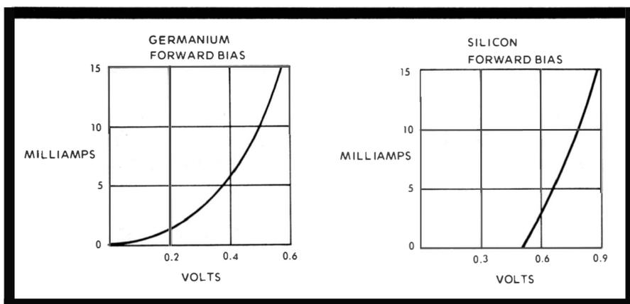
Fig. 76. Germanium transistors turn on as the forward bias approaches 0.2 volts. Silicon needs about 0.6 volts.
