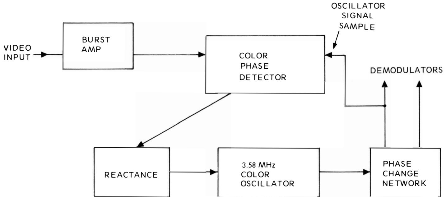
Fig. 31. The color burst has the job of locking in the frequency and phase of the color oscillator.
