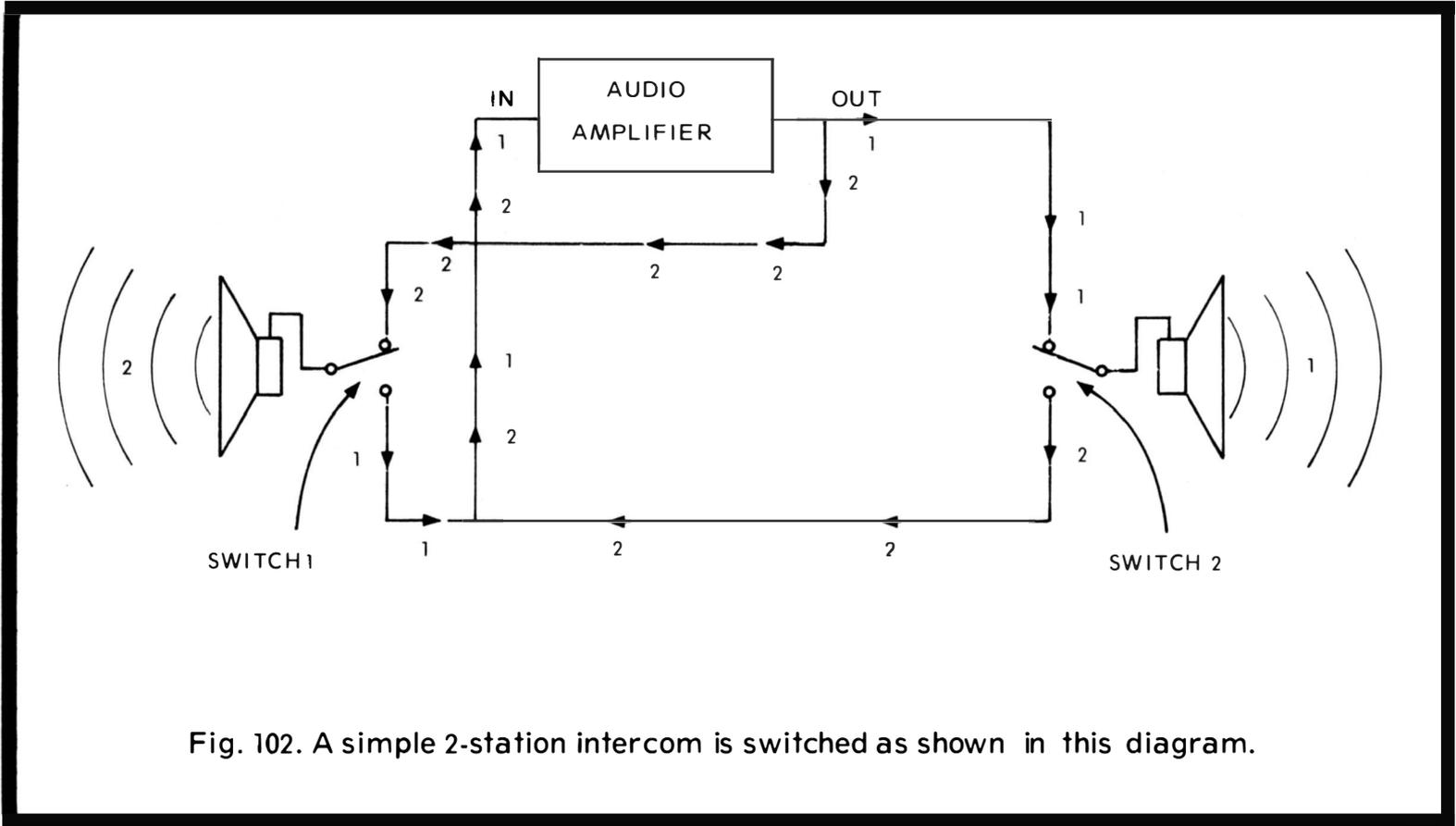
Fig. 102. A simple 2-station intercom is switched as shown in this diagram.
