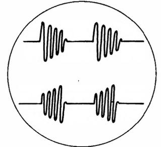
FIG. 3—Excessive or insufficient feedback produces waveforms shown.
