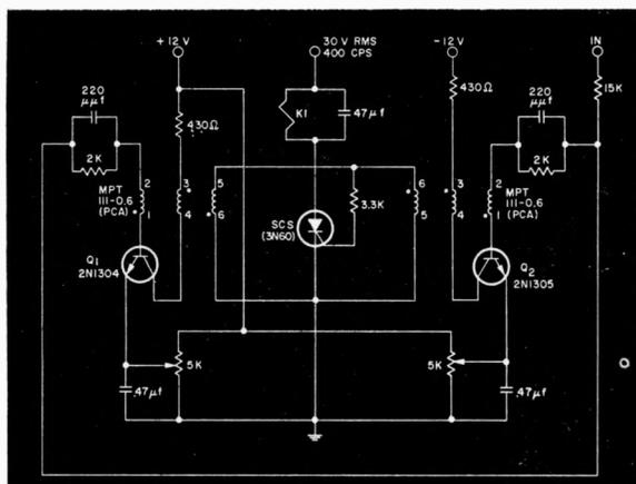
Complementary transistors  $Q_1$  and  $Q_2$  provide high input impedance for this voltage-monitoring circuit.
