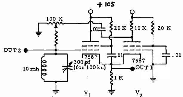
Resistive degeneration allows isolation of the tank circuit from the driving tube while eliminating all grid current from the tank.
