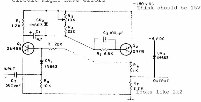
Neither transistor of this monostable multivibrator conducts until an input pulse is applied.
