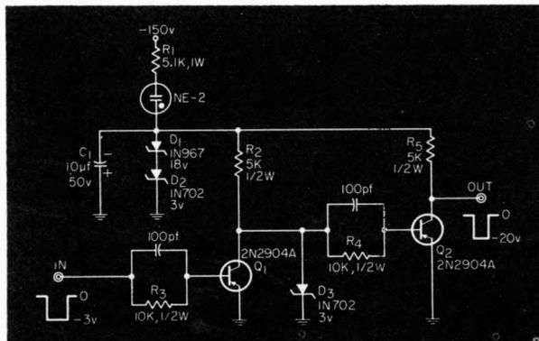
Z-axis modulation circuit.
