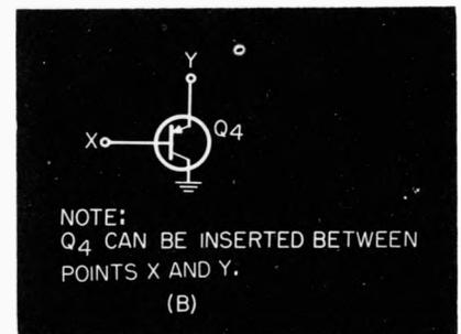
Fig. 2. Oscillator doubles as power driver with extra driver transformer. Power capabilities can be increased by adding transistor as shown in 2b.
