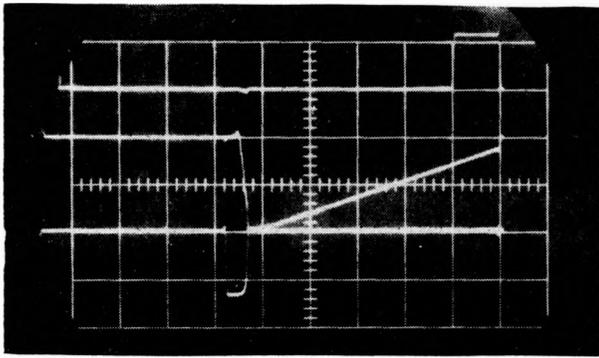
Phantastran wavelshapes. Time is read from right to left. Upper trace: input (10 v/cm); center trace: ramp (5 v/cm); lower trace: gate (10 v/cm).
