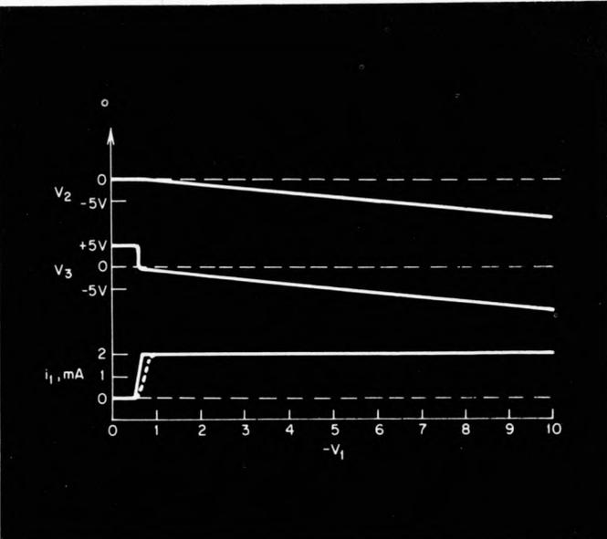
Fig. 3. Voltage-current relationships for a test circuit in which a negative-going ramp replaces the pulse generator and a meter and power supply replace the IC.
