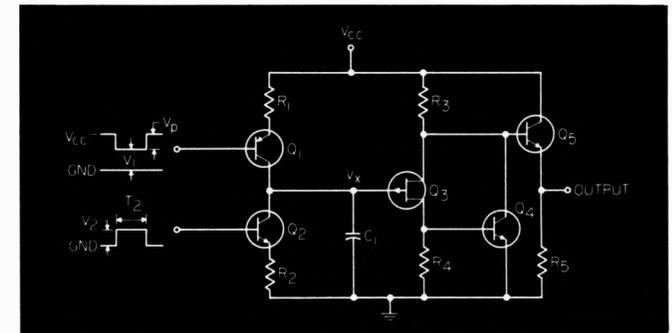
Fig. 1. Constant-current charge and discharge circuit integrates pulses.
