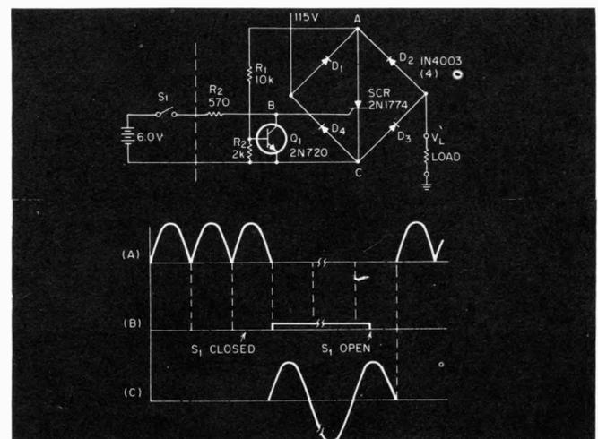
Fig. 1. Schematic and waveforms of zero-crossing solid-state switch. ■
