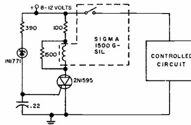
Voltage-limit sensing circuit.
