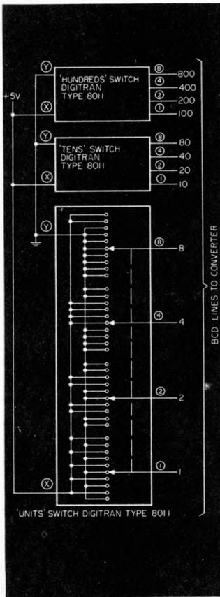
Fig. 2. Typical manual input circuit using thumbwheel switches.
