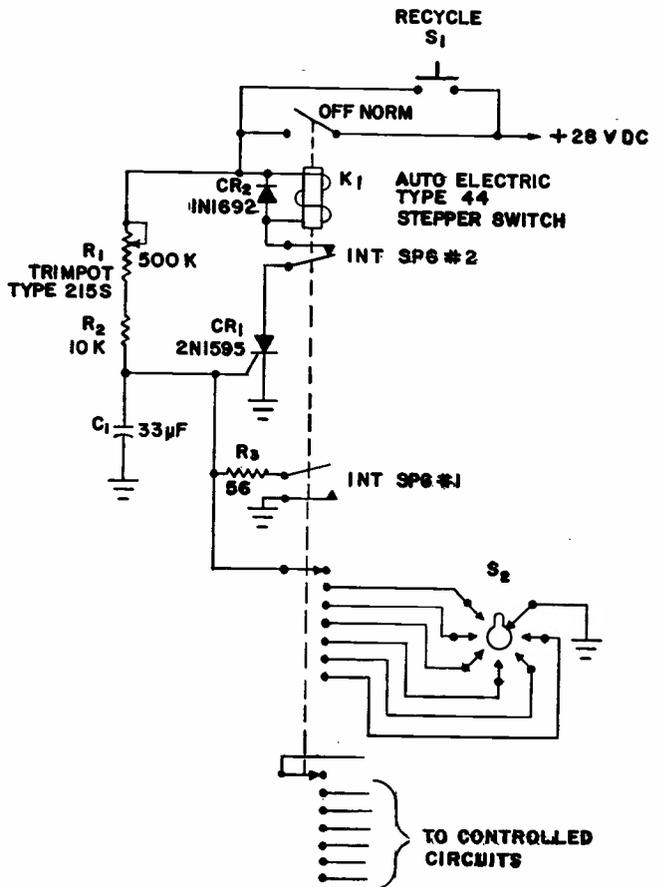
FIG. 1—Stepping switch control requires only seven components.
