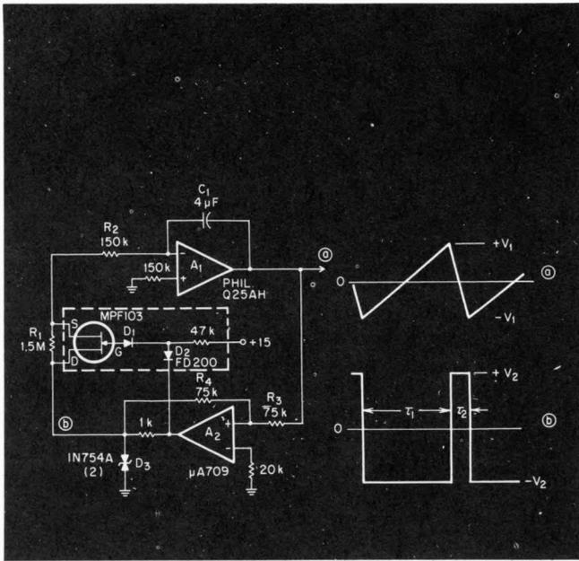
$D_2$  to the gate of the FET, occurs,  $A_2$  saturates positive, pinching off the source-gate junction. The time constant during this part of the cycle is  $(R_1 + R_2) C_1$ .  $C_1$  charges until the output of  $A_1$  reaches the positive trip level of the Schmitt trigger. When this
