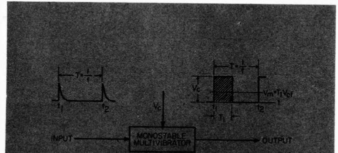
Fig. 1. Voltage-controlled one-shot multivibrator gives output pulses of constant width and variable height. Total period  $T$  is the reciprocal of input frequency, therefore mean output voltage is proportional to the product of  $f$  and  $V_c$ .
