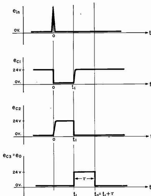
Fig. 2. Circuit waveforms.
