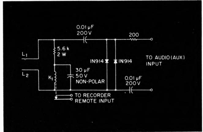
The circuit starts a tape recorder when a telephone receiver is lifted to make a call or receive one. The relay is a Sigma 65F1A — 24 Vdc or equivalent.
