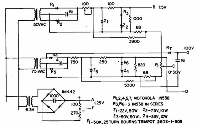
FIG. 2—Rectifiers *R*<sub>3</sub> and *R*<sub>6</sub> each consist of three in series.
