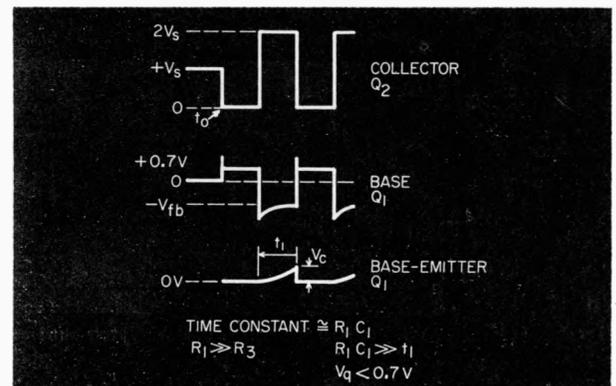
Fig. 2. Waveforms.
