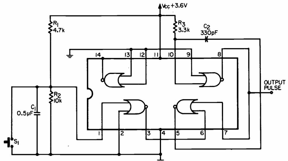
Fig. 1. Because switch  $S_1$  is shunted by  $C_1$  and has one side grounded, noise generated by the switch is normally below the threshold of the IC. The circuit generates output pulses from 1  $\mu$ s to 80 ms, wide depending on the value of  $C_2$ .
