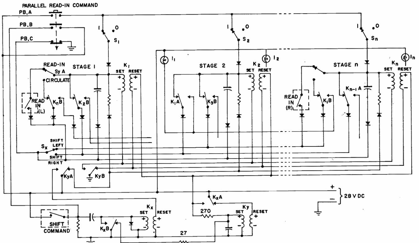
In the shift register, all A and B normally open contacts of relays  $K_1$  through  $K_n$  are tied together and go to readout indicators  $I_1$  through  $I_n$ . Capacitors are 8  $\mu$ f and diodes are 1N537. Unmarked resistors are 250-ohm, 5-watt.
