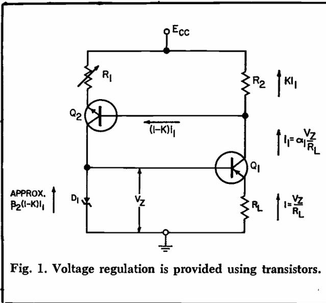
Fig. 1. Voltage regulation is provided using transistors.
