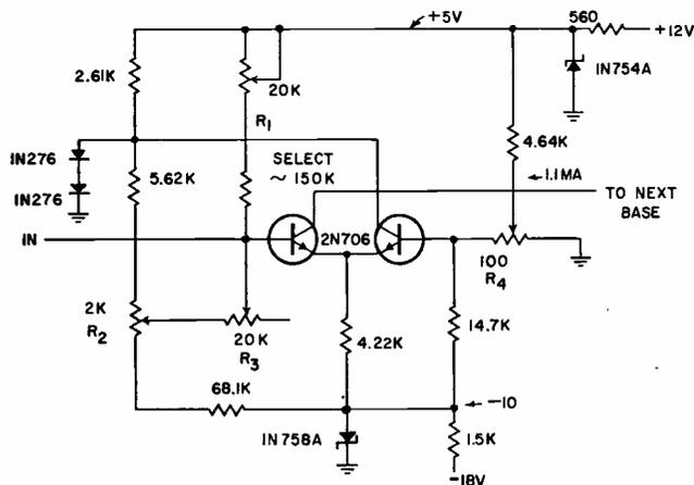
FIG. 1—Temperature coefficient is controlled by  $R_3$ .
