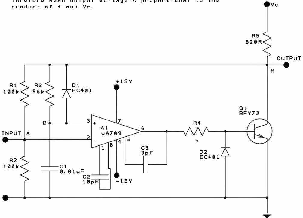
Fig. 2 This practical circuit accepts input frequencies from 1Hz to 1kHz and control voltages from 0.1 to 15 V. Note that voltage balance between points A and B doesn't depend on  $V_c$ . Therefore pulse width depends only on the values of  $R_3$  and  $C_1$ .
