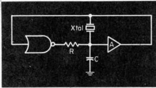
Fig. 1. Basic circuit of simple crystal-controlled pulse generator.
