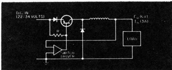
Fig. 1. Emitter-rectifier biasing.
