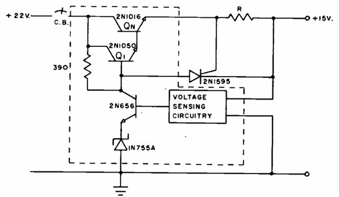
Transistor protection circuit for regulated power supply.
