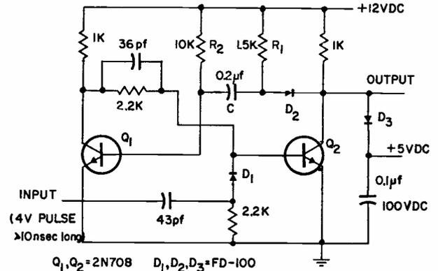
**FIG. 1**—Monostable multivibrator circuit designed for fast turnoff.
