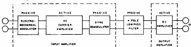
FIG. 1—Arrangement of stages of open loop amplifier.
