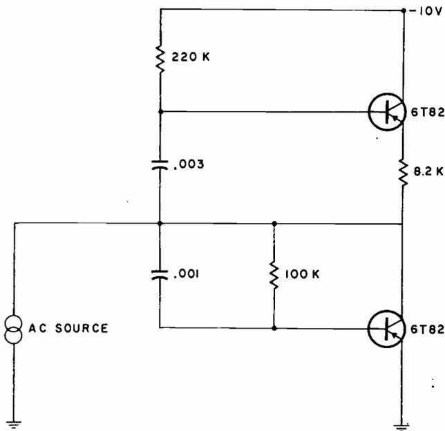
FIG. 2—Parallel-tuned circuit resonant at about 1 kc.
