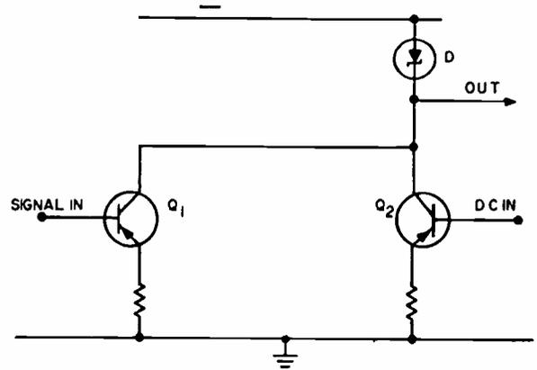
Fig. 1. Basic circuit of amplifier with dc controlled gain.
