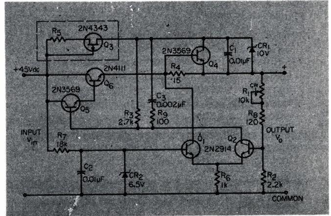
Fig. 1. In this voltage regulator, the FET constant-current source (inside the dashed rectangle) provides improved regulation, because current through  $CR_1$  is independent of input and output voltages.
