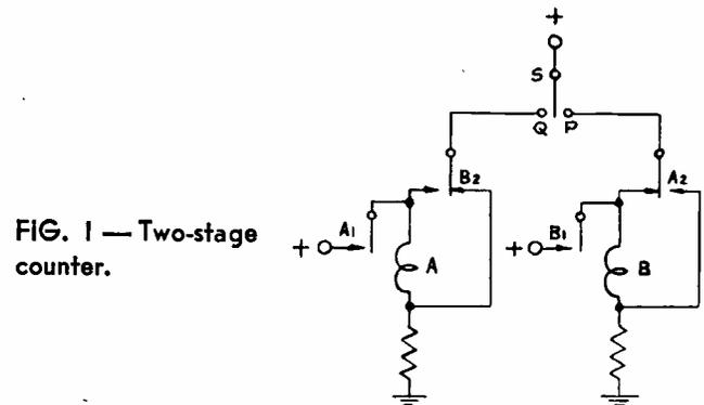
FIG. 1—Two-stage counter.
