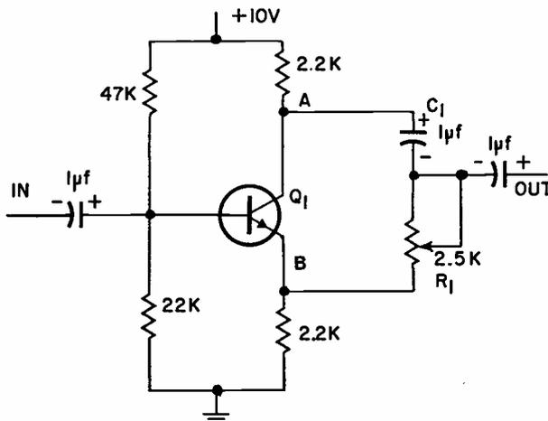
FIG. 1—Simple transistorized phase shifter, 0-180 deg. continuous.
