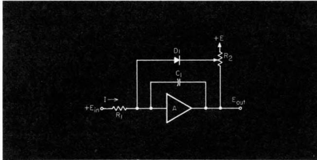
Fig. 1. This commonly-used limiter circuit for integrators has the disadvantage that calibration varies with input level.
