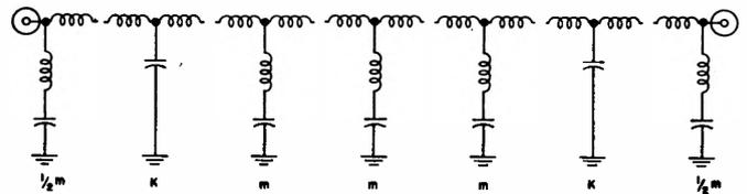
FIG. 2—Low pass filter.
