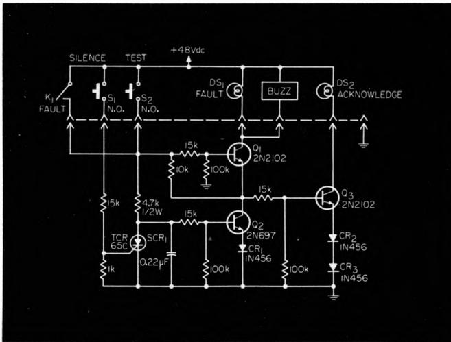
conduct momentarily, but not long enough to light the "acknowledge" lamp. The collector voltage of  $Q_2$  reverse-biases  $Q_1$  to hold it "off." The voltage drops of diodes  $CR_1$ ,  $CR_2$  and  $CR_3$  give suitable bias conditions for  $Q_2$  and  $Q_1$ . Both Transistor  $Q_1$  now conducts, the "fault" lamp and the buzzer remain energized until the fault is removed or the "silence" switch is actuated.
