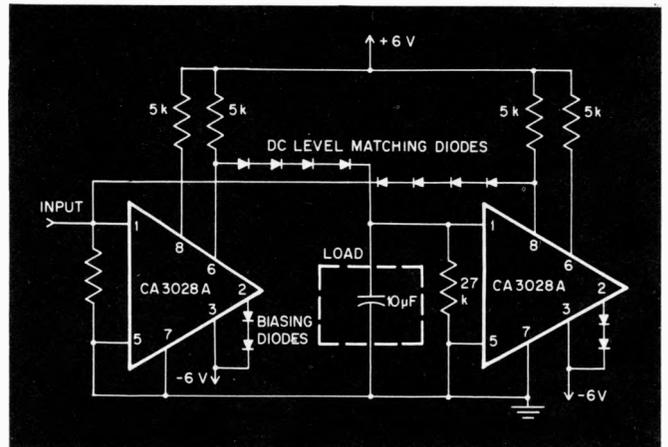
Fig. 2. This specific gyrator, with a 10- $\mu$ F load, effectively forms a 12- $\mu$ H inductor.
