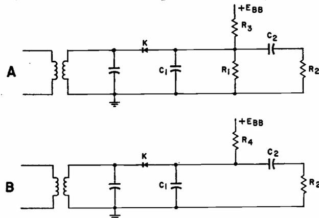
FIG. 2—Modified circuits avoid peak clipping.
