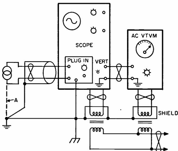
For preferred low level signal measurement: isolation power transformers, short twisted shielded cables, and single point grounding are emphasized.
