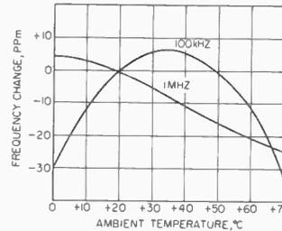
Fig. 3. Frequency varies less than  $\pm 30$  ppm over the temperature range 0 to  $+70^\circ\text{C}$ . Stability is determined primarily by the crystal.
