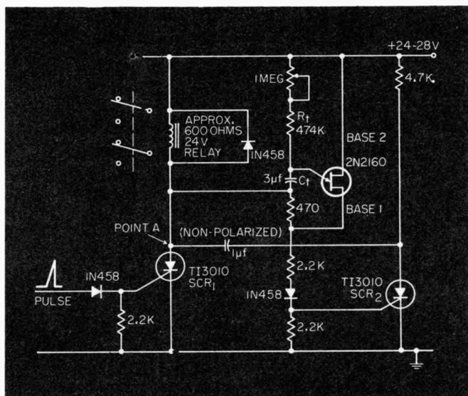
Low-cost intervalometer using unijunction transistor and two SCRs.
