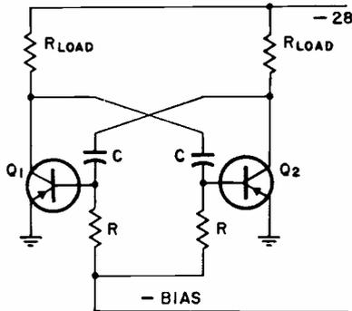
FIG. 2—Modified bias arrangement assures starting of multivibrator.
