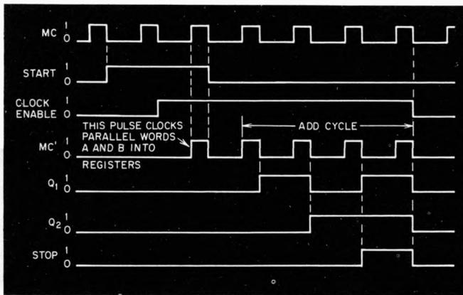
Fig. 3. Timing diagram for the 8-bit split adder.
