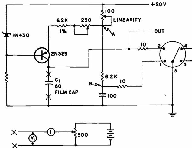
Test circuit at bottom is substituted for  $C_1$  during adjustment of linearity control of ramp generator.
