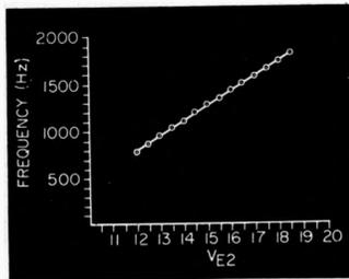
Fig. 3. Output frequency of the second stage is a linear function of the emitter voltage of  $Q_2$ .
