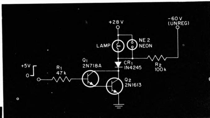
Fig. 1. In this simple lamp driver, the neon indicator provides failure indication for the incandescent lamp.
