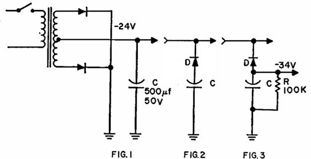
Devices requiring pure dc, such as transistor amplifiers, can be run off the same supply by attaching the load to C.
