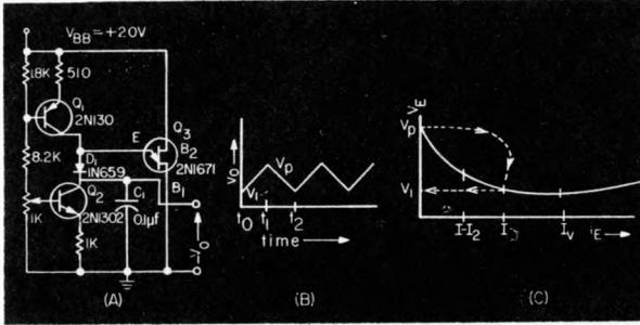
Fig. 1. UJT triangular wave generator (1a) with output wave (1b) and UJT switching path (1c).
