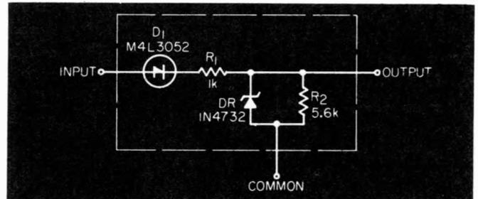
Simple, three-terminal active filter works like a Schmitt trigger, yet needs no external dc supply.
