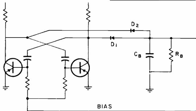
shown in Fig. 1. On initial turn on, or if in use with test equipment, both capacitors are switched simultaneously, and conditions may arise in which both  $Q_1$  and  $Q_2$  will be fully conducting. (Amount of saturation is determined by  $R$  and the negative bias voltage.) With both  $Q_1$  and  $Q_2$  saturated, their incremental gain is low. Loop gain may not be sufficient to ensure oscillation.
