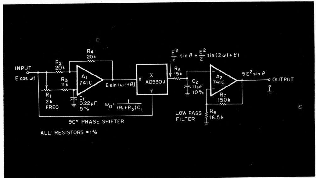
Two IC op-amps and a multiplier form a frequency discriminator circuit.
