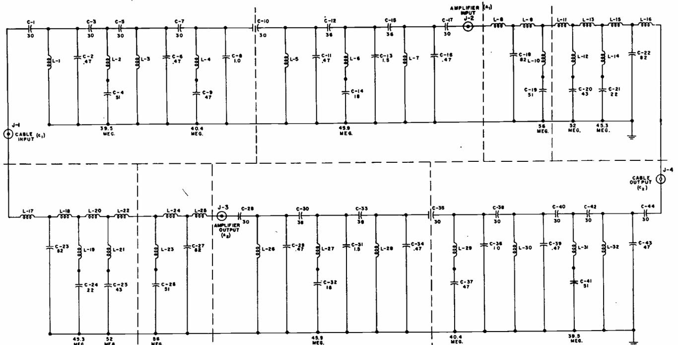
FIG. 6—Complete circuit of frequency splitter. All capacitor values are in  $\mu\text{f}$ .
