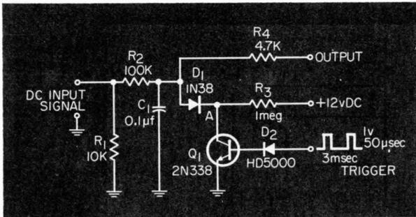
Clearing circuit for  $R_2$ - $C_1$  integrator network.
