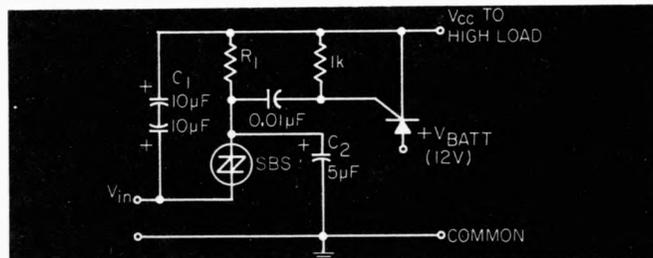
Simple switching circuit uses a bilateral trigger device which provides a high input impedance and draws negligible standby current.
