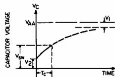
Fig. 2. Voltage waveform across capacitor  $C_1$  while charging.
