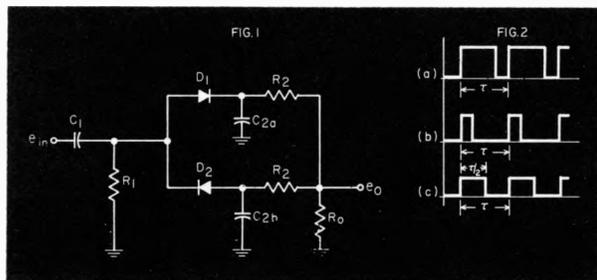
Fig. 1. Square-wave symmetry detector.
