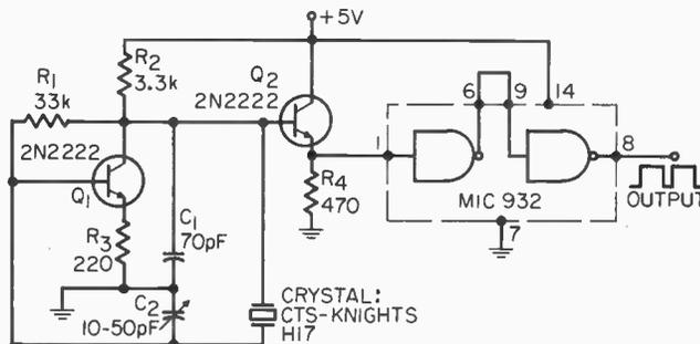
Fig. 1. Simple 1-MHz clock oscillator operates from +5 V supply and gives output levels compatible with digital ICs.
