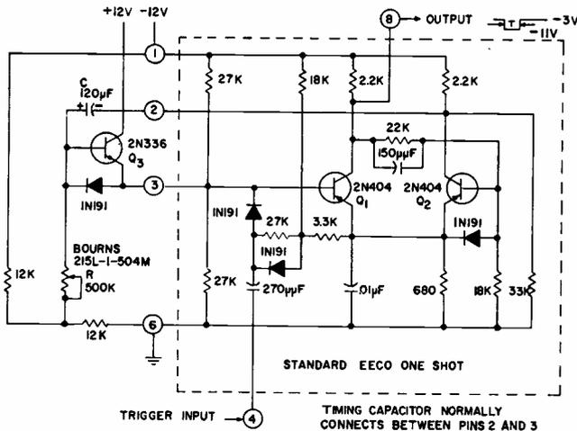
Output pulse width of one-shot mv is variable from one second to one minute.
