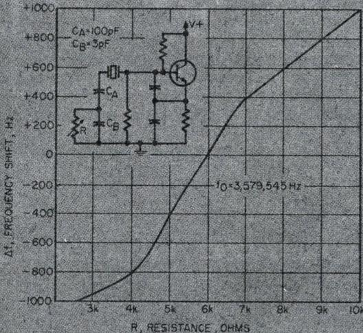
circuit of the basic crystal oscillator without FET control. Oscillation frequency is given by Eq. 1.
