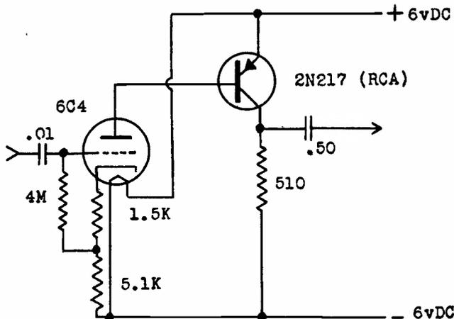
Hybrid circuit provides high input impedance, low output impedance with voltage gain.
