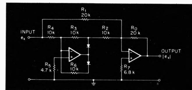
Fig. 1. This widely used absolute-value circuit has the disadvantage that many of the resistors must be accurately matched.
