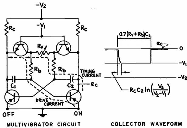
FIG. 2—New mv circuit and its collector waveform.
