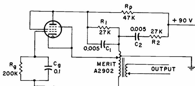
FIG. 1—Plate-tuned RC oscillator circuit for 1000 cps.
