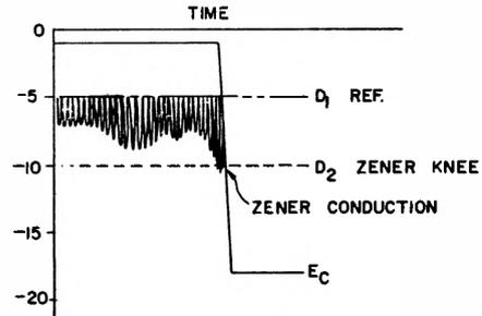
Level switch circuit (top) has snap action effect when ac signal goes over zener conduction point (bottom).
