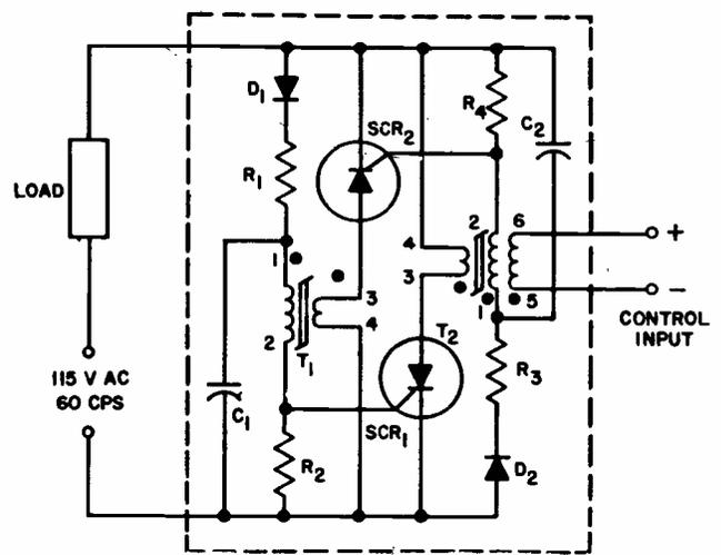
$R_1, R_3$  10 K, 1 W,  $T_1, T_2$  Magnetics Inc.
