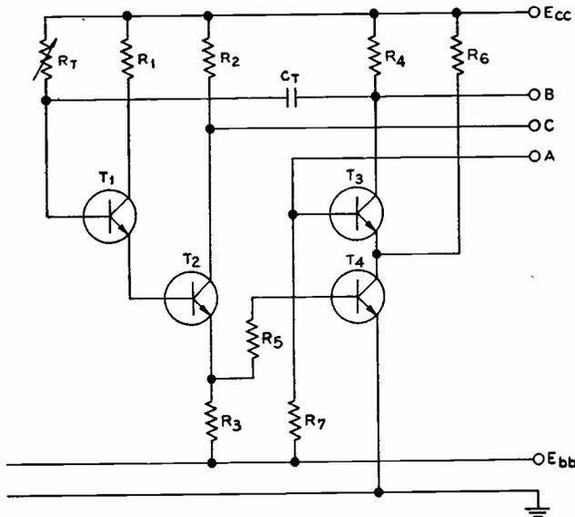
FIG. 1—Ohmic values of resistors follow:  $R_1$  and  $R_5$  —100;  $R_2$  —2700;  $R_3$ ,  $R_4$  and  $R_6$  —4700;  $R_7$  —100K. All transistors are 2N388 and  $E_{cc}$  is —22v, and  $E_{bb}$  is —6v.
