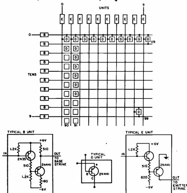
Fig. 2. Matrix form of XY code converter.
