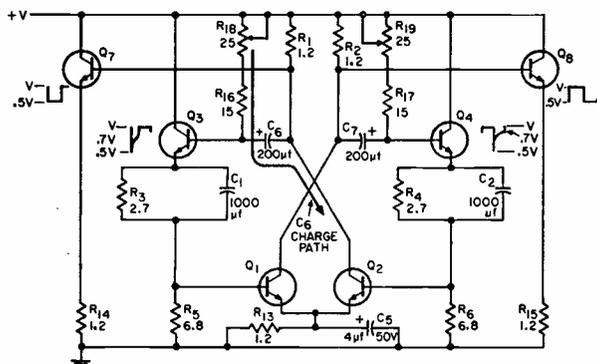
Pulse generator provides variable frequencies from low impedance pulses. All resistors are in kilohms, 10 percent,  $\frac{1}{2}$  w; all transistors are 2N35 or similar; all unmarked capacitors are in picofarads.
