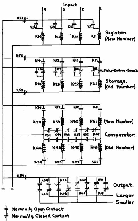
Corresponding bits of the two binary numbers are compared in the relay circuit. The larger number is the one with the highest order 1 that is not matched by the other number.
