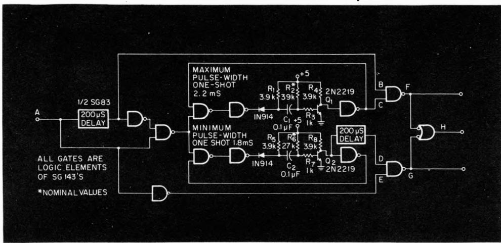
Fig. 3. Circuit for measuring 2-ms pulses with a  $\pm 10\%$  window.
