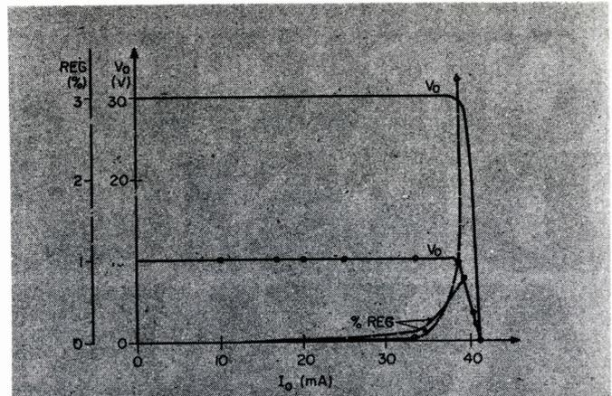
Fig. 2. Typical output characteristics and regulation characteristics for nominal output voltages of 30 V and 10 V. Note the current limiting at around 40-mA load current.
