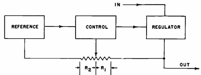
FIG. 1—Conventional two-transistor regulator.
