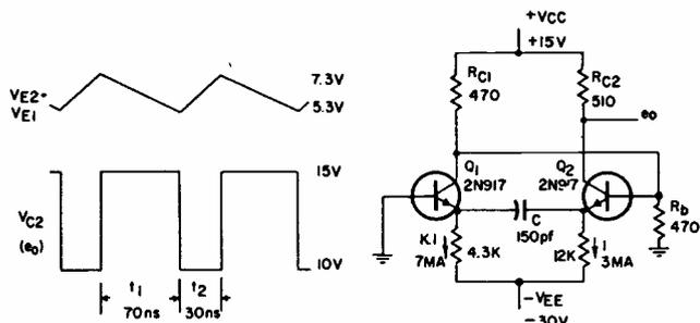
FIG. 1—Current switching astable multivibrator and its waveforms.
