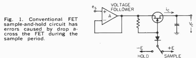
**Fig. 1.** Conventional FET sample-and-hold circuit has errors caused by drop across the FET during the sample period.
