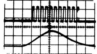
The circuit is now in the configuration of a Schmitt trigger in which saturation is prevented by using the small collector resistor. Thus, drift transistors may be used and biased properly to achieve high-speed operation.
