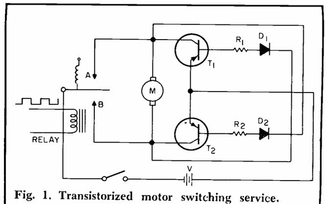
Fig. 1. Transistorized motor switching service.
