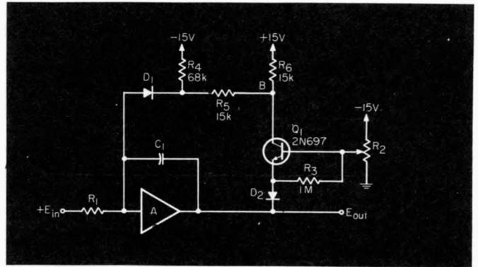
Fig. 2. Modified circuit gives improved accuracy because of the gain of grounded-base amplifier  $Q_1$ .
