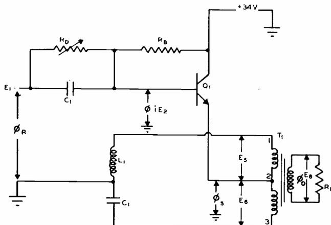
FIG. 2—Suggested values:  $R_D = 100K$ ;  $R_B = 18K$ ;  $C_1 = 1500 \mu\text{mf}$ ;  $C_2 = .047 \mu\text{f}$ ;  $Q_1 = \text{T12N1050}$ ;  $T_1 = 1:1.4, 10 \text{ kc}$ ;  $L_1 = 2-4 \text{ mh}$  in series.
