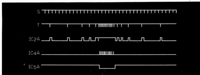
Fig. 2. Timing diagram shows the effects of  $T$  frequencies higher and lower than the  $S$  frequency.
