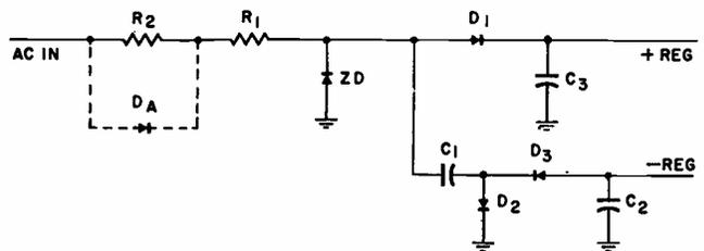
FIG. 2—Zener diode replaces two diodes of Fig. 1.
