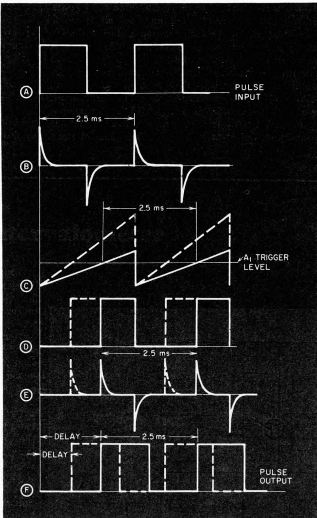
When the input goes positive,  $Q_2$  turns on and discharges  $C_s$ . Negative excursions are bypassed by  $CR_T$ . When the input goes low at the end of the positive excursion, voltage comparator  $A_1$  senses the low voltage and its output goes low.  $C_s$  begins to charge through the variable current source ( $R_1, R_2, Q_1$ ), which determines the slope of the charging curve. When the voltage across  $C_s$
