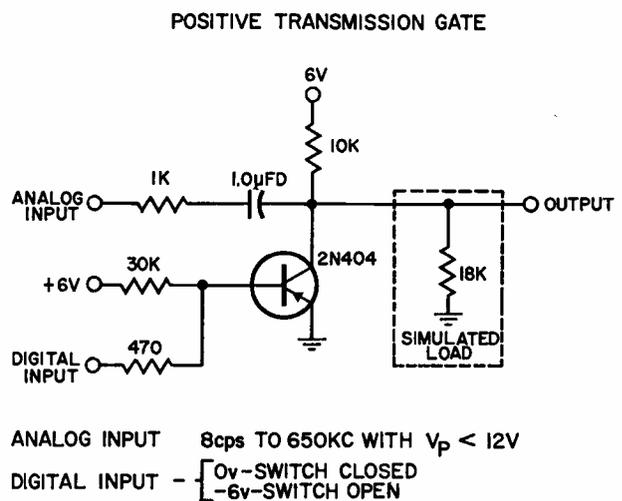
Fig. 1—Positive transmission gate.
