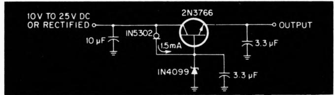
This simple zener regulator covers a very wide range of input voltages — even with large ripple content. It delivers at least 40 mA at a nominal 6 V. ■
