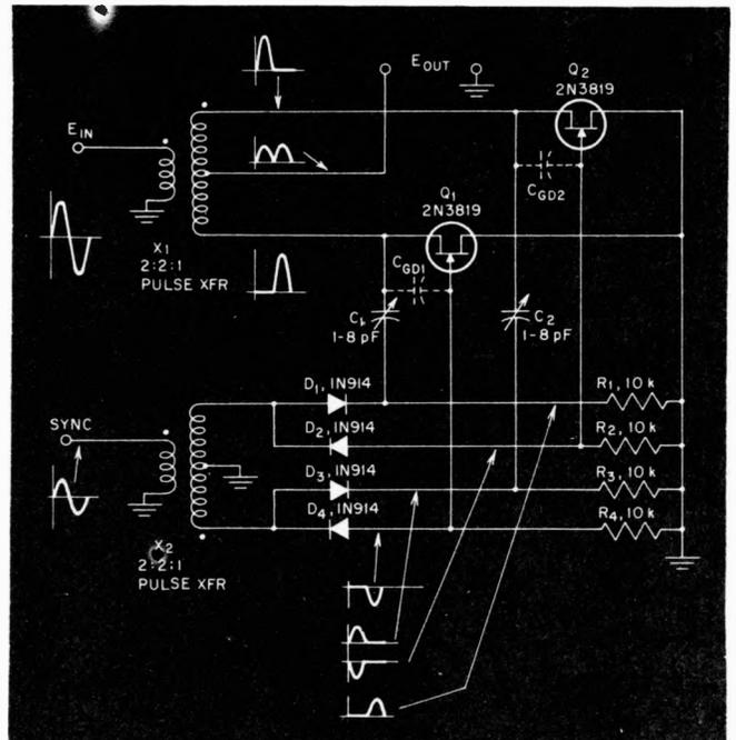
Capacitive feedback of gate signals eliminates forward sync-signal feedthrough, boosting synchronous-detector frequency capability.
