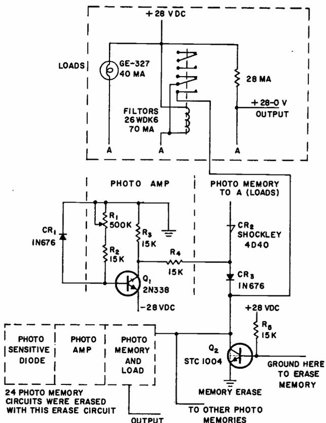
Diode CR<sub>1</sub> is a conventional silicon type with paint removed to allow light to reach junction.
