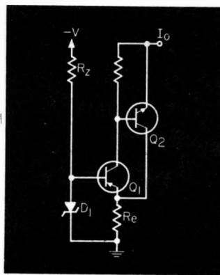
Fig. 2. Temperature drift can be minimized by matching the TCs of  $D_1$  and  $Q_1$ 's  $V_{be}$ . There is little internal temperature rise in  $Q_2$ , because  $Q_2$  handles the bulk of the load current.
