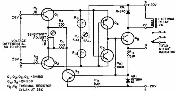
Fig. 1 Voltage comparator.
