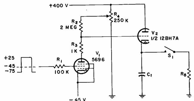
FIG. 1—Circuit of voltage controlled high voltage switch.
