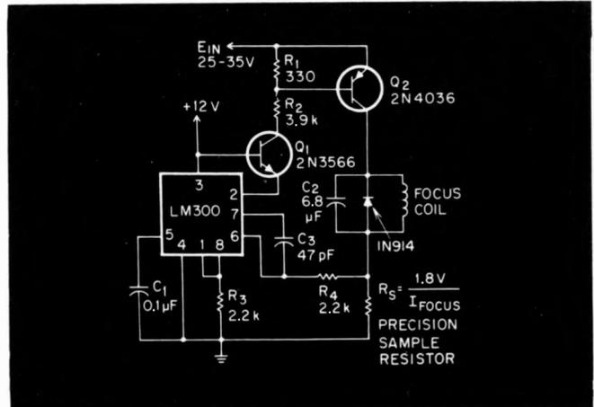
**In this precision focus-current regulator, the focus coil and the IC regulator are fed from separate voltage sources. Thus the unregulated input voltage can exceed the allowable maximum for the IC.**
