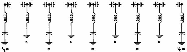
FIG. 4—High pass filter.
