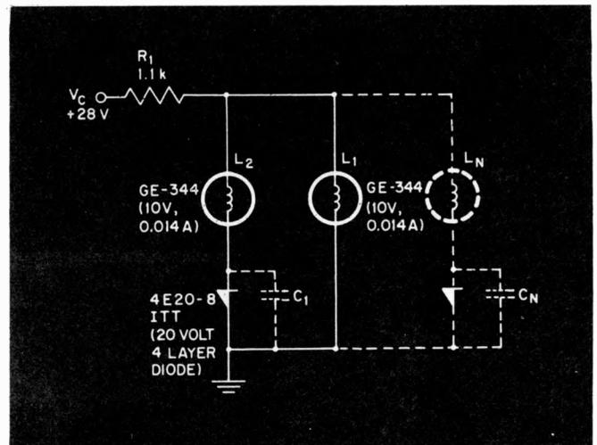
Automatic lamp back-up circuit using 4 layer diodes.
