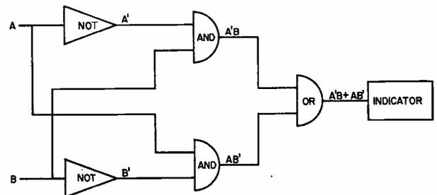
Fig. 1-Logic Performed.
