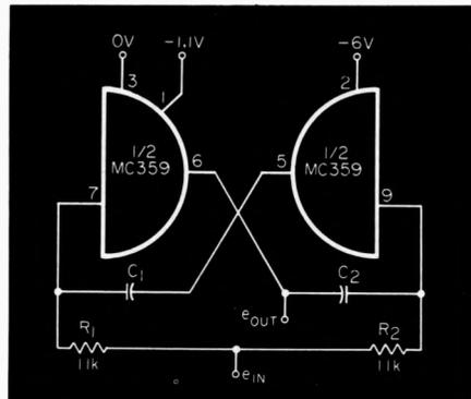
Fig. 1. Cross-coupled NOR gate provides sensitive low-cost VCO.
