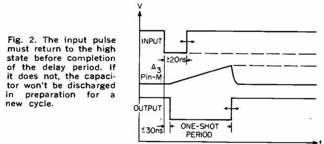
Fig. 2. The input pulse must return to the high state before completion of the delay period. If it does not, the capacitor won't be discharged in preparation for a new cycle.
