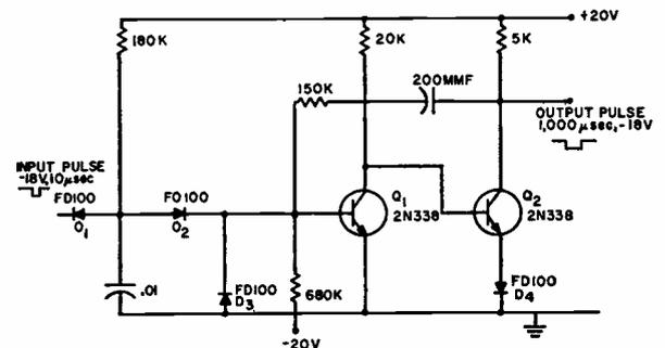
Monostable circuit with less than zero recovery time.
