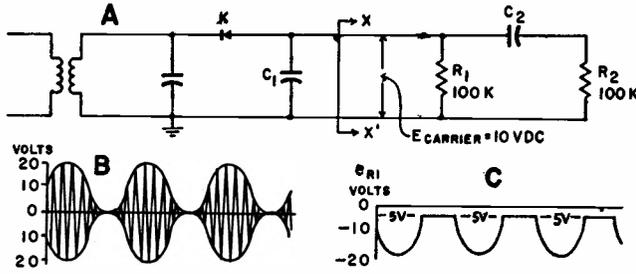
FIG. 1—Diode a-m detector and inherent clipping effect.
