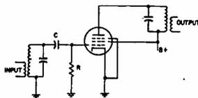
FIG. 2—Conventional limiter  $E_c$ ,  $I_p$  relationship demonstrates degradation of limiting action caused by grid circuit time constant.
