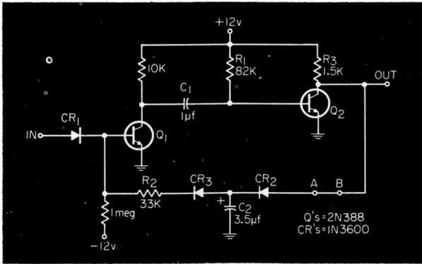
Fig. 3. Frequency-divider circuit.
