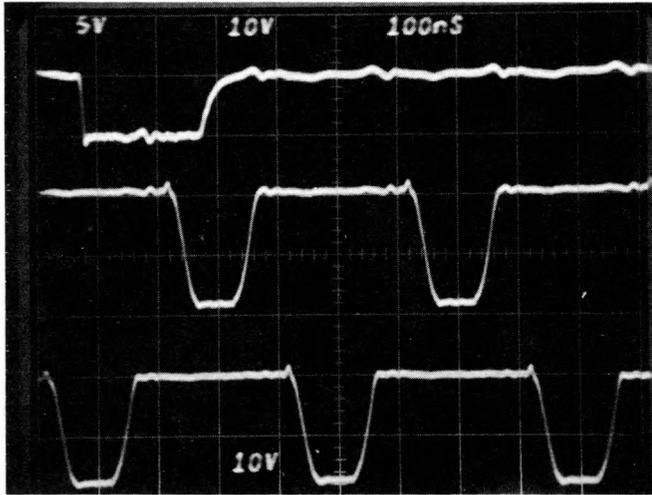
Fig. 2. In the photo, the top trace is data output and the next two traces are the two-phase clock signals. Data rate is 5 MHz and clock rate is 2.5 MHz.
