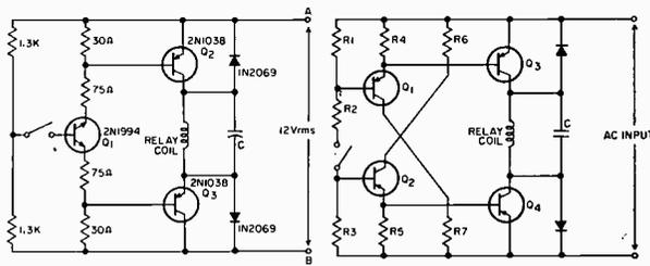
Fig. 1. Circuit drives a 12v ac relay. (left)
