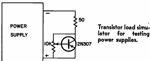
is in saturation. The load current is therefore established by  $R_1$  at 30 V/50 ohms or 0.6 amp. As the pot arm is turned down towards the emitter the transistor comes out of saturation and the load current decreases. With the base shorted to the emitter the collector current is some small value essentially equal to  $I_{co}/(1-\alpha_n\alpha_i)$ . At 30 v this may be about 10 ma in germanium and less in silicon.
