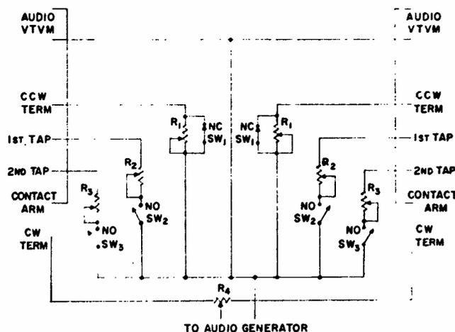
FIG. 1—Basic circuit for measuring tracking of stereo controls.
