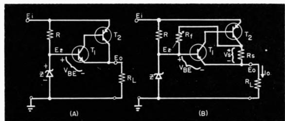
Fig. 1. Two-transistor voltage regulator; a. without feedback; b. with positive feedback; c. with positive feedback and temperature compensation.
