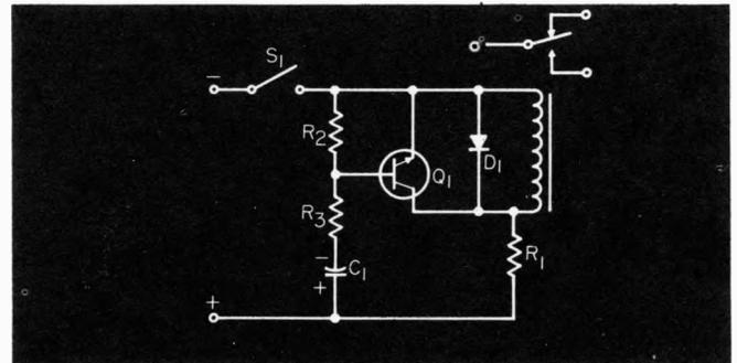
Fig. 1. In this simple time-delay circuit, transistor  $Q_1$  reduces the size of capacitor  $C_1$  needed for a given time delay. But this circuit has slow reset because  $C_1$  must discharge through the resistors and the relay coil.
