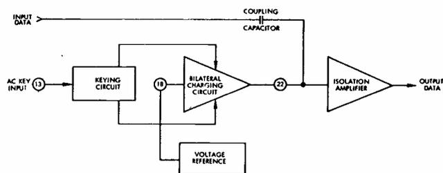
FIG. 2—Bilateral charging circuit used in dc restoration.
