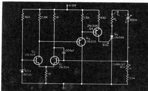
Fig. 2. Constant-current supply using SCR as load control.
