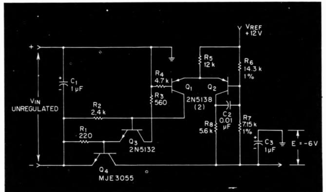
Low-cost voltage regulator provides high efficiency by reducing the required input voltage.
