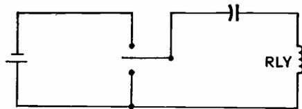
FIG. 1 — Basic circuit for switching polarized relay.
