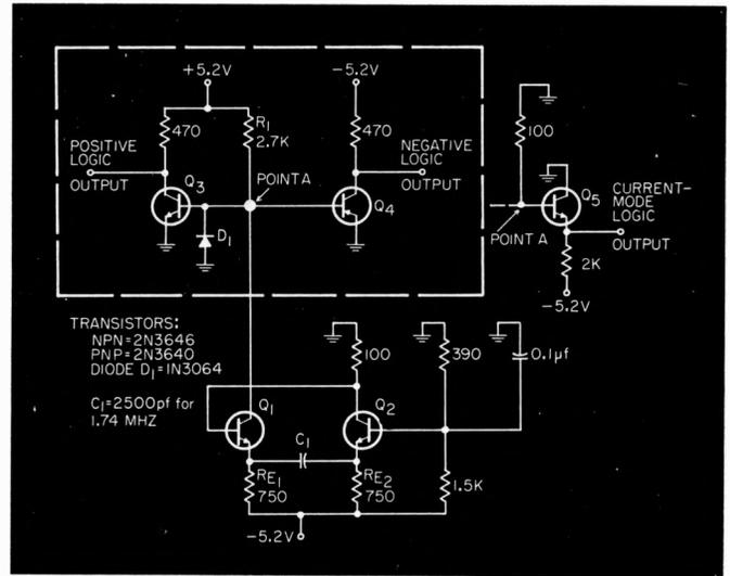
Emitter coupled astable; the circuitry in the dashed box may be replaced by  $Q_5$  as shown.
