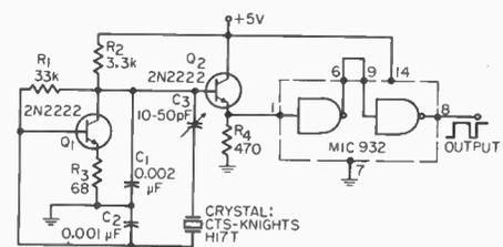
Fig. 2. For lower frequencies, as in this 100-kHz circuit, an additional capacitor  $C_3$  is needed to provide the correct shunt capacitance for the crystal.
