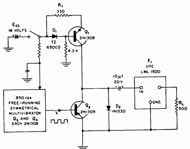
FIG. 1—Circuit for generating constant amplitude sine waves.
