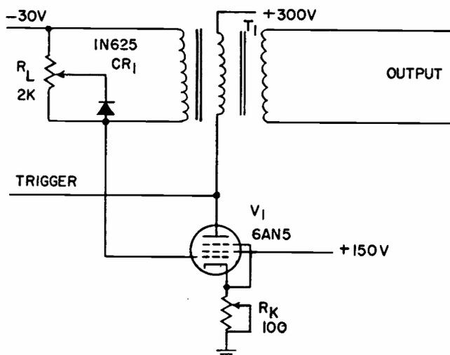
Pulse width can be varied over a range of four to one by adjusting the diode current.
