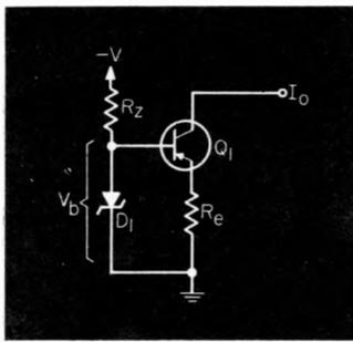
Fig. 1. A conventional ground-base current source has the disadvantage of poor temperature stability.
