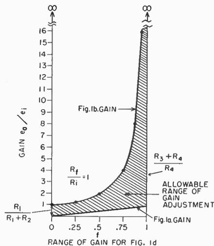
Fig. 2. Range of gain for control circuit of Fig. 1d.
