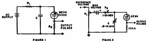
Fig. 1. Basic pulse circuit.
