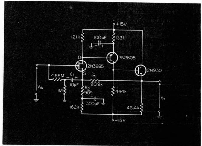
Low-noise preamplifier for low-capacitance transducer.
