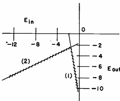
FIG. 4—Approximate values of output versus input voltage.
