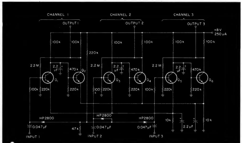
This 3-input amplitude comparator is based on repetitive 2-transistor sections that lend themselves to construction of an n-input comparator. The transistors are 2N4286.
