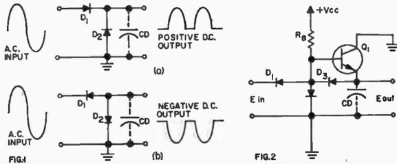
Fig. 1. Basic clamping circuits.
