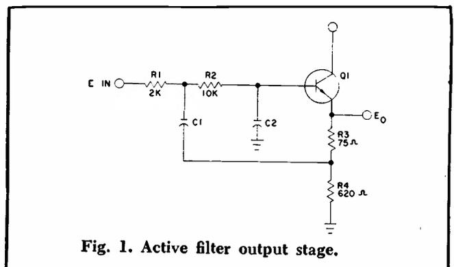
Fig. 1. Active filter output stage.
