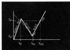
Fig. 2. Tunnel-diode characteristic with operating load lines.
