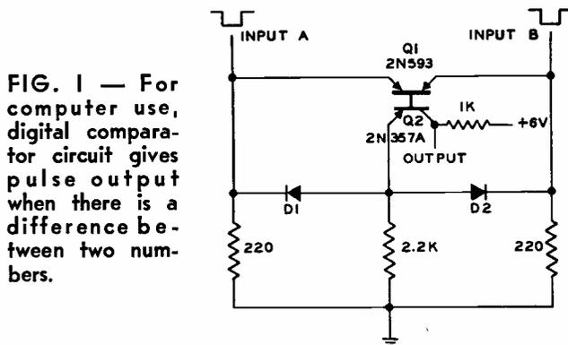
FIG. 1 — For computer use, digital comparator circuit gives pulse output when there is a difference between two numbers.
