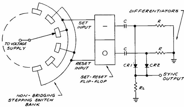
FIG. 1—Synchronizer eliminates noise problems in high-speed switching.
