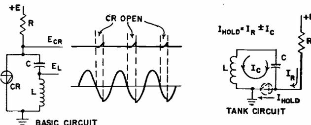
Waveforms and tank circuit action in quasi-sinusoidal relaxation oscillator circuit.
