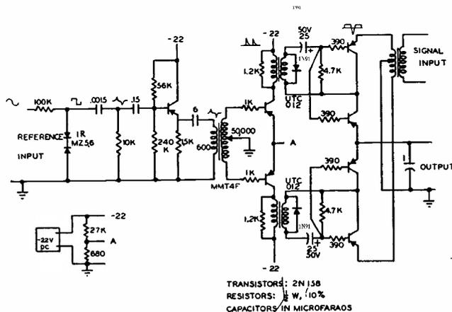
FIG. 2—Circuit of pulse demodulator with pulse reference.
