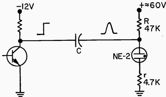
Small voltage changes are adequate to drive this neon readout.
