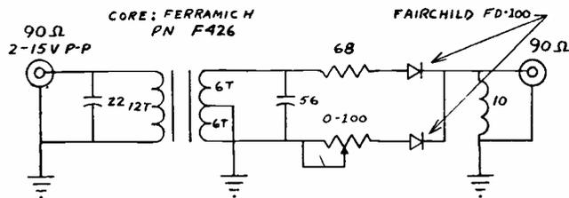
Circuit for doubling frequency from 25 to 50 mc.
