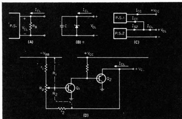
Constant-voltage current sinks: bleed resistor, 1a; zener diode, 1b; two supplies, 1c; and recommended dc-amplifier, emitter-follower circuit, 1d.
