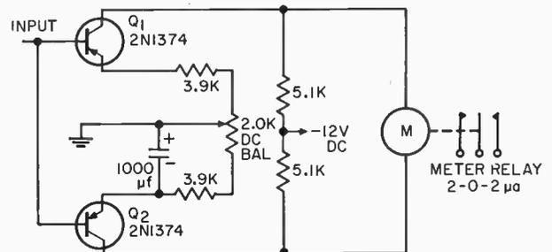
Rate circuit triggers relay on rapid input voltage changes.
