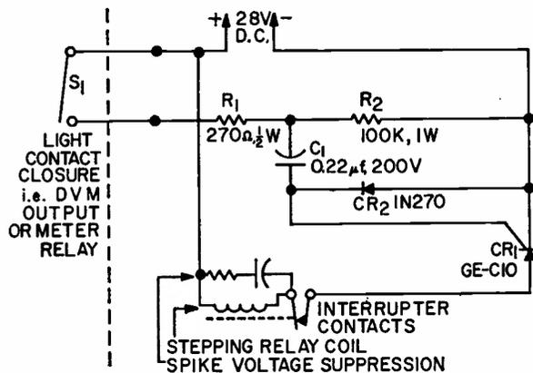
Circuit converts a switch closure to a one-shot step for a stepping relay.
