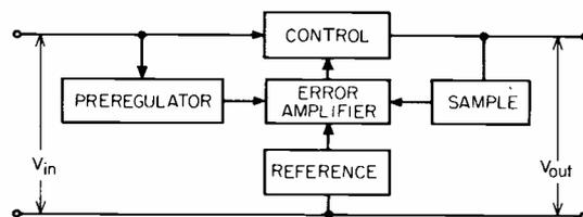
Fig. 3. Simplified block diagram of feedback voltage regulator. Prereg circuit biases the error amplifier.
