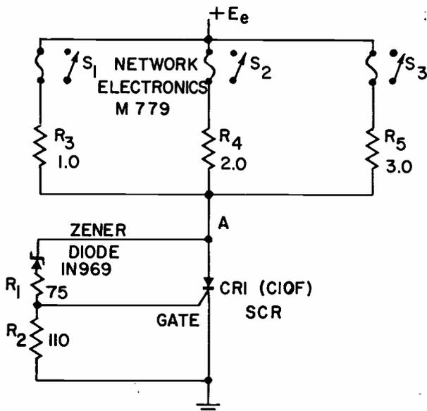
FIG. 1—Voltage sensitive trigger circuit initiates sequenced time delays.
