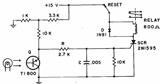
FIG. 1—Phototransistor controls silicon controlled rectifier operated relay.
