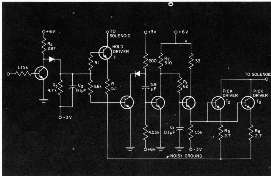
To eliminate transient noise problems, networks  $R_1, R_2, C_1, R_3, R_5,$  and  $R_3, R_5, C_2, R_6,$  control the switching speed of high-current drivers  $T_1, T_2$  and  $T_3$ .
