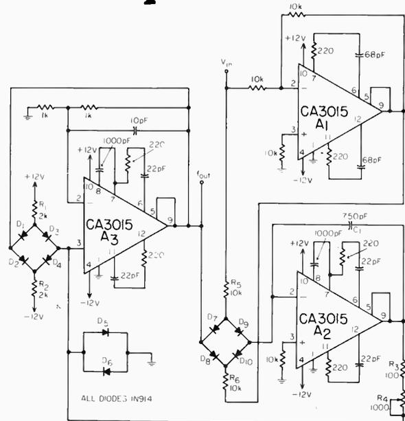
Fig. 1. IC op amps simplify the design of this VCO which gives a triangular wave at the output of  $A_2$  and a square wave at the output of  $A_3$ .
