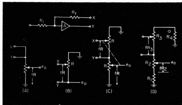
Fig. 1. Four methods of gain control. Method shown in 1d is most practical for control from zero to infinity.
