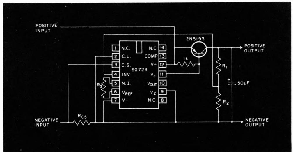
Positive high-efficiency regulator uses an external pnp transistor. Minimum  $V_{in} = V_{out} + 0.5 \text{ V} = R_{cs} I_L$ . Output = 7 to 37 V. er biasing for the rest of the circuitry.
