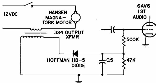
Noise pulses from motor are rectified and used to bias audio stage to cutoff.
