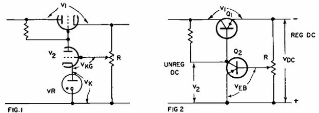
**FIG. 1**—Tube regulator using VR tube as reference.
