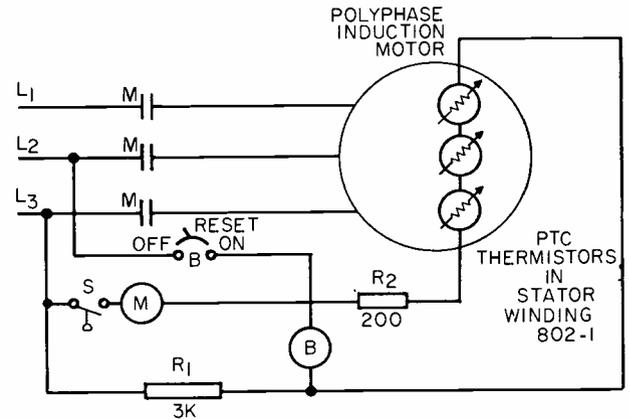
Fig. 3. PTC used with a 3-phase induction motor.
