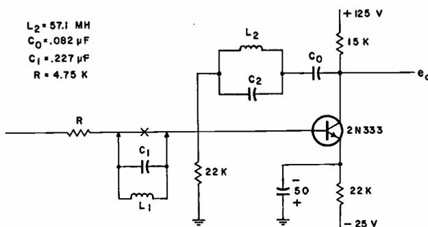
FIG. 3—Modified circuit has antiresonant circuit  $C_1, L_1$
