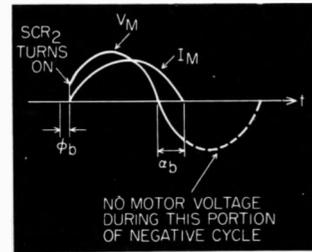
Fig 2 b (right) In this example, however,  $\phi_b$  is less than  $\alpha_b$  so there is no motor voltage during the latter part of the negative half cycle.
