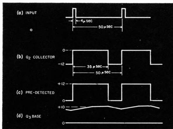
**Fig. 2. Waveforms at various points of missing-pulse detector.**
