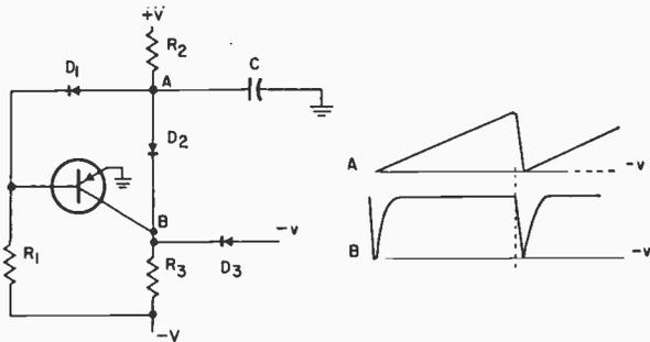
Single-transistor generator employs germanium diodes at  $D_1$  and  $D_3$ , and a silicon type at  $D_2$ . Waveforms shown occur at points A and B.
