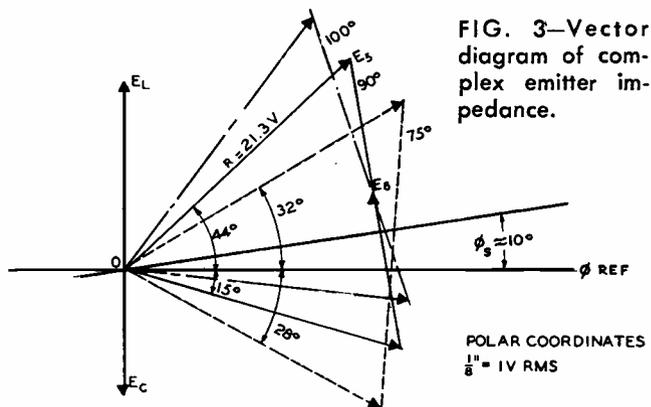
FIG. 3—Vector diagram of complex emitter impedance.
