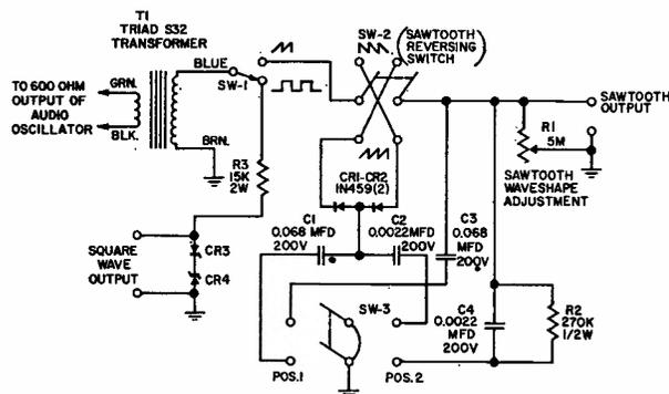
Converter changes 50-17000 cps sine waves to sawtooth or square waves.
