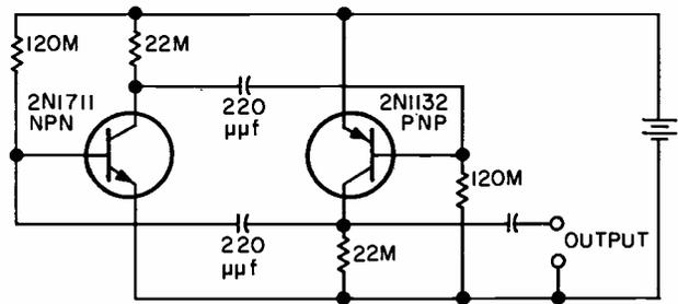
Fig. 1 Multivibrator having extremely low power consumption.
