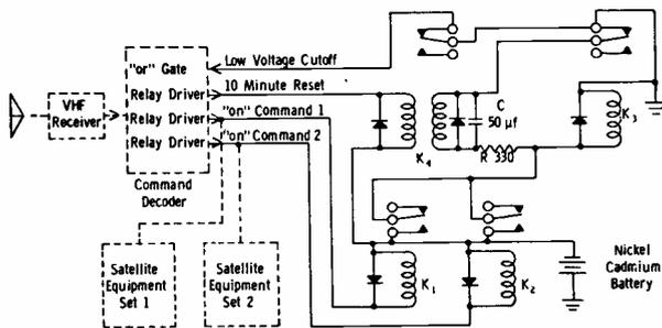
FIG. 1—Low-voltage de-energizer.
