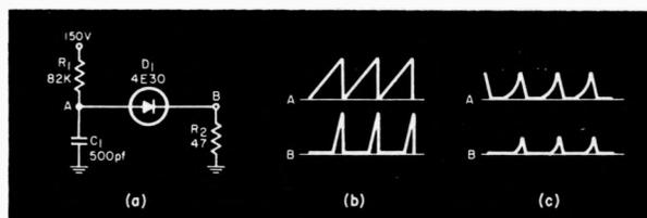
Fig. 1. Basic negative-resistance sawtooth oscillator with associated waveforms.
