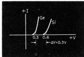
Fig. 2. Threshold voltages for germanium and silicon diodes.
