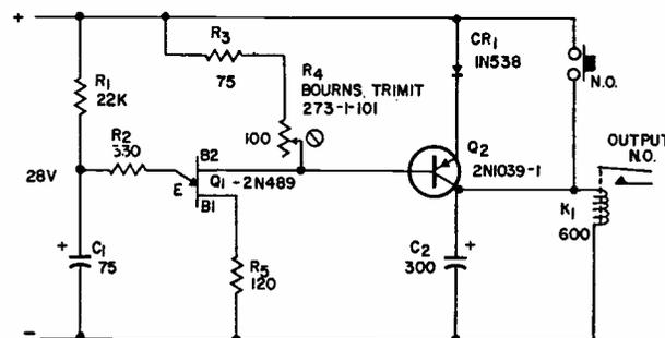
Change of dc input to power supply is accomplished by this low-frequency switching circuit. Adjust  $R_4$  for best symmetrical waveform at relay contacts (time on-time off).
