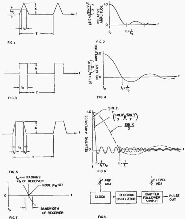
This wave shape has a spectral distribution of the form  $(\sin x/x) (\sin y/y)$  where  $x = n\pi t_1/T$  and  $y = n\pi(t_1 + t_0)/T$ . A plot of this function in  $x$  and  $y$  is shown in Fig. 6.
