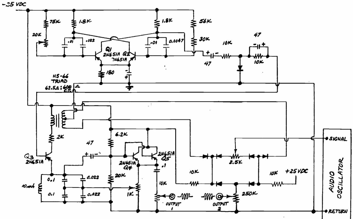
FIG. 1—All diodes are 1N645A and all transistors are Motorola 2N651A. Type 236S-1-203 Bourns Trimpot was used for the 20K pot at top left, 224S-1-252 for the 2.5K pot, and 224S-1-102 for the 1K pot at Q
