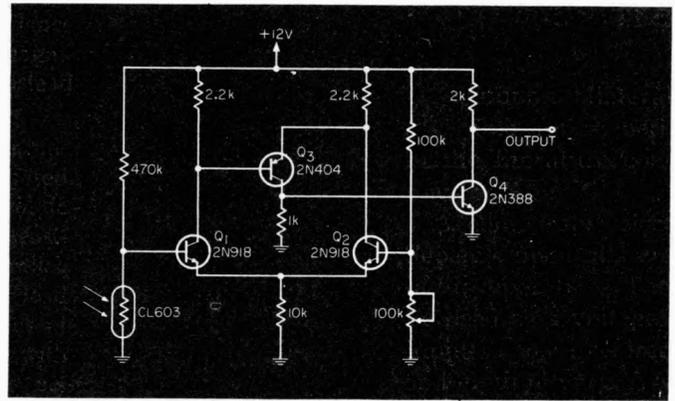
Light-activated switching circuit uses a resistive photocell.
