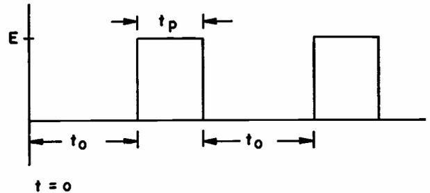
Fig. 2. Output wavelshape shows on and off times.
