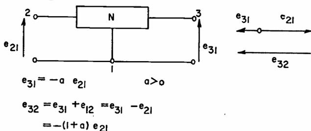
FIG. 1—Three-terminal network provides 180-deg phase shift.
