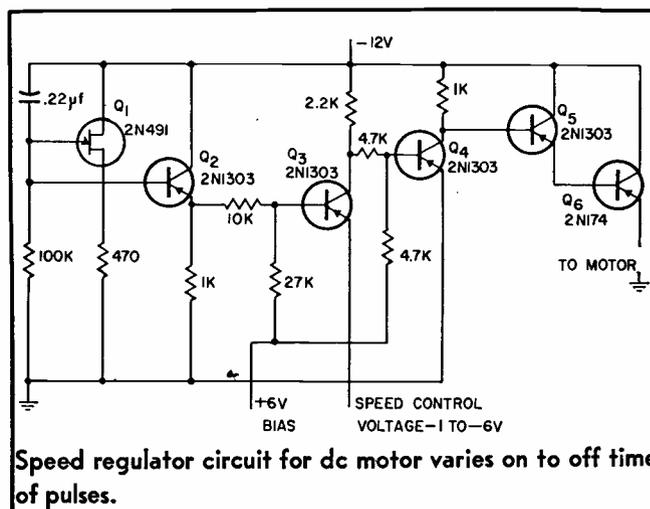
Speed regulator circuit for dc motor varies on to off time of pulses.
