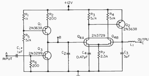
Fig. 1. In this simple D/A converter,  $Q_1$  generates a ramp voltage across  $C_2$ . Duration and height of the ramp are controlled by the input signal which turns on  $Q_3$  to discharge the capacitor.
