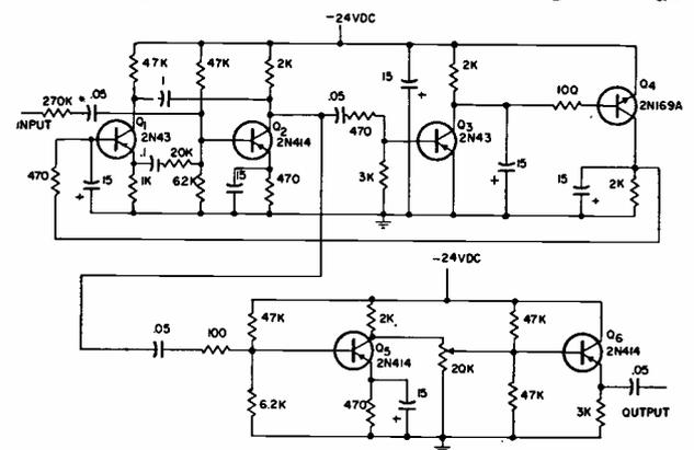
Wide range of input voltage is handled by this agc amplifier.
