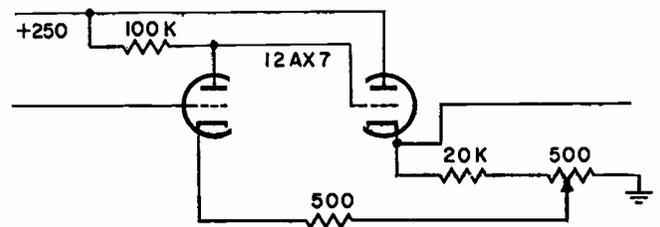
Additional gain circuit is similar to  $Q$  multiplier. original gain of the amplifier. In this case the amplifier's gain would be about 50, so that for high gain the pot arm would be raised to nearly 400 ohms.
