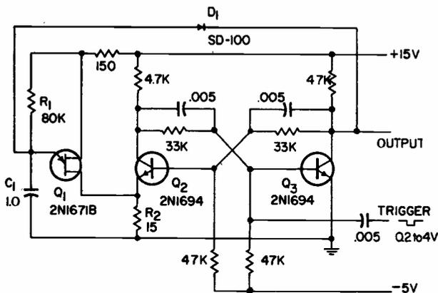
Timing interval of this circuit can be varied from 10 millisecond to 0.3 second.
