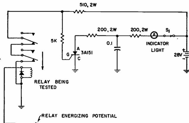
FIG. 1—Lamp lights if any relay contact opens for 0.1 microsecond.
