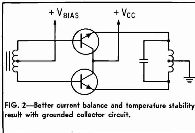
FIG. 2—Better current balance and temperature stability result with grounded collector circuit.
