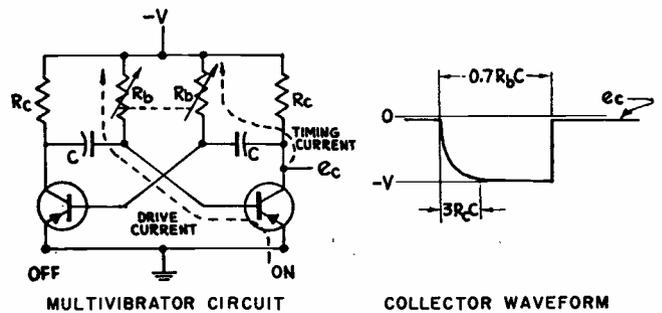
FIG. 1—Classical multivibrator circuit and its output waveform.
