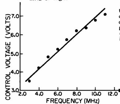
Fig. 2. Linearity is better than 5% of full-scale frequency. Above 5 MHz, frequency is approximately proportional to the product of control voltage and timing capacitance.
