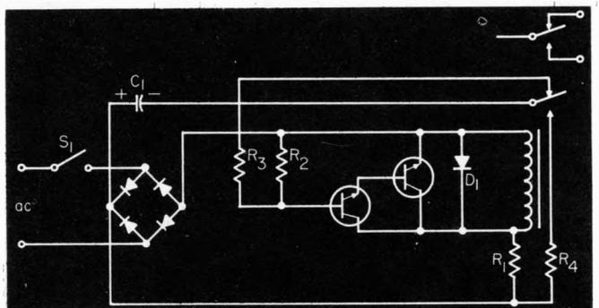
Fig. 2. In an improved circuit,  $C_1$  is rapidly discharged through  $R_4$ . Darlington connection gives increased gain and further reduces the size of  $C_1$ . A bridge rectifier allows ac operation.
