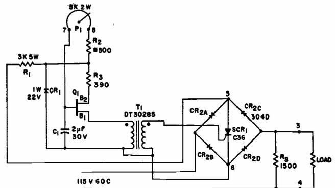
FIG. 1—Full-wave output is provided with one unijunction trigger and one controlled rectifier.
