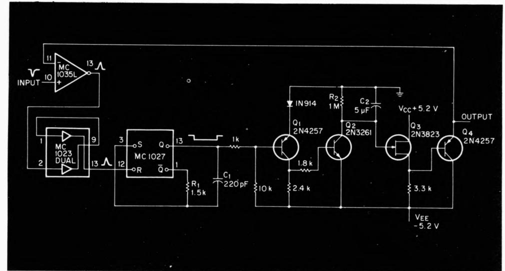
Fig. 1. This circuit responds to the peak amplitude of narrow pulses and is insensitive to their widths.
