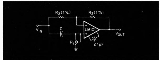
This IC-phase shifter produces 0 to 180° with a constant-amplitude output.
