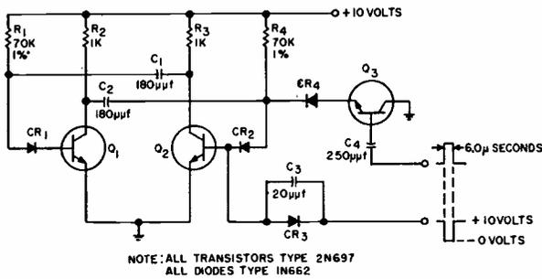
Fig. 1—Synchronized oscillator.
