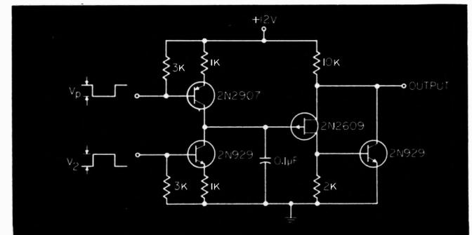
Fig. 2. Simplified pulse integrator with typical component values.
