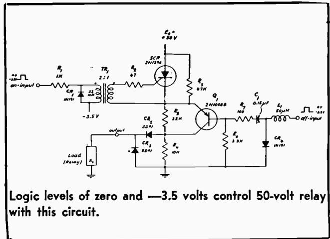
Logic levels of zero and  $-3.5$  volts control 50-volt relay with this circuit.
