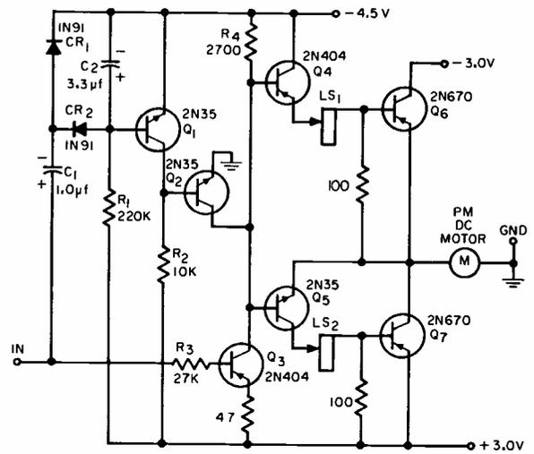
Fig. 1. Pulse absence detector and actuator amplifier.
