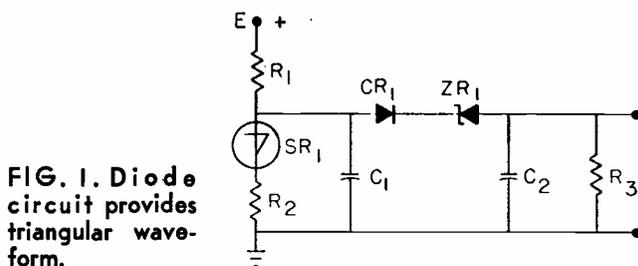
FIG. 1. Diode circuit provides triangular waveform.
