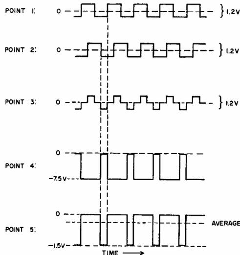
Fig. 2. Waveforms in phase comparator.
