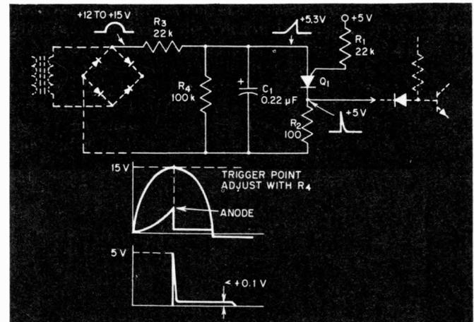
This simple and inexpensive circuit provides a reliable sync pulse from the 60-Hz power line.
