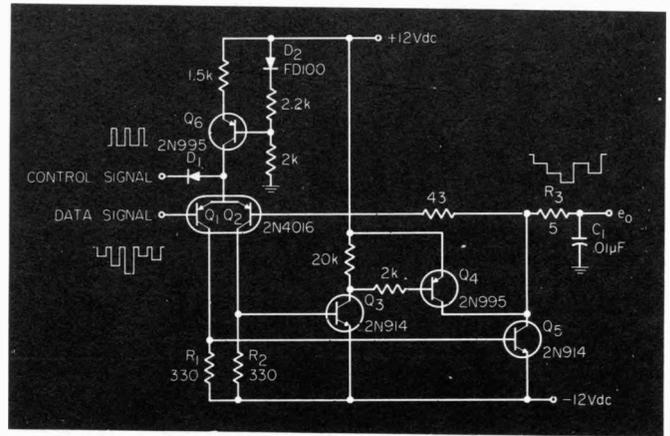
**Fast and accurate sample-and-hold circuit.** Matched transistors ( $Q_1, Q_2$ ) give low offset between the sampled input and held output.
