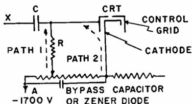
FIG. 2—Transient current paths in a c-r tube.
