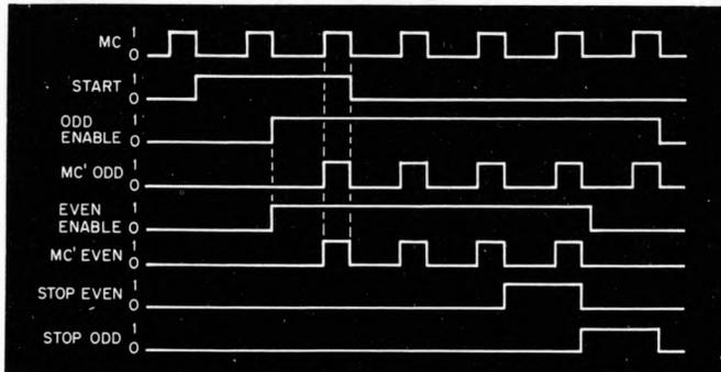
Fig. 5. Timing diagram for the 7-bit split adder.
