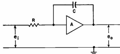
FIG. 1—Basic feedback circuit.
