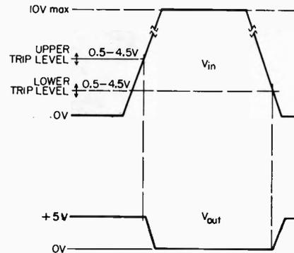
Fig. 2. When the input voltage exceeds the upper trip level, the output voltage drops to its low state. Later, when the input voltage falls below the lower trip point, the output voltage is restored to its high state.
