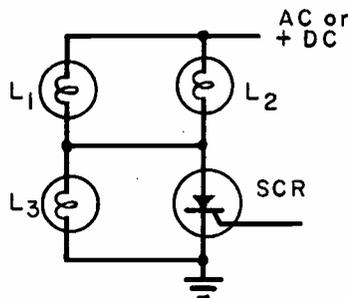
Fig. 1. Basic inversion circuit for incandescent lamp readout.
