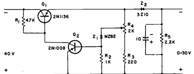
FIG. 2—Simple regulator provides zero to 30 volts output.
