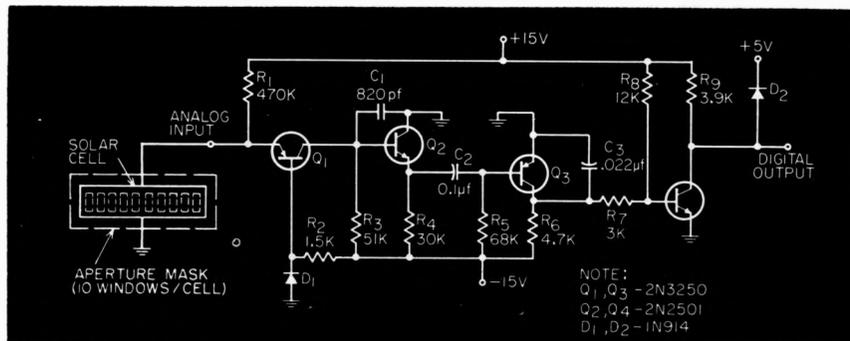
Fig. 1. Solar-cell amplifier for reading punched cards.
