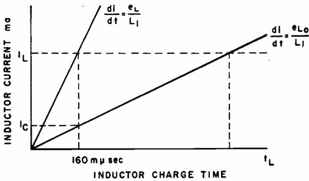
FIG. 2—Graph shows advantages of positive emitter circuit.
