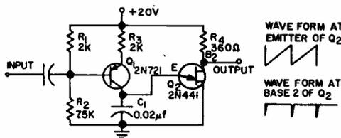
The output frequency is determined by the time needed for constant-current source  $Q_1$  to charge  $C_1$  to the peak-point voltage of UJT  $Q_2$ .
