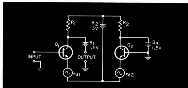
Fig. 1. Simplified circuit showing floating power supply.
