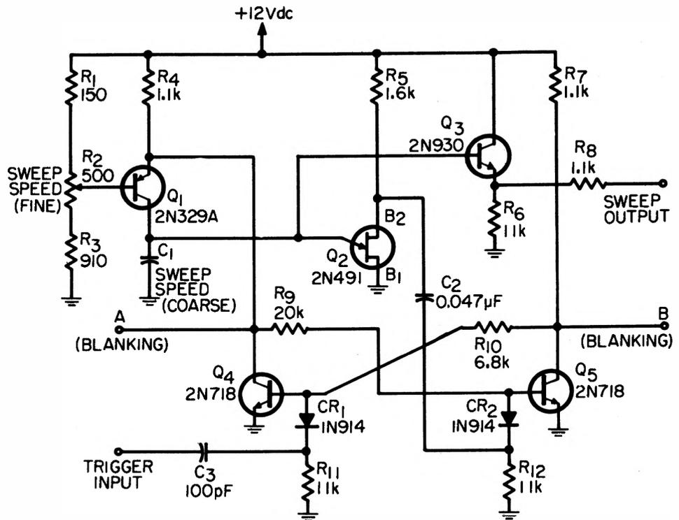
Fig. 1. Flip-flop ( $Q_4$ ,  $Q_5$ ) in this sweep generator allows a single sweep output for each trigger pulse. Positive and negative blanking pulses are generated at points A and B respectively.
