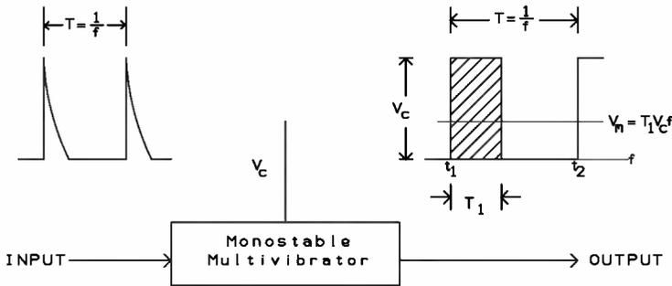
Fig. 1. Voltage-controlled one-shot multivibrator gives output pulses of constant width and variable height. Total period  $T$  is the reciprocal of input frequency, therefore mean output voltage is proportional to the product of  $f$  and  $V_c$ .
