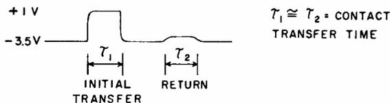
FIG. 1—Pulse generator is driven by switch transient.
