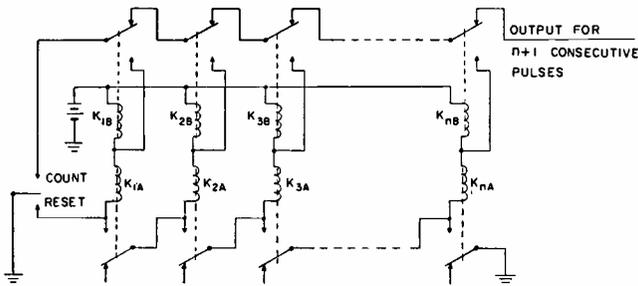
Counter relay chain provides low-cost fail-safe operation.
