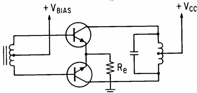
FIG. 1—Conventional circuit for driving servo motors.
