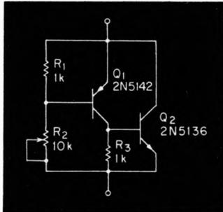
This circuit is particularly useful in the 1- to 3-V range, where conventional zeners have much higher impedance.
