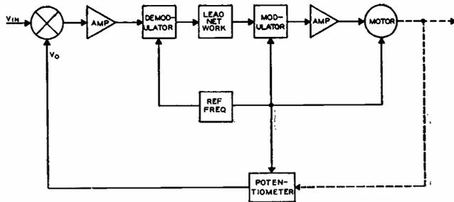
FIG. 1—Servo using demodulator and lead network stabilization.
