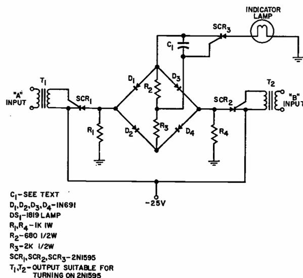
Fig. 3—Anti-Coincidence Detector.
