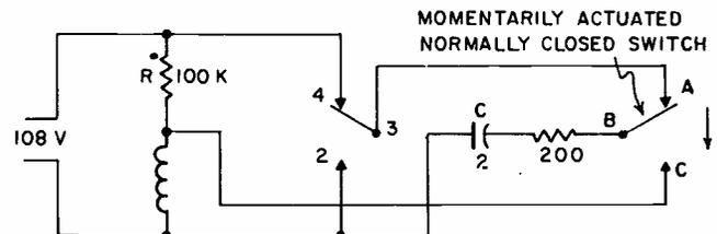
Switch actuated by machine tool operates binary counter relay.
