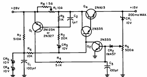
Overload cut-out current level is adjustable with  $R_1$ .
