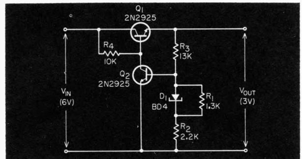
Fig. 2. Series regulated power supply with backward-diode reference.
