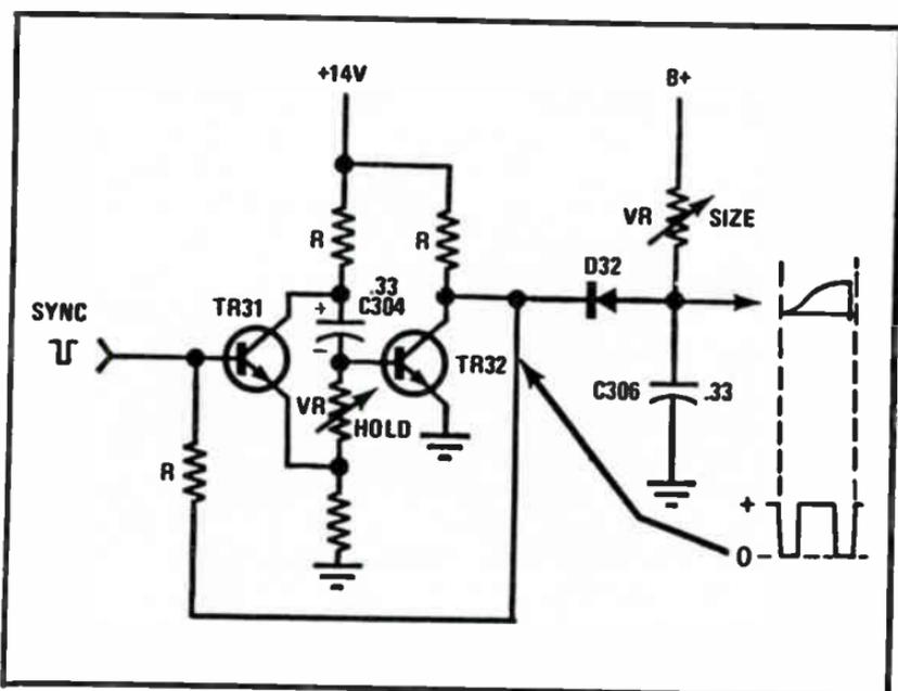
Fig. 4-1. Transistor type vertical oscillator circuit.
