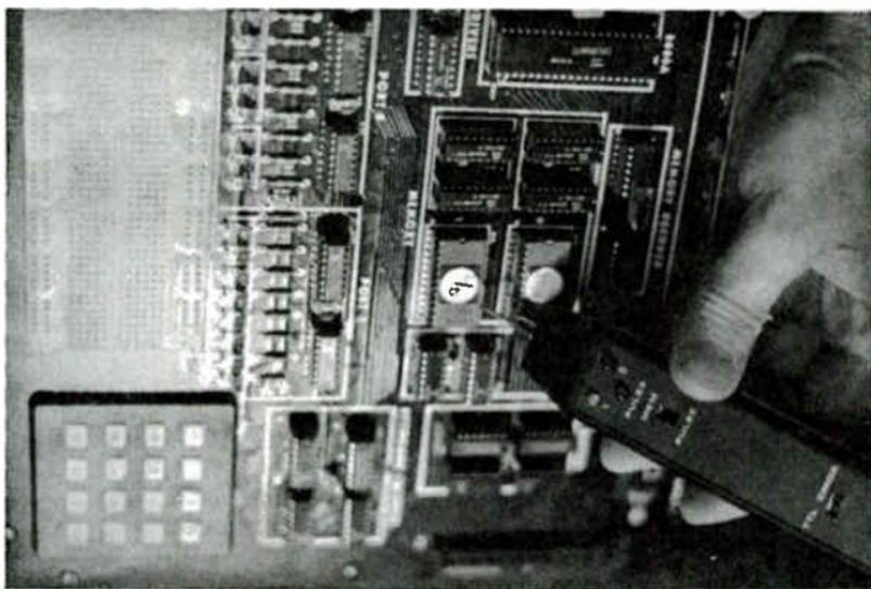
Fig. 6-13. B & K DP-50 Logic Probe.
