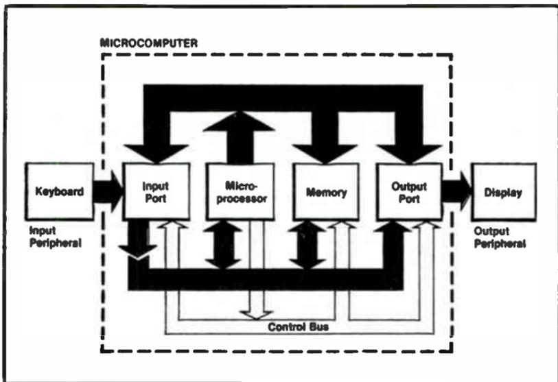
Fig. 12-1. Block diagram of microprocessor system.
