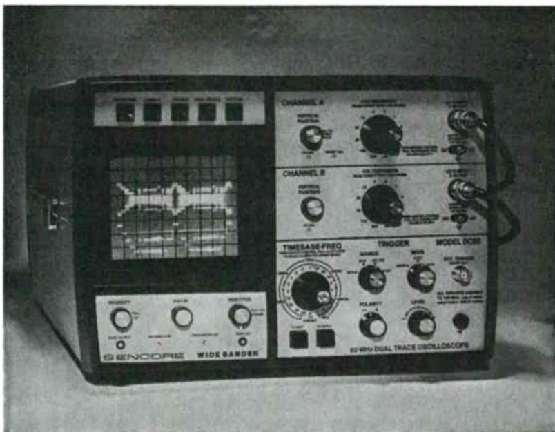
Fig. 5-19. SENCORE model SC60 dual-trace oscilloscope.
