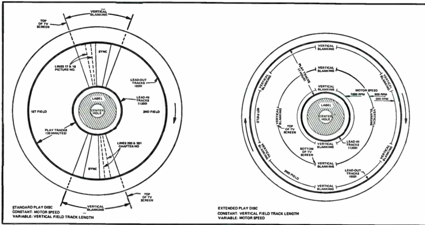
Fig. 11-5. Comparison of video discs.
