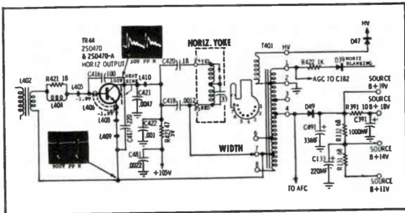
Fig. 4-5. Horizontal sweep output stage.
