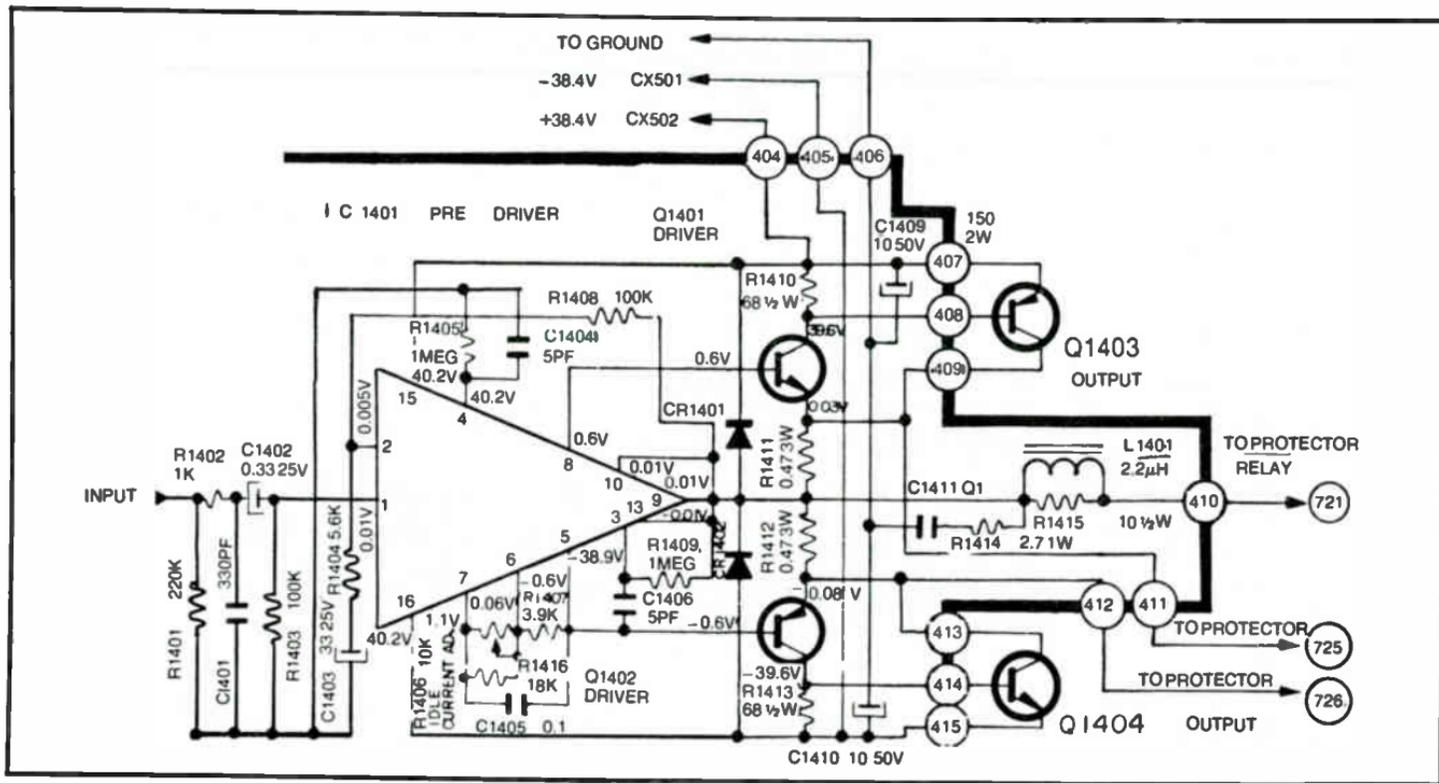
Fig. 5-14. Audio amplifier output circuit (IC).
