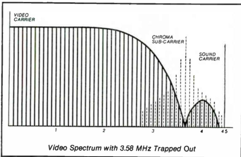
Fig. 3-39. Trapped 3.58 MHz video spectrum drawing.
