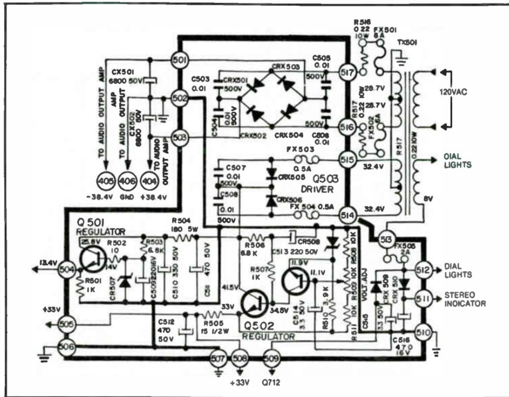
Fig. 5-16. Stereo receiver power supply circuit.
