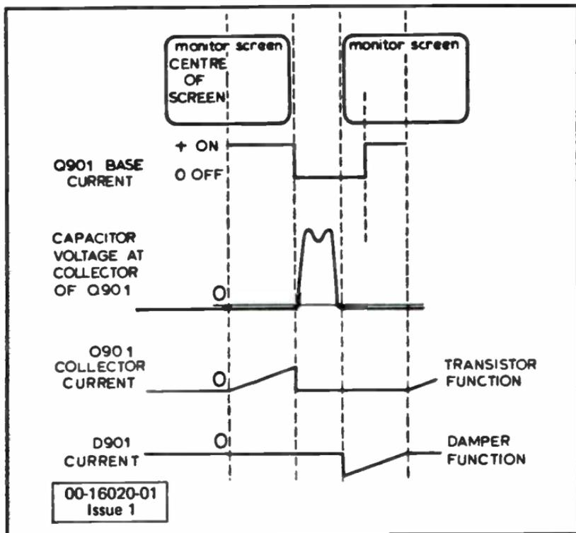
Fig. 4-14. Waveforms for horizontal scan system.
