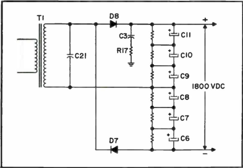
Fig. 11-7. Laser power supply circuit.
