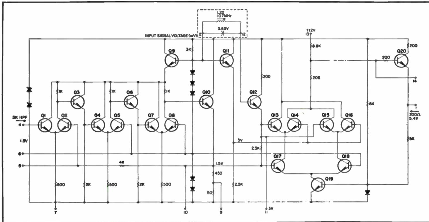
Fig. 5-5. Circuit inside FM detector IC.
