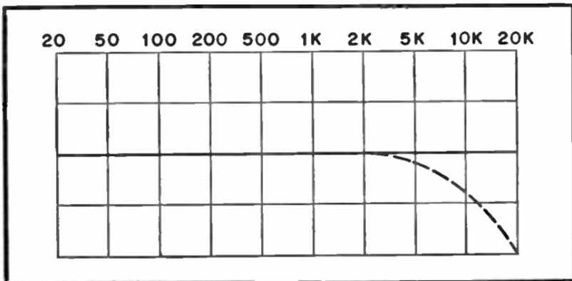
Fig. 7-8. Passive HI-CUT filter curve.
