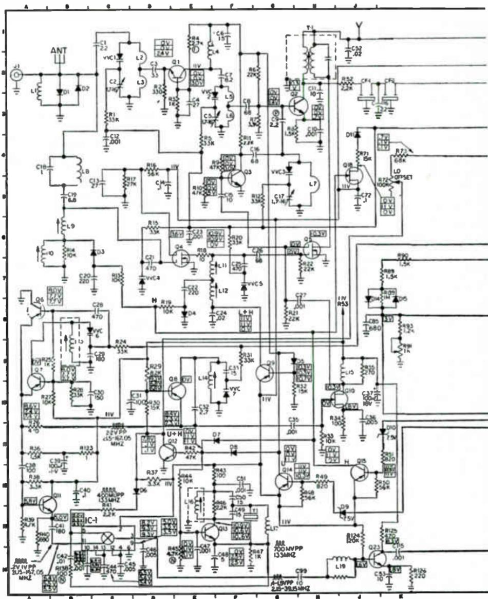
Fig. 8-7. Complete schematic for BEARCAT model BC250.
