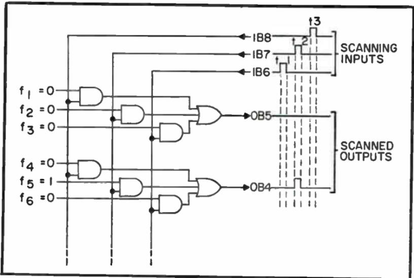
Fig. 2-7. Strobbed output logic.
