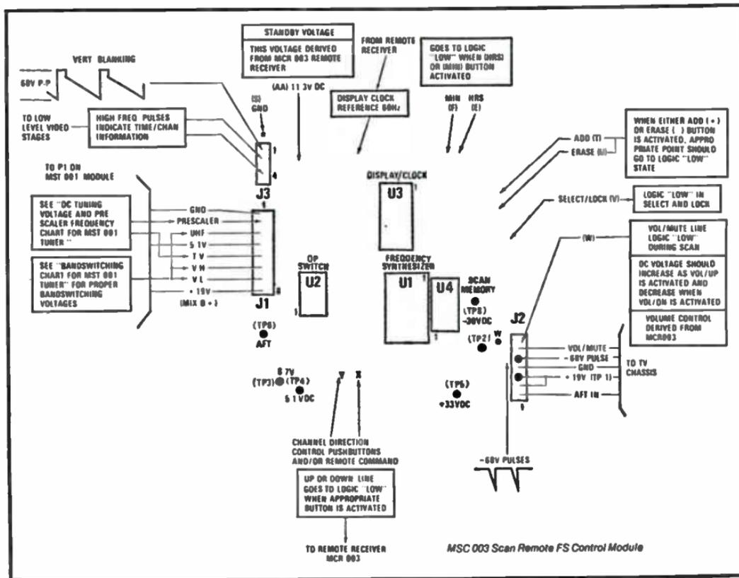
Fig. 2-8. RCA scan remote control module.
