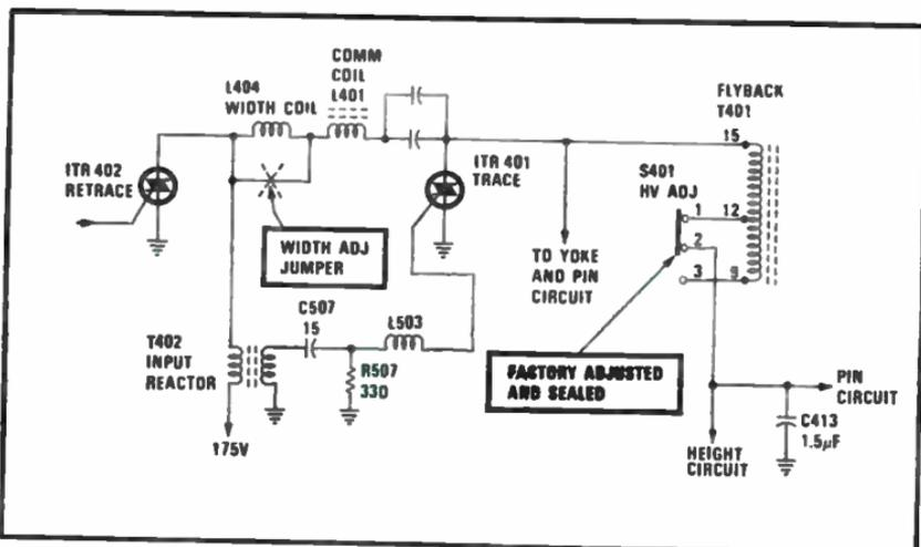
Fig. 3-31. Simplified horizontal deflection circuit.
