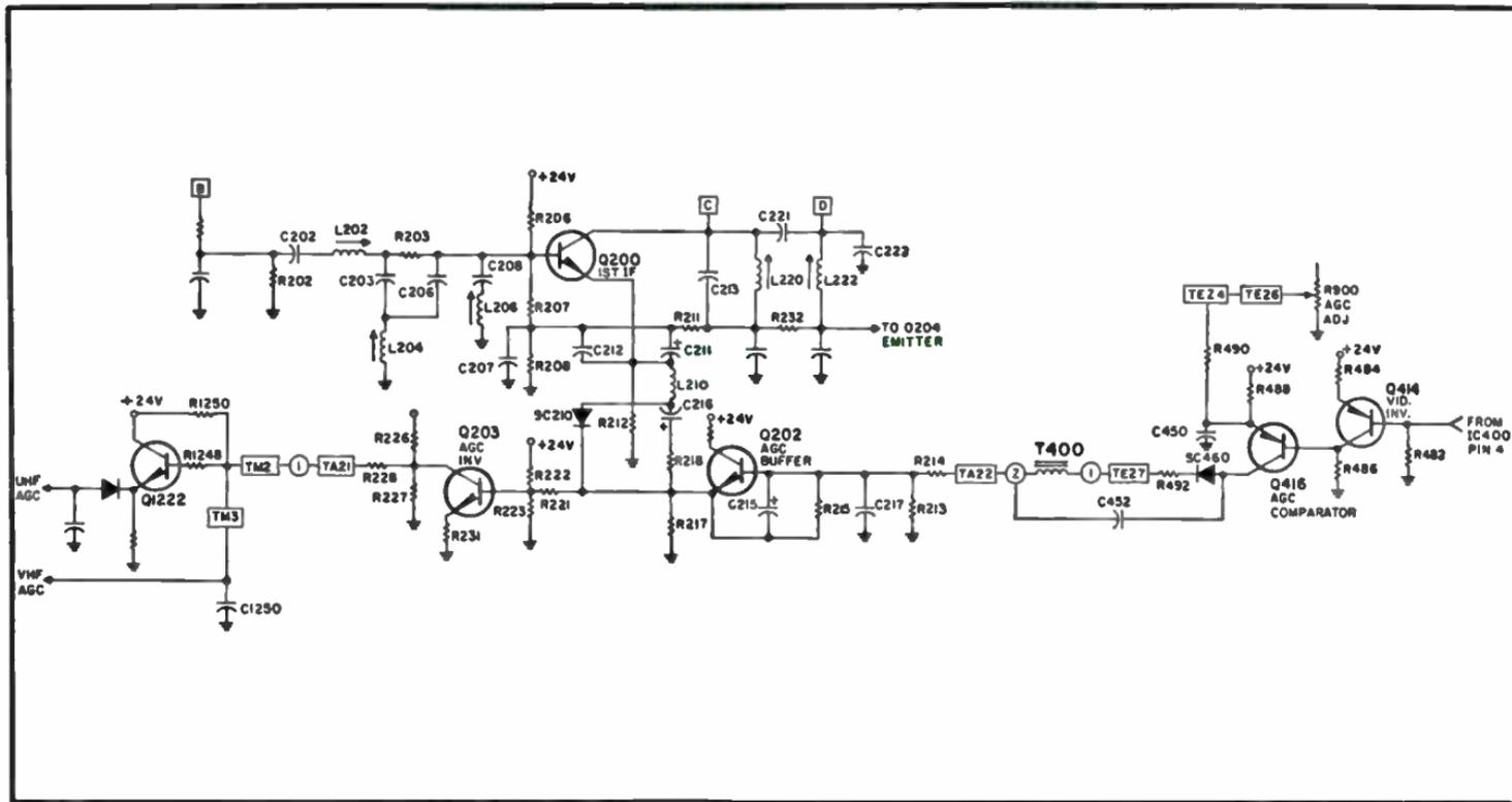
Fig. 3-49. Transistor AGC circuit.
