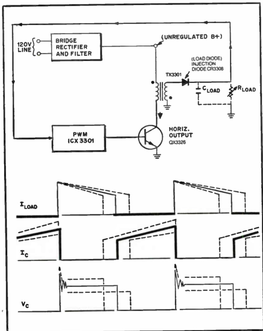
Fig. 3-53. Chopper circuit and waveforms.
