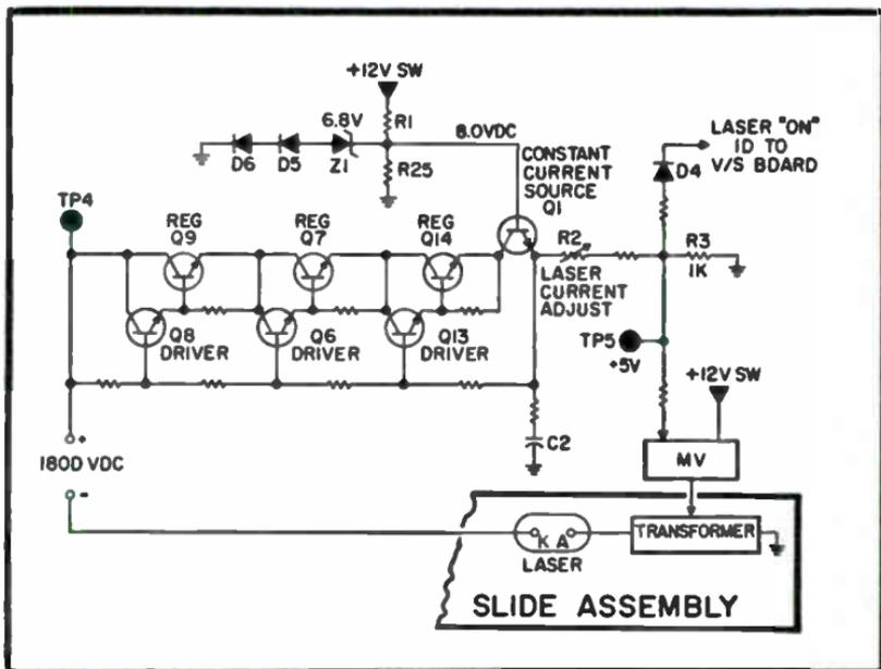
Fig. 11-9. Laser supply regulator circuit.
