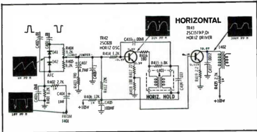
Fig. 4-4. Horizontal AFC and oscillator.
