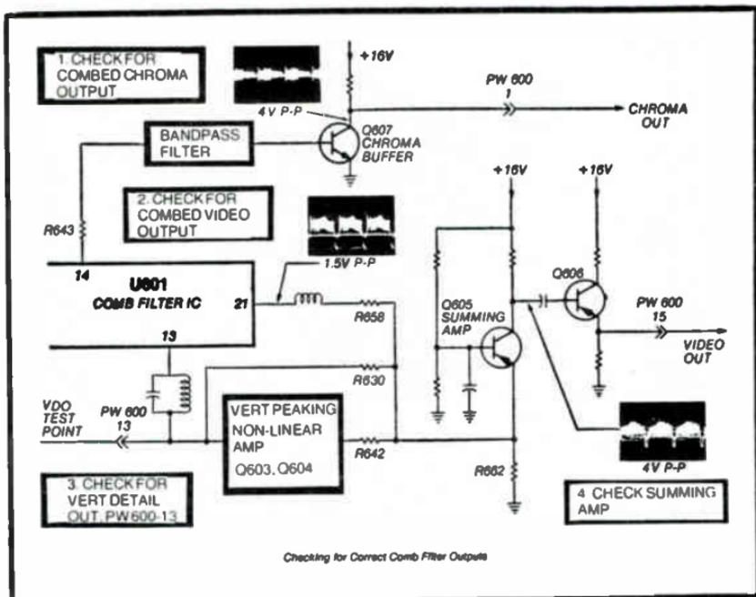
Fig. 3-41. Correct comb filter output signals.
