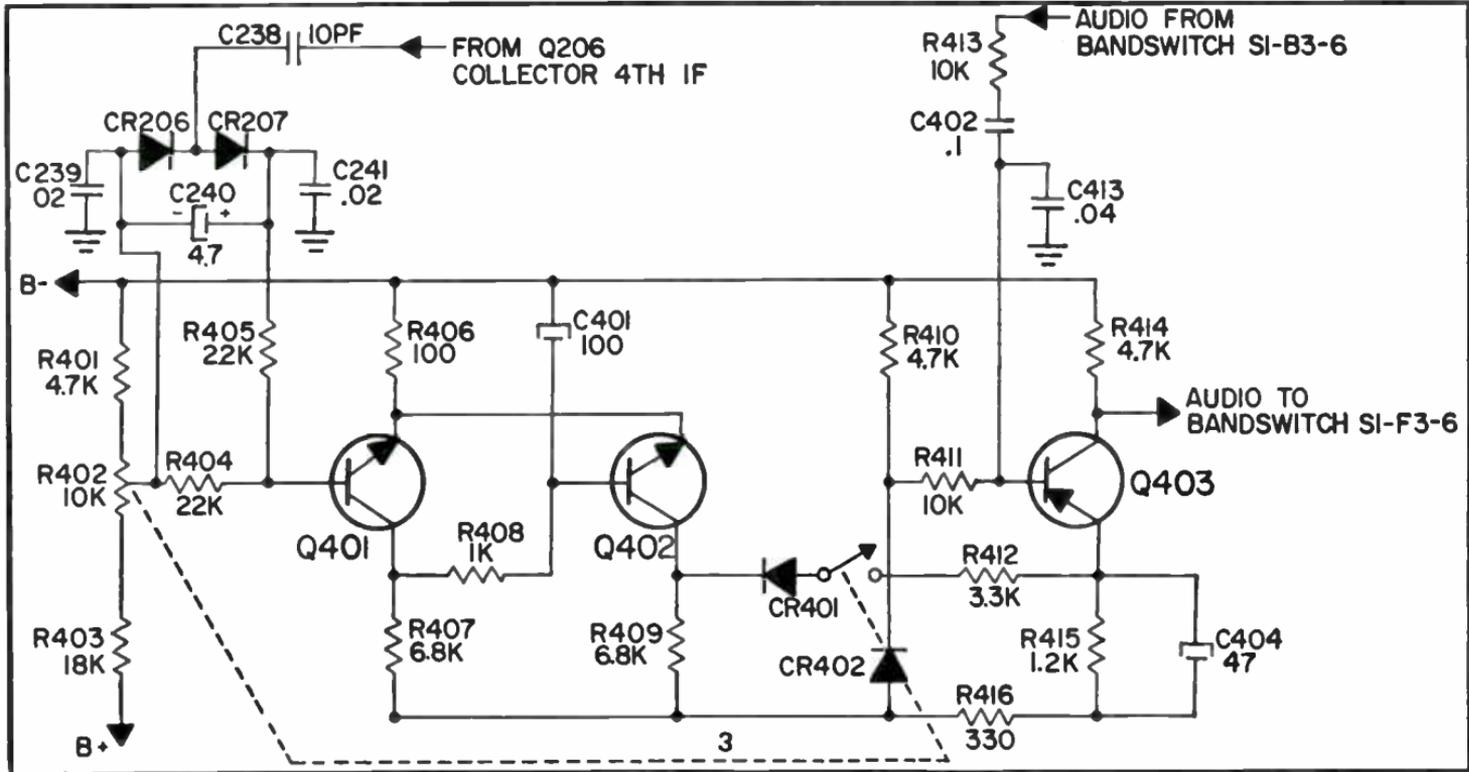
† Fig. 9-5. Transistor squelch circuit.
