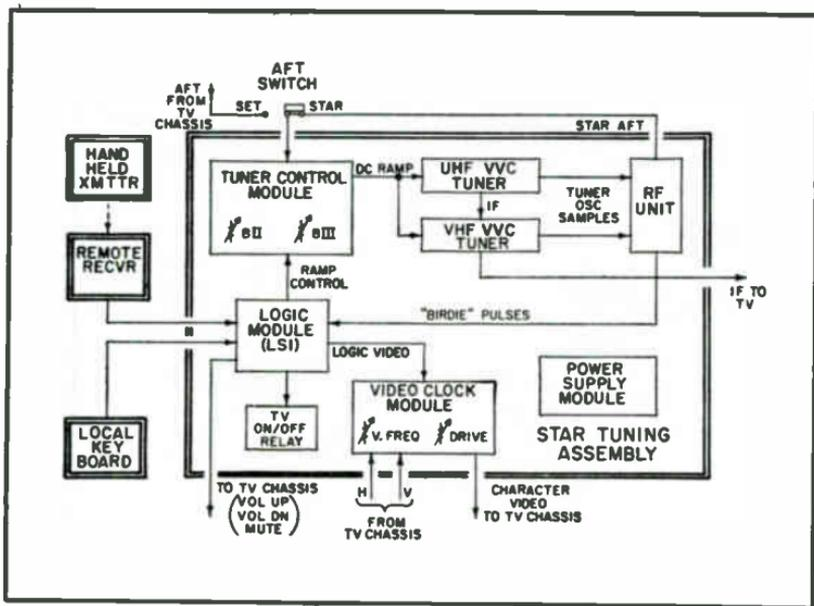
Fig. 2-11. Block diagram of Magnavox STAR remote system.
