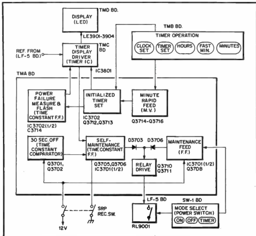
Fig. 10-17. Clock timer block diagram for KR9000 VCR.
