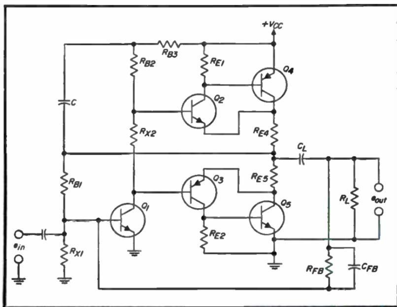
Fig. 5-18. Audio output circuit using complementary pairs.
