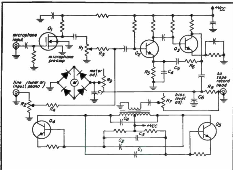
Fig. 7-1. Tape recorder pre-amplifier circuit.
