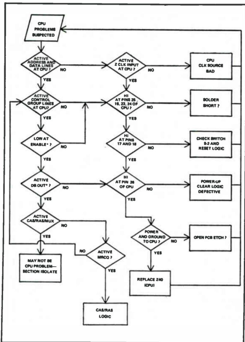
Fig. 12-19. CPU section isolation flowchart.
