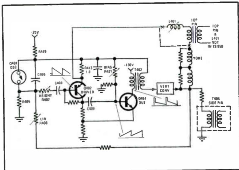
Fig. 3-69. Transistor type vertical sweep circuit.
