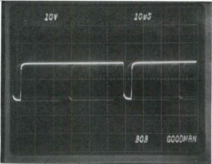
Fig. 3-18D. Horizontal sync pulses.
