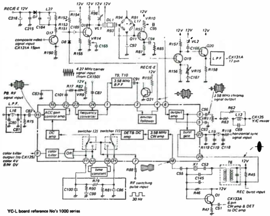
Fig. 10-13. Block diagram of CX136A chroma processor IC.
