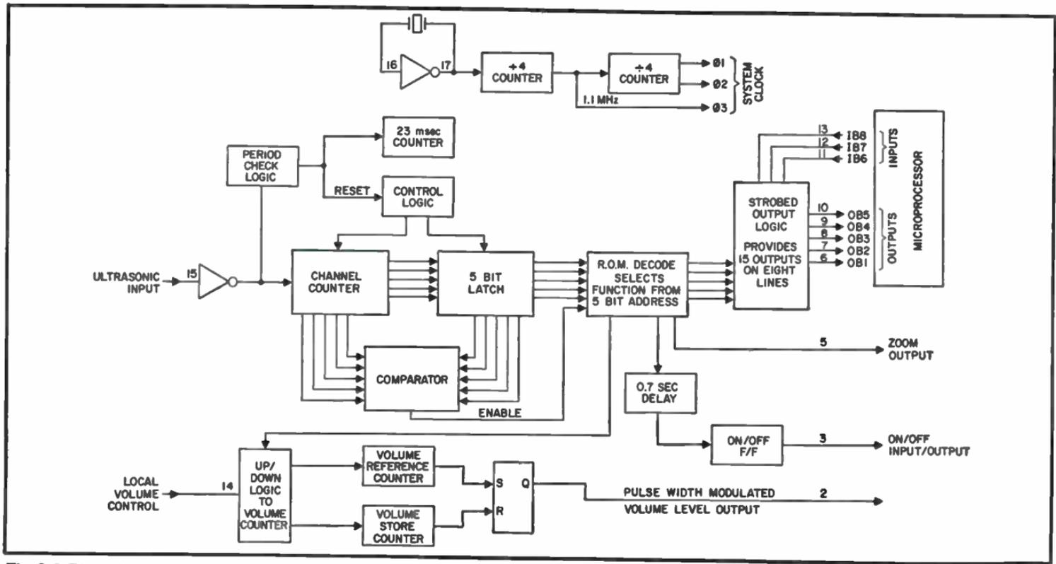
Fig. 2-6. Block diagram of IC201 in remote receiver.
