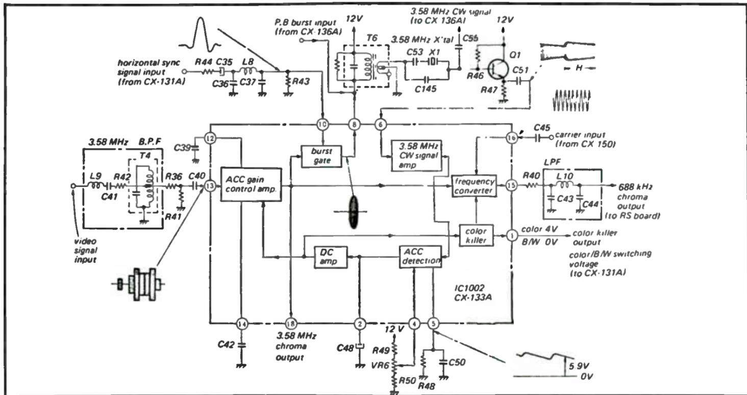
Fig. 10-9. Record chroma signal processing circuit.
