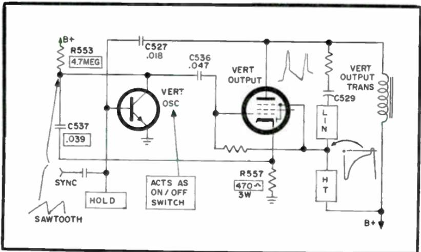
Fig. 3-7. Vertical sweep circuit with operational guide.
