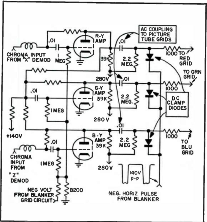
Fig. 3-44. Color difference amplifier circuits.
