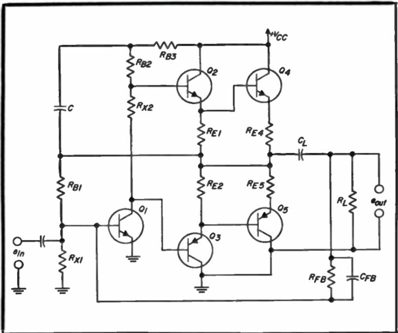
Fig. 5-17. Darlington pairs used in audio output circuit.
