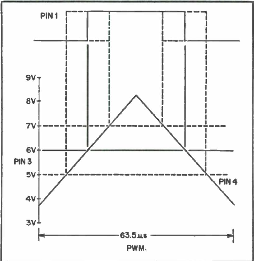
Fig. 3-60. Variations of transfer PWM characteristics.
