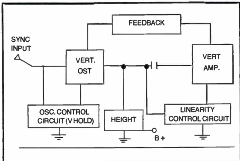
Fig. 3-9. Block diagram of plate-coupled vertical sweep system.
