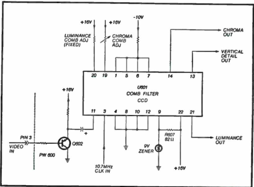
Fig. 3-38. Simplified comb filter diagram.
