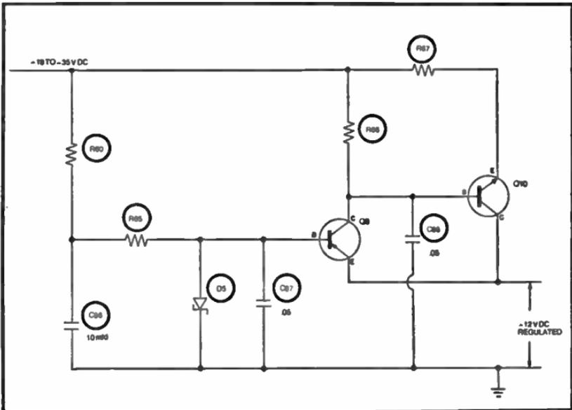
Fig. 5-3. Voltage regulator for stereo receiver.
