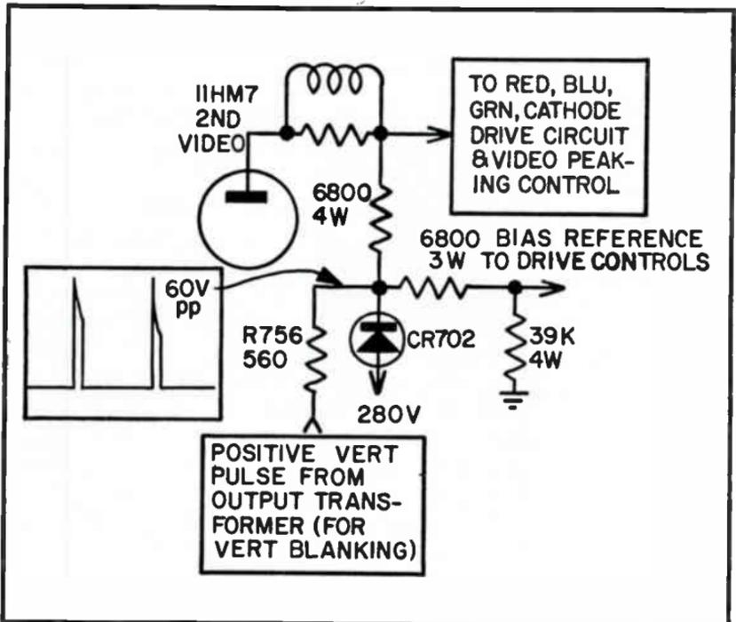
Fig. 3-43. Vertical retrace circuit.
