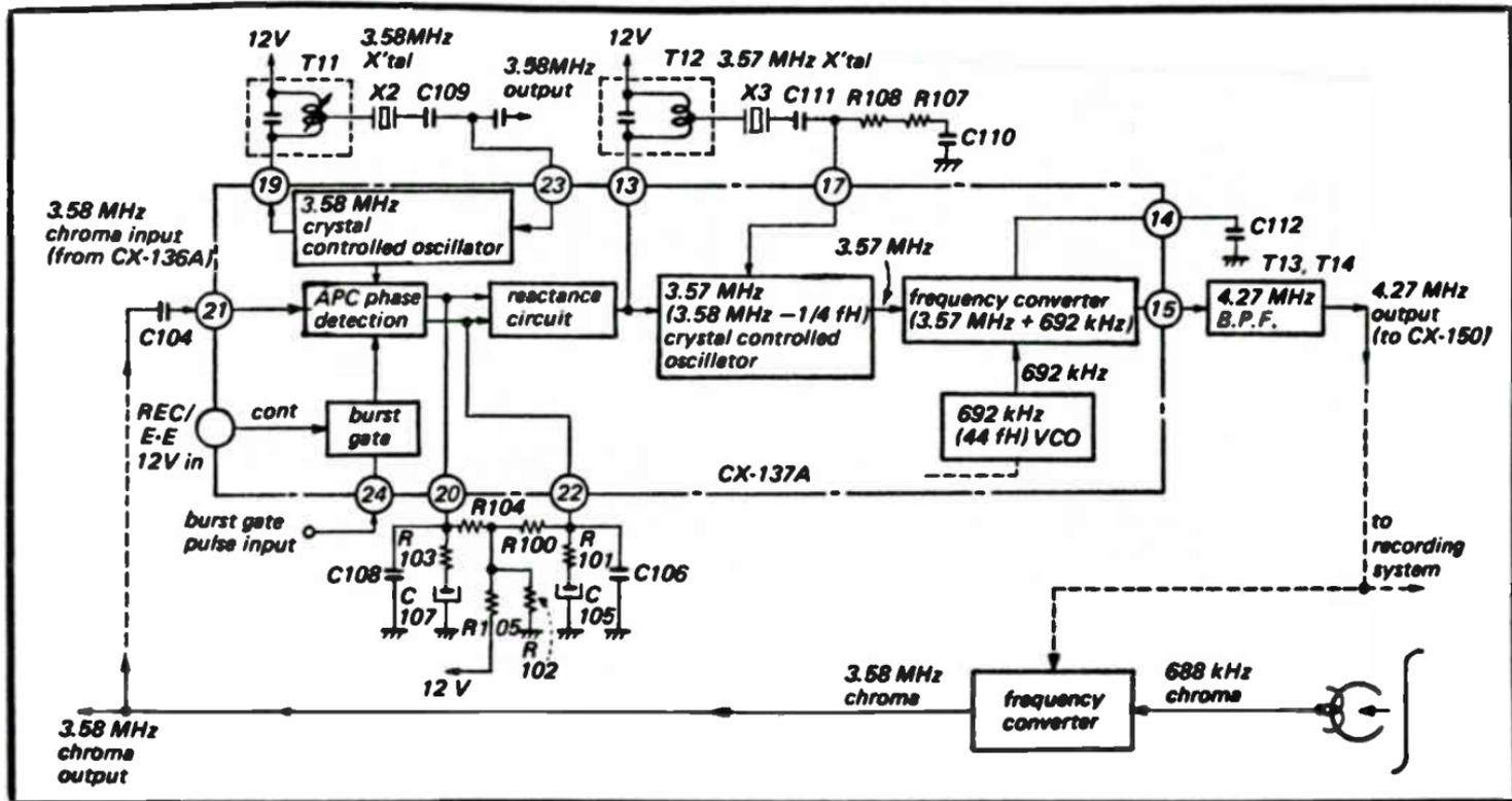
Fig. 10-7. Block diagram of APC circuit.
