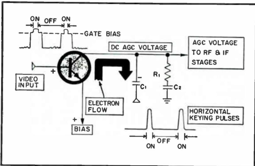
Fig. 3-47. Gated AGC amplifier circuit - simplified.
