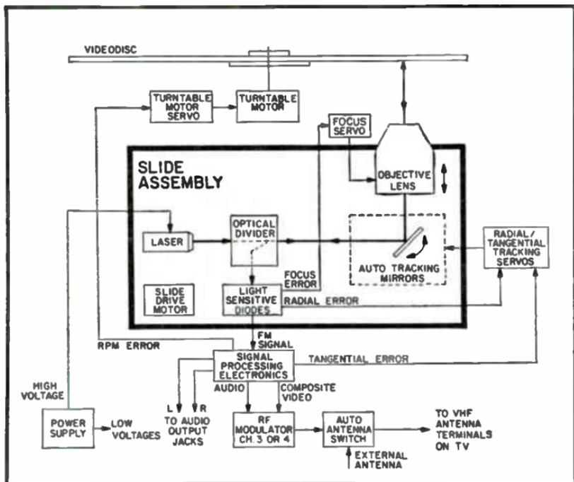
Fig. 11-6. Block diagram of disc player.
