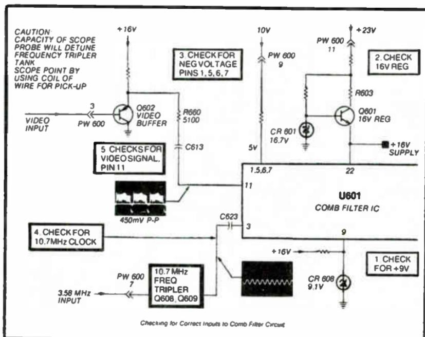
Fig. 3-40. Correct signal inputs of the comb filter.
