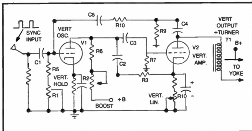
Fig. 3-10. Simplified diagram of a multivibrator.
