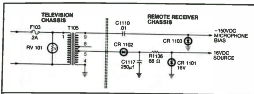
Fig. 2-9. Power supply circuit for remote receiver.
