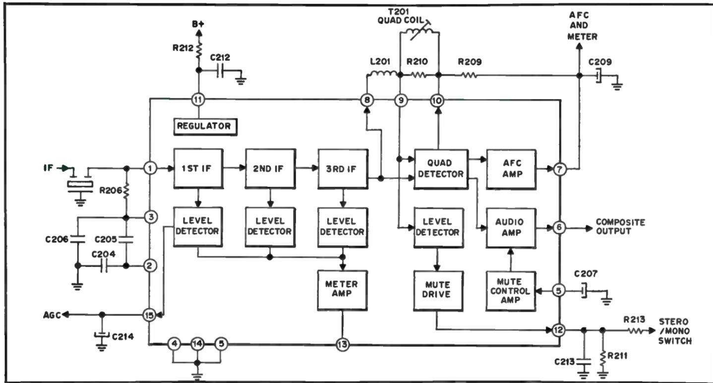
Fig. 5-8. Block diagram of FM IF chip.
