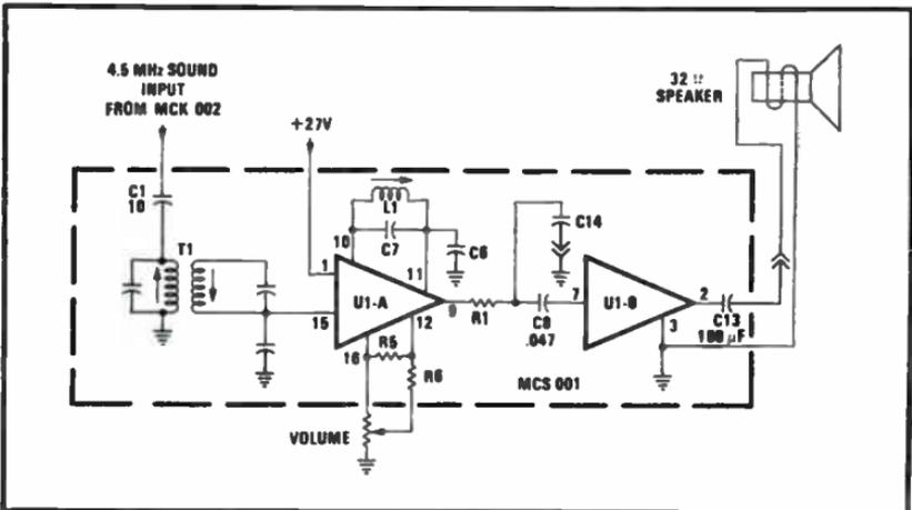
Fig. 3-45B. Simplified schematic MDS 001.
