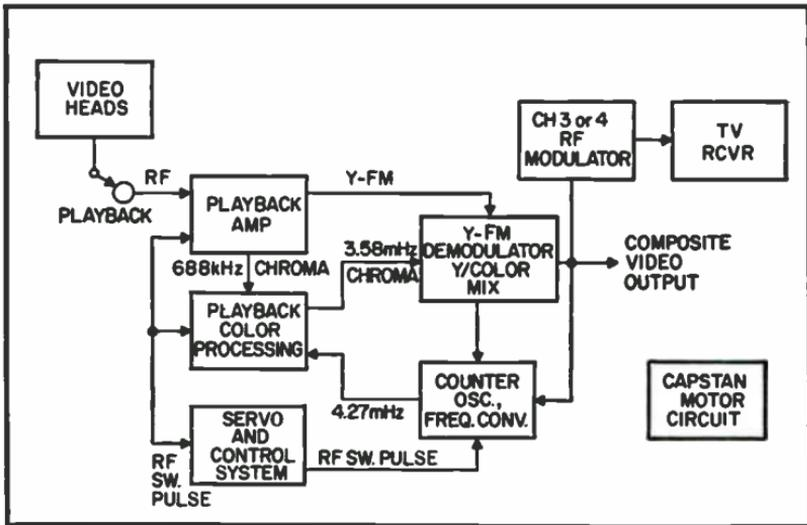
Fig. 10-6. Block diagram of playback mode.
