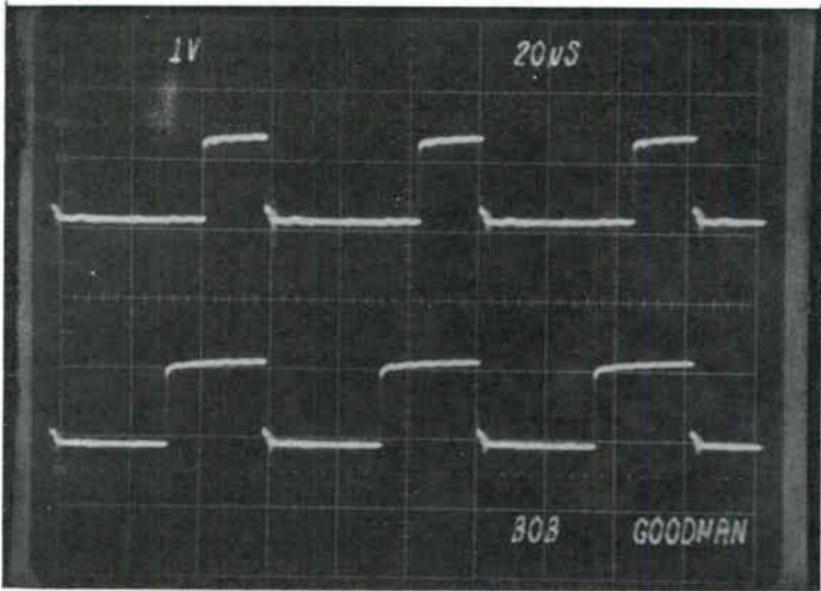
Fig. 3-61. Scope pulse illustration of pulse width modulator in action.
