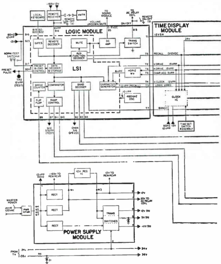
Fig. 2-14. Remote system signal flow block diagram.
