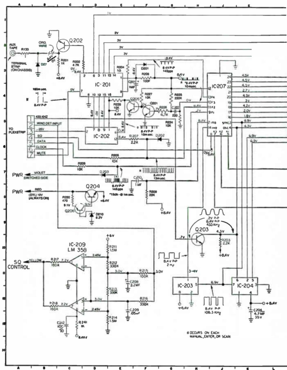
Fig. 8-5. Feature board circuit.
