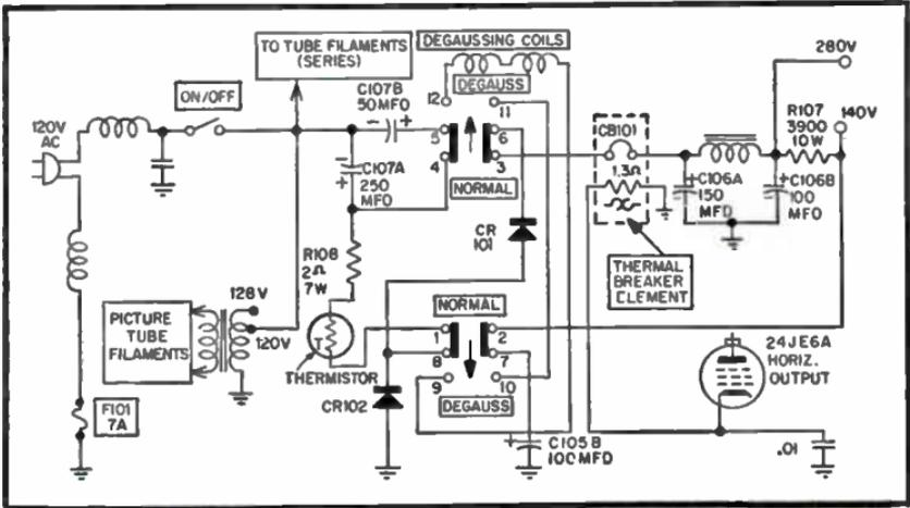
Fig. 3-27. Power supply and degauss circuit.
