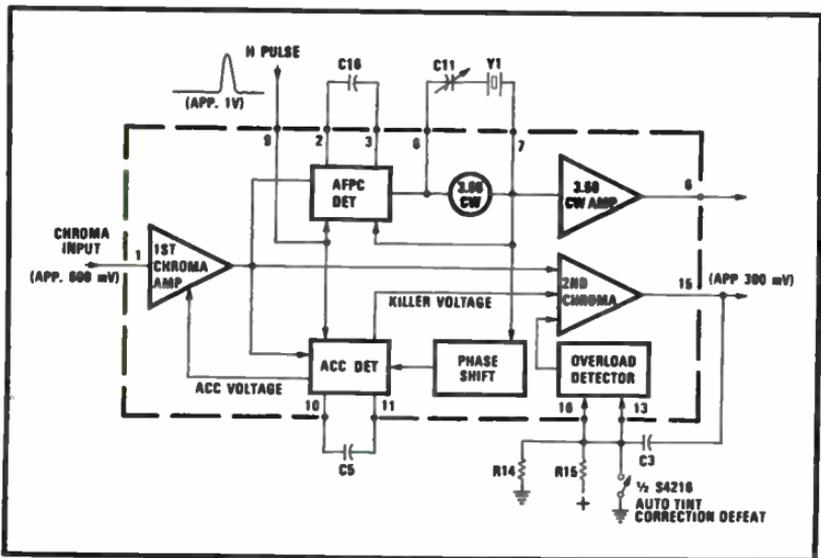
Fig. 3-36. Block diagram of chroma processor module.
