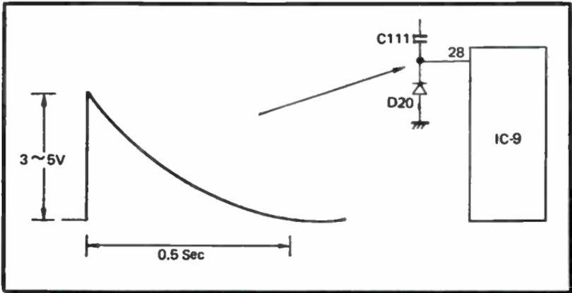
Fig. 8-11. Initializing waveform.
