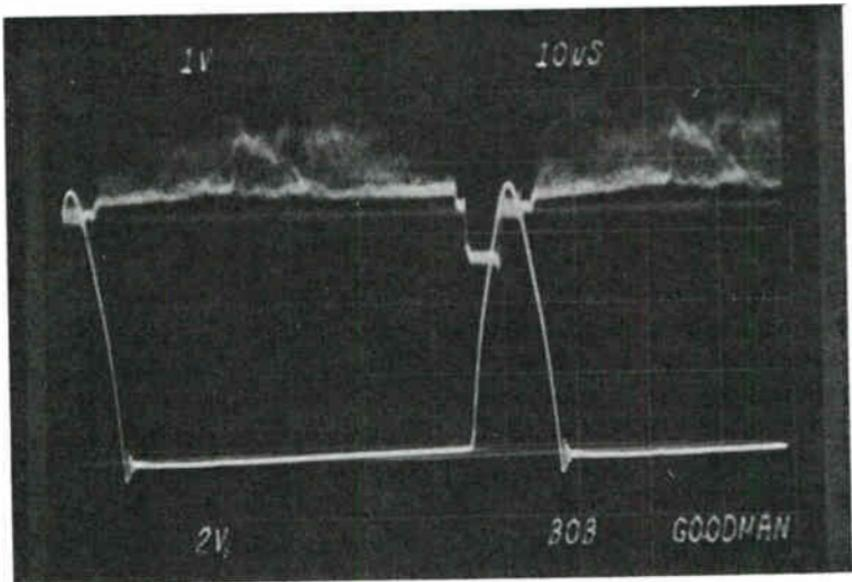
Fig. 3-22. Dual-trace scope showing mis-timed pulse.
