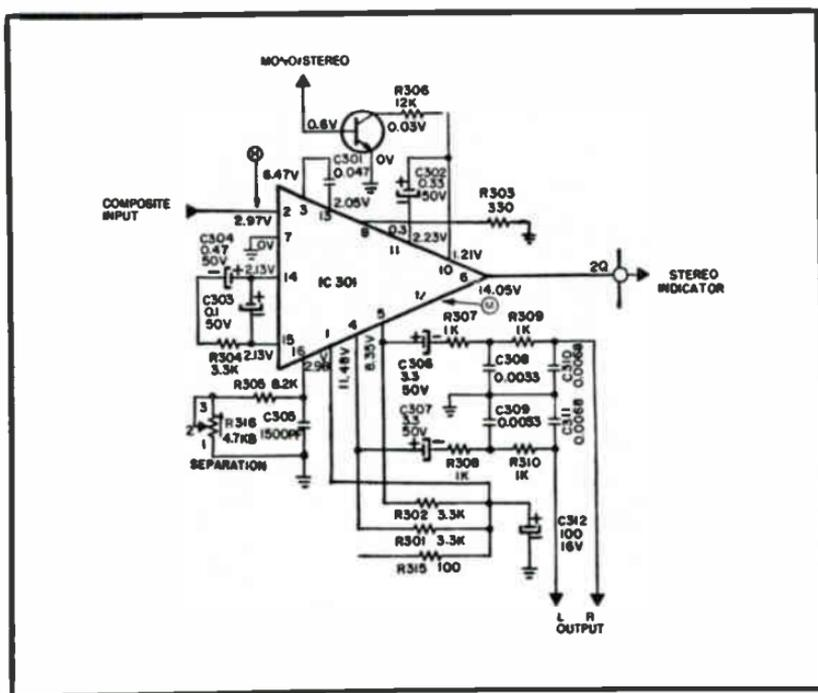
Fig. 5-10. FM Multiplex circuit (chip).
