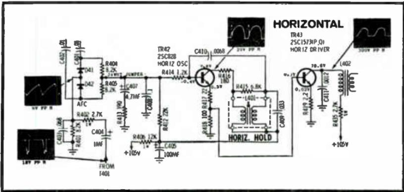
Fig. 4-11 Horizontal oscillator and driver circuit.
