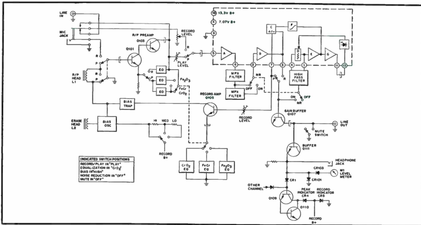
Fig. 7-6. Block diagram of a cassette tape recorder.
