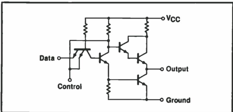
Fig. 12-4. Diagram of three-state driver.
