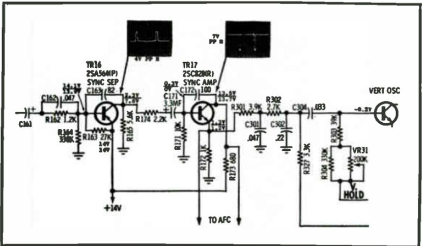
Fig. 4-8. Solid-state sync circuit.
