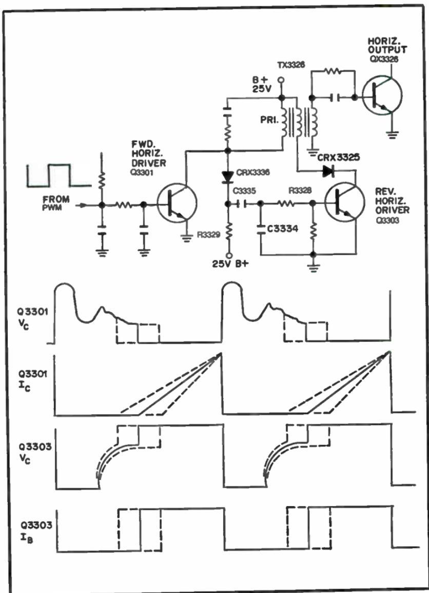
Fig. 3-55. Evolved chopper circuit and waveform.
