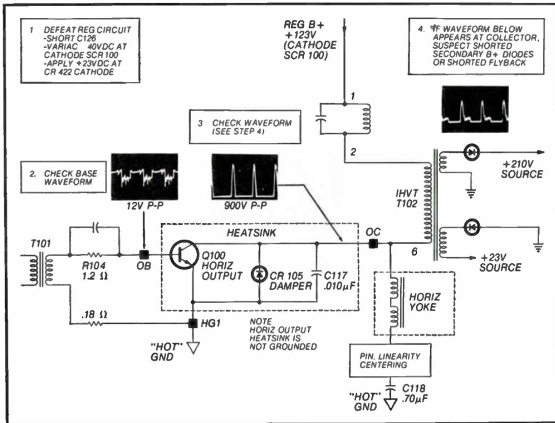
Fig. 3-5. Horizontal sweep output with scope waveforms.
