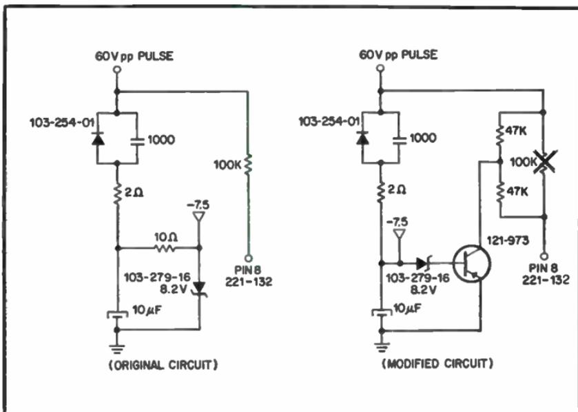
Fig. 3-62. Modification of horizontal output circuit.
