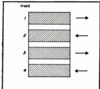
Fig. 7-3. Directions tape tracks are recorded.
