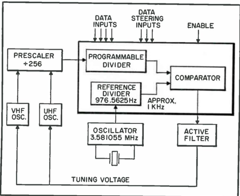
Fig. 1-4. Phase locked-loop block diagram.
