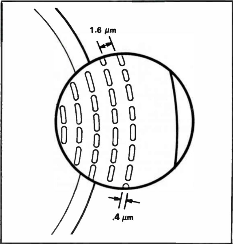
Fig. 11-1. Magnified view of a video disc track.
