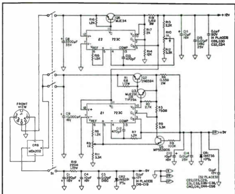
Fig. 12-16. Power supply circuit.
