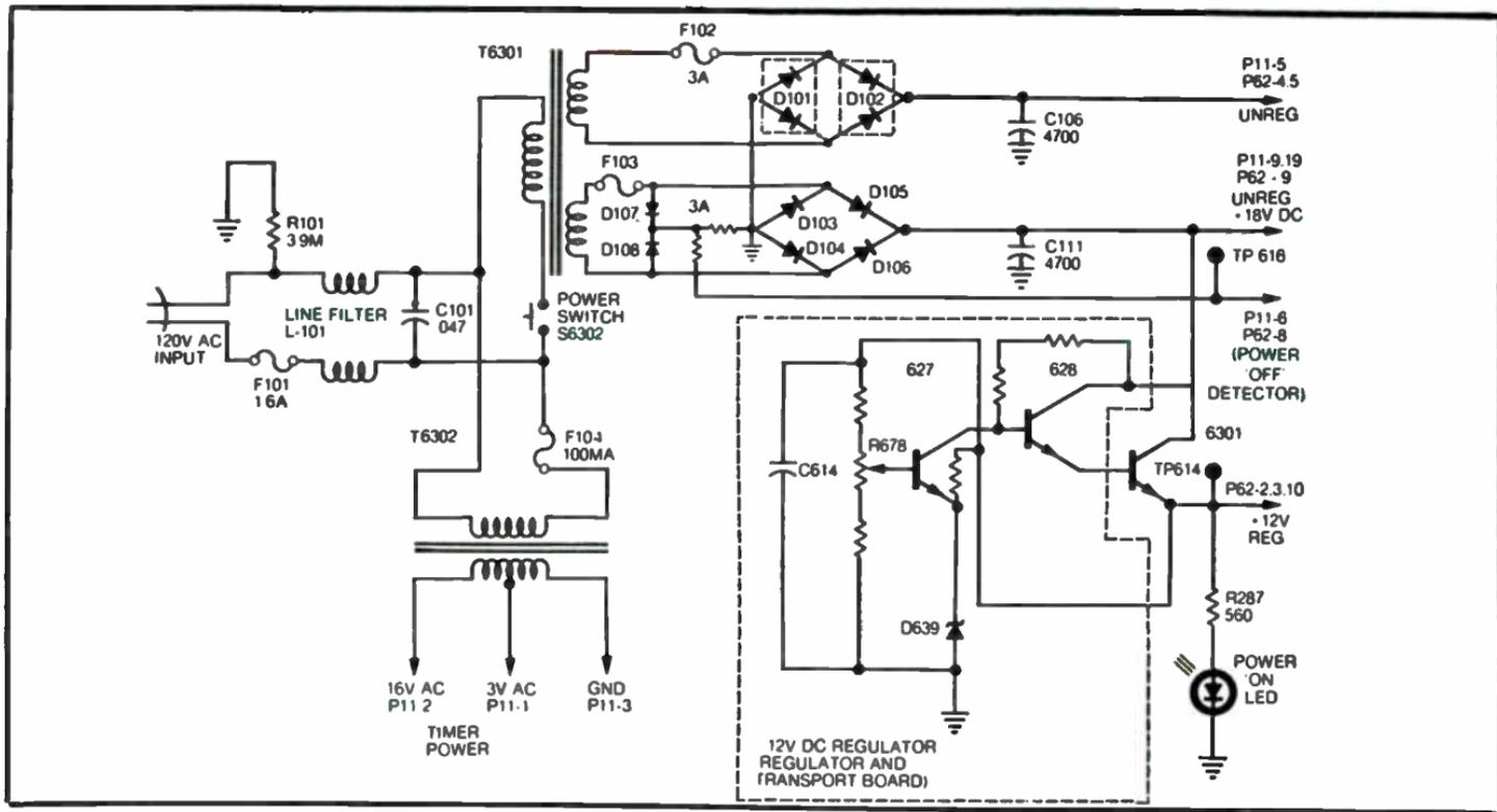
Fig. 10-1. Power supply circuit with +12 volt regulator.
