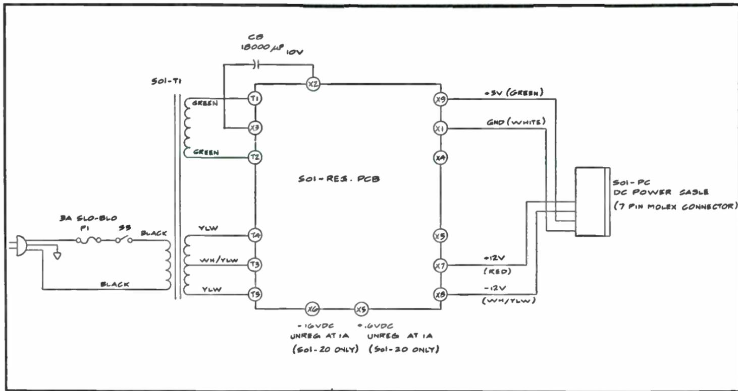
Fig. 12-21. SOL-10 power supply block diagram.
