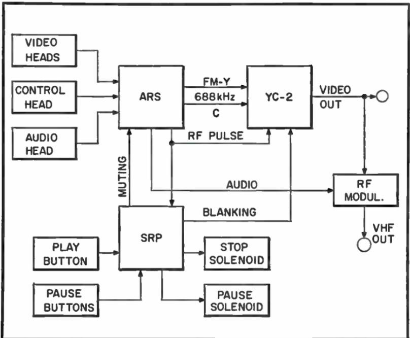
Fig. 10-15. Block diagram of KR9000 units playback mode.
