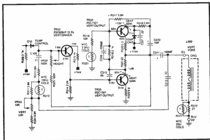
Fig. 4-3. Vertical output and driver circuit.
