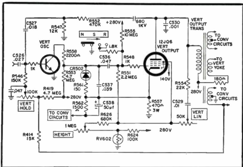
Fig. 3-8. Vertical oscillator and output circuit.
