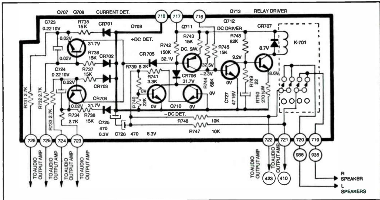
Fig. 5-15. Automatic speaker protection circuit.
