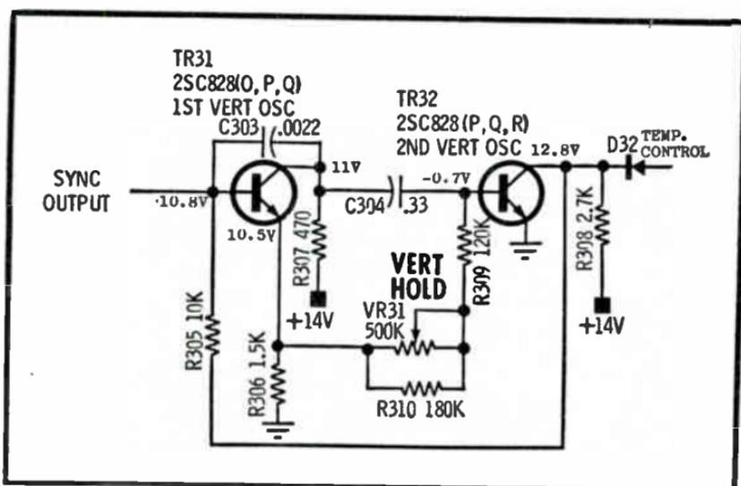
Fig. 4-2. Vertical oscillator and sawformer.
