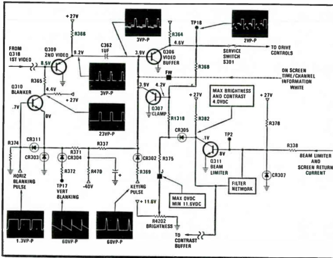
Fig. 3-25. Low-level video stage with scope waveforms.
