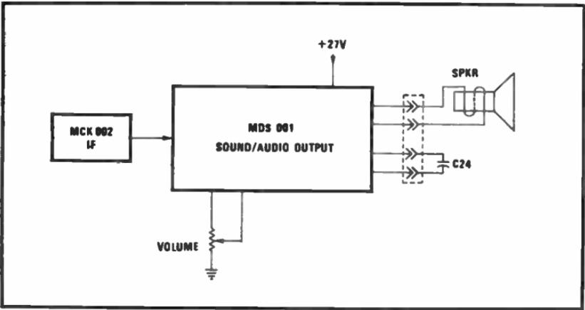
Fig. 3-45A. Block diagram of IC sound circuit.
