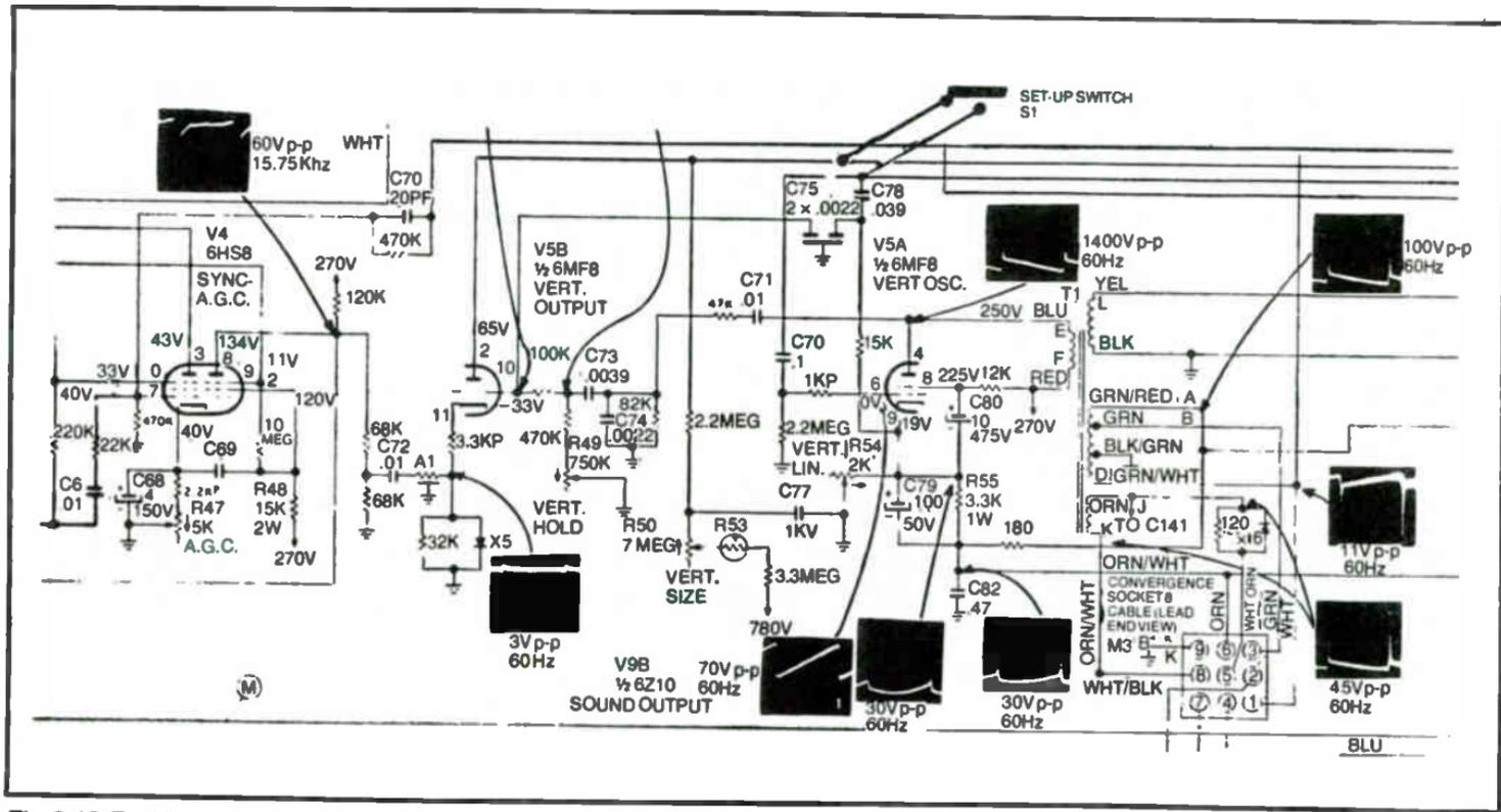
Fig. 3-12. Zenith vertical sweep circuit.
