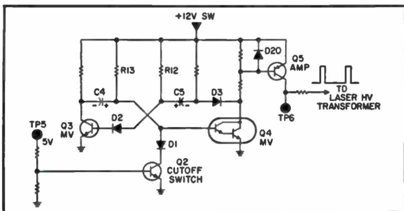
Fig. 11-10. Laser multivibrator circuit.
