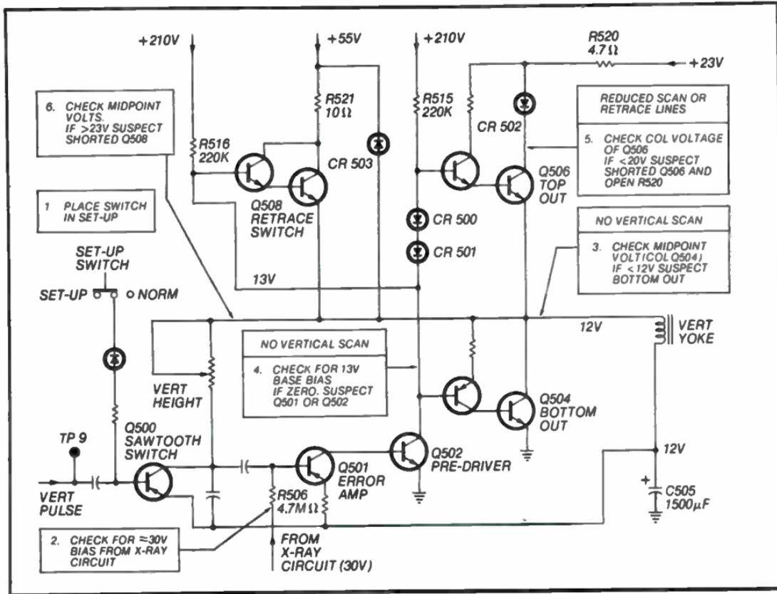
Fig. 3-4. Vertical amplifier circuit with check point call-outs.
