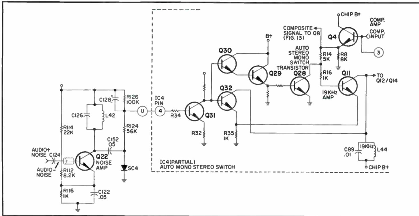
Fig. 5-4. Mono/Stereo IC4 auto switching circuit.
