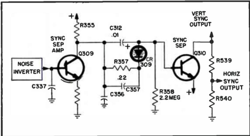
Fig. 3-46. Transistor sync separator circuit.
