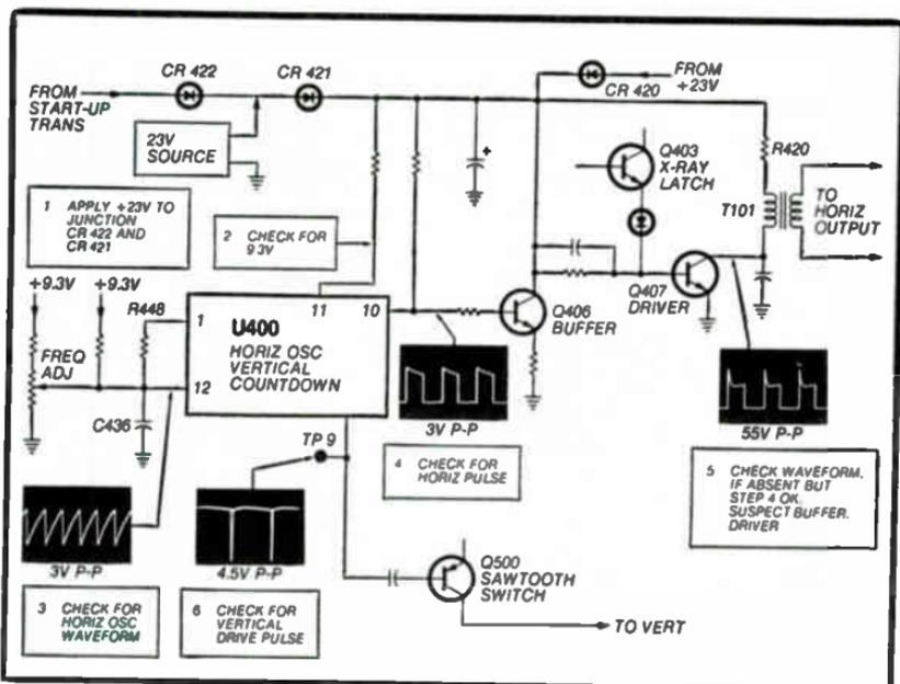
Fig. 3-3. Count-down circuit with waveform checkpoints.
