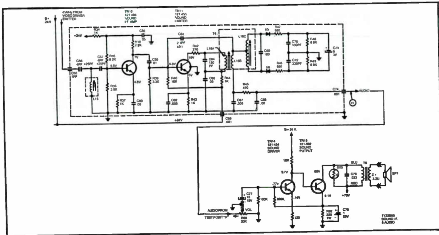
Fig. 4-20. Audio IF and sound output circuits.
