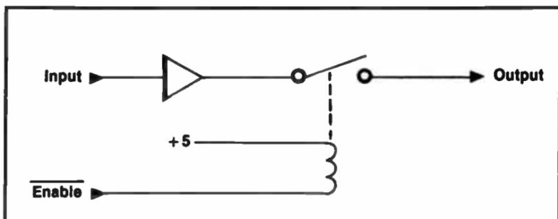
Fig. 12-3. Equivalent Three-State Driver.
