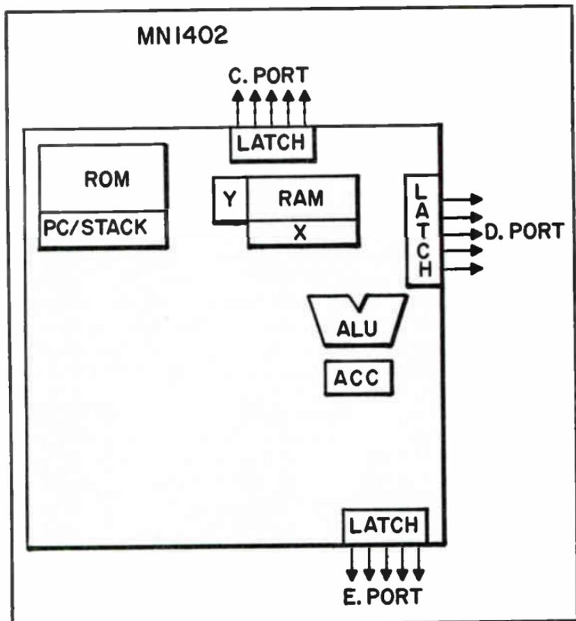
Fig. 1-6. Microprocessor organization diagram.
