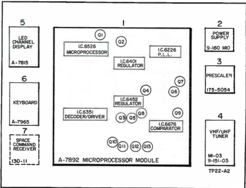
Fig. 1-2. Direct access system block diagram.
