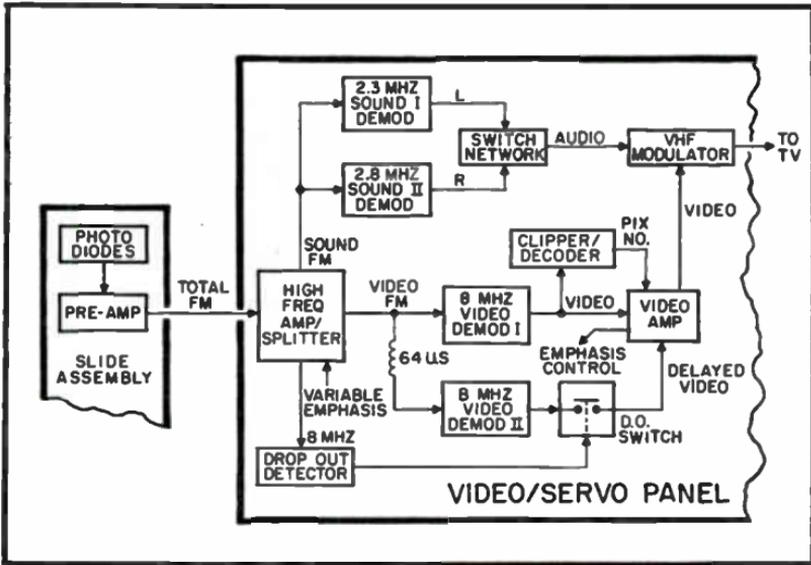
Fig. 11-12. Signal processing block diagram.
