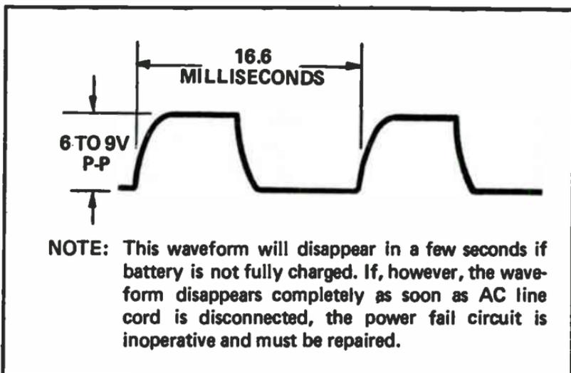
Fig. 9-3. Correct waveform change after radio is unplugged for two seconds.
