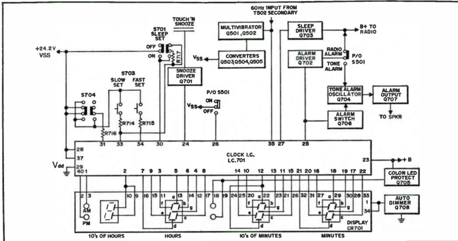
Fig. 9-1. Simplified digital clock readout circuit.
