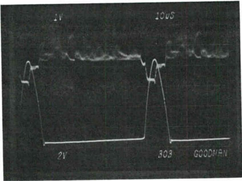
Fig. 3-21. Dual-trace scope indicates correct timing of the horizontal keying pulse.
