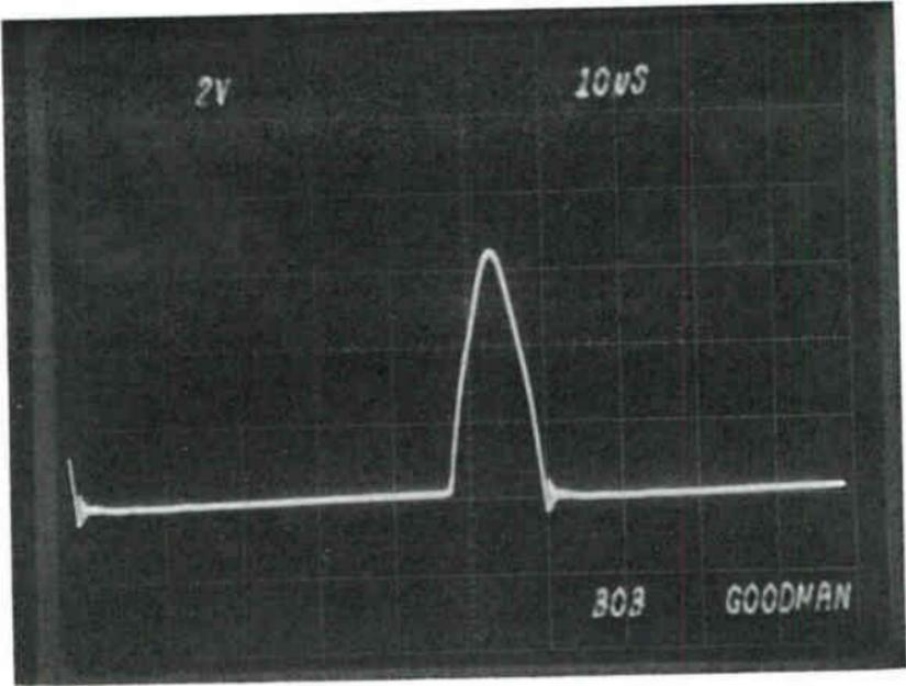
Fig. 3-18B. Horizontal keying pulse.
