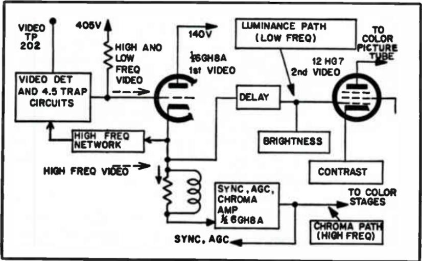
Fig. 3-42. Simplified first video amplifier circuit.
