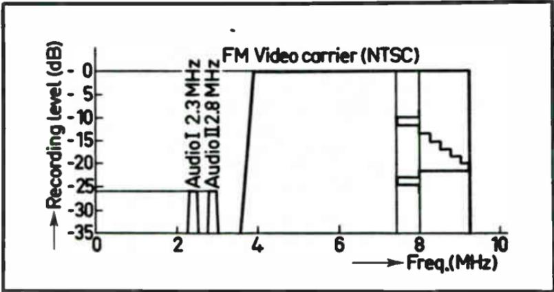
Fig. 11-3. Frequency spectrum of video disc information.
