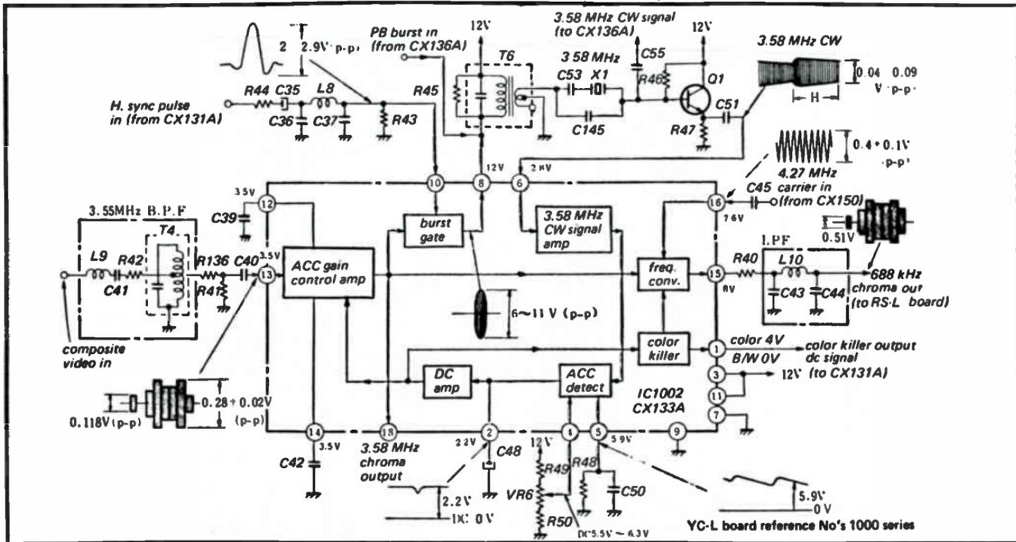
• Fig. 10-11. Block diagram of CX133A chip.
