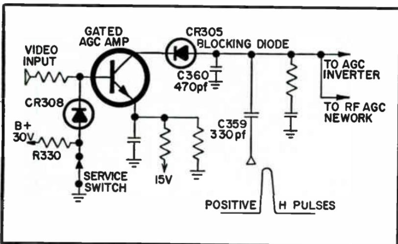
Fig. 3-48. Gated AGC amplifier circuit.
