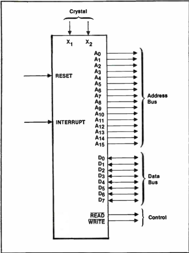
Fig. 12-5. Basic microprocessor signals.
