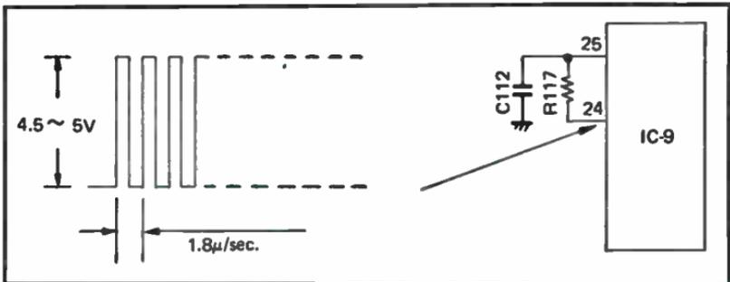
Fig. 8-12. Clock waveform.
