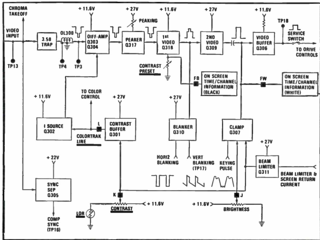
Fig. 3-26. Block diagram of low-level video stage.
