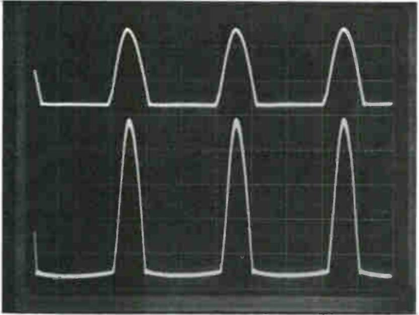
Fig. 3-63. Top pulse shows an open yoke, while bottom trace is for a good yoke.
