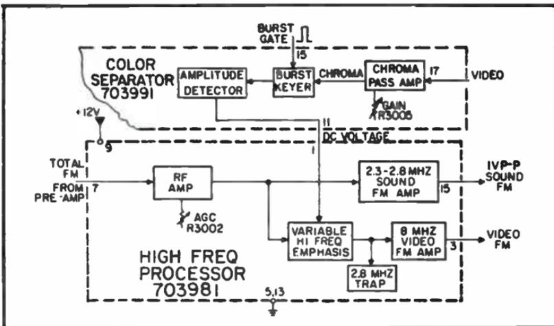
Fig. 11-13. FM signal processing circuit.
