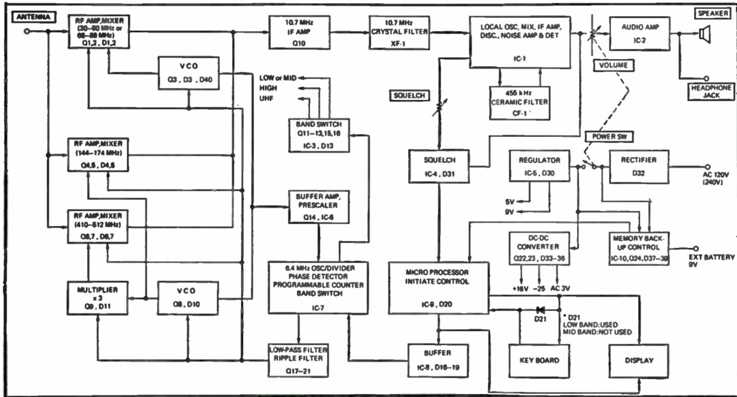
Fig. 8-9. PRO-2008 scanner block diagram.
