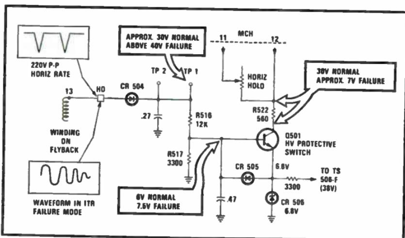
Fig. 3-32. High Voltage protection circuit - RCA CTC74.
