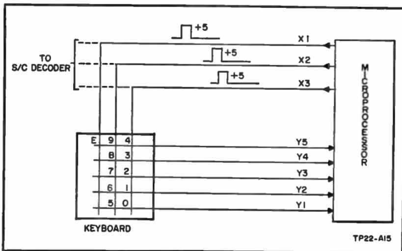
Fig. 1-5. Keyboard scanning block diagram.
