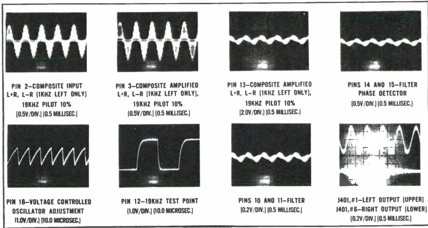
Fig. 5-12. Multiplex decoder scope waveforms.
