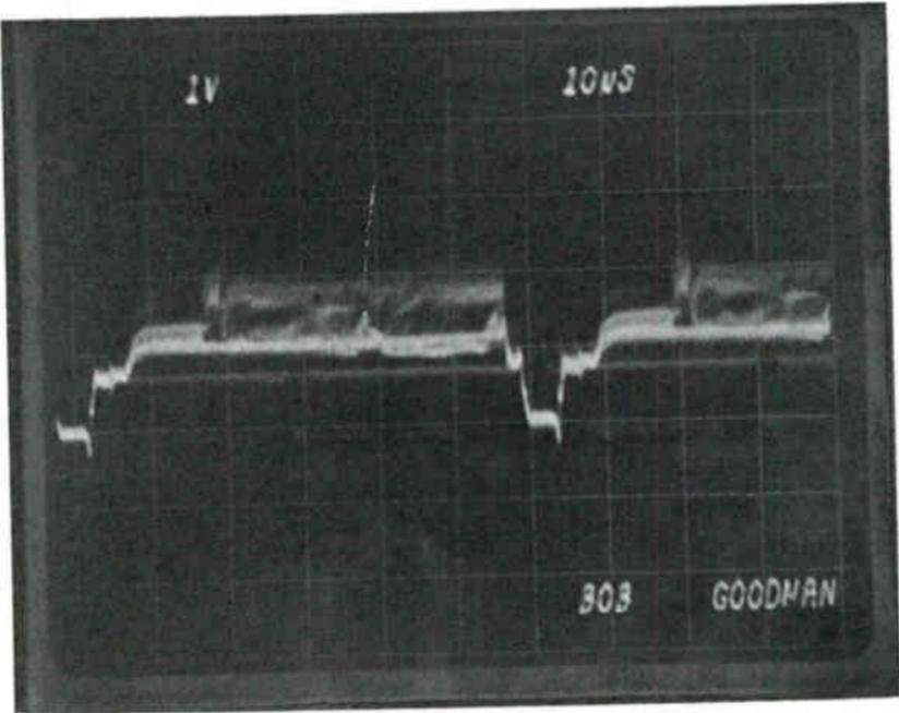
Fig. 3-18C. Composite video signal.
