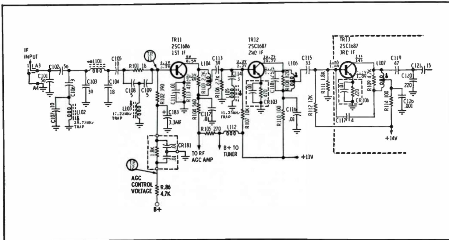
Fig. 4-9. Transistor video IF system.
