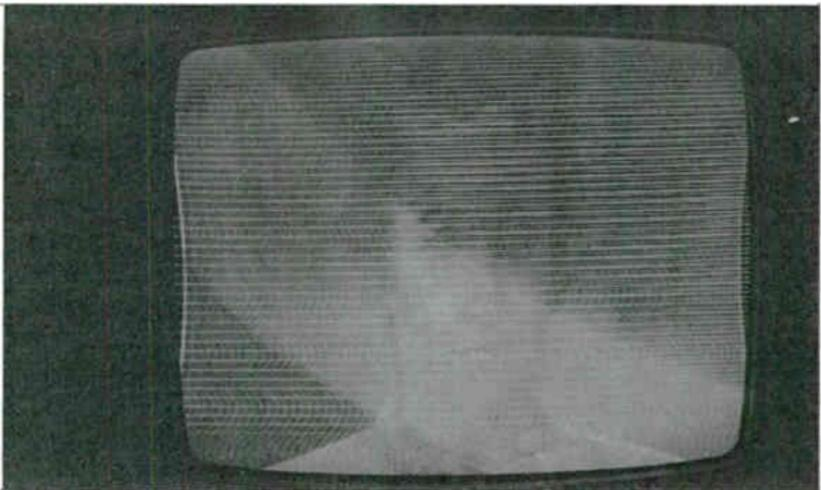
**Fig. 3-15. Faulty VDR causes picture to stretch-out.**
