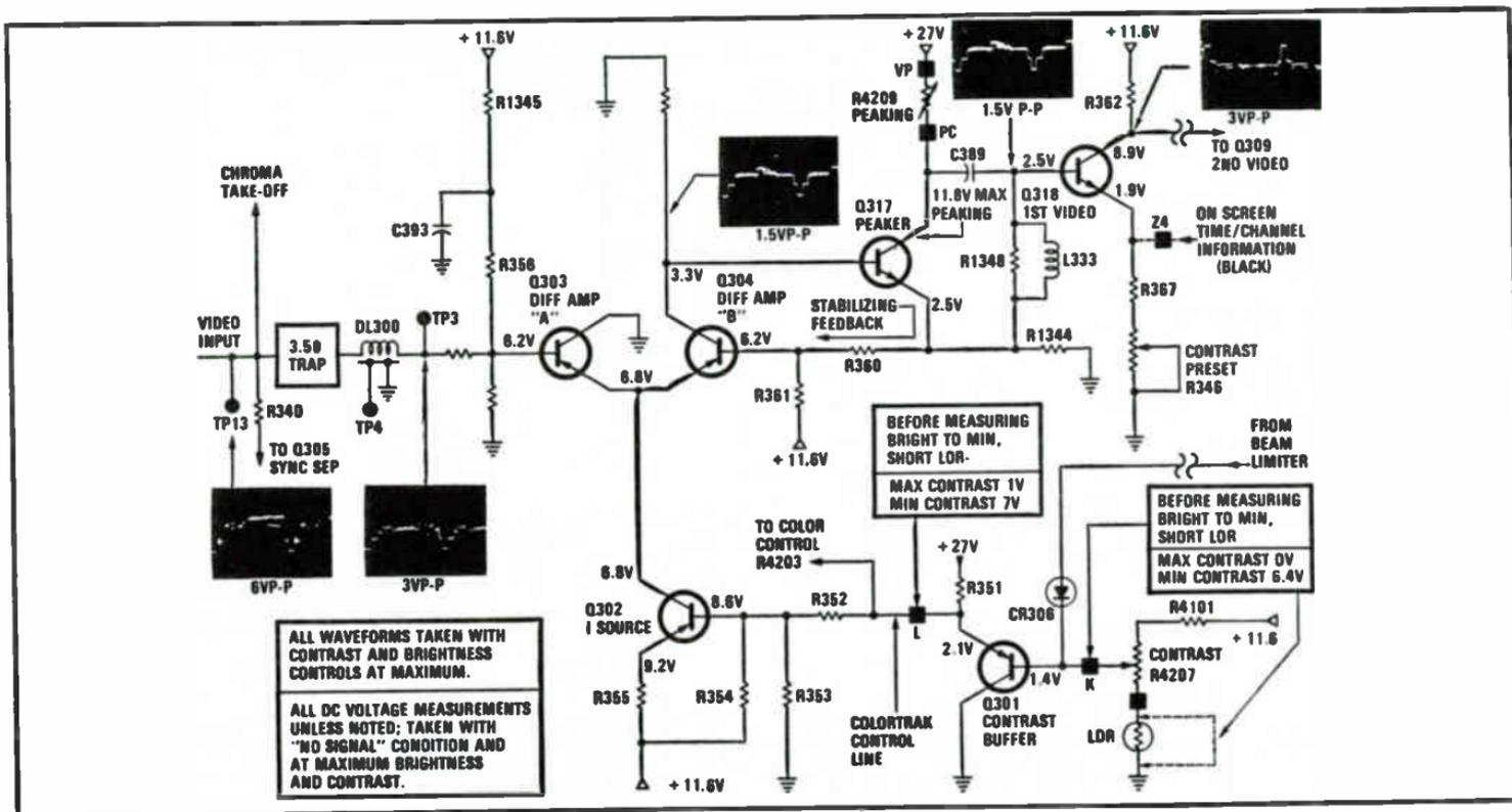
Fig. 3-24. Low-level video stage with check points.
