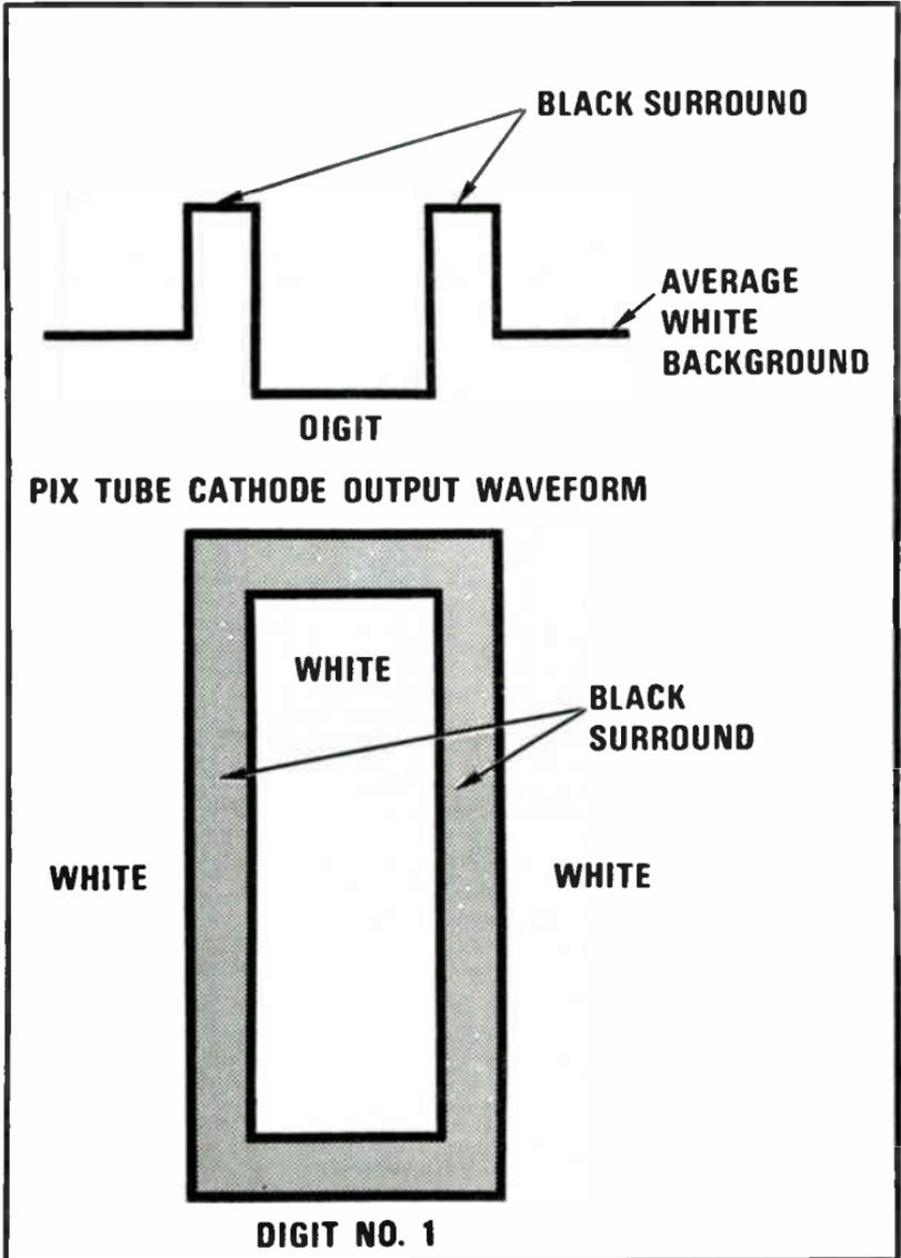
Fig. 9-10. Comparison of white 1 digit to output waveform.
