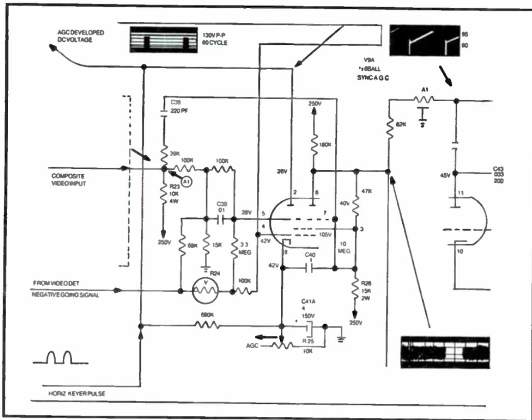
Fig. 3-50. Tube-type sync/AGC circuit.
