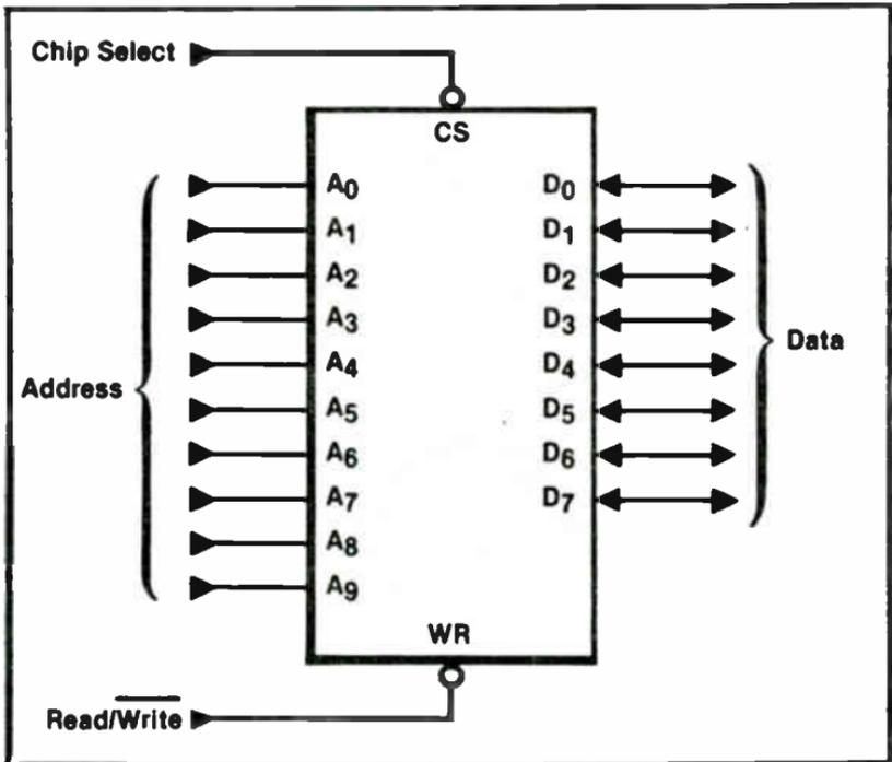
Fig. 12-8. Drawing of a 1K x 8 RAM chip.
