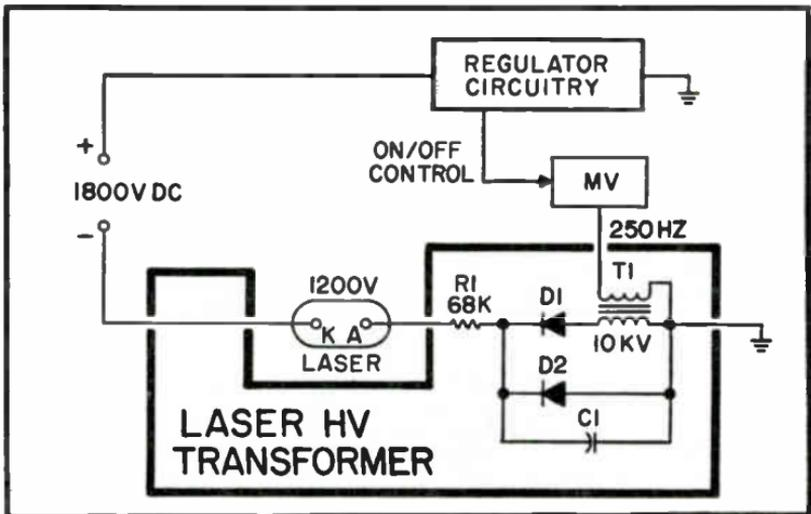
Fig. 11-8. Laser and High Voltage transformer.
