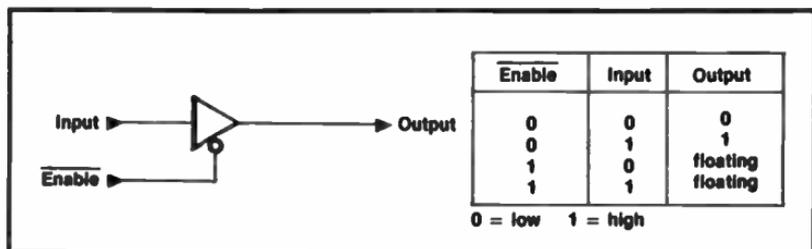
Fig. 12-2. Three-State Driver and Truth Table.
