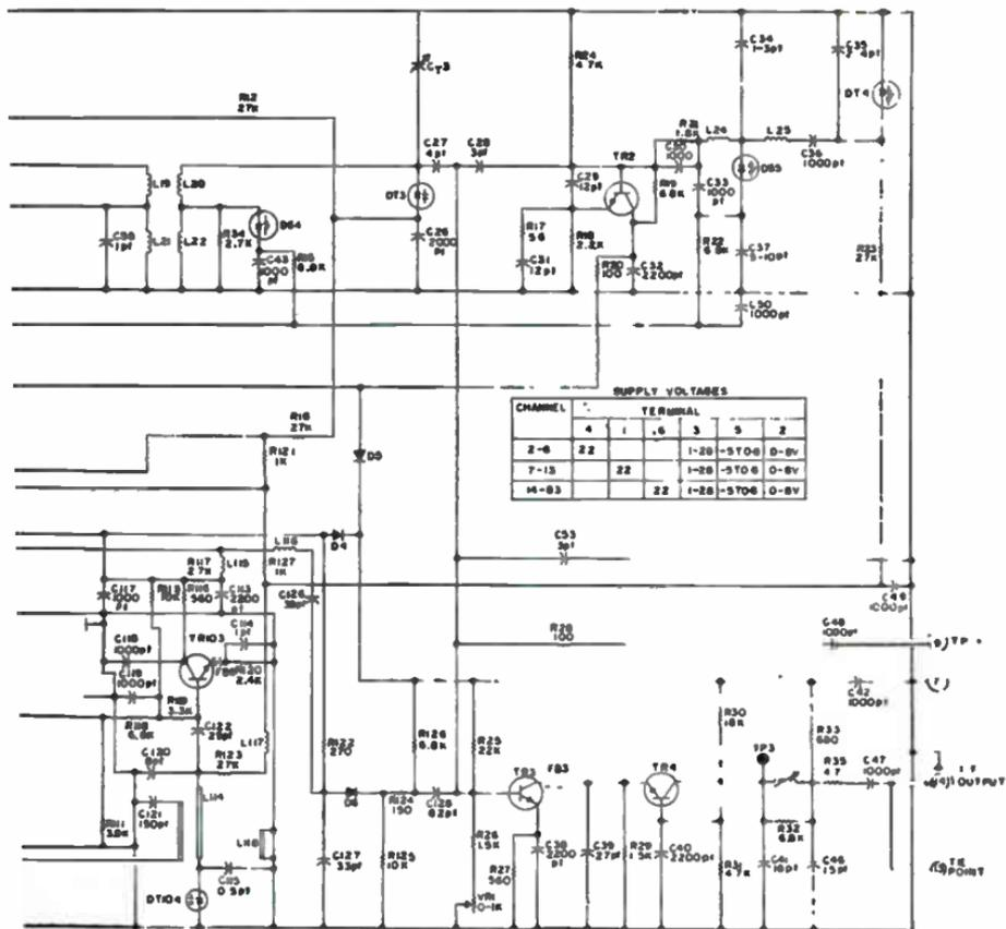
decreases, from the low to high channels, three levels of attenuation are needed. These are provided by voltage-dividing resistors and are switched by the varactor control bandswitch to the base of KQ04. The divider network KR16 and KR17 is used for AFC level correction on the UHF band. KR13 and KR15 are used to attenuate the voltage for high VHF channels, while the collector voltage of KQ02 is used directly on the VHF low band channels.
