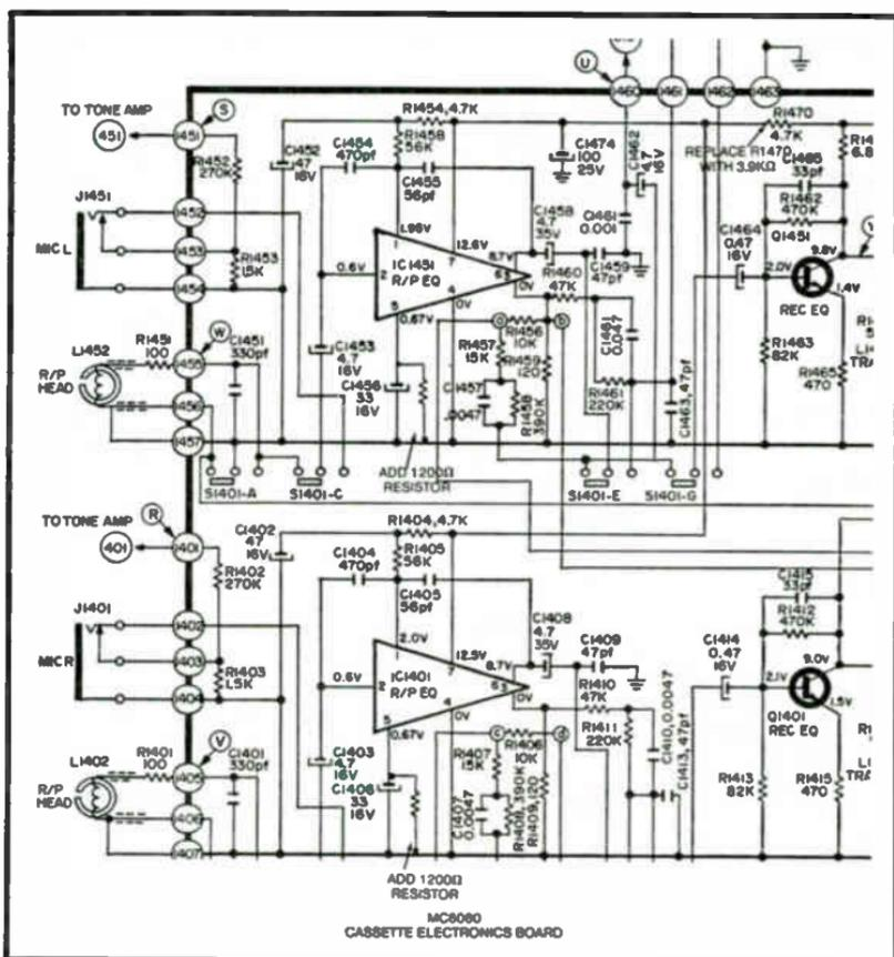
Fig. 7-5. Cassette electronic circuits (stereo).
