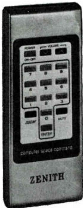
Fig. 2-1. Zenith 2000 remote transmitter.
