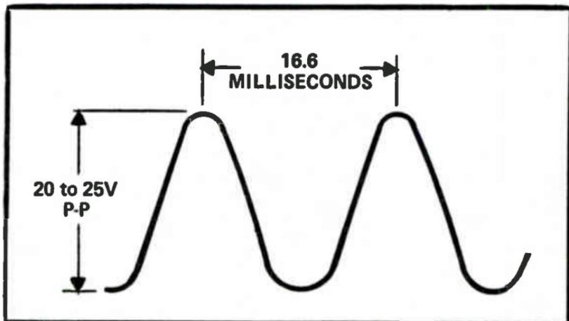
Fig. 9-2. Correct 60 Hz waveform.
