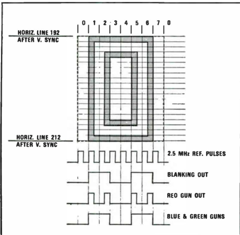
Fig. 9-8. Display format of red "0" with output waveform.
