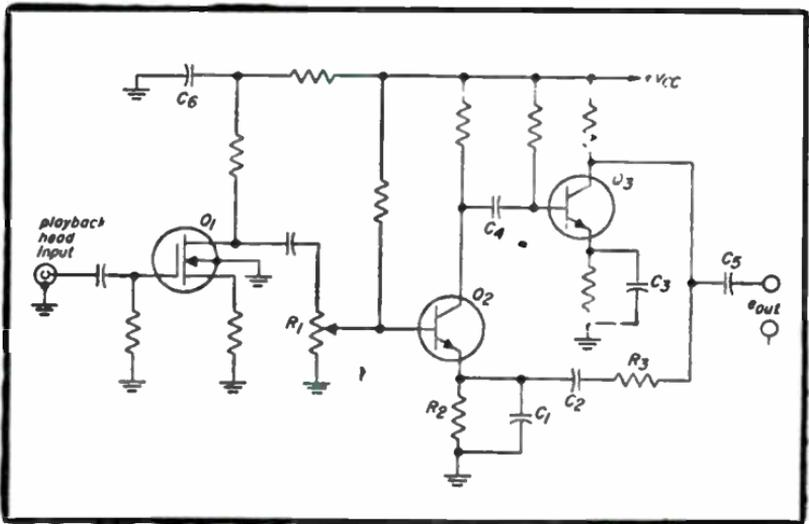
Fig. 7-2. Tape playback pre-amplifier circuit.
