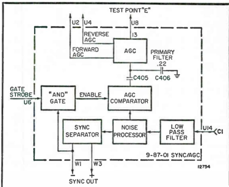
Fig. 3-17. Functional block diagram of the 9-87 module.
