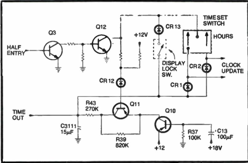
Fig. 9-11. Display timing circuitry.
