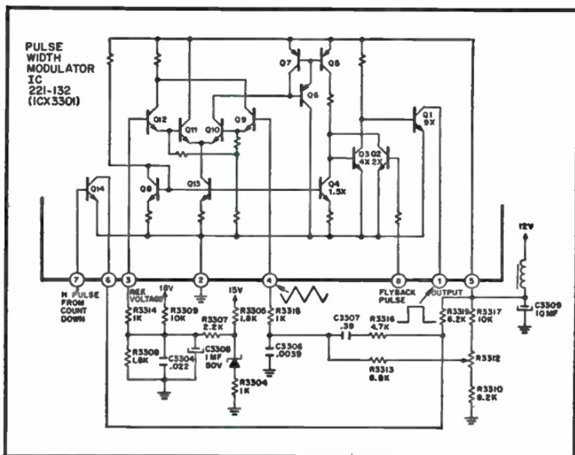
Fig. 3-57. Pulse width modulator IC.
