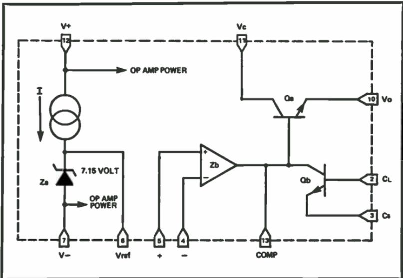
Fig. 2-15. Block diagram of 723 regulator Z2.
