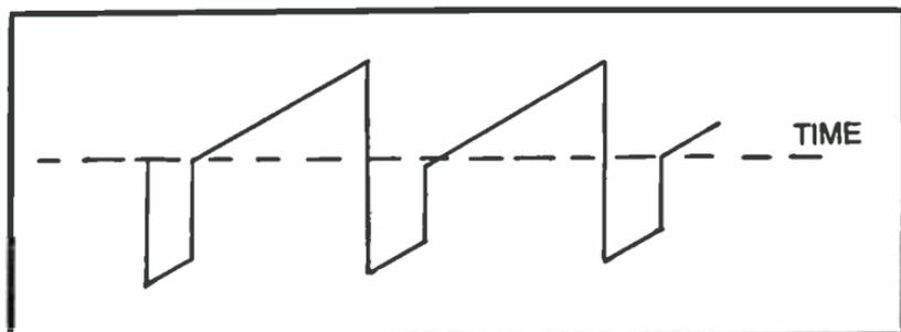
Fig. 3-11. Trapezoidal waveform for the vertical sweep.
