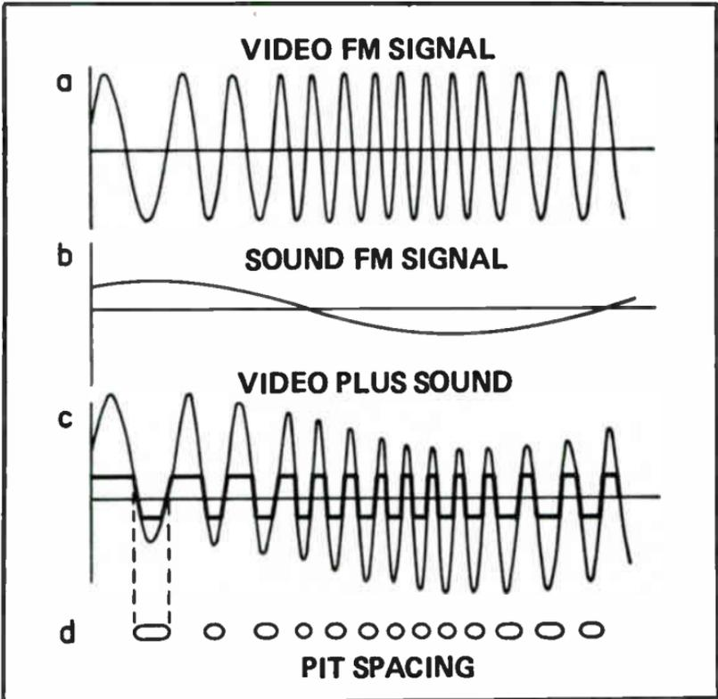
Fig. 11-4. Encoding of disc information.
