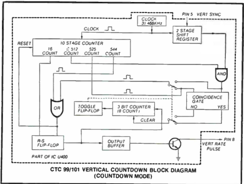
Fig. 3-2. Vertical count-down block diagram.
