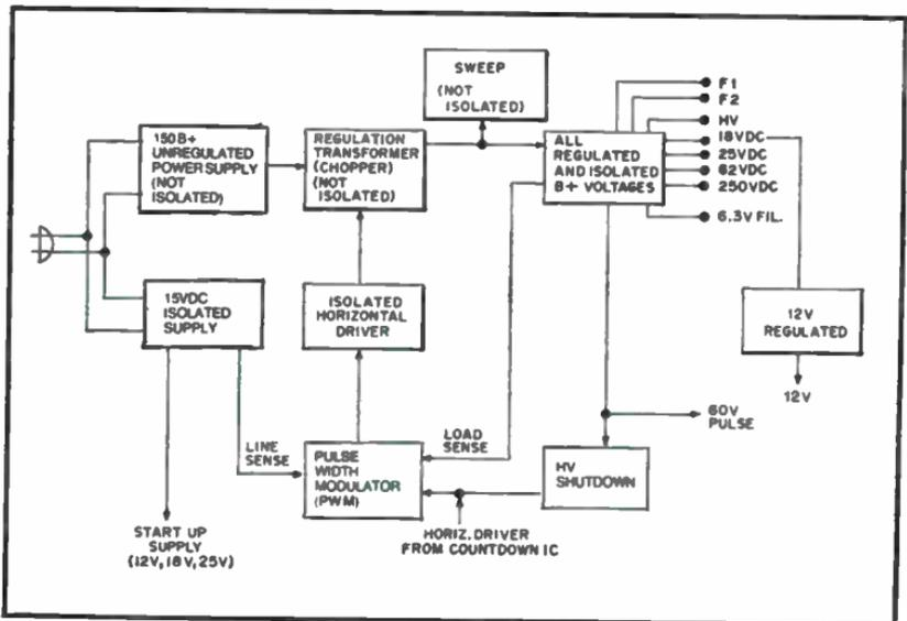
Fig. 3-52. Block diagram of the Electronic Power Supply.
