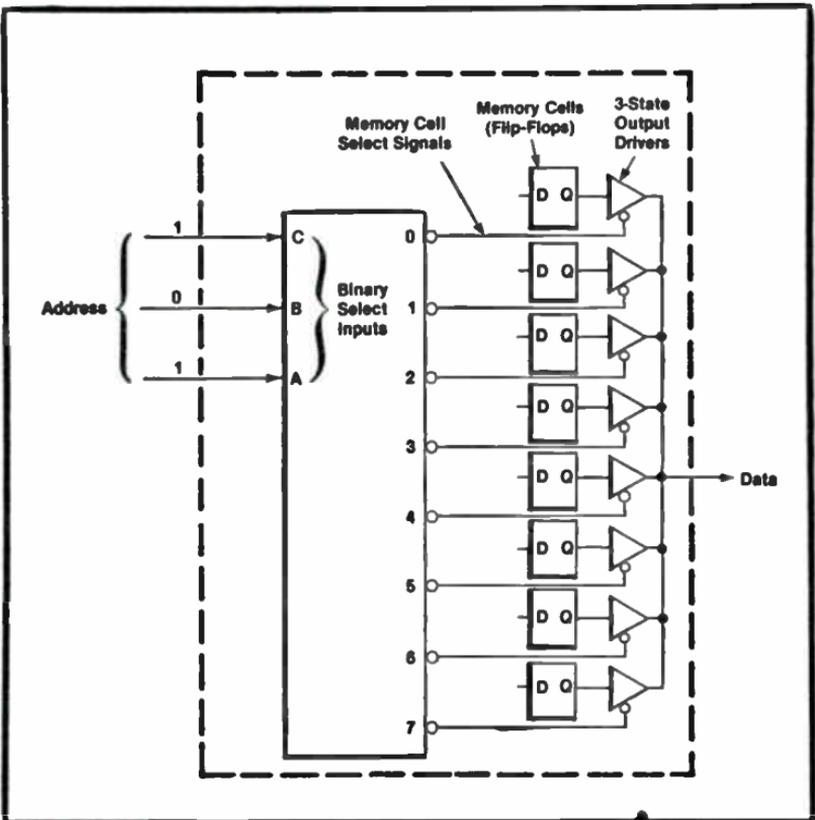
Fig. 12-6. Drawing of eight-bit memory.
