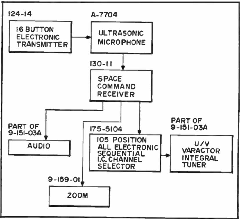
Fig. 2-3. Block diagram for Zenith 2000 remote system.
