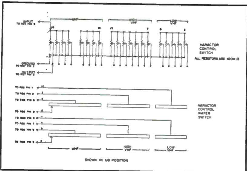
Fig. 1-13. Varactor control assembly diagram.
