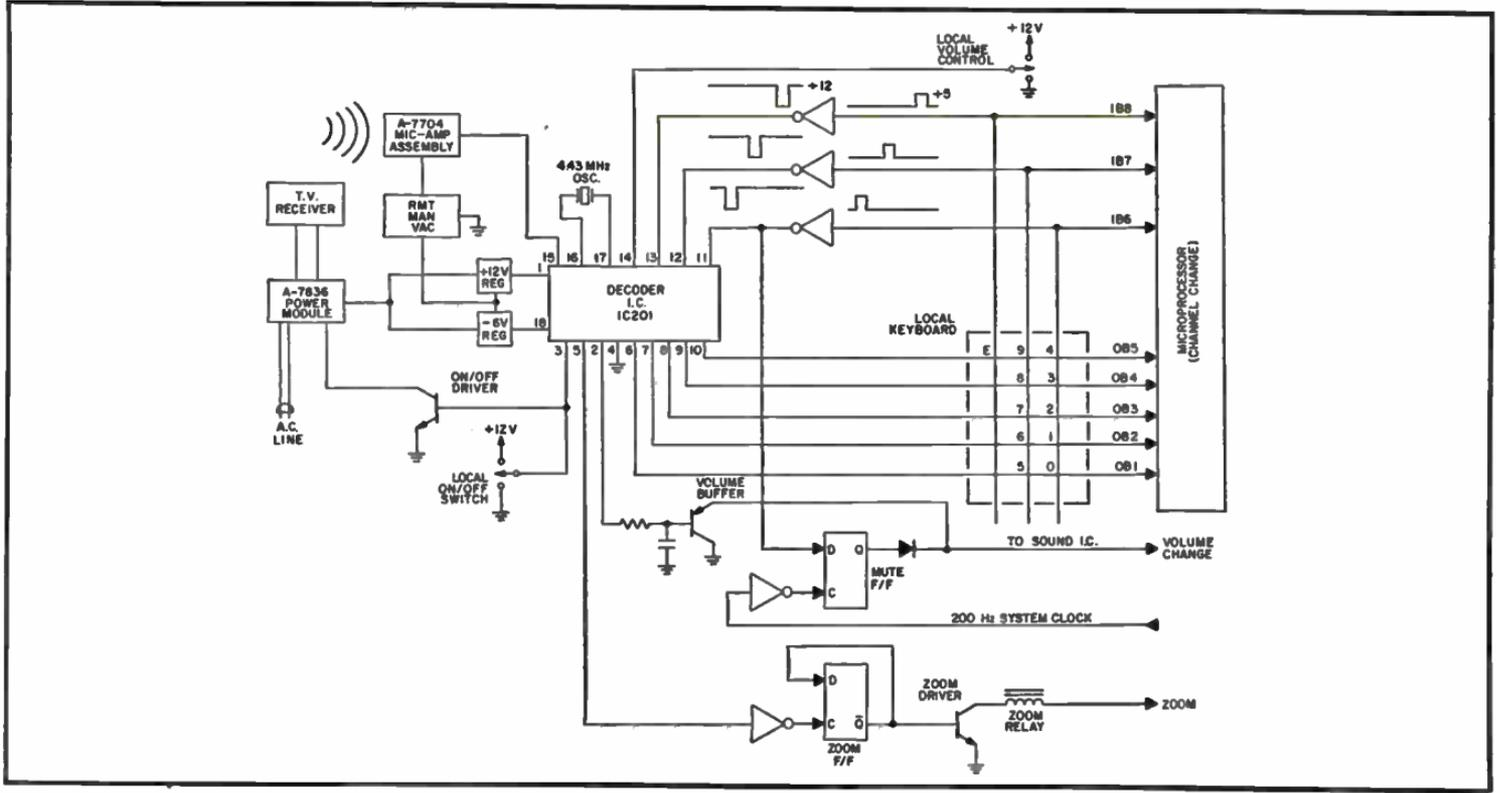
Fig. 2-5. Block diagram of Zenith 130-11 remote receiver.
