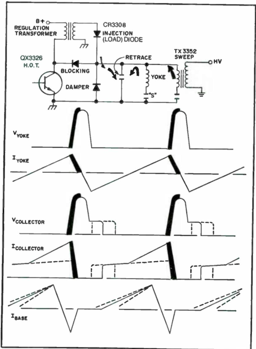
Fig. 3-56. Waveform drawings for start of retrace.
