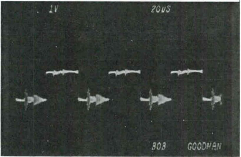
Fig. 3-59. Correct "H" pulse to PWM IC.
