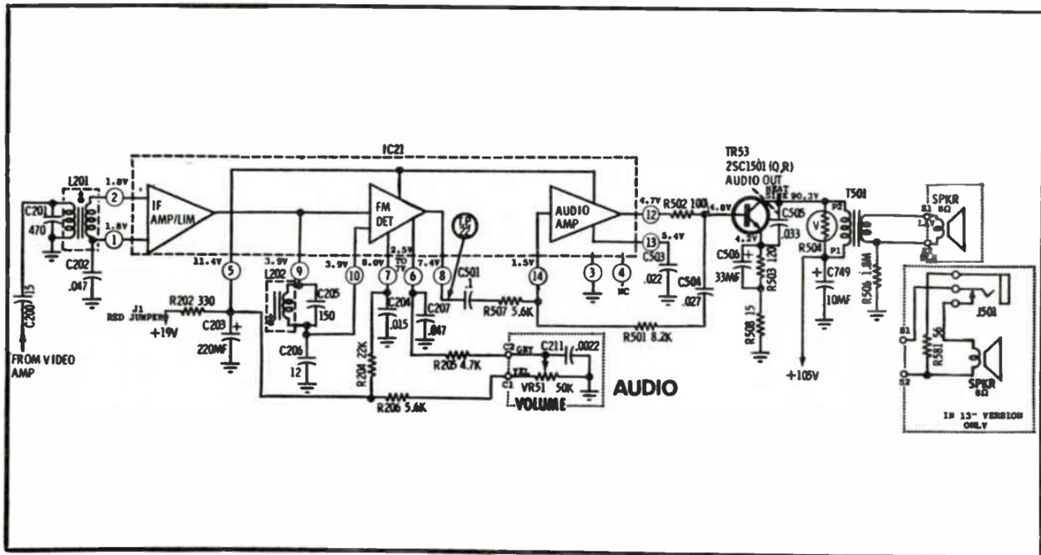
Fig. 4-10. Audio system - IC type.
