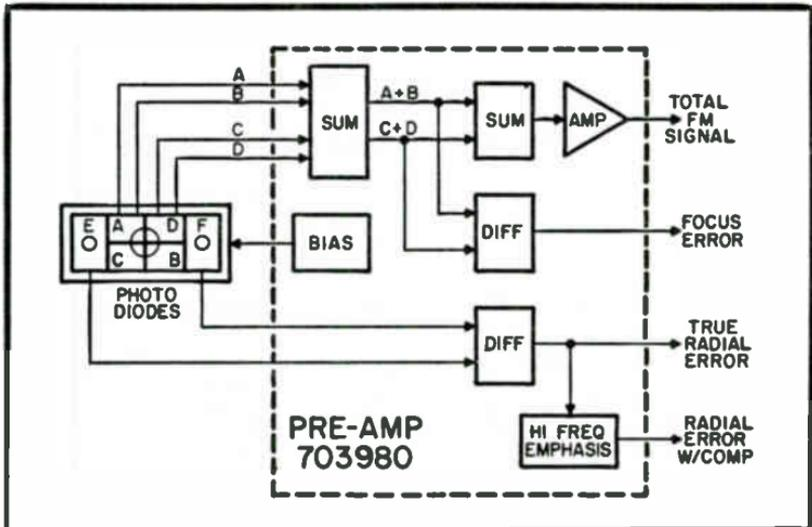
Fig. 11-11. Photo diodes and pre-amp module.
