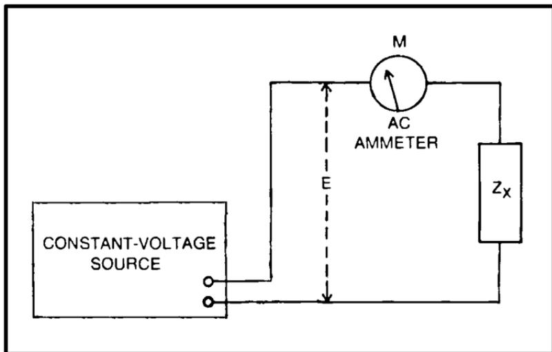
Fig. 3-2. Ammeter method for measuring an unknown impedance.
