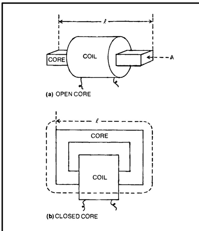
Fig. 4-3. Coils with a magnetic core: (a) open core, (b) closed core.
