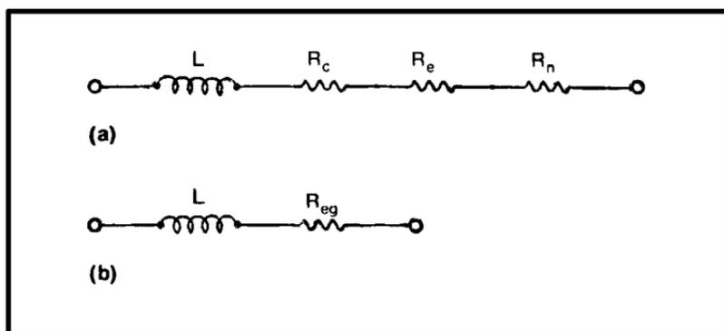
Fig. 4-5. Equivalent circuits of core-type inductors with: (a) losses shown as series-resistive components, and (b) losses simplified to the equivalent resistance.
