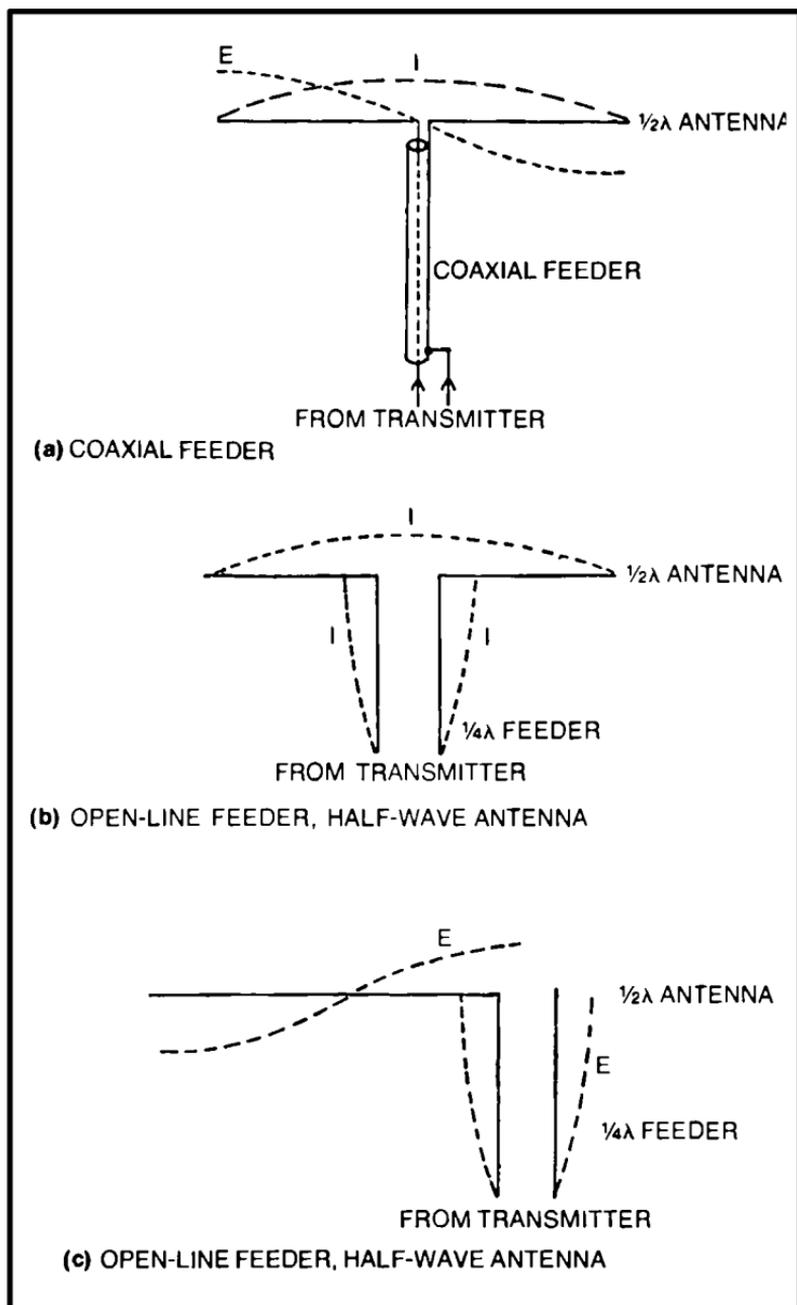
Fig. 2-15. Transmission line feeders used for the maximum transfer of energy from the transmitter to the antenna: (a) a coaxial feeder is connected to the center of a half-wave antenna; (b) a resonant open-line feeder is used to current-feed the center of a half-wave antenna; (c) a resonant open-line feeder is used to voltage-feed a half-wave antenna.
