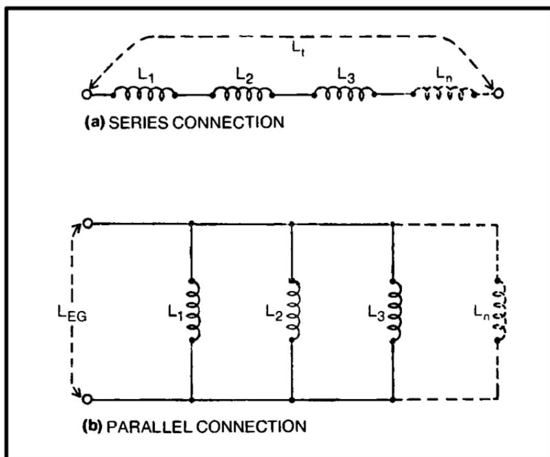
Fig. 4-6. Basic inductor circuits connected in (a) series and (b) parallel.
