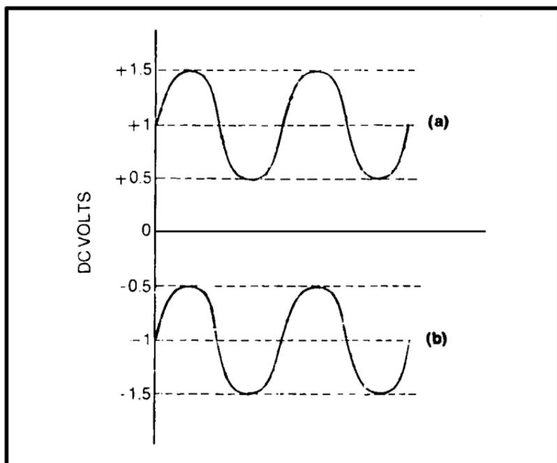
Fig. 1-9. Two examples of AC superimposed on DC. In (a) the alternating voltage is superimposed on  $+1V$  dc; in (b) the alternating voltage is superimposed on  $-1V$  dc.
