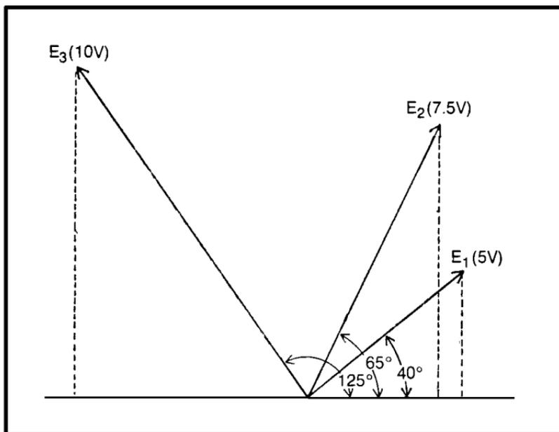
Fig. 1-7. Vector diagram of out-of-phase components.
