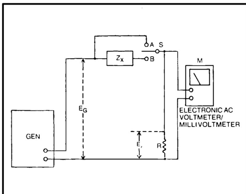
Fig. 3-3. Voltmeter method for measuring an unknown impedance.
