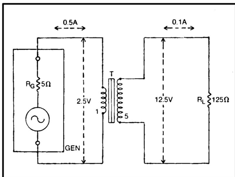
Fig. 2-14. Impedance-matching transformer.
