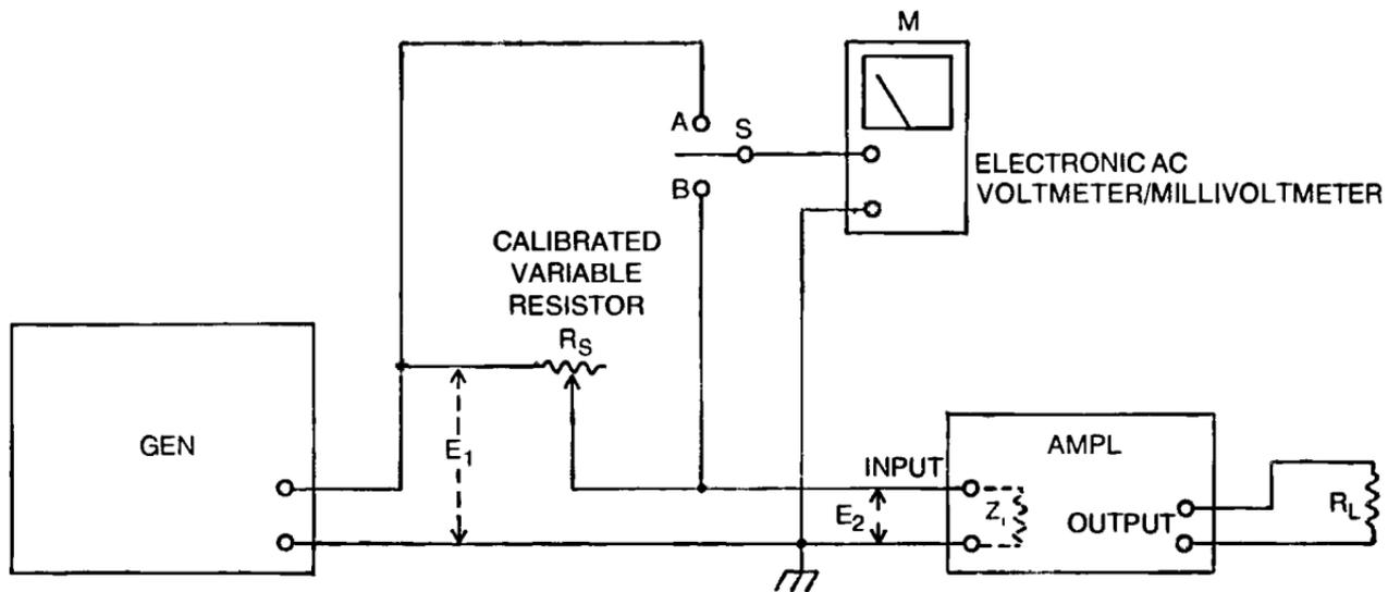
Fig. 3-9. Calibrated output-voltage dividers are used to measure the input impedance of an amplifier.
