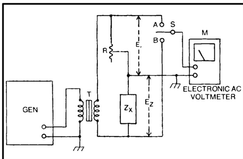
Fig. 3-4. Resistance/balance method of measuring an unknown impedance.
