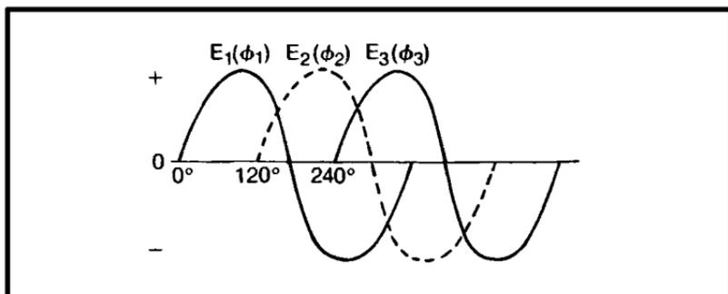
Fig. 1-5. Three-phase voltage. Three equal-amplitude voltages are spaced  $120^\circ$  apart.
