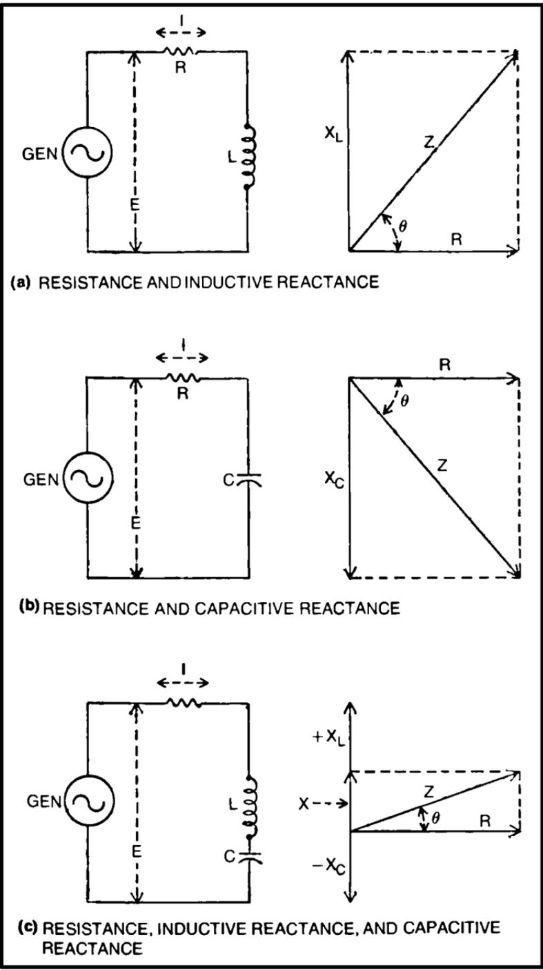
Fig. 2-1. Basic R-C-L-Z relationships with vectors showing how resistance and reactance combine to form impedance.
