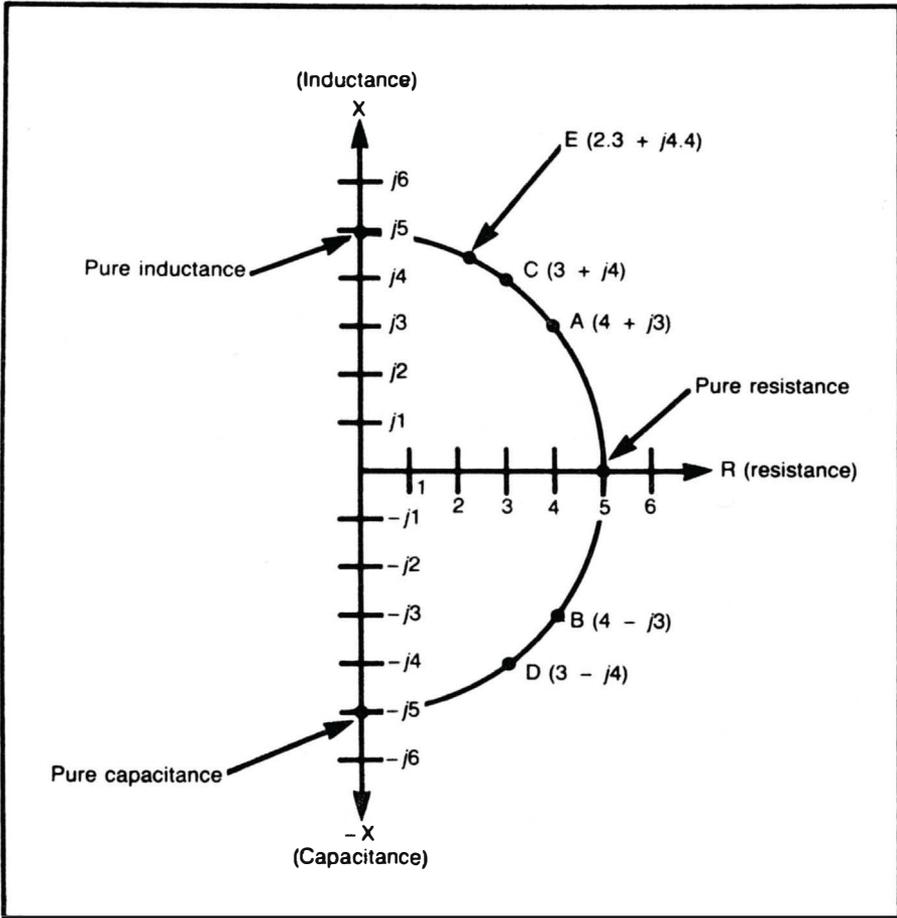
Fig. 5-9. Eight ways to produce an absolute-value impedance of 5 ohms.
