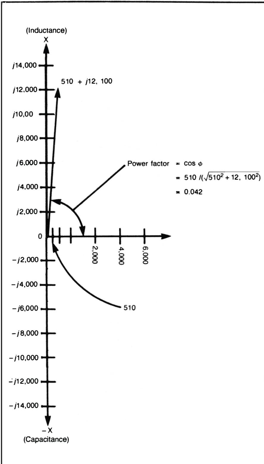
Fig. 5-7. Example of determination of phase angle by means of plotting a vector on the complex plane.
