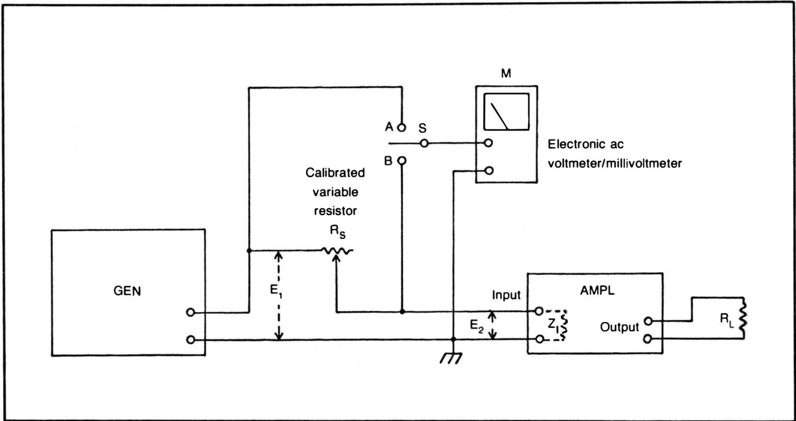
Fig. 3-9. Calibrated output-voltage dividers are used to measure the input impedance of an amplifier.
