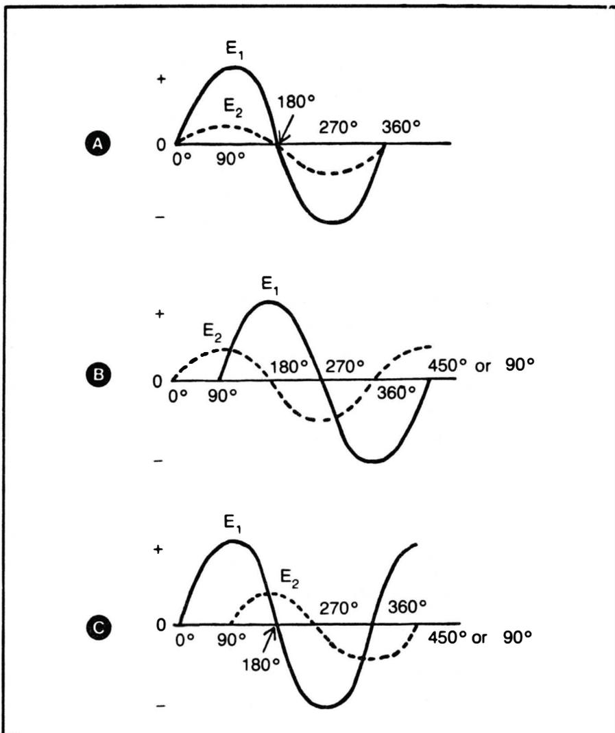
Fig. 1-4. Basic phase relationships of voltages and currents: (A) in phase, (B) leading phase, (C) lagging phase.
