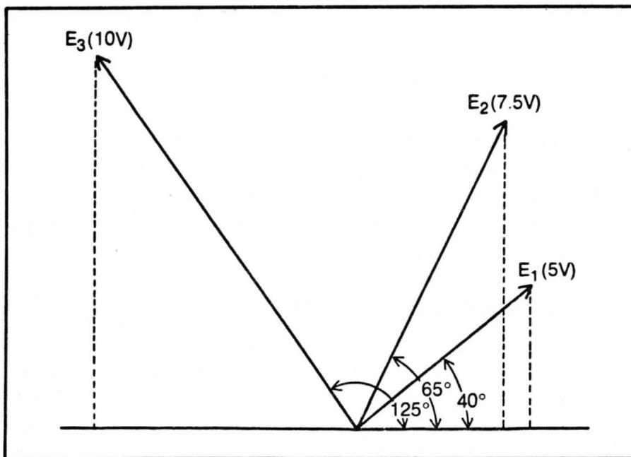
Fig. 1-7. Vector diagram of out-of-phase components.
