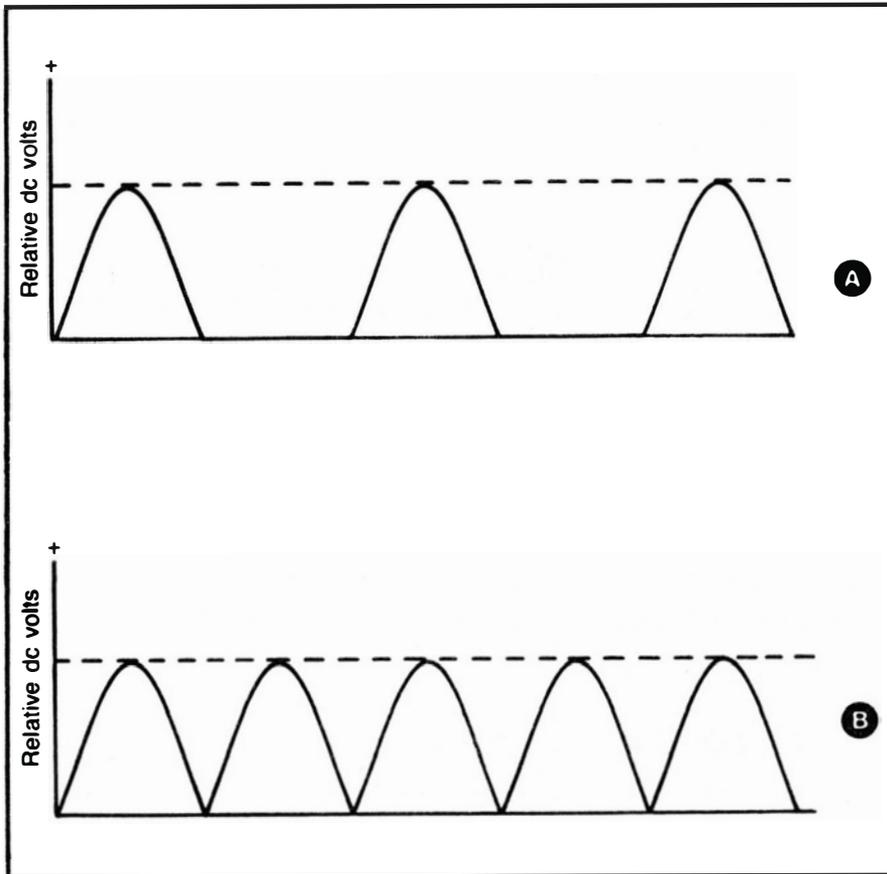
Fig. 1-9. At A, the output of a half-wave rectifier; at B, the output of a full-wave rectifier, assuming sine-wave ac input.
