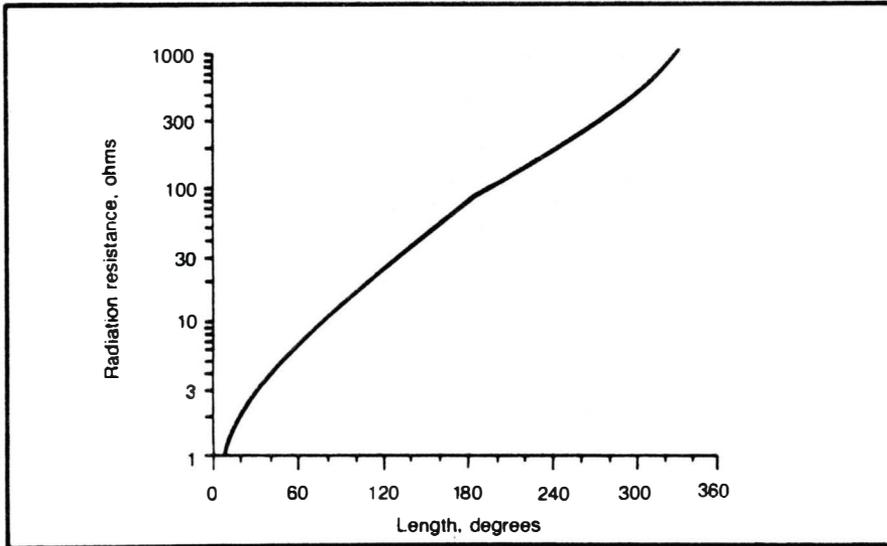
Fig. 6-3. Radiation resistance versus free-space length, in wavelengths, for a vertical radiator fed at the base and mounted over perfectly conducting ground.
