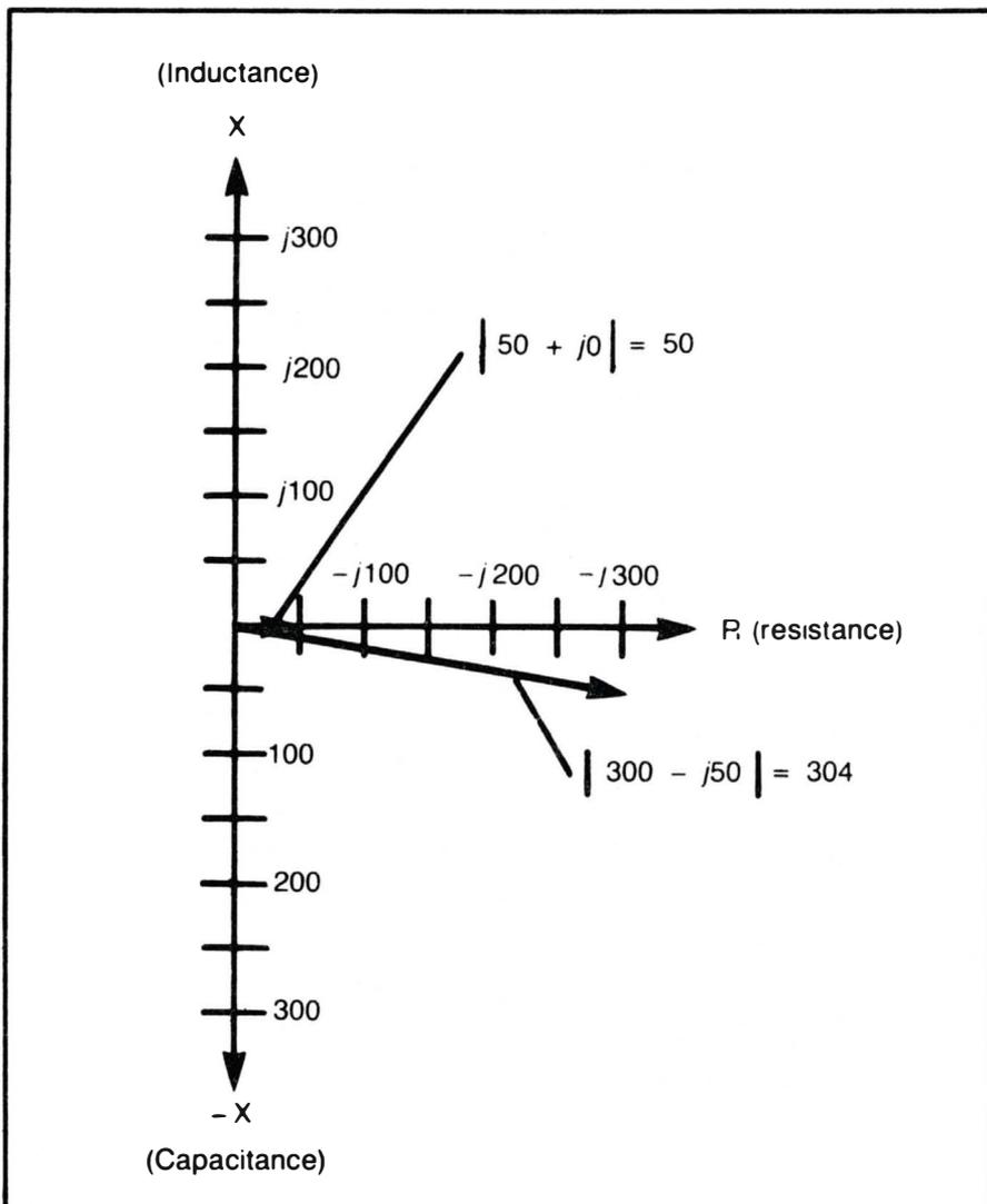
Fig. 5-5. Two examples of complex impedance vectors.
