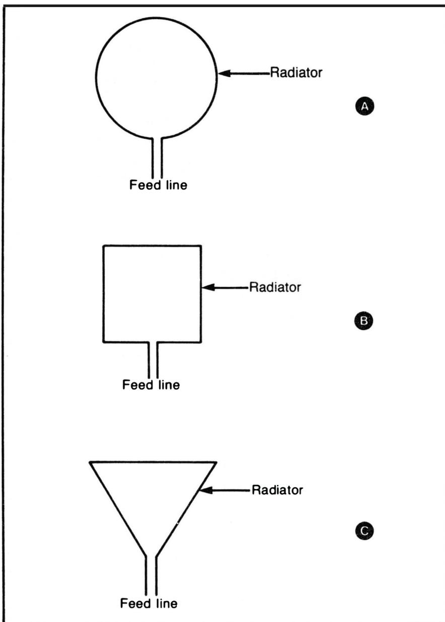
Fig. 6-14. Three common configurations for a full-wave loop.
