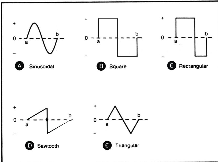
Fig. 1-1. Representative ac waveforms. The period is the duration from point **a** to point **b** in any of these waveshapes.
