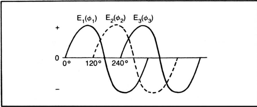
Fig. 1-5. Three-phase voltage. Three equal-amplitude voltages are spaced 120° apart.
