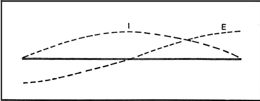
Fig. 2-4. Current and voltage distribution for a half-wave antenna operating at its fundamental frequency.
