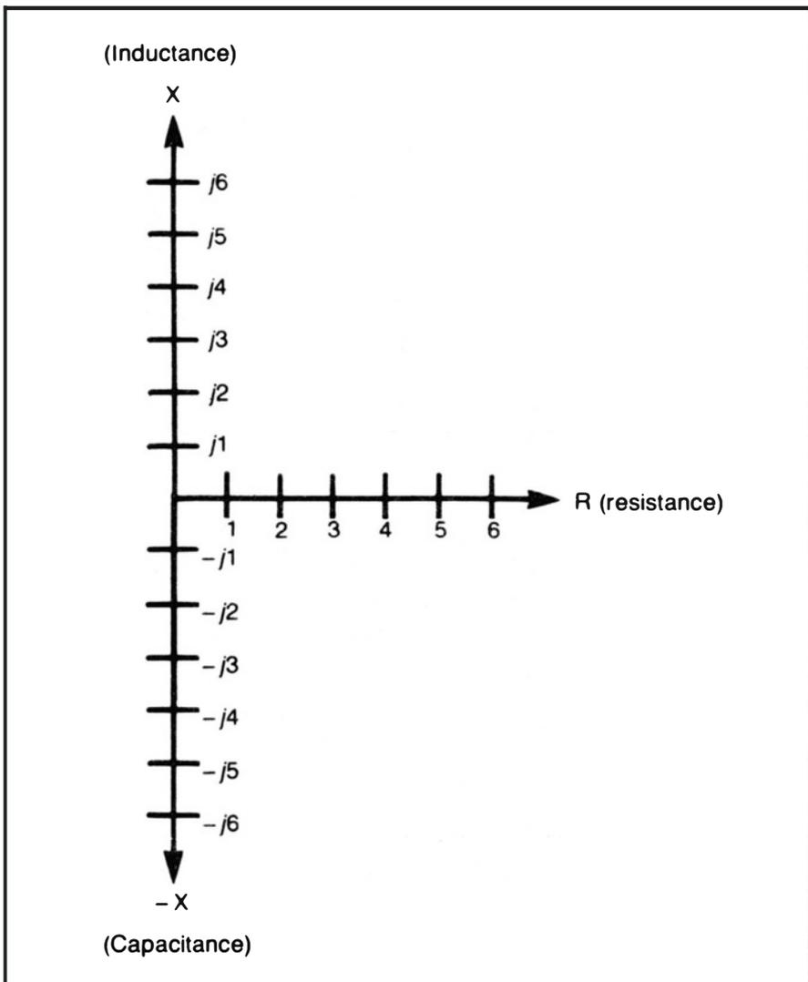
Fig. 5-4. Half-plane representation for impedance.
