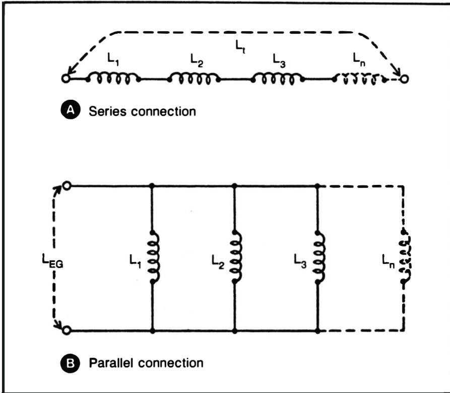
Fig. 4-6. Basic inductor circuits connected in (A) series and (B) parallel.
