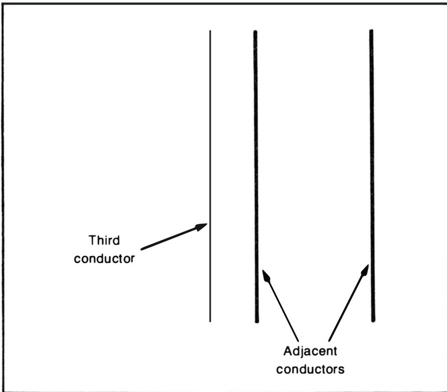
Fig. 4-9. When a third conductor is brought near two adjacent conductors, the mutual capacitance between the adjacent conductors increases.
