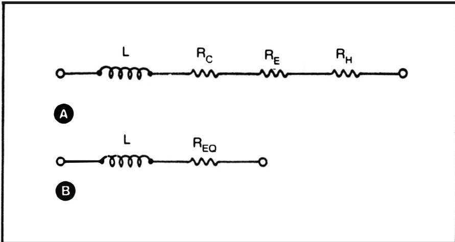
Fig. 4-5. Equivalent circuits of core-type inductors with: (A) losses shown as series-resistive components, and (B) losses simplified to the equivalent resistance.
