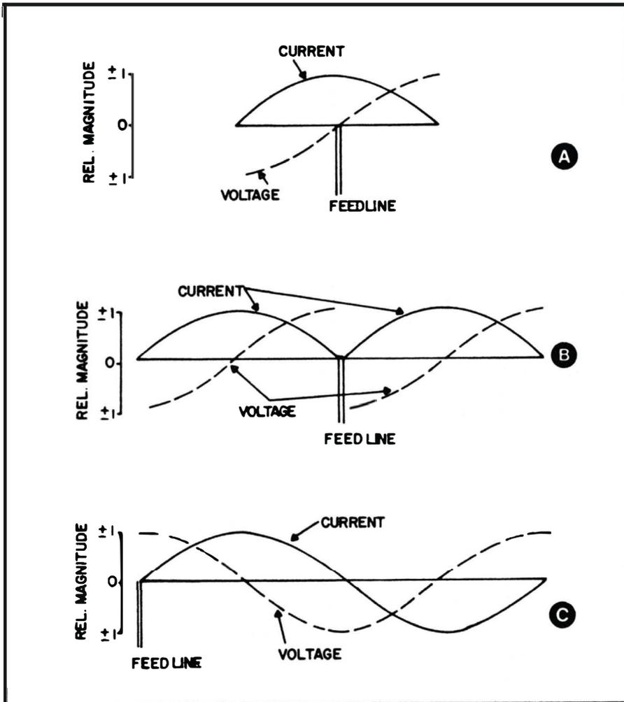
Fig. 6-12. Current and voltage distribution along a half-wave antenna.
