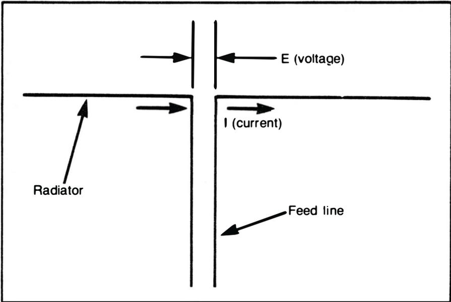
Fig. 6-1. A center-fed, half-wave radiator.
