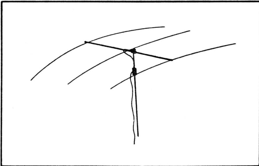
Fig. 6-15. A typical three-element Yagi. The driven element is at the center.
