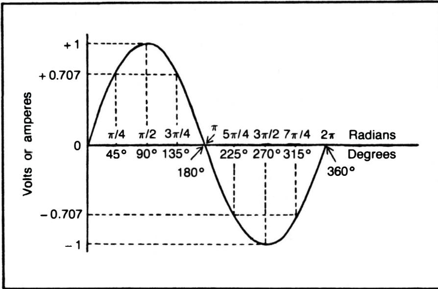
Fig. 1-2. A single sine-wave cycle with voltage plotted against the angle of rotation in both degrees and radians.
