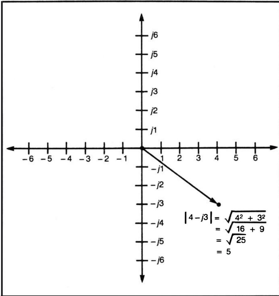
Fig. 5-3. The absolute value of a complex number is the length of its representative vector in the complex plane.
