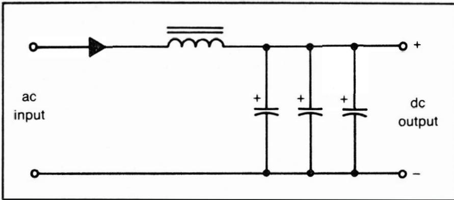
Fig. 4-10. An example of an application of connecting parallel capacitors to obtain greater capacitance than would be possible with a single capacitor.
