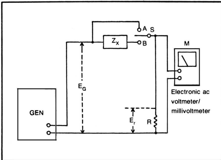
Fig. 3-3. Voltmeter method for measuring an unknown impedance.
