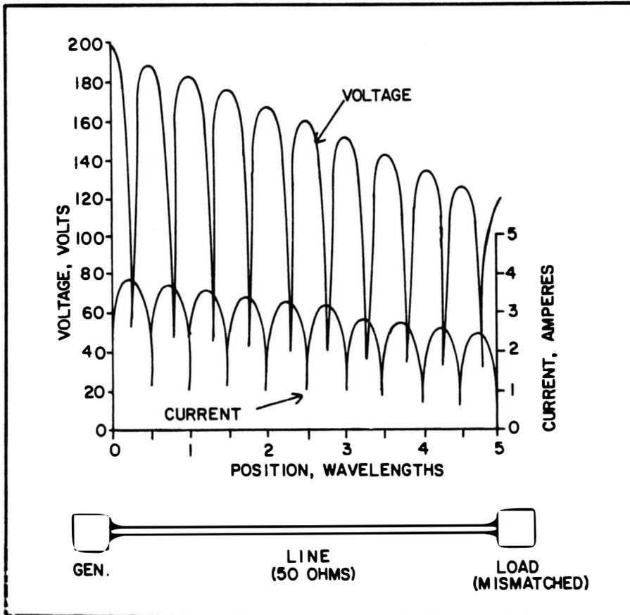
Fig. 6-9. Current and voltage loops along a mismatched line.
