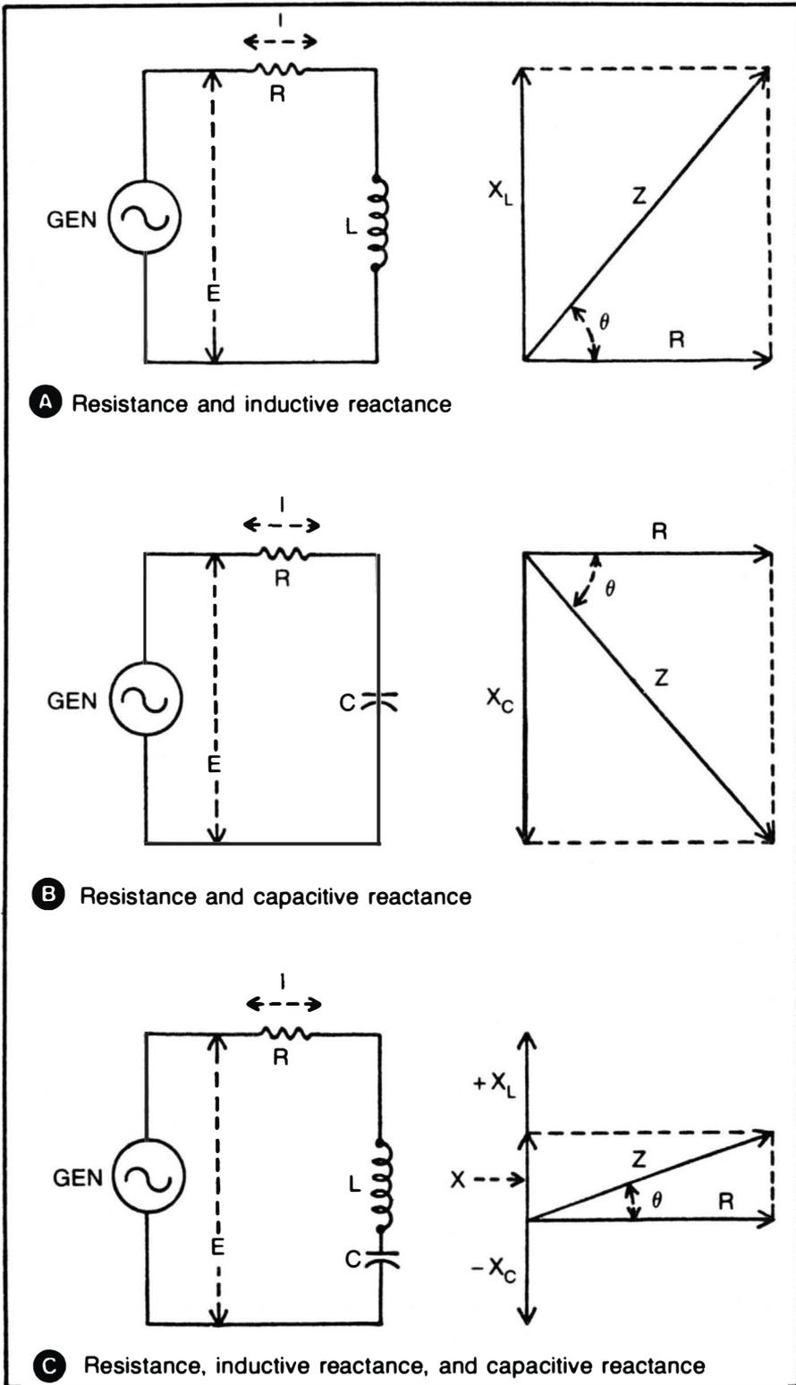
Fig. 2-1. Basic R-C-L-Z relationships with vectors showing how resistance and reactance combine to form impedance.
