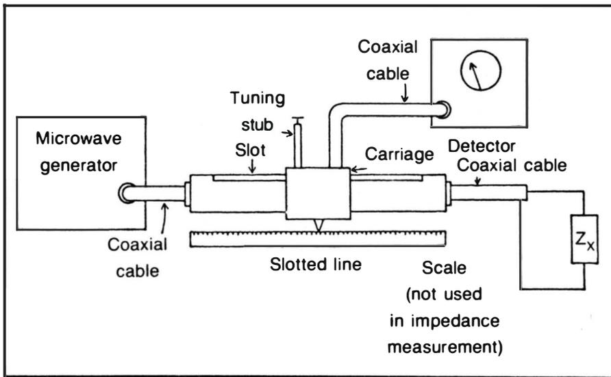
Fig. 3-8. Test setup using the slotted line to measure impedance at microwave frequencies.
