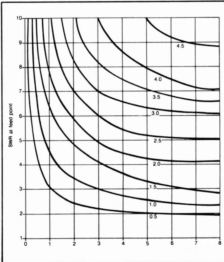
Fig. 6-8. Calculation of SWR-caused loss on the basis of feed-point SWR. Find the line loss for 1: SWR on the horizontal axis; then locate the feed-point SWR in the vertical axis. Find the point on the graph where these two data intersect; the additional loss can be read from the family or curves.
