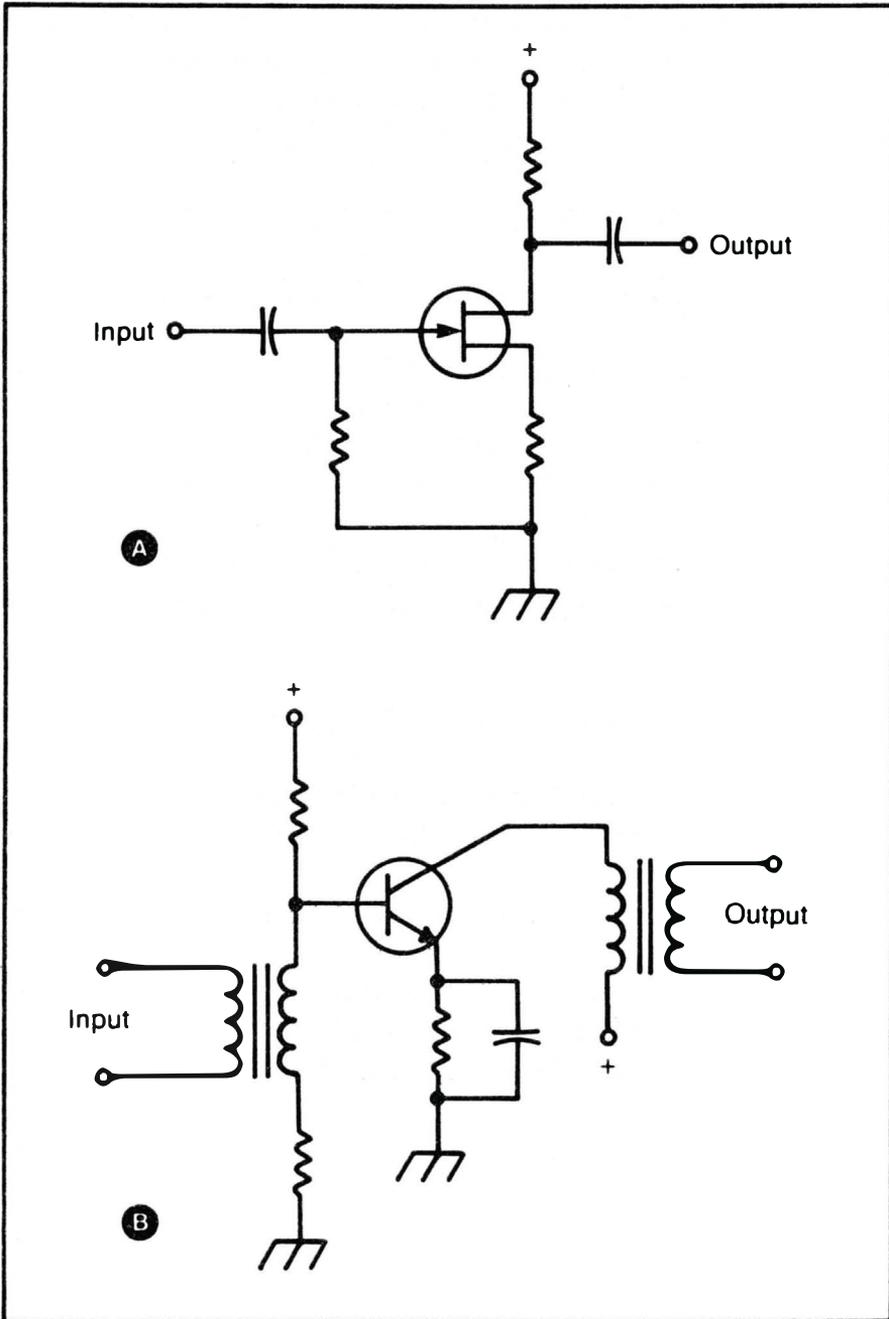
Fig. 4-12. At (A) the capacitor is used to allow biasing of an FET amplifier; at (B) the bypass capacitor is in an emitter circuit of a bipolar-transistor amplifier.
