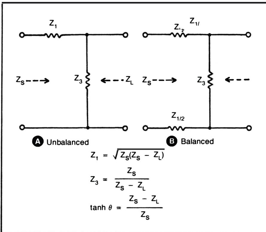
Fig. 2-20. L-type pad attenuators: (A) unbalanced and (B) balanced. Equations given are for finding impedance values.
