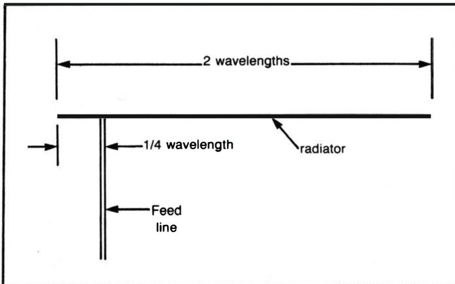
Fig. 6-17. Current feed for a two-wavelength longwire.
