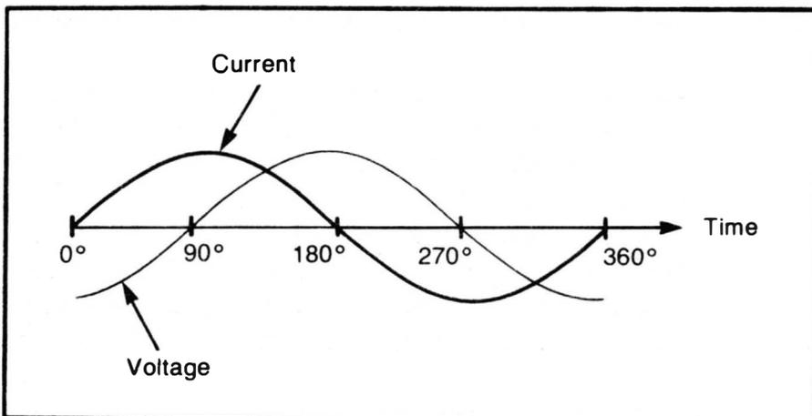
Fig. 4-7. In a pure capacitance, the current is 90 degrees ahead of the voltage.
