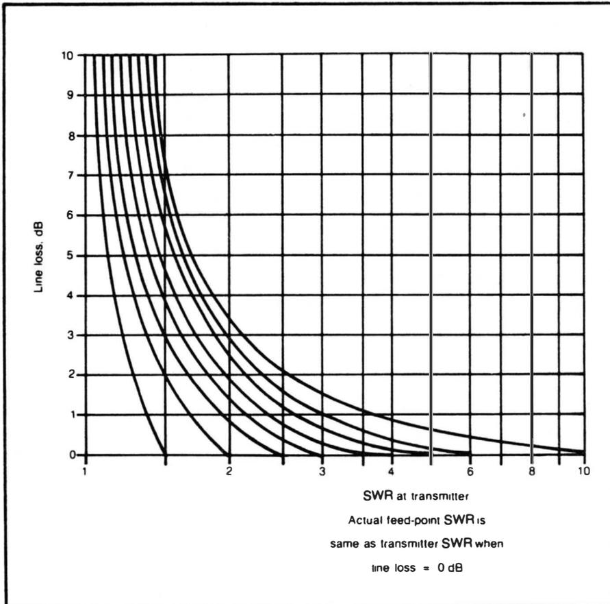
Fig. 6-7. Calculation of feed-point swr on the basis of transmitter swr. Find the transmitter swr on the horizontal scale and the line loss in dB (perfectly matched) on the vertical scale. Then read from the curves to find the actual feed-point swr.
