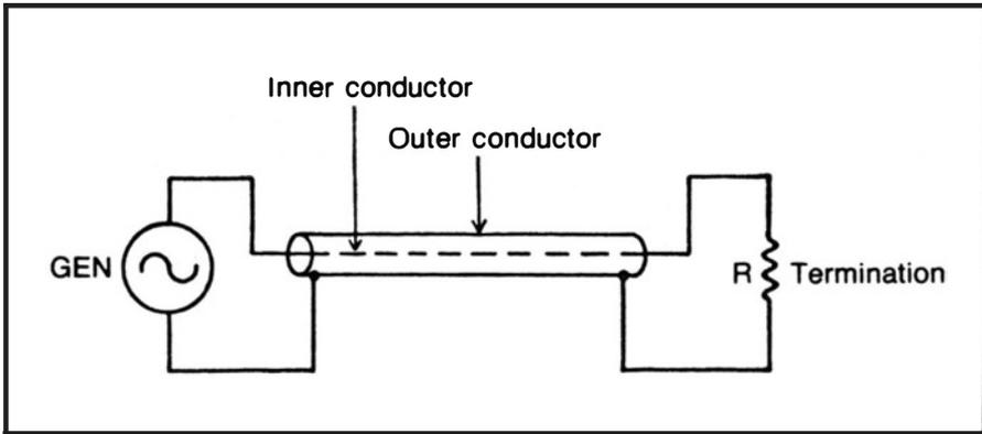
Fig. 2-8. Coaxial-type transmission line consisting of two concentric conductors connected between a generator and a load resistor.
