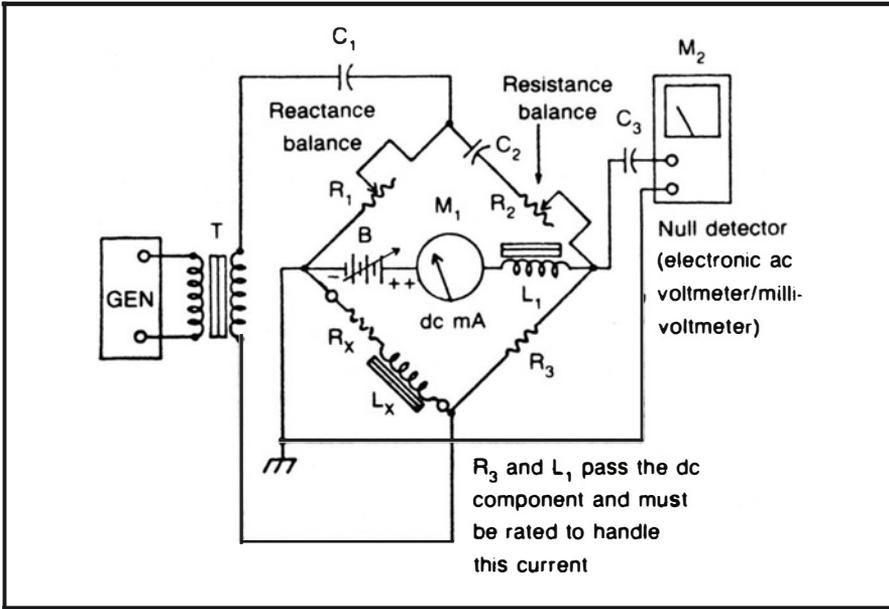
Fig. 3-14. A typical bridge circuit used for choke-coil measurement. The circuit shown is a Hay bridge.
