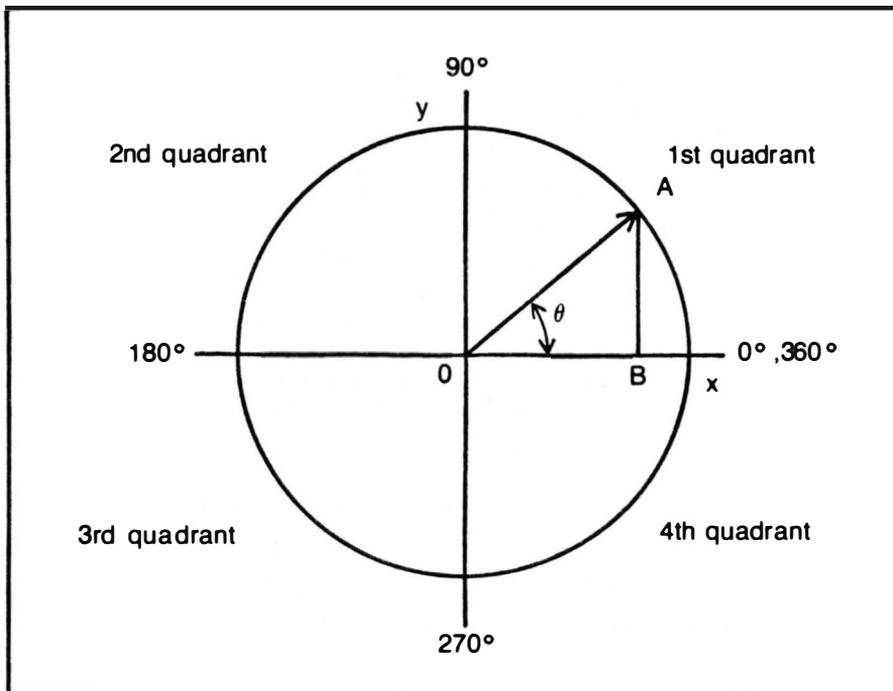
Fig. 1-6. Vector representation of ac components.
