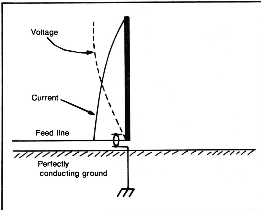
Fig. 6-13. Current and voltage distribution along a resonant, quarter-wave antenna operating over perfectly conducting ground.
