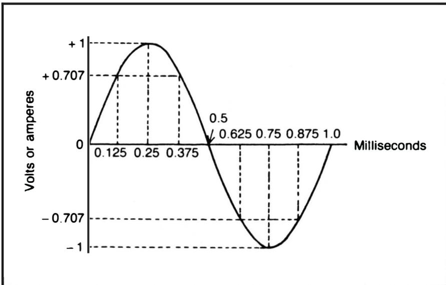
Fig. 1-3. A single-cycle 1000 Hz sine wave with the time axis plotted and several instantaneous voltages noted.
