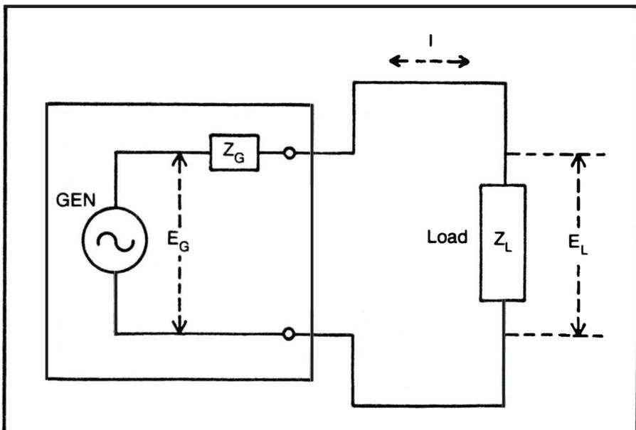
Fig. 2-10. Circuit illustrating an ac generator feeding a load impedance ( $Z_L$ ). Current must flow through both the generator impedance ( $Z_G$ ) and the load impedance.
