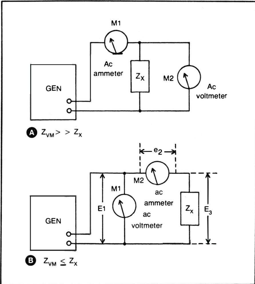
Fig. 3-1. Voltmeter/ammeter method for measuring an unknown impedance: (A) when the impedance of the meter ( $Z_{VM}$ ) is higher than the unknown impedance ( $Z_X$ ); (B) when the impedance of the meter is equal to or less than the unknown impedance.
