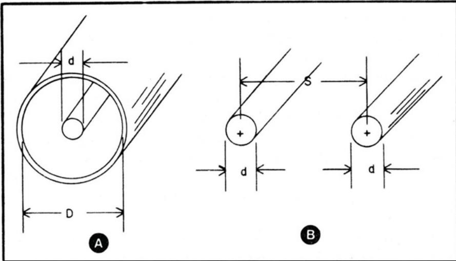
Fig. 6-4. Characteristic impedance depends on the physical dimensions and the spacing of conductors in a feed line. At (A), coaxial line; at (B), parallel-wire line.
