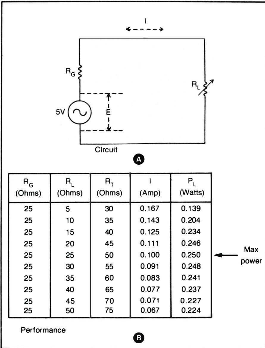
Fig. 2-13. Illustration of impedance matching. The circuit (A) has a variable load resistance connected to a generator. The chart (B) shows the performance of the circuit as the resistance ( $R_L$ ) is varied.
