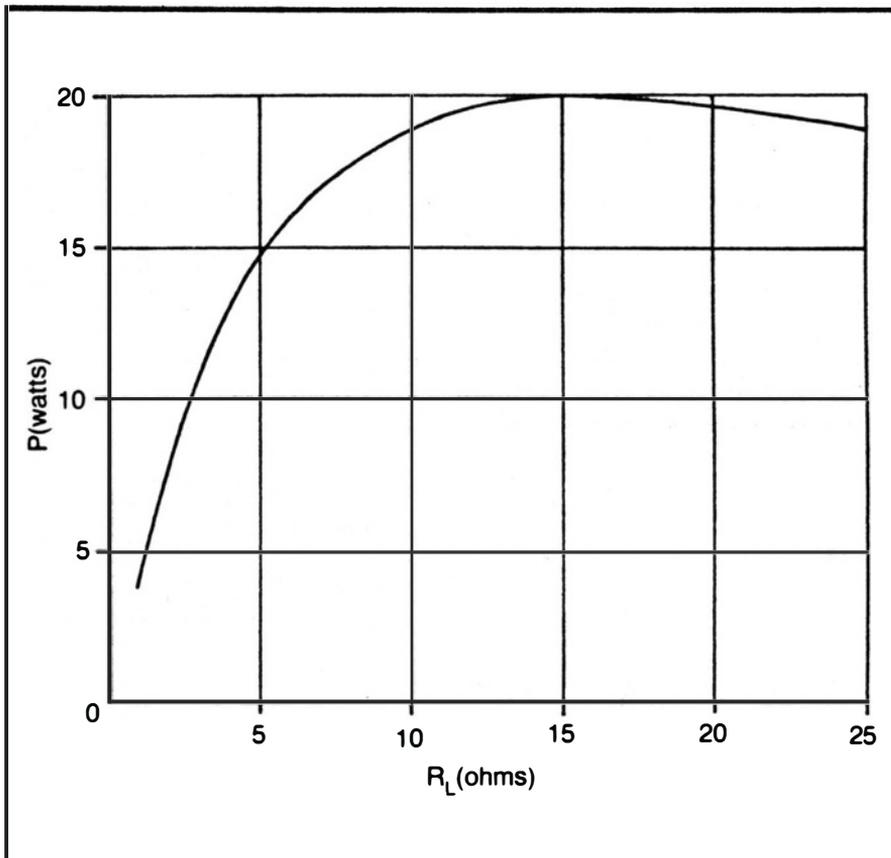
Fig. 3-11. The typical response curve for the resistor/wattmeter method of measuring amplifier output impedance.
