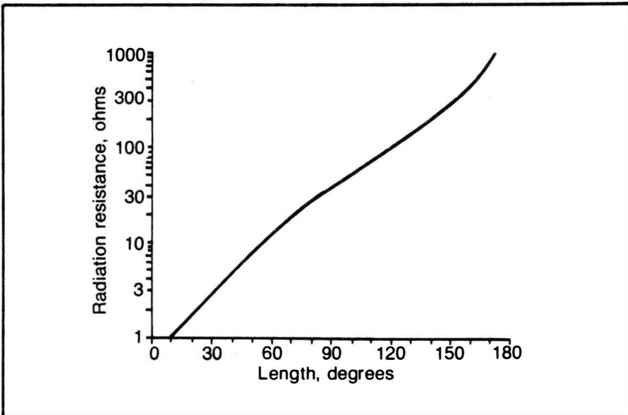
Fig. 6-2. Radiation resistance versus free-space length, in wavelengths, for a center-fed radiator.
