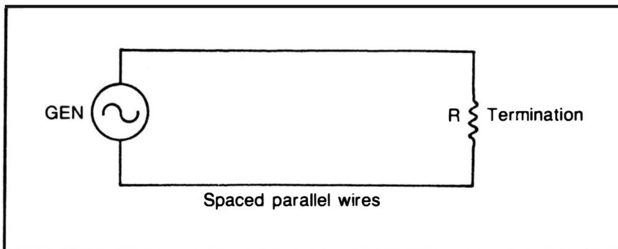
Fig. 2-6. Two-wire transmission line connected to an rf generator and a load resistor (termination).
