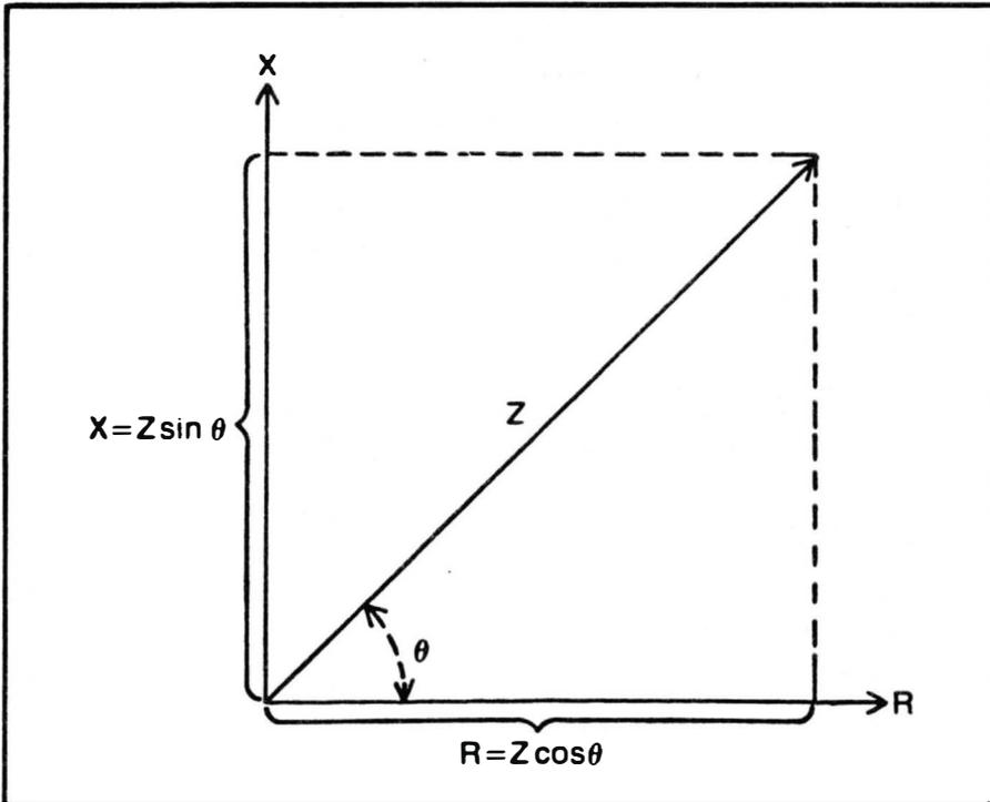
Fig. 2-2. Determination of resistance and reactance from impedance and phase angle. The resistance magnitude may be measured along the horizontal axis and the reactance along the vertical axis.
