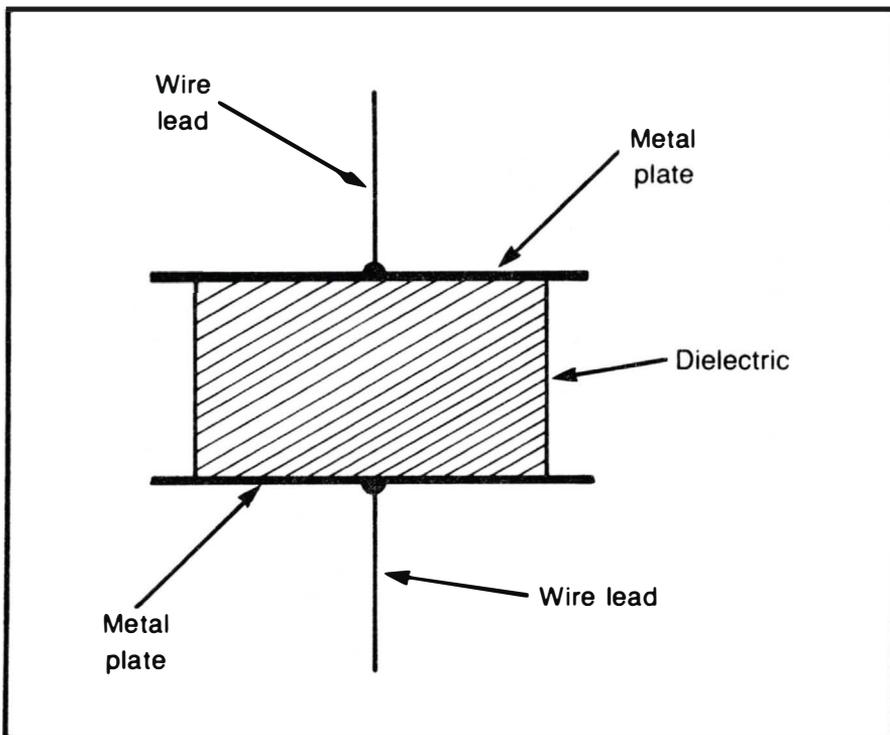
Fig. 4-8. Simplified cross-sectional diagram of a capacitor.
