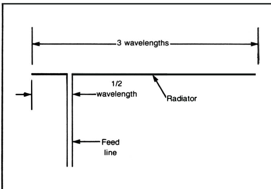
Fig. 6-18. Voltage feed for a three-wavelength longwire.
