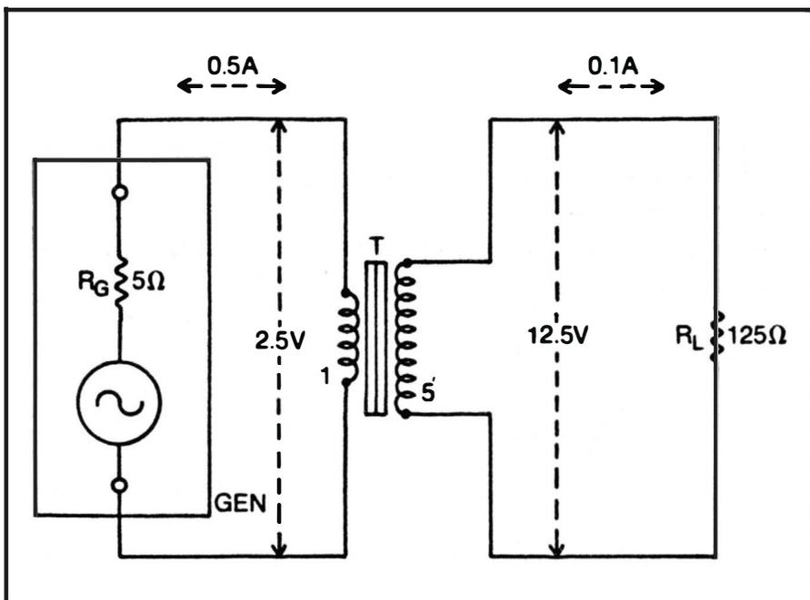
Fig. 2-14. Impedance-matching transformer.
