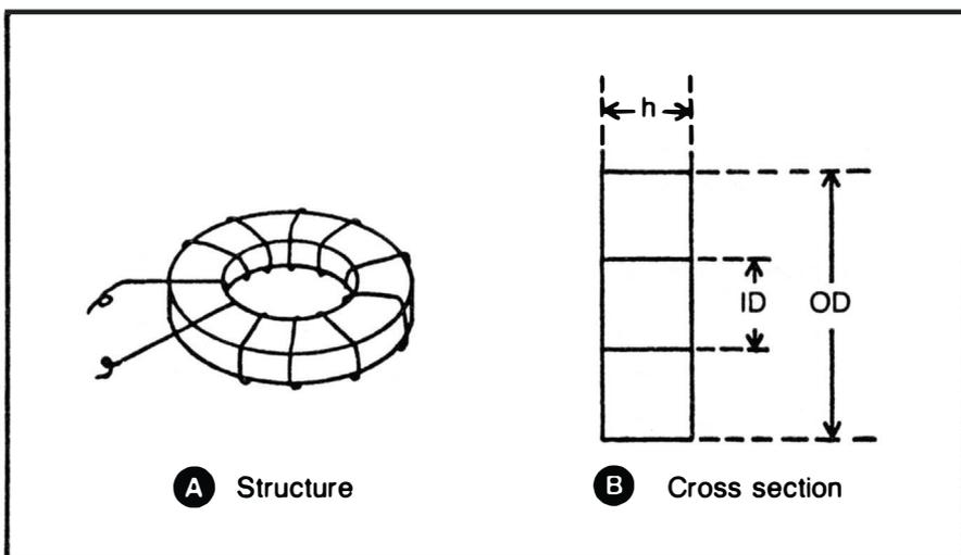
Fig. 4-4. Illustration of coils with toroidal cores showing (A) structure and (B) the cross section.
