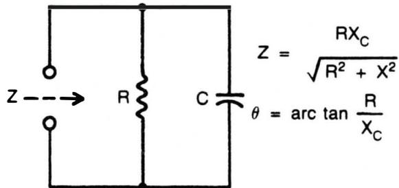
**D** Resistance and capacitance in parallel
