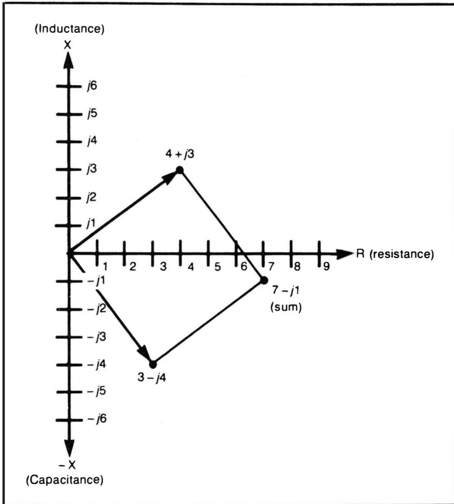
Fig. 5-8. Addition of vectors by the parallelogram method.
