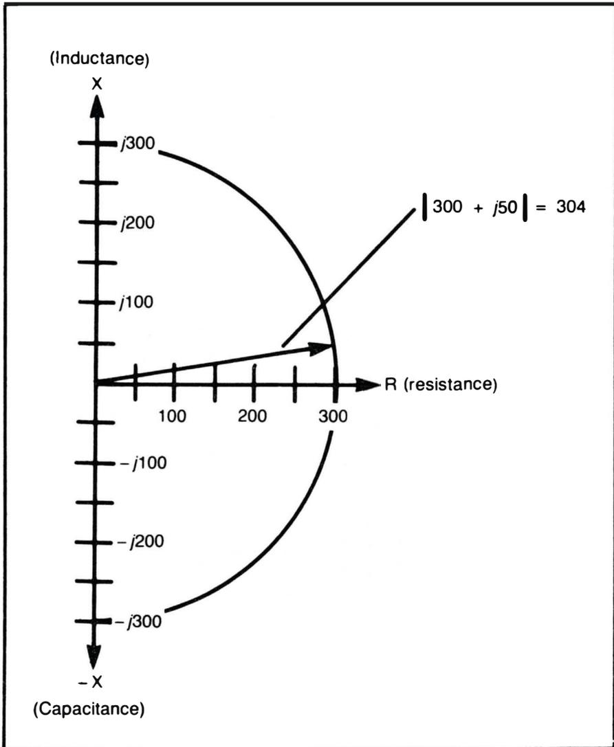
Fig. 5-6. For any particular absolute value of impedance, the representation in the complex plane is a half circle, in this case with a radius of 304.
