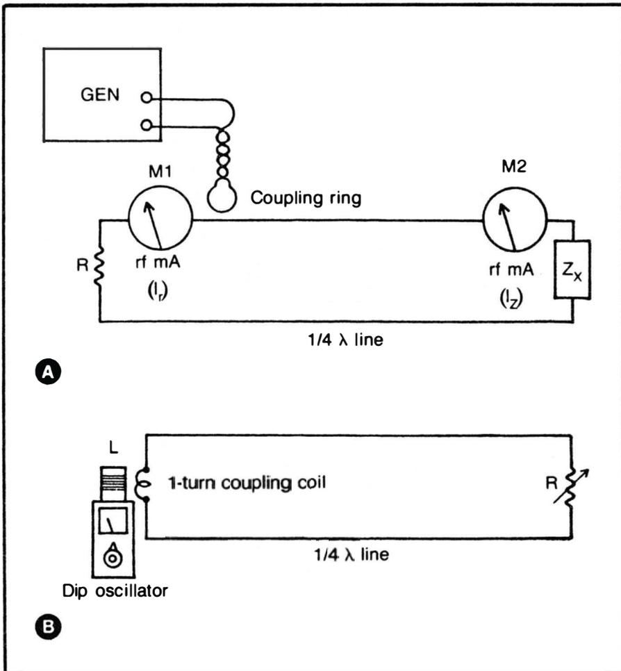
Fig. 3-7. Practical uses of the transmission line method to measure impedance: (A) using a noninductive resistor; (B) using a dip oscillator.
