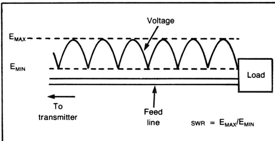
Fig. 6-5. Voltage distribution along a line terminated in a resistance different from the characteristic impedance.
