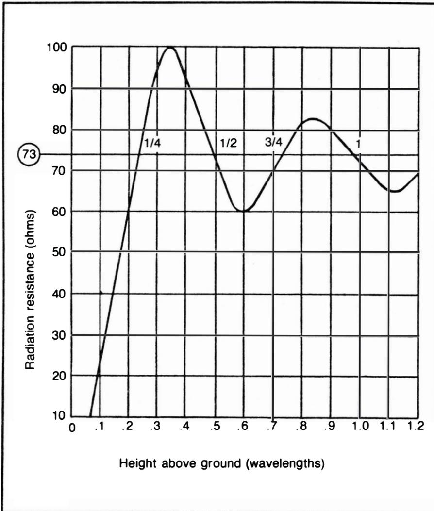
Fig. 2-5. Radiation resistance of a half-wave horizontal antenna plotted for various heights from zero to two wavelengths above ground.
