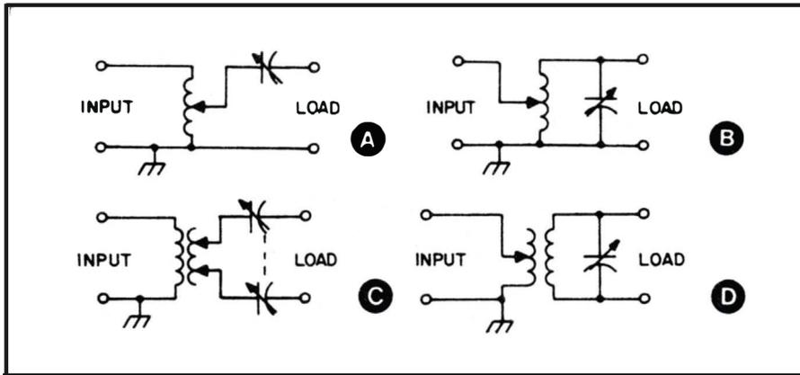
Fig. 6-19. Four commonly used types of transmatches. At (A) is a circuit for unbalanced loads having low impedance. At (B) is a circuit for unbalanced loads having high impedance. At (C) is a circuit for balanced loads having low impedance. At (D) is a circuit for balanced loads having high impedance.
