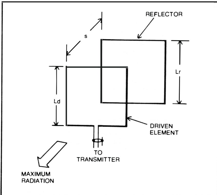
Fig. 6-16. Configuration of a two-element quad antenna.
