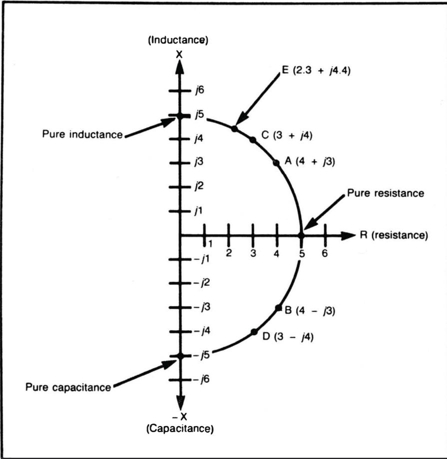
Fig. 5-9. Eight ways to produce an absolute-value impedance of 5 ohms.
