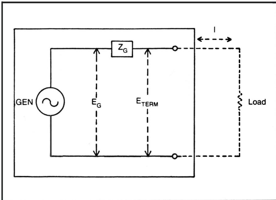
Fig. 2-9. Circuit illustrating impedance ( $Z_G$ ) of an ac generator.
