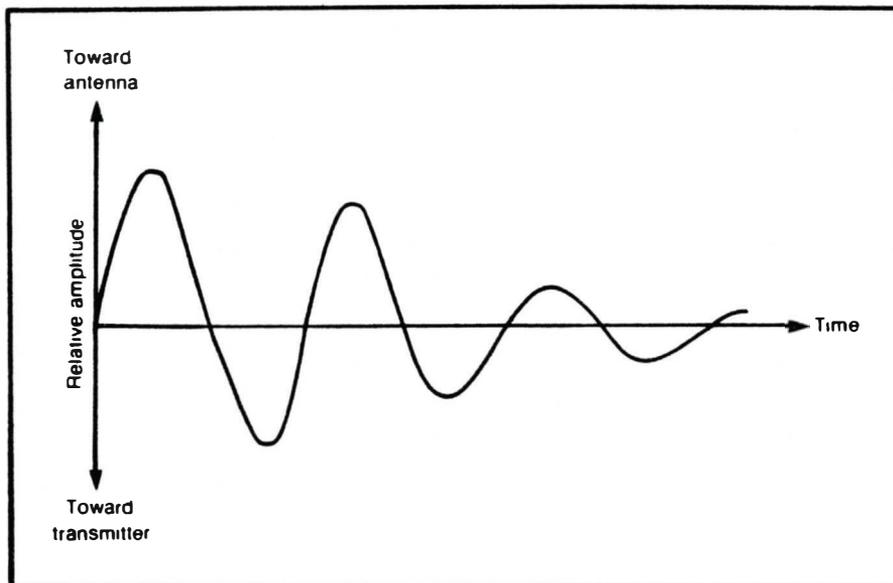
Fig. 6-6. Amplitude of reflected power in a feed line not terminated in a perfect match, as a function of time. Note the directional distinction on the vertical axis.
