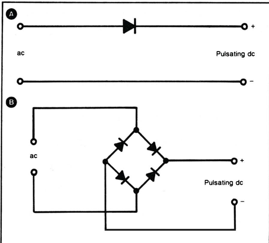
Fig. 1-10. At (A), a half-wave rectifier; at (B), a typical full-wave rectifier circuit.
