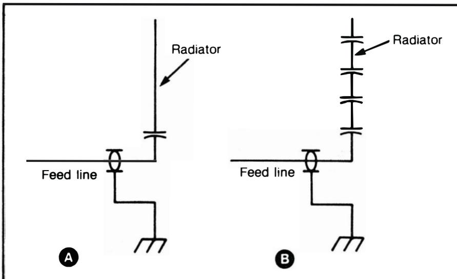
Fig. 4-11. Examples of series connection of capacitors to raise the resonant frequency of an antenna. At (A) is a single capacitor. At (B) are several capacitors spaced along the length of the radiator.
