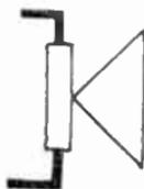
**V o l u m e Control.**—Now regarding the volume control. A powerful local station will, of course, give a much stronger signal than a distant one and, therefore, it would overload the output stage of a receiver operating without grid bias. To give the operator a means of preventing this overloading a *volume control* is used. The
