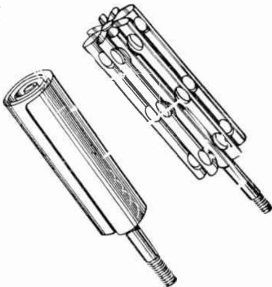
Fig. 50.—Two typical anode designs used in electrolytics.
