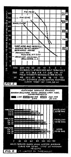
in the wide-band system of F.M. espoused by Major Armstrong. The pros and cons of such characteristics as fidelity, noise threshold, triangular noise spectrum, deviation ratio, field intensity, etc., upon which tests were made at a cost of \$30,000 by N.B.C., were described.
