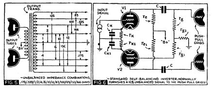
riety of impedances, which are obtained either by balanced or unbalanced loading. A balanced loading circuit is illustrated in Fig. 4. Figure 5 shows the unbalanced output terminals available, ranging from 0.175ohm to 166 ohms. It will be noted that a total of 16 impedance combinations are available, ranging from 0.175-ohm to 500 ohms.
