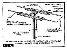
obtain the requisite rigidity, only wire of a heavy gauge, either No. 10 or No. 12, should be used, supported by low-loss insulators. The transmission line must be run at right-angles to the dipole for at least a ¼-wavelength, at least 5 feet, before any bends in the line are made.
