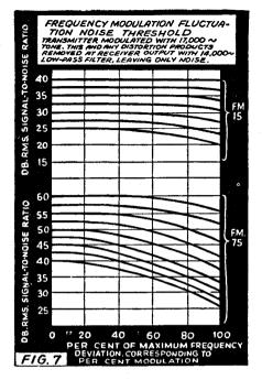
when the noise peaks equal or exceed the peaks of the carrier. The result is a rapid increase of the noise level or decrease of the signal-to-noise ratio with modulation.
