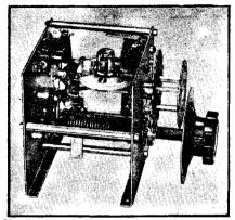
Chassis of the Weston model 787 oscillator tuner,
