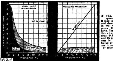
✓ Fig. 4. High-frequency pre-emphasis is used in the transmitter and de-emphasis is used in the receiver to improve the signal/noise ratio. The importance of this characteristic in ultra - H.F. broadcating and its greater effectiveness in F.M. are illustrated at left. Comparison is on the same scale of relative amplitude.
