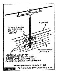
Fortunately, the current and voltage distribution on a half-wave doublet or dipole antenna, which is the most effective and popular type employed for F.M. reception, is such that the voltage at the center of the dipole is theoretically zero. This is shown at Fig. 1. For this reason, and since the 2 sections of the antenna are generally sup-
