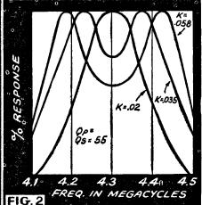
characteristics, which are symmetrically loaded with shunt resistors across the primary and secondary. These resistors have the two-fold purpose of providing (a) the proper Q and (b) a dissipative circuit which prevents the rapidly changing frequency from setting up transients. The latter may be heard as a "fuzz," particularly on loud, high-frequency passages.
