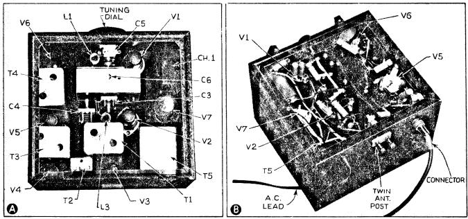
The aeat and compact construction of this new F.M. Adapter is illustrated in photo A. Even an underview, photo B, will not scare the constructor.
