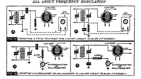
precaution mentioned in connection with matters without zero center must be observed. It is possible to change the zero adjustment of the meter to read up-scale to avoid slamming of the needle off-scale when the secondary trimmer is adjusted.
