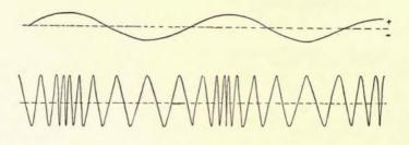
FIG. 25—Frequency modulation of a carrier current, using the same alternating current wave as that in figure 24.
