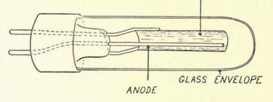
FIG. 3-Construction of a photoelectric cell.
