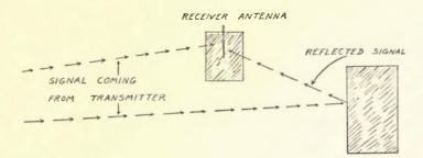
FIC. 48—Diagram showing double signal reception by an antenna; one signal coming direct from the transmitter, the other being reflected from a tall building behind the home of the televiewer.
