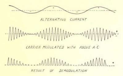
FIG. 24—Amplitude modulation of a carrier current.
