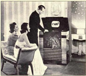
Courtesy Radio Corporation of America Fig. 50—Here the image is seen reflected in a mirror.
