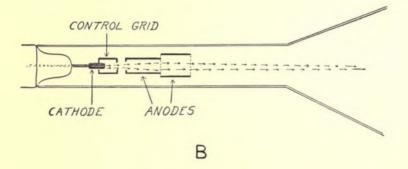
FIG. 15—A, Braun's cathode ray tube, with arrows indicating electron stream; B, portion of modern cathode ray tube used in television, showing the units of the electron gun, or electronemitting and control apparatus. Arrows indicate electron beam.
