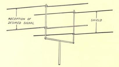
FIG. 49—A dipole television antenna, with a shield (looking like the receiving portion) to absorb unwanted signals.
