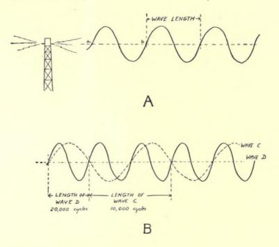
FIG. 27—A, an electromagnetic wave leaving the transmitting antenna; B, two electromagnetic waves with one having twice the frequency of the other.
