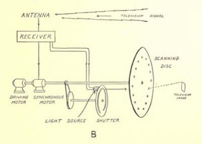
FIG. 9-An early Baird television apparatus.
