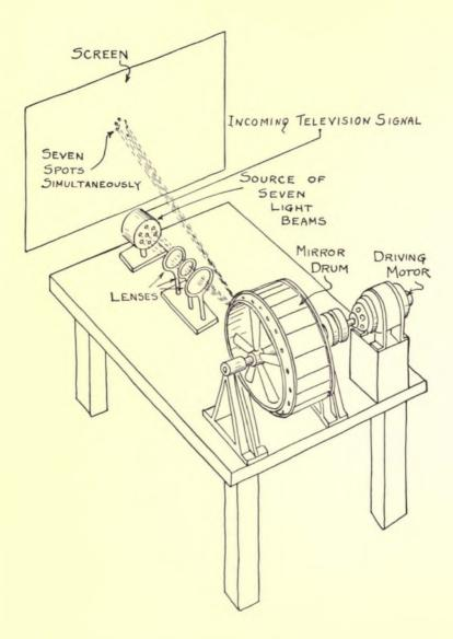
FIG. 11—The mechanical television system developed by Alexanderson, which used a mirror drum for scanning.
