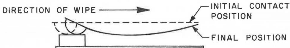
Figure 4-19. Exaggerated Wiping Action of Relay Contacts
