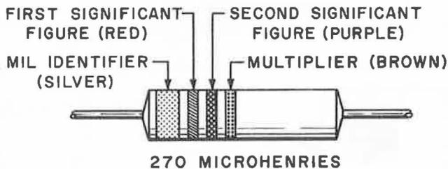
It is significant to note that there have been isolated instances when, for no apparent reason, the manufacturer has not followed this marking code. If there is any question or doubt about the value of a choke, it should be checked by actual measurement on a suitable bridge.
