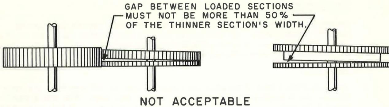
Figure 4-6. Separation of Sections of Loaded Gears
