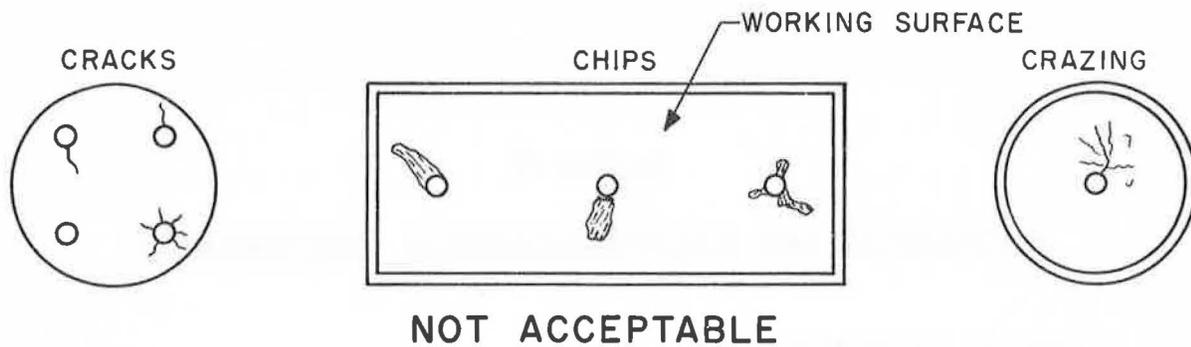
Figure 4-1. Cracks, Chips and Crazing around Sealed Terminals
