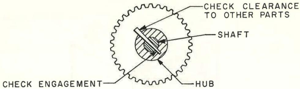
Figure 4-21. Pin Engagement and Clearance Checks
