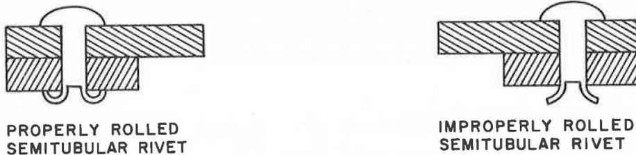
Figure 3-23. Rolled Semitubular Rivet
