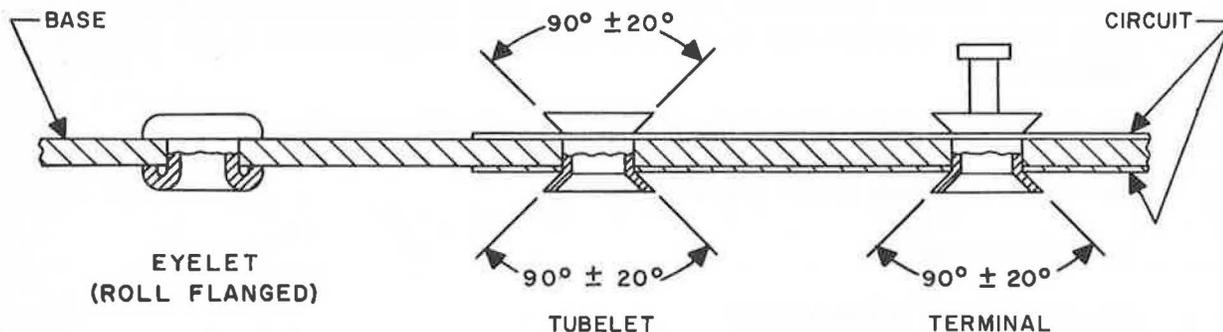
Figure 5-1. Eyelet, Tubelet and Terminal on a Board
