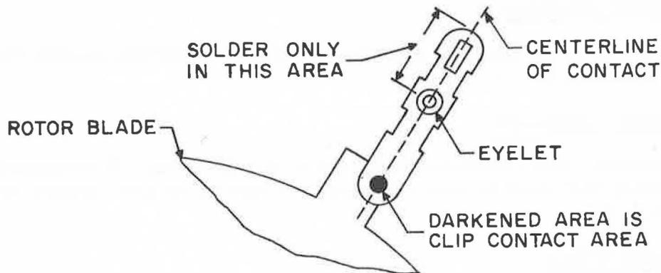
Figure 4-18. Wafer Switch Soldering and Contact Areas
