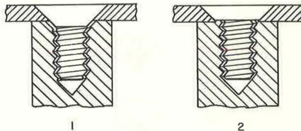
Figure 3-2B. Using Flathead Screws on a Thin Panel
