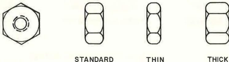
Figure 3-10. Nut Thickness
