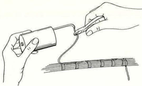
Step F. Cut, leaving enough cord to terminate as in step 8 through 13, figure 1-8B. Also cut off excess cord at Collins knot at start of lacing.
