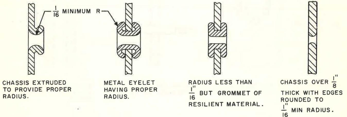
Figure 1-1. Protection for Wire Through a Hole
