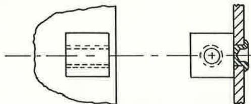
Figure 3-13. Typical Angle Nut
