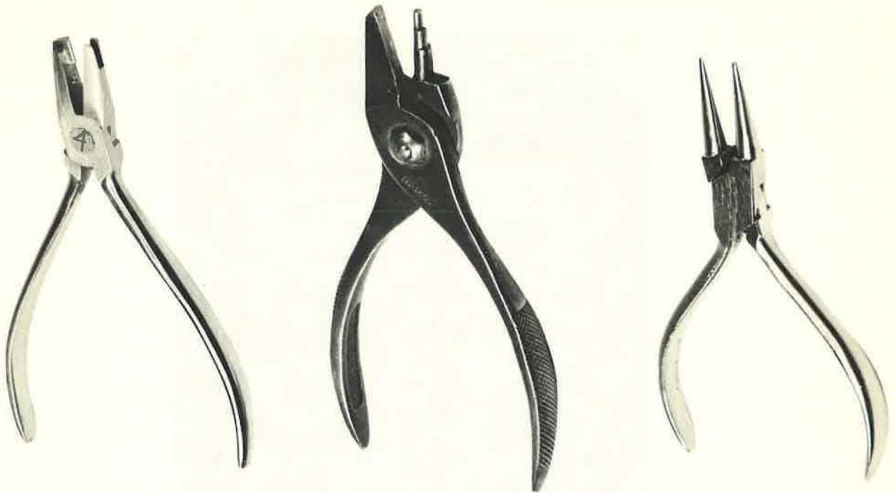
Figure 2-2. Examples of Specialized Pliers for Lead Forming
