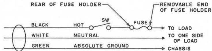
Figure 1-25. Correct Method of Connecting 3-Wire AC Cord for 115 Volts
