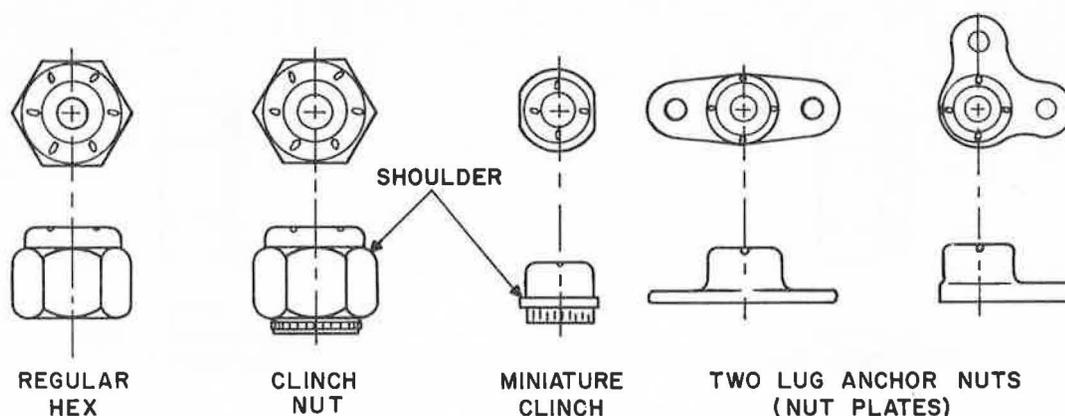
Figure 3-14. Common Elastic Stop Nuts
