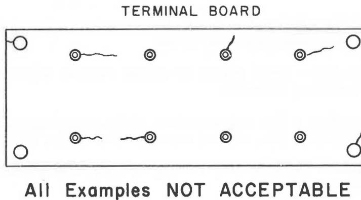
Figure 4-2. Unacceptable Cracks in a Terminal Board
