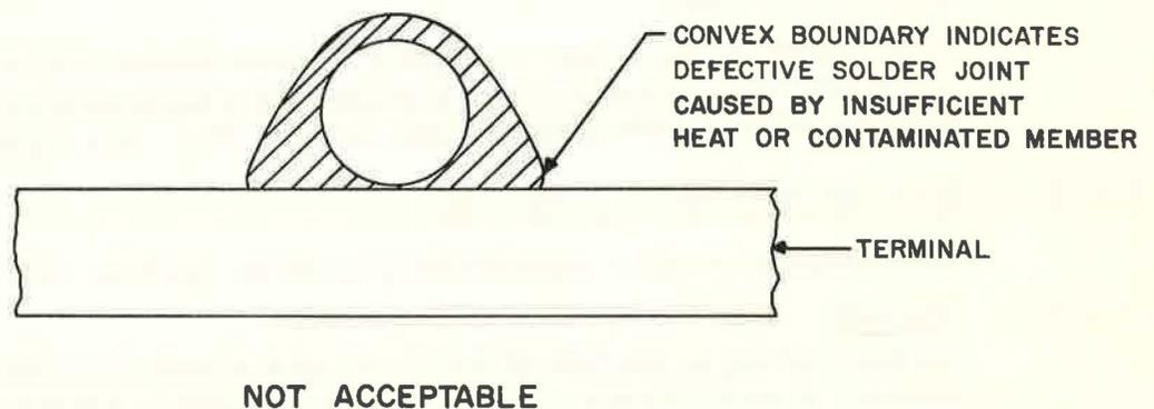
Figure 1-21. Section of Unacceptable Soldered Joint
