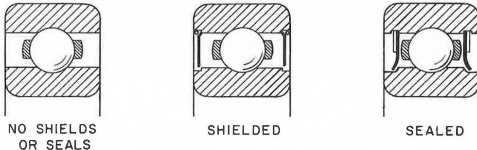
Figure 4-13. Typical Ball Bearing Constructions
