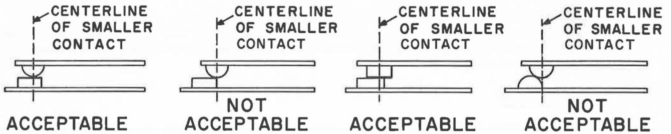
Figure 4-17. Contact Alignment for Low Current Applications
