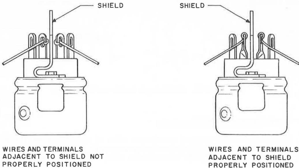
Figure 1-17. Miniature Tube Socket with Shield
