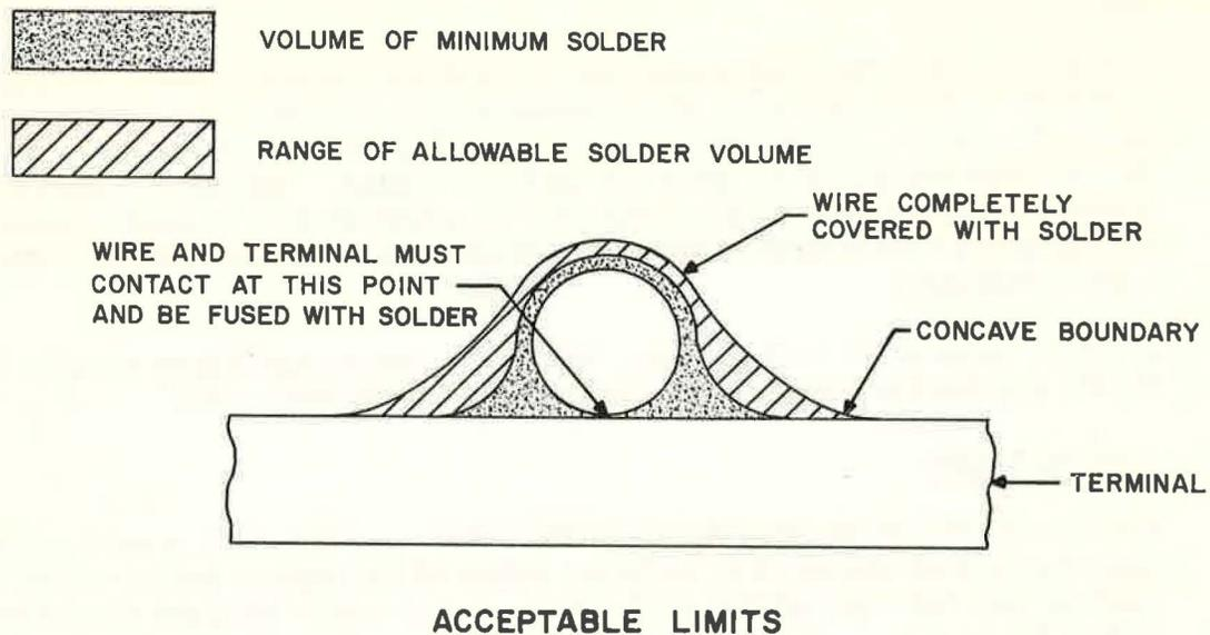
Figure 1-20. Section Showing Acceptable Limits of Solder Volume
