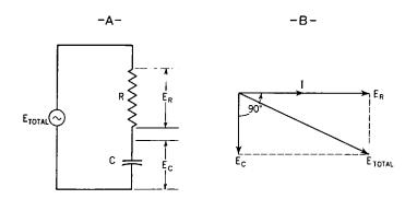
Fig. 35-6. A -Circuit with resistance (R) and capacitance (C) in series. B—Vector diagram showing how the voltage drop across the resistor ( $E_R$ ) is added to the voltage drop across the capacitor ( $E_c$ ).
