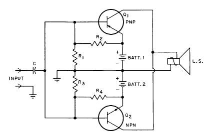
**Fig. 28-14.** Circuit of a stage of complementary push-pull a-f amplification.
