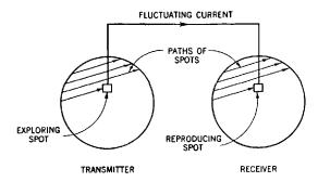
**Fig. 43-19.** The basic principle of lelevision. The two spots keep in step with each other.
