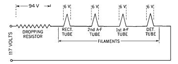
**Fig. 21-2.** Diagram showing how the dropping resistor and the filaments of the rectifier, detector, and first and second audio-frequency amplifier tubes are connected in series across the 117-volt house line.
