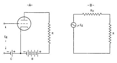
Fig. 38-12. A -Circuit of the triode as an amplifier. B-The equivalent circuit of A.
