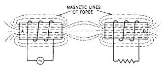
Fig. 33-3. Diagram showing magnetic coupling between two inductors.
