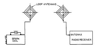
The loop antennas may be made by winding about 15 turns of bell wire on crossed dowel sticks, spacing the turns about 1 in. apart. Place the spark coil in a felt-lined box to absorb the spark noise. The radio receiver will pick up the spark over a fairly large distance.
