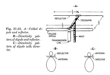
5 per cent longer than the antenna mounted parallel to it and a quarter-wavelength behind it (that is, away from the desired transmitting station). The directivity pattern resulting from such an array is shown in Figure 37-31B.
