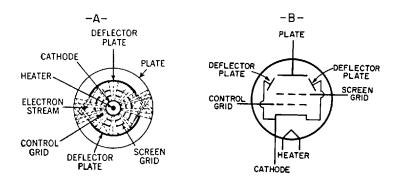
Fig. 27-12. A-Looking down on beam power tube, showing electron streams threading their ways through the grids. B-Symbol of the beam power tube.
