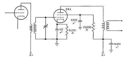
Fig. 27-8. Circuit of a stage of radio-frequency amplification using the 24A type of screen-grid tube.
