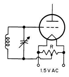
**Fig. 19-3.** Circuits showing the use of a 20- to 40-ohm center-tapped resistor (R) to reduce hum.
