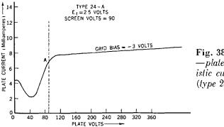
Fig. 38-13. Plate-current —plate-voltage characteristic curve for the tetrode (type 24-A).
