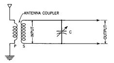
**Fig. 35-12.** The luning circuit of the radio receiver as a resonant circuit.
