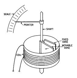
Fig. 32-23. Diagram of a moving-vane a-c meter.
