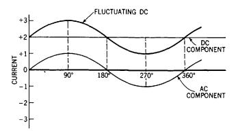
Fig. 32-22. Curves showing how a fluctuating direct current may be broken down to its steady d-c component and its a-c component.
