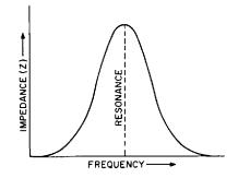
Fig. 35-19. Resonance curve for the parallel resonant circuit with impedance (Z) plotted against the frequency (f). C and L are kept constant.
