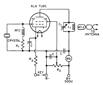
Close the key. The transmitter is now oscillating. This condition is indicated by the drop in plate current as shown on the milliammeter. If a 2-watt lamp is touched to the plate-circuit tank coil, the lamp will glow. Observe the caution against connecting this set to an antenna.
