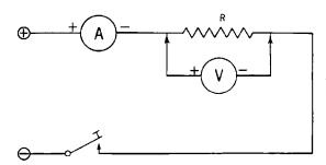
**Fig. 31-28.** The voltmeterammeter method of finding the resistance of (R).
