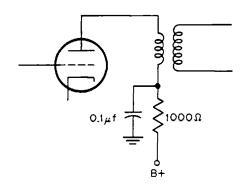
Fig. 23-12. How a decoupling filter is used to bypass any radio-frequency current leaking across the B supply.
