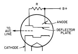
Fig. 43-8. How the triode and tuning eye are contained in one envelope.
