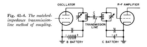
tance apart and yet be able to transfer the excitation from the oscillator to the radio-frequency amplifier. Figure 41-4 shows one type of such a transmission line.
