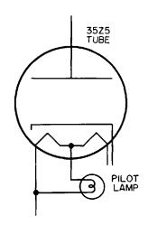
Fig. 21-5. How the tap on the heater of the type 35Z5 rectifier tube is used to supply current to the pilot lamp.
