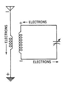
Now let us examine the electron flow in the tuning circuit. You will recall that this circuit consists of a capacitor and inductor connected together. We will examine each part separately, with special attention to the behavior of the electrons.
