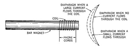
**Fig. 7-3.** This diagram shows the positions of the diaphragm as a fluctuating current flows through the electromagnet of the phones. The bending of the diaphragm is greatly exaggerated in this drawing.
