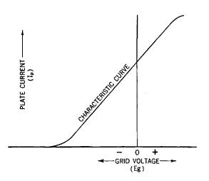
**Fig. 38-5.** The grid-voltage—plate-current characteristic curve for a triode.
