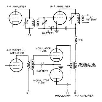
Fig. 42-7. Plate modulation, transformer coupling. Neutralization is omitted for the sake of simplicity.
