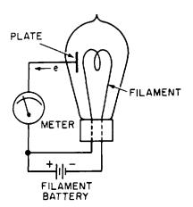
Fig. 14-1. A diagram of Edison's experiment.
