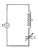
Fig. 35-9. Use of a variable capacitor to vary the resonant frequency of the circuit.
