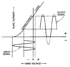
Fig. 39-4. Distortion of the signal due to overloading.
