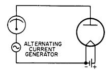
received a negative charge. This charge repelled the electrons from the filament, and the meter showed that no current was flowing. The effect of this action upon the graph of the waveform is shown in Figure 14-5. Only a pulsating direct current is passing through the meter.
