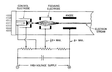
**Fig. 43-10.** Voltage relationship between the various portions of the electron gun.
