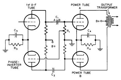
Fig. 27-5. The phase-inverter circuit.
