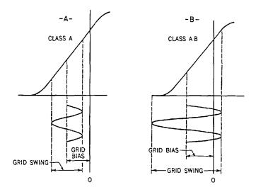
Fig. 39-7. Graphs showing how a greater grid swing is possible with the class AB amplifier.
