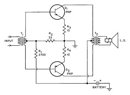
Fig. 28-13. Typical push-pull transistor circuit.
