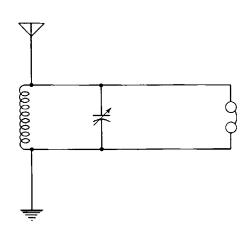
Fig. 8-1. Diagram of the antenna-ground system and the tuner connected to a set of phones. This circuit will not work.
