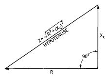
**Fig. 34-12.** Diagram showing how to add resistance (R) and capacitive reactance (Xc) in series.
