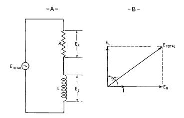
Fig. 35-5. A—Circuit with resistance (R) and inductance (L) in series. B—Vector diagram showing how the voltage drop across the resistor  $(E_R)$  is added to the voltage drop across the inductor  $(E_L)$ .
