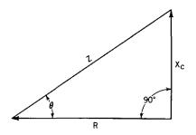
Fig. 34-13. Diagram showing the calculation of the power factor.
