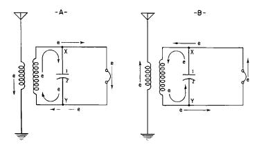
Fig. 13-1. Parallel circuits. A—Flow of electrons during a half-cycle. B—Flow of electrons during the next half-cycle.
