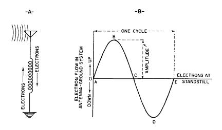
Fig. 11-4. A—Electrons flow up and down the antenna-ground system.
