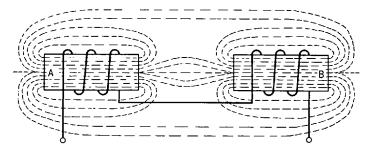
**Fig. 33-4.** Inductors in series with their magnetic fields aiding each other. Note the windings are in the same direction on both coils.
