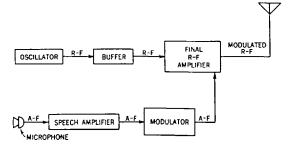
amplifier should be modulated. This final ampifier may be a class C amplifier with the advantage of greatest efficiency.
