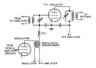
Fig. 42-9. Grid modulation, transformer coupling.
