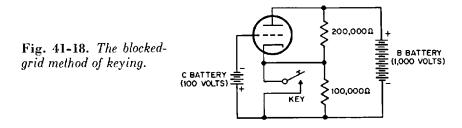
the grid circuit controls the excitation to the grid of the tube. Since the voltages involved in this circuit are relatively low, this method of keying is preferred.
