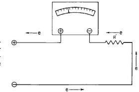
Fig. 31-23. Circuit showing how the galvanometer is used to measure the electriccurrent flowing through a resistor (R). current into it so that it does rotate in this clockwise direction, else the pointer may be twisted. For this reason, the binding posts are marked plus (+) and minus (-), respectively. The plus binding post must be connected to the positive side of the electrical circuit, and the minus binding post to the negative side.
