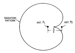
Fig. 37-25. Unidirectional pattern (cardioid) for two vertical, half-wave antennas, a quarter-wave apart with currents 90° out of phase.
