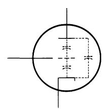
Fig. 23-8. Diagram showing the capacitive effect existing between the electrodes of the triode. The result is the same as if small capacitors were connected between the electrodes.
