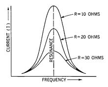
Fig. 35-16. Resonance curves showing changes produced by changes in resistance (R). Inductance and capacilance are kept constant.
