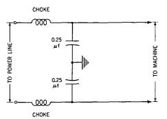
**Fig. 36-11.** Filler circuit to prevent radio-frequency currents set up by a sparking machine from traveling back into the power lines.
