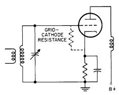
Fig. 39-20. Diagram showing that the grid-cathode resistance of the tube is in parallel with the tuned circuit.
