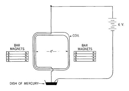
The coil consists of about 25 turns of bell wire. Both ends are bared. One end is connected to a piece of thin copper wire (No. 30 or finer) which suspends the coil. The other end dips into a small dish of mercury. A 6-volt battery is connected to the coil through the thin wire at one end and the mercury at the other.
