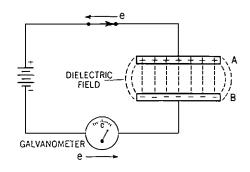
Fig. 34-2. Capacitor being charged.
