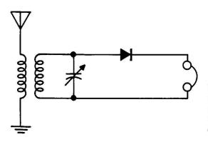
Fig. 10-6. An improved crystal receiver, using an antenna coupler. This set will tune sharper than the one shown in Fig. 8-3.
