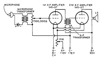
Fig. 17-14. Diagram showing circuit of the public-address system.
