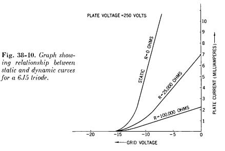
How We Use the Characteristic Curves. An examination of the family of curves shown in Figure 38-8 shows us the interrelation of the grid-bias voltage, the plate voltage, and the plate current. Knowing any two values will give us the third. Thus, if we know we are to apply a grid bias of -8 volts to the 6J5 tube and place 250 volts on the plate, we can determine the plate current that will flow during the
