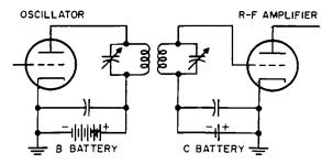
Fig. 41-3. The inductive method of coupling the oscillator to the radio-frequency amplifier.
