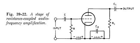
alternating-current signal voltage, but keeps the direct-current plate voltage off the grid of the following tube.  $C_2$  is a bypass capacitor.
