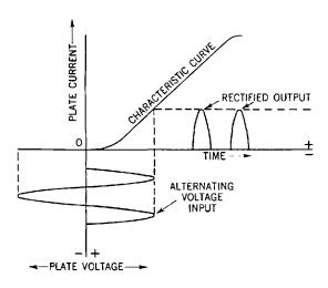
Fig. 38-3. How the characteristic curve of the diode is used to show the relationship between voltage input and the current output.
