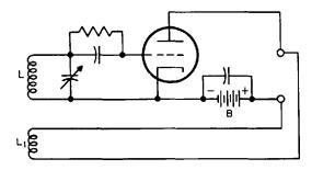
Fig. 40-3. The output is fed back into the oscillatory circuit by means of an inductor  $(L_1)$ .
