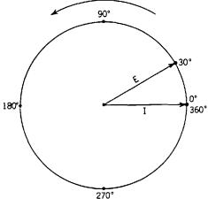
Fig. 32-18. Vector diagram showing the current (I) lagging 30° behind the emf (E). Compare this diagram with the curve in Figure 32-15.
