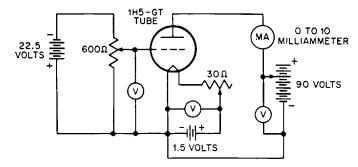
(a) Keeping the grid bias fixed, vary the plate voltage and draw the  $I_p$ - $E_p$  characteristic curve.
