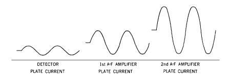
**Fig. 17-2.** Graphs showing plate current in the detector, the first audio amplifier, and the second audio amplifier.
