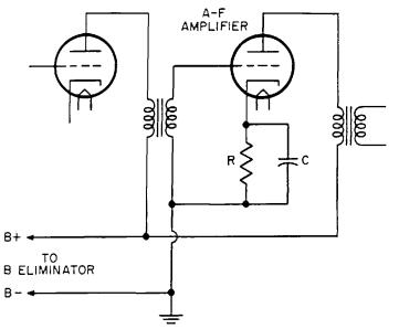
Fig. 20-4. Circuit showing cathode resistor (R) and bypass capacitor. (C).
