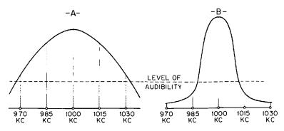
**Fig. 26-11.** *A*-Tuning curve for the tuned radio-frequency receiver tuned to 1,000 kc. Note that stations whose frequencies are 970 kc and 1,030 kc lie above the level of audibility. This condition means that they may be heard faintly in the background of the desired station.
