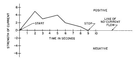
**Fig. 9-3.** Graph of the curve or waveform of a fluctuating direct current. Note that the strength of the current may assume different values at different times.
