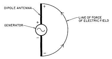
Fig. 36-1. An electric field exists between the wires of the dipole antenna.
