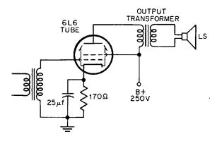
Fig. 27-14. Circuit of beam power tube used as a power tube.
