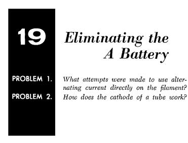
Attempts to Use Alternating Current for the Filament. The next battery to be eliminated was the A or filament battery. It is simple enough to use a step-down filament transformer to reduce the voltage from the 117-volt alternating current to  $1\frac{1}{2}$ -volt alternating current. But alternating current is unsatisfactory for heating the filament of the radio tube even at this reduced voltage.
