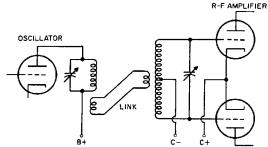
portant differences, however. Whereas the tank in the grid circuit is tuned to the same frequency as is the oscillator (the fundamental frequency), the tank in the plate circuit is tuned to the harmonic of that frequency (usually the second harmonic). To obtain a rich harmonic output, we need a high negative grid bias on the tube, considerably more than double the cutoff value. The excitation\_voltage must be quite high. (It is suggested that you review Chapter 39 on amplifiers.)
