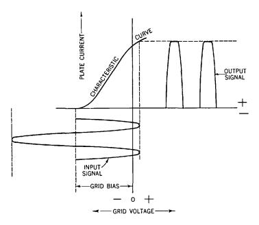
**Fig. 40-4.** Graph showing how plate current goes up as the grid bias approaches zero.
