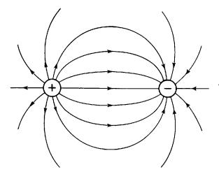
Fig. 31-2. The lines of force between two opposite charges.
