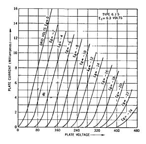
**Fig. 38-8.** Family of plate characteristic curves for the 6J5 triode.
