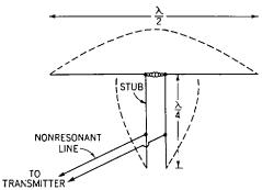
Fig. 37-19. Current distribution on an antenna using quarter-wave matching stub.
