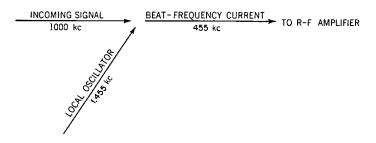
**Fig. 26-1.** Diagram showing how the incoming signal mixes with the current produced by the local oscillator to produce the beat-frequency current.
