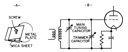
**Fig. 23-15.** *A*—*Trimmer capacitor used to align the radio-frequency amplifier stages.*
