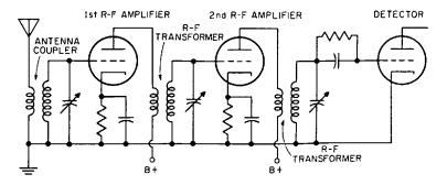
**Fig. 23-2.** Diagram showing the circuit of two tuned radio-frequency amplifier stages.
