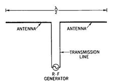
**Fig. 37-12.** Transmission line connecting the r-f generator to the antenna.
