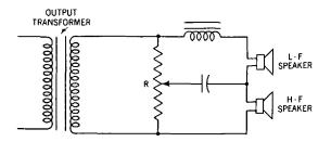
**Fig. 25-4.** Circuit showing how tone control may be obtained through the use of high-frequency and low-frequency loudspeakers. The potentiometer (R) determines which speaker shall obtain the greater current.
