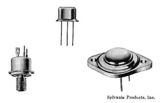
Fig. 28-18. Different types of transistors.
