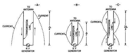
Fig. 37-13. Standing waves of current on resonant transmission lines of various lengths.
