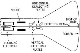
Fig. 43-11. The cathode-ray tube.
