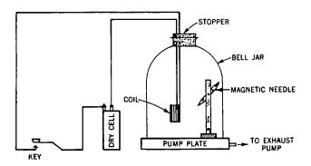
**Fig. 3-1.** This apparatus shows that electric current flowing through a coil of wire will set up a magnetic field around that coil. This field is created even though the coil is surrounded by a vacuum.
