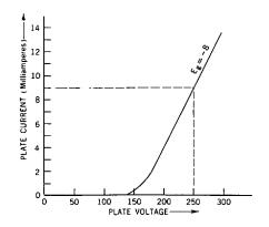
**Fig. 38-11.** Plate-current—platevollage characteristic curve for the 6J5 triode. Grid bias is -8 volts.
