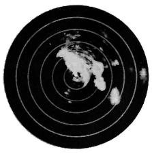
Fig. 43-24. PPI radar screen located in an airplane showing the presence and location of storm clouds ahead.
