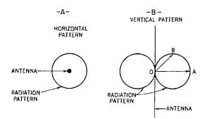
Fig. 37-21. Radiation pattern of a vertical antenna. A—The horizontal
