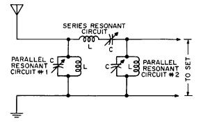
Fig. 35-32. Diagram showing how series and parallel resonant circuits are used to allow signals of only one band of frequencies to pass. The bandpass filter.
