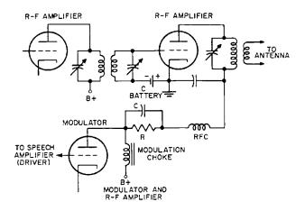
Fig. 42-8. Plate modulation, choke coupling.
