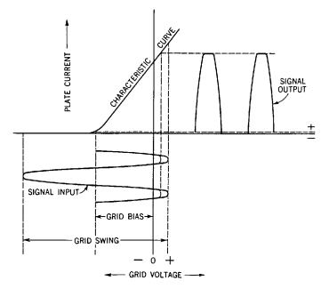
**Fig. 39-8.** Graph showing relationship between the input and output signals in a class B amplifier.
