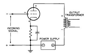
this primary winding are 180° out of phase with each other. Also, the grid and plate of the tube are 180° out of phase with each other.
