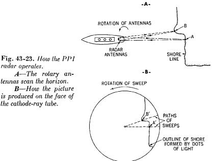
along a radius to the periphery, and back to the center (see Fig. 43-23B). Further, the stream can be rotated around this center. The rotation of this electron stream is synchronized with the rotation of the radar antennas.
