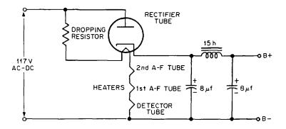
**Fig. 21-4.** Diagram showing the circuit of the complete ac-dc power supply. The symbol 15h stands for a filter choke coil of 15 henrys.
