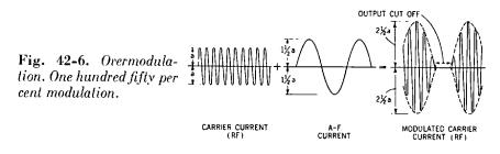
cut off. The waveform of the signal heard in the loudspeaker of the receiver will not be equal to that of the original. In consequence, we have distortion.
