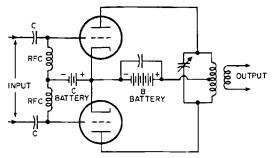
Fig. 41-6. The push-pull radio-frequency amplifier.
