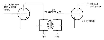
**Fig. 26-10.** Circuit of an intermediate-frequency transformer employing fixed capacitors and movable powdered-iron cores for tuning.
