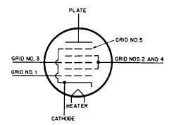
Fig. 27-16. Diagram showing the arrangement of electrodes in the pentagrid converter lube.
