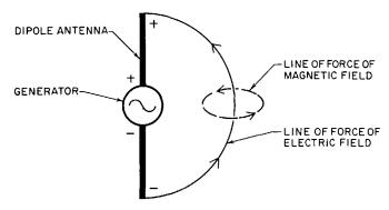
**Fig. 36-2.** A moving electric field produces a magnetic field. (The solid line indicates the line of force of the electric field, the dashed line the line of force of the magnetic field.)
