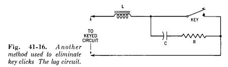
In what stage should the key be placed? Since an open key is required to cut off all radiation, it may be placed in any stage and in any circuit of that stage which will make it inoperative, thereby breaking the radio-frequency signal chain to the antenna. It should be pointed out that if a stage is keyed, the succeeding stages must have sufficient fixed bias to prevent the flow of damaging currents, which would result from no grid-exciting signal.
