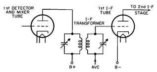
Fig. 26-8. Circuit of the intermediate-frequency transformer.
