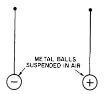
Fig. 30-9. Figure showing two oppositely-charged balls suspended far apart in air. Although there is a potential difference between them, no current flows because the resistance of the path between them is too great.
