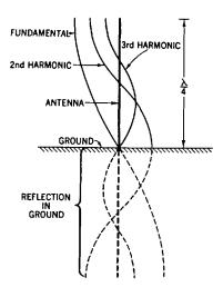
Fig. 37-10. Voltage distribution on a quarter-wave Marconi antenna at the fundamental, 2nd harmonic, and 3rd harmonic frequencies. Only half the voltage wave is shown for the sake of simplicity. Note the voltage loop at the ground for the 2nd harmonic.
