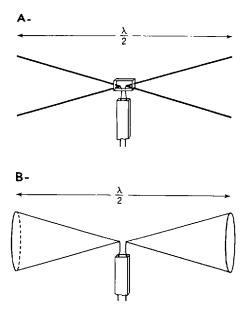
Fig. 37-30. A—The double-V antenna. B—The double-cone antenna.
