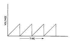
**Fig. 43-15.** Waveform of the output of a sawtooth oscillator.
