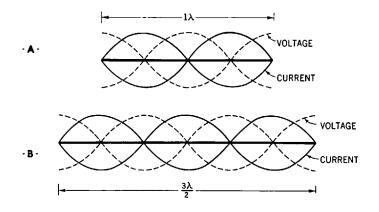
**Fig. 37-6.** *A*—Full-wave antenna, showing distribution of standing waves of current and voltage. *B*—One-and-one-half-wave antenna.
