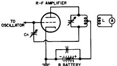
Fig. 41-19. Circuit showing how a radio-frequency amplifier is neu-tralized.
