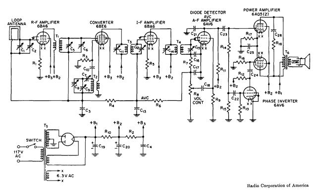
Fig. 29-1. A-C superheterodyne receiver.
