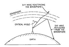
Fig. 36-6. Diagram showing the critical angle. Sky waves of a certain frequency, striking the ionosphere at an angle less than the critical angle, penetrate and do not return to earth. the critical angle penetrate and never return. Those that strike the ionosphere at angles greater than the critical angle are reflected back to earth, as shown in Figures 36-6 and 36-7. The greater the frequency of the sky wave, the greater the critical angle. When
