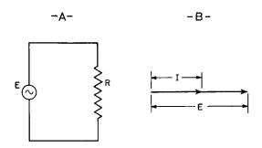
Fig. 35-3. A Circuit containing resistance only. B—Vector diagram showing voltage (E) and current (I) in phase.
