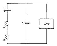
**Fig. 35-26.** The capacitor (C) is now in parallel with the load and acts as a low-pass filter — that is, the low-frequency currents can pass to the load.
