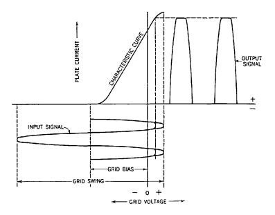
Fig. 39-19. Graph showing relationship between the input and output signals in a class C amplifier.
