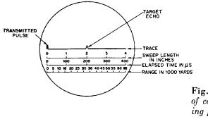
Fig. 43-21. Trace on face of cathode-ray tube showing pips.
