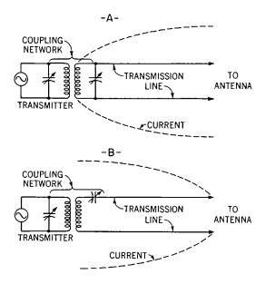
Fig. 37-16. A—Coupling network with a current node at input end of the transmission line.
