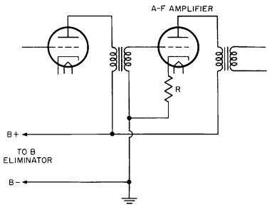
Fig. 20-3. Circuit showing how a cathode resistor (R) is used to get grid bias
