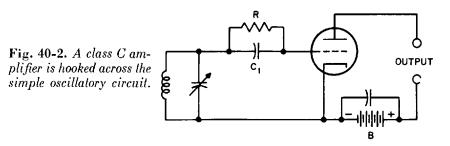
leak (R). As a result, the signal, in greatly amplified form, appears at the output of the tube (Chap. 39).
