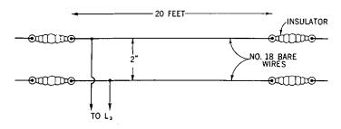
Solder a one-turn loop of wire about  $\frac{1}{2}$  inch in diameter to the base terminals of a low-current flashlight lamp. When this loop is brought near or placed over the end of  $L_2$ , the lamp should glow. Connect the ends of the Lecher system to  $L_3$ . A shorting bar (a metal strip with a knife edge) is slid along the Lecher wires outward from the oscillator until the flashlight shows a sharp dip in brightness. Mark this point on the wires and move on until a second dip is obtained.
