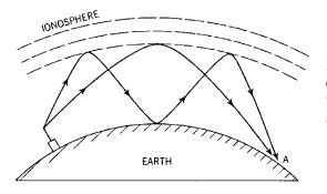
Fig. 36-13. Another cause of fading. Here two sky waves arrive at the same point  $(\Lambda)$  out of step.
