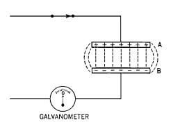
Fig. 34-3. Capacitor fully charged. The battery has been removed.
