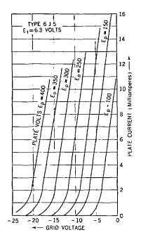
Fig. 38-7. Family of transfer. or mutual-characteristic. curves for the triode (type 6.J5).
