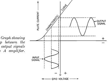
Fig. 39-5. Graph showing relationship between the input and output signals in a class A amplifier.
