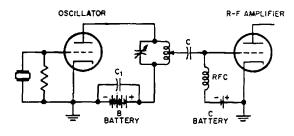
Fig. 41-2. The direct or capacitive method of coupling the oscillator to the radio-frequency amplifier.
