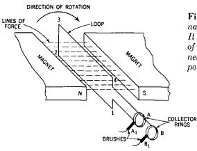
Fig. 32-4. A simple alternating-current generator. It consists of a single loop of wire rotating in the magnetic field between two poles of a magnet. are usually made of copper or carbon. This arrangement of loop, magnetic field, collector rings, and brushes constitutes a simple generator.
