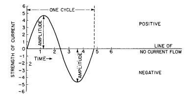
**Fig. 9-4.** Graph of the curve or waveform of an alternating current. A curve whose current strength rises and falls in the smooth, even, and regular glide pictured here is called a sine curve.
