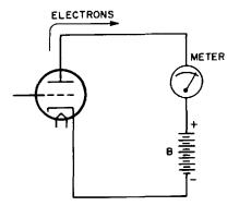
**Fig. 27-1.** Meter connected in the plate circuit of the triode to show the flow of electrons.
