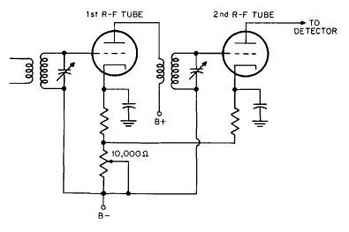
Fig. 24-7. Circuit showing how the rheostal used as a volume control varies the grid bias of both radio-frequency lubes.
