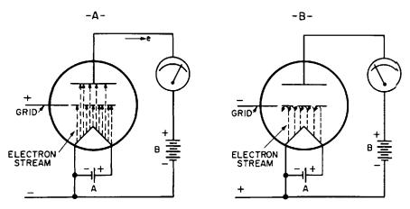
**Fig. 15-3.** A—This diagram shows how a positive charge on the grid of De Forest's tube helps pull electrons from the heated filament to the plate. The meter shows that an electron current is flowing through it.
