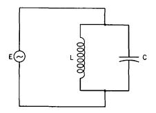
**Fig. 35-17.** The parallel resonant circuit with inductance (L) and capacitance (C) in parallel.
