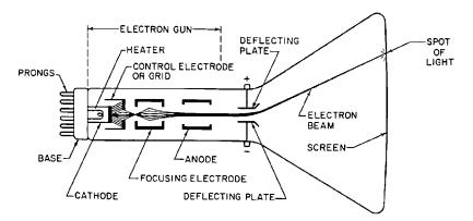
Fig. 43-9. The basic diagram of the cathode-ray tube.
