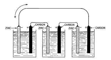
Fig. 30-16. Three voltaic cells in series. Note that in series connections the + pole of one cell is always joined to the - pole of the next cell.
