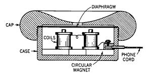
Fig. 7-4. A sectional view of an earphone of the type used in radio receivers. Note how flat it is compared to the telephone receiver. The permanent magnet can be either circular or horseshoe shaped.
