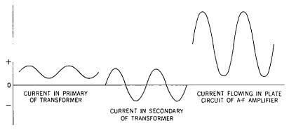
**Fig. 17-5.** Graphs showing current flowing in primary and secondary of the transformer and in the plate circuit of the a-f amplifier. Note that the shape of all three curves is the same although the amplitudes vary.
