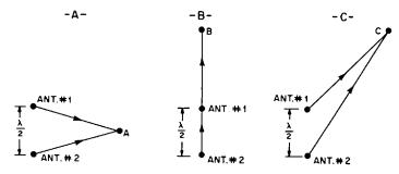
**Fig. 37-23.** Diagrams explaining how the radiation pattern in Figure 37-22 is formed.
