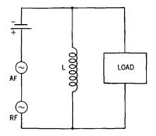
**Fig. 35-27.** The inductor (L) is now in parallel with the load and acts as a high-pass filter—that is, the high-frequency currents can pass to the load.
