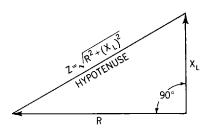
**Fig. 33-2.** Diagram showing how to add resistance (R) and inductive reactance (XL) in series.
