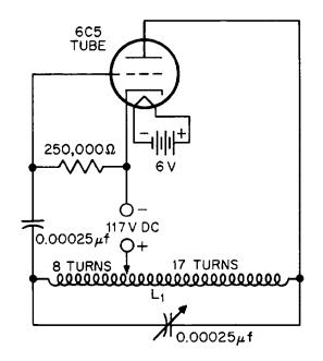
$L_1$  is 25 turns of No. 14 double-cotton-covered wire on a cardboard tube 3 in. in diameter.
