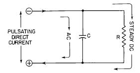
Fig. 34-10. How a capacilor may be used to separate a-c from d-c components of a current.
