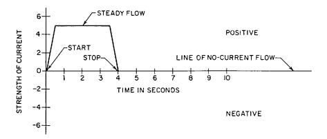
Fig. 9-2. A graph of the curve or waveform of a steady direct current.
