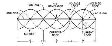
Fig. 37-2. Sinusoidal distribution of current and voltage along an antenna. The Greek letter lambda  $(\lambda)$  is the symbol for the wavelength.
