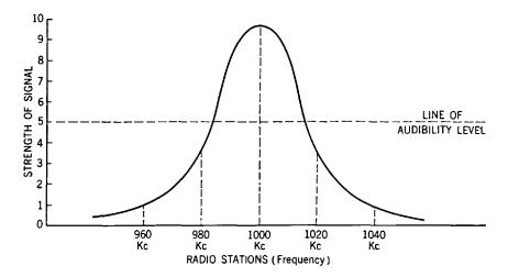
Fig. 10-2. Graph or tuning curve for a sharply tuning receiver. Note that all unwanted radio stations fall below the line of audibility level.
