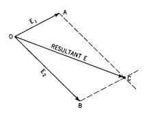
Fig. 32-20. Vector diagram showing how two voltages  $(E_1 \text{ and } E_2)$ are added together to give the resultant voltage (Resultant E).
