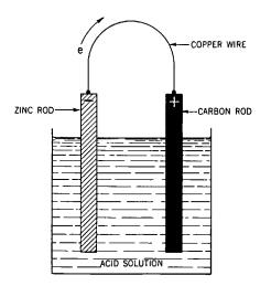
Fig. 30-15. The voltaic cell.
