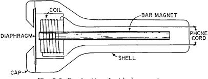
Fig. 7-2. Construction of a telephone receiver.
