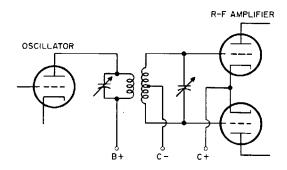
Fig. 41-8. The inductivemethod of coupling a pushpull radio-frequency amplifier to the oscillator.
