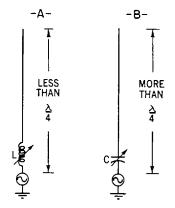
**Fig. 37-11.** A—Adding inductance to an antenna to increase its effective length.
