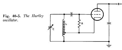
and stability thus increased by using a low L (that is, a low L-to-C ratio). The smaller the inductance, the smaller the dimensions of the coil, and the lower the inherent resistance.
