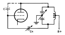
Fig. 39-25. Circuit of a radio-frequency amplifier showing the neutralizing capacitor  $(C_n)$ . This is an example of plate neutralization.
