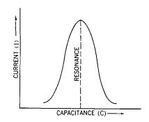
Fig. 35-10. Graph showing the effect on the current (I) as the capacitance of the variable capacitor of Figure 35-9 is changed. The inductance and frequency are kept constant.
