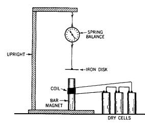
Fig. 7-1. This apparatus is used to show that a varying electric current passing through an electromagnet exerts a varying pull on the iron disk.
