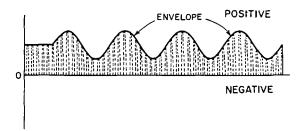
**Fig. 9-11.** Graph of the waveform of fluctuating direct current through the phones. This waveform is indicated by the envelope, which has the same shape as the fluctuating direct current from the microphone in Figure 9-7A.
