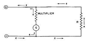
Fig. 31-25. Circuit showing how a voltmeter (galvanometer plus multiplier) is used to measure the voltage of the line.
