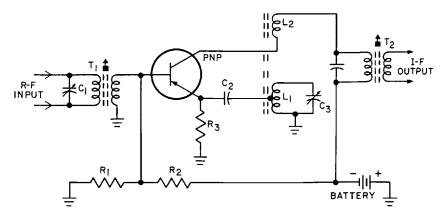
Fig. 28-17. Typical circuit of a transistorized frequency-converter stage.
