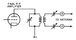
Fig. 41-13. One method of coupling the final radio-frequency amplifier to a center-fed Hertz antenna.
