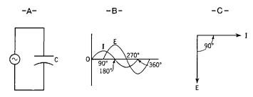
Fig. 34-11. A—Circuit containing capacitance only.
