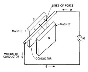
Fig. 32-3. Diagram of a conductor culting across lines of force between poles of a magnet.
