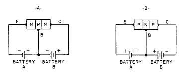
Fig. 28-9. The basic transistor circuit. *A*—*NPN* transistor. *B*—*PNP* transistor.
