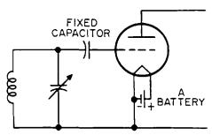
**Fig. 15-11.** This diagram shows how a fixed capacitor is connected to place a negative charge. or bias, on the grid of the triode.
