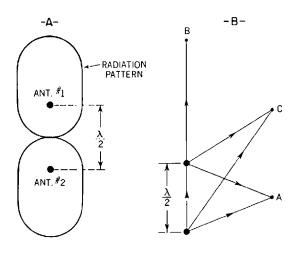
Fig. 37-24. A -The horizontal pattern of two vertical half-wave antennas, a half-wave apart, with their currents 180° out of phase. **B**—Diagram showing how this pattern is formed.
