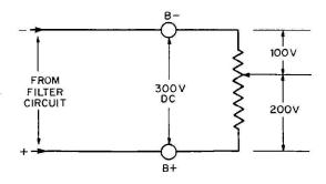
Fig. 18-12. Diagram showing how a potentiometer is hooked up as a voltage divider.
