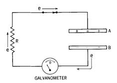
**Fig. 34-4.** Capacitor discharging through resistor (R).
