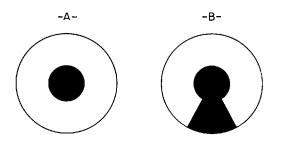
Fig. 43-6. Top view of tuning-eye tube.
