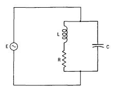
**Fig. 35-18.** The parallel resonant circuit. The resistance is usually found in the inductive branch of the circuit.
