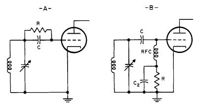
Fig. 39-21. Methods of obtaining grid bias by the grid-leak-capacitor method. *A*—Series method. *B*—Shunt or parallel method.
