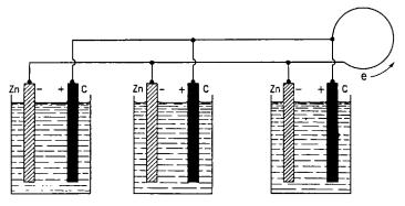
Fig. 30-17. Three voltaic cells in parallel.
