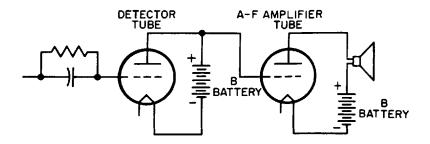
Fig. 17-3. Diagram showing plate of detector tube connected to the grid of the amplifier tube. The filament circuits are omitted for the sake of simplicity.
