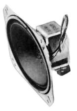
Oxford Components, Inc. Fig. 22-2. Electromagnetic dynamic speaker.
