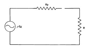
Fig. 39-11. The equivalent circuit for an amplifier.
