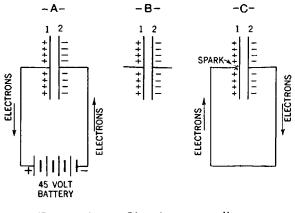
Fig. 12-3. A—Charging a capacilor. B—A charged capacitor. C—Discharging a capacitor.
