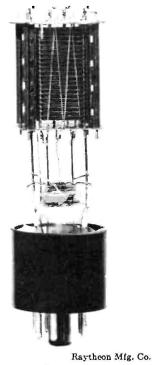
Fig. 15-6. Cutaway view of the triode.
