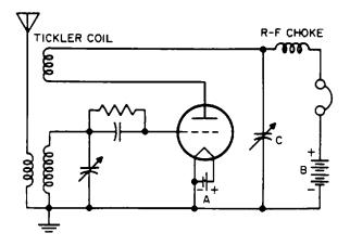
Fig. 16-3. Three-circuit tuner using the variable capacitator (C) to control the amount of feedback. The inductor marked R-F Choke is a small coil of wire used to force some of the plate energy through C.
