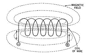
Fig. 31-16. The magnetic field around an electromagnet.
