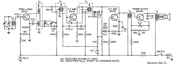
Fig. 29-4. Portable Transistor Receiver.
