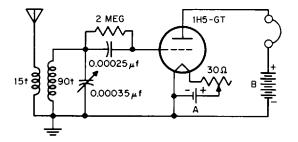
Volume Control. In the filament circuit, between the A battery and one end of the filament, you will notice a device shown by the symbol  $\neg \neg \uparrow \neg \uparrow \neg$ . This is the symbol for a variable resistor, or a *rheostat*, which consists of a length of resistance material, usually wire, over which slides a movable contact. This
