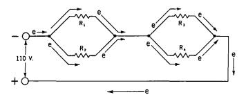
Fig. 30-14. Another arrangement of the series-parallel circuit.
