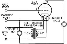
Place a 1 or 2 watt split-plate neon lamp into socket No. 1 to show how both plates are illuminated on alternating current. If direct current is available show how only one plate (the negative) is illuminated. Now place the neon lamp into socket No. 2. Only one of the neon plates lights up, showing that the alternating current has been rectified to direct current by the diode.
