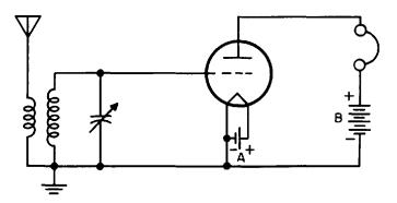
Fig. 15-4. This diagram shows how alternating current from the tuning circuit places positive and negative charges on the grid of De Forest's lube.
