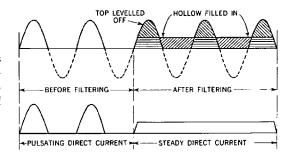
The action of the filter is to hold back the pulsating electron flow until a steady average flow is reached and maintained. When this steady flow results, we say we have *filtered* the current flowing from the rectifier tube.
