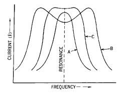
**Fig. 35-22.** Resonant curves showing the effect of coupling.
