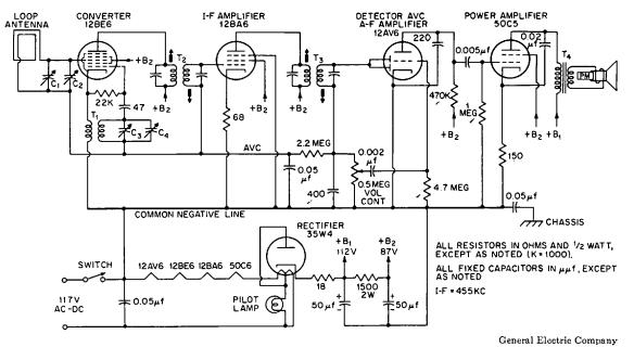
Fig. 29-2. AC-DC superheterodyne receiver.
