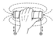
**Fig. 31-17.** Method for determining the polarity of an electromagnet.
