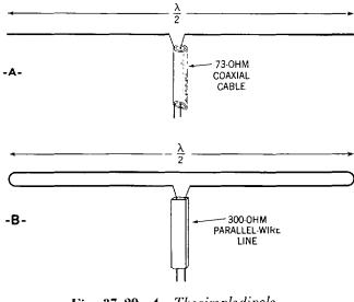
Fig. 37-29. A-The simple dipole. B—The folded dipole.
