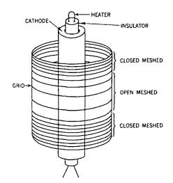
Fig. 27-9. Diagram showing the construction of the control grid of a variablemu tube.
