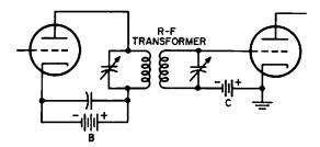
Fig. 39-24. Circuit of a transformer -coupled radio-frequency amplifier.
