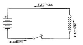
**Fig. 12-5.** This hookup of coil, key, and battery illustrates self-induction.
