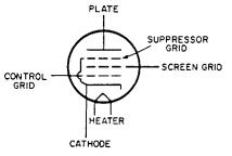
Fig. 27-10. Arrangement of electrodes in the pentode tube.
