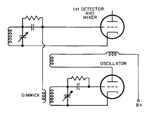
Fig. 26-7. How the "gimmick" is used for coupling.
