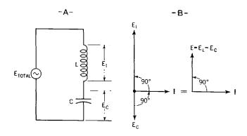
Fig. 35-7. A--Circuit diagram with inductance (L) and capacitance (C) in series. B--Vector diagrams showing  $E_L$  greater than  $E_c$ .
