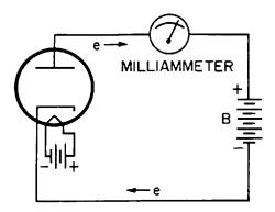
**Fig. 38-1.** Circuit to show relationship between plate current and plate voltage.
