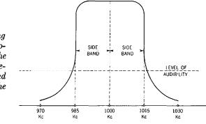
Fig. 26-12. Ideal luning curve for the superheterodyne receiver. Note that the side bands are fully received, but the unwanted stations are well below the level of audibility.
