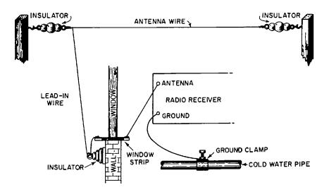
Fig 5-1. Diagram of the antenna-ground system.
