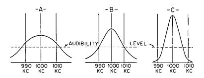
Fig. 23-3. A—Tuning curve with one tuned circuit. Notice that stations at 990 kc and 1,010 kc are heard when the set is tuned to 1,000 kc.
