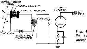
Fig. 42-11. Hookup for the carbon-grain microphone.
