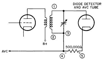
Fig. 24-8. Circuit showing how the diode acts as a detector and automaticvolume-control tube.
