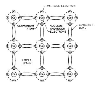
Fig. 28-1. Structure of germanium crystal. Each germanium atom is attached to its neighbor by a covalent bond.
