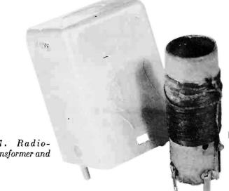
Fig. 23-7. Radiofrequency transformer and its shield.
