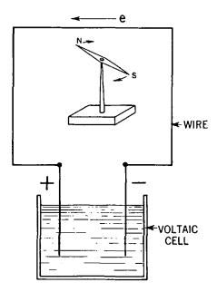
**Fig. 31-15.** Showing how the magnetic field around a conductor carrying an electric current deflects the compass needle.
