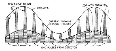
**Fig. 13-4.** This graph shows how the capacitor levels off the peaks and fills in the hollows between the pulses of direct current coming from the detector. Note that the resulting curve resembles the envelope quite closely.
