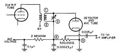
Fig. 24-10. The complete AVC circuit.
