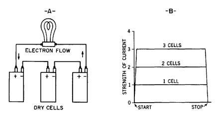
Fig. 11-3. A. Three dry cells connected in a series. B - A graph showing the flow of current from one, two, and three dry cells respectively.
