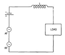
**Fig. 35-25.** The current is now being fed to the load through an inductor (L).
