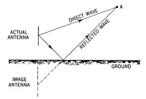
Fig. 37-27. Diagram showing the effect of the ground upon the vertical radiation pattern of an antenna.
