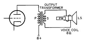
Fig. 39-13. How the output transformer is used to match the impedance of the voice coil to the resistance of the tube.
