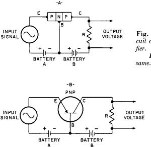
Fig. 28-10. A—Basic circuit of the transistor amplifier. B—Symbolic circuit of
