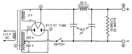
The power transformer should be able to deliver about 250v on either side of the center tap. The rectifier tube is a type 5Y3-GT. The filter capacitors are  $8\mu$ f at 450v direct-current working voltage. The choke is an ordinary 30-henry choke coil. The voltage divider is 15,000 ohms rated at 25w. Connect a 2-watt split-plate neon lamp in series with a magnetic speaker and test as follows:
