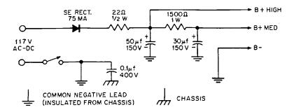
unit (50-30  $\mu$ f, 150 volts d-c working). The symbol  $\pm$  represents the common negative line (insulated from the chassis). The symbol  $\rightarrow$  represents the chassis. When using on direct current, reverse the plug to the wall outlet if the power supply fails to work.
