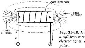
**Fig. 31-18.** Diagram showing, by use of a soft-iron core, how lines of force of an electromagnet are concentrated at the poles.
