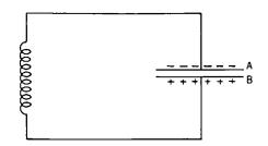
**Fig. 12-6.** Tuning circuit, showing a charged capacitor.
