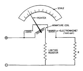
Fig. 31-33. Circuit of waltmeter connected to measure power consumed by resistor (R).
