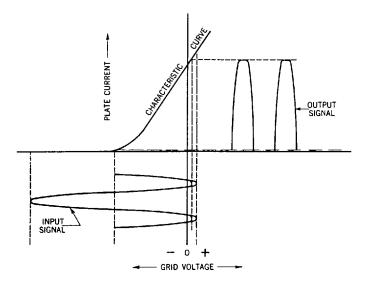
**Fig. 39-18.** Distortion of the output signal in a class B amplifier. While this distortion would prevent us from using a single tube in class B as an audio-frequency amplifier, we can do so in the radio-frequency amplifier because of the "flywheel" effect.
