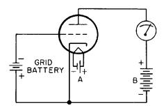
set of values against the other, we may get the characteristic curve shown in Figure 38-5. From this curve, you will notice that a certain amount of current flows in the plate circuit even though the grid may be charged somewhat negatively. We previously learned the cause of this condition: The stream of electrons to the plate is not cut off completely until an appreciable negative charge is placed on the grid.
