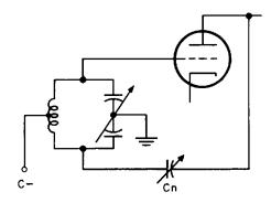
Fig. 39-26. Circuit showing grid neutralization.
