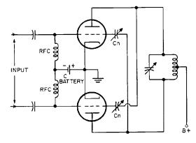
**Fig. 41-20.** Circuit showing how neutralizing capacitors  $(C_n)$  are hooked up to neutralize a pushpull radio-frequency amplifier.
