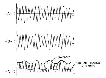
**Fig. 15-8.** These graphs show the flow of electric current in various parts of the triode circuit.
