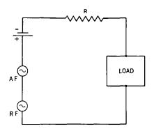
Fig. 35-23. A battery, a low-frequency (AF) generator, and a highfrequency (RF) generator supplying current to a load through a resistor (R).
