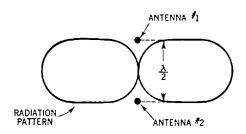
Fig. 37-22. The horizontal pattern of lwo vertical half-wave antennas, a halfwave apart, with their currents in phase.
