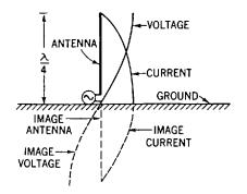
Fig. 37-7. The quarter-wave Marconi antenna. showing current and voltage distribution. Note that this antenna corresponds to the halfwave Hertz antenna. Only half the current and voltage waves is shown here for the sake of simplicity.
