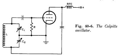
the tap is not on the coil, but on the capacitor. This is accomplished by using two tuning capacitors,  $C_1$  and  $C_2$ . Just as with the Hartley circuit, where the amount of feedback is controlled by varying the tap point on the coil, so the feedback in the Colpitts circuit is con-
