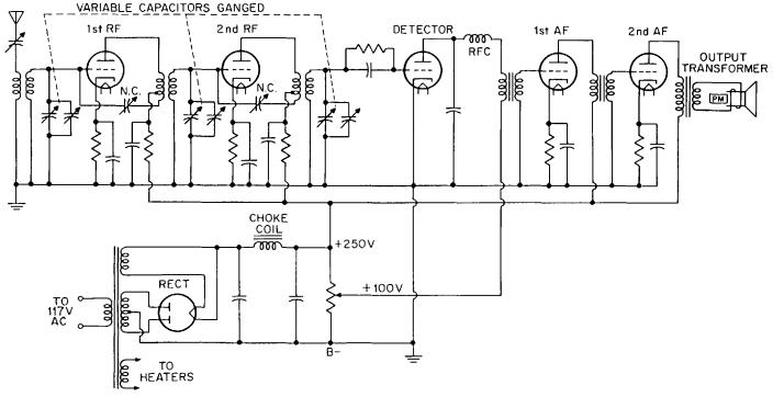
Fig. 23-17. Circuit for a complete, tuned radio-frequency receiver.
