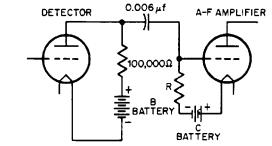
Fig. 17-12. Diagram showing how grid resistor (R) is placed in the circuit.
