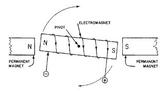
**Fig. 31-21.** An electromagnet is pivoled between the poles of a permanent magnet. Since like poles repel, the electromagnet is rotated in a clockwise direction.
