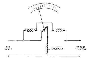
**Fig. 32-27.** Diagram showing how the dynamometer type of meter is hooked into the circuit to read alternating voltage. (The effective current must be kept constant.)
