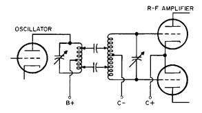
Fig. 41-9. The matchedimpedance transmission line method of coupling an oscillator to a push-pull radio-frequency amplifier.
