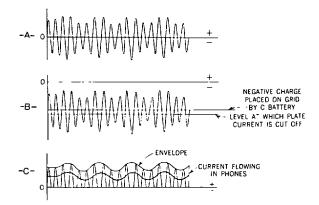
**Fig. 15-10.** These graphs show the effects of placing a steady negative charge, or bias, on the grid of the triode.
