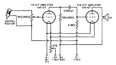
Fig. 17-17. Diagram showing circuit of the electrical phonograph.
