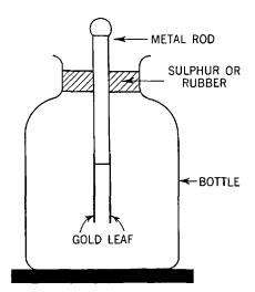
Fig. 30-2. The gold-leaf electroscope.
