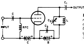
Fig. 39-23. A stage of radio-frequency amplification. Note the resemblance to the audio-frequency stage in Figure 39-22.
