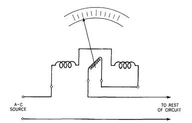
**Fig. 32-26.** Diagram showing how the dynamometer type of meter is hooked into the circuit to read alternating current.
