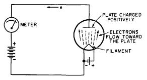
Fig. 14-2. Fleming's experiment with a positive charge on the plate of the tube. The meter showed that an electric current was flowing through it.
