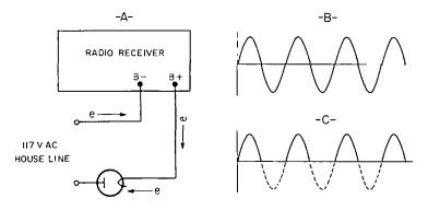
Fig. 18-1. A—The diode as a rectifier tube.
