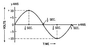
Fig. 32-10. Curve showing relationship between time and the induced voltage.
