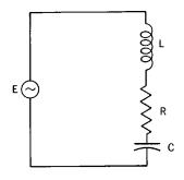
Fig. 35-13. The series resonant circuit showing inductance, capacitance, and resistance in series.
