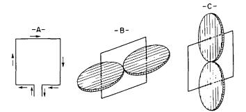
Fig. 37-28. A—Current flow in a loop antenna. B - Pattern for the vertical arms of the loop. C—Pattern for the horizontal arms of the loop.
