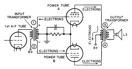
Fig. 27-4. Circuit showing how two power tubes are connected in push-pull.
