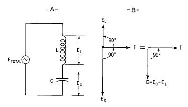
Fig. 35-8. A—Circuit diagram with inductance (L) and capacitance (C) in series. B—Vector diagrams showing  $E_c$  greater than  $E_L$ .
