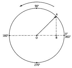
Fig. 32-16. Diagram showing what is meant by a vector.
