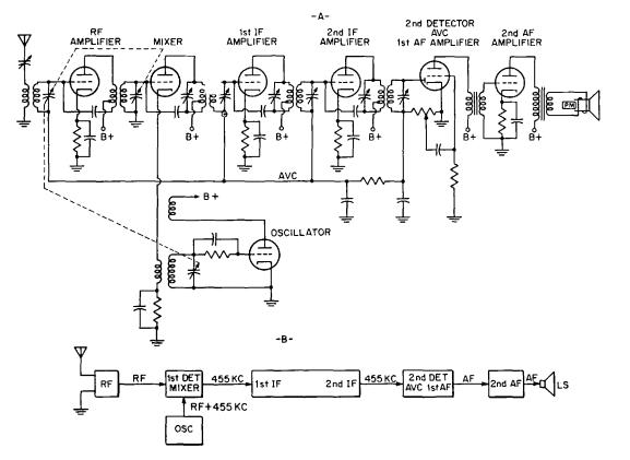
Fig. 26-13. A-Circuit of the complete superheterodyne receiver. B-Block diagram showing arrangement of the component parts.
