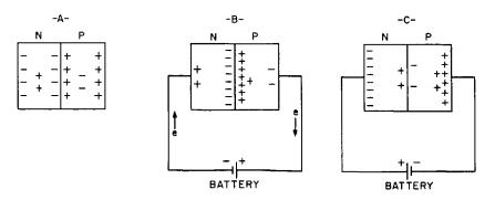
Fig. 28-4. A—Distribution of free electrons (-) and holes (+) in a PN junction diode.
