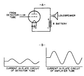
Fig. 17-1. A—Audio amplifier showing how signal from the detector tube is fed to the grid of the audio-amplifier tube.
