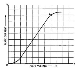
**Fig. 38-2.** Graph showing the characteristic curve of the diode.
