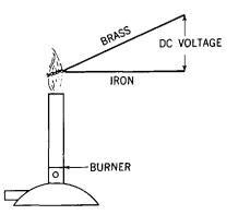
Fig. 32-29. Diagram illustrating the principle of a thermocouple.
