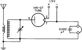
The tuner is the one shown in Figure 10-6 except that the crystal detector has been replaced by a diode (part of the 1H5-GT tube). Only filament connections Nos. 2 and 7 and diode-plate connection No. 5 of the tube are used.
