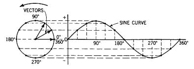
**Fig. 32-17.** Diagram showing the relationship between the vector and sinecurve methods of representing alternating currents and voltages.
