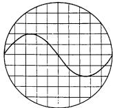
Fig. 43-14. Trace described by a sine wave.
