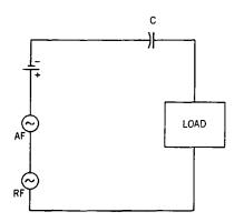
**Fig. 35-24.** The resistor of Figure 35-23 has been replaced by a capacitor (C).
