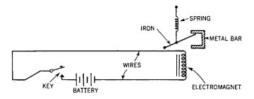
Fig. 31-20. How the electromagnet is used in the telegraph.
