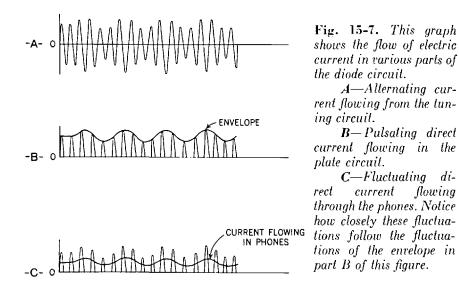
negative charge, because of the relatively high positive charge on the plate. Thus, plate current, and current through our phones, would flow during part of each negative cycle.
