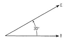
Fig. 32-19. In practice, the circle is omitted from the vector diagram. This is analogous to Figure 32-18.
