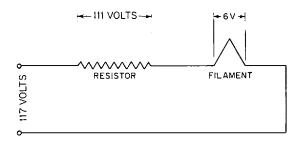
Fig. 21-1. Diagram showing how a resistor is used to cut down the 117-volt house current to a value suitable for use on the filament of the tube.
