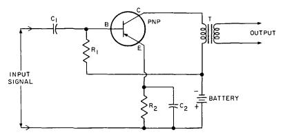
Fig. 28-12. Circuit of practical a-f transistor amplifier.
