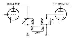
Fig. 41-5. The link-coupled transmission line.
