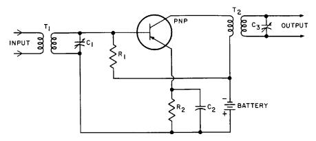
Fig. 28-15. Basic circuit of a transistorized stage of tuned r-f amplification.
