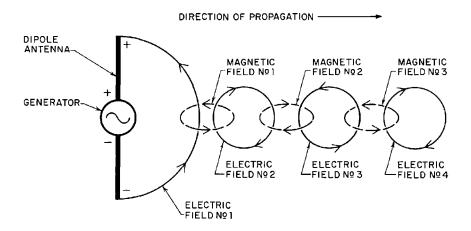
Fig. 36-3. How alternate electric and magnetic fields are set up.
