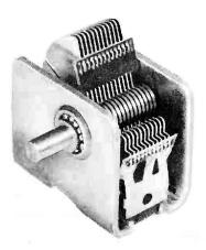
Fig. 6-3. Variable capacitor.
