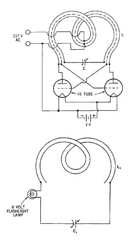
nected to the grids of the tubes.  $L_1$  is the same as L, except that there is no wire running through the tubing.  $C_1$  is the same as C.
