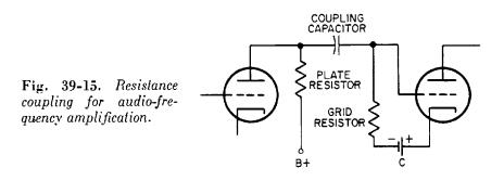
The coupling capacitor must keep the large positive charge from the B battery off the grid of the second tube and, at the same time, offer a minimum impedance to the signal voltage. This requirement calls for a large value for this capacitor, usually about 0.01  $\mu$ f. If the capacitor is made too large, the charge on the grid will take too long a time to leak off through the grid resistor. The coupling capacitor must keep direct-current leakage to a minimum.
