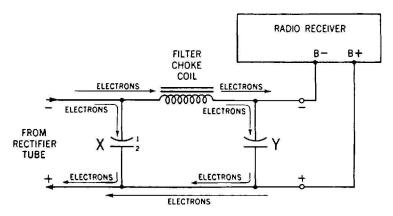
Fig. 18-2. Hookup showing the filter system.
