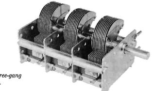
Fig. 23-14. Three-gang variable capacitor.
