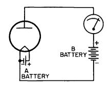
**Fig. 15-1.** Diode using a B battery to place a positive charge on the plate of the tube. Current flows through the meter.
