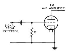
Fig. 20-5. Contact-bias circuit.
