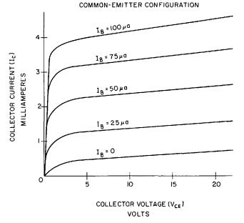
**Fig. 38-15.** Typical set of  $I_C$ - $V_{CE}$  characteristic curves for a transistor in a common-emitter configuration.
