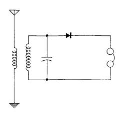
Fig. 13-2. Diagram showing crystal detector and phones.
