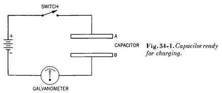
with a battery. a switch, and an ammeter (Fig. 34-1). The ammeter is of a type which has the zero point in the center of the scale. Thus current flowing through it in one direction causes the pointer to deflect to the right, and current in the opposite direction deflects the pointer to the left.
