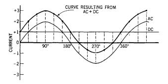
Fig. 32-21. Curve showing the result of adding alternating and direct currents.
