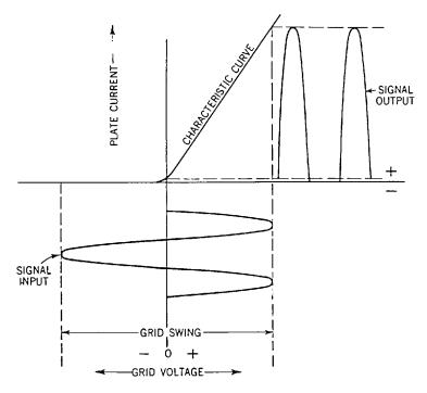
Fig. 39-9. Graph showing how the special class B tubes operate on zero grid bias.
