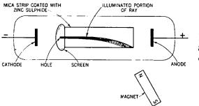
Fig. 43-3. How the electron stream is deflected by a magnet.
