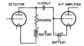
Fig. 17-11. Diagram showing how the C battery is connected in the grid circuit of the amplifier tube.
