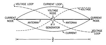
**Fig. 37-5.** Diagram showing standing current and voltage waves on a halfwavelength doublet antenna.
