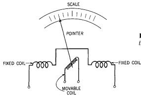
**Fig. 32–25.** Diagram of the dynamometer principle.
