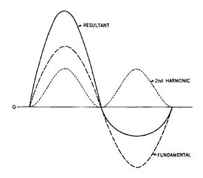
**Fig. 39-2.** Graph showing the effect of adding the fundamental to the second harmonic which is above the X axis.
