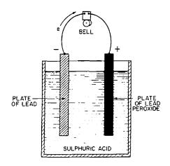
Fig. 30-20. The lead-acid storage cell.
