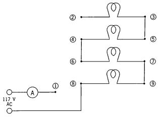
The lamps are each 117-volt, 50-watt. The ammeter is an alternatingcurrent 0 to 5-amp ammeter.
