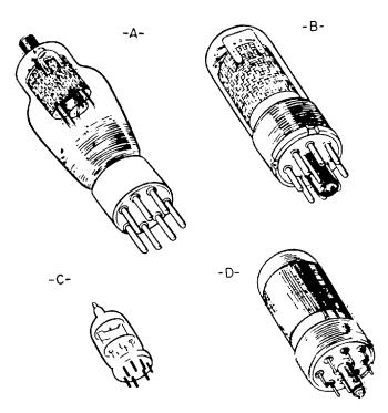
Fig. 27-20. Types of tube bases. A-Early type base. These may have 4, 5, 6, or 7 prongs. B-Octal base. D-Lock-in Loktal base.
