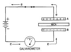
**Fig. 34-5.** The effect of placing a dielectric (such as mica) belween the plates of a fully-charged capacitor.
