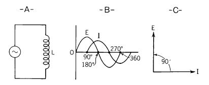
Fig. 33-1. A—Circuit containing inductance only.
