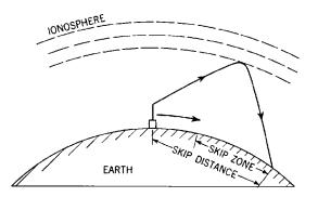
Fig. 36-9. Diagram showing what is meant by skip zone. In this zone no signals are received.
