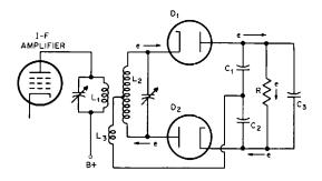
Fig. 42-16. The basic circuit of the ratio detector.
