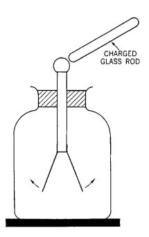
**Fig. 30-3.** The effect of a charged rod on the gold-leaf electroscope.
