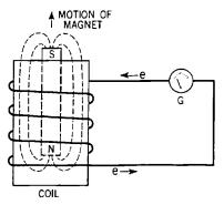
Fig. 32-2. The magnet is pulled out of the coil. Once again an electric current is induced in the coil. the pointer swings to the left, showing that once more an electric current is set flowing, but this time in the opposite direction.
