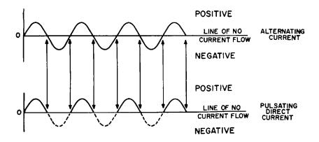
**Fig. 9-9.** This graph shows how the crystal detector changes alternating current into pulsating direct current. The negative halves of the cycle which were stopped by the crystal detector are shown by the dotted lines. For practical purposes, we may disregard the small amount of curent flow in the negative direction.
