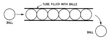
Fig. 30-6. Diagram to illustrate motion of electrons through a conductor.
