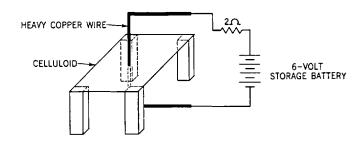
(a) Trace the magnetic lines of force by a small compass moved around on the sheet of celluloid.
