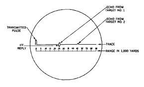
Fig. 43-22. Trace showing two targets, one of which (the nearest) is friendly, as indicated by the IFF reply.
