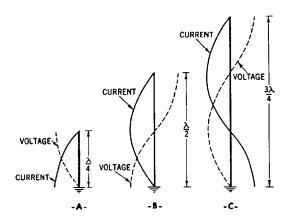
Fig. 37-8. Marconi-type anlennas of different lengths.
