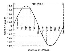
**Fig. 32-13.** Curve showing relationship between angles (in  $30^{\circ}$  steps) and their respective sines. Note that this is merely another way of presenting the table in Figure 32-12.
