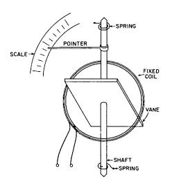
Fig. 32-24. Diagram of the inclined-coil a-c meter.
