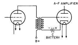
Fig. 20-1. Circuit showing a C battery connected in the grid circuit of an amplifying tube. Using a Voltage Divider. Turn back to Figure 18-15. The most negative point of the B eliminator is the negative terminal. Note that the filaments of the radio tubes are connected to that point. Now consider a point on the voltage divider a little distance away from the negative terminal and toward the positive terminal. As you now know, this point is a little more positive than the negative terminal.
