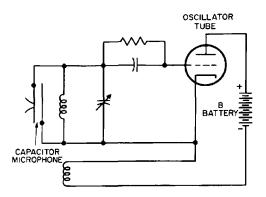
Fig. 42-14. Theoretical circuit of the frequency-modulation transmitter.
