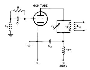
In this oscillator diagram,  $C_1$  is a 0.0001- $\mu$ f mica capacitor,  $C_2$  is a 15- $\mu\mu$ f variable capacitor,  $C_3$  is a 0.0005- $\mu$ f mica capacitor; R is 10,000 to 50,000 ohms;  $L_1$  and  $L_2$  are made of four turns of No. 14 copper wire
