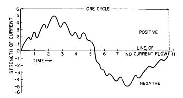
**Fig. 9-5.** Graph of the curve or waveform of an alternating current. Notice that this curve is not smooth but irregular.
