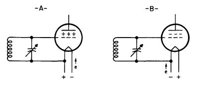
Fig. 19-2. Circuits showing how alternating current flowing through the filament places an alternating charge on the grid of the lube.
