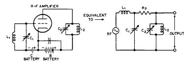
Fig. 41-21. Diagram showing the equivalent circuit of a radio-frequency amplifier.  $R_p$  is the internal resistance of the tube.
