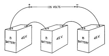
Fig. 30-19. Circuit showing three B batteries in series.
