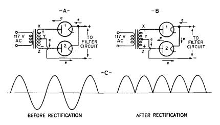
Fig. 18-8. Full-wave rectification using two rectifier tubes. For the sake of simplicity, the complete filament circuits are omitted.
