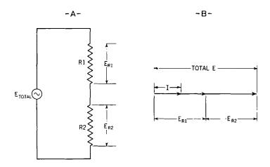
Fig. 35-4. A—Circuit containing two resistors (R<sub>1</sub> and R<sub>2</sub>) in series. The voltage drop across each (E<sub>R1</sub> and E<sub>R2</sub>), when added together, will give the total voltage (E) of the circuit.
