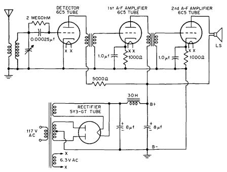
Fig. 20-6. Diagram showing the circuit of an all-electric receiving set.
