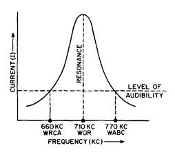
Fig. 35-11. Curve of a resonant circuit showing the relationship of current (I) to changes in frequency. The inductance and capacitance of the circuit are kept constant.
