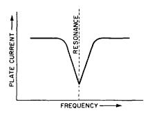
**Fig. 41-23.** Graph showing the dip in plate current which indicates that the plate tank circuit is at resonance.
