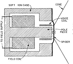
Fig. 22-1. Diagram of an electromagnetic dynamic speaker.
