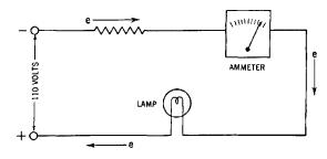
Fig. 30-11. The series circuit. Electrons can follow only one path from negative to positive.
