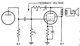
Fig. 39-16. Circuit showing inverse feedback in the audio-frequency amplifier. The values of R and  $R_1$  determine the amount of feedback.
