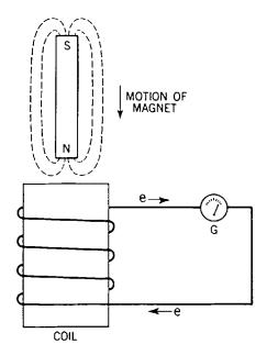
**Fig. 32-1.** The magnet is plunged into the coil of wire. An electric current is induced in the coil.
