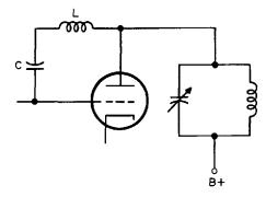
**Fig. 39-27.** Circuit using direct plate-togrid neutralization.
