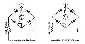
Fig. 32-32. Circuit of the full-wave bridge rectifier. A—Current flow during one allernation. B—Current flow during the next allernation.
