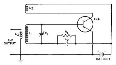
Fig. 28-16. Typical circuit of a transistorized oscillator stage.
