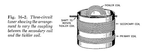
The same effect is obtained by changing the angle which the tickler coil makes with the secondary of the antenna coupler. When the two coils are parallel, you get the maximum feedback. When the two coils are at right angles, you get the minimum feedback. By making the angle adjustable, you are able to get the desired amount of feedback. When we use these methods of controlling the
