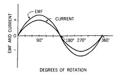
Fig. 32-14. Curves showing the relationship between emf and current and the degree of rolation (in phase).
