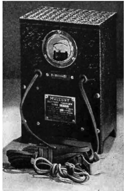
FIG. 3-28.—A copper oxide battery charger. (P. R. Mallory & Co., Inc.)
