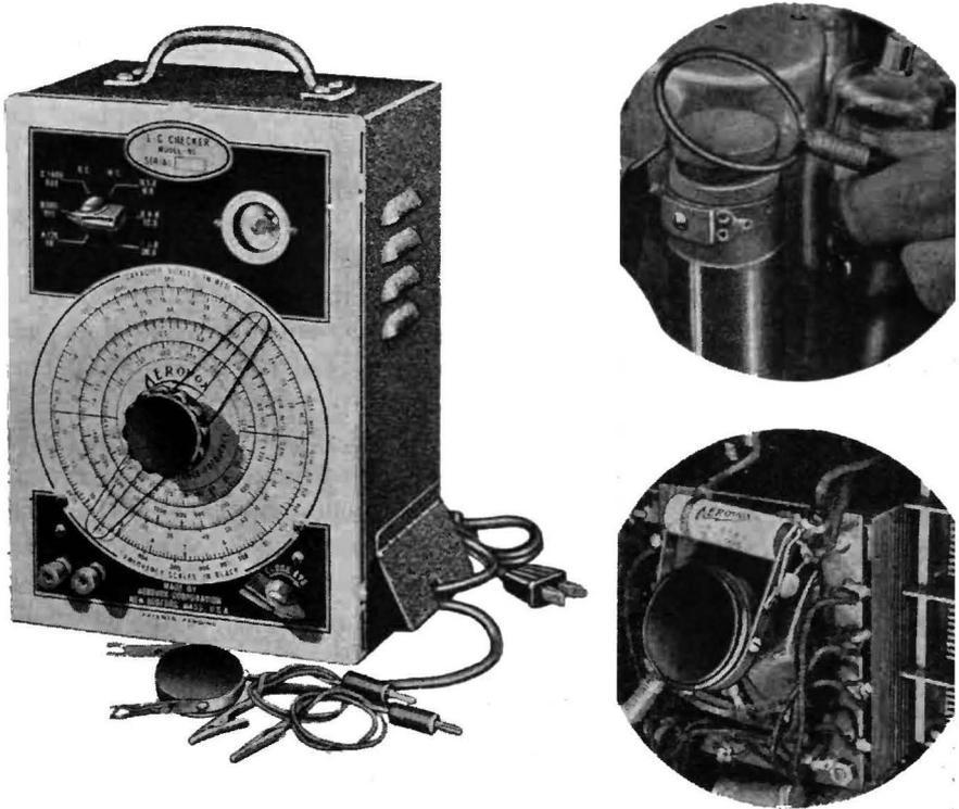
FIG. 11-6.—An  $LC$  checker and two of its applications. Left, the  $LC$  checker; upper right, checking the inductance of a coil; lower right, checking the capacitance of a capacitor in a radio receiver. (Aerovox Corporation.)
