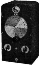
Frequency meter or wave meter.
