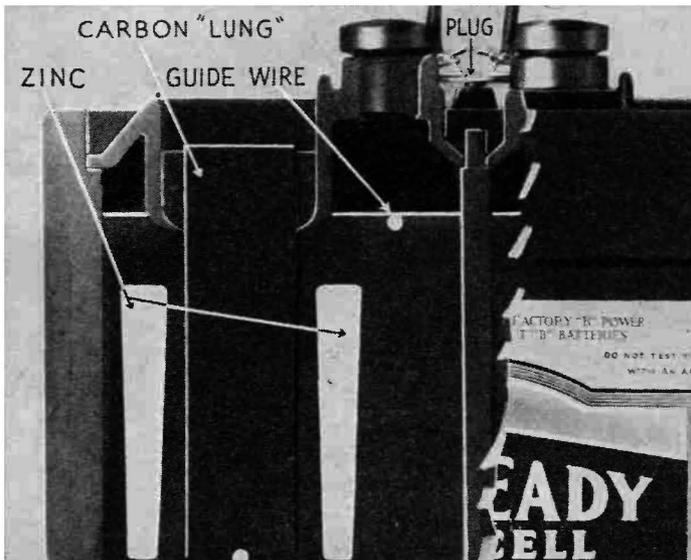
FIG. 3-15.—Cross-sectional view of an air-cell battery. (National Carbon Company.)
