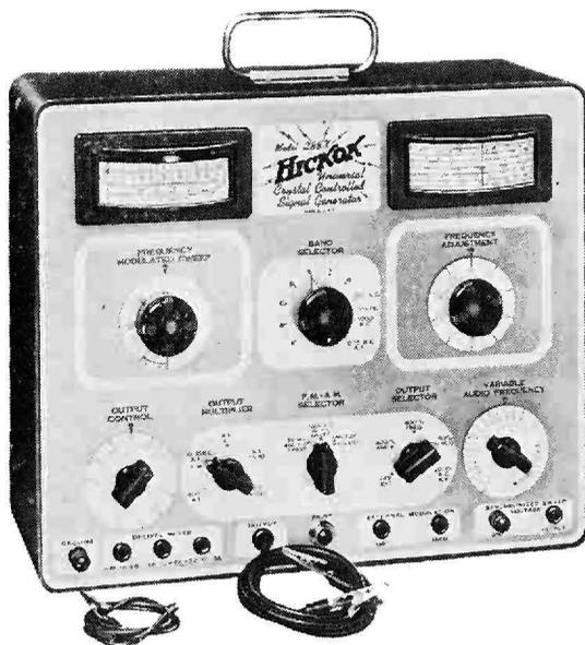
FIG. 15-16.—A commercial universal crystal-controlled signal generator. (Courtesy of The Hickok Electrical Instrument Company.)
