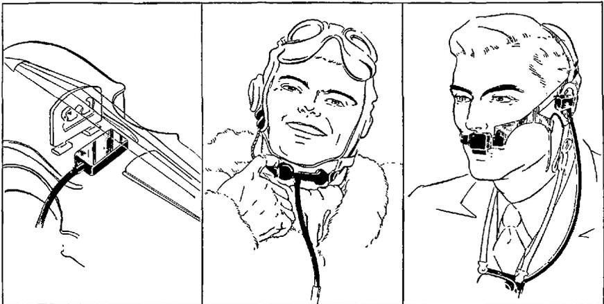
FIG. 12-2.—Contact-type microphones. (a) For musical instruments, (b) throat microphone, (c) lip microphone.
