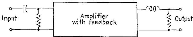
FIG. 8-24.—A feedback amplifier with equalizing filter networks for neutralizing the amplification peaks.
