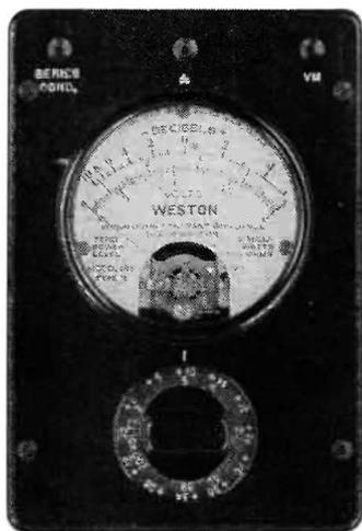
FIG. 15-8.—Output or power-level meter. (Courtesy of Weston Electrical Instrument Corporation.)
