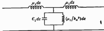
FIG. 8.17. Equivalent circuit for the transverse electric wave.
