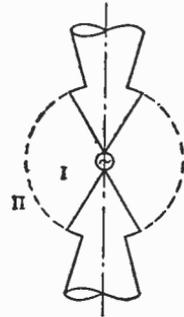
FIG. 11.03d. Discontinuity in conical line.
