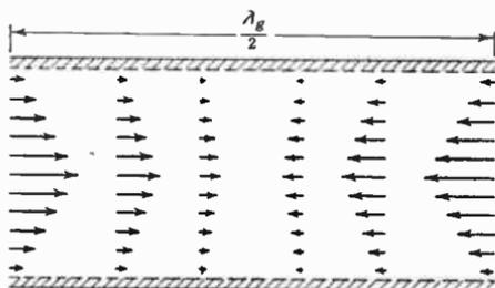
FIG. 9.05b. Top view indicating longitudinal current flow along guide in  $TE_{10}$  wave.
