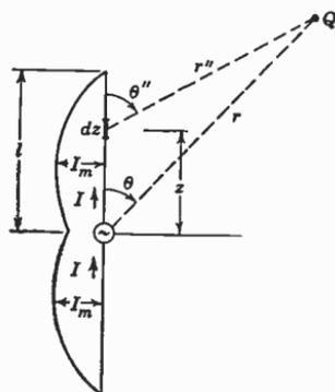
FIG. 11.07. Long straight dipole antenna.
