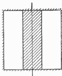
FIG. 10.08. Cylindrical resonator with dielectric core.
