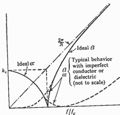
FIG. 9.14. Modification of propagation characteristics due to losses.
