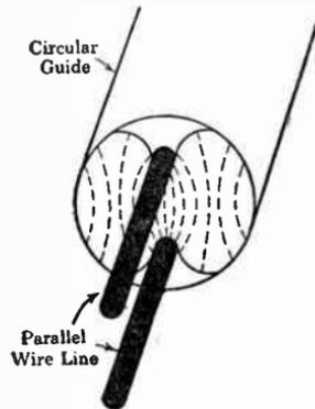
FIG. 9.11d. Parallel wire line for excitation of  $TE_{11}$  wave in circular guide.
