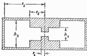
FIG. 10.10b. Axially symmetric resonator.
