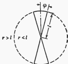
FIG. 11.31a. Biconical antenna.
