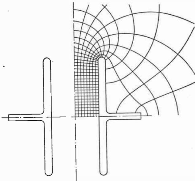
FIG. 3.05c. Map of fields between transmission line conductors of special shape.
