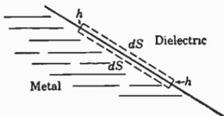
FIG. 2.10. Cross section, showing surface separating a dielectric and a conductor.
