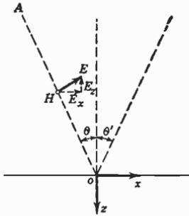
FIG. 7.11. Wave polarized with  $E$  in plane of incidence striking a plane boundary at angle  $\theta$ .
