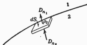
If two very small elements of area  $\Delta S$  are considered (Fig. 4.22), one on either side of the boundary between any two materials, with a surface charge density  $\rho_s$  sitting on the boundary, the application of Gauss's law to this elemental volume gives
