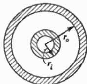
FIG. 9.02a. Cross section of a coaxial line.
