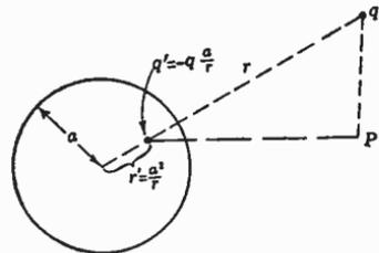
FIG. 3.30b. Image of a point charge in a conducting sphere.
