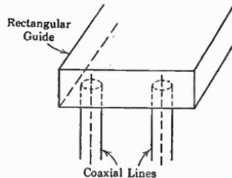
FIG. 9.11f. Excitation of the  $TE_{20}$  wave in rectangular guide by two oppositely phased antennas.
