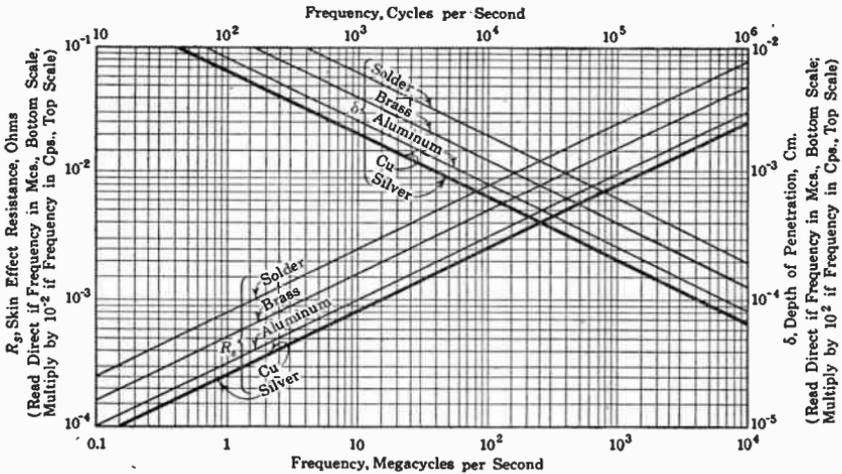
FIG. 6.05a. Skin effect quantities for plane conductors.
