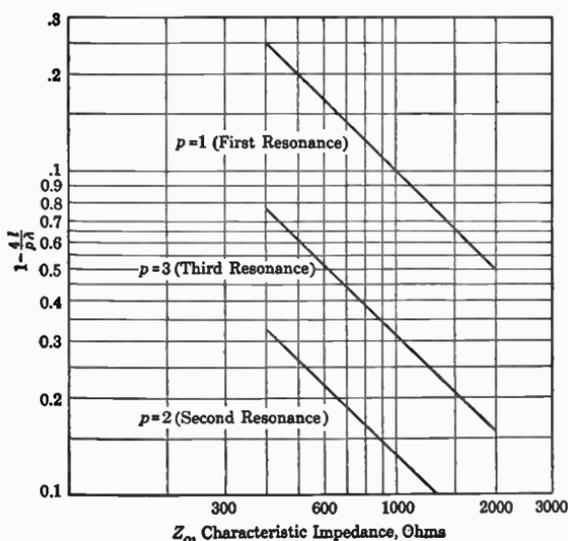
FIG. 11.32d. Per unit foreshortening of biconical antenna.
