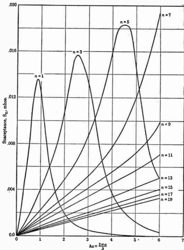
FIG. 11.28b. Susceptance of individual spherical  $TM$  wave orders.
