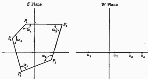
FIG. 3.10. Transformation from a general polygon to a straight line.
