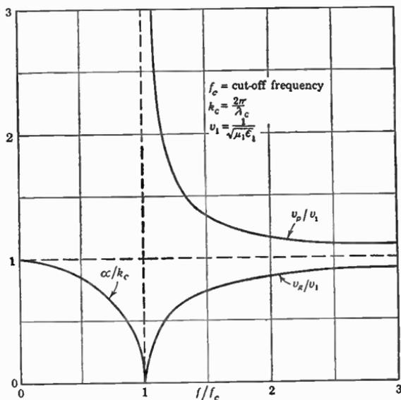
FIG. 8.18. Frequency characteristics of all  $TE$  and  $TM$  wave types.
