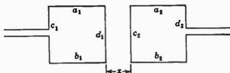
FIG. 6.14a. Two square coupling loops.
