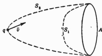
FIG. 4.06. Evaluation of  $\oint \bar{H} \cdot d\bar{l}$  for charge  $q$  moving toward loop  $A$ .
