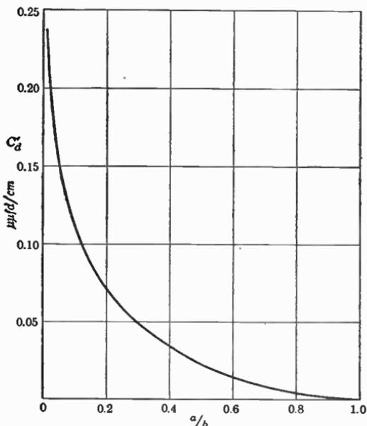
FIG. 9.15b. Curve of discontinuity capacitance for Fig. 9.15a.
