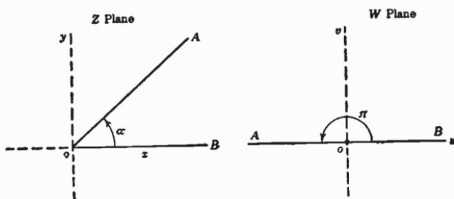
FIG. 3.09a. Transformation  $W = (Z)^{\pi/\alpha}$  applied to a wedge of angle  $\alpha$ .
