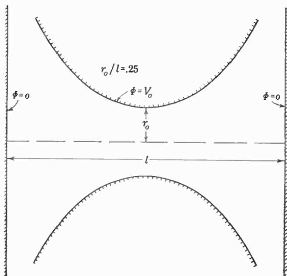
FIG. 3.13. Shape of electrodes for field described by  $\Phi = CI_0\left(\frac{\pi r}{l}\right) \sin\left(\frac{\pi z}{l}\right)$ .
