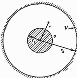
FIG. 3.04. Two coaxial conducting cylinders.
