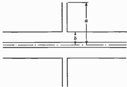
FIG. 9.08e. Coaxial line with open radial line in series with outer conductor.
