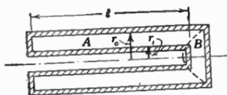
FIG. 10.09a. Foreshortened coaxial line resonator.
