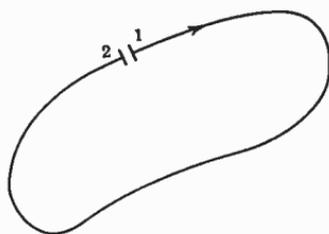
FIG. 5.05. Circuit containing a lumped capacitance.
