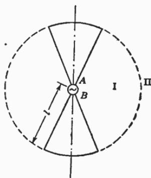
FIG. 11.02. Axial section through biconical antenna.
