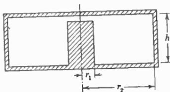
FIG. 10.10a. Foreshortened radial line resonator.
