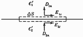
FIG. 2.31. Cross section, showing surface separating two dielectrics.
