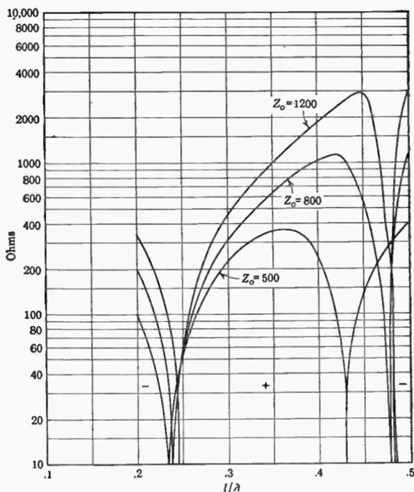
FIG. 11.33c. Input reactance for cylindrical dipole antenna.
