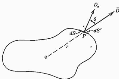
FIG. 2.06. Charge  $q$  and arbitrary surrounding surface.
