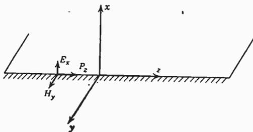
Fig. 8.02. Electromagnetic field vectors for a wave guided by a conducting plane.
