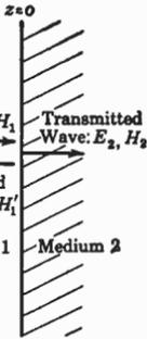
FIG. 7.07a. Reflection and transmission at a plane boundary between two media.
