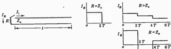
FIG. 1.19d. Charged line of length  $l$  suddenly connected to a resistor.
