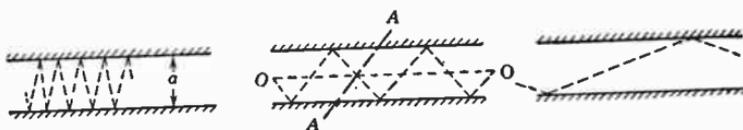
FIG. 8.07. Waves guided by two parallel conducting planes.
