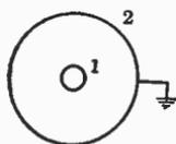
FIG. 6.26a. Electrostatic shielding by a grounded sphere.
