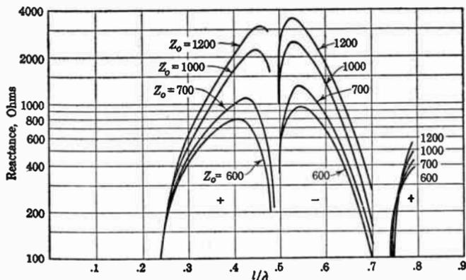
FIG. 11.32c. Input reactance of biconical antenna.
