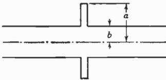
FIG. 9.08d. Circular waveguide with shorted radial line in series with cylinder wall.
