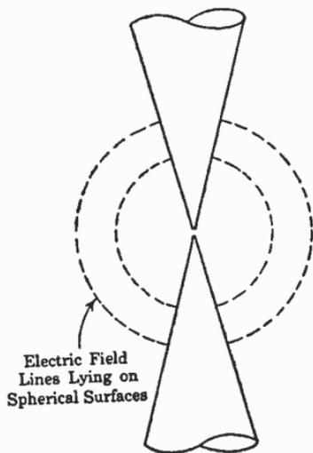
FIG. 11.03a. Portion of conical line.
