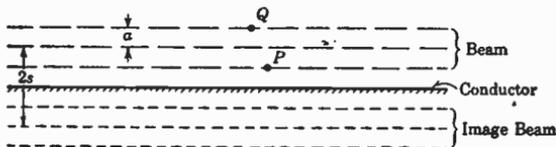
FIG. 3.31. Image of an electron beam in a conducting plane.
