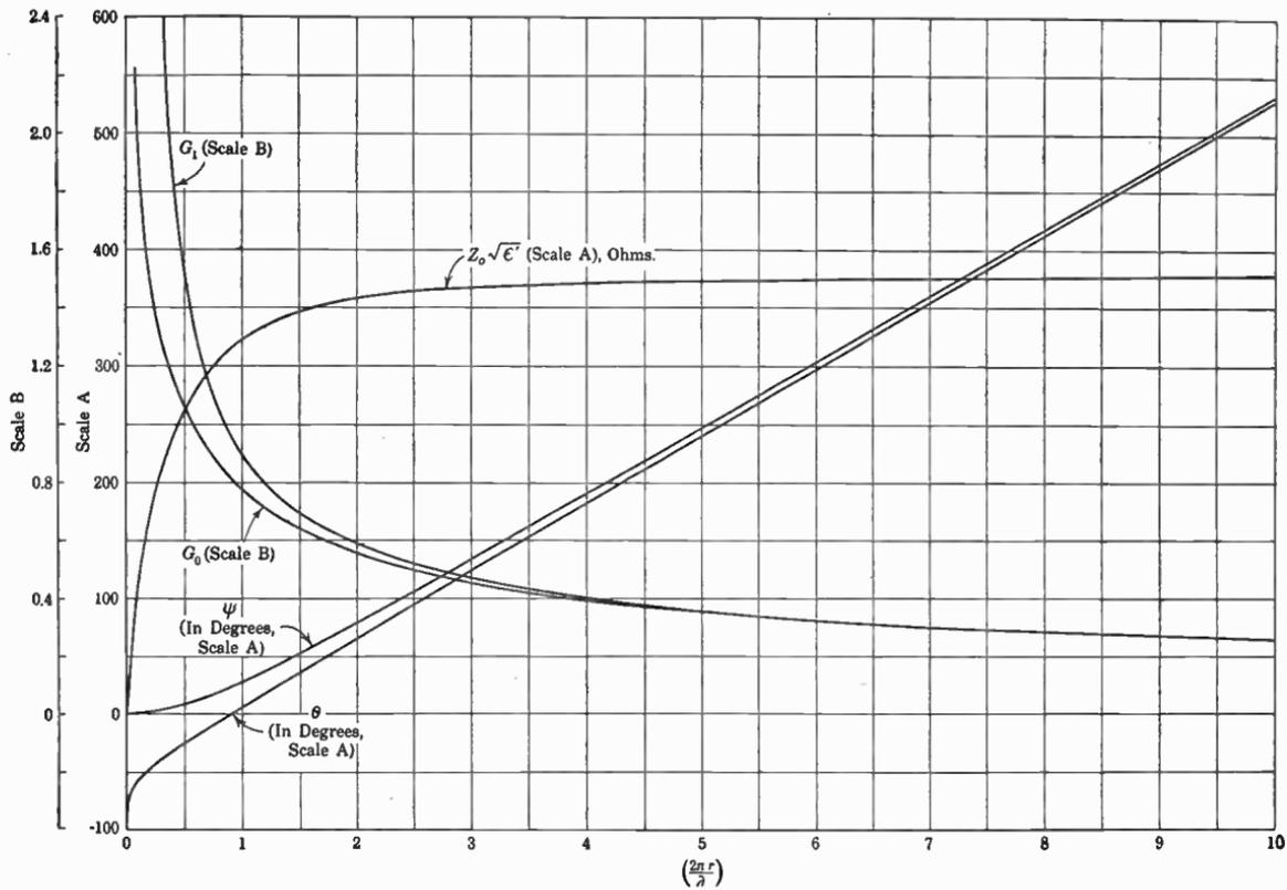
FIG. 9.08c. Radial transmission line quantities.
