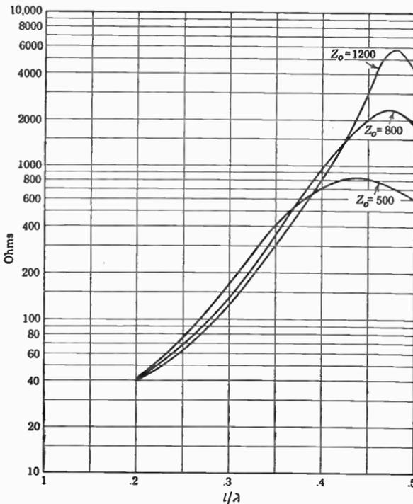
FIG. 11.33b. Input resistance for cylindrical dipole antenna.
