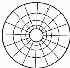
FIG. 3.05b. Map of fields between coaxial conducting cylinders.
