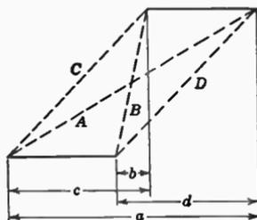
FIG. 6.14b. Parallel current elements displaced from one another.
