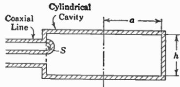
FIG. 10.14b. Magnetic coupling to a cylindrical cavity.
