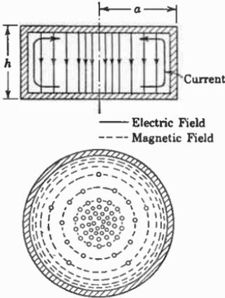
FIG. 10.06. Sections through a cylindrical cavity.
