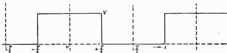
FIG. 1.14. Periodic wave of rectangular shape.
