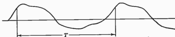
FIG. 1.13. Periodic wave of arbitrary shape.
