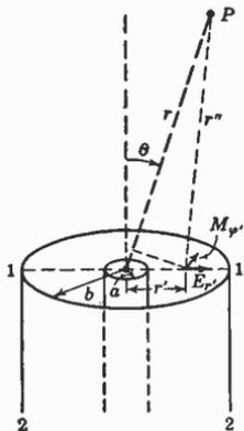
FIG. 11.15. Open end of coaxial line.
