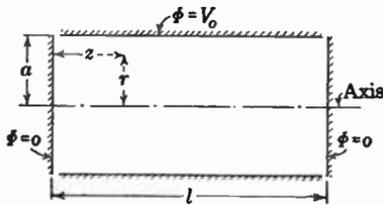
(a) Cylindrical region ( $l/a = 0.25$ ).
