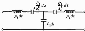
FIG. 8.13. Equivalent circuit for the transverse magnetic wave.
