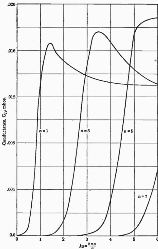
FIG. 11.28a. Conductance of individual spherical  $TM$  wave orders.
