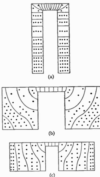
FIG. 10.11. Transition between foreshortened coaxial line and foreshortened radial line.
