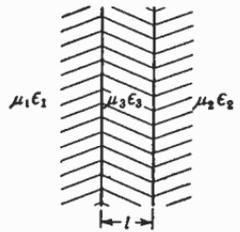
FIG. 7.09. Matching section for plane waves.
