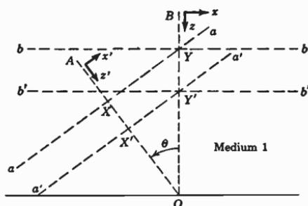
FIG. 7.10. Uniform plane wave moving at angle  $\theta$  toward a plane.
