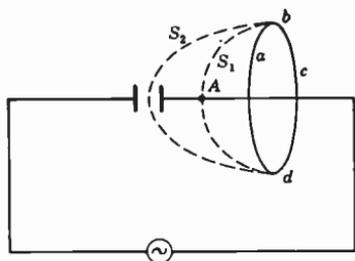
FIG. 4.05. Evaluation of  $\oint \vec{H} \cdot d\vec{l}$  for an A-C circuit with a condenser. The law from statics states that the result obtained should be  $4\pi$  times the current enclosed, that is,
