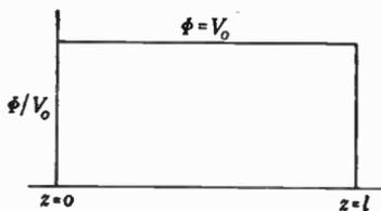
(b) Plot of potential vs.  $z$  at  $r = a$ .
