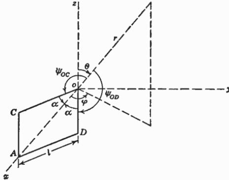
FIG. 11.23. Rhombic antenna and selected coordinate system.
