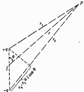
FIG. 2.32. Dipole and distant point  $P$ .
