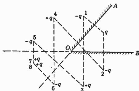
FIG. 3.30d. Multiple images in intersecting planes.
