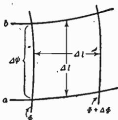
FIG. 3.05a. Element of a field map.
