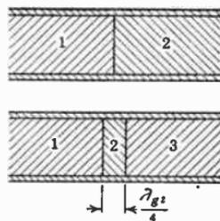
FIG. 9.12c. Insertion of matching section in a guide.
