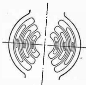
FIG. 11.26. Axial section showing electric field lines in first order symmetrical *TM* waves.
