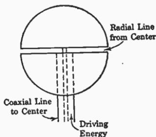
FIG. 11.24. Spherical antenna and possible driving system.
