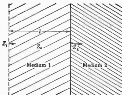
Fig. 7.07b. Region of wave propagation terminated by a second medium.
