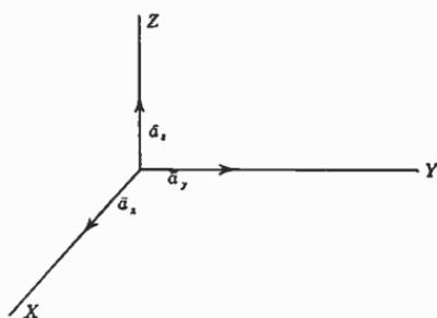
FIG. 2.20. A right-handed system of rectangular coordinates.
