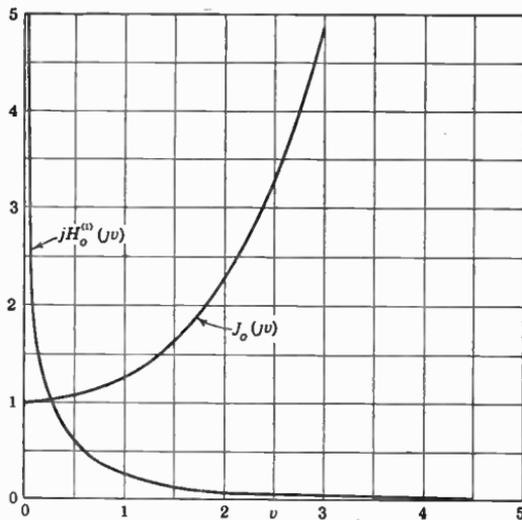
FIG. 3.17. Plot of zero order Bessel functions of imaginary arguments.
