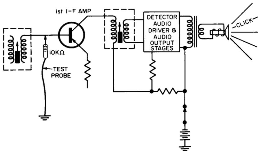
Fig. 5-6. Quick check of i-f amplifier stage.
