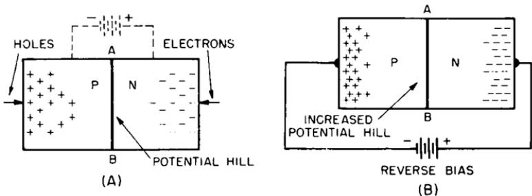
Fig. 1-10. If the battery is reversed, the potential hill is increased and conduction ceases. The unit is "reverse biased."
