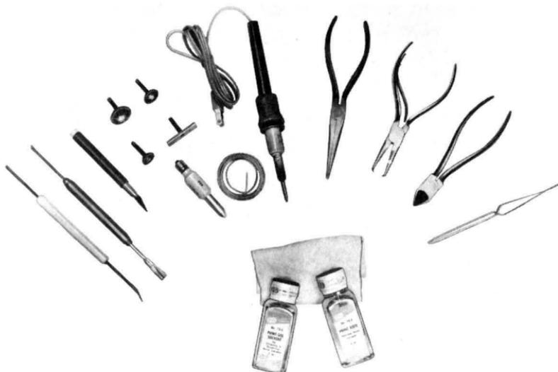
Fig. 11-1. Small servicing tools for servicing compact transistor radios. Courtesy RCA.
