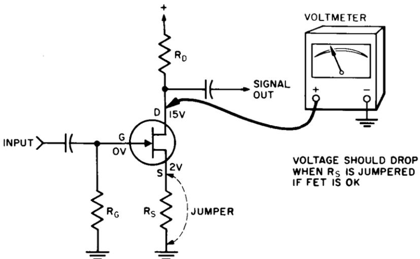
Fig. 10-11. In-circuit testing of FET by momentarily shorting bias resistor.
