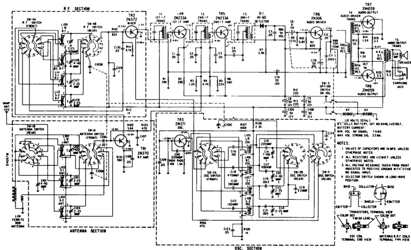
Fig. 8-13. Sears Roebuck model 222 multiband AM radio receiver.
