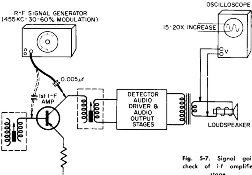
Fig. 5-7. Signal gain check of i-f amplifier stage.
