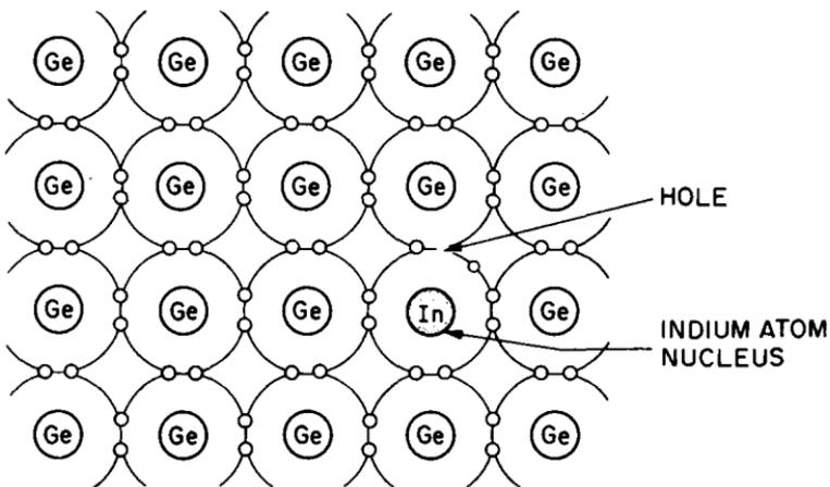
Fig. 1-7. The addition of an indium atom to the germanium lattice structure creates a hole (deficiency of electrons). This material is now known as p-type germanium.
