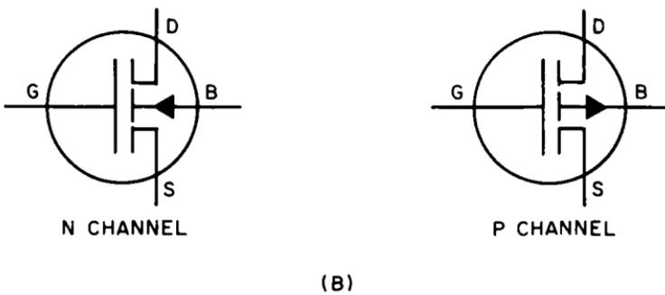
Fig. 1-23. MOS-FET transistor, enhancement type: (A) construction, and (B) schematic symbols.
