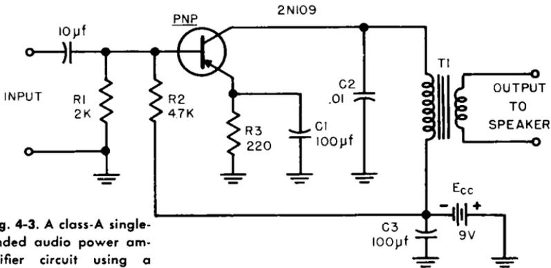
Fig. 4-3. A class-A single-ended audio power amplifier circuit using a 2N109 junction transistor.
