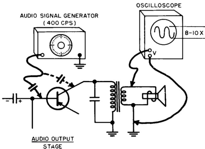
Fig. 4-12. Signal gain check of audio output stage.
