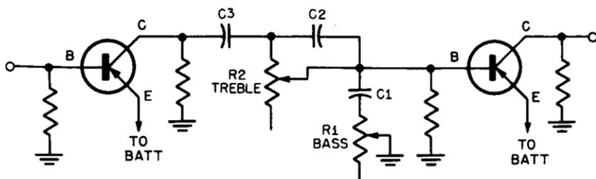
Fig. 3-17. Base and treble tone control circuitry.
