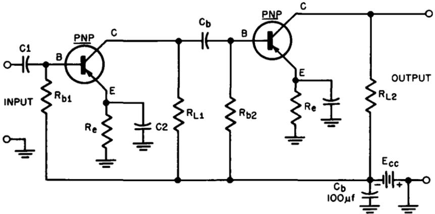
Fig. 3-12. A typical R-C coupled amplifier circuit.
