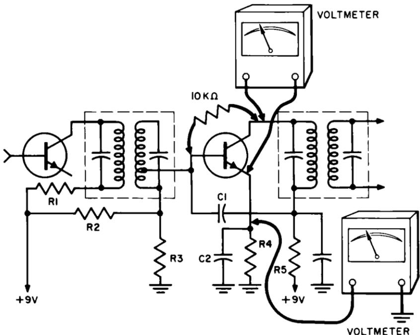
Fig. 10-9. In-circuit transistor testing.
