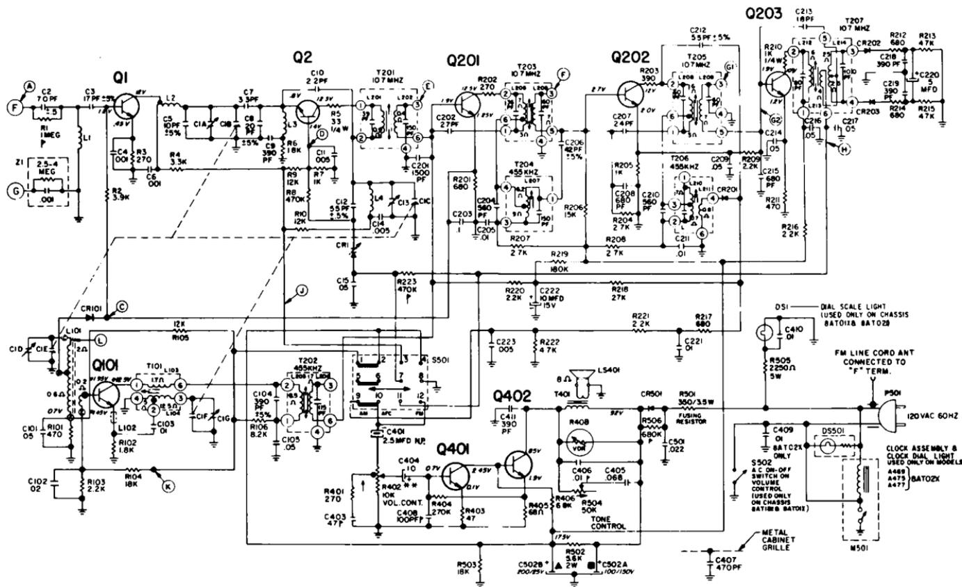
Fig. 8-16. Zenith model A418 AM-FM radio.
