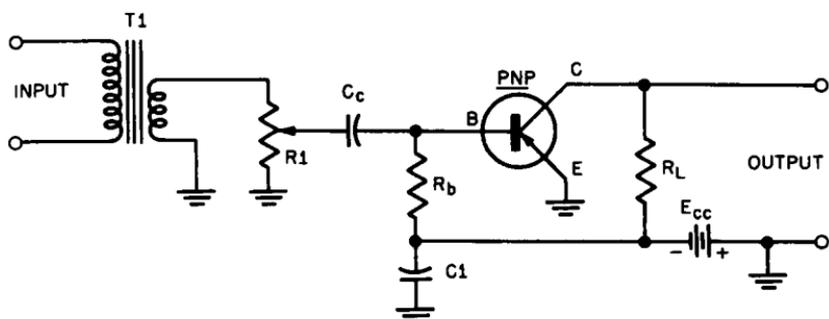
Fig. 3-16. The gain control in a transformer-coupled circuit is 2 to 3 times the impedance of the transformer secondary to prevent excessive loading.
