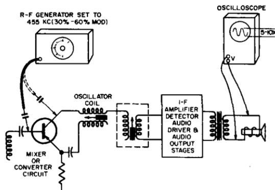
Fig. 6-11. Setup for checking mixer (or converter) stage gain.
