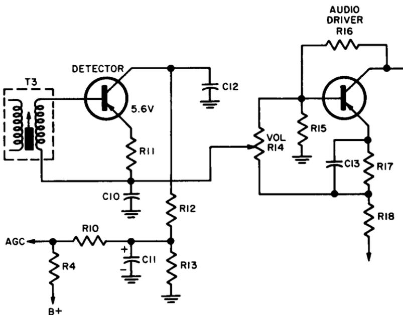
Fig. 7-4. A transistor detector circuit in which the audio signal is d-c coupled between the detector and audio driver transistors. The agc voltage is amplified to increase the agc range.
