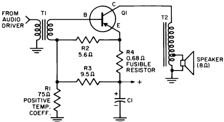
Fig. 9-1. Typical single-ended audio-power output stage for auto radios.
