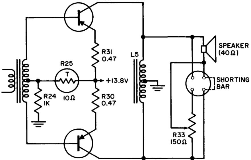
Fig. 9-2. Typical push-pull audio-output stage for auto radios (Motorola type CTA63).
