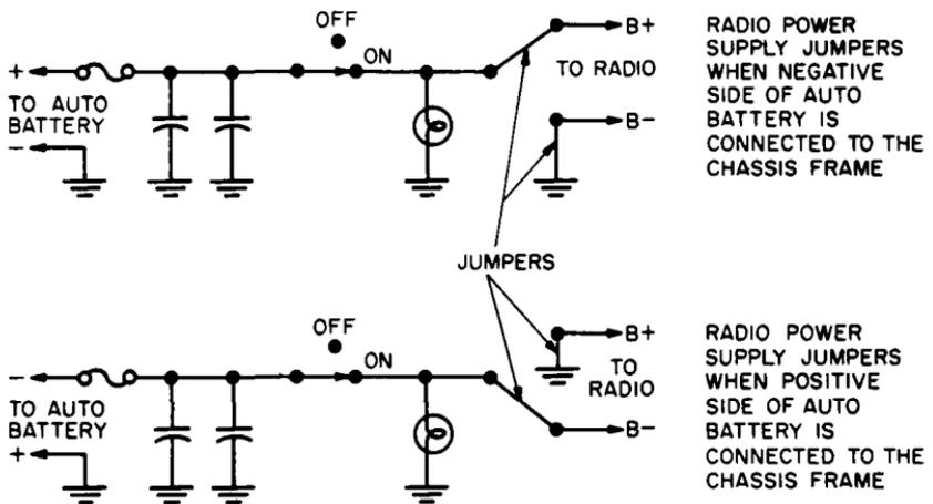
Fig. 9-9. Motorola model 406 AM auto radio shows a typical method used to reverse the input polarity of a transistor radio supply.
