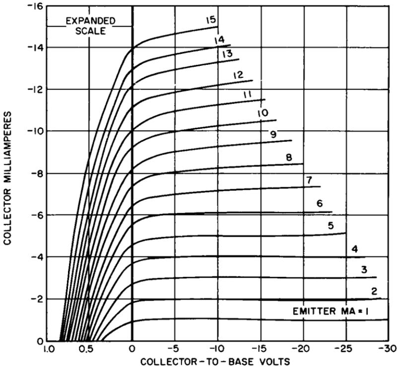
Fig. 3-2. The characteristic curve of a grounded-base circuit using a 2N105 pnp junction transistor. Courtesy RCA.
