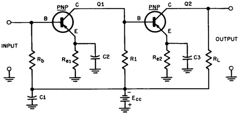
Fig. 3-14. A direct-coupled amplifier circuit. No coupling capacitor is used.  $R_1$  serves as both collector load for  $Q_1$  and bias resistor for  $Q_2$ .
