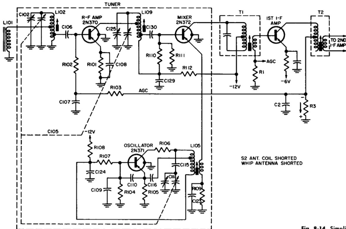
Fig. 8-14. Simplified schematic of Sears Roebuck model 222 front end in long-wave mode of operation.
