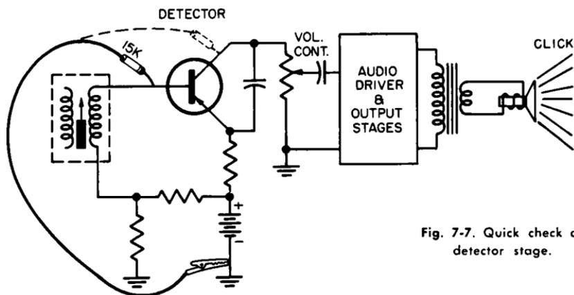
Fig. 7-7. Quick check of detector stage.
