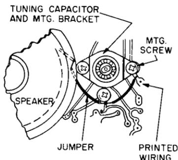
Fig. 6-13. Typical AM receiver using printed wiring where oscillations may occur because of poor ground connections in converter circuit. Jumpers interconnect ground circuits, reducing ground circuit impedance.
