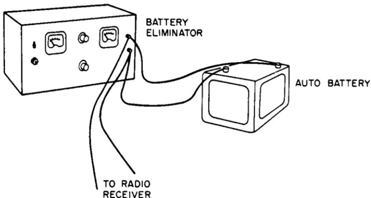
Fig. 9-7. A battery shunted by a rectified a-c source makes an ideal supply.
