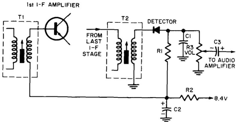
Fig. 7-1. A basic diode detector-agc circuit.
