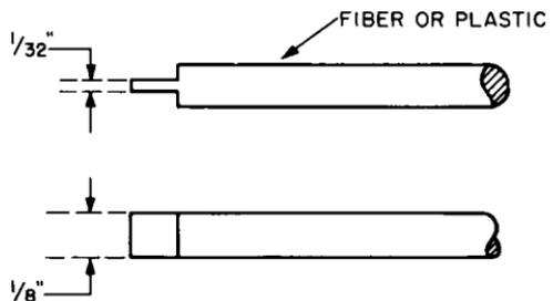
Fig. 5-10. Alignment tool.
