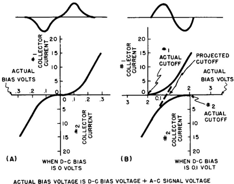
Fig. 4-6. (A) Crossover distortion as it appears in a push-pull class-B audio power amplifier. (B) Elimination of distortion by a small amount of forward bias (class-AB) operation. Courtesy RCA.
