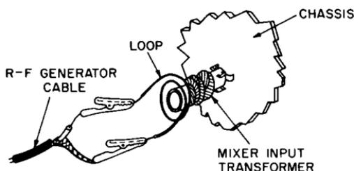
Fig. 6-10. A 2- to 3-loop wire placed across the r-f generator output cable is used to couple the r-f signal to the mixer input transformer.
