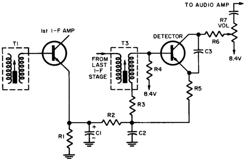
Fig. 7-2. A detector circuit using a transistor to detect. This circuit provides an audio gain of approximately 10–15 db.
