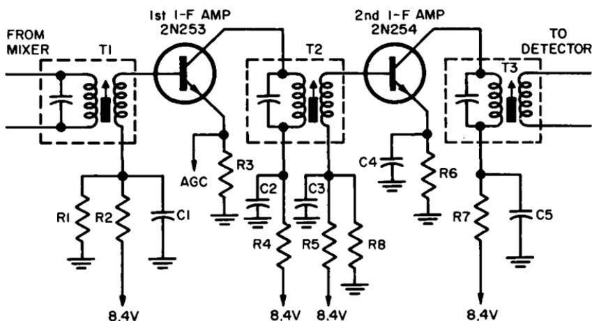
Fig. 5-1. Two-stage i-f strip used in many current AM standard broadcast receivers. The i-f frequency is 455 kc.
