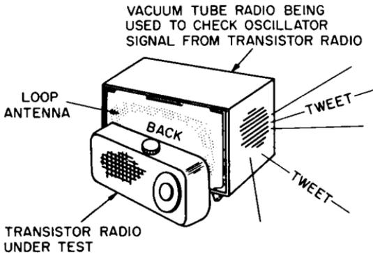
Fig. 6-9. Another working receiver can be used to check oscillator frequency and calibration.
