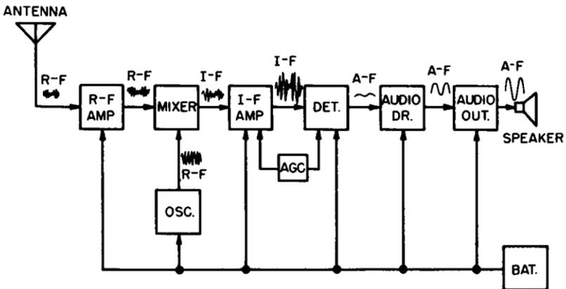
Fig. 2-1. Block diagram of a typical AM superheterodyne receiver. Signals at various points in receiver are shown.
