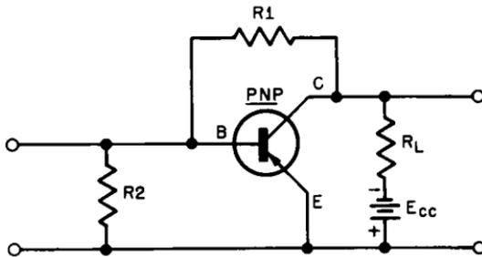
Fig. 3-8. Both fixed and self-bias can be used to provide even better circuit stability.
