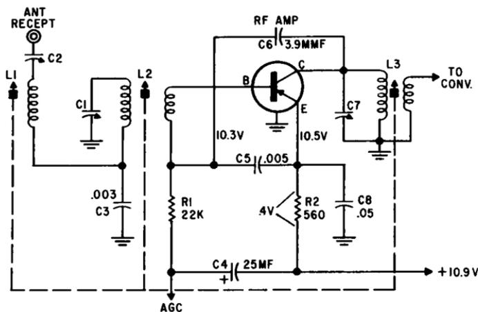
Fig. 9-3. Typical circuit for r-f amplifier.
