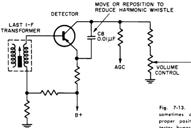
Fig. 7-13. Tweets are sometimes due to improper position of detector bypass capacitor.
