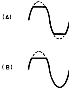
up the volume to just under the distortion level. Measure the emitter voltage across the emitter resistors of the two transistors. The average value of fluctuations in voltage will be the same if the transistors are balanced.
