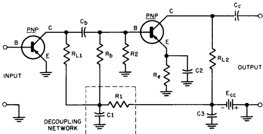
Fig. 3-13. Cascaded R-C coupled amplifiers require decoupling networks to prevent regenerative feedback.
