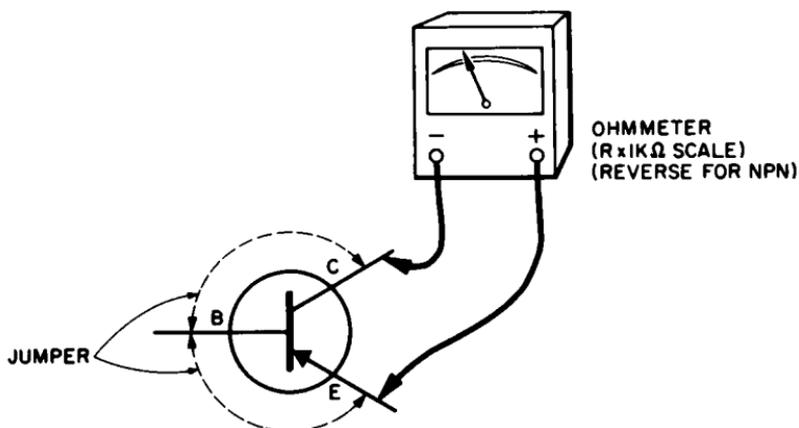
Fig. 10-8. Checking transistor with ohmmeter to determine approximate gain.
