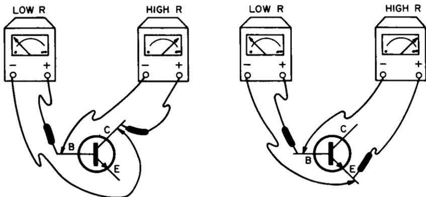
Fig. 10-6. Testing npn transistors with an ohmmeter. The low resistance should be 50 to 500 ohms. The high resistance should be 50K to 5 megohms. The forward-to-back ratio should be 100:1 or better.
