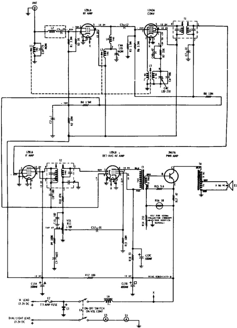
Fig. 9-5. Motorola model 825, a typical hybrid automobile radio receiver for cars with a 12-volt electrical system.
