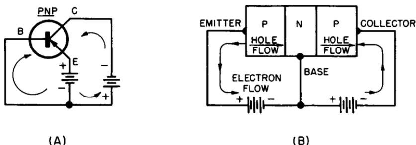
Fig. 1-14. A forward-biased pnp transistor with current flow shown.
