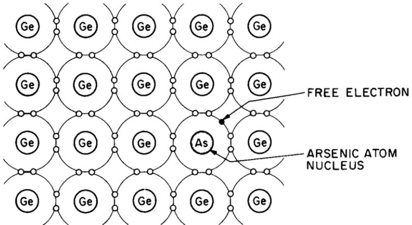
Fig. 1-5. When a germanium atom is replaced by an arsenic atom, a free electron remains. This is known as n-type donor germanium.
