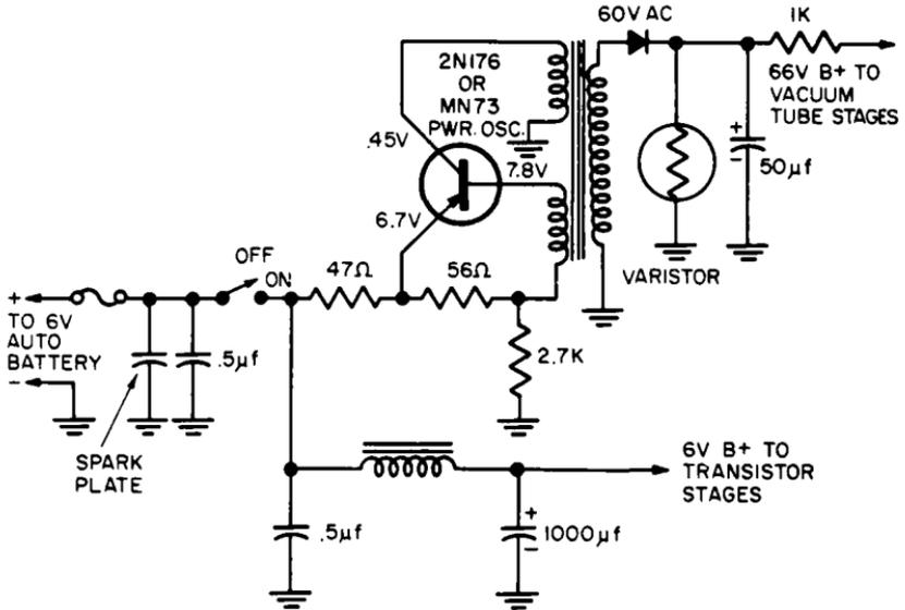
Fig. 9-8. The Motorola model 406 AM auto radio is a typical circuit, used in hybrid auto radios (operated from a 6-volt battery) to increase the voltage necessary for the vacuum tube circuits. Note the use of the varistor for voltage regulation.
