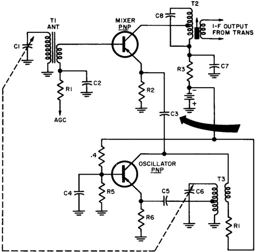
Fig. 6-6. An example of a mixer-oscillator arrangement using capacitive coupling of the oscillator signal to the mixer.
