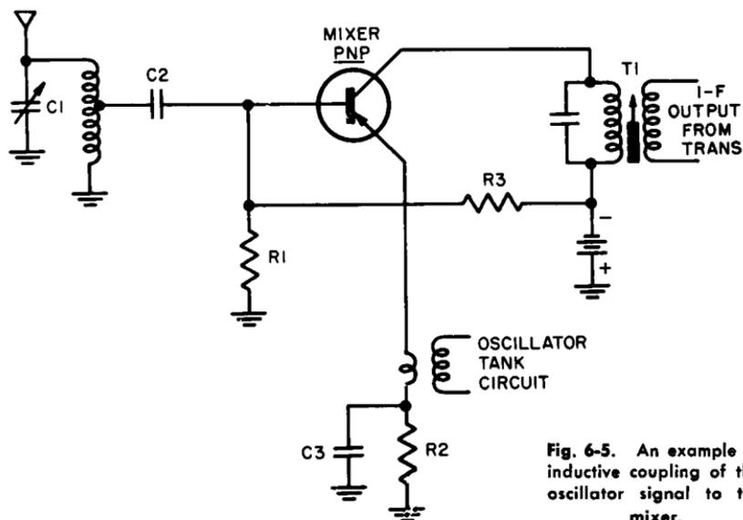
Fig. 6-5. An example of inductive coupling of the oscillator signal to the mixer.
