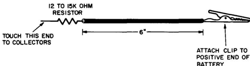
Fig. 10-1. Test lead for signal tracing transistorized radios using the click test method.
