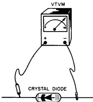
Fig. 7-10. Checking the back resistance of a crystal diode.
