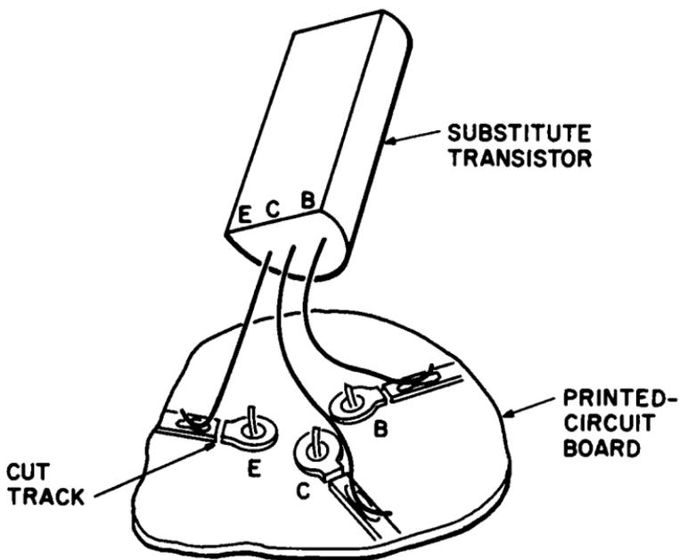
Fig. 10-16. Easy substitution of new transistor in circuit by leaving old transistor in place, cutting tracks, and soldering replacement to tracks.
