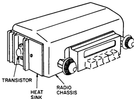
**Fig. 9-10.** The power audio output transistor(s) is most often mounted on the outside of the receiver case in a special heat-dissipating device.
