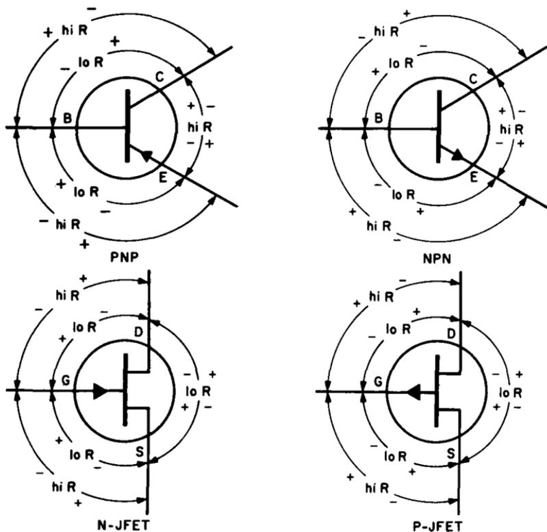
Fig. 10-14. Resistance readings for low-power type transistors.
