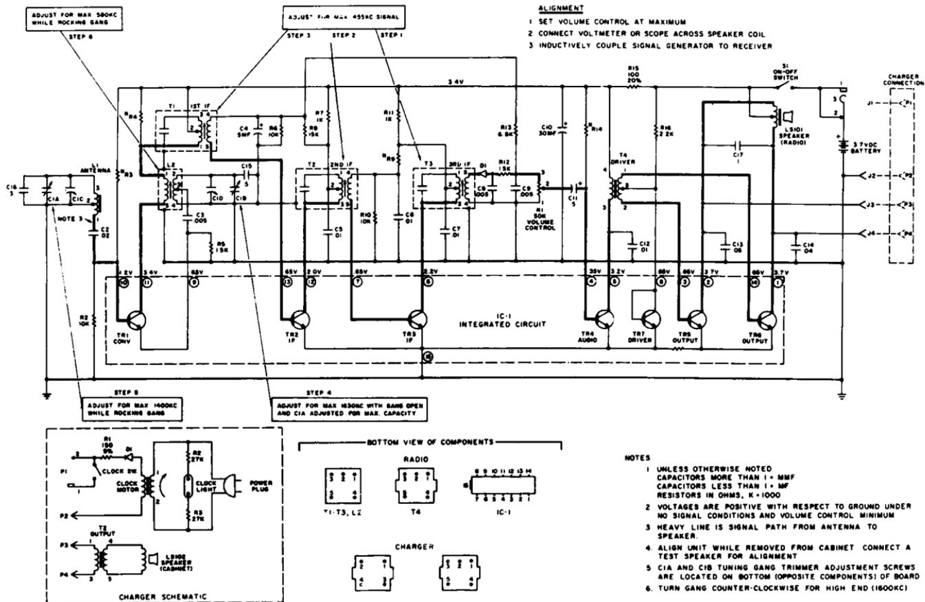
Fig. 8-9. GE model C2450 integrated circuit receiver, with all transistors in one integrated circuit, IC-1.
