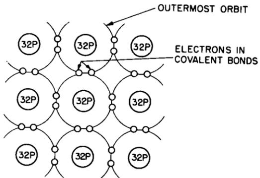
Fig. 1-4. A germanium crystal is composed of atoms in a covalent state. It is, therefore, a nonconductor.
