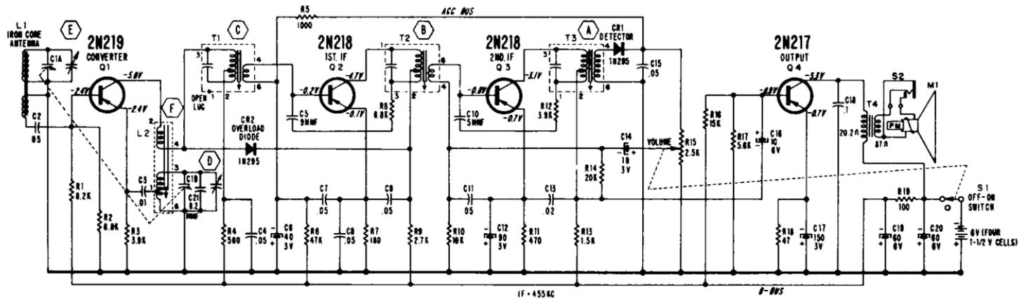
Fig. 8-3. Representative four-transistor superheterodyne AM portable radio receiver—Admiral 4P2 series. The second i-f amplifier is a reflexed circuit also acting as the audio driver stage.
