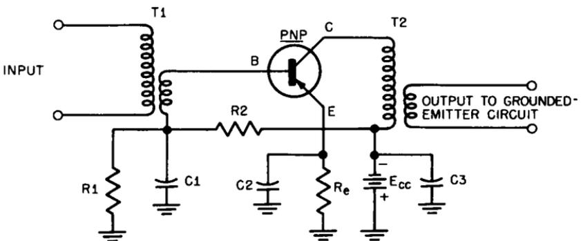
Fig. 3-11. A basic transformer-coupled amplifier.
