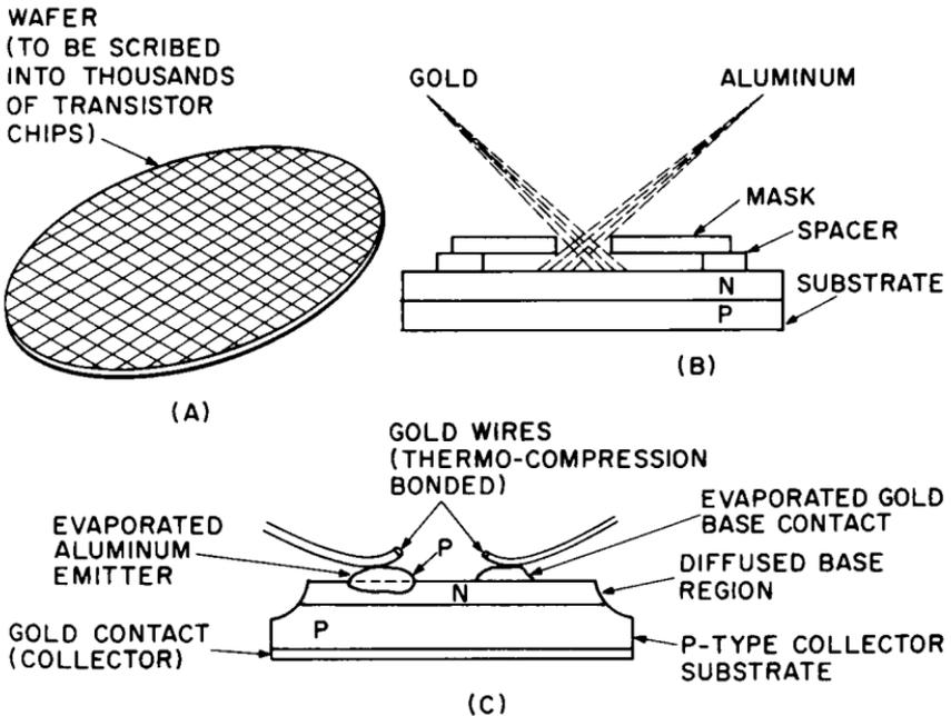
Fig. 1-18. Fabrication of diffused-base mesa transistor: (A) the wafer, (B) cross evaporation of emitter region and base contact, and (C) cross section.
