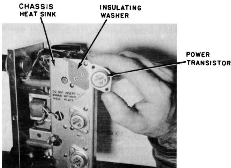
Fig. 4-2. When installing a power transistor, be sure that the insulating washer is placed between the transistor and chassis heat sink.
