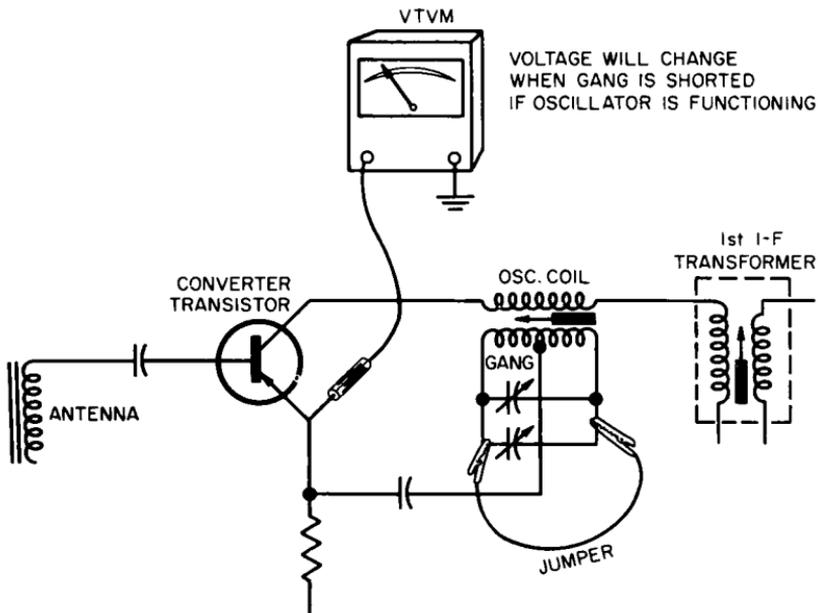
Fig. 6-8. Quick check for oscillator operation.
