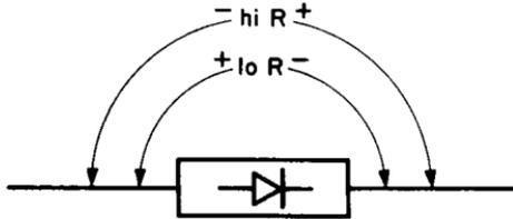
Fig. 10-17. Resistance test of a diode with an ohmmeter.
