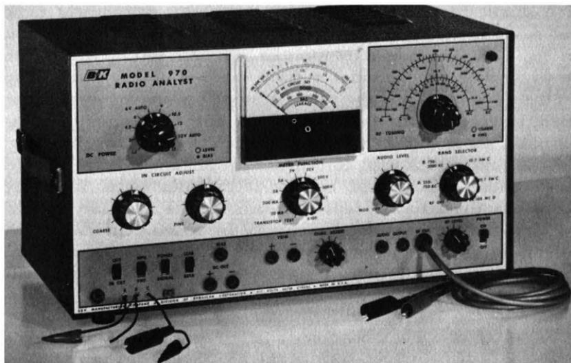
Fig. 11-9. B & K model 970 Radio Analyst (including a d-c power supply, volt-amp-ohmmeter, signal generator, and transistor tester).
