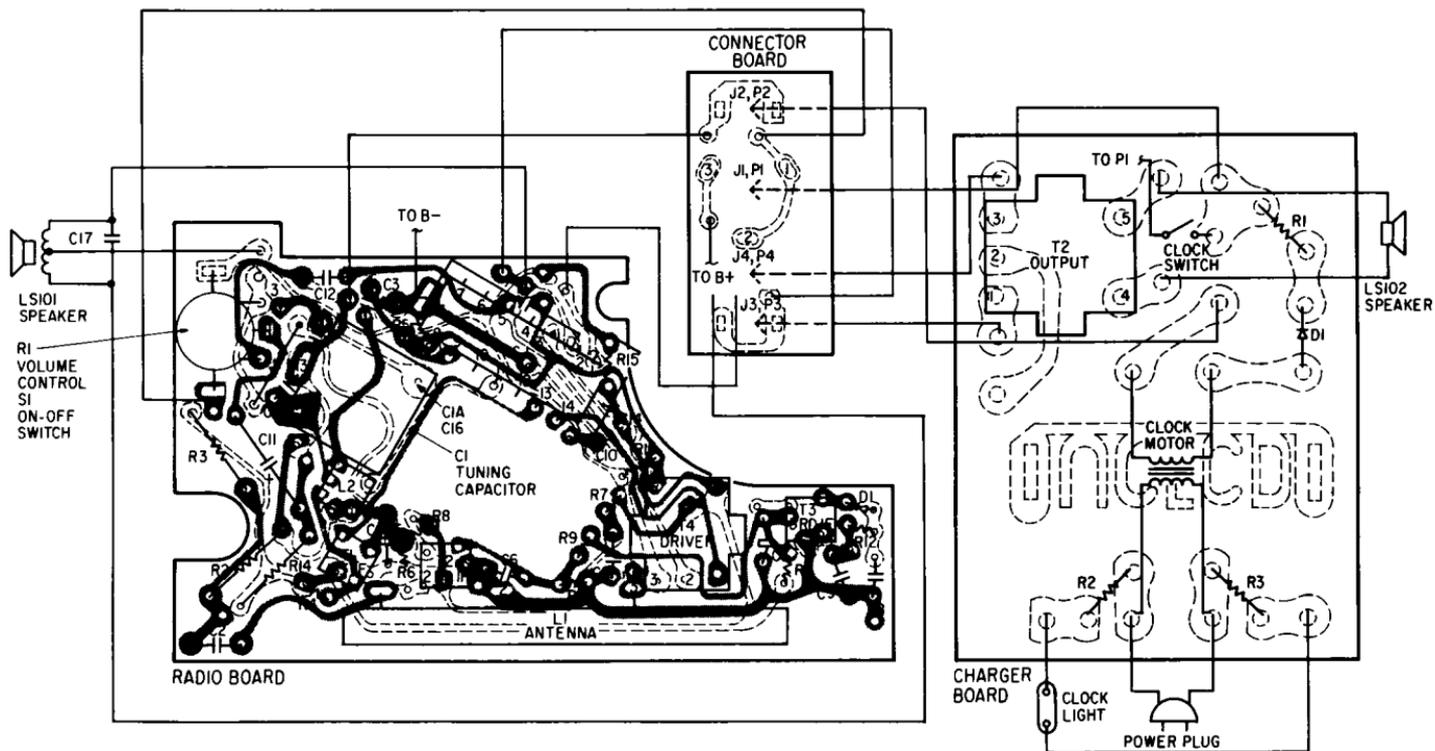
Fig. 8-10. Printed circuit and component layout for GE C2450 integrated circuit receiver.
