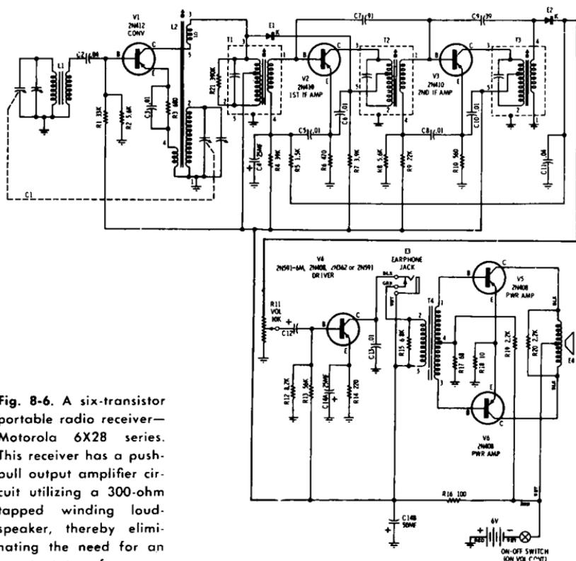
Fig. 8-6. A six-transistor portable radio receiver—Motorola 6X28 series. This receiver has a push-pull output amplifier circuit utilizing a 300-ohm tapped winding loud-speaker, thereby eliminating the need for an output transformer.
