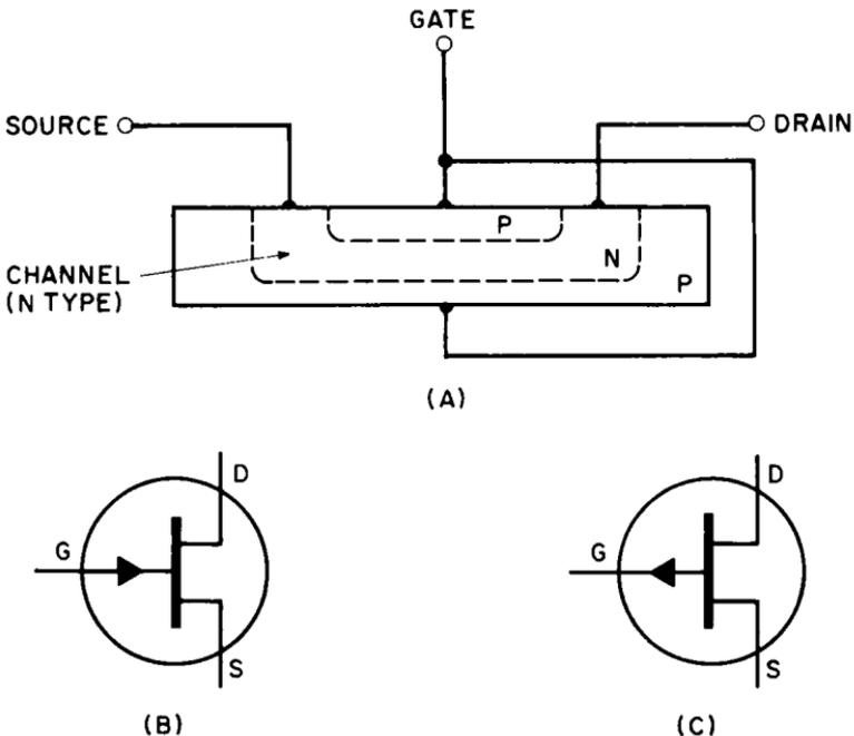
Fig. 1-20. Junction field-effect transistor (J-FET), n-channel type: (A) construction, (B) n-channel schematic symbol, and (C) p-channel schematic symbol.
