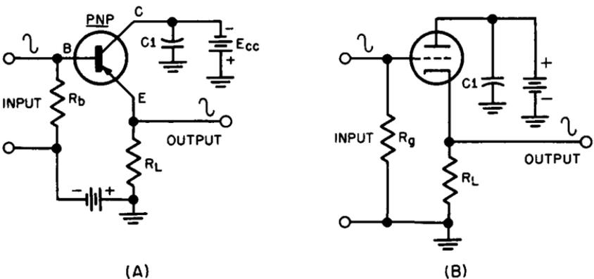
Fig. 3-10. (A) Grounded-collector transistor amplifier circuit compared to (B) cathode-follower vacuum tube amplifier circuit.
