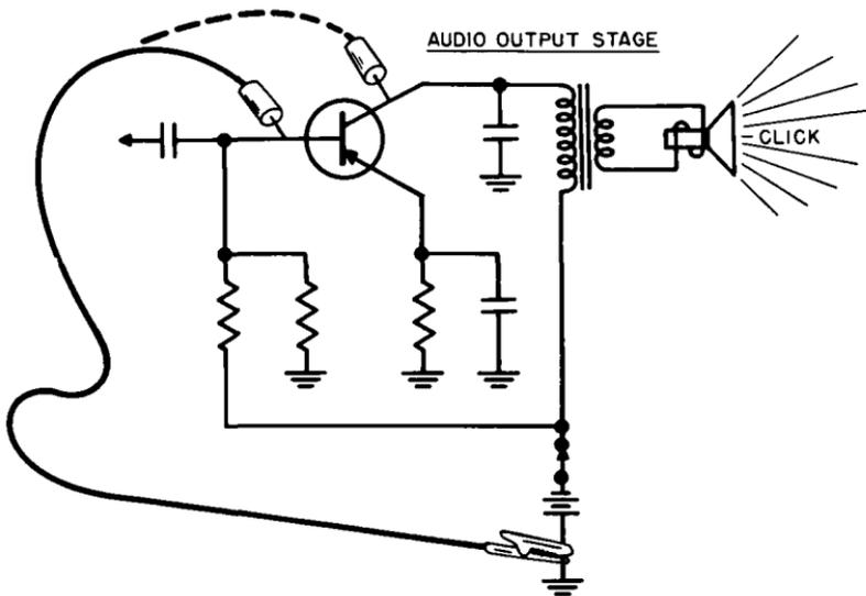
Fig. 4-11. A quick check of the audio driver stage.
