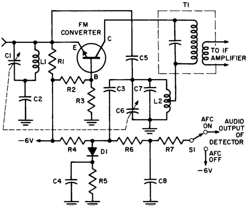
Fig. 6-7. Representative AFC circuit used to control FM oscillator frequency.
