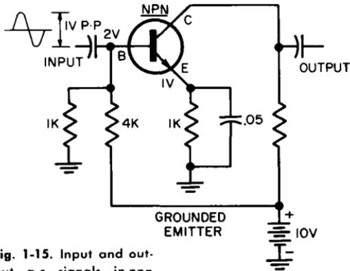
Fig. 1-15. Input and output a-c signals in npn grounded-emitter circuit.
