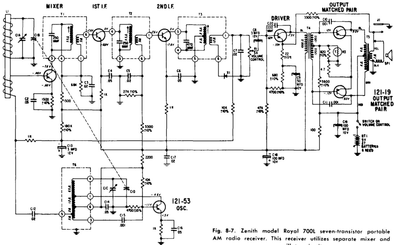
Fig. 8-7. Zenith model Royal 700L seven-transistor portable AM radio receiver. This receiver utilizes separate mixer and oscillator circuits.
