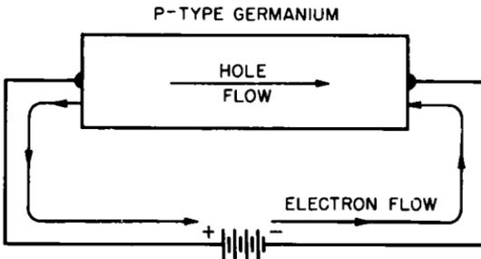
Fig. 1-8. Conduction in p-type germanium is by hole movement from the positive side of the battery to the negative side.
