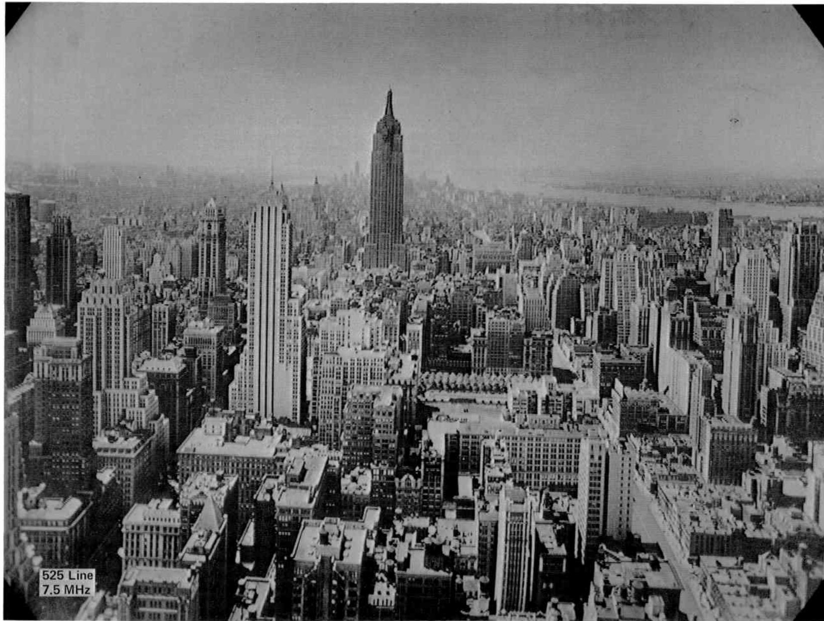
Fig. 61 TV reproduction of master print, 525 lines, 7 MHz, 30 frames/sec, 4.5-inch image orthicon. Photographed from 17-inch CRT.
