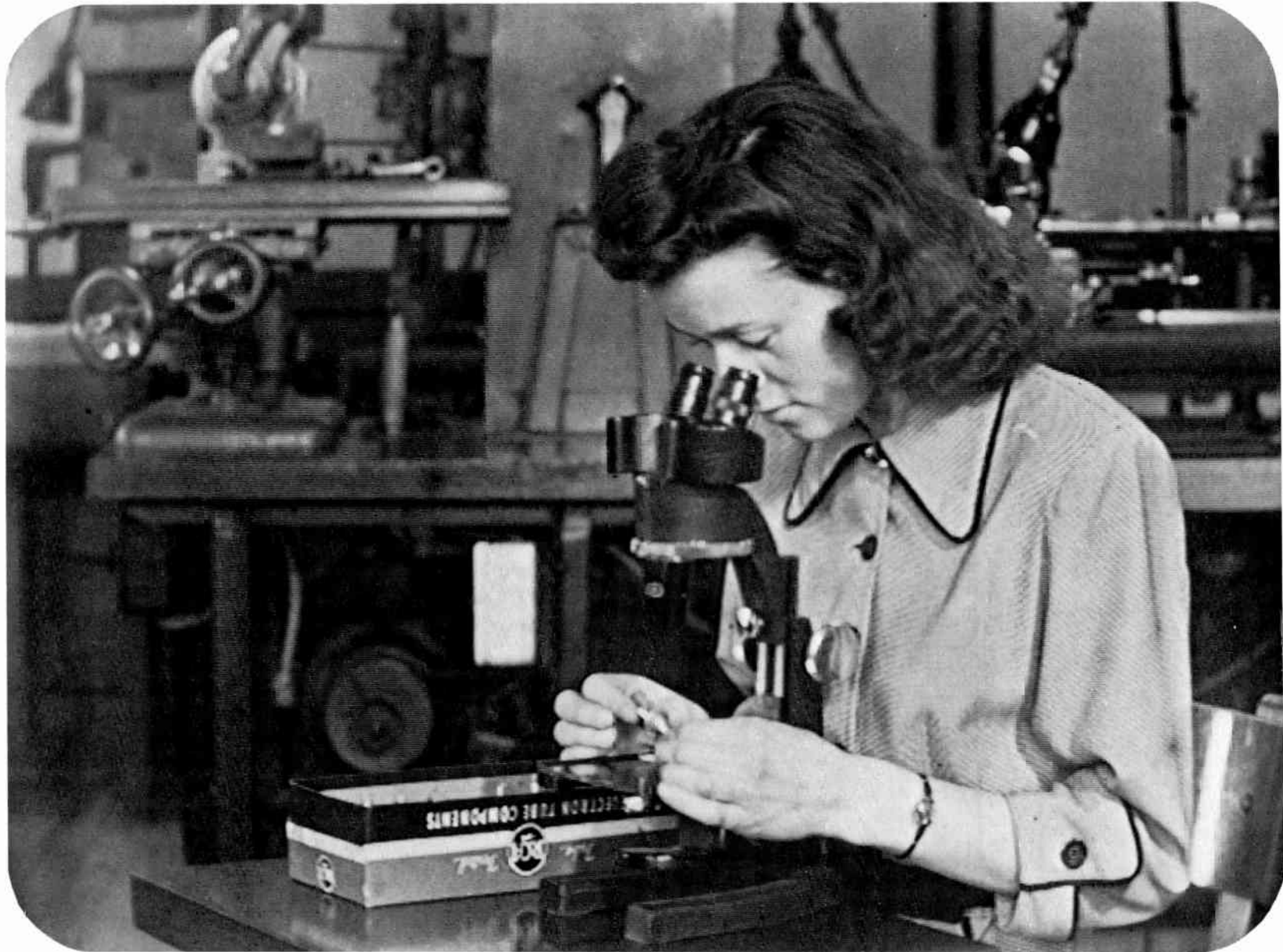
Fig. 31 Live pick-up with 4½-inch image orthicon, 525-lines, 8-MHz, 30 frames/sec; photograph of 16-inch cathode-ray-tube image.
