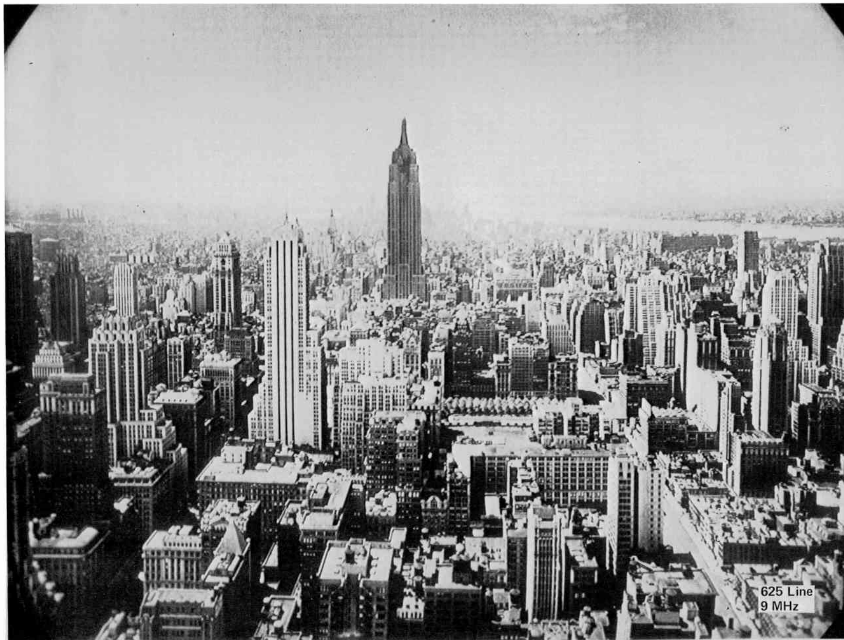
Fig. 60 TV reproduction of master print, 625 lines, 9 MHz, 30 frames/sec, 4.5-inch image orthicon. Photographed from 17-inch CRT.
