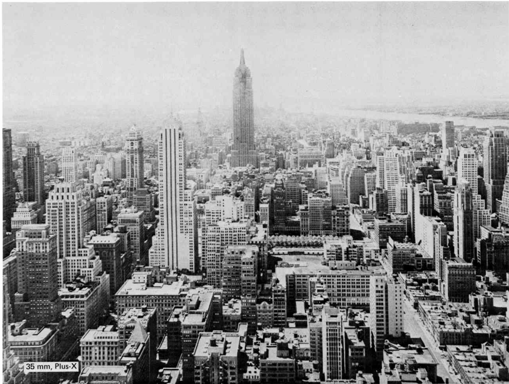
Fig. 64 Reproduction of 8X10-inch master print by 35-mm motion-picture frame; medium-speed Plus-X film (ASA 120). Magnification from film to reproduction shown here: 10.5.
