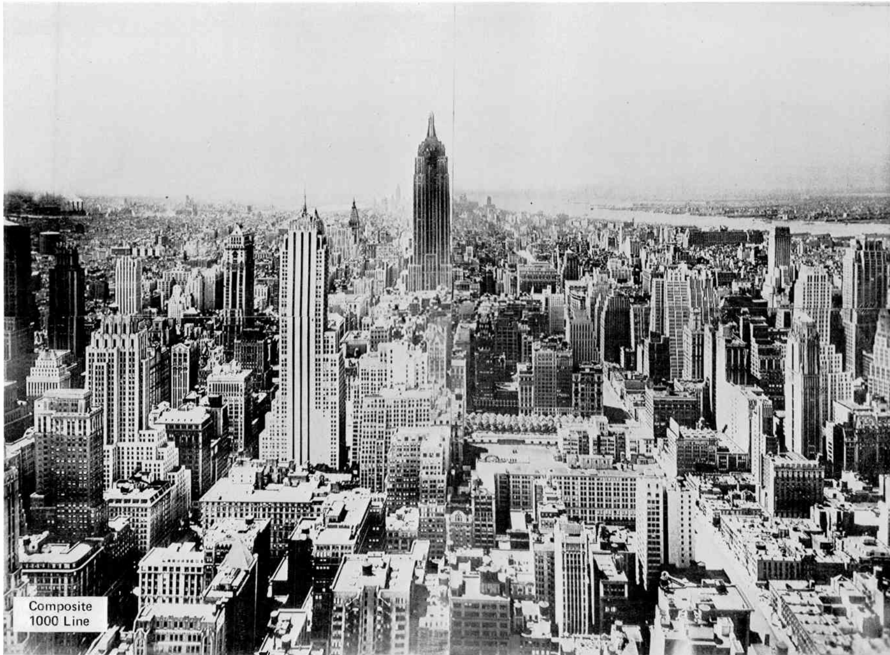
Fig. 59 Composite 1000-line TV picture ( N_o = 650 ) assembled from four 500-line 7 MHz, 30 frames/sec. TV pictures.
