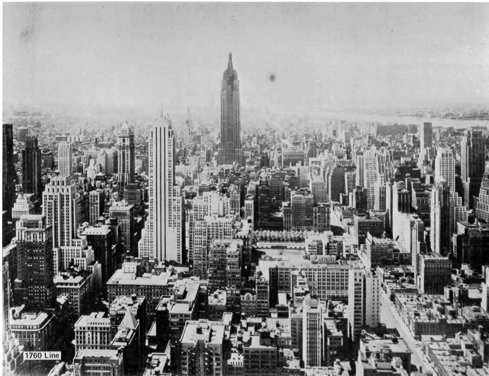
Fig. 57 TV reproduction of master print, 1760 lines, 60 MHz, photographed with 4.5-inch return-beam vidicon on 17-inch CRT. The photographic copy used to make the reproduction shown here has a resolution of 1500 lines, N_o = 600 .
