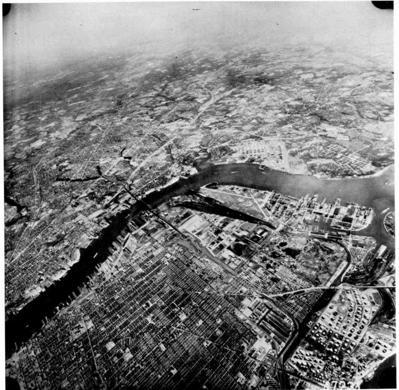
Fig. 54 TV reproduction of aerial photograph; 4\frac{1}{2} -inch return-beam vidicon, 1870 lines, 20 frames/sec, 3:1 interlace, 60-MHz-bandwidth; photographed from 17-inch cathode-ray tube. Resolution is bandwidth limited. Scanning lines are not visible because of spot-wobble applied to the beam of the CRT.
