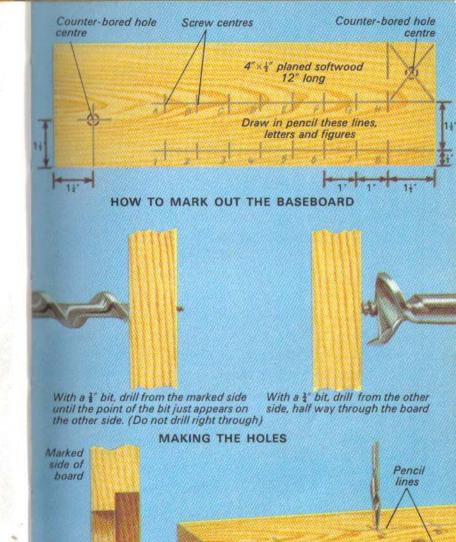
Section of the counterbored holes Use a gimlet or bradawl to make holes for the screws. (Do not fully tighten the screws at this stage)
