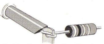
3) Put the hot bit of the iron firmly upon the joint and allow a few seconds for the joint to heat up. Take care. The soldering iron bit and metal shaft can burn the skin!
