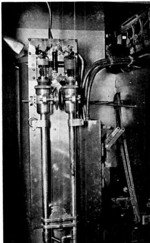
FIG. 157.—Transmission-line controlled oscillator of station W2XAB, New York. Note that the anodes of the tubes are enclosed in the transmission-line conductors, which serve to conduct the cooling water to them.
