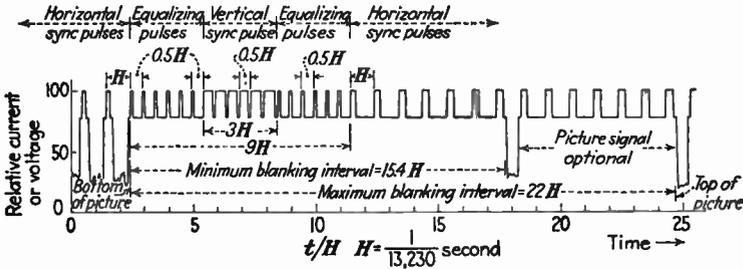
FIG. 100A.—The R.M.A. Standard Video Signal during the vertical blanking (field retrace) period, representing the beginning of the first field.
