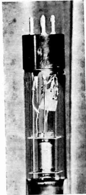
FIG. 200A.—Ion trap used to eliminate ion spot in electrostatically focused, magnetically deflected tube. The cathode (top) is inclined to the axis of the tube.
