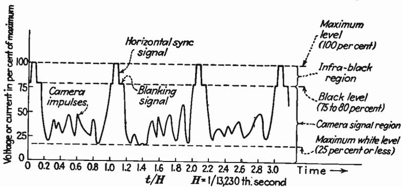
FIG. 98.—Three lines and blanking periods of the R.M.A. Standard Video Signal.
