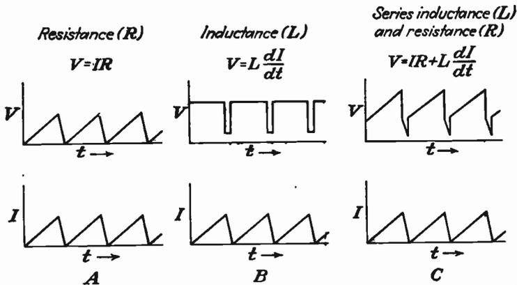
FIG. 81.—Saw-tooth waves of current produced by voltage waves in a resistive circuit (A), an inductive circuit (B), and a combination resistive-inductive circuit (C). The voltage wave (C) is that commonly applied to the deflecting coils in magnetic deflection systems.
