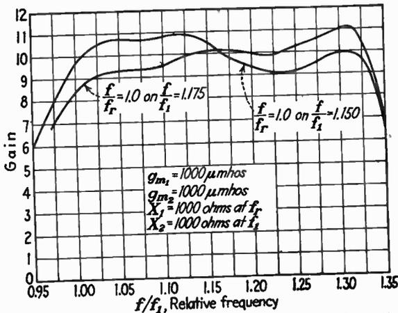
Fig. 186.—Examples of mid-band compensation obtained from the curves in Figs. 182 and 166.
