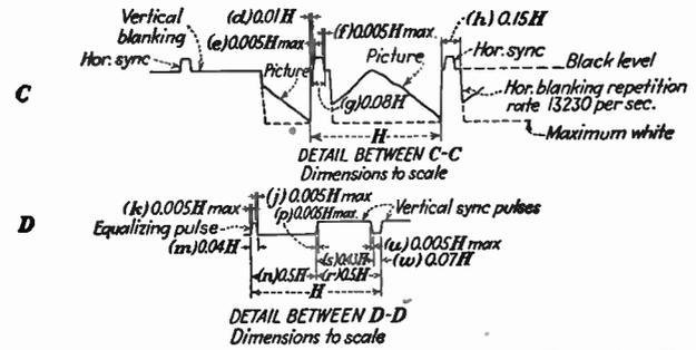
1. Diagram C shows enlarged detail view of signal in view B between lines C-C
