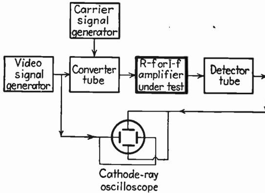
FIG. 186.—Method of investigating phase response of r-f or i-f amplifiers.
