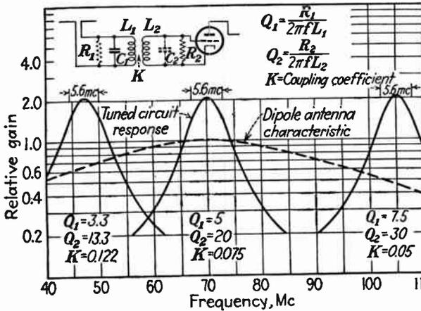
FIG. 175.—Response of r-f stage to three channels, computed by Lyman.
