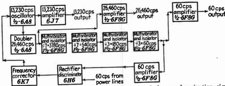
FIG. 248.—Block diagram of the timing unit of the synchronization signal generator, which produces 60-c.p.s. and 13,230-c.p.s. timing impulses and coordinates them with the power supply.
