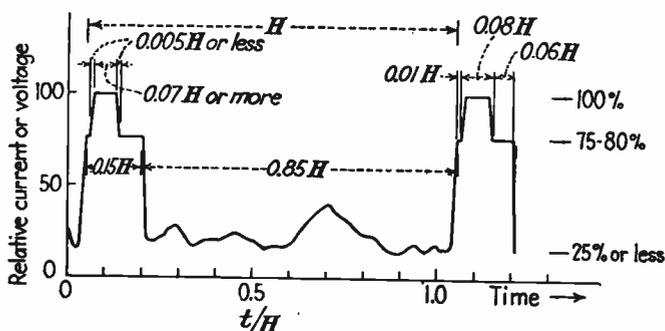
Fig. 99.—Dimensions of the blanking and synchronizing signals (R.M.A. Standard) in terms of the line-scanning interval  $H$  ( $= 1/13,230$ th sec.).
