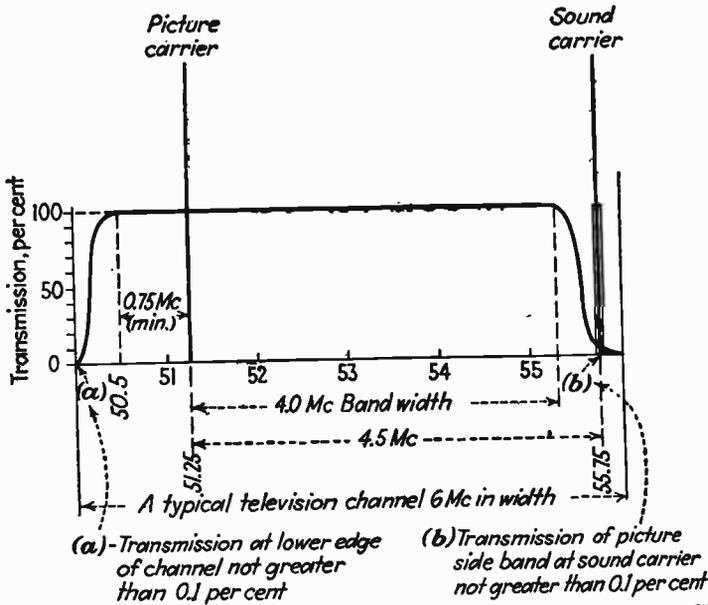
Fig. 813.—Reprint of R.M.A. Standard T-115, Transmitter Amplitude Characteristic, as defined by the R.M.A. Television Committee.
