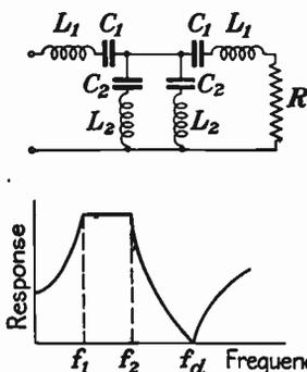
FIG. 179.—Elementary band-pass filter (*m*-derived) and idealized response characteristic.
