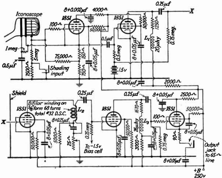
Fig. 242.—Complete diagram of iconoscope preamplifier.
