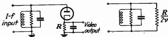
FIG. 191.—Actual and equivalent circuits of the video detector, from i-f input to video output.
