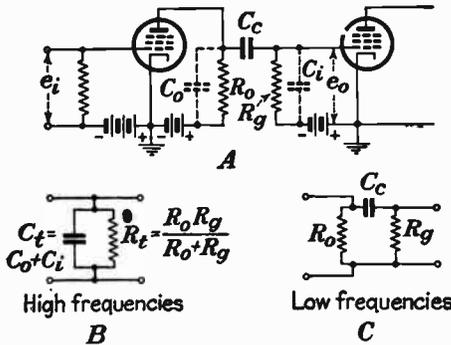
FIG. 117.—Uncompensated amplifier coupling connection (A), with equivalent circuits at high (B) and low (C) frequencies.
