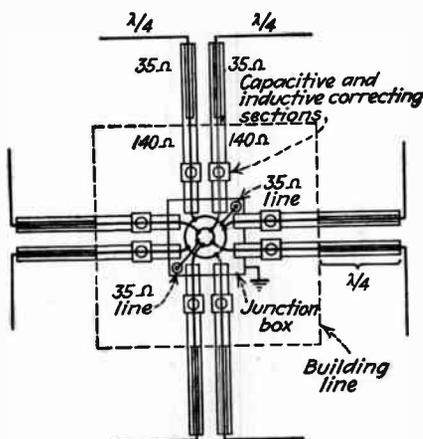
FIG. 168.—Arrangement of transmission lines and crossed dipoles in the radiator array used at station W2XAX, the Columbia Broadcasting System's transmitter in New York City.
