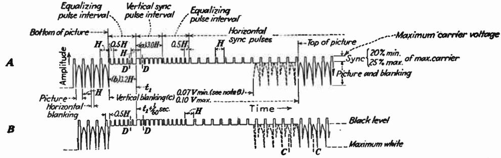
Diagram A and B show blanking and synchronizing signals in regions of successive vertical blanking pulses. (Horizontal dimensions not to scale. All dimensions are from black level unless otherwise specifically indicated)
