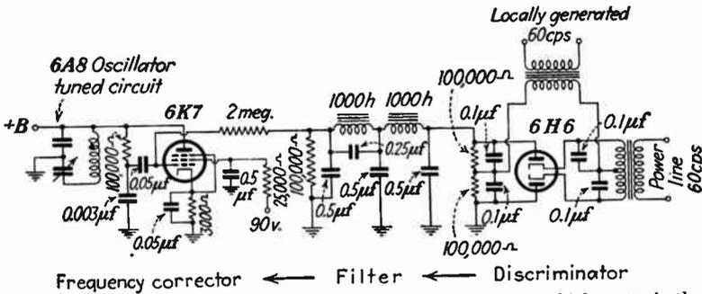
FIG. 250.—Frequency-correction circuit of the timing unit, which controls the frequency of the 13,230-c.p.s. oscillator when a difference develops between the 60-c.p.s. timing signal and the 60-c.p.s. power-supply frequency.
