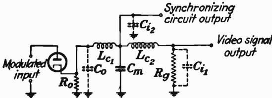
FIG. 129.—Filter coupling (two series-peaking coils in cascade) applied to a detector load circuit. Two sources of the signal are made available without loading the circuit with additional capacitance.
