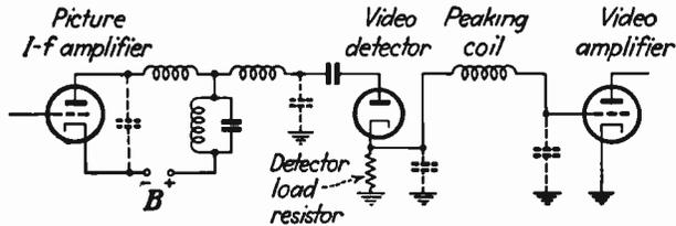
FIG. 139.—Typical video detector circuit.
