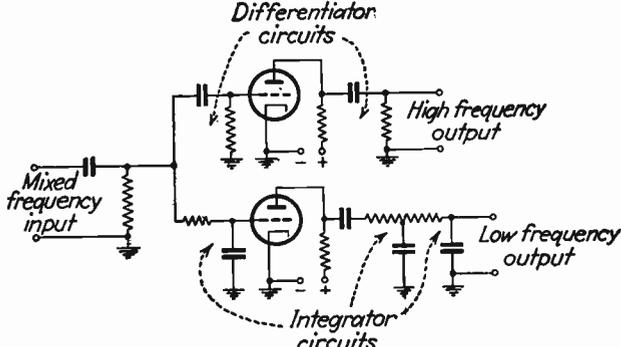
FIG. 96.—Typical waveform separator circuit, employing integrators and differentiators in the grid and plate circuits of two triode tubes.
