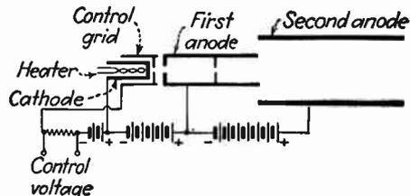
Fig. 61.—Elements of a typical electrostatic electron gun which employs two electron lenses for focusing the electron beam, and a control grid for varying its power density.
