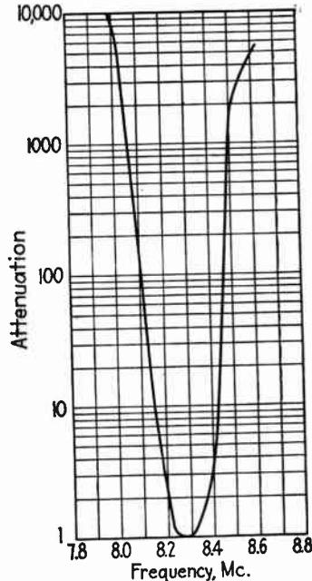
FIG. 287.—I-f sensitivity curve of sound channel of receiver shown in Fig. 284.
