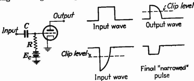
FIG. 253A.—The narrowing function in wave-shaping circuits. The initial square wave is passed through the differentiating circuit ( $RC$  circuit, left) and clipped (upper right). Then the portion above the clip level is amplified and clipped again. The final pulse is thus narrowed but not delayed.
