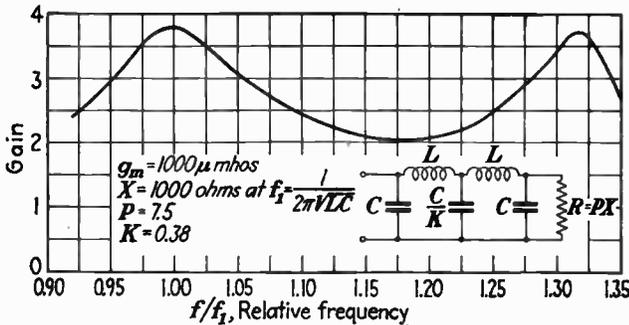
Fig. 182.—Response curve of the capacitively coupled band-pass circuit shown in the inset (after Sealey and Barden).
