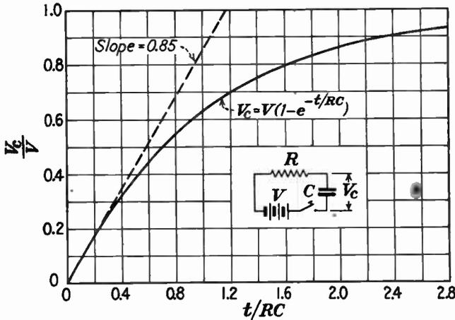
FIG. 76.—Capacitance charge-*vs.*-time curve (solid line) in the series resistance-capacitance circuit shown in the inset. The dashed line represents a linear relation (slope 0.85) somewhat below the initial slope of the charge curve (cf. Fig. 77).
