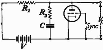
FIG. 82.—Peaking circuit used to produce the voltage waveform of Fig. 81C. The combination of  $R_2$  and  $C$  acts to produce a voltage wave, part impulse, part saw-tooth, necessary to produce a saw-tooth of current in an inductive-resistive circuit.
