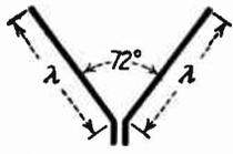
FIG. 171.—V antenna, consisting of two full wave sections, which displays maximum sensitivity along the bisector of the angle between the elements.
