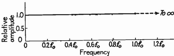
FIG. 104.—Ideal amplitude-frequency response characteristic, which displays no discrimination in its response to any frequency from zero to infinite frequency.
