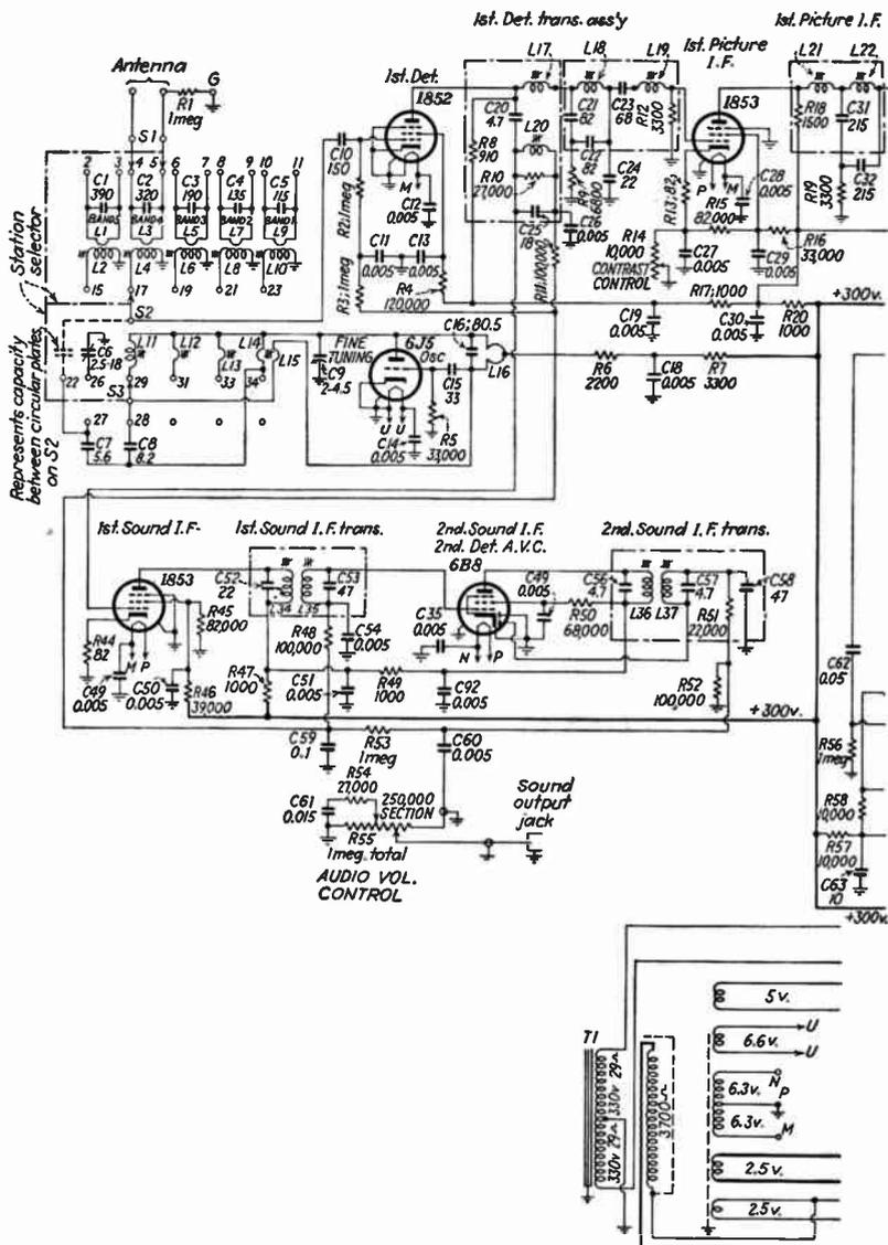
Fig. 279.—Complete circuit diagram of the
