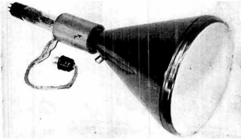
FIG. 85.—Typical magnetically-deflected picture tube. The scanning yoke (cylindrical structure) contains two sets of coils which produce horizontal and vertical deflecting fields at right angles to the axis of the tube.
