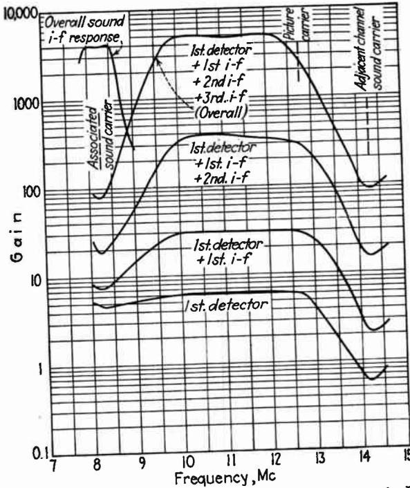
FIG. 280.—Cumulative response curves of the receiver shown in Fig. 279, at output of first detector and successive i-f stages. Note improvement in sound channel attenuation as the number of coupling circuits increases.
