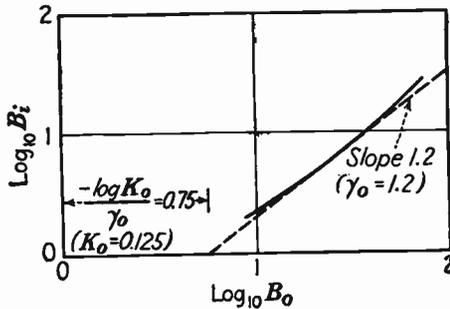
FIG. 198.—Transfer characteristic of Fig. 197 plotted in logarithmic coordinates. The gamma is the slope of the straight line (dashed) which most nearly fits the actual curve. The proportionality constant is determined from the intercept of the straight line with the  $\log_{10} B_o$  axis.
