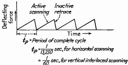
FIG. 78.—Saw-tooth waveform of deflecting force, required to produce a scanning pattern of uniform horizontal and vertical scanning velocities.
