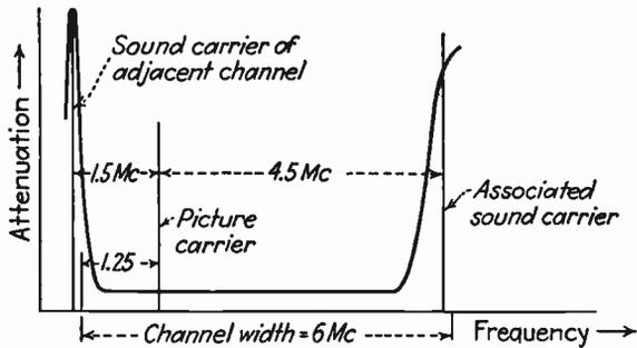
FIG. 162.—Attenuation characteristic required to transmit the vestigial sideband carrier according to the R.M.A. transmission standards.
