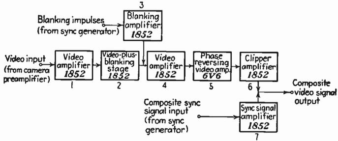
FIG. 243.—Block diagram of control amplifier (blinking and mixing amplifier) which produces the composite video signal from its camera, blanking, and synchronization components.
