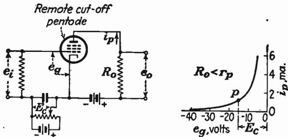
FIG. 137.—Typical distorting amplifier circuit used for obtained nonlinear reproduction (“gamma-control” amplifier). By adjusting the bias voltage  $E_c$ , different portions of the  $i_p$ - $e_g$  operating characteristic may be chosen.
