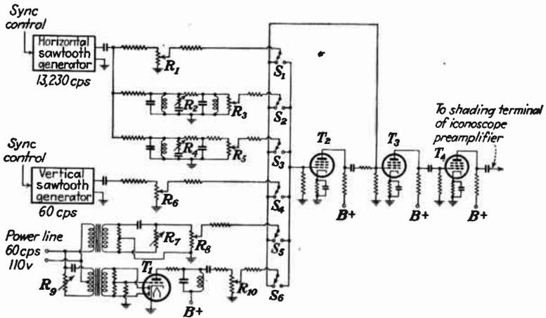
FIG. 256.—Shading correction generator which produces synchronised wave shapes for application to the iconoscope preamplifier (Fig. 242) to correct irregularities in shading due to secondary electron redistribution.
