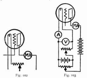
control or a voltmeter may be substituted therefor with better results, as already stated. Note in Fig. 100 that the voltmeter is connected directly across the filament between the rheostat and the tube. Fig. 102 indicates how a milliammeter should be inserted in the plate circuit.
