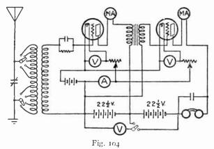
receiving circuit. It is not essential that the two filament voltmeters be used as shown in the diagram, but in a manner similar to that shown for using the plate voltmeter on either the detector or
