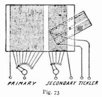
the minds of the novice but its operation can be easily understood by the following analogy; in the gasolene motor of an automobile it is known that there is plenty of unused fuel ejected from the muffler. Now, if it were possible to sift out the good unused gas from the exhaust and feed it back into the motor to be used over again, this process could be called a "feedback." This is exactly what happens in the regenerative circuit. The tickler coil is affected through induction in a way
