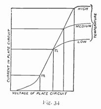
has thence no further influence on the flow. We can interpret this result as follows: Up to the point (m) there is a fixed relation between voltage and current, that is, the tube follows Ohm's law. From (m) to (n) the resistance of the space between the filament and the plate has somehow been decreased, and the current flows more easily. Beyond (n) the resistance increases, however, to such an extent that no additional pressure can force a greater current across the space. The explana-
