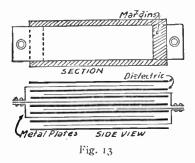
plates that were charged positively will now discharge back through the circuit. Thus an alternate charging and discharging is produced which corresponds to the phase changes in the circuit.
