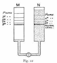
tanks, M and N connected through a water pipe in the manner shown, the stopcock corresponding to the gap. These can then be compared to two
