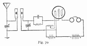
detector. This circuit is highly sensitive, and through the wide range obtainable in the coils
