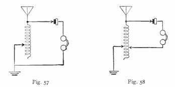
second slide instead of the same one that the ground wire is. The slide to which the ground wire is connected is used for adjustment of wavelength in the antenna circuit, but the second slide permits an adjustment of the crystal and phone circuit that will materially improve the reception.
