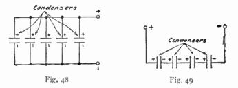
the figure all have the same capacity, the capacity of the whole will then be one fourth of that of each. The above relations can be expressed as follows:
