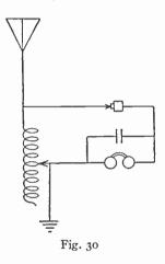
the reception is thus intensified. As two sensitive spots have to be found simultaneously, this type requires a finer adjustment, and is therefore not suited for instruments of the portable type, or that have to stand any amount of rough handling.
