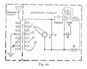
wavelength as the primary or antenna circuit. It will be noticed that a condenser "C" is shunted across the secondary coil; the capacity of this need not be more than .0005 microfarads. If the desired maximum wavelength in meters is known, the required inductance in the secondary can be calculated from the formula
