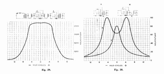
We will now consider a complete receiver made up of the above described aerial band pass filter, the valve plate band pass filter, and between the second valve and the detector valve, the simple H.F. transformer. Figure 29 shows this, and the curve for  $\frac{E}{c}$  the total amplification. We have clearly, in such a combination, obtained something very closely approaching our ideal compromise.
