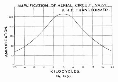
(a) When the resistance R2 of the first circuit is 20 ohms and R3 of the second is 50 ohms.
