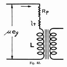
The valve and transformer become equivalent to the above figure.
