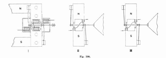
Inductor Speaker. The second type of speaker, Figure 106, is known as the "inductor speaker."
