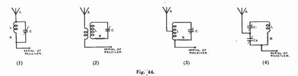
In Figure 44 (1), (2), (3), and (4) a tuned circuit (L, R, and C) is tuned to the unwanted station. The aerial is connected to some point on the circuit, and from some some other point a connection is brought to the aerial connection of the set. We have found, both by calculation and by measurement, that the simplest direct form (1) is *not less* effective than the others, and so we shall deal with it alone.
