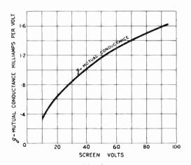
Fig. 35. S4V Valve. Plate Volts 153. Grid Bias - 3 Volts.
