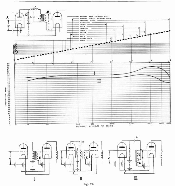
Combined Resistance and Transformer Coupling. II and III in Figure 76 shows two forms of this.
