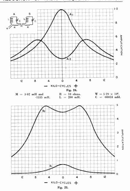
This is illustrated by curves in Figures 24 and 25. First, the coils A and B are far apart, so that A is hardly affected by the current induced in B. Curves A1 and B1 show the currents in the two circuits when 10 volts is produced in A. Notice that A1 and B1 are similar to standard resonance curves; in fact, A1 departs by only  $\frac{1}{2}\%$  from this, because the mutual inductance between A and B (the measure of the amount of the coupling) is only 133 microhenries.
