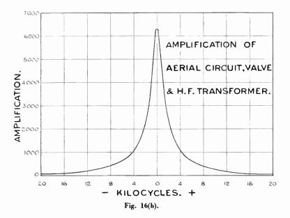
(b) When R2 is 16 ohms and R3 is 1.46 ohms.
