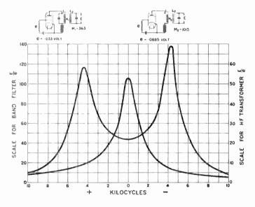
Fig. 34. Wavelength 2.270 metres. S4V Valve. Anode Volts = 162. G.B. Volts =  $-1\frac{1}{2}$ .  $L_1 = 4.610~\mu$ . Screen Volts = 70. g ... = .95.  $L_2 = 4.730~\mu$ .
