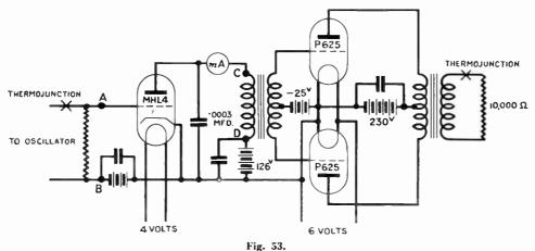
Set used for Anode Bend Measurements.
