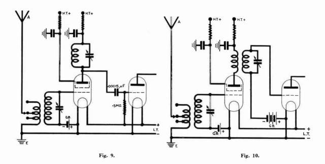
Figures 9 and 10 show the theoretical circuits for tuned anode and H.F. transformer coupling, using the screened grid valve.
