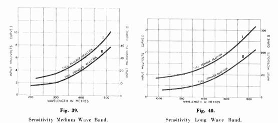
A.C. Mains 32. Input to Standard Aerial Modulation 30% to give 50 Milliwatts Output.
