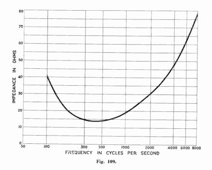
Its impedance varies least of any type over the frequency range. Figure 109 gives the impedance curve of the Ferranti Magno-dynamic Speaker.
