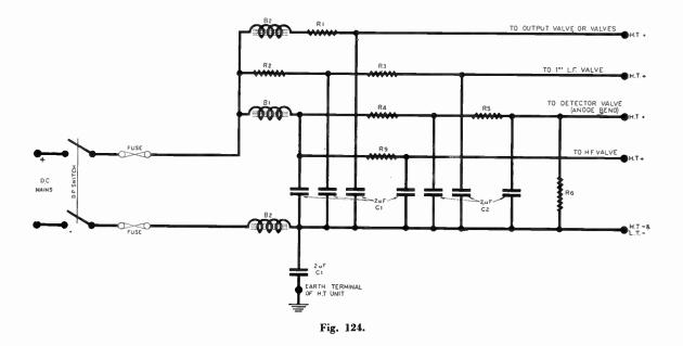
Figure 124 shows an H.T. supply unit for use on D.C. mains for supplying a set consisting of one ordinary high frequency transformer-coupled stage, an anode bend rectifier, and two audio frequency stages. The maximum output is 100 milliamps. through the "B.2" chokes.
