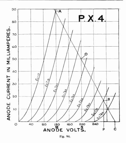
The whole matter can be better examined by changing our valve curves into another form. Figure 94 shows plate voltage, plate current curves, each for a definite grid bias, for the same PX4 valve.
