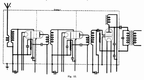
Figure 12 shows a circuit diagram with the above precautions.
