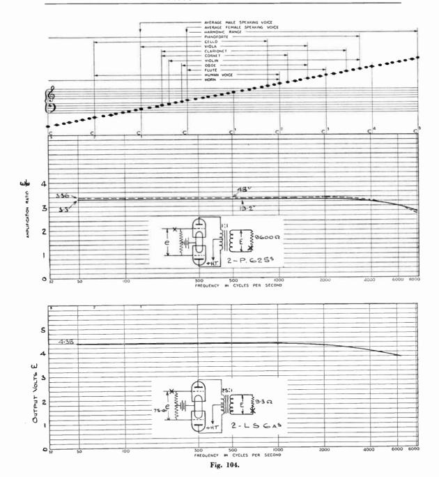
Push Pull Output Transformers. The last two formulæ apply equally to transformers in push pull provided Eg is the voltage applied across the two grids and Rp is the resistance of the two valves in series, or twice the resistance of one valve.
