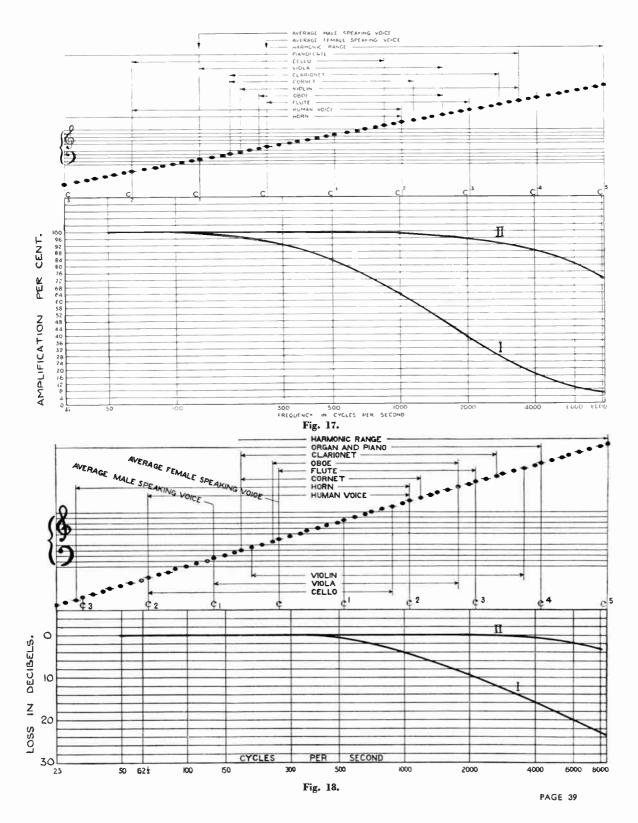
The figures given above are for one stage of radio frequency amplification, but all that has been said applies to two or more stages. Low resistance circuits, unless other correcting devices are used, mean the loss of the higher notes.
