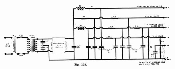
Figure 128 shows an H.T. supply unit for use on A.C. mains for the same purpose as the D.C. unit in Figure 127.
