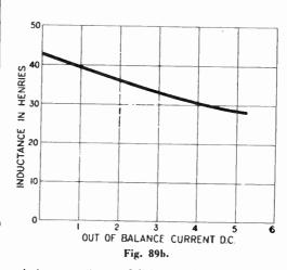
Inductance Curve of Primary of OPM1 Output Transformer, D.C. Resistance of Primary 180 ohms.
