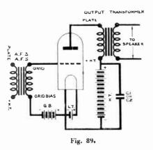
Output Transformers. Figure 89 shows the third method of connecting a speaker to a power valve by the use of what is known as an output transformer. The primary winding is connected in the plate circuit between the plate and the H.T. supply, and the speaker across the terminals of the secondary winding. Here, the speaker is completely isolated from the H.T. supply, so this is certainly the safest connection, and in receivers connected to mains this method should always be used where possible.
