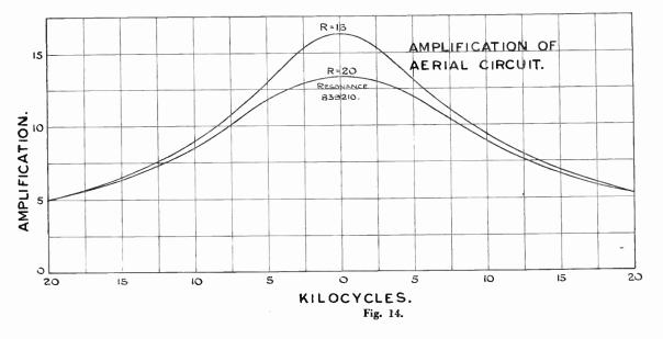
When the in-coming signal is 357 metres, that is the carrier wave, for R2 = 20 ohms, we have  $\frac{e_2}{e_1} = 13.4$ , but if the signal is 8,000 cycles more (353.63 metres) or 8,000 cycles less (360.44 metres),  $\frac{e_2}{e_1}$  is only 9.9. Hence the side bands
