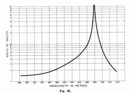
Wavetrap in A.C. 32 Mains. For New North Regional, 479·2 Metres. 101·6  $\mu$ h. R = 3 ohms. Measured Input for Constant Output.
