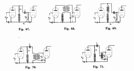
In circuits 67, 70, and 71, the impedance directly in the plate circuit is the resistance R. They differ from each other in the way in which the voltage across R is passed on to the next valve. In 68 and 69, an iron cored inductance is the impedance in the plate circuit.
