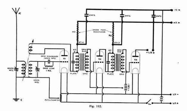
nearest to the transformer primary, to the H.T. negative; these condensers are usually incorporated in well designed sets. Figure 112 shows an ordinary 3-valve circuit, the anode feed resistances, and associated condensers, being more heavily lined. The principle on which this system depends is as follows:—
