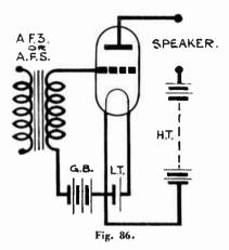
the H.T. battery is of small power and of a voltage not exceeding 150. It must not be used where higher voltages are utilised, or where the set is connected in any way to the electric light mains, unless the speaker is combined with the receiver in a cabinet so that it cannot be touched, on account of the danger should contact be made with either speaker terminals. The alternative methods will be shown later.
