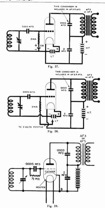
The other figures are for battery valves, and some positive bias is necessary. In Figure 57 it is obtained from a 1½ volt bias battery, the negative end of which goes to the negative filament and positive to the grid leak. In Figure 58 the return is taken to 2 volts positive for 4 or 6 volt valves, or direct to the positive of the filament for 2 volt valves.
