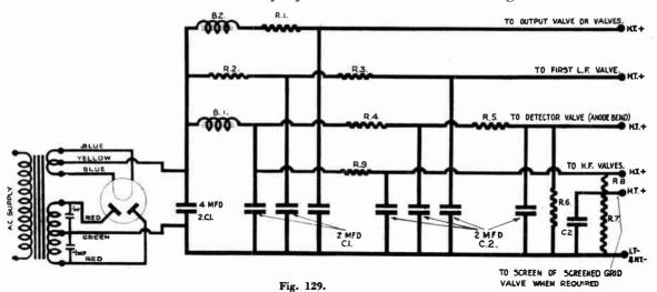
Figure 129 shows a similar unit but incorporating a valve rectifier instead of a metal rectifier:—
