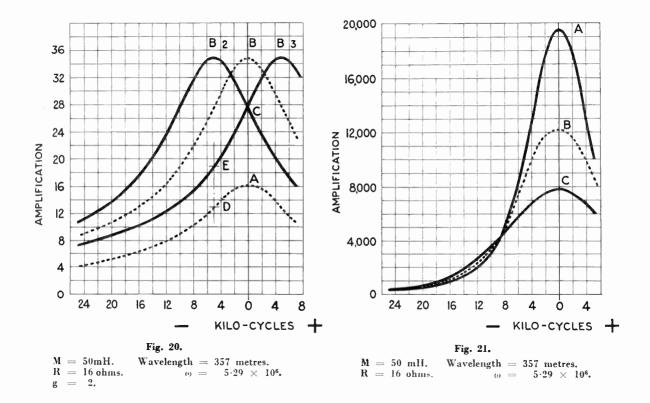
Figures 20 and 21 will enable the reader to visualise the process. In Figure 20, A is the amplification curve of the first circuit; B is that of each of the other circuits. But the
