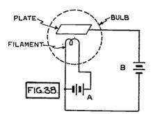
Fig. 38. Two-Electrode Vacuum Tube.
