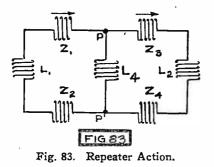
pedances to the left of PP' are equal to those on the right, no difference of potential between the points P and P' results from the electromotive forces induced in the main circuit from the output circuit of the amplifier.
