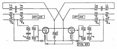
Fig. 85. Telephone Repeater Type 22.
