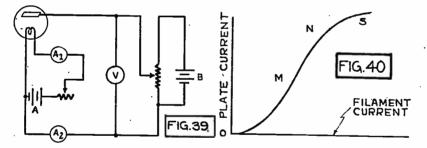
Fig. 39. Circuit for Obtaining Characteristic Curve of the Two-Electrode Vacuum Tube,
