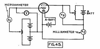
Fig. 43. Circuit for Obtaining Plate Current Grid Voltage Characteristic Curve of Three-Electrode Vacuum Tube.
