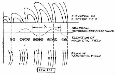
Fig. 131. Electromagnetic Field in One Direction About Vertical Wire Antenna.
