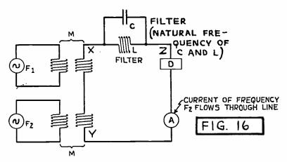
Fig. 16. Showing Use of Simple Filter.
