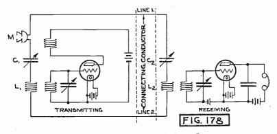
Fig. 178. Line Radio Telephone Set.
