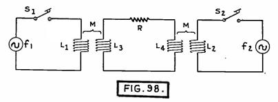
Fig. 98. Circuit Illustrating Heterodyne Action.
