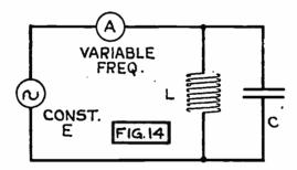
Fig. 14. Simple Parallel Circuit.
