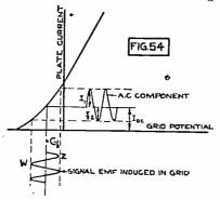
Fig. 54. Showing Rectification of Signal Current by Curvature of Plate Current Characteristic. plate current-grid voltage curve of such a tube, for the particular plate voltage and filament current used. The grid bias is represented by the abscissa  $G_B$ , and the constant plate current is represented by the ordinate  $I_{dc}$ . This, of course, refers to the stable condition of the tube with no current flowing in the antenna circuit.
