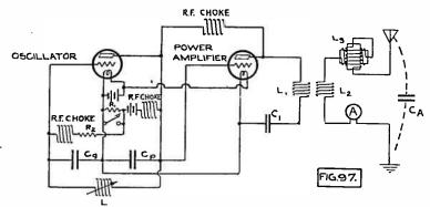
Fig. 97. Master Oscillator of Colpitts Type with Power Amplifier.
