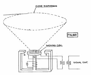
Fig. 160. Moving Coil or Dynamic Loud Speaker.
