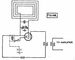
Fig. 148. Coil Antenna Circuit with Balancing Condenser, for Use as Direction Finder.
