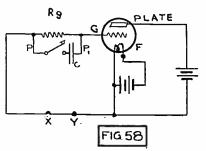
Fig. 58. Grid Condenser-Grid Leak Detector.
