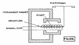
Fig. 159. Balanced Armature Loud Speaker.
