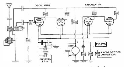
Fig. 173. Transmitting Circuit of a Broadcasting Station.
