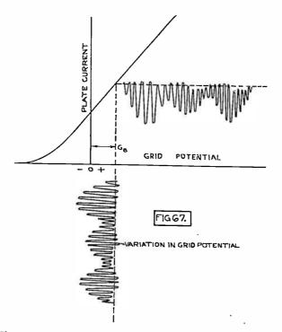
Fig. 67. Operation of Tube on Straight Section of Curve.
