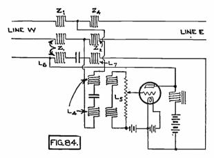
Fig. 84. Telephone Repeater Type 21.
