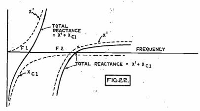
Fig. 22. Reactance Diagrams for Fig. 21, Showing Two Frequencies at Which Reactance is Zero.
