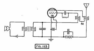
Fig. 123. Modulation of Output of a Tube Generator by Microphone Connected in Grid Circuit.
