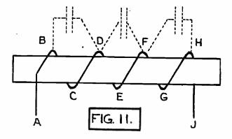
Fig. 11. Inductance Coil, Showing Distributed Capacity.
