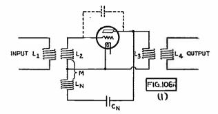
Fig. 106(1). Schematic Diagram of Rice Method of Neutralization.
