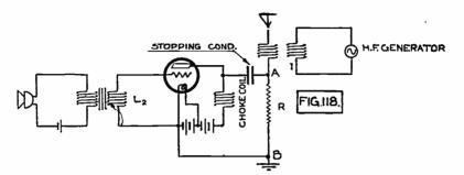
Fig. 118. Antenna Modulation.
