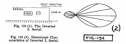
transmitting and receiving in various directions is graphically indicated by the length of the radius vector for any vectorial angle, shown in Fig. 134(2), which shows that the best transmitting and receiving direction is in prolongation of the horizontal wire toward the end to which the vertical wire is attached. The horizontal wire is known as the *aerial* and the vertical wire is known as the *lead-in*.
