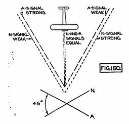
Fig. 150. Radio Beacon System for Aircraft.
