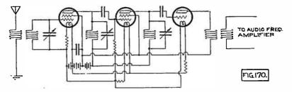
Fig. 170. Screen-Grid Tube Circuit.
