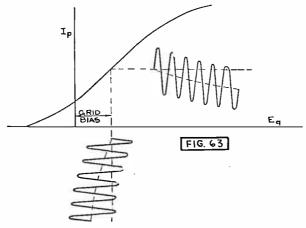
Fig. 63. How the Plate Current Changes with the Grid Potential.
