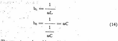
The susceptances  $b_L$  and  $b_c$  would, then, vary as shown in Fig. 15. The total susceptance is the algebraic sum of  $b_L$  and  $b_c$ .
