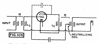
Fig. 105. Schematic Diagram of Hazeltine Neutralization.
