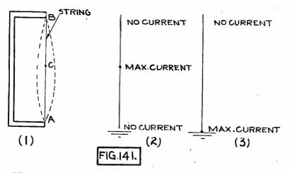
Fig. 141. Illustrating Similarity of Radio Aerial and Vibrating String.
