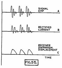
Fig. 55. Detector Action of the Vacuum Tube.
