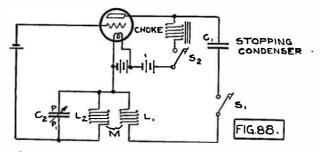
Fig. 88. Simple Oscillator-Modified Hartley Type.
