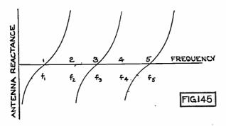
Fig. 145. Showing Relationship Between Antenna Reactance and Frequency.
