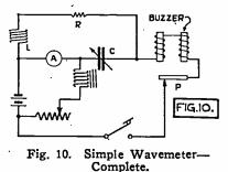
There is also a momentary surge of current through the condenser C, which charges the condenser to the battery voltage.
