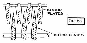
Fig. 155. Cross-Section of One Type Straight Line Frequency Condenser.
