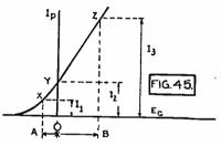
Fig. 45. Showing Grid Bias and Operating Point.
