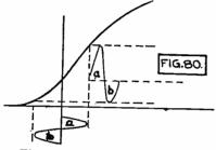
Fig. 80. Action of Tube with Non-Linear Characteristic.
