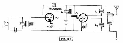
Fig. 125. Circuit for Radio Telephone Transmitter. Modulation by Variation of Power Input of Generator Tube or Heising Method.
