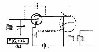
Fig. 106(2). Showing Method of Connecting Phasatrol to Prevent Oscillations in Radio-Frequency Amplifiers.
