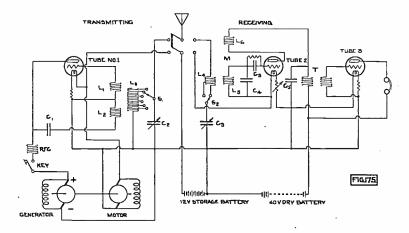
Fig. 175. Complete Transmitting and Receiving Set.
