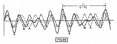
Fig. 99. How Two Oscillations Heterodyne to Produce a Third.
