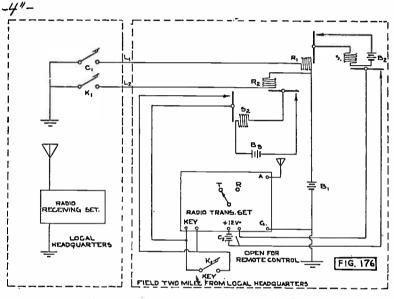
Fig. 176. Remote Control of Radio Set.
