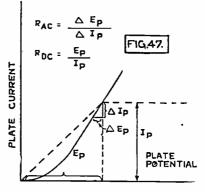
Fig. 47. Showing Difference Between A.C. and D.C. Resistance of Tube.
