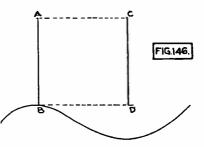
top ends are connected by a conductor, a current will flow through the rectangular loop circuit thus formed, and this current may be detected in the usual way. Obviously, in this case, the greatest difference of potential between corresponding points on AB and CD would be obtained when these two vertical wires are separated by one-half a wavelength.
