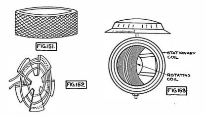
Fig. 151. Honeycomb or Lattice Wound Coil. Fig. 152. Stagger Wound Coil. Fig. 153. Variometer.
