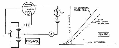
Fig. 49. Circuit for Study of Effects of Resistance in Plate Circuit.
