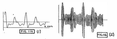
Fig. 116(1). Wave Form of the Sound of "a" as in "Father." Fig. 116(2). Antenna Current in Radio Telephony Transmitting Sound of "a" as in "Father," Modulated Radio-Frequency Wave.
