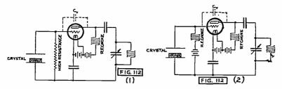
Figs. 112 (1) (2). Typical Oscillator Circuits Using Quartz Crystals.
