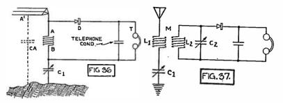
Fig. 36. Simple Crystal Detector with Telephone Condenser. Fig. 37. Simple Crystal Detector with Two Tuned Circuits.
