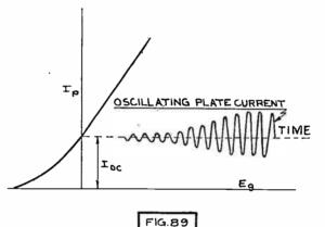
Fig. 89. Build-Up of Oscillation.
