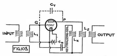
Fig. 103. Roberts Neutralization of Radio-Frequency Amplifier.
