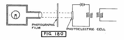
Fig. 180. Schematic Diagram Showing Manner of Producing Changes in Current, Which Are Proportional to Changes in Density of a Photographic Film.
