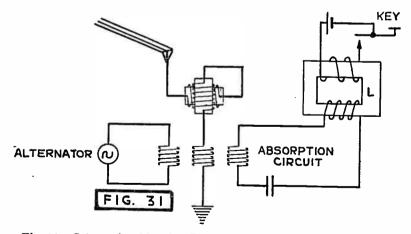
Fig. 31. Schematic of Keying System in Alexanderson Alternator.
