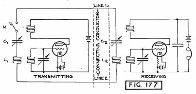
Fig. 177. Line Radio Telegraph Set.
