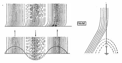
Fig. 132. Field About Vertical Receiving Antenna.
