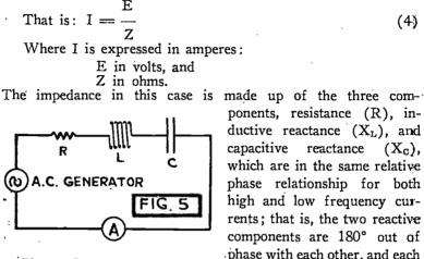
Fig. 5. Series A.C. Circuit-Fixed C, L, and R.
