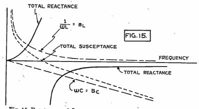
Fig. 15. Reactance and Susceptance Curves for L and C in Parallel.
