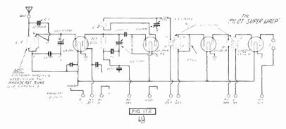
Fig. 172(1). Circuit of the "Super-Wasp" Receiver.
