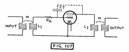
Fig. 107. Losser Method of Preventing Oscillations.
