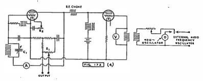
Fig. 172 (4). A Simple Microvolter.
