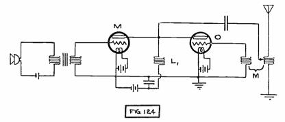
Fig. 124. Circuit for Radio Telephone Transmitter. Modulation by Absorption of Power Output of Generator Tube.
