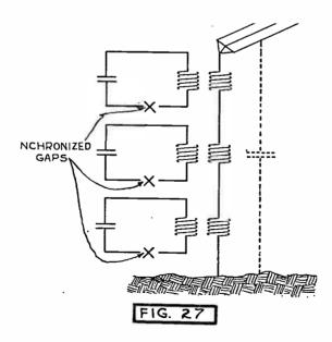
Fig. 27. Schematic of Timed Spark Set.
