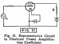
plate resistance to the alternating-current power supplied to the grid. This coefficient may be very high and in practical forms of tubes is sometimes as great as ten thousand. Of course, the alternating-current power supplied to the grid circuit is the product of the square of the grid current and the resistance of the com-
