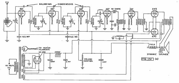
Fig. 172 (2). Schematic Diagram of a Modern All-Electric Broadcast Receiver. There Are Three Stages of R. F. Amplification, a Detector of the Grid Condenser-Grid Leak Type, and Two Stages of Audio Amplification with Two 245 Tubes in the Push-Pull Output Stage. A Dynamic Loud Speaker is Used.
