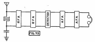
Fig. 73. Symbolical Arrangement of Amplifiers and Detector.
