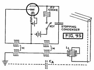
Fig. 95. One-Tube C.W. Telegraph Transmitter Employing Meisner Circuit.
