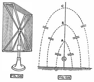
Fig. 138. Typical Loop Fig. 139. Capacity Effect of a Antenna. Single Wire Vertical Aerial.
