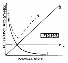
Fig. 143. Variation of the Effective Resistance of an Antenna.
