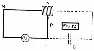
Fig. 13. Showing Effect of Dead Turns of Coil.
