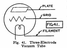
which consists of a mesh of fine wire interposed between the filament and plate and provided with an external contact. A tube of this type was first designed by DeForest, who called it the *audion*. The tube was rapidly developed by the efforts of several scientists. Such a tube is schematically
