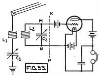
shown in Fig. 53. The portion Fig. 53. Simple "C" Bias Detector.
