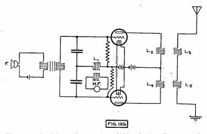
Fig. 126. Modulator System in Which Carrier Frequency is Suppressed.
