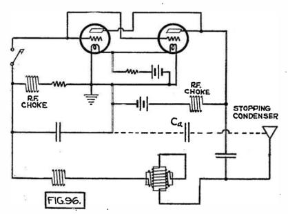
Fig. 96. C.W. Telegraph Transmitter Employing Two Parallel Tubes in a Colpitts Circuit.
