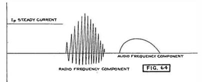
Fig. 64. Components of Plate Current.
