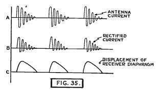
Fig. 35. Wave Forms in Circuit Fig. 34.
