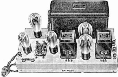
Typical Combination "B" Eliminator and Audio Amplifier Using 280 Rectifier Tube.
