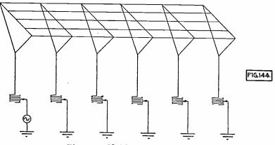
Fig. 144. Multiple-Tuned Antenna.
