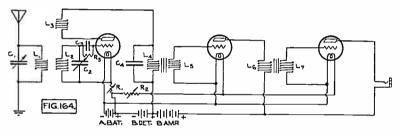
Fig. 164. Receiving Set—Regenerative Detector and Two Audio-Frequency Amplifiers.
