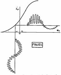
Fig. 121. Showing Principle of Modulation.
