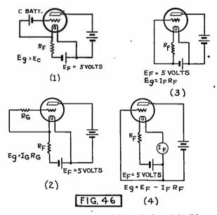
Fig. 46. Four Methods of Establishing Grid Bias.
