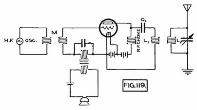
Fig. 119. Grid Modulator.
