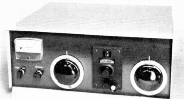
Fig. 6-5 — The universal Transmatch shown here will couple a transmitter to almost any antenna system. The meter is part of an optional built-in SWR indicator. Suitable indicators for inclusion, if the builder desires, are given in Chapter Seventeen.
