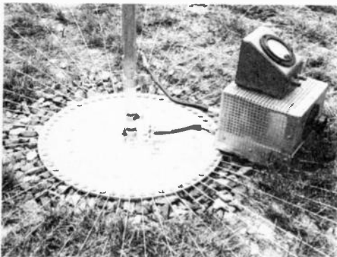
Fig. 10-7 — Base of the vertical antenna showing the 60 radials. The aluminum disk is 15 inches in diameter and 1/4-inch thick. Sixty tapped holes for 1/4-20 aluminum hex-head bolts form the outer ring and 20 form the inner ring. The insulator is polystyrene material (phenolic or Plexiglas suitable) with a one-inch diameter. Also shown is the impedance bridge used for measuring input resistance.
