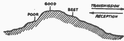
Fig. 1-7 — Propagation conditions are generally best when the antenna is located just below the top of a hill on the side that faces the distant station. Communication is poor when there is a sharp rise immediately in front of the antenna in the direction of communication.
