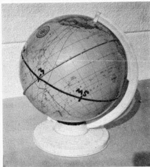
Fig. 18-4 — A simple direction finder made by modifying a globe. Bearing and distance to other locations from yours may be determined quickly after modification, no calculations being required.
