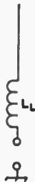
Fig. 15-3 — The capacitive reactance at frequencies lower than the resonant frequency of the whip can be canceled out by adding an equivalent inductive reactance in the form of a loading coil in series with the antenna.
