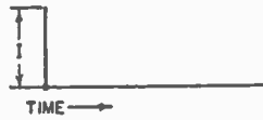
Fig. 3-3 — A current pulse traveling along a transmission line at the speed of light would reach the successive positions shown at intervals of 0.1 microsecond.
