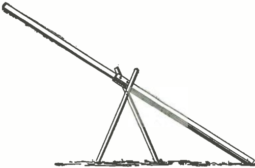
Fig. 11-13 — "Scissors" for putting up masts. As the mast goes up, the scissors are moved in to keep it from falling and to prevent sideway.
