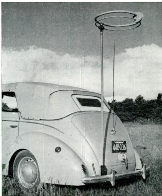
◆ Fig. 9-21 — The "halo" antenna, as used by W1MUX for nondirectional horizontal polarization in 50-Mc. mobile work. ◆
