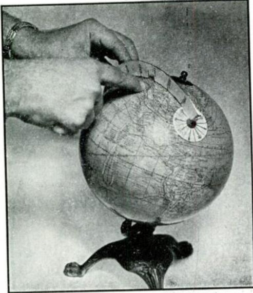
Fig. 13-4—A direction indicator made from a semicircle of thin metal can be fitted easily to a small globe. Pins at the ends permit fastening one end to the home location, the other to the antipodes. The paper scale is marked in miles to show approximate distances (12,500 miles to the semicircle).
