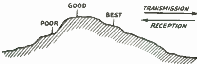
Fig. 1-6 — Propagation conditions are generally best when the antenna is located slightly below the top of a hill on the side that faces the distant station. Communication is poor when there is a sharp rise immediately in front of the antenna in the direction of communication.
