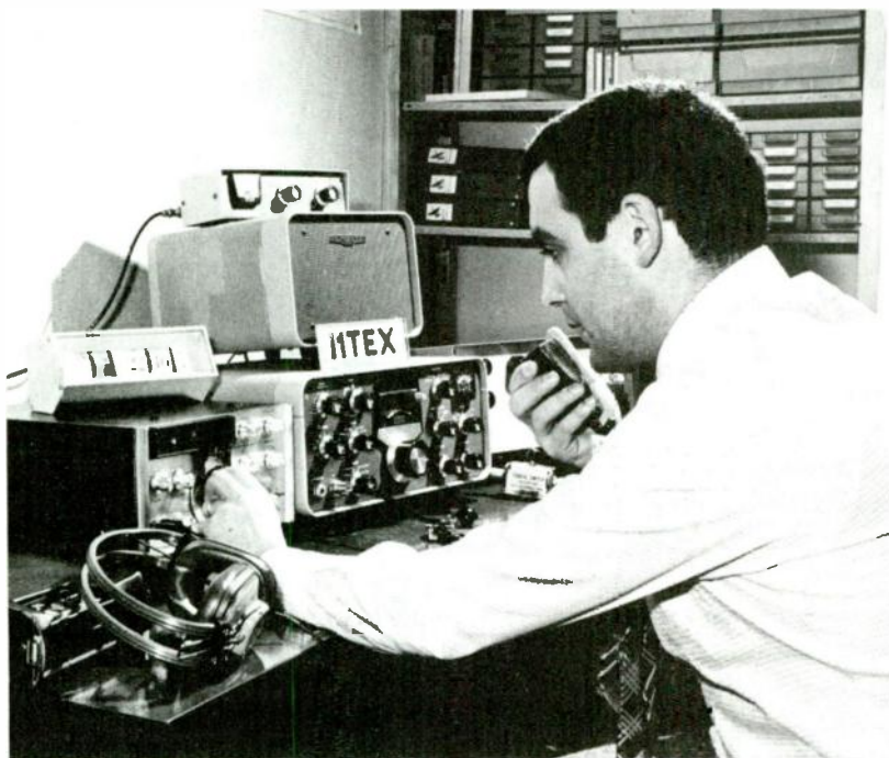
FIG. 3-3 Most hams prefer radiotelephone, or voice, communication. This mode of operation was greatly stimulated by the development of single-sideband after World War II.
