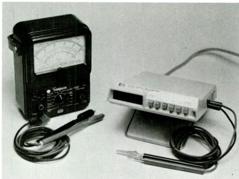
FIG. 6-17 The volt-ohm-milliammeter, or VOM, is the ham's basic test instrument.
