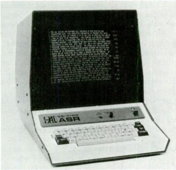
FIG. 10-1 This type of silent, easy-to-use video terminal demonstrates how well microprocessors and amateur radio go together. This microprocessor-controlled machine will send and receive three types of codes: Morse, Baudot, and ASCII.
