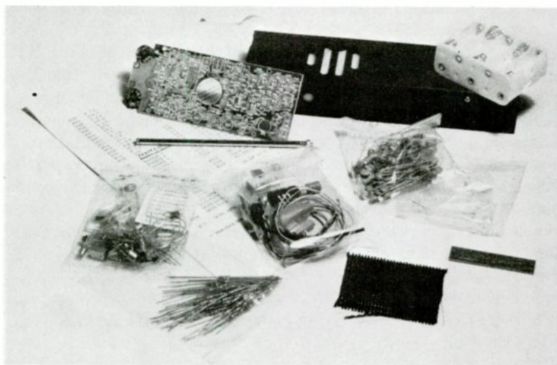
FIG. 8-7 After just a couple of weekends of building time, these components will fit into an amateur's hand as a 2-meter transceiver.
