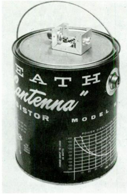
FIG. 6-16 A dummy load replaces the antenna but does not radiate a signal—use it to avoid interfering with other on-the-air contacts when making band changes and transmitter adjustments.
