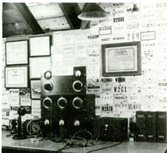
FIG. 2-2 A typical amateur station of the 1930s boasted both homemade and commercial equipment. Despite an explosion in communications technology, two elements are still in common use today—the telegraph key and the QSL cards on the wall.
