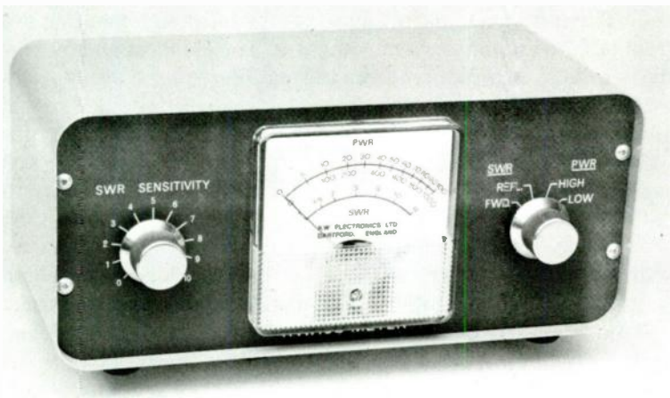
FIG. 6-14 The SWR meter is a must for keeping antenna system efficiency high.
