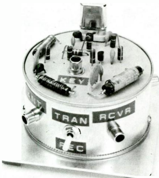
FIG. 6-3 No larger than a fist, this low-power code transmitter is entirely homemade—in a tunafish can!
