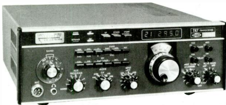
FIG. 3-6 Transceivers offer the amateur a compact unit that combines the functions of a transmitter and receiver. They are the choice of most amateurs today, in part because they are lower in cost and smaller in size than comparable separate units. The Heathkit model is a low-power, easy-to-use, and inexpensive piece of equipment, while the Drake TR7 offers convenient options such as digital readout.
