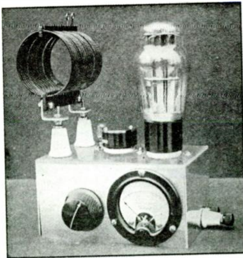
A famous transmitter design of the late '30s, the "QSL 40" was widely duplicated. The caption for this picture read: "With chassis area the same as that of a postcard, this little rig packs quite a wallop."
