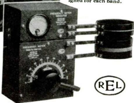
Illustrating the 3500 to 4000 K.C. frequency meter. Separate frequency meters are designed for each band.
