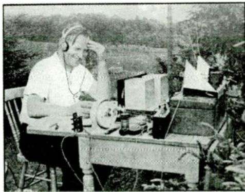
This was VE2BV operating VE2KH in the 1938 Field Day. A 6L6 ran 12 watts input from a 6-volt Genemotor, while the receiver was a t.r.f.
