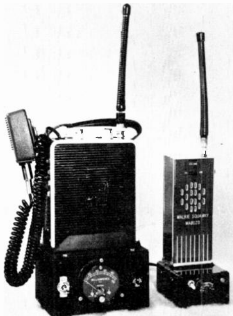
Two homemade walkie-talkies on top of their respective chargers. The batteries are left on charge continuously.
