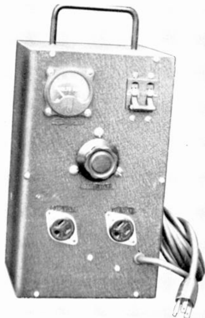
Fig. 1-15—The protected variable-voltage test unit. The double-pole circuit breaker is opposite the a.c. voltmeter. The control of the variable-voltage transformer is at the center, and the outlets for fixed and variable voltages at the bottom. This steel cabinet (Bud CU-1124) measures 12 by 7 by 6 inches, but a size should be selected to accommodate the particular components used.
