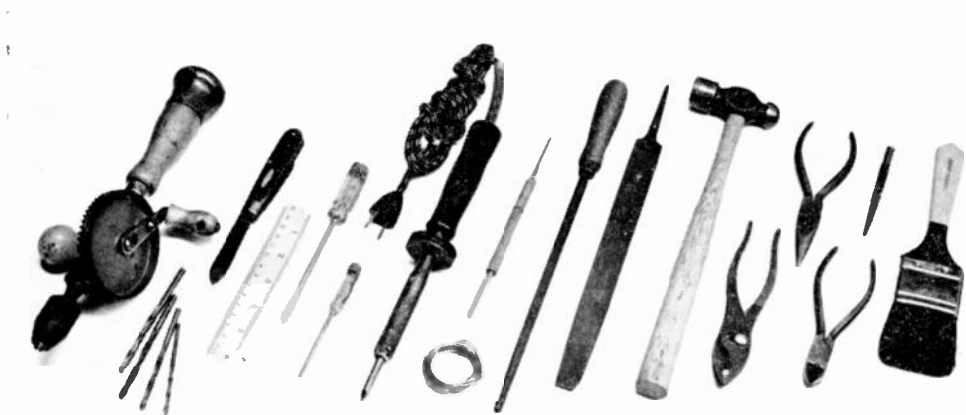
Fig. 1-7 — Representative group of the tools needed in a beginner's tool box. They include hand drill, twist drills, knife, scale, screwdrivers, soldering iron, solder, soldering aid, files, hammer, pliers, center punch and brush.
