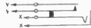
Fig. 1004 — Diagram showing connections to the filament-lighting jack. Terminals marked X go to the head-phone circuit, while those marked Y are connected in series with one side of the filament.
