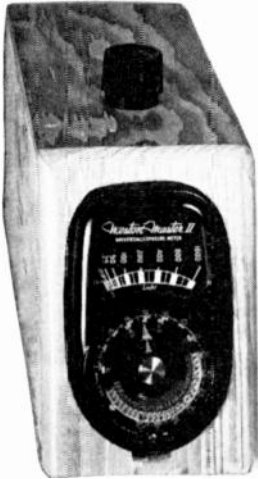
Fig. 10-14 — W5TAY's dummy antenna uses an exposure meter as a means of registering power output from his transmitter.
