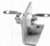
Fig. 11-23—Feedthrough insulator made from the nylon wheels of a curtain runner.
