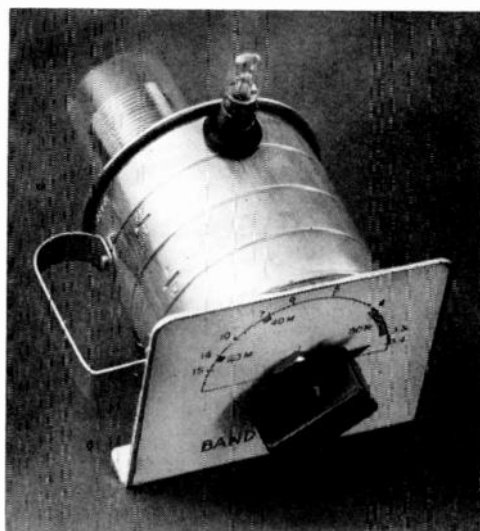
Fig. 10-4—One of the handiest "tools" in ham radio is the absorption wavemeter. This unit, built around an aluminum measuring cup, is designed to fit the requirements of the Novice licensee or old-timer. Construction is simple—the entire assembly is held together with one nut.
