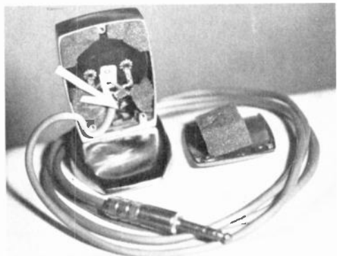
Fig. 4-11—The mercury switch is mounted at the bottom of the case, as indicated by the arrow.
