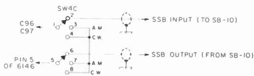
Fig. 3-4—Switch connections for Valiant modification. SW_{4c} —Centralab type RRD switch wafer.
