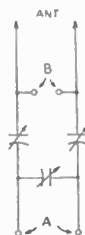
Fig. 619 — W3FEG's arrangement for feeder tuning. Series tuning is obtained with the antenna coil plugged in at A, and parallel tuning with the coil plugged in at B.
