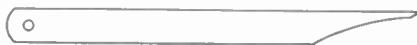
Fig. 1-5—An illustration of the unsoldering aid suggested by W7JJP. The tool is made from a hacksaw blade.
