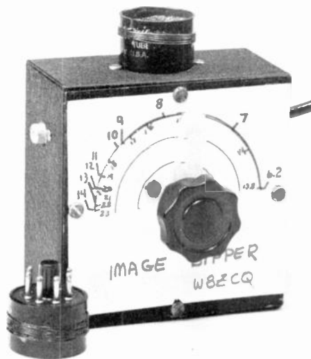
Fig. 10-25—W8ZCQ's image dipper. The cable at the right is part of a two foot length of RG-58/U that terminates in a phono plug.
