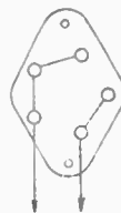
Fig. 325 — When the crystal socket is wired in this manner, correct connections will be made whether the crystal is inserted in any of the three possible ways.
