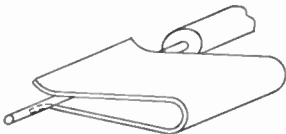
Fig. 1-13 — A copper-strip heat-dissipating clip as described in the text.
