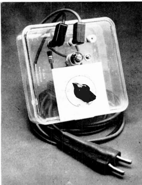
Fig. 10-13 — Top view of the neon-bulb voltmeter. The calibrated dial was mounted on a piece of cardboard and then mounted under the shaft nut of R_2 .
