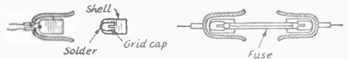
Fig. 518 — A miniature lamp socket may be used as an insulated cartridge-type fuse holder.
