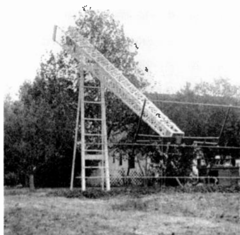
Fig. 6-10 — Antenna adjustments are made easily at the ground. Raising and lowering the antenna and mast top section take but a few minutes.
