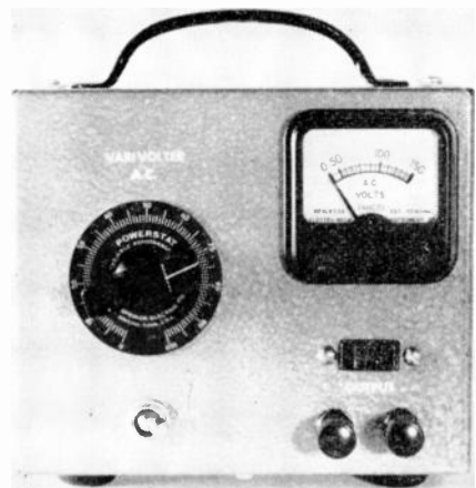
Fig. 5-16—Front view of the "A.C. Vari-volter." The bakelite binding post must be well insulated from the panel.
