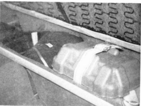
Fig. 9-4—The auxiliary 12-volt battery is mounted under the left rear seat in a plastic battery box.
