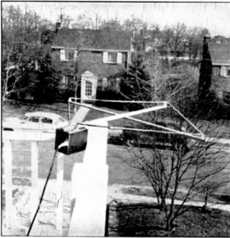
Fig. 8-3 — If you live in an apartment house or are having trouble with TVI, this compact horizontal loop for 7 Mc. may be your answer.
