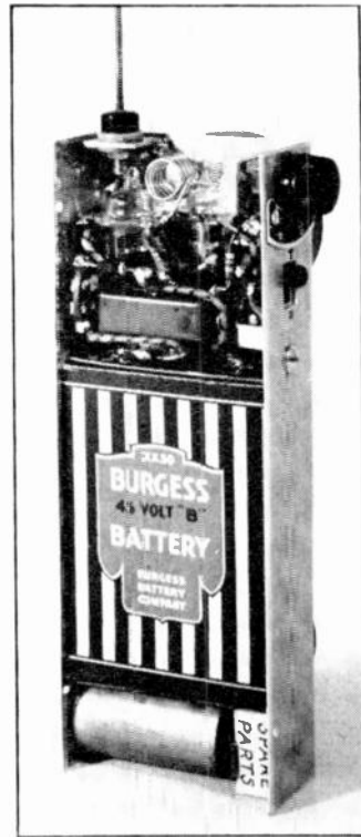
Fig. 7-13 — Inside the handie-talkie. Over half the case is occupied by the battery power supply. To save space no tube sockets are used, the connections being soldered directly to the tube pins.
