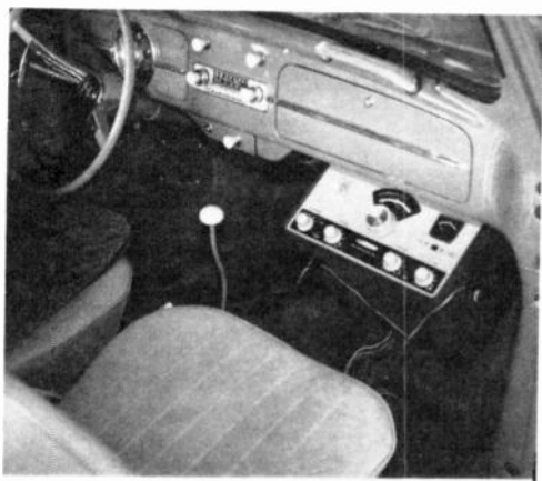
Fig. 9-3—The Heath HW-22 s.s.b. transceiver is powered by an HP-13 transistor power supply.
