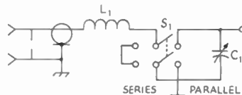
Fig. 8-3—Circuit of the antenna coupler with series-parallel tuning feature added.
