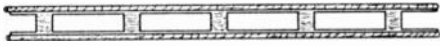
Fig. 6-3 — Method of "weatherproofing" feed lines made of Twin-Lead. Some of the dielectric is removed, leaving only enough to maintain line spacing.
