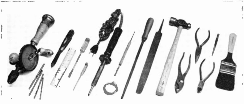
Fig. 1-30—Representative group of the tools needed in a beginner's tool box. They include hand drill, twist drills, knife scale, screwdrivers, soldering iron, solder, soldering aid, files, hammer, pliers, center punch and brush.
