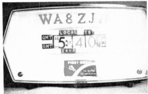
Fig. 6-2—By modifying a 12-hour digital clock as described in the text and shown above, you can read 24-hour GMT and 24-hour local time without any calculating.
