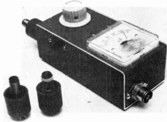
The FET Dipper has power applied. With no resonant circuit near, the meter reads 90 percent of full scale when one of the coils is plugged in. The jack J1 at the bottom feeds a portion of the oscillator signal to a frequency counter.
