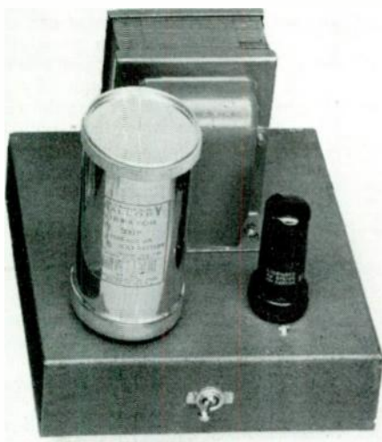
A 300-volt 100-ma. vibrator power supply.
