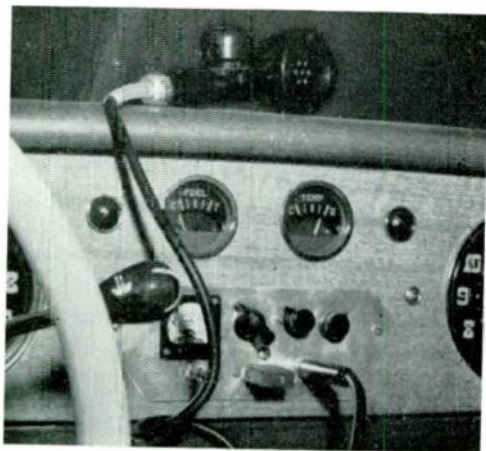
The control unit of the W7MRX 10-meter mobile rig fits neatly into the instrument panel of the author's Hudson.
