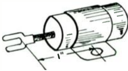
Fig. 2 — Conventional type by-pass capacitor. Because units of this type have considerable inductance, their by-passing effectiveness is poor except for a narrow range in their vicinity of 2 Mc., as shown in Fig. 3.
