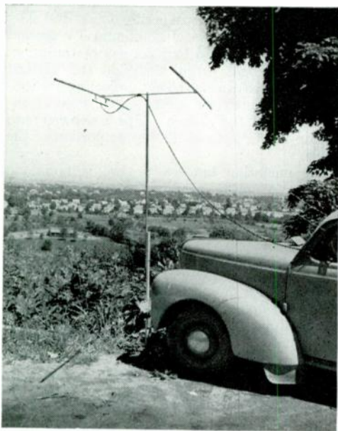
A collapsible array for 50-Mc. portable use.
