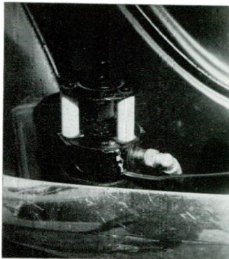
The mounting for the slider-tuned antenna is made up of standard parts and fittings.
