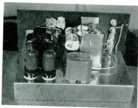
Rear view of the amplifier-modulator portion of the W7MRX mobile station. The 815 amplifier tube is mounted inside the aluminum shielding enclosure.
