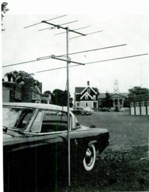
The portable 6- and 2-meter arrays ready for use. They are shown here on a 10-foot support, but another 5-foot section can be added to the mast without need for guying.
