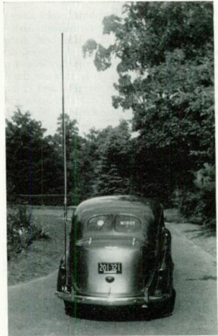
W1BDV's slider-tuned center-loaded mobile antenna for 75 meters at full extension.
