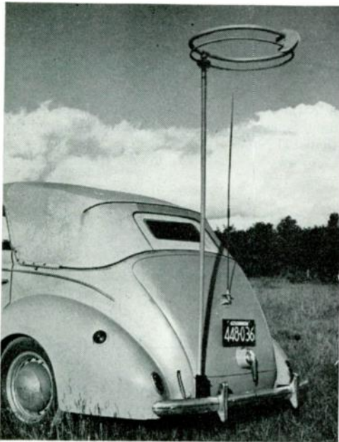
The 50-Mc. halo used by W1MUX is mounted atop a pipe mast, the base of which is bolted to a metal angle plate welded to the rear bumper.
