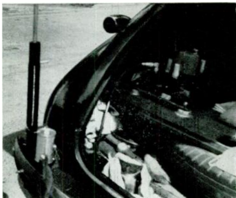
Close-up view showing the base loading coil and the enclosed tuning condenser.
