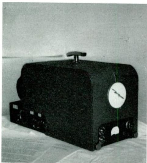
This unit contains separate r.f. sections for 80, 20 and 10 meters. It is designed for trunk mounting.
