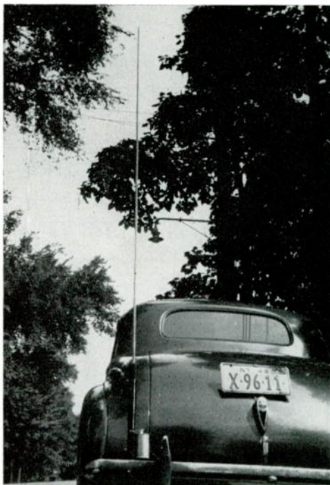
W2NNK's 75-meter mobile antenna is mounted on the rear bumper of the car.
