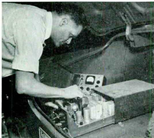
● Warren Montanye, W2WRO, servicing the mobile two-way radio of a large industrial concern, which utilizes radio for plant protection and materials handling purposes. Warren has been using his ham experience to service mobile radio systems during his spare time for many years.
