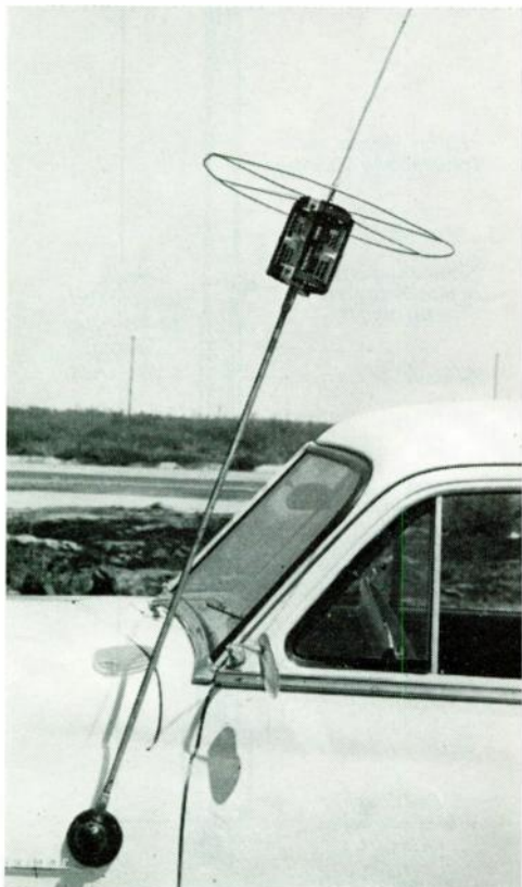
The top-loaded 4-Mc. antenna used by W6SCX. The loading coil is a B & W transmitting coil. The coil can be tuned by the variable link which is connected in series with the two halves of the coil.
