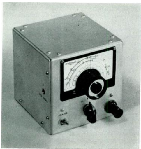
A bandswitching converter for 6, 10 and 11 meters. The pilot light at the lower right has an adjustable beam, for convenience in mobile work.
