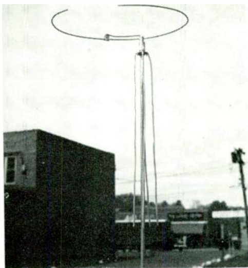
Horizontal dipole for mobile work. A 38-inch brass rod, fed with a gamma match, is bent into a circle of about one-foot diameter. It is attached to the same assembly as is used for the coaxial dipole. Matching tap and variable capacitor are about 4 inches from the center.
