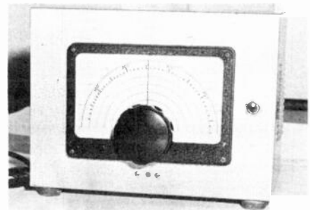
The external VFO for the SB-100 transceiver. The case is 6-1/2 x 5-1/2 x 9 inches (165 x 140 x 229 mm). Below the frequency-control knob is a small screwdriver-adjust capacitor for calibrating the VFO.
