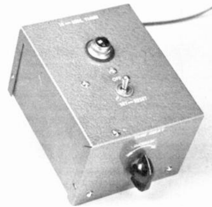
A 3 x 4 x 5-inch (76 x 102 x 127-mm) Minibox houses the components of the 10-minute timer. Once the Time Delay control has been properly set, the indicator light on the top of the unit will begin to glow 10 minutes after the toggle switch next to the lamp has been thrown to Set-Reset.
