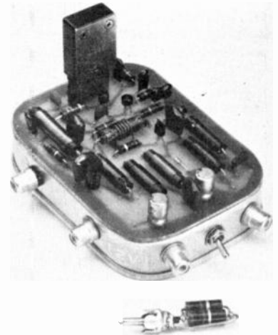
The Sardine Sender, sequel to the Tuna-Tin 2, 40-meter transmitter. The sardine-can chassis is optional. Note that the key jack is insulated from the chassis by a piece of phenolic or plastic on each side of the metal chassis.
