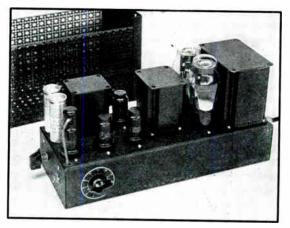
FIG. 1010 — TEN-WATT SPEECH-AMPLIFIER OR DRIVER FOR USE WITH EITHER CRYSTAL OR DOUBLE-BUTTON CARBON MICROPHONES
