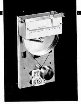
Front view shows dial scale and drive assembly. Note trimmer has only two adjustments.
