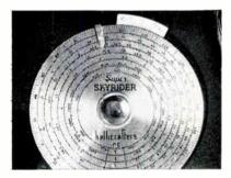
The Super Skyrider 6 Band Directly Calibrated Dial, characteristic of all Hallicrafters receivers.
