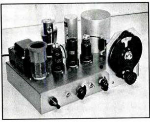
FIG. 1614 — THIS UNIT WILL GENERATE SIGNALS FOR FRE-QUENCY CHECKING AT INTERVALS OF 10 KC. AT ANY POINT IN THE HIGH-FREQUENCY SPECTRUM
