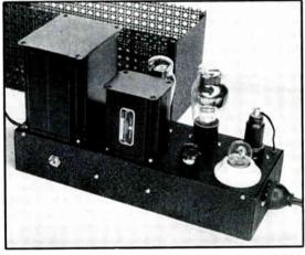
FIG. 1013 — POWER-SUPPLY FOR THE 10-WATT AMPLI-FIFR
