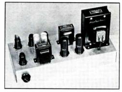
FIG. 1024 — METAL-TUBE SPEECH UNIT WITH PUSH-PULL 6L6 OUTPUT
