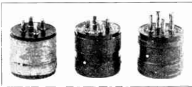
PLUG-IN RECEIVER COILS BUILT ON TUBE BASES
