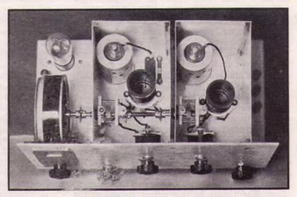
FIG. 517 - PLAN VIEW OF THE THREE-TUBE AUTODYNE WITH SHIELD COVER REMOVED
