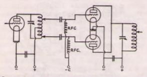
FIG. 718 — A CIRCUIT DESIGNED ESPECIALLY FOR FREQUENCY DOUBLING
