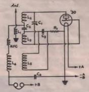
FIG. 909 - THE CIRCUIT OF THE MIDGET RECEIVER
