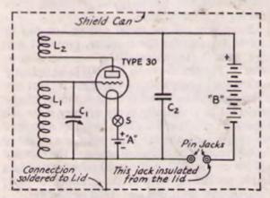
FIG. 602 - WIRING DIAGRAM OF THE MONITOR
