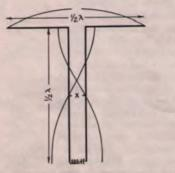
FIG. 1215 - CURRENT-FED ANTENNA WITH TUNED FEEDERS
