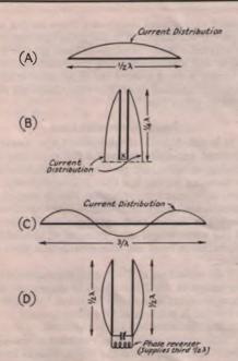
FIG. 1210 — CURRENT DISTRIBUTION ON TUNED FEEDERS Tuned feeders can be considered simply to be an antenne folded so that the fields about the wires oppose each other, thus cancelling the radiation.
