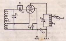
FIG. 711 — ESSENTIALS OF THE ELECTRON-COUPLED OSCILLATOR CIRCUIT
