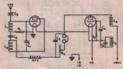
FIG. 907 - THE WIRING OF THE TWO-TUBE 56-MC. RECEIVER
