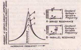
FIG.402 — CHARACTERISTICS OF SERIES AND PARALLEL RESONANT CIRCUITS
