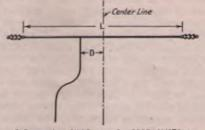
FIG. 1219 — SINGLE-WIRE FEED SYSTEM The length L and coupling D are determined from the chart
