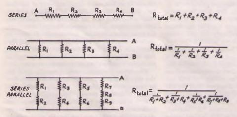
FIG. 303 - RESISTANCES CONNECTED IN SERIES, PARALLEL, AND SERIES-PARALLEL
