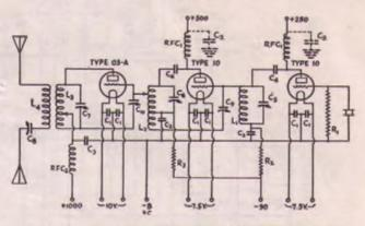
FIG. 732 - THE THREE-TUBE TRANSMITTER-CIRCUIT
