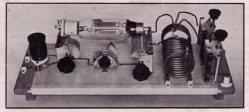
FIG. 726 — AN AMPLIFIER OF MODERATE POWER OUTPUT USING AN RK-18 TUBE Although built particularly to go with the exciter unit, it can be used with any low-power transmitter. With adequate excitation — about five watts from the driver — an output of 50 watts can be obtained at the rated tube input of 1000 volts and 85 milliamperes.
