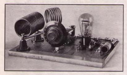
FIG. 703 — THE LOW-POWER SINGLE-TUBE TRANSMITTER The plate tank circuit is at the left. The grid coil, leak and grid condenser are to the right of the Type 10 tube. The antenna coil is shown swung away from the plate coil to give loose antenna coupling.
