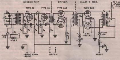
FIG. 815 - CIRCUIT OF THE SPEECH AMPLIFIER AND MODULATOR UNIT
