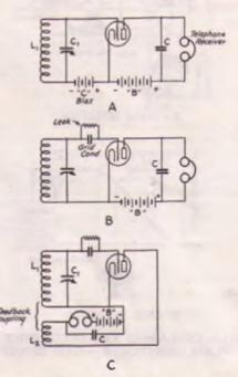
FIG. 410 — DETECTOR CIRCUITS OF THREE TYPES A — Plate detection, B — Grid detection, C — Regenerative grid detection.
