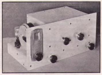
FIG. 501 — A MODERN THREE-TUBE TUNED R.F. AMATEUR-BAND RECEIVER DESCRIBED IN THIS CHAPTER
