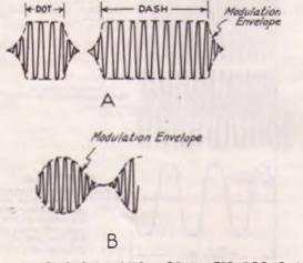
FIG. 409 - RADIO WAVES MODULATED FOR C. W. TELEGRAPHY AND TELEPHONY
