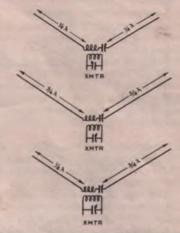
FIG. 1907 - CURRENT-FED HERTZ ANTENNAS
