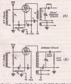
FIG. 504 - UNTUNED R. F. AMPLIFIER DIAGRAMS
