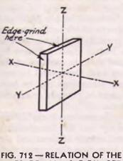
AXES OF AN X-CUT QUARTZ PLATE
