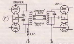
FIG. 716 - SIX WAYS OF COUPLING AN OSCILLATOR OR DRIVER TUBE TO AN AMPLIFIER
