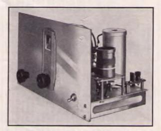
FIG. 510 — THE FRONT PANEL AND PART OF THE "CHASSIS" OF THE TWO-TUBE D.C.-A.C. RECEIVER This photograph shows the detail of the coll and antenna condenser mountings. The detector tube shield is also visible.
