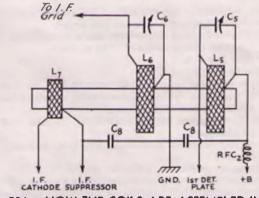
FIG. 524 -- HOW THE COILS ARE ASSEMBLED IN THE REGENERATIVE I.F. TRANSFORMER
