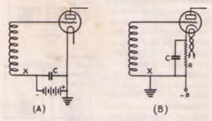
FIG. 506-BATTERY AND CATHODE-RESISTOR BIASING
