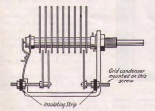
FIG. 516 - HOW THE TUNING CONDENSER IS RE-MODELLED FOR THE TWO-TUBE RECEIVER
