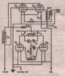
FIG. 904 — THE CIRCUIT OF THE PORTABLE TRANSMITTER ILLUSTRATED IN FIG. 905
