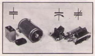
FORMS OF CONDENSERS The variable condenser symbols are interchangeable. Both are widely used.
