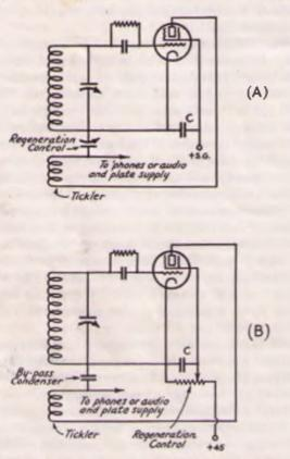
FIG. 503 - CONDENSER AND RESISTOR CONTROL OF REGENERATION
