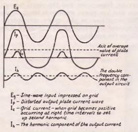
FIG. 413 — HOW DISTORTION CAUSES HARMONICS IN VACUUM TUBE OPERATION
