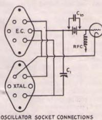
FIG. 725 - COIL AND SOCKET WIRING
