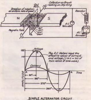
Diagram shows instantaneous volues of current and vollage with electrical degrees of cail rotation - there are soo electrical degrees for every pair of poles so that ane camplete mechanical revalution may correspond to more than one electrical revalution.
