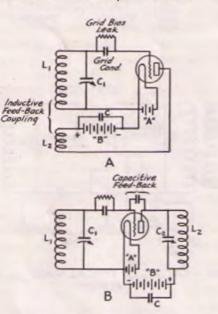
FIG. 407 — TWO GENERAL TYPES OF OSCILLATOR CIRCUITS
