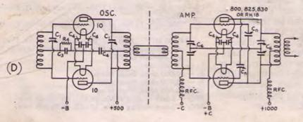
output circuit, although odd harmonics will be present to the same degree as in single-tube amplifiers of equivalent power output. Since the second harmonic is the most serious offender, however, the use of push-pull will do much to eliminate harmonic radiation. Those circuits utilizing a grounded-rotor split-stator tuning condenser — see Fig. 715-G — are more effective in eliminating harmonics than the type shown in 715-F.
