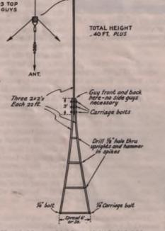
DETAILS OF A 40-FOOT MAST SUITABLE FOR ERECTION IN LOCATIONS WHERE SPACE IS LIMITED
