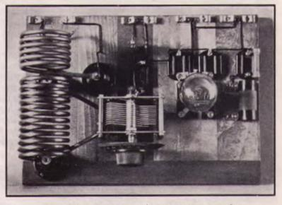
FIG. 705 - PLAN VIEW OF THE TRANSMITTER
