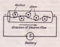
FIG. 301 — HOW CURRENT IS CONDUCTED IN A WIRE Electrons are relayed from atom to atom, from the negative to the positive end of the conductor.
