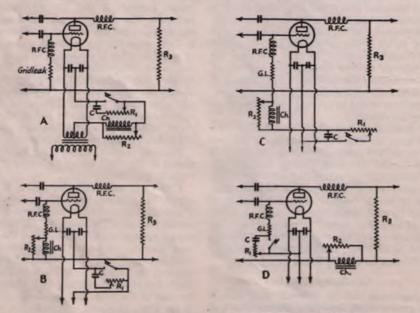
FIG. 1102 - HOW LAG CIRCUITS MAY BE ADDED TO SOME REPRESENTATIVE KEYING METHODS
