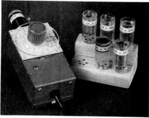
Fig. 21-20 — A compact and light-weight grid-dip meter for one-hand operation. It is built in a 1\frac{1}{8} \times 2\frac{1}{8} \times 4 -inch "Channel-lock" box and uses six plug-in coils to cover the range 1600 kc. to 160 Mc. The power supply and milliammeter for reading grid current are in a separate unit.
