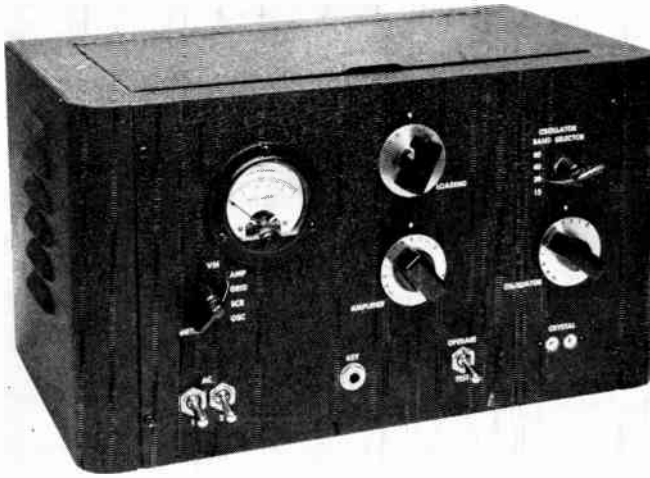
Fig. 6-47 — The complete 75-watt 6-band transmitter fits into an 8 × 11 × 8-inch cabinet. Along the bottom, from left to right, are the two power switches ( S_5 and S_6 ), the key jack ( J_7 ), the "operate-test" switch ( S_4 ) and the crystal socket. Across the center are the meter switch ( S_3 ), the amplifier tank control ( C_9 ) and the oscillator tuning condenser ( C_6 ). To the right of the meter at the top are the loading condenser ( C_{10} ) and the oscillator bandswitch ( S_2 ).
