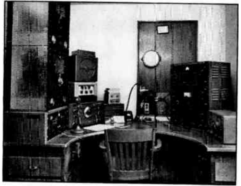
One of the most convenient station arrangements is to build a semicircular operating table as shown here. All operating controls are readily available, and considerably more equipment can be grouped around the operator than when an ordinary desk is used. (W2SAT, Riverton, N. J.)
