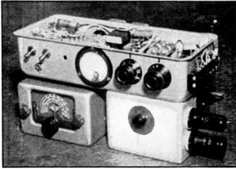
Fig. 12-16 — The crystal-filter SSB exciter, as designed for mobile work, complete with receiver converter and VFO. The top dish is the exciter (with cover removed). The meter reads cathode current to a pair of 807s driven by the unit, and the two knobs handle carrier reinserion and 6AG7 plate tuning. (W1JEO/9, Nov., 1950, QST.)
