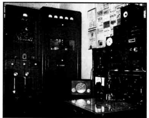
In this arrangement, the two receivers (with separate loudspeakers) and the transmitter VFO are all within easy reach of the operator, while the monitoring oscilloscope on the left-hand transmitter rack can be easily seen from the operating position. (W7JU, Boulder City, Nev.)
