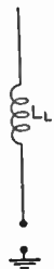
Fig. 20-36 — Placing the loading coil at the center of the whip antenna, instead of at the base, increases the radiation resistance, although a larger coil must be used.
