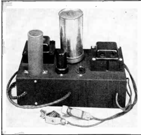
Fig. 7-34 — A typical combination a.c.-d.c. power pack for low-power emergency work. The two transformers are mounted at either end of the chassis. The filter condenser is at the left, the two rectifier sockets at the center and the vibrator to the rear.
