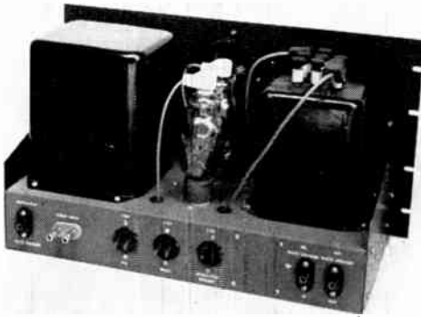
Fig. 9-29 — A typical Class B modulator arrangement. This unit uses a pair of 811As, capable of an audio power output of 340 watts, and includes a splatter filter. The modulation transformer is at the left and the splatter choke at the right. All high-voltage terminals are covered so they cannot be touched accidentally.
