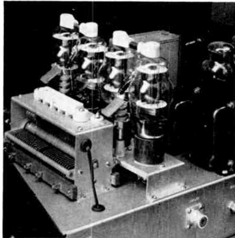
Fig. 12-19 — Close-up view of the plate circuit with the tank coil removed to show the blocking condensers, parallel-feed plate chokes and parasitic-suppressor coils. The double lead through the grommets runs from the output-circuit coil to the coupling condenser and coax connector underneath the chassis.
