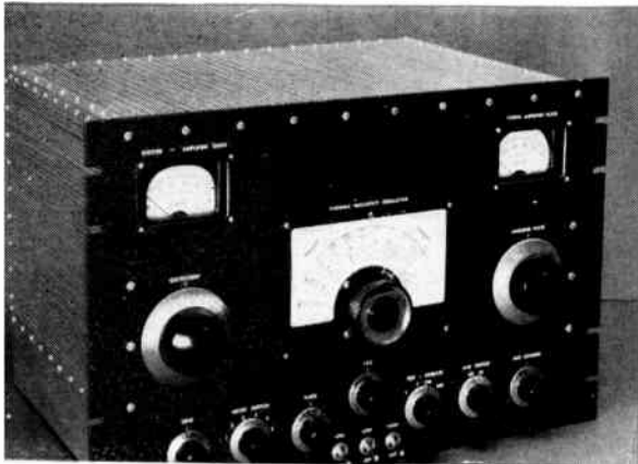
Fig. 6-61 — The standard-rack panel is 12\frac{1}{4} inches high. Controls (National HRS) along the bottom, centers spaced at intervals of 2\frac{1}{8} inches either side of center, are, left to right, for C_4 , S_3 , C_3 , C_2 , S_1 (Centralab 1405), S_2 and C_{10} . Power toggles are below at the center, spaced 1 inch apart. The calibrated VFO dial (National SCN) for C_1 is at the center, with the excitation control (National P dial) to the left, and the dial (National AV) for C_9 to the right. National CFA chart frames outline the rectangular openings for the recessed meters, 50-ma. to the left, 500-ma. to the right. The shielding enclosure is built up using aluminum angle, perforated sheet (also used for the bottom plate), and self-tapping screws.
