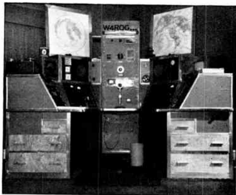
This example of a "console" shows how it is possible to find room for a receiver and multiband kilowatt transmitter (plus power supplies and modulator), together with a wide variety of accessories including a 7-inch TV receiver, tape recorder and panoramic adapter. (WARQC, Winston-Salem, N. C.)
