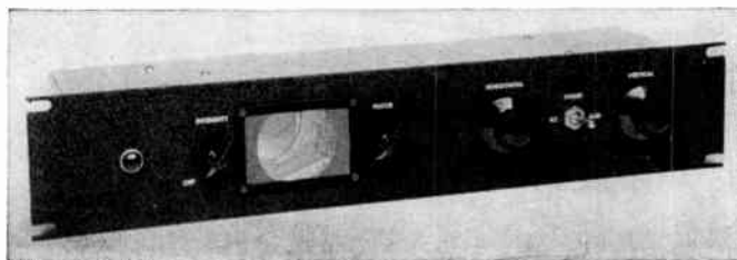
Fig. 21-48 — Two-inch oscilloscope for rack mounting. Everything needed for modulation monitoring is included except the high-voltage d.c. supply, which can be obtained from the transmitter.
