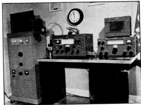
This compact station is arranged for clean-cut c.w. operation, with no frills or extras. The homemade modern-style table provides adequate operating space, a cubbyhole for log and Call Book, and drawers for QSL cards and spare parts. ( W9NN, Des Plaines, Ill. )
