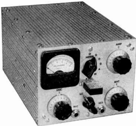
Fig. 20-16 — Front view of the 6-band mobile transmitter. The control knob for S_2 is located in between the meter and the dial for C_3 and C_4 . S_1 is directly below the crystal socket, with the knobs for C_2 and C_6 to the left and right, respectively. J_1 and J_5 are at the bottom of the 4\frac{7}{8} \times 6\frac{1}{4} -inch panel. The perforated aluminum cover is 9\frac{1}{8} inches deep and has a hole punched in the left side to permit adjustment of C_1 .
