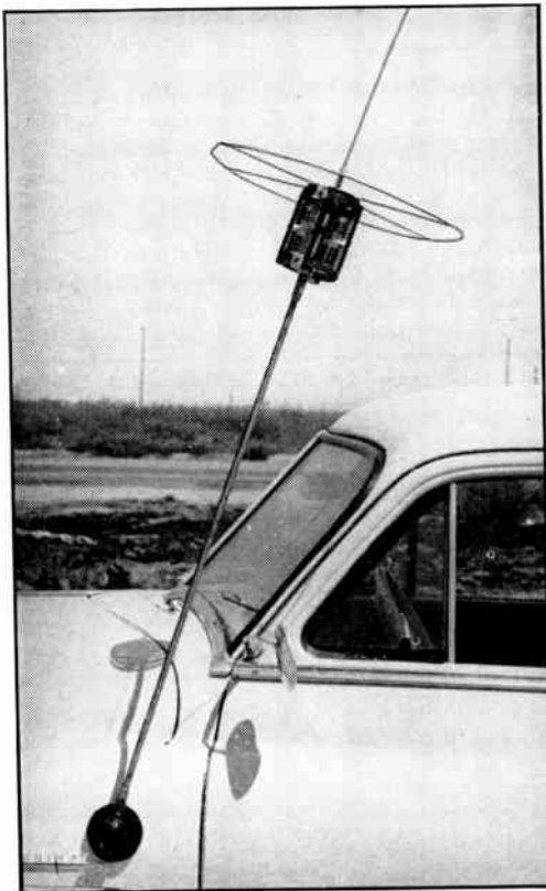
Fig. 20-37 — The top-loaded 4-Mc. antenna used by W6SCX. The loading coil is a B & W transmitting coil. The coil can be tuned by the variable link which is connected in series with the two halves of the coil.
