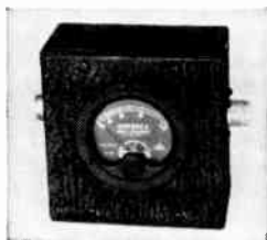
Fig. 21-28 — R.f. ammeter mounted for connecting into a coaxial line for measuring power. A "2-inch" instrument will fit into a 2 \times 4 \times 4 metal box. The shunt capacitance of an ammeter mounted in this way has a negligible effect on the accuracy at frequencies as high as 30 Mc. if the instrument has a bakelite case. Metal-cased meters should be mounted on a bakelite panel which can in turn be mounted in a cut-out which clears the meter case by about \frac{1}{4} inch.
