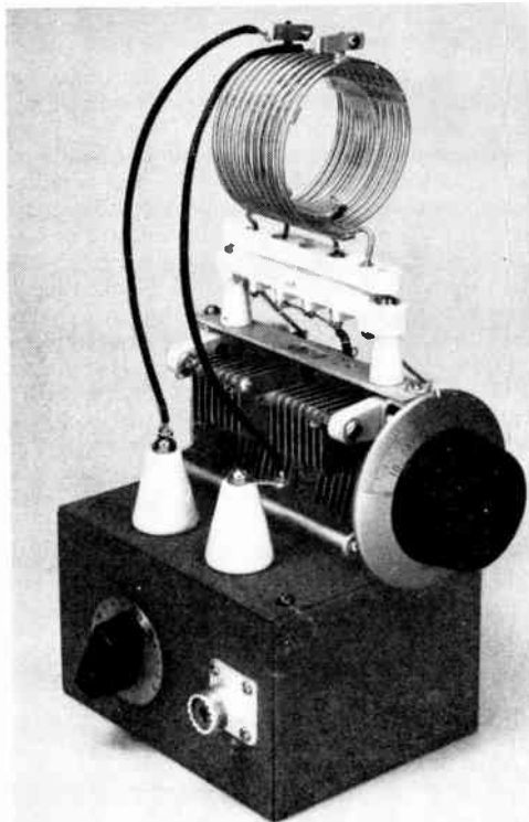
Fig. 13-31 — A coax-coupled matching circuit of simple construction. The entire circuit is mounted on a 3 by 4 by 5 box. C_1 is inside; C_2 and the plug-in coil assembly are mounted on top.
