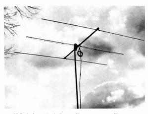
Fig. 18-7—Lightweight 3-element 50-Mc. array. Feedline is 52-ohm coax, with a balun for connection to the folded-dipole driven element. Balun may be coiled as shown or taped to supporting pipe.
