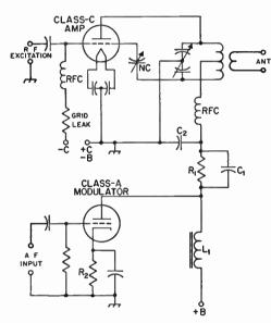
Fig. 10-8—Choke-coupled Class A modulator. The cathode resistor, R<sub>2</sub>, should have the normal value for operation of the modulator tube as a Class A power amplifier. The modulation choke, L<sub>1</sub>, should be 5 henrys or more. A value of 0.001 to 0.005 μf. is satisfactory at C<sub>2</sub>, the r.f. amplifier plate bypass capacitor. See text for discussion of C<sub>1</sub> and R<sub>1</sub>.
