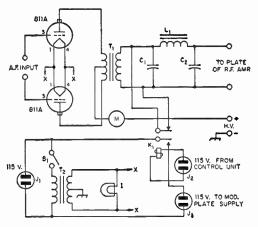
Fig. 9-27—Circuit diagram of the Class B modulator. C<sub>1</sub>, C<sub>2</sub>, L<sub>1</sub>—See text. (L<sub>1</sub> is Chicago Transformer type SR-300).
