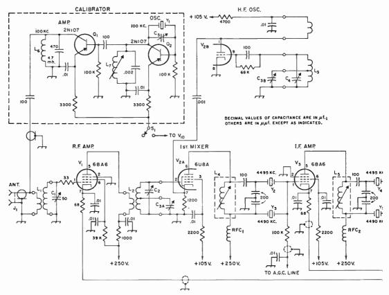
Fig. 5-52—Front-end circuit of the receiver. Unless otherwise specified, resistors are ½ watt; 0.01 and 0.02-μf. capacitors are disk ceramic, 600 volts; 0.5 capacitors are tubular paper or Mylar; capacitors below 0.01 μf. are mica; capacitors marked with polarities are electrolytic.
