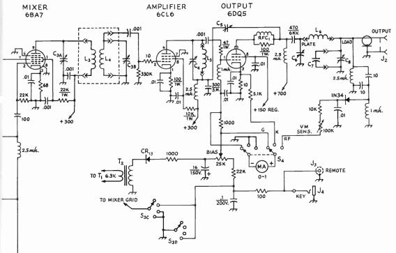
Fig. 11-7—Circuit diagram of the crystal-filter sideband generator. Unless specified otherwise, capacitances are in μμf., decimal capacitances are in μf., resistors are ½ watt, resistances are in ohms. Capacitors marked with polarity are electrolytic.
