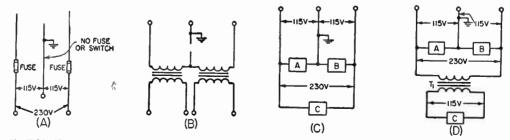
Fig. 7-30—Three-wire power-line circuits. A—Normol 3-wire-line terminotion. No fuse should be used in the gounded (neutrol) line. B—Showing that a switch in the neutral does not remove voltage from either side of the line. C—Connections for both 115- and 230-volt transformers. D—Operating a 115-volt plate transformer from the 230-volt line to avoid light blinking. I<sub>1</sub> is a 2-to-1 step-down transformer.
