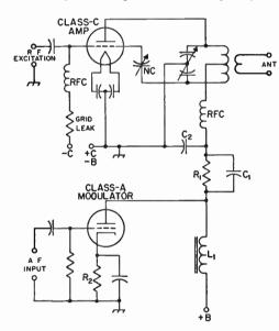
Fig. 10-8—Chake-coupled Class A modulator. The cathode resistor,  $R_{2r}$  should have the normal value far aperatian af the madulatar tube as a Class A pawer amplifier. The madulatian chake,  $L_{1r}$ , shauld be 5 henrys or mare. A value af 0.001 ta 0.005  $\mu$ f. is satisfactory at  $C_{2r}$ , the r.f. amplifier plate bypass capacitor. See text for discussion af  $C_{1r}$  and  $R_{1r}$ .
