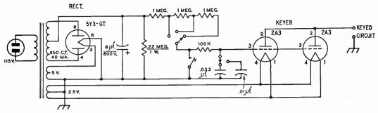
Fig. 8-6—Wiring diagram of a practical vacuum-tube keyer.
