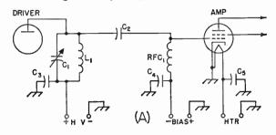
Fig. 6-21—Capacitive-coupled amplifiers.
