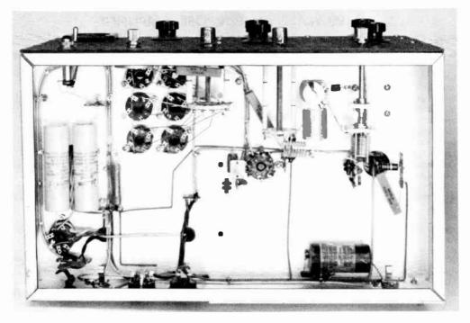
Fig. 6-47—Group of six octal sockets (upper left) serves as crystal sockets. Socket at center of chassis holds 6AG7 oscillator tube; the 3-30- $\mu\mu$ f. mica compression trimmer mounted alongside is excitation control for oscillator stage. Small midget capacitor above coil is neutralizing capacitor adjusted from above chassis; this capacitor and grid tuning capacitor to right must be insulated from chassis.
