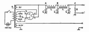
Fig. 7-13—Typical a.c. powersupply circuit for receivers, exciters, or low-power transmitters. Representative values will be found in Table 7-11. The 5-volt winding of 7<sub>1</sub> should have a current rating of at least 2 amp. for types 5Y3-GT and 5V4-GA, and 3 amp. for 5U4-GB.
