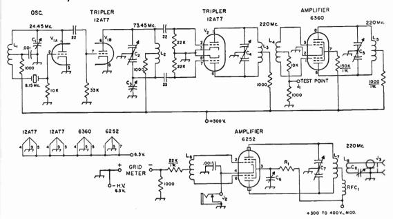
Fig. 17-31—Schematic diagram and parts information for the 220-Mc. transmitter. Capacitor values below 0.001  $\mu$ f. are in  $\mu$ uf. Resistors  $\frac{1}{2}$  watt unless specified.
