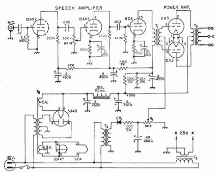
Fig. 9-8—Speech-amplifier driver for 10-15 watts output. Capacitances are in μf. Resistors are ½ watt unless specified otherwise. Capacitors with polarity indicated are electrolytic; others may be paper or ceramic. CR<sub>1</sub>—Selenium rectifier, 20 ma.
