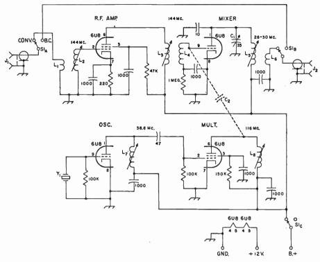
Fig. 19-13—Schematic diagram for the 144-Mc. converter. All resistors  $\frac{1}{2}$  watt unless otherwise specified. Capacitor values below 0.001  $\mu$ f. are in  $\mu\mu$ f. All 1000- $\mu\mu$ f. capacitors are disk ceramic. Other fixed capacitars are tubular ceramic.
