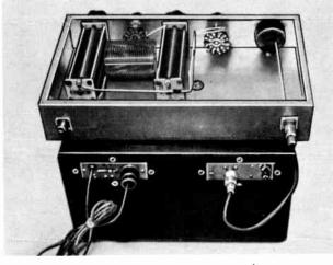
Fig. 13-20—An example of how the antenna caupler can be built. In this case the companents are installed in a 10 × 17 × 3-inch aluminum chassis that serves as the support for the transmitter. An r.f. ammeter (right) is used as an output indicator. (W4UWA/DL4, QST, Navember, 1958).
