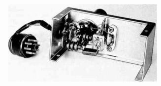
Fig. 6-90—This bottom view of the crystal oscillator shows the arrangement of components. Terminal strips are used for the cable connections and also as a support for C<sub>1</sub>, the feedback capacitor.
