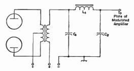
Fig. 9-13—Splatter-suppression filter for use at high level, shown here cannected between a Class B madulatar and plate-madulated r.f. amplifier. Values for  $L_1$ ,  $C_1$  and  $C_2$  are determined as described in the text.
