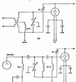
Fig. 6-25—When a pi-network output circuit is used with a triode, a balanced grid circuit must be provided for neutralizing. A—Inductive-link input. B—Capacitive input caupling.
