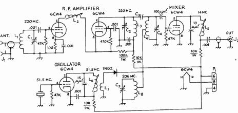
Fig. 16-14—Circuit diagram of the 220-Mc. crystal-controlled converter. Unless specified otherwise, resistors are  $\frac{1}{2}$  watt, resistances are in ohms, capacitances in  $\mu$ f.
