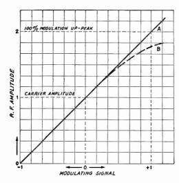
Fig. 10-4—The modulotion chorocteristic shows the relationship between the instantaneous envelope amplitude of the r.f. output (or voltage) and the instantaneous omplitude of the modulating voltage. The ideal charocteristic is a straight line, as shown by curve A.
