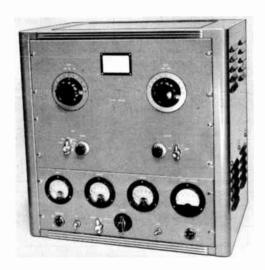
Fig. 6-77—The kilowott 4-400A omplifier ond its control unit ore mounted in a 21-inch groy hommertone rack cobinet (Bud CR-1727). Shelf brackets (Bud SA-1350) are mounted on both sides of the cobinet to hold the amplifier chassis. Below the meters, from left to right: filament pilot light, key-type a.c. switch,
