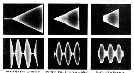
Fig. 10-21—Improper operation or design. These pictures are to the same scale as thase in Fig. 20-20, on the same transmitter and with the same test setup.
