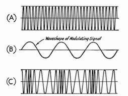
Fig. 12-1—Graphical representation of frequency modulation. In the unmodulated carrier at A, each r.f. cycle occupies the same amount of time. When the modulating signal, B, is applied, the radio frequency is increased and decreased according to the amplitude and polarity of the modulating signal.
