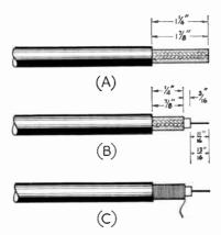
Fig. 20-3—Cable-stripping dimensions for Jones Type P-101 plugs. Smaller dimensions are for ¼-inch plugs, the larger dimensions for ½-inch plugs. As indicated in C, the remaining copper braid is wound with bare or tinned wire and then tinned, to make a snug fit in the sleeve of the plug. Hold a hot iron to the sleeve after the cable is inserted to solder
