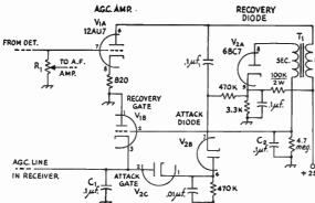
Fig. 5-18—Audio "hang" a.g.c. system. Resistors are ½ watt unless specified otherwise.
