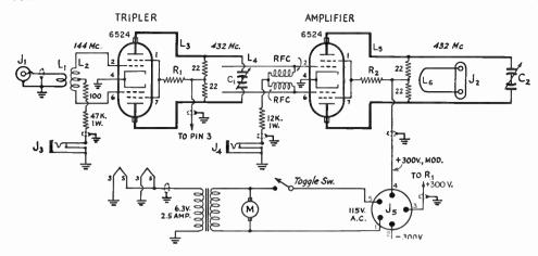
Fig. 17-36—Schematic diagram for the 432-Mc. tripler-amplifier.
