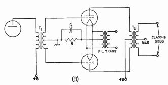
Fig. 9-7—Triode driver circuits far Class B modulators. A, resistance coupling to grids; B, transformer coupling.  $R_1$  in A is the plate resistor for the preceding stage, value determined by the type of tube and aperating canditions as given in Table 9-1.  $C_1$  and  $R_2$  are the coupling capacitor and grid resistor, respectively; values also may be taken from Table 9-1.
