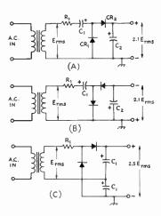
Fig. 7-28—Voltage-doubling circuits. Typical values, for  $E_{\rm rms} = 117$  and a load current of 75 ma.: C<sub>1</sub>-50-µf. 150-v. electrolytic.
