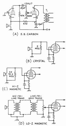
Fig. 9-1—Speech input circuits used with various types of microphones.
