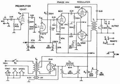
Fig. 9-15—Circuit of the speech amplifier and modulator. All capacitances are in  $\mu f$ .; capacitors with polarities marked are electrolytic, others are ceramic. Resistors are  $\frac{1}{2}$  watt except as noted below. Voltages measured to chassis with v.t. voltameter.
