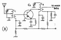
Fig. 5-27—Transistor r.f. amplifier circuit. The low-impedance connections to the base and collector can be
