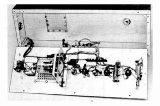
Fig. 17-32—Interior view of the 220-Mc. transmitter. All r.f. components are mounted on an aluminum plate, which is screwed to the top of a standard 6 × 17-inch chassis. Screen trimmer capacitor C₀ mounts on the tube socket mounting plate.
