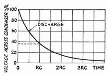
Fig. 2-20—How the voltage across a capacitor rises, with time, when charged through a resistor. The lower curve shows the way in which the voltage decreases across the capacitor terminals on discharging through the same resistor.
