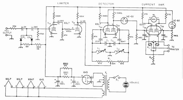
Fig. 12-12—Receiving converter far f.s.k. teletype signals (W2PAT). Unless atherwise indicated, capacitances are in μf. resistances are in ahms, resistars are ½ watt. Capacitors of 0.01 μf. ar less may be mica or ceramic; larger values may be paper. Capacitors with polarities indicated are electrolytic.
