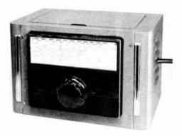
Fig. 6-58—The remote v.f.o. tuning unit is housed in a stondord metal cobinet. The cable at the right plugs into the main chassis.
