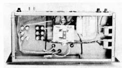
Fig. 9-28—The relay and filament transformer are mounted below the chassis. C<sub>1</sub>, C<sub>2</sub> and K<sub>1</sub> are mounted on small stand-off insulators.
