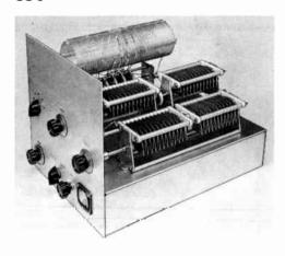
Fig. 13-21—This wide-range antenna coupler can be used with parallel-line or coaxial transmission lines, as well as with a wire af randam length. The capacitors at the center of the chassis are insulated from the chassis and from each other; the near capacitor is o normal split-statar copacitar and is mounted an the chassis. The coil of the far side is supported by its leads above the band switch.
