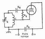
Fig. 3-23—Shawing how the plate may be grounded for r.f. in a typical ascillator circuit (Hartley).
