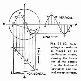
wave in the same way that it is usually represented graphically. If the period of the a.c. voltage applied to the vertical plates is considerably less than the time taken to sweep horizontally across the screen, several cycles of the vertical or "signal" voltage will appear in the pattern.
