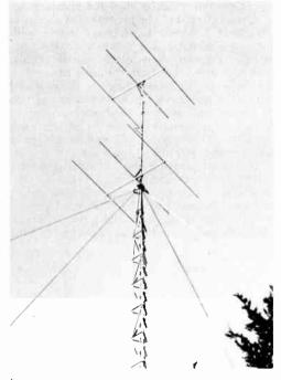
Fig. 18-13—Stacked array for 50 Mc. using two of the 3-element bays of Fig. 18-7. Phasing system and flexible section for rotation are of coaxial line. A "Q" section matches this to 450-ohm apen-wire line far run to the station.
