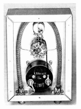
poorer the null reading. The operation of the bridge is such that when an exact null cannot be secured, the readings approximate the resistive component of the load for very low values of impedance, and approximate the total impedance at very high values of impedance. In the mid-range the approximation to either is poor, for loads having considerable reactance.
