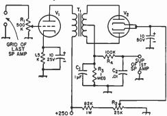
Fig. 9-11—Speech-amplifier output compression circuit.
