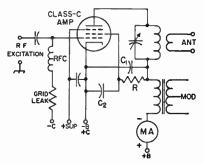
Fig. 10-6—Plate and screen modulation of a Class C r.f. amplifier using a screen-grid tube. The plate r.f. bypass capacitor,  $C_{1}$ , should have reasonably high reactance at oll audio frequencies; a value of 0.001 to 0.005  $\mu$ f. is generally satisfactory. The screen bypass,  $C_{2}$ , should not exceed 0.002  $\mu$ f. in the usual case.
