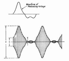
Fig. 10-2—Modulation by an unsymmetrical wave form. This drawing shows 100% downward modulation along with 300% upward modulation. There is no distortion, since the modulation envelope is an accurate reproduction of the wave form of the modulating voltage.
