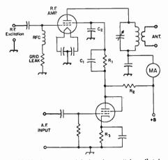
Fig. 10-11—Screen modulation by a "clomp" tube. The grid leak is the normal value for c.w. operation and  $C_2$  should be 0.002  $\mu$ f. or less. See text for discussion of  $C_1$ ,  $R_1$ ,  $R_2$  and  $R_3$ .  $R_3$  should have the proper value for Closs A operation of the modulator tube, but cannot be colculated unless triade curves for the tube are available.
