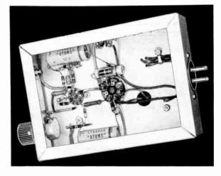
Fig. 17-29—Looking at the underside of the modulator.
