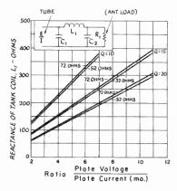
Fig. 6-14—Reactance of tank cail, L<sub>1</sub>, as a function of plate valtage and current, for pi networks.
