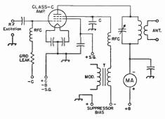
Fig. 10-13—Suppressar-grid madulation of an r.f. amplifier using a pentade-type tube. The suppressar-grid r.f. bypass capacitar, C, shauld be the same as the grid bypass capacitar in cantral-grid madulation.
