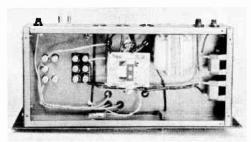
Fig. 9-28—The relay and filament transformer are mounted below the chassis. C<sub>1</sub>, C<sub>2</sub> and K<sub>1</sub> are mounted on small stand-off insulators.
