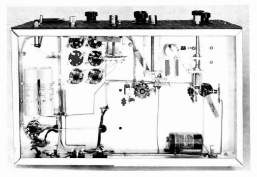
Fig. 6-47—Group of six octal sockets (upper left) serves as crystal sockets. Socket at center of chassis holds 6AG7 oscillator tube; the 3-30- $\mu\mu$ f. mica compression trimmer mounted alongside is excitation control for oscillator stage. Small midget capacitor above coil is neutralizing capacitor adjusted from above chassis; this capacitor and grid tuning capacitor to right must be insulated from chassis.
