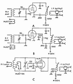
Fig. 16-5—Typical v.h.f. mixer circuits for triode (A), pentode (B) and push-push triode (C). Circuits A and B may be used with one portion of various dual-purpose tubes. Plate current of pentode (B) should be held at lowest usable value if no r.f. stage is used.
