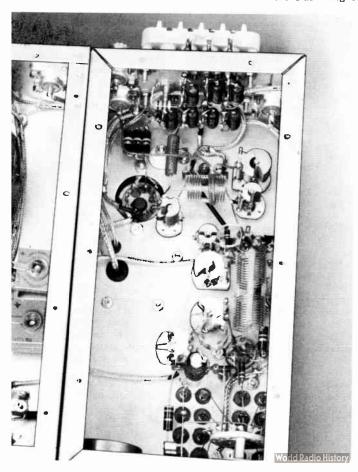
Fig. 17-5—Bottom view of the 50-Mc. exciter, showing band-pass circuits and TVI protective measures.
