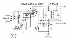
Fig. 5-11—Typical circuits for triode-hexode (A) and pentagrid (B) converters. Values for  $R_1$ ,  $R_2$  and  $R_3$  can be found in Table 5-1; others are given below.
