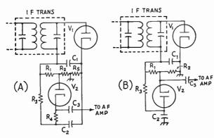
Fig. 5-21—Self-adjusting series (A) and shunt (B) noise limiters. The functions of V<sub>1</sub> and V<sub>2</sub> can be combined in one tube like the 6H6 or 6AL5.
