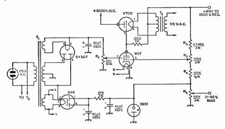
Fig. 7-22—Shunt screen regulator used by W2AZW. Resistances are in ohms (K == 1000). C<sub>1</sub>-0.01 µf., 400 volts if needed to suppress
