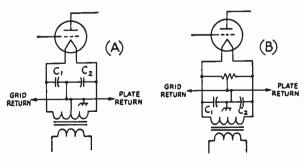
Fig. 3-18—Filoment center-topping methods for use with directly heated tubes.
