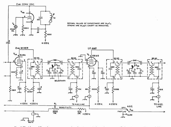
Fig. 5-53—1.f. amplifier, detector, a.g.c. and audio circuits. Unless otherwise specified, resistors are ½ watt; 0.01-and 0.02-μf. capacitors are disk ceramic, 600 volts; 0.5-μf. capacitors are tubular paper or Mylar; capacitors below 0.01 μf. are mica; capacitors marked with polarities are electrolytic.
