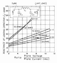
Fig. 6-15—Reactance of laading capacitor,  $C_2$ , as a function of plate voltage and current, for pi networks.
