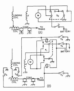
Fig. 19-37—Circuit of the remote mobile-whip tuning systems.
