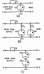
Fig. 7-24—Illustrating the use of VR tubes in stabilizing protective-bias supplies. R<sub>1</sub> is a resistor whose value is adjusted to limit the current through each VR tube to 5 ma. before amplifier excitation is applied. R and R<sub>8</sub> are current-equalizing resistors of 50 to 1000 ohms.
