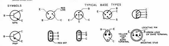
Code for identifying typical junction transistors. The leads are marked C-collector, 8-base, E-emitter and S-interlead shield and metal case.
