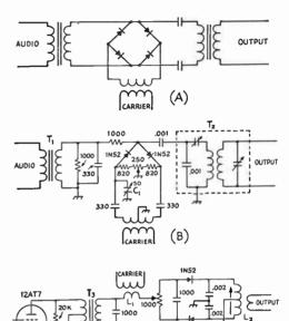
Fig. 11-1—Typical rectifier-type balanced modulators.
