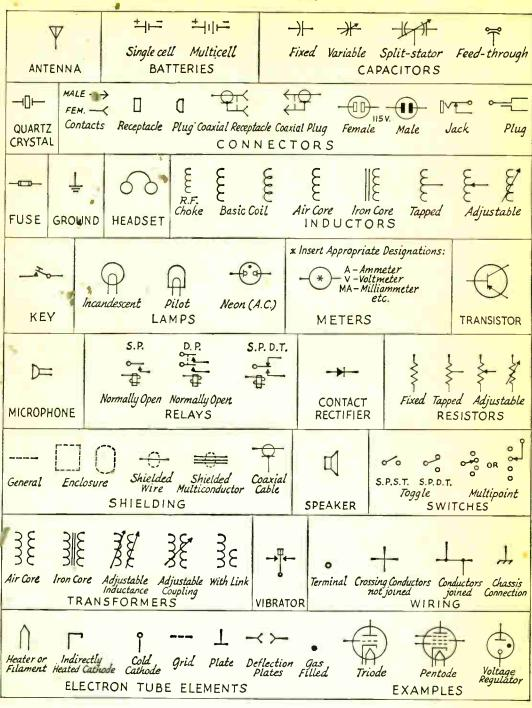
Where it is necessary or desirable to identify the electrodes or capacitors, the curved element represents the *outside* electrode (marked "outside foil," "ground," etc.) in fixed paperand ceramic-dielectric capacitors, and the *negative* electrode in electrolytic capacitors. In variable or adjustable capacitors (regardless
