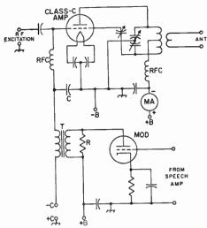
Fig. 10-14—Control-grid modulation af a Class C amplifier. The r.f. grid bypass capacitar, C, shauld have high reactance at audio frequencies (0.005  $\mu$ f. ar less).
