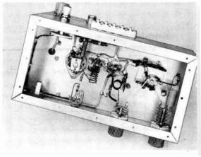
Fig. 17-23—Bottom of the 144-Mc. transmitter, with oscillator-tripler at the right. Doubler stage is near the middle of the chassis and amplifier at the left.
