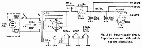
$C_{18}$ —0.25- $\mu$ f. paper, 600 volts.  $L_{10}$ —Filter choke, 10.5 henry, 110 ma. (Knight 62 G 139).  $P_1$ —Fuse plug.
