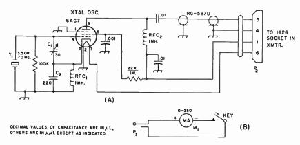
Fig. 6-89—(A) Circuit diagram of external crystal-controlled oscillator. Unless otherwise specified, resistances are in ohms, resistors are  $\frac{1}{2}$  watt. The 0.01- and 0.001- $\mu$ f. capacitors are disk ceramic. (B) Method of connecting the milliammeter in series with the key.
