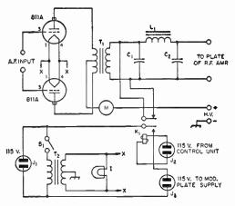
Fig. 9-27—Circuit diagram of the Class B modulator. C<sub>1</sub>, C<sub>2</sub>,  $L_1$ —See text. ( $L_1$  is Chicago Transformer type SR-300).
