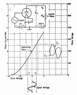
Fig. 3-8—Amplifier operation. When the plate current various in response to the signal applied to the grid, a varying voltage drop appears across the load,  $R_p$ , as shown by the dashed curve,  $E_p$ .  $I_p$  is the plate current.
