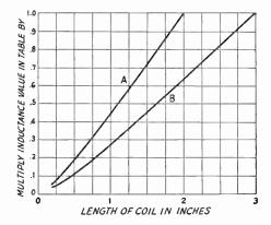
Fig. 2-15—Factor to be applied to the inductance of coils listed in the table below, as a function of coil length.
