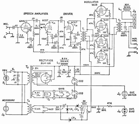
Fig. 9-21—Circuit diagram of the 50-watt modulator. Unless specified otherwise, capacitances are in μf., resistors are ½ watt.
