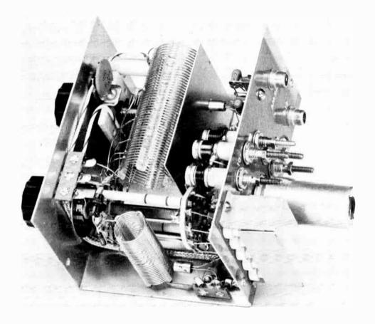
Fig. 19-9—The 12-volt hybrid crystal-controlled converter with the hausing removed. The large cail (center) is the interstage coupling coil between r.f. tube and mixer transistor. The tube and crystals plug in at the rear, and the input tuning slugs project out the rear. The antenna jack cannot be seen; it is below the tube socket.
