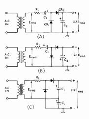
Fig. 7-28—Voltage-doubling circuits. Typical values, for  $E_{\rm rms} = 117$  and a load current of 75 ma.: C1-50-µf. 150-v. electrolytic.
