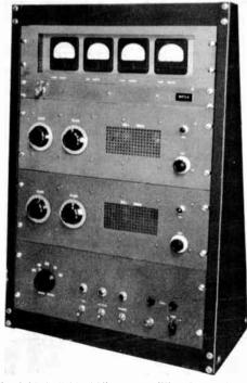
Fig. 6-64—Individual kilawatt amplifiers far twa bands plus camplete metering and all cantral circuits and pawer supplies (except plate) fit handily into a table rack. Amplifiers far five bands plus the plate supply will maunt in flaar rack. Band switch at lawer left (S<sub>B</sub> in Fig. 6-65) switches filament supply, excitation and autput cannectians ta all amplifiers in use; screen and plate supplies are cannected to all amplifiers at all times.
