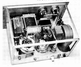
Fig. 6-75—Another view of the grounded-grid amplifier, showing the large switch used in the plate circuit. Tubes visible in the upper right are used in a regulated grid-bios supply. Metal shields on the two panel meters minimize radiation.
