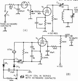
Fig. 12-14—Frequency-shift keyer circuits. Unless otherwise indicated, capacitances are in  $\mu\mu$ f., resistances are in ohms, resistors are ½ watt. A—Reactance-tube keyer far use with variable-frequency ascillator (W6OWP). B—Crystal oscillator circuit (W2PAT). It is essential that all leads associated with the crystal portion of the circuit be held to a small fraction of an inch in length if maximum shift is desired.
