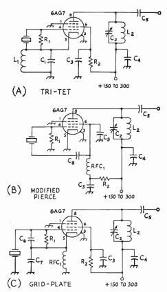
Fig. 6-3—Commonly used crystal-controlled oscillator circuits. Values are those recommended for a 6AG7 or 5763 tube. (See reference in text for other tubes.) C<sub>1</sub>—Feedback-control capacitor—3.5-Mc. crystals—approx. 220-μμt. mica—7-Mc. crystals—approx. 150-μμt. mica.
