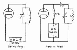
Fig. 2-57—Illustrating series and parallel feed.
