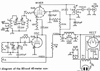
Fig. 5-40—Circuit diagram of the 80-and 40-meter converter. All capacitances given in  $\mu\mu f$ , unless otherwise noted.
