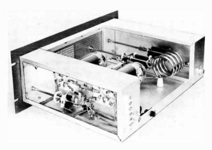
Fig. 6-68—As in the other amplifiers, the 10-meter final uses shielded wires in the filament, screen, and grid-return circuits. For tuning this amplifier uses a small variable capacitor connected across half of the plate coil, to maintain a favorable L/C ratio.
