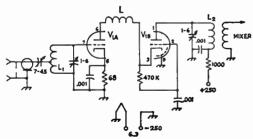
Fig. 16-3—Simplified cascade circuit far use with dual triades having separate cathodes. Cail and capacitance values nat given depend an frequency. Bifilar r.f. chakes are accasianally used in heater leads. L matches impedances between tubes and impraves averall naise figure.
