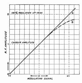
Fig. 10-4—The modulotion chorocteristic shows the relotionship between the instantaneous envelope amplitude of the r.f. output (or voltage) and the instantaneous omplitude of the modulating voltage. The ideal charocteristic is a straight line, as shown by curve A.
