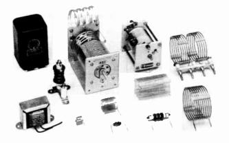
Inductors for power and radio frequencies. The two iron-core coils at the left are "chokes" for power-supply filters. The mounted air-core coils at the top center are adjustable inductors for transmitting tank circuits. The "pie-wound" coils at the left and in the foreground are radio-frequency choke coils. The remaining coils are typical of inductors used in r.f. tuned circuits, the larger sizes being used principally for transmit-
