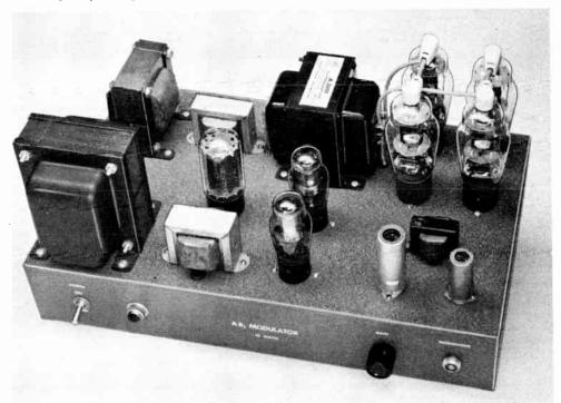
Fig. 9-20—A 50-watt modulator, using four 1625-type tubes in Class AB<sub>1</sub>. With higher plate voltage and a larger modulation transformer, the tubes can deliver up to 140 watts of audio power.
