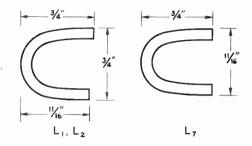
Fig. 16-27—Details of "coils" L<sub>1</sub>, L<sub>2</sub> and L<sub>7</sub>. Material is No. 10 tinned copper wire. Taps on L<sub>1</sub> and L<sub>2</sub> are ½ up from ground end; taps on L<sub>7</sub> are ½ and ½ up from ground end.
