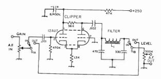
Fig. 9-12—Practical speech clipper circuit with law-pass filter. Capacitances belaw 0.001  $\mu$ f. are in  $\mu\mu$ f. Resistars are ½ watt. L<sub>1</sub>—20 henrys, 900 ohms (Stancar C-1515). S<sub>1</sub>—D.p.d.t. taggle ar ratary.
