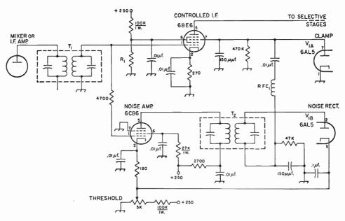
Fig. 5-22—Practical circuit diagram of an i.f. noise silencer. For best results the silencer should be used ahead of the high-selectivity portion of the receiver. T<sub>2</sub>—Interstage i.f. transformer
