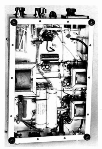
Fig. 6-51-Bottom view of the all-purpose amplifier. The 150-ma, filter choke is mounted on the left-hand wall; the smaller filter choke, the small filament transformer (Ta in Fig. 6-50) and the selenium rectifier are mounted on the righthand wall. The strap of aluminum, visible below the meter at the top right, provides additional support for the length of RG-58/U cable that runs to the output coaxial connector. All power leads except the high voltage to the plate are run in shielded wire.
