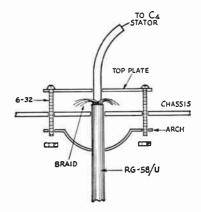
Fig. 6-53—Exploded view of the cable clamp used to hold the coaxial cable running to  $J_2$ . The top plate is a  $1\frac{1}{2}$ -inch square of sheet aluminum with holes at the four corners for 6-32 screws. The arch is a  $\frac{1}{2}$ 6-inch wire strap that mounts diagonally under the chassis. When tightened, the top plate clamps the cable braid to the chassis; the arch lends support to the cable.
