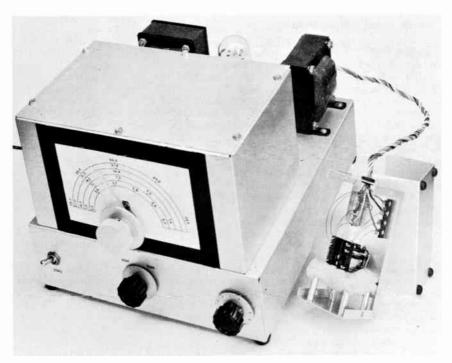
Fig. 6-83—The two-band v.f.o. provides suitable output to drive a former crystal-oscillator stage on 80 or 40 meters. A differential-keying circuit is included that requires no modification of the transmitter following the v.f.o.
