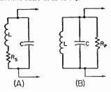
Fig. 2-41—Series and parallel equivalents when the twa circuits are resanant. The series resistar,  $R_{\rm e}$ , in A can be replaced by an equivalent parallel resistar,  $R_{\rm p}$ , in B and vice versa.
