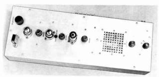
Fig. 17-30—Top view of the 220-Mc. transmitter. Final amplifier tube is inside the chassis, below the screened ventilation hole. Power connections, keying jack and output terminal are on the back of the chassis.
