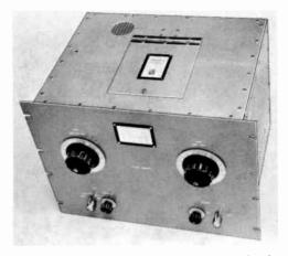
Fig. 6-79—This view of the amplifier shows the bandswitch trap daar, air-exhaust part and hale far adjusting neutralization, all in the tap of the shielding enclasure. The large knab an the left of the panel is for the 20/15/10-meter plate tuning capacitor, and the matching knob adjusts the capacitar used an 80 and 40. Farther down, fram left to right: grid band switch, grid tuning control, variable loading adjustment and loading switch.
