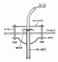
Fig. 6-53—Exploded view of the cable clamp used to hold the coaxial cable running to  $J_2$ . The top plate is a  $1\frac{1}{2}$ -inch square of sheet aluminum with holes at the four corners for 6-32 screws. The arch is a  $\frac{1}{16}$ -inch wire strap that mounts diagonally under the chassis. When tightened, the top plate clamps the cable braid to the chassis; the arch lends support to the cable.
