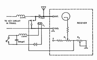
Fig. 8-9—Wiring diagram for smooth break-in operation. The lead shown as a heavy line and the lead from bottom relay contact to ANT post on receiver should be kept as short as possible for minimum pickup of transmitter signal. R<sub>1</sub>—Receiver manual gain control.
