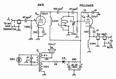
Fig. 8-17—Circuit diagram of the electronic t.r. switch. Unless otherwise specified, resistances are in ohms, resistors are  $\frac{1}{2}$  watt, capacitances are in  $\mu$ f.
