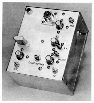
Fig. 16-13—The 220-Mc. converter uses four 6CW4 tubes and a semi-conductor frequency quadrupler.
