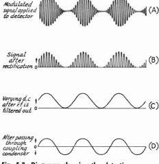
Fig. 5-3—Diagrams showing the detection process.
