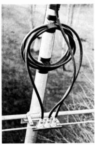
of phenolic that is supported below the driven element by three aluminum straps. The two T rods are also supported by the phenolic sheet at the inner ends and by suitable straps at the outer ends where they make up to the driven element.
