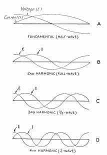
Fig. 14-14—Standing-wave current and voltage distribution along an antenna when it is operated at various harmonics of its fundamental resonant frequency.
