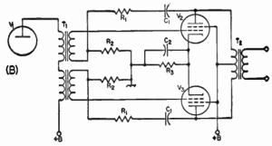
Fig. 9-9—Negative-feedback circuits for drivers for Class B modulators. A-Single-ended beam-tetrode driver. If V1 and V2 are a 615 and 6V6, respectively, or one section of a 6CG7 and a 6AQ5, the following values are suggested: R<sub>1</sub>, 47,000 ohms; R<sub>2</sub>, 0.47 megohm; R<sub>8</sub>, 250 ohms; R<sub>4</sub>, R<sub>5</sub>, 22,000 ohms; C<sub>1</sub>, 0.01 μf.; C2, 50 μf.
