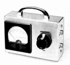
Fig. 19-41-A front view of the field-strength meter. Sensitivity control R<sub>1</sub> is to the right of the 0-1 indicating meter. Antenna input and ouput connectors are mounted on the right end of the box.
