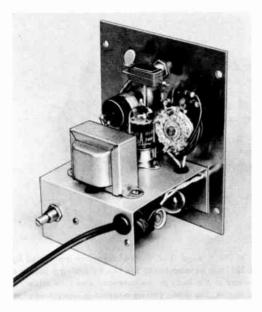
Fig. 21-22—Inside view of the audio oscillator. The a.c. switch,  $S_3$ , is mounted on the output control at the left on the panel. The ceramic capacitors in the frequency-determining circuits are mounted on the rotary switch,  $S_1$ , at the right.  $S_2$  is above the tube, and  $T_1$  is on the near edge of the chassis, which is a U-shaped piece of aluminum  $3\frac{1}{2}$  inches deep with  $1\frac{1}{2}$  inch lips.  $R_1$  is mounted on the near lip at the left,
