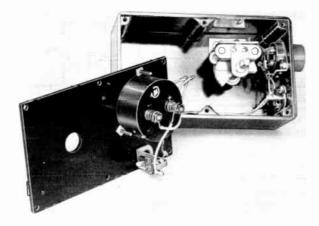
Fig. 21-12—Inside the wavemeter. Only the milliammeter and phone jack are mounted on the removable panel. The tuning capacitor is mounted vertically on an aluminum bracket fastened to the bottom of the case. The crystal diode is mounted between a coil-socket prong and a tie point. The phono lack for the pick-up cables is of the lower right.
