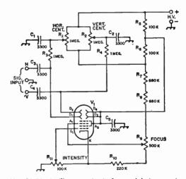
Fig. 21-54—Oscilloscope circuit for modulation monitoring. Constants are for 1500- to 2500-volt h.v. supply. For 1000-1500 volts, omit R<sub>8</sub> and connect the bottom end of R<sub>7</sub> to the top end of R<sub>9</sub>.
