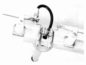
bearing point against the top of the sleeve. Another ¼-inch hole was drilled through the mast about three feet above the bottom wall mount. A piece of ¼-inch metal rod, six inches long, was forced through the hole so that the rod projected on each side of the mast. To turn the mast, a piece of rope was attached to each end
