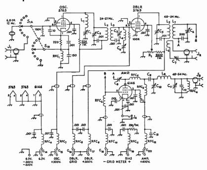
Fig. 17-4—Schematic diagram of 48–54-Mc. exciter. All capacitances less than .001  $\mu$ f. are in  $\mu\mu$ f. All .001- $\mu$ f. capacitors are disk ceramic. All resistors are  $\frac{1}{2}$ 2 watt unless otherwise specified.
