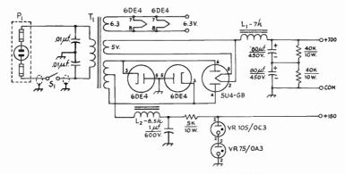
Fig. 6-52—Power supply section of the all-purpose amplifier.
