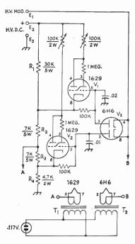
Fig. 10-24—Circuit diagram of the modulation manitar. Unless specified atherwise, resistars are  $\frac{1}{2}$  watt, resistances are in ahms, capacitances are in  $\mu f$ .
