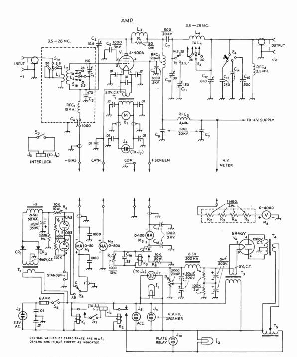
Fig. 6-78—Circuit diagram of the 4-400A amplifier (above the dashed line) and power supply/control unit.
