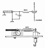
Fig. 23-12—Additional lead filtering for harmonics or ather spurious frequencies in the high v.h.f. TV band (174-216 Mc.)
