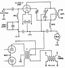
Fig. 10-15—Circuit arrangement for cathode madulation of a Class C r.f. amplifier. Values of bypass capacitors in the r.f. circuits should be the same as far other modulation methads.
