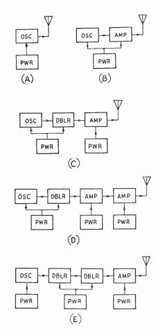
Fig. 6-1—Block diagrams showing typical cambinations of ascillatar and amplifiers and pawer-supply arrangements for transmitters. A wide selection is passible, depending upon the number of bands in which aperation is desired and the power autput.
