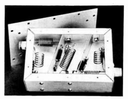
Fig. 23-21—An inexpensive low-pass filter using silvermica postage-stamp capacitors. The box is a 2 by 4 by
