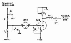
Fig. 8-10—Circuit diagram of a receiver muter for use with grid-block or tube keying.
