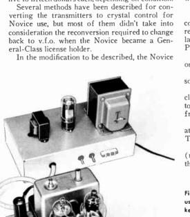
requirement for crystal control is met by using a separate crystal-controlled oscillator. The output of the external oscillator is fed into the transmitter through a plug that fits into the 1626 oscillator socket. The 1626 is not used. The transmitter modifications are such that when it is desired to restore the transmitter to v.f.o. operation the external oscillator is unplugged and the 1626 is put back in its socket. No wiring changes are needed to go from crystal control to v.f.o.
