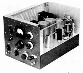
above a small CAL control knob that sets the signal level into the receiver when the function switch (left, below VXO control) is on "Calibrate." Small knob at lower left is sideband-selector switch. Switch to left of meter switches meter to grid or cathode of output tube or to r.f. voltmeter on output line; knob just below adjusts sensitivity of r.f. voltmeter.
