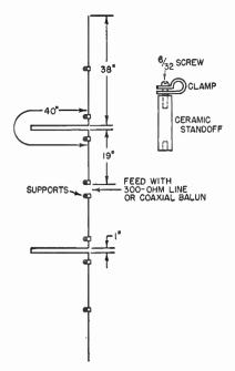
Fig. 18-4—Dimensions and supporting method for the 144-Mc. vertical array.
