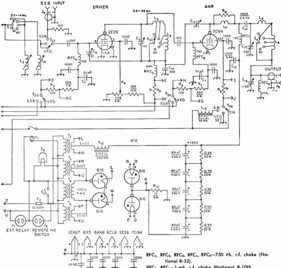
L<sub>10</sub>-7-hy. 150-ma. filter choke (Stancor C-1710). L<sub>11</sub>-15-hy. 75-ma. filter choke (Stancor C-1002).  $L_{12}$ -5/25-hy. 300-ma. swinging filter choke (Triad C-33A).
