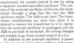
In addition to the external oscillator, a power supply is required for the oscillator and transmitter (Fig. 6-88), and certain wiring changes are needed to make the transmitter itself suitable for aniateur use. These changes consist primarily of removing two relays, changing the tube heater circuit for operation on 12 volts instead of 24 volts, and the addition of a power plug.
