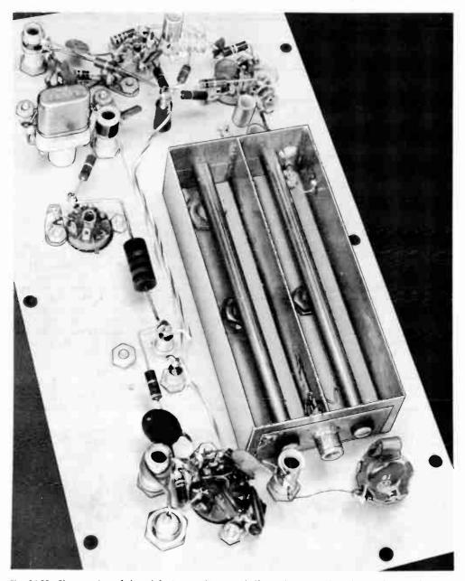
Fig. 16-32—Close-up view of the u.h.f. circuits. These are halfwave lines, tuned at their midpoints. The mixer crystal is held in place by a slotted brass sleeve, soldered to a capacitor plate on the outside of the trough. Though it is not visible in the picture, the capacitor plate is insulated from the trough end with a thin film of plastic. Screws that hold the inner conductors in position are insulated from the capacitor plate by fiber washers.
