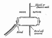
Fig. 23-13—The best method of using the "Hypass" type feed-through capacitar. Capacitances of 0.01 to 0.1 \( \mu \). Capacitars of this type are useful for high-current circuits, such as filament and 115-valt leads, as a substitute for the r.f. chake shown in Fig. 23-11, in cases where additional lead filtering is needed.
