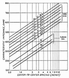
Fig. 13-8—Chart showing the characteristic impedance of spaced-conductor parallel tronsmission lines with air dielectric. Tubing sizes given ore for outside diameters.
