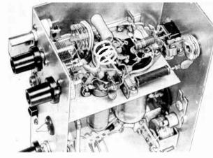
$I_1$  will light. This r.f. indicator is not only a tuning aid in the car but also acts as a continuous monitor to show that the transmitter is in operation. Capacitor  $C_4$  is the loading control and should be adjusted for maximum plate current after the amplifier is resonated.
