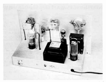
Fig. 6-37—Rear view of the transmitter showing the placement of components above chassis. The loading capacitor,  $C_8$ , is at the left,  $L_8$  is the vertical coil and  $L_2$  the horizontal one. Rubber grommets are used to prevent chafing and to furnish additional insulation on the leads coming from below chassis.
