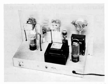
Fig. 6-37—Rear view of the transmitter showing the placement of components above chassis. The loading capacitor,  $C_8$ , is at the left,  $L_3$  is the vertical coil and  $L_2$  the horizontal one. Rubber grommets are used to prevent chafing and ta furnish additional insulation on the leads coming from below chassis.
