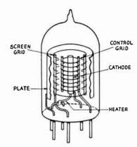
Fig. 3-16—Representative arrangement of elements in a screen-grid tetrade, with part of plate and screen cut away. This is "single-ended" construction with a button base, typical of miniature receiving tubes. To reduce capacitance between control grid and plate the leads fram these elements are brought aut at opposite sides; actual tubes prabably would have additional shielding between these leads.
