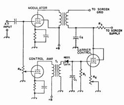
Fig. 10-12—Circuit for carrier control with screen modulation. A small triode such as the 6C4 can be used as the control amplifier and a 6Y6G is suitable as a carrier-control tube.  $T_1$  is an interstage audio transformer having a 1-to-1 or larger turns ratio.  $R_4$  is a 0.5-megohm volume control and also serves as the grid resistor for the modulator. A germanium crystal may be used as the rectifier. Other values are discussed in the text.
