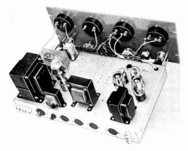
Fig. 6-80—Tap view of the cantral unit. The valtmeter multiplier resistars are haused in a cane-metal protective shield (upper left). Resistars R<sub>8</sub> and R<sub>9</sub> are maunted under the sets af ventilation hales (center near panel).
