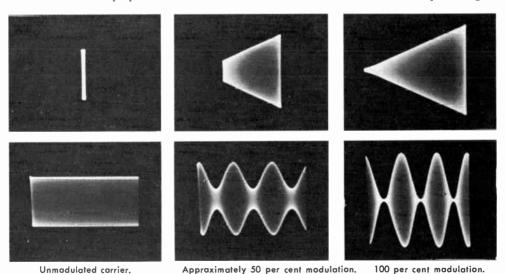
Fig. 10-20—Oscillascope patterns showing proper modulation of a plate-and-screen modulated tetrode r.f. amplifier. Upper row, trapezoidal patterns; lower row, corresponding wave-envelope patterns. In the latter a linear sweep having a frequency one-third that of the sine-wave audio modulating frequency was used, sa that three cycles of the modulation envelope show in the pattern.
