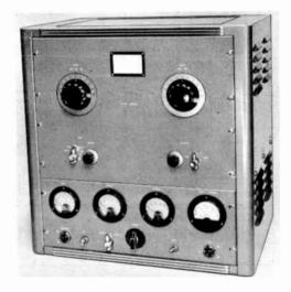
Fig. 6-77—The kilowatt 4-400A amplifier and its control unit are mounted in a 21-inch gray hammertone rack cabinet (Bud CR-1727). Shelf brackets (Bud SA-1350) are mounted on both sides of the cabinet to hold the amplifier chassis. Below the meters, from left to right: filament pilot light, key-type a.c. switch,
