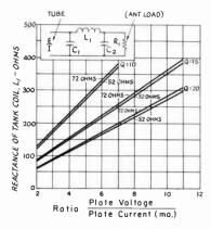
Fig. 6-14—Reactance of tank cail, L<sub>1</sub>, as a function of plate voltage and current, for pi networks.
