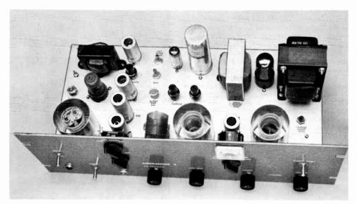
Fig. 11-10—This phosing-type single (ond double) sidebond generator features the 7360 beam-deflection tube in the balanced-modulator section. The 6CL6 output amplifier (behind meter) delivers sufficient output to drive one or more 6146 amplifier tubes in Class AB<sub>1</sub>. Plug-in coils are used to simplify construction.
