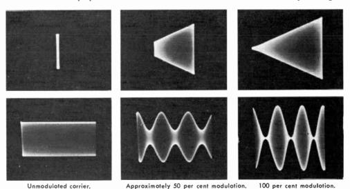
Fig. 10-20—Oscilloscope potterns showing proper modulotion of a plote-ond-screen moduloted tetrode r.f. omplifier. Upper row, tropezoidal patterns; lower row, corresponding wave-envelope potterns. In the lotter a lineor sweep hoving o frequency one-third that of the sine-wave outloo moduloting frequency was used, so that three cycles of the modulotion envelope show in the pottern.
