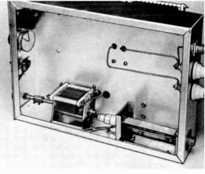
Fig. 13-23—The link capacitor and the Monimatch are mounted underneath the chassis.
