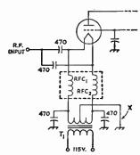
Fig. 11-17—When filament-type tubes are used in a grounded-grid circuit, it is necessary to use filament chokes to keep the filament above r.f. graund. In the portion of a typical circuit shown here, the filament chokes. RFC1 and RFC2, can be a manufactured unit (e.g., B&W FC15 and FC30) or homemade as described in the text. Total plate and grid current can be read on a milliammeter inserted at x.
