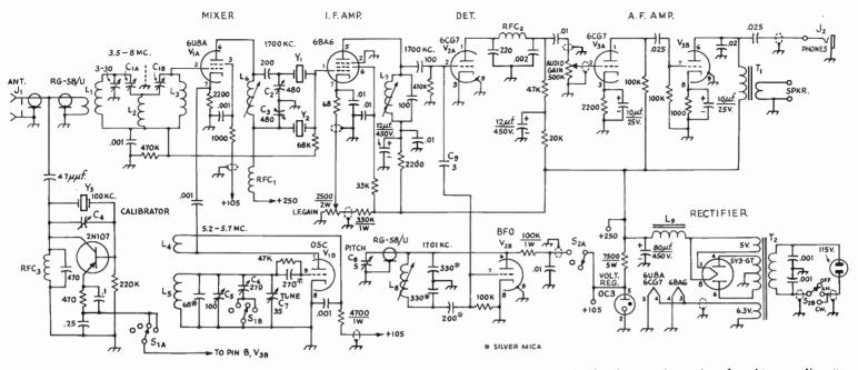
Fig. 5-36—Circuit diagram of the 2X4 + 1 super-heterodyne. Unless indicated otherwise, decimal capacitances are in μf., other capacitances in μμf., resistors are ½ watt.
