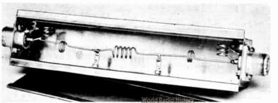
Fig. 23-26—A 52-ohm low-pass filter for 144-Mc. Transmitters. Case is made from flashing copper and is 1½ inches square by 7½ inches long. Cover slips on flanges folded out at the bottom; ends are folded down and soldered.
