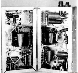
tor-to-emitter rating. The amplitudes of these spikes can be held to a safe value if the primary and secondary coils on the power transformer are tightly coupled and a large capacitor is connected across the low-voltage supply.
