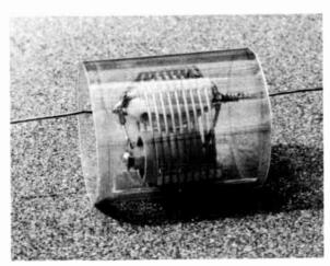
Fig. 14-25—Method of connecting the antenna wire to the strain insulator. The antenna wire is cut off close to the wrap before checking the resonant frequency of the trap.
