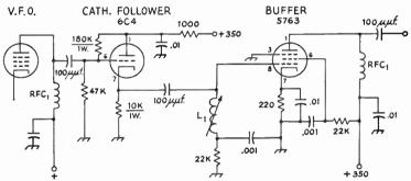
Fig. 6-6—Circuit af an isalating amplifier far use between v.f.a. and first tunable stage. Unless atherwise specified, all capacitances are in  $\mu f$ ., all resistars are  $\frac{1}{2}$  watt.  $L_1$ , for the 3.5-Mc. band, consists of 100-140  $\mu h$ . adjustable inductor. RFC<sub>1</sub> is 100  $\mu h$ . All capacitars are disk ceramic.
