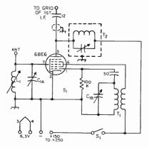
Fig. 5-62—Converter circuit for monitoring broadcast stations in connection with a communications receiver. Capacitances are in  $\mu\mu$ f.
