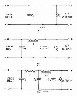
Fig. 7-4—Capacitive-input filter circuits. A—Simple capacitive. B—Single-section. C—Double-section.
