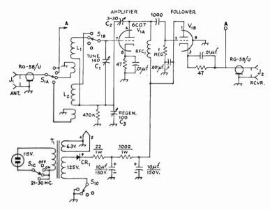
Fig. 5-50—Circuit diagram of the regenerative preselector. Unless otherwise specified, resistors are  $\frac{1}{2}$  watt, capacitors are in  $\mu\mu$ f., capacitors marked in polarity are electrolytic.
