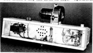
Fig. 17-37—Bottom view of the 432-Mc. transmitter.
