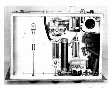
Fig. 6-76—A view under the chassis shows the filament choke between the two voriable capacitors, with the input tuning coil mounted on the input band switch. The small shield compartment at the top surrounds a filter in the B+ lead.
