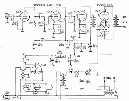
Fig. 9-8—Speech-amplifier driver for 10-15 watts output. Capacitances are in  $\mu$ f. Resistors are  $\frac{1}{2}$  watt unless specified otherwise. Capacitors with polarity indicated are electrolytic; others may be paper or ceramic. CR<sub>1</sub>—Selenium rectifier, 20 ma. Class-B tubes used; 15 watt rating.
