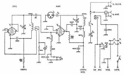
Fig. 19-23—Schematic diagram of the 50-Mc. mobile transmitter. Unless otherwise indicated, capacitances are in  $\mu\mu f$ ., resistances are in ohms, resistors are ½ watt unless specified otherwise.
