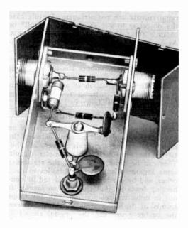
Fig. 21-40—An inexpensive bridge for matching adjustments using the circuit of Fig. 21-39. It is built in a  $1\% \times 2\% \times 4$ -inch "Channel-lock" box. The standard resistor,  $R_3$ , bridges the two coax connectors. A pin jack is provided for connection to the d.c. meter, 0-1 ma. or 0-500  $\mu$ a.; the meter negative can be connected to the case or to one of the coax fittings.
