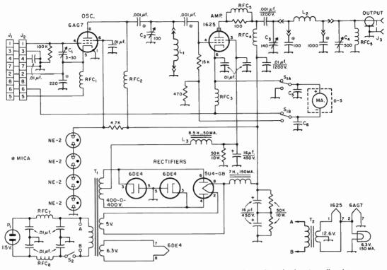
Fig 6-40—Circuit diagram of the inexpensive 75-watt transmitter. Unless indicated otherwise, all resistors are  $\frac{1}{2}$  watt, all resistances are in ohms, all capacitances are in  $\mu\mu$ f. Electrolytic capacitors are marked with polarity, mica capacitors are marked with \*, other fixed capacitors are ceramic.
