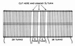
Fig. 13-24—Details of the coil assembly. Not shown are the taps needed for changing bands. The tap points listed below all are counted from the outside ends of the coil.
