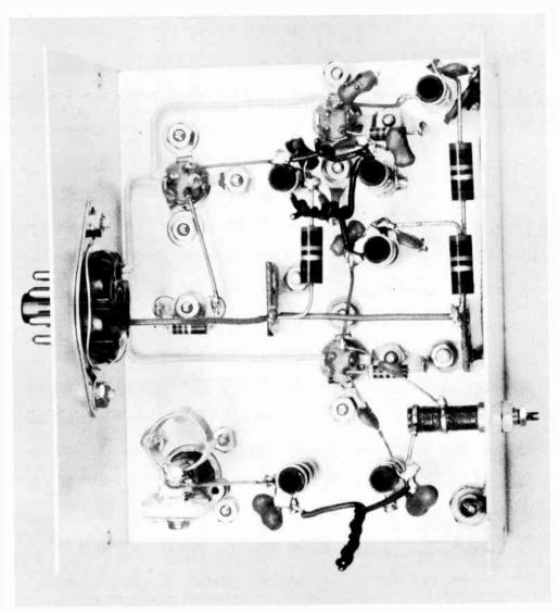
Fig. 16-10—Bottom view of the 50-Mc. converter. The antenna connector and trap circuit are in the lawer left corner. The neutralizing cail,  $L_4$ , is mounted horizontally, at lower right.
