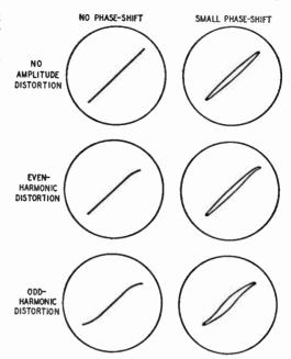
Fig. 9-33—Typical patterns obtained with the connections shown in Fig. 9-32. Depending on the number of stages in the amplifier, the pattern may slope upward to the right, as shown, or upward to the left. Also, depending on where the distortion originates, the curvature in the second row may appear either at the top or bottom of the line or ellipse.
