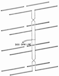
Fig. 18-15—Schematic drawing of a 16-element array.
