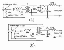
Fig. 19-46—Basic types of vibrator power-supply circuits.
