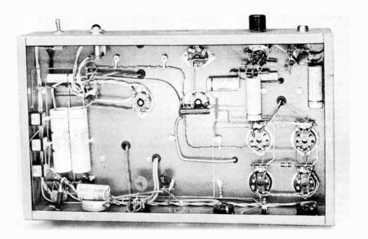
Fig. 9-22—Under the chassis of the 50-watt madulator. Three selenium rectifiers in the bias supply are mounted on the left-hand wall of the chassis. Associated camponents are grouped around the speech-amplifier sockets (upper right).
