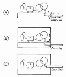
Fig. 23-20—Right (B) and wrong (A and C) ways to connect o coaxial line to the transmitter. In A or C, harmonic energy coupled by stray copacitance to the outside of the cable will flow without hindronce to the antenna system. In B the energy cannot leave the shield and can flow out only through, not over, the cable.
