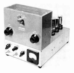
Fig. 6-48—Front view of the 6146 all-purpose amplifier. The upper panel is part of an  $8\times6\times31/2$ -inch Minibox (Bud CU-2109); the ventilated shielding of Reynalds Aluminium cane metal is fastened to the Minibox and base with sheet-metal screws.
