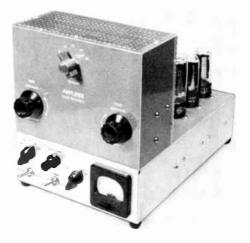
Fig. 6-48—Front view of the 6146 all-purpose amplifier. The upper panel is part of an  $8\times6\times31/2$ -inch Minibox (Bud CU-2109); the ventilated shielding of Reynolds Aluminium cane metal is fastened to the Minibox and base with sheet-metal screws.
