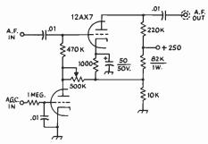
Fig. 5-29—A practical squelch circuit for cutting off the receiver output when no signal is present.
