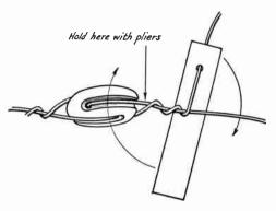
Fig. 14-50-Using a lever for twisting heavy guy wires.
