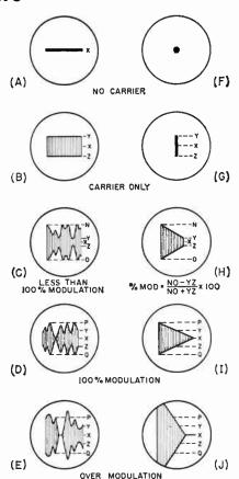
Fig. 10-18—Wave-envelope and trapezoidal patterns representing different conditions of modulation.
