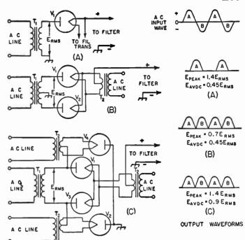
Fig. 7-2—Fundamental vacuum-tube rectifier circuits. A—Half-wave. B—Full-wave. C—Full-wave bridge. A.c.-input and pulsating-d.c. output wave forms are shown at the right. Output-voltage values indicated do not include rectifier drops. Other types of rectifiers may be substituted.
