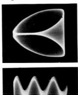
Fig. 10-22—Upper photo—Audio phose shift in coupling circuit between transmitter and horizontal deflection plates. Lower photo—Hum on vertical deflection plates.
