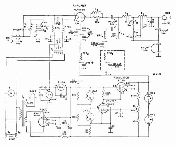
Fig. 6-74—Circuit diagram of the kilowatt graunded-grid linear amplifier. Unless indicated oherwise, capacitances are in μf., resistances are in ohms, resistors are ½ watt. Capacitors marked with polarity are electrolytic, capacitors marked \* are mica.
