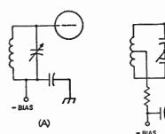
Fig. 6-34—The voltage rating of the grid tank capacitor in A should be equal to the biasing voltage plus about 20 per cent of the plate voltage.
