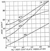
Fig. 10-16—Cathode-modulation performance curves, in terms of percentage of plate modulation plotted against percentage of Class C telephony tube ratings. W<sub>in</sub>-D.c. plate input watts in terms of percentage of plate-modulation rating.
