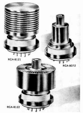
The air-cooled RCA-8121 and RCA-8122 high-perveance "tetrodes" offer more UHF power than ever in compact "low-cost" mobile communications. Featuring a 13.5-volt heater, these beam power tubes give dependable performance with battery operation. The RCA-8072 is a conduction-cooled version of the radiator types. These three unique types employing ceramic-metal construction represent another first from RCA for mobile use.
