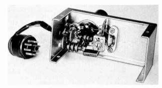
Fig. 6-90—This bottom view of the crystal oscillator shows the arrangement of components. Terminal strips are used for the cable connections and also as a support for C<sub>1</sub>, the feedback capacitor.
