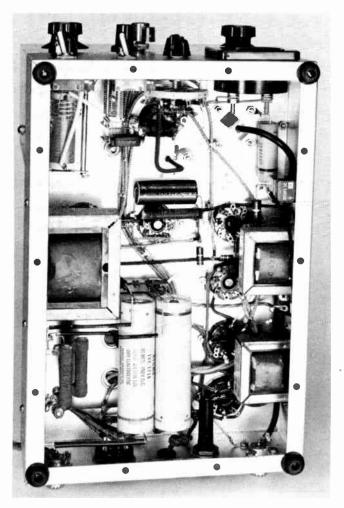
Fig. 6-51—Battam view af the all-purpose amplifier. The 150-ma, filter chake is maunted on the left-hand wall; the smaller filter chake, the small filament transfarmer (Ta in Fig. 6-50) and the selenium rectifier are maunted an the righthand wall. The strap of aluminum, visible below the meter at the tap right, pravides additional support for the length of RG-58/U cable that runs to the output coaxial cannectar. All power leads except the high voltage to the plate are run in shielded wire.
