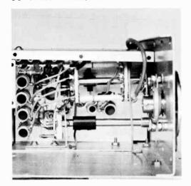
Fig. 19-16—View into the 6883 socket housing; the v.f.o. section has been removed. The short length of coaxial cable running from the front section of the switch is terminated in  $P_1$ . Coils  $L_4$ ,  $L_5$  and  $L_6$  are visible between the two switch wafers; the other coils are the driver plate-circuit inductors. The driver plate tuning capacitor is mounted an a small bracket.
