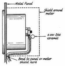
Fig. 23-14—Meter shielding and bypassing. It is essential to shield the meter mounting hale since the meter will carry r.f. through it to be radiated. Suitable shields can be made from 2½- or 3-inch diameter metal cans ar small metal chassis baxes.
