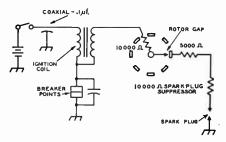
Fig. 19-1—Ignition system with recommended suppression methods.
