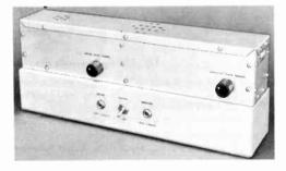
Fig. 17-34—A tripler-amplifier for 432 Mc. using dual tetrodes. Shielded construction and forced-air cooling are employed.
