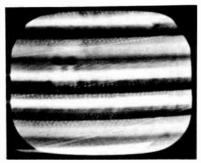
Fig. 23-6—"Saund bars" ar "madulatian bars" accampanying amplitude madulatian af an interfering signal. In this case the interfering carrier is strang enough ta destray the picture, but in mild cases the picture is visible thraugh the harizantal bars. Saund bars may accampany madulatian even thaugh the unmadulated carrier gives no visible crass-hatching.
