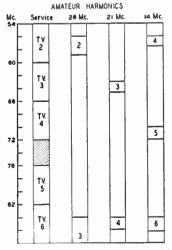
Fig. 23-3—Relationship of amateur-band harmonics to v.h.f. TV channels, Harmonic interference from transmitters operating below 30 Mc. is most likely to be serious in the low-channel group (54 to 88 Mc.).
