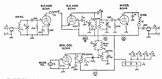
Fig. 16-11—Schematic diagram and parts information for the 144-Mc. converter. Resistors  $\frac{1}{2}$  watt unless specified. Fixed capacitors are ceramic unless specified. Decimal values in  $\mu$ f., others in  $\mu$  $\mu$ f.
