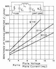
Fig. 6-13—Reactance of input capacitar, C<sub>1</sub>, as a function the ratio of plate valtage to plate current.
