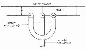
Fig. 14-56—Details of a coaxial-line termination board and T-match support for a 10-meter beam. The balun of a half-wavelength of coaxial line is coiled and then fastened to the boom with tape.
