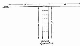
Fig. 14-19—Practical arrangement of a shortened antenna. When the total length, A+B+B+A, is the same as the antenna length plus twice the feeder length of the center-fed antennas of Table 14-I, the same type of coupling circuit will be used. When the feeder length or antenna length, or both, makes the sum different, the type of coupling circuit may be different but the effectiveness of the antenna is not changed, unless A+A is less than a quarter wavelength.
