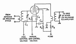
Fig. 5-28—Typical radio-frequency amplifier circuit for a superheterodyne receiver. Representative values for components are as follows:
