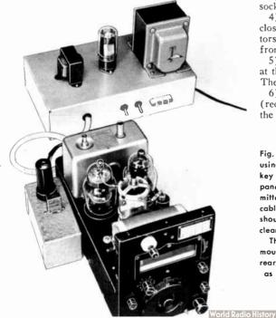
Fig. 6-87—The complete Novice setup, in this case using the 80-meter (BC-696) transmitter. Note the key jack at the lower-left corner of the transmitter panel. The crystal oscillator is connected to the transmitter oscillator-tube socket with o short length of cable terminating in on octal plug. A small notch should be cut in the transmitter cover to provide clearance for the cable when the cover is installed.
