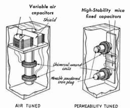
Fig. 5-15—Representative i.f.-transformer construction. Coils are supported on insulating tubing. The shield in the air-tuned transformer prevents capacity coupling between the tuning capacitors. In the permeability-tuned transformer the cores consist of finely-divided iron particles supported in an insulating binder, formed
