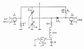
Fig. 21-46—Circuit of the impedance bridge. Resistors are composition, ½ watt except as noted. Fixed capacitors are ceramic.
