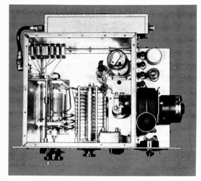
The inductor is fitted with a Groth turns counter, making it easy to return to the proper setting for each band. Until the settings for each band have been found,  $S_3$  should be turned so that all of the output capacitance is in circuit. The inductor should be set near maximum for 80, and approximately half maximum for 40. On the higher-frequency bands, the inductor should be set so that the circuit resonates with the tank capacitor near minimum capacitance. Loading
