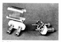
Fig. 21-34—A convenient mounting, using binding-post plates, for L and C standards made from commercially-available parts. The capacitor is a 100- $\mu\mu$ f. silver mica unit, mounted so the lead length is as nearly zero as possible. The inductance standard, 5  $\mu$ h., is 17 turns of No. 3015 B & W Miniductor, 1-inch diameter, 16 turns per inch.
