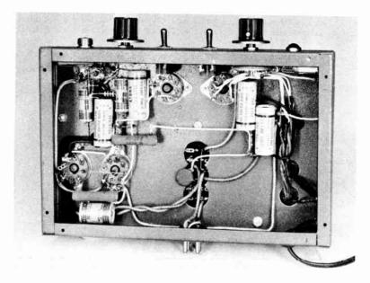
Fig. 9-19-Underchassis view of the 6BQ6GT modulator. The two large capacitors at the right are the filter capacitors in the power supply. The modulator bias resistor and bypass capacitor  $(R_1C_3)$  are at lower left. Leads from the modulation transformer go through the three holes in the chassis. Shielded wire is used for heater, microphone input, and gaincontrol leads.
