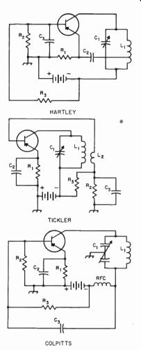
Fig. 4-12—Typical transistor oscillator circuits. Component values are discussed in the text.
