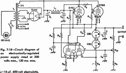
C<sub>1</sub>, C<sub>2</sub>, C<sub>5</sub>-16-\(\mu f\). 600-volt electrolytic.
