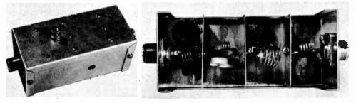
Fig. 23-24—Low-pass filter for use with 50-Mc. transmitters at powers up to about 300 watts. The housing is a 21/4-inches square by 5-inches long Minibox. Connections between the various sections of the filter are made through 5/16-inch clearance holes cut in the centers of the shielding partitions.
