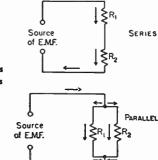
Fig. 2-4—Resistors connected in series and in parallel.
