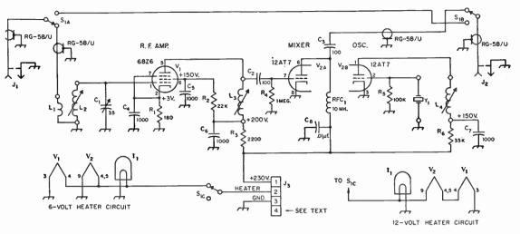
Fig. 19-5—Circuit diagram of the crystal-controlled mobile converter. Unless otherwise indicated, capacitances are in  $\mu\mu f$ ., resistances are in ohms, resistors are  $\frac{1}{2}$  watt.
