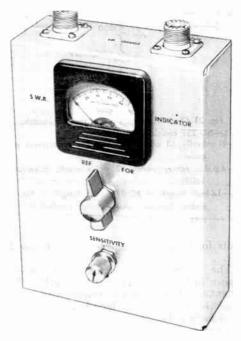
Fig. 21-42—The Monimatch, an s.w.r. monitor that can be left in the line at all times. The unitshawn here will handle a kilowatt.
