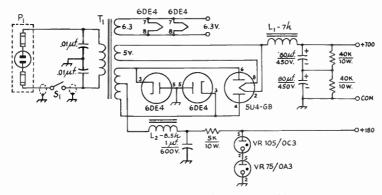
Fig. 6-52—Power supply section of the all-purpose amplifier.
