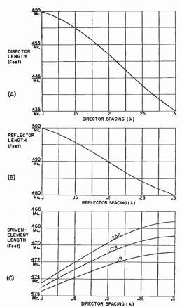
Fig. 14-36—Element lengths for a 3-element beam. These lengths will hald closely for tubing elements supported at an near the center.
