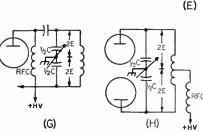
Fig. 6-33—Diagrams showing the peak voltage for which the plate tank capacitor should be rated for c.w. operation with various circuit arrangements. E is equal to the d.c. plate voltage. The values should be doubled for plate modulation. The circuit is assumed to be fully loaded. Circuits A, C and E require that the tank capacitor be insulated from chassis or ground, and from the control.
