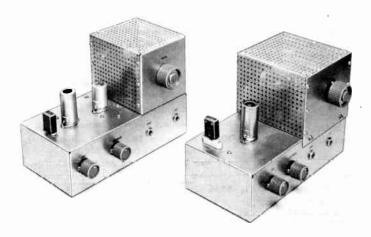
Fig. 17-17—Transmitters far 50 (right) and 144 Mc. Designs are similar and many parts are interchangeable. Pawer ratings may be varied fram under 10 ta mare than 50 watts input, depending an tube used in the autput stage.
