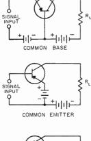
or by resistance-capacitance coupling. In any case it is to be understood that a d.c. path must exist between the base and emitter.
