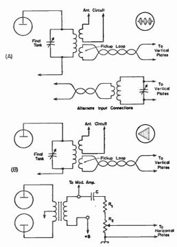
Fig. 10-17—Methods of connecting the oscilloscope for modulation checking. A—connections for wave-envelope pottern with any modulation method; B—connections for trapezoidol pottern with plote or screen modulation.
