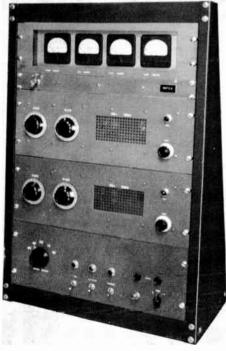
Fig. 6-64—Individual kilowatt amplifiers for two bands plus complete metering and all control circuits and power supplies (except plate) fit handily into a table rack. Amplifiers for five bands plus the plate supply will mount in floor rack. Band switch at lower left (S<sub>B</sub> in Fig. 6-65) switches filament supply, excitation and output connections to all amplifiers in use; screen and plate supplies are connected to all amplifiers at all times.
