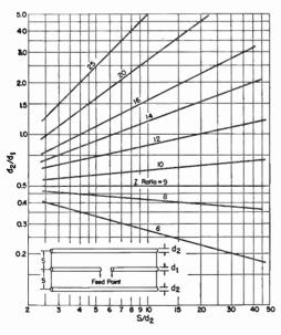
Fig. 14-44—Impedance transformation ratio, three-conductor folded dipole. The dimensions  $d_1$ ,  $d_2$  and s are shown on the inset drawing. Curves show the ratio of the impedance (resistive) seen by the transmission line to the radiation resistance of the resonant antenna system.
