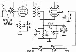
Fig. 9-11—Speech-amplifier output compression circuit.
