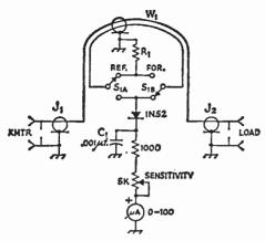
Fig. 21-43—Wiring diagram of the Monimatch. J<sub>1</sub>, J<sub>2</sub>—SO-239 coaxial receptacle.
