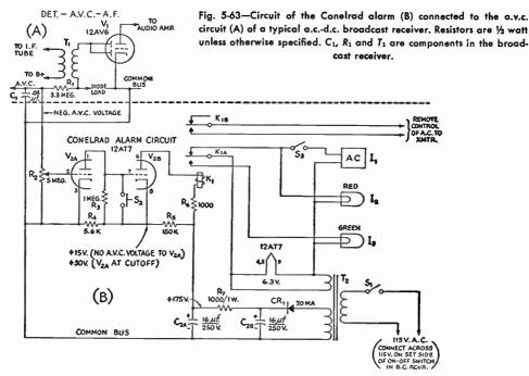
l<sub>1</sub>—6-volt a.c. buzzer (Edwards 725). l<sub>2</sub>, l<sub>8</sub>—6-volt pilot lamp, No. 47. K<sub>1</sub>—D.p.d.t. sensitive relay, 5000-ohm coil. R<sub>2</sub>—5-megohm potentiometer.
