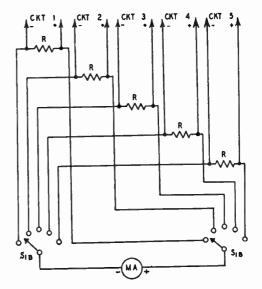
Fig. 6-32—Switching a single milliammeter. The resistors, R, should be 10 to 20 times the internal resistance of the meter; 47 ohms will usually be satisfactary.  $S_1$  is a 2-section rotary switch. Its insulation should be ceramic for high voltages, and an insulating coupling should olways be used between shaft and control.
