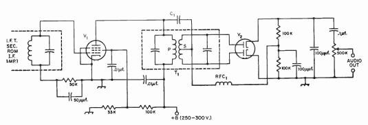
Fig. 12-8—Limiter-discriminator circuit. This type of circuit is frequently used at 455 kc. in the form of an "adapter" for communications receivers, for reception of narrow-band f.m. signals.
