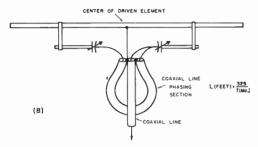
Fig. 14-37—The most popular methods of feeding the driven element of a beam antenna are (A) the gamma match and (B) the T match. The aluminum tubing or rod used for the matching section is usually of smaller diameter than the antenna element; its length will vary somewhat with the spacing and number of elements in the beam. The coaxial line in the phasing section can be coiled in a 2- or 3-foot diameter coil instead of hanging as shown.
