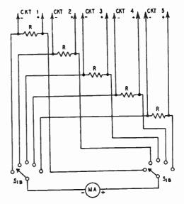
Fig. 6-32—Switching a single milliammeter. The resistors, R, should be 10 to 20 times the internal resistance of the meter; 47 ohms will usually be satisfactory.  $S_1$  is a 2-section rotary switch. Its insulation should be ceramic for high voltages, and an insulating coupling should always be used between shaft and control.
