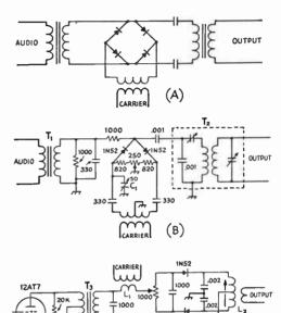
Fig. 11-1—Typical rectifier-type balanced modulators.
