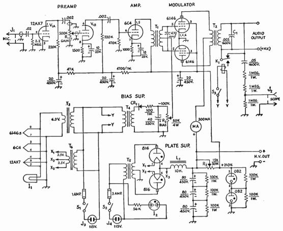
Fig. 9-24—Circuit diagram of the 6146 modulator and power supply. Capacitances are in  $\mu$ f. unless indicated otherwise; capacitors marked with polarity are electrolytic, others may be paper or ceramic as convenient.
