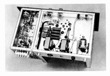
adjustment of the amplifier grid circuit, insert an s.w.r. bridge unit such as a Micromatch in the coax connecting the driver and amplifier, and tune  $C_1$  and  $C_2$  in the amplifier alternately for minimum reflected power. Adjust the driver tuning for maximum forward power.
