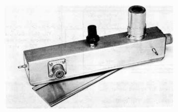
Fig. 16-17—220-Mc. trough-line preamplifier. Unit connects by cable to a remote receiver or converter.
