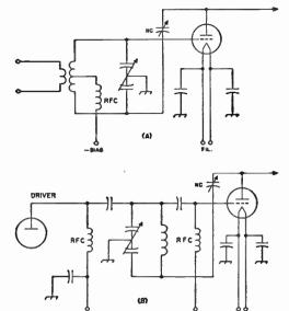
Fig. 6-25—When a pi-network output circuit is used with a triode, a balanced grid circuit must be provided for neutralizing. A—Inductive-link input. B—Capacitive input caupling.
