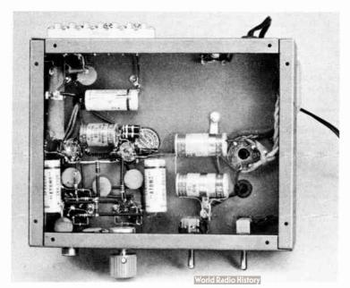
9-16—Below-chassis Fia. view of the modulator. The rectifier tube socket and electrolytic filter capacitors are at the right in this view. The 12AX7 socket is at the lower left. Bleeder resistor R5 is at the upper left, near the 6-terminal connection strip on the rear edge of the chassis. Placement of components is not critical, but the leads in the first two stages should be kept short and close to the chassis to minimize hum troubles
