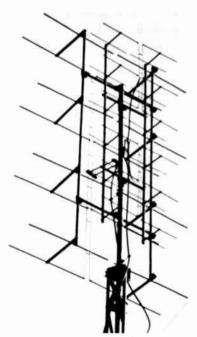
Fig. 18-18—A 24-element array for 420 Mc. and a 16element for 220 mounted back-to-back on a single support.
