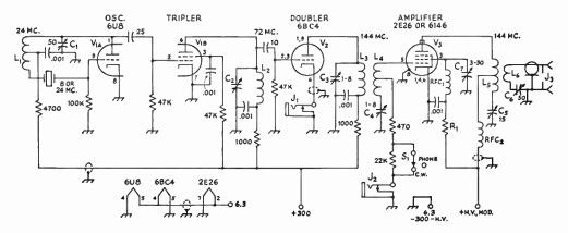
Fig. 17-24—Schematic diagram and parts information for the 144-Mc. transmitter.
