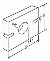
Fig. 13-25—Dimensions of the insulating spacers used to hold the pick-up wires in place in the Monimatch.
