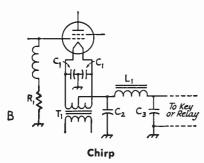
The frequency-stability reference in the opening paragraph refers to the "chirp" observed on many signals. This is caused by a change in frequency of the signal during a single dot or dash.
