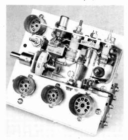
Fig. 19-15—The v.f.o. section is built in the U-shaped portion of a  $3\frac{1}{4} \times 2\frac{1}{6} \times 1\frac{3}{6}$ -inch Minibox (Bud CU-2101-A) mounted on a sheet of aluminum; the other half of the Minibox serves as the cover. The Nuvistor socket and the oscillator coils are mounted on one side of the Minibox. Jack  $J_1$  is mounted on the other side of the Minibox and is visible between the two right-hand tube sockets.
