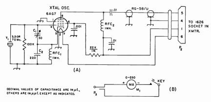
Fig. 6-89—(A) Circuit diagram of external crystal-controlled oscillator. Unless otherwise specified, resistances are in ohms, resistors are  $\frac{1}{2}$  watt. The 0.01- and 0.001- $\mu$ f. capacitors are disk ceramic. (B) Method of connecting the milliammeter in series with the key.
