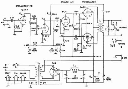
Fig. 9-15—Circuit of the speech amplifier and modulator. All capacitances are in  $\mu f$ .; capacitors with polarities marked are electrolytic, others are ceramic. Resistors are  $\frac{1}{2}$  watt except as noted below. Voltages measured to chassis with v.t. voltagetre.
