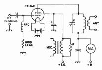
Fig. 10-10—Screen-grid madulation of beam tetrade. Capacitar C is an r.f. bypass capacitar and should have high reactance at audia frequencies. A value af 0.002  $\mu$ f, is satisfactory. The grid leak can have the same value that is used far c.w. aperation af the tube.
