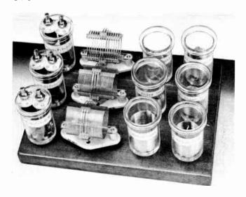
Fig. 11-13—Plug-in coils and r.f. phase-shift networks for the sideband generator. Output tank coils (right) include additional padding capacitor for C<sub>7</sub>, as given in the coil table. Polystyrene coil forms are 4-pin (Allied Radio 24-4P) and 5-pin (Allied Radio 24-4P).
