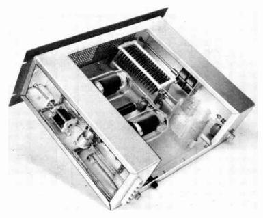
Fig. 6-66—View of the 40-meter amplifier with its cane-metal covering removed. As in each amplifier, the chassis is made from two 5 × 13 × 3-inch chassis and a 13 × 17-inch bose plote. Input and low-voltage leads make up to terminols and jack in center foreground.
