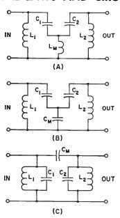
Fig. 2-46-Three methods of circuit coupling.
