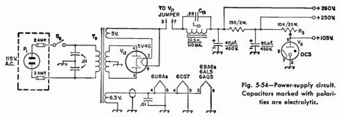
$C_{18}$ —0.25- $\mu$ f. paper, 600 volts.  $L_{10}$ —Filter choke, 10.5 henry, 110 ma. (Knight 62 G 139).  $P_{1}$ —Fuse plug.
