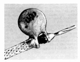
Fig. 23-9—Proper method of bypassing the end of a shielded lead using disk ceramic capacitor. The 0.001μf, size should be used for 1600 volts or less; 500 μμf, at higher voltages. The leads are wrapped around the inner and outer conductors and soldered, so that the lead length is negligible. This photograph is about four times actual size.
