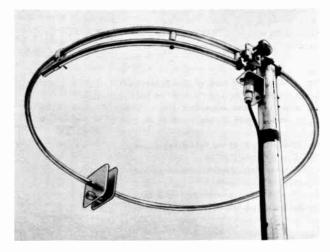
Tuning up at 145 Mc., for example, will give quite satisfactory operation from the low end to 146 Mc., the halo being much broader in frequency response when it is operated on its third harmonic. In this model the series capacitor in the gamma arm was at about the middle of its range for 50 Mc., and near minimum for 144 Mc. Slight differences in mechanical construction may change the value of capacitance required, so these settings should not be taken as important.
