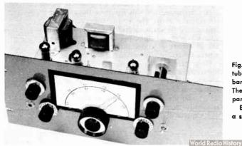
Fig. 5-30—The SimpleX Super receiver uses three dual tubes and a crystal filter to cover the 80- and 40-meter bands, and it can tune to 5 Mc. for copying WWV. The dial scale is made from white paper held to the panel by black tape; the index is clear plastic.
