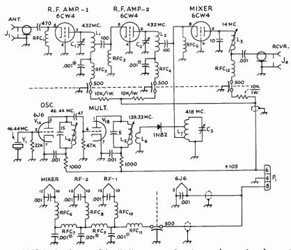
Fig. 16-25—Wiring diagram of the 430-Mc. converter. Capacitance values are in  $\mu\mu f$ ., except decimal values which are in  $\mu f$ . Resistors are ½ watt unless specified otherwise. All 0.001- $\mu f$ . capacitors marked \* are button-type (Centralab ZA-102); other 0.001- $\mu f$ . capacitors are disk ceramic. All 500- $\mu\mu f$ . feedthrough capacitors are Centralab FT-500.
