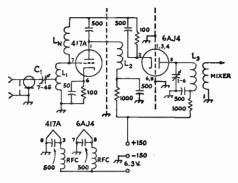
Fig. 16-2—Circuit af the cascade r.f. amplifier. Caupling capacitar,  $C_1$ , may be amitted if spuriaus receiver responses are not a problem. Neutralizing winding,  $L_{\rm N}$  should resonate at the signal frequency with the gridplate capacitance of the first tube. Base cannections are far 417A and 6AJ4, but ather small triades may be used.
