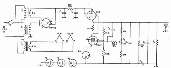
Fig. 7-19—High-voltage regulator circuit by W4PRM. Resistors are 1 watt unless indicated otherwise.
