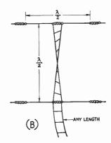
Broadside arrays may be fed either by tuned open-wire lines or through quarter-wave matching sections and flat lines. In Fig. 14-30B, note the "crossing over" of the phasing section, which is necessary to bring the elements into proper phase relationship.
