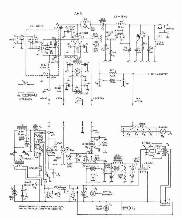
Fig. 6-78—Circuit diagram of the 4-400A amplifier (abave the dashed line) and power supply/cantrol unit.
