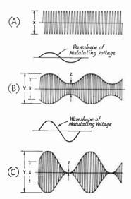
Fig. 10-1—Graphical representation of (A) r.f. output unmodulated, (B) modulated 50%, (C) modulated 100%. The modulation envelope is shown by the thin outline on the modulated wave.
