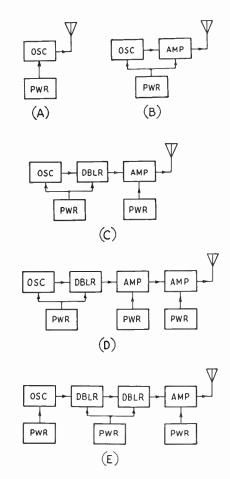
Fig. 6-1—Block diagrams showing typical combinations of oscillator and amplifiers and power-supply arrangements for transmitters. A wide selection is possible, depending upon the number of bands in which operation is desired and the power output.
