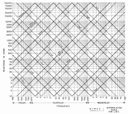
Fig. 2-28—Inductive and capacitive reactance vs. frequency. Heavy lines represent multiples of 10, intermediate light lines multiples of 5; e.g., the light line between 10  $\mu$ h. and 100  $\mu$ h. represents 50  $\mu$ h., the light line between 0.1  $\mu$ f. and 1 µf. represents 0.5 µf., etc. Intermediate values can be estimated with the help of the interpolation scale shown.
