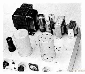
Fig. 6:39—An inexpensive 75-watt transmitter using plug-in coils and an "economy" power supply. The oscillator (left) is a 6AG7; the 1625 output tube is mounted underneath the chassis. Shield cans are baking-powder tins painted gray; the can for the output coil (right) is ventilated for better cooling, as is the chassis behind the can.
