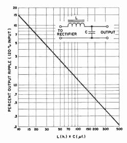
Fig. 7-10—Graph showing combinations of inductance and capacitance that may be used to reduce ripple with a single-section choke-input filter.
