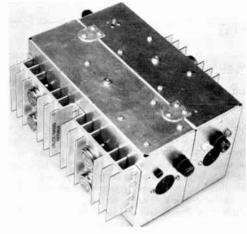
Fig. 19-49—Triple transistar pawer supply delivers +600, +250 and -300 valts. Ribbed aluminum heat sinks are standard item, were painted black after picture was taken. Tube sackets are used as jacks for autput and cantral circuits, tip jacks are valtage test paints. Twa chassis are hinged an underside, lacked tagether an tap by twa tabs af aluminum and sheetments.
