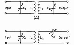
Fig. 2-48—Inductively-coupled resonant circuits. Circuit A is used for high-resistance loads (load resistance much higher than the reactance of either  $L_2$  or  $C_2$  at the resonant frequency). Circuit B is suitable for low resistance loads (load resistance much lower than the reactance of either  $L_2$  or  $C_2$  at the resonant frequency).
