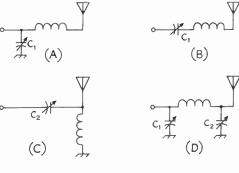
Fig. 13-19—The variaus configurations that can be obtained from the "randam-wire" antenna caupler.
