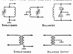
Fig. 2-59—Single-ended and balanced circuits.
