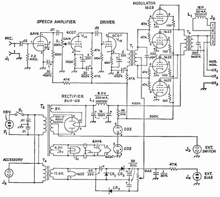
Fig. 9-21—Circuit diagram of the 50-watt modulator. Unless specified otherwise, capacitances are in  $\mu$ f., resistors are  $\frac{1}{2}$  watt.
