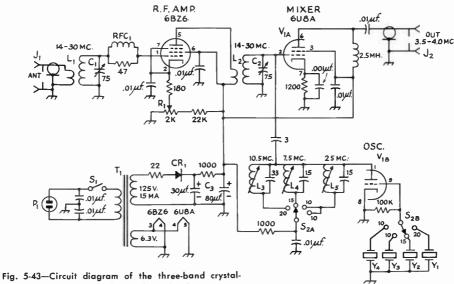
Fig. 5-43—Circuit diagram of the three-band crystalcontrolled converter. Unless indicated otherwise, capacitances are in  $\mu\mu f$ ., resistors are  $\frac{1}{2}$  watt.
