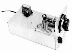
Fig. 5-48—The regenerative preselector covers the range 7 to 30 Mc.; it can be used ahead of any receiver to improve gain, image rejection and, in many cases, sensitivity. A dual triode 6CG7 is used a r.f. amplifier and cathode follower.
