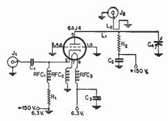
Fig. 16-22—Schematic diagram of the 420-Mc. r.f. amplifier.
