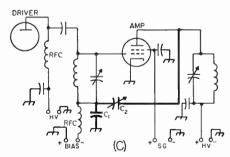
Fig. 6-23—Screen-grid neutralizing circuits. A—Inductive neutralizing. B-C—Capacitive neutralizing.
