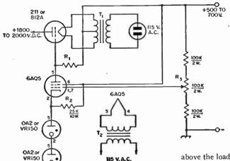
Fig. 7-20—Screen regulator circuit designed by W9OKA. Resistances are in ohms (K = 1000).
