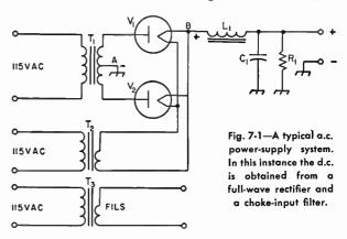
mary winding to withstand the peak value of the rectified voltage.  $T_s$  is a similar transformer to supply the filaments or heaters of the tubes in the equipment operating from the supply. Frequently these three transformers are combined in a single unit having the 115-volt primary winding and the three secondary windings on one core.
