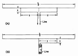
Fig. 14-45—The "T" match and "gamma" match.
