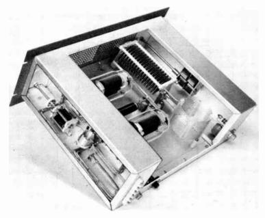
Fig. 6-66—View of the 40-meter amplifier with its cane-metal covering removed. As in each amplifier, the chassis is made from two 5 × 13 × 3-inch chassis and a 13 × 17-inch base plate. Input and low-voltage leads make up to terminals and jack in center foreground.
