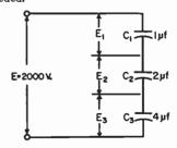
Fig. 2-11—An example of copacitors connected in series.
