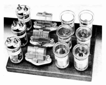
Fig. 11-13—Plug-in coils and r.f. phase-shift networks for the sideband generator. Output tank coils (right) include additional padding capacitor for C<sub>7</sub>, as given in the coil table. Polystyrene coil forms are 4-pin (Allied Radio 24-4P) and 5-pin (Allied Radio 24-4P).
