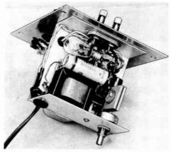
Fig. 21-20—Bottom view of the audio oscillator, showing the power-supply components and amplitude-control lamp, I1. The lamp is mounted by wires soldered to its base. The selenium rectifier is supported by a tie-point strip. Placement of resistors, which are hidden by the other components, is not critical. The unit fits in a  $4 \times 5 \times 6$  inch box.
