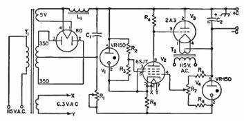
Fig. 7-25—Circuit diagram of an electronically-regulated bias supply.
