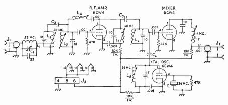
Fig. 16-9—Schematic diagram and parts information for the 50-Mc. converter. Resistors ½ watt unless specified. Fixed copacitors are ceramic; decimal values in μf., others in μμf.
