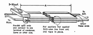
Fig. 23-31—Absorption-type wave trap using sections of 300-ohm line tuned to have an electrical length of ¼ wavelength at the transmitter frequency. Approximate physical lengths (dimension A) are 40 inches for 50 Mc. and 11 inches for 144 Mc., allowing for the loading effect of the capacitance at the open end. Two traps are used in parallel, one on each side of the line to the receiver.
