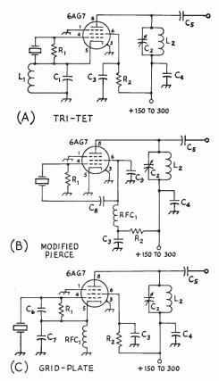
Fig. 6-3—Cammanly used crystal-cantralled ascillatar circuits. Values are thase recommended for a 6AG7 ar 5763 tube. (See reference in text for other tubes.) C<sub>1</sub>—Feedback-contral capacitor—3.5-Mc. crystals—apprax. 220-μμt. mica—7-Mc. crystals—approx. 150-μμt. mica.
