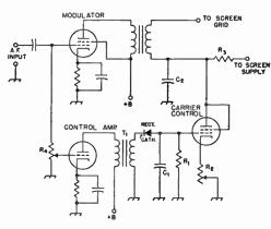
Fig. 10-12—Circuit far carrier cantral with screen madulation. A small triade such as the 6C4 can be used as the cantral amplifier and a 6Y6G is suitable as a carrier-cantral tube.  $T_1$  is an interstage audia transfarmer having a 1-ta-1 ar larger turns ratia.  $R_4$  is a 0.5-megahm valume cantral and alsa serves as the grid resistar far the madulatar. A germanium crystal may be used as the rectifier. Other values are discussed in the text.
