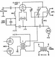
Fig. 10-15-Circuit arrangement for cathade modulation of a Class C r.f. amplifier. Values of bypass capacitors in the r.f. circuits should be the same as for other modulation methods.
