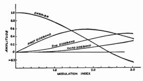
Fig. 12-2—How the amplitude of the pairs of sidebands varies with the modulation index in an f.m. or p.m. signal. If the curves were extended for greater values of modulation index it would be seen that the carrier amplitude goes through zero at several points. The same statement also applies to the sidebands.
