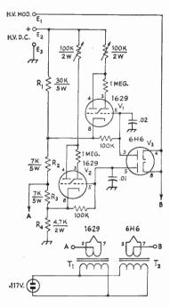
Fig. 10-24—Circuit diagram of the modulatian manitor. Unless specified otherwise, resistars are  $\frac{1}{2}$  watt, resistances are in ahms, capacitances are in  $\mu f$ .
