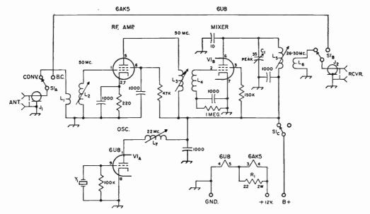
Fig. 19-11—Schematic diagram for the 50-Mc. mobile converter. All resistors ½ watt unless otherwise specified. Capacitor values below 0.001 μf. are in μμf. All 0.001 μf. capacitors are disk ceramic. Other fixed capacitors are tubular ceramic.
