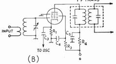
At high and very-high frequencies it is difficult to secure an adequate image ratio when the intermediate frequency is of the order of 455 kc. To reduce image response the signal frequently is converted first to a rather high (1500, 5000, or even 10,000 kc.) intermediate frequency, and then — sometimes after further amplification—reconverted to a lower i.f. where higher adjacent-channel selectivity can be obtained. Such a receiver is called a double-conversion superheterodyne.
