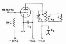
Fig. 6-10—Inductive-link output coupling circuits.
