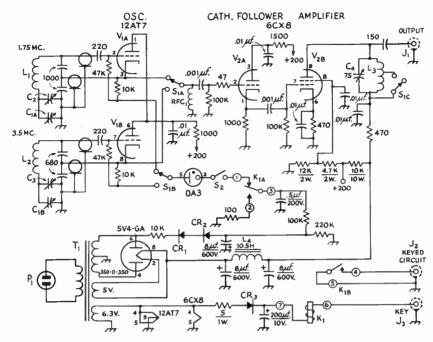
Fig. 6-84—Circuit diagram of the two-band v.f.o. Unless specified otherwise, resistances are in ohms, resistors are  $\frac{1}{2}$  watt, capacitances are in  $\mu\mu$ f. Fixed capacitors associated with  $V_1$  are silvered mica, all decimal capacitors are ceramic, capacitors marked with polarity are electrolytic.
