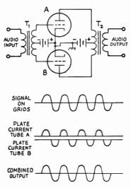
Fig. 3-13—Class B amplifier operation.
