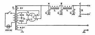
Fig. 7-13—Typical a.c. powersupply circuit for receivers, exciters, or low-power transmitters. Representative values will be found in Table 7-II. The 5-volt winding of 71 should have a current rating of at least 2 amp. for types 5Y3-GT and 5V4-GA, and 3 amp. for 5U4-GB,
