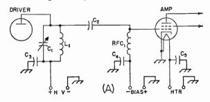
Fig. 6-21—Capacitive-coupled amplifiers.
