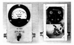
Fig. 21-28—Dual-range r.f. voltmeter for use in coaxial line, using a 0-1 d.c. milliammeter. The voltage-divider resistors,  $R_1$  and  $R_2$  (Fig. 21-27) are at the center in the lower compartment. The bypass capacitors and  $R_3$  are mounted on a tie-point strip at the right. The unit is built in a  $4\times 6\times 2$  inch aluminum chassis, with an aluminum partition connecting the two sides of the box to form a shielded space. A bottom plate, not shawn, is used to complete the shielding.
