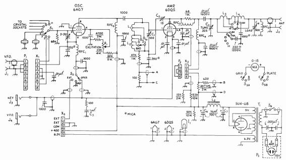
Fig. 6-45—Circuit diagram of the 75-watt 6DQ5 transmitter. Unless specified otherwise, capacitance is in μμf., resistance is in ohms, resistors are ½ watt. C<sub>1</sub>—100-μμf. midget variable (Hammarlund HF-100). C<sub>2</sub>—15-μμfd. midget variable, .025 inch spacing (Johnson 15J12).
