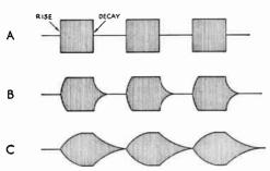
Fig. 8-1—Typical oscilloscope displays of a code transmitter. The rectangular-shaped dots or dashes (A) have serious key clicks extending many kc. either side of the transmitter frequency. Using proper shaping circuits increases the rise and decay times to give signals with the envelope form of B. This signal would have practically no key clicks. Carrying the shaping process too far, as in C, results in a signal that is too "soft" and is not easy to copy.
