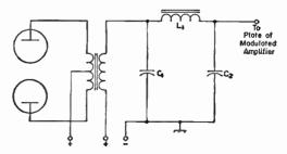
Fig. 9-13—Splatter-suppression filter for use at high level, shawn here connected between a Class B modulator and plate-modulated r.f. amplifier. Values for  $L_1$ ,  $C_1$  and  $C_2$  are determined as described in the text.
