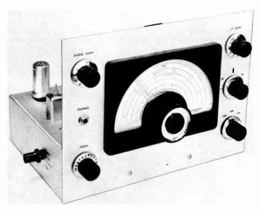
Fig. 5-35—The 2X4 + 1 superheterodyne is a four-tube receiver with 7-tube performance. It tunes the 80- and 40meter amateur bands, and provision is included for receiving WWV on 5 Mc. A built-in crystal oscillator provides 100-kc. frequency markers throughout the bands. Black knob on the left-hand side controls the calibration oscillator and the WWV reception.
