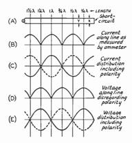
Fig. 13-2—Standing waves of valtage and current along shart-circuited transmission line.
