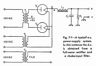
mary winding to withstand the peak value of the rectified voltage.  $T_s$  is a similar transformer to supply the filaments or heaters of the tubes in the equipment operating from the supply. Frequently these three transformers are combined in a single unit having the 115-volt primary winding and the three secondary windings on one core.
