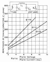
Fig. 6-13—Reactance of input capacitar, C<sub>1</sub>, as a function the ratio of plate voltage to plate current.
