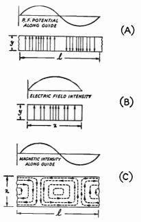
Fig. 2-63—Field distribution in a rectangular waveguide. The  $IE_{1/0}$  mode of propagation is depicted.
