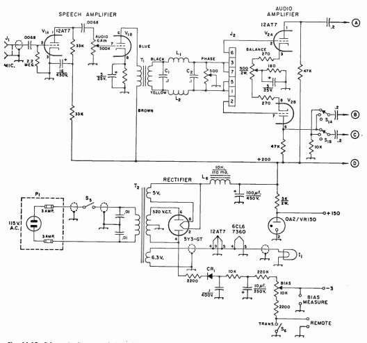
Fig. 11-12—Schematic diagram of the sideband generator. Unless specified otherwise, resistors are ½-watt, .01and .002-µf. capacitors are disk ceramic, 600 volts; .1- and .2-µf. capacitors are tubular paper, 400 volts; capacitors marked with polarities are electrolytic.
