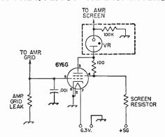
Fig. 6-18—Screen clomper circuit for protecting screen-grid power tubes. The VR tube is needed only for complete cut-off.
