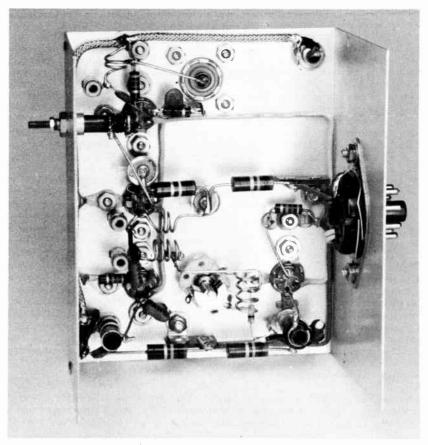
Fig. 16-15—View underneath the chassis of the 220-Mc. converter. The long shielded wire runs from  $L_{\rm b}$  at the lower left to the output jack. Silver-button mica capacitors (Centralab ZA-102) that bypass the plate coil and the control grid of the second 6CW4 (center left) are also used to support several resistors. Coil  $L_{\rm b}$  is supported by the terminals of  $C_{\rm b}$  (bottom center). Chassis is part of  $3\times4\times5$ -inch Minibox.
