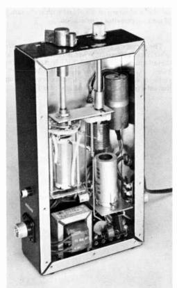
The t.r. switch shown in Fig. 8-16 differs in several ways from the preceding example. It contains its own power supply and consequently can be used with any transmitter/receiver combination without "borrowing" power. It will add gain and front-end selectivity to the receiver. A commercial switch-coil-capacitor combination is shown in the unit, although the constructor could-build his own if desired.
