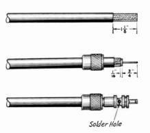
Fig. 20-4—Dimensions for stripping ½-inch cable to fit Amphenol Type 83-1SP (PL-259) plug.
