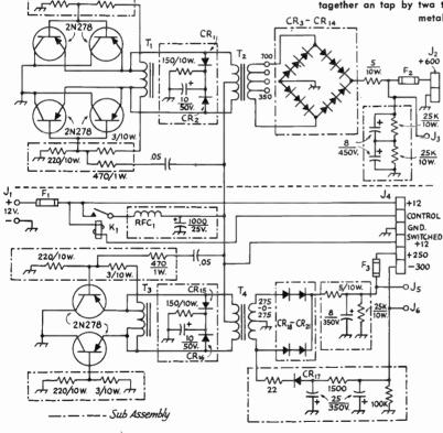
Fig. 19-50—Circuit diagram of the triple transistarized power supply. Capacitances are in μf., resistars are ½ watt unless specified atherwise. Capacitars marked with palarity are electralytic; athers are paper.
