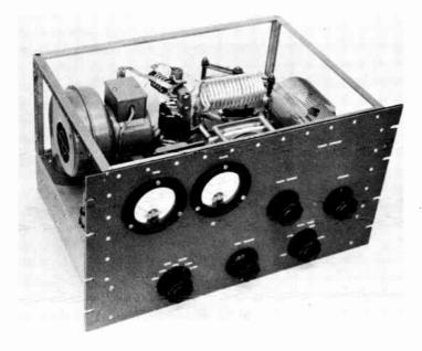
Fig. 6-73-A grounded grid amplifier using the PL-6580 triode. Able to handle a kilowatt p.e.p. input with 3000 volts on the plate, and even more with a higher plate voltage, a chimney surrounds the tube to improve the forced ventilation. In this view the side and top cane-metal panels have been removed.
