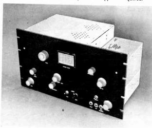
Fig. 17-9—The high-power 2-meter rig, with shielding enclosures in place. The small unit at the right houses the tripler and driver stages.
