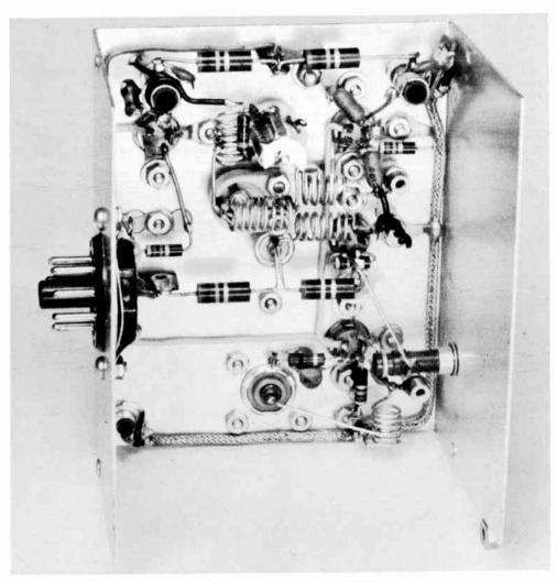
Fig. 16-12—Interior of the 144-Mc. converter. Details of parts arrangement are given in the text. The i.f. output from the mixer plate coil, L<sub>5</sub>, (upper right) is brought through a shielded lead down the side and across the bottom to the output connector, J<sub>2</sub>, at the lower left.
