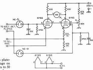
The zero-center meter,  $M_1$ , is not a necessity but is a convenience in making adjustments.  $R_1$  should be adjusted on receiver noise for zero reading. With a 2125-cycle tone the pointer will swing to the left and  $L_1$  should be adjusted for maximum deflection. With a 2975-cycle tone the pointer will swing to the right and  $L_2$  should be adjusted for maximum deflection. Equal deflections should be obtained from both channels.
