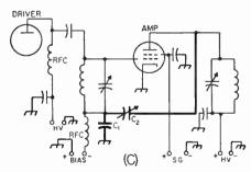
Fig. 6-23—Screen-grid neutralizing circuits. A—Inductive neutralizing. B-C—Capacitive neutralizing.
