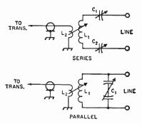
Fig. 13-14—Link-coupled series and parallel tuning.
