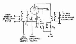
Fig. 5-28—Typical radia-frequency amplifier circuit far a superheteradyne receiver. Representative values far campanents are as fallaws:
