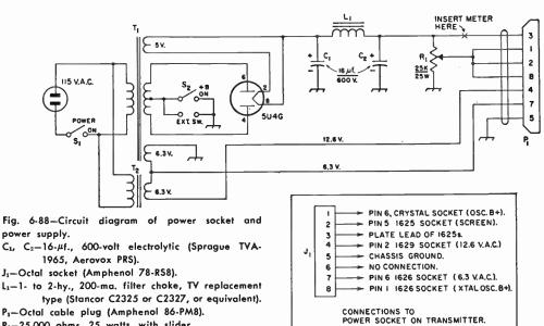
T<sub>2</sub>—Filament transformer, 6.3 volts, 3 amp. (Triad F-16X, Knight 62-G-031, or equivalent).
