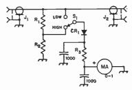
Fig. 21-27—Dual-range r.f. voltmeter circuit. Capactances are in  $\mu\mu$ f.; capacitors are disk ceramic.
