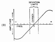
Fig. 12-7—F.m. or p.m. detection characteristics. A—
