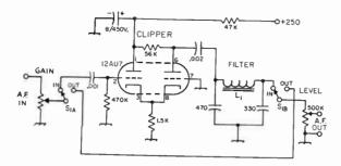
Fig. 9-12—Practical speech clipper circuit with law-pass filter. Capacitances belaw 0.001  $\mu$ f. are in  $\mu\mu$ f. Resistars are ½ watt. L<sub>1</sub>—20 henrys, 900 ahms (Stancar C-1515). S<sub>1</sub>—D.p.d.1. taggle ar ratary.
