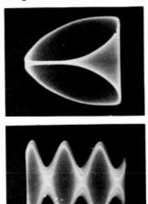
Fig. 10-22—Upper photo—Audio phose shift in coupling circuit between transmitter and harizantal deflection plates. Lower photo—Hum an vertical deflection plates.
