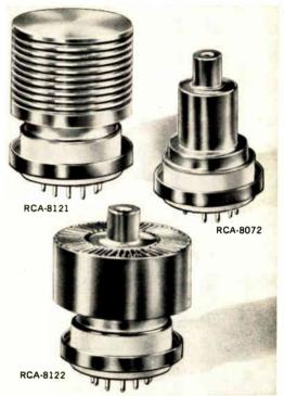
The air-cooled RCA-8121 and RCA-8122 high-perveance "tetrodes" offer more UHF power than ever in compact "low-cost" mobile communications. Featuring a 13.5-volt heater, these beam power tubes give dependable performance with battery operation. The RCA-8072 is a conduction-cooled version of the radiator types. These three unique types employing ceramic-metal construction represent another first from RCA for mobile use.
