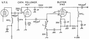
Fig. 6-6—Circuit af an isalating amplifier far use between v.f.a. and first tunable stage. Unless atherwise specified, all capacitances are in  $\mu f$ ., all resistars are  $\frac{1}{2}$  watt. L<sub>1</sub>, for the 3.5-Mc. band, consists of 100-140  $\mu h$ . adjustable inductor. RFC<sub>1</sub> is 100  $\mu h$ . All capacitars are disk ceramic.
