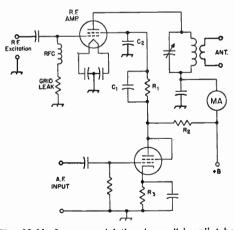
Fig. 10-11—Screen modulation by a "clomp" tube. The grid leak is the normal value for c.w. operation and  $C_2$  should be 0.002  $\mu$ f. or less. See text for discussion of  $C_1$ ,  $R_1$ ,  $R_2$  and  $R_3$ .  $R_3$  should have the proper value for Closs A operation of the modulator tube, but cannot be colculated unless triade curves for the tube are available.
