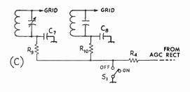
Fig. 5-17—Delayed automatic gain-control circuits using a twin diode (A) and a dual-diode triode. The circuits are essentially the same and differ only in the method of biasing the a.g.c. rectifier. The a.g.c. control voltage is applied to the controlled stages as in (C). For these circuits typical values are:
