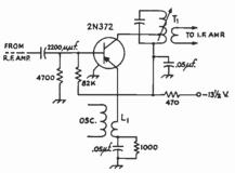
Fig. 5-12—Typical transistor mixer circuit.
