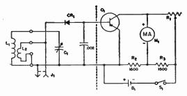
Fig. 21-36—Transistor d.c. amplifier applied to the wavemeter of Fig. 21-10 to increase sensitivity. Components not listed below are the same as in Fig. 21-10. B<sub>1</sub>—Small flashlight cell.
