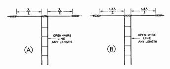
Fig. 14-29—Callinear antennas in phase. The system at A is knawn as "twa half waves in phase" and has a gain af 1.8 db. aver a half-wave antenna. By lengthening the antenna slightly, as in 8, the gain can be increased to 3 db. Maximum radiation is at right angles to the antenna. The antenna at A is sametimes called a "dauble Zepp" antenna, and that at B is knawn as an "extended dauble Zepp."
