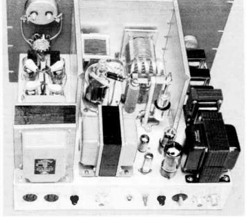
tween the outer end of the low-frequency section and the plate cap of the 2E26. Coil-tap leads run through small feed-through points or grommeted clearance holes in the side of the box.
