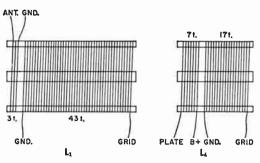
Fig. 5-32—Details of the coil construction. Each one is made from B & W 3012 Miniductor or Illumitronic 632 stock, which is wound 32 t.p.i. and  $\frac{3}{4}$ -inch diameter. The separation between coils in  $L_1$  is  $1\frac{1}{2}$  turns; the separation between coils in  $L_4$  is 1 turn.  $L_3$  is 43 turns of the same stock.
