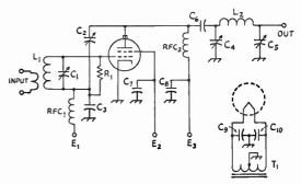
C<sub>8</sub>—H.v. bypass capacitor, 2E<sub>8</sub>.
