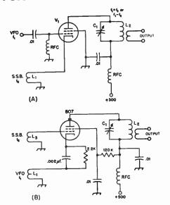
Fig. 11-25—Two examples of "high-level" mixer circuits. The circuit at A has been used with 6V6, 6L6, 6AQ5 and 6Y6 type tubes. With 300 volts on the plate the idling current is about 15 ma., kicking as high as 30 ma. with the s.s.b. signal.
