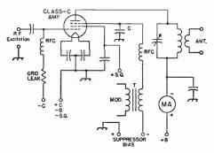
Fig. 10-13—Suppressor-grid modulation of an r.f. amplifier using a pentode-type tube. The suppressor-grid r.f. bypass capacitor, C, should be the same as the grid bypass capacitor in control-grid modulation.
