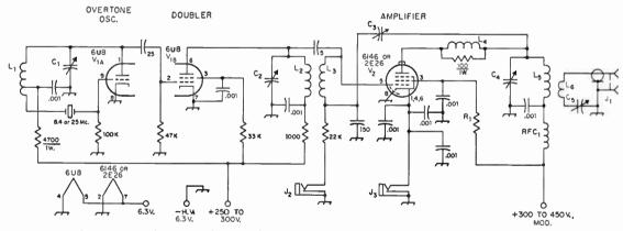
Fig. 17-20—Schematic diagram and parts information for the 50-Mc. transmitter. Capacitors are ceramic unless specified. Values under .001 are in μμf. Resistors ½ watt unless specified.
