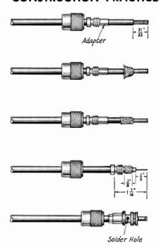
Fig. 20-5—Method of assembling ¼-inch cable, Amphenol Type 83-1SP (PL-259) plug and adapter.
