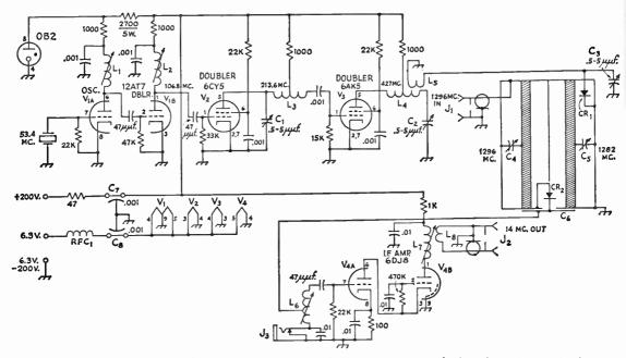
Fig. 16-29—Circuit diagram and parts information for the 1296-Mc. converter. Decimal values of capacitors are in  $\mu$ f.
