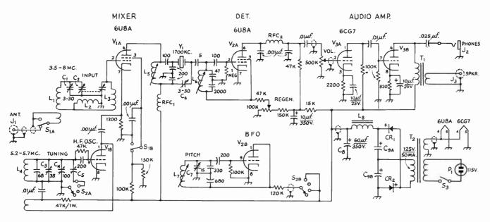
Fig. 5-31—Circuit diagram of the SimpleX Super receiver. Unless otherwise indicated, capacitances are in μμf., resistances are in ohms, resistors are ½ watt. Polarity is shown on electrolytic capacitors, 680 μμf. or less are silver mica or NPO ceramic, 2000-μμf. fixed capacitor is mica. Capacitors specified in decimal-μf. values are ceramic.
