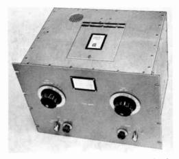
Fig. 6-79—This view of the amplifier shows the bandswitch trap door, air-exhaust port and hole for adjusting neutralization, all in the top of the shielding enclosure. The large knob on the left of the panel is for the 20/15/10-meter plate tuning capacitor, and the matching knob adjusts the capacitor used on 80 and 40. Farther down, from left to right: grid band switch, grid tuning control, variable loading adjustment and loading switch.
