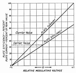
Fig. 10-9—In a perfect grid-madulated amplifier bath plate current and plate efficiency would vary with the instantaneous madulating voltage as shawn. When this is sa the madulatian characteristic is as given by curve A in Fig. 10-4, and the peak envelape output power is faur times the unmodulated carrier power. The variations in plate current with madulation, indicated above, da nat register an a d.c. meter, so the plate meter shows na change when the signal is modulated.
