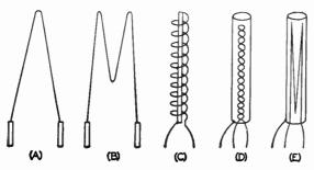
Fig. 3-2—Types of cathode construction. Directly heated cathodes or filaments are shown at A, B, and C. The inverted V filament is used in small receiving tubes, the M in both receiving and transmitting tubes. The spiral filament is a transmitting tube type. The indirectly-heated cathodes at D and E show two types of heater construction, ane a twisted loop and the other bunched heater wires. Both types tend to cancel the magnetic fields set up by the current through the heater.
