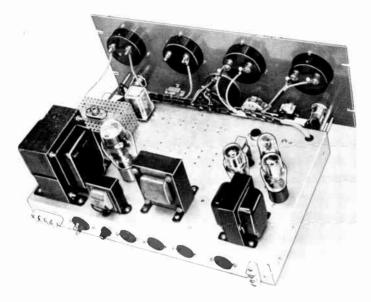
Fig. 6-80—Top view of the control unit. The voltmeter multiplier resistors are housed in a cane-metal protective shield (upper left). Resistors R<sub>8</sub> and R<sub>9</sub> are mounted under the sets of ventilation holes (center near panel).
