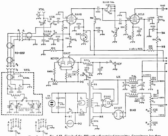
Fig. 6-57—Circuit of the 500-watt self-contained transmitter. Capacitance less than 0.001  $\mu$ f. are in  $\mu\mu$ f. Fixed capacitors of capacitance greater than 100  $\mu\mu$ f. should be disk ceramic, except as noted below. Fixed capacitors of 100  $\mu\mu$ f. and 220 μμf. should be mica. Capacitors marked with polarity are electrolytic. Resistors not otherwise marked are  $\frac{1}{2}$  watt. R.f. chokes in  $\mu$ h. unless otherwise marked.
