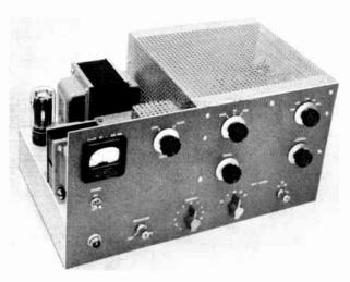
Fig. 6-44—This 75-watt crystal-controlled transmitter has provision for the addition of v.f.o. control. A 6AG7 oscillator drives a 6DQ5 amplifier on 80 through 15 meters.
