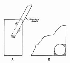
Fig. 20-2—To cut rectangular hales in a chassis corner, holes may be filed out as shown in the shaded portion of B, making it possible ta start the hack-saw blade along the cutting line. A shows how a single-ended handle may be canstructed for a hack-saw blade.
