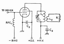
Fig. 6-10—Inductive-link output coupling circuits.
