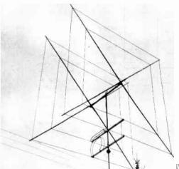
of collinear driven and parasitic elements and combination broadside-collinear-parasitic elements. Thus two or more collinear elements might be provided with a collinear reflector or director set, one parasitic element to each driven element. Or both directors and reflectors might be used. A broadside-collinear array can be treated in the same fashion.
