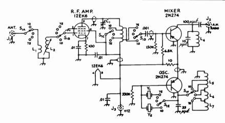
Fig. 19-8—Circuit diagram of the hybrid crystal-controlled converter. Unless specified otherwise, capacitances are in μf., resistances are in ohms, resistors are ½ watt.
