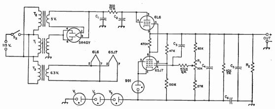
Fig. 7-19—High-voltage regulator circuit by W4PRM. Resistors are 1 watt unless indicated otherwise. C<sub>1</sub>, C<sub>2</sub>—4-μf. paper, voltage rating above peak-voltage
