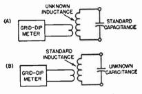
Fig. 21-33—Setups for measuring inductance and capacitance with the grid-dip meter.
