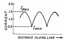
Fig. 13-5—Measurement of standing-wave ratio. In this drawing,  $I_{\text{max}}$  is 1.5 and  $I_{\text{min}}$  is 0.5, so the s.w.r.  $=I_{\text{max}}I_{\text{min}}=1.5/0.5=3$  to 1.
