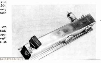
by the use of a tuned circuit in the cathode lead. Output is taken off through a coupling loop at the point of lowest r.f. voltage along the line.
