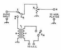
Fig. 21-55—Circuits for supplying r.f., audio, and a.c. voltages to oscilloscope deflection plates for modulation monitoring.
