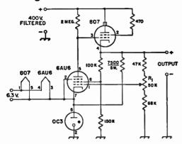
Fig. 7-17—Electronic voltage-regulator circuit. Resistors are ½ watt unless specified otherwise.
