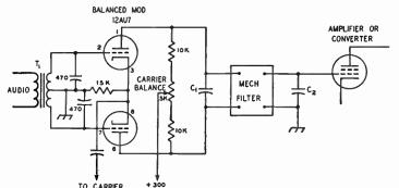
Fig. 11-4—One type of balanced-modulator circuit that can be used with a mechanical filter (Collins F455-31 or F500-31 series) in the i.f. range. The filters are furnished in various types of mountings, and the values of C<sub>1</sub> and C<sub>2</sub> will depend upon the type of filter selected.
