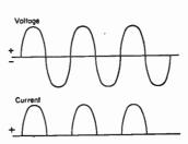
the polarity of the voltage across the load is as indicated. If the diode were reversed, the polarity of the voltage developed across the load R would be reversed.
