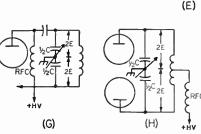
Fig. 6-33—Diagrams showing the peak voltage for which the plate tank capacitor should be rated for c.w. operation with various circuit arrangements. E is equal to the d.c. plate voltage. The values should be doubled for plate modulation. The circuit is assumed to be fully loaded. Circuits A, C and E require that the tank capacitor be insulated from chassis or ground, and from the control.
