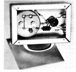
Fig. 19-43—Inside view of the meter. The back plate shown in the photograph is used as a cover for the box.
