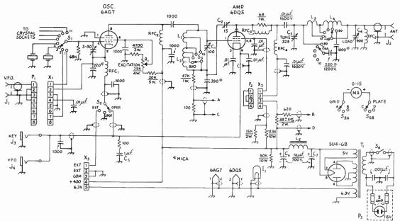
Fig. 6-45—Circuit diagram of the 75-watt 6DQ5 transmitter. Unless specified otherwise, capacitance is in μμf., resistance is in ahms, resistors are ½ watt. C<sub>1</sub>—100-μμf. midget variable (Hammarlund HF-100). C<sub>2</sub>—15-μμfd. midget variable, .025 inch spacing (Johnson 15J12).
