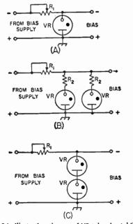
Fig. 7-24—Illustrating the use of VR tubes in stabilizing protective-bias supplies.  $R_1$  is a resistor whose value is adjusted to limit the current through each VR tube to 5 ma. before amplifier excitation is applied. R and  $R_8$  are current-equalizing resistors of 50 to 1000 ohms.
