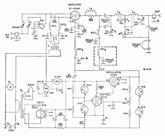
Fig. 6-74—Circuit diagram of the kilowatt grounded-grid linear amplifier. Unless indicated oherwise, capacitances are in μf., resistances are in ohms, resistors are ½ watt. Capacitors marked with polarity are electrolytic, capacitors marked \* are mica.
