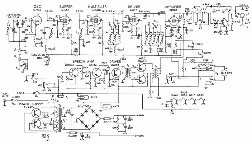
Fig. 19-19—Circuit diagram of the mobile transmitter. Unless specified otherwise, capacitances are in  $\mu\mu$ f., decimal values are in  $\mu$ f., resistances are in ohms, resistors are ½ watt.
