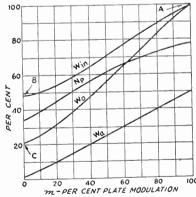
Fig. 10-16—Cathade-modulation performance curves, in terms of percentage of plate madulation plotted against percentage af Class C telephany tube ratings. W<sub>in</sub>-D.c. plate input watts in terms of percentage of plate-madulation rating.
