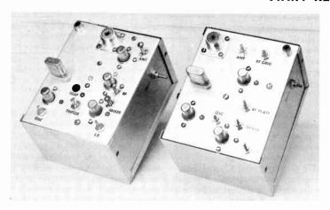
Fig: 16-8—The 50- and 144-Mc. crystal-controlled converters are built in 3  $\times$  4  $\times$  5-inch Miniboxes and are designed to work into a receiver that tunes 14 to 18 Mc. Plate voltage required is +150, and use of a 0D3-stabilized supply is suggested.
