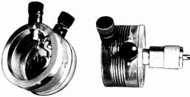
Fig. 21-50 — Balun construction (W2ZE). 150-ohm Twin-Lead may be used for the bifilar winding in place of the ordinary wire shown. Symmetrical construction with tight coupling between the two coils is essential to good performance.
