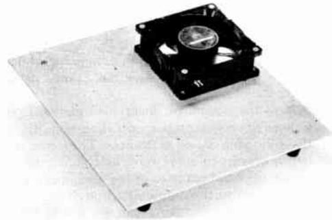
Fig. 6-82—Blower is mounted on bottom plate of amplifier near the front panel (not directly under the tube). A.c. power connector for blower is made from microphone-connector fittings.
