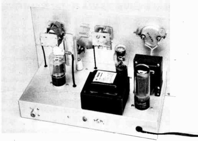
Fig. 6-37—Rear view of the transmitter showing the placement of components above chassis. The loading capacitor, C_8 , is at the left, L_3 is the vertical coil and L_2 the horizontal one. Rubber grommets are used to prevent chafing and to furnish additional insulation on the leads coming from below chassis.
