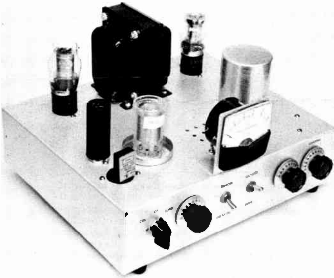
Fig. 6-39—The inexpensive 75-watt transmitter is a two-tube five-band crystal-controlled transmitter; v.f.o. control can be added at any time. To simplify construction and testing, plug-in coils are used, housed in the two shield cans (Millen 80011 or Miller S-42 with S-42C base). The crystal-oscillator tube, a 12BY7, is housed in the black tube shield at the left; the 1625 amplifier tube is mounted under the chassis.
