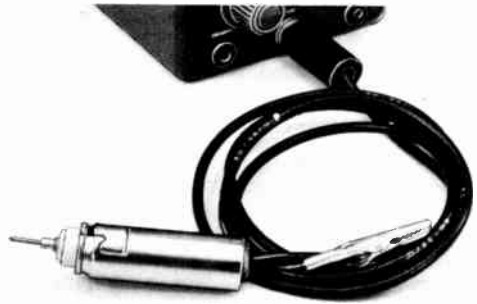
Fig. 21-32—The r.f. probe is used in conjunction with a vacuum-tube voltmeter. The case of the probe is constructed from a 7-pin ceramic tube socket and a 2 1/4-inch tube shield. A half-inch grommet at the top of the tube shield prevents the output lead of the probe from chafing. The flexible copper-braid grounding lead and alligator clip provide a low-inductance return path from the test circuit. The d.c. output of the probe goes to the phone plug, which plugs into the d.c. input jack of the v.t.v.m.
