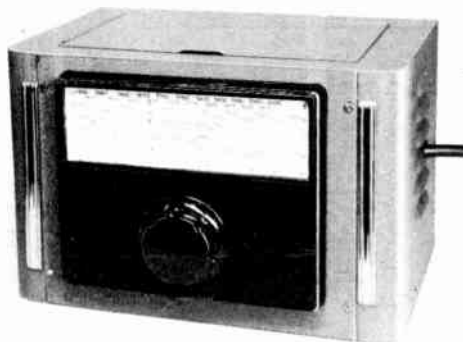
Fig. 6-61—The remote v.f.o. tuning unit is housed in a standard metal cabinet. The cable at the right plugs into the main chassis.
