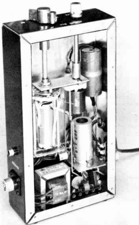
Fig. 8-16—The electronic t.r. switch is built in a 5 x 9 x 2 1/2-inch chassis; the bottom plate has been removed to show the placement of parts. Although two receiver outlets are shown on the near face (a phono jack and a coaxial receptacle), only one is required, depending upon one's choice of cable termination.
