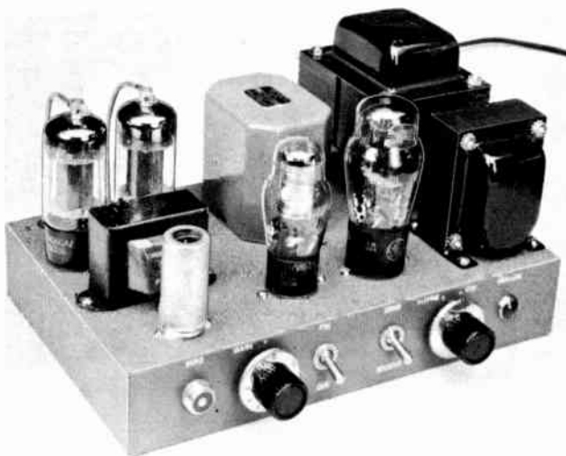
Fig. 9-17—A modulator for transmitters operating at plate inputs up to 50 watts. The speech amplifier and modulator are at the left in this view; power supply components are at the right. The chassis is 7 × 11 × 2 inches.
