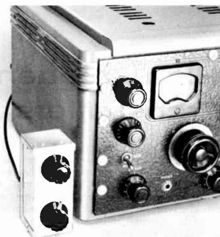
Fig. 5-60—View of the Q multiplier showing its single connecting cable to the receiver. The box can be placed in any convenient spot on or around the receiver.
