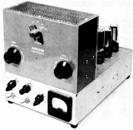
Fig. 6-47—Front view of the 6146 all-purpose amplifier. The upper panel is part of an 8 × 6 × 3½-inch Minibox (Bud CU-2109); the ventilated shielding of Reynolds Aluminium cane metal is fastened to the Minibox and base with sheet-metal screws.
