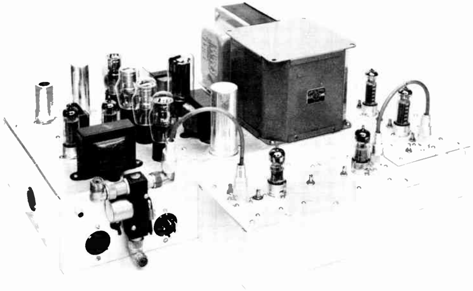
Fig. 17-13—Rear view of the power supply and modulator, with the 144- and 432-Mc. units in place, for 432-Mc. operation. The 432-Mc. unit is in the foreground; its power plug plugs into a socket on the 144-Mc. driver.
