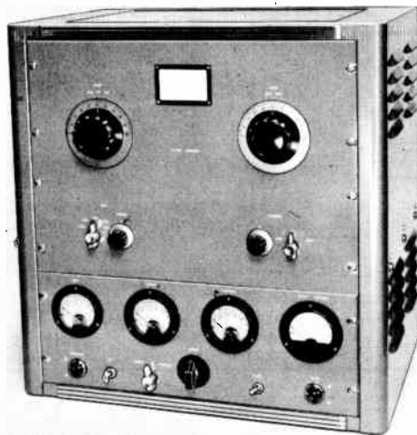
Fig. 6-67—The kilowatt 4-400A amplifier and its control unit are mounted in a 21-inch gray hammerstone rack cabinet (Bud CR-1727). Shelf brackets (Bud SA-1350) are mounted on both sides of the cabinet to hold the amplifier chassis. Below the meters, from left to right: filament pilot light, key-type a.c. switch, Class AB 1 /C bias switch, screen autotransformer, plate switch and plate pilot light.
