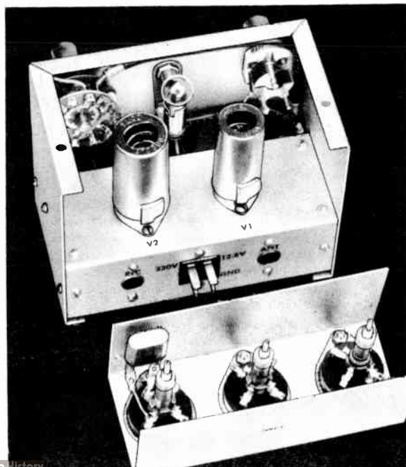
Fig. 19-7—Homemade L-shaped chassis, mounted on small brackets fastened to the side walls of the converter housing, is 4\frac{1}{8} inches long, 2 inches wide and 1\frac{1}{2} inches deep. V_1 is mounted on the chassis to the right of V_2 as seen in this rear view. J_1 , J_2 and J_3 are in line in that order from right to left across the rear wall of the chassis. An interior view of a coil compartment is shown in the foreground. Terminals of the coils are soldered directly to the socket terminals. Notice that the crystal for the oscillator is mounted adjacent to L_4 .
