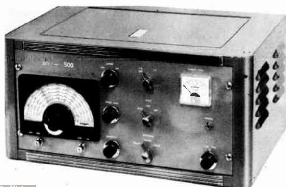
Fig. 5-51—The DCS-500 double-conversion superheterodyne. Left bottom, antenna trimmer, 100-kc. calibrator switch; center, left, top to bottom, noise-limiter switch, volume control, sensitivity control; center, right, b.f.o. switch, a.g.c. speed, selectivity; right, headphone jack, b.f.o. pitch control. The dial is a National ICN. Front panel is 8¾ inches high; the receiver is mounted in a Bud CR-1741 rack cabinet.
