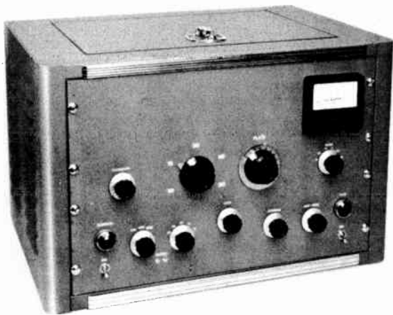
Fig. 6-57—A 500-watt transmitter. Power supplies and a differential keyer are included. It operates with the external v.f.o. tuner shown in Fig. 6-58. Controls along the bottom, from left to right, are for low-voltage power, v.f.o./crystals/s.s.b. switch, driver tank switch, driver tank capacitor, final loading, v.f.o. set switch, and high-voltage. Above, from left to right, are controls for excitation, final tank switch, final tank capacitor and meter switch. The bond-switch pointer is made by cutting down the metal skirt of a dial similar to the one to the right.
