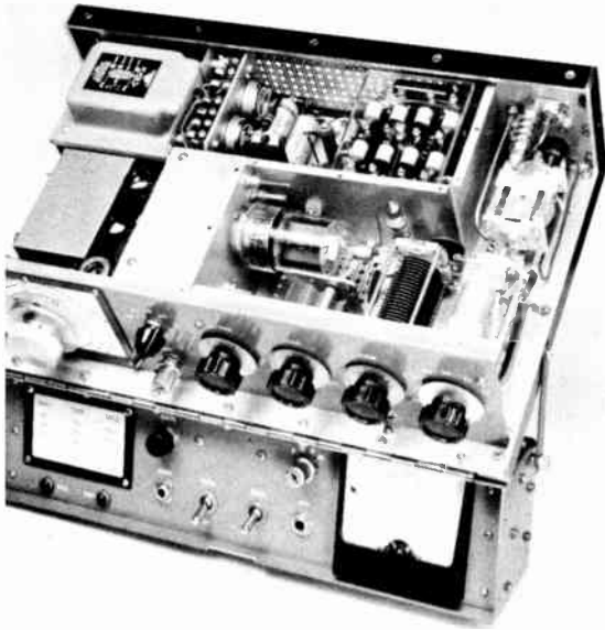
Fig. 19-21—The 65-watt mobile transmitter has a Nuvistor v.f.o., a 6146 output stage and transistors in the modulator and power supply. In this view the sheet-metal top and sides have been removed to show the arrangement of parts. The panel carrying the meter and switches (see Fig. 19-23) is recessed in a 3½ high \times 2¾ deep by 14-inch box; the box is hinged and folds up when the transmitter is not in use. Major chassis is built from ¾-inch wide by ½-inch thick aluminum angle and a 9 \times 14-inch sheet of aluminum. A ventilation hole covered with cane metal is partially visible below the 6146 (center).
