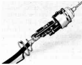
Fig. 21-34—Close-up of the inside of the probe. The 1N34A crystal diode rectifier, calibrating resistor, and input capacitor are mounted tight to the terminal strip with shortest leads possible. Spaghetti tubing is placed on the diode leads to prevent accidental short circuits. The tube-shield spring and REXIBLE-copper grounding lead are soldered to the cable braid (the cable is RG-58/U coax). The tip can be either a phone tip or a short pointed piece of heavy wire.
