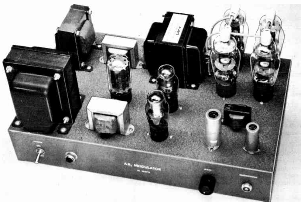
Fig. 9-20—A 50-watt modulator, using four 1625-type tubes in Class AB 1 . With higher plate voltage and a larger modulation transformer, the tubes can deliver up to 140 watts of audio power.
