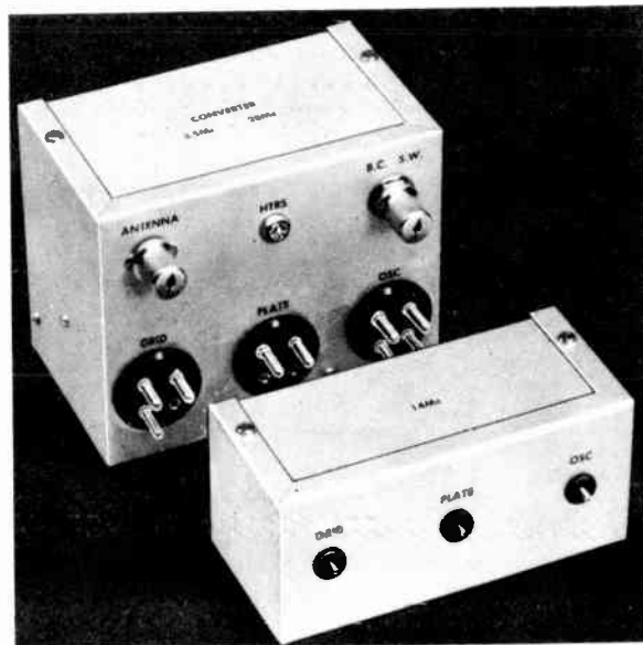
Fig. 19-4—The aluminum case for the converter measures 3 \times 4 \times 5 inches (Bud CU-3005 or Premier AMC-1005). Amphenol type 86-CP4 male jacks mounted on the front of the box mate with MIP 4-prong sockets mounted on the rear of the coil compartment shown in the foreground. Knobs for C_1 and S_1 are to the left and right, respectively, of the pilot lamp. The coil box measures 2\frac{1}{4} \times 2\frac{1}{4} \times 5 inches (Bud CU-3004 or Premier AMC-1004). Slug-adjustment screws for L_2 , L_3 and L_4 protrude through rubber grommets mounted on the front wall of the plug-in coil assembly.
