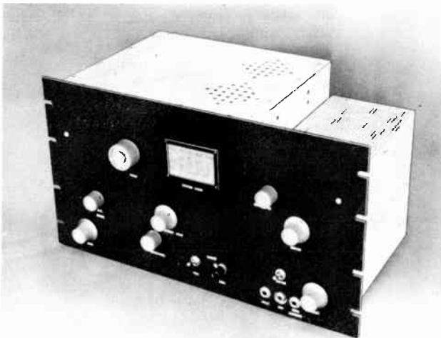
Fig. 17-23—The high-power 2-meter rig, with shielding enclosures in place. The small unit at the right houses the tripler and driver stages.
