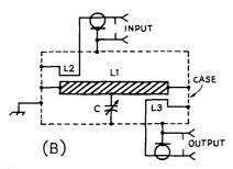
Fig. 23-23—Equivalent circuits for the strip-line fiters. At A, the circuit for the 6- and 2-meter filters is shown.  $L_2$  and  $L_3$  are the input and output links. These filters are bilateral, permitting interchanging of the input and output terminals.
