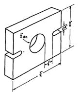
Fig. 21-50—Dimensions of the insulating spacers used to hold bridge wires and outer conductor strips in place.
