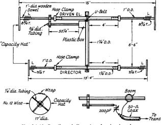
Fig. 14-46—Details and dimensions for the short beam. Reynolds aluminum tubing is used throughout. Homemade aluminum clamps permit adjustment of the gamma rod. The gamma tuning capacitor is enclosed in a plastic box which is secured to the boom. Hose clamps permit the tubing sections to be secured after they are telescoped together.
