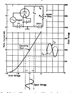
Fig. 3-8—Amplifier operation. When the plate current various in response to the signal applied to the grid, a varying voltage drop appears across the load,  $R_p$ , as shown by the dashed curve,  $E_p$ .  $I_p$  is the plate current.
