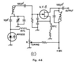
Fig. 4-6 illustrates how a voltage-variable capacitor diode can be used to tune a v.f.o. These diodes can be used to tune other r.f. circuits also, and are particularly useful for remote tuning of r.f. circuits, such as might be encountered in
