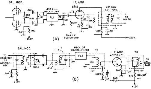
Fig. 9-6—Typical circuits showing how s.s.b. filters are connected in the circuit.
