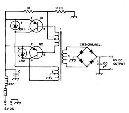
Fig. 19-26—Typical dc-to-dc converter. Ratings for  $CR_8$ - $CR_6$ , and the 100- $\mu$ F filter capacitor can be selected from data in Chap. 12.
