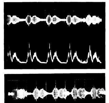
showing the clipper action. In each picture the top trace is the s.s.b. input to the clipper. (Above) Rectified s.s.b. output from the transceiver, no clipping. Peak power is set just below "flattopping." The word is, "Hello." Zero power is the bottom line. (Below) Same as above, but with clipping. The increase in average power is apparent.
