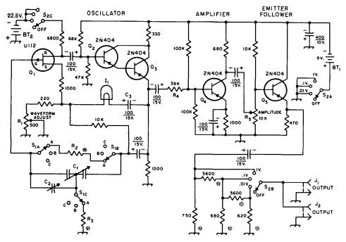
Fig. 21-21—Circuit diagram of the transistor audio oscillator. Unless specified otherwise, all capacitors are miniature electrolytics, all capacitances are in microfarads ( $\mu$ f.) Resistors marked with an asterisk are ½ watt  $\pm$  5 percent, others are  $\pm$  10 percent, resistances are in ohms.
