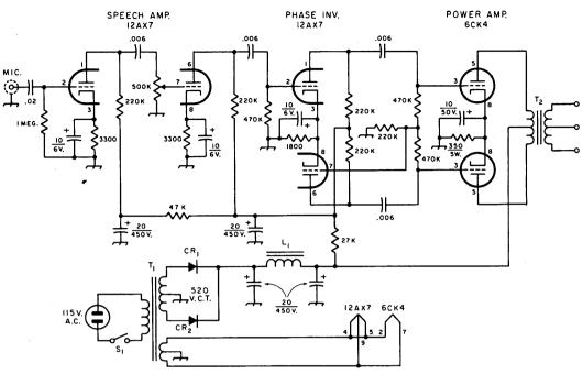
Fig. 8-7—Typical speech-amplifier driver for 5-10 watts output. Capacitances are in μf. Resistors are ½ watt unless specified otherwise. Capacitors with polarity indicated are electrolytic.
