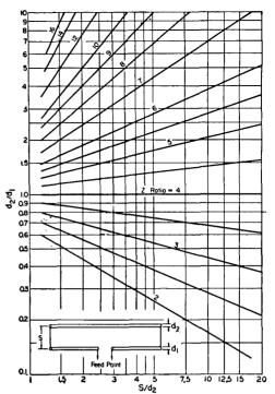
Fig. 14-36—Impedance transformation ratio, two-conductor folded dipole. The dimensions  $d_1$ ,  $d_2$  and s are shown on the inset drawing. Curves show the ratio of the impedance (resistive) seen by the transmission line to the radiation resistance of the resonant antenna system.
