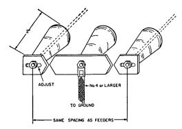
Fig. 22-1—A simple lightning arrester made from three stand-off or feed-through insulators and sections of ½x½-inch brass or copper strap. It should be installed in the open-wire or Twin-Lead line at the point where it is nearest the ground outside the house. The heavy ground lead should be as short and direct as possible. Gap setting should be minimum for transmitter power.
