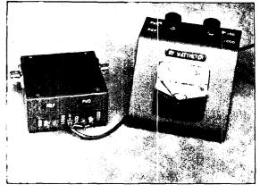
Fig. 21-52—Outside view of the power meter. The rf head is built in a  $4 \times 4 \times 2$ -inch utility box. A slopingpanel cabinet houses the controls and meter. A fourwire shielded cable joins the two pieces.
