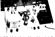
Fig. 8-15—A look at the top of the modulator chasis. The power supply is located on the right, the speech amplifier tubes are at the upper left, and the modulation transformer is at the lower left. The control relay, K<sub>1</sub>, is at the center of the chassis, just behind the meter.
