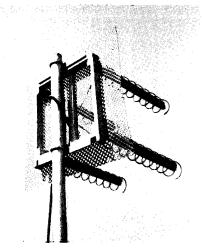
Fig. 18-14—An example of a 4-bay helical array cut for 1296-Mc. use. This stacked system offers approximately 6 db. more gain than a single bay is capable of providing. (Described in detail, QST, August 1963, by K6UQH.)
