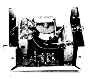
Fig. 5-39—Parts arrangement inside the filter cabinet. The toroids are held in place by a long 6-32 screw, a washer, and a 6-32 hex nut. There is nothing critical about the layout.
