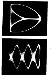
Fig. 11-7—Upper photo—Audio phase shift in coupling circuit between transmitter and horizontal deflection plates. Lower photo—Hum on vertical deflection plates.
