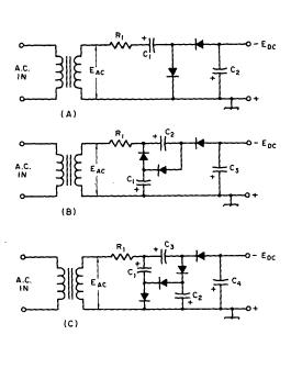
Fig. 12-19—Voltage-multiplying circuits with one side of transformer secondary grounded. (A) Voltage doubler (B) Voltage tripler (C) Voltage quadrupler.
