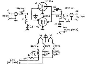
Fig. 17-34—Representative circuit of the 1296-Mc. cavity amplifier. The plate cavity and tuning device are indicated by  $L_2C_3$ , the cathode inductance and tuning capacitor by  $L_3C_2$ . Note that the heater supply must not be grounded.
