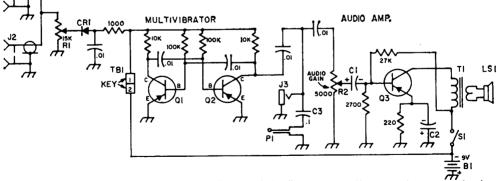
Fig. 40A—Circuit diagram of the cw monitor. Unless specified, all resistors are  $\frac{1}{2}$  watt; resistances are in ohms (K = 1000). All values of capacitors are in microfarads ( $\mu$ F, all 0.01- $\mu$ F capacitors are disk ceramic. Capacitors marked with polarity are electrolytic.
