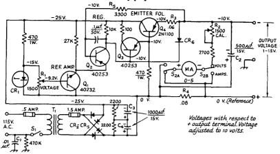
Fig. 12-38—Circuit of the transistor power supply. Resistances are in ohms; resistors are ½-watt, 10-percent tolerance, unless otherwise specified. Capacitors with polarity indicated are electrolytic; others are ceramic. Voltages shown are with respect to positive output terminal with R<sub>1</sub> adjusted for 10 volts output. Components not listed below are numbered for reference.
