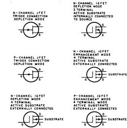
Fig. 4-23—Symbols for most-commonly available fieldeffect transistors.
