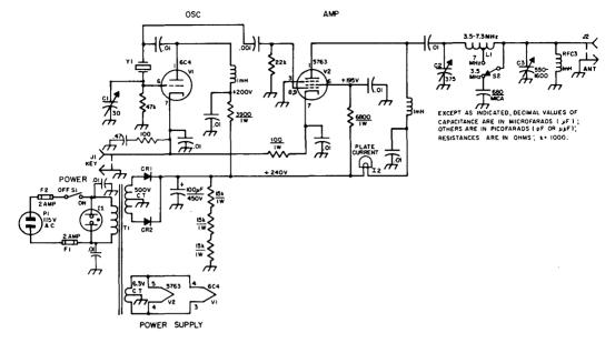
Fig. 6-40—Circuit of the Novice Special. Fixed-value capacitors are disk ceramic unless noted differently. Capacitors with polarity marking are electrolytic. Fixed-value resistors are ½-watt composition unless otherwise noted.
