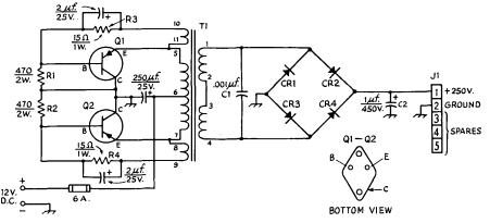
Fig. 19-28—Schematic diagram of the converter. Resistance is in ohms. Resistors are composition units. Polaritymarked capacitors are electrolytic. C<sub>1</sub> is a 1000-volt disk ceramic. CR<sub>1</sub>-CR<sub>4</sub>, inc., are 600 PRV, 750-mA top-hat rectifiers. Q<sub>2</sub> and Q<sub>2</sub> are 2N2869/2N301s. (2N376, 2N235A, or 2N1146 types are suitable). J<sub>1</sub> is a 5-pin female tube socket. T<sub>1</sub> is a Triad TY-78 transformer (Newark Electronics).
