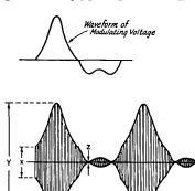
Fig. 8-21—Modulation by an unsymmetrical wave form. This drawing shows 100% downward modulation along with 300% upward modulation. There is no distortion, since the modulation envelope is an accurate reproduction of the wave form of the modulating voltage.
