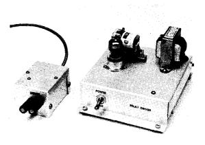
Fig. 7-12—The relay driver is at the right and is a self-contained unit. The smaller assembly at the left is the tape-recorder adaptor of Fig. 7-13B.
