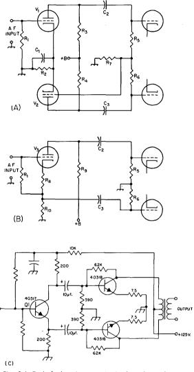
Fig. 8-4—Typical phase-inverter circuits for tube and transistor applications. V<sub>1</sub>, V<sub>2</sub>, and V<sub>3</sub> can be tubes such as the 12AX7, 12AT7, or 12AU7. Component values should be selected from the tube charts in the RCA Tube Manual and will depend on the frequency response and operating conditions needed.
