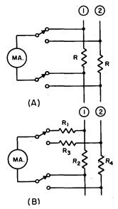
Fig. 6-32—Two circuits for switching a single milliammeter. (A) Where all currents are of the same order, the single meter is switched across resistors having 10 to 20 times the internal resistance of the meter. (B) Where a wide range of currents is to be metered, a low-current meter is used as a voltmeter.
