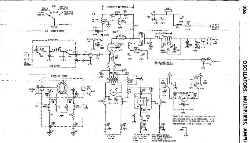
Fig. 6-71—Schematic diagram of the SS-70. Fixed-value capacitors are disk ceramic unless noted differently. Fixed-value resistors are 1/2-watt carbon unless otherwise indicated.
