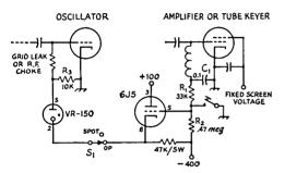
Fig. 7-7—When satisfactory blocked-grid or tube keying of an amplifier stage has been obtained, this VRtube break-in circuit can be applied to the transmitter to furnish differential keying. The constants shown here are suitable for blocked-grid keying of a 6146 amplifier; with a tube keyer the 6J5 and VR tube circuitry would be the same.
