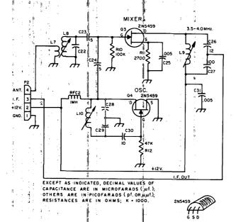
Fig. 5-51—Schematic diagram of the plug-in converters. These units can be used with any communications receiver that covers the 80-meter band. Capacitors are the disk ceramic unless marked S.M. (silver mica). Numbered components not listed below are for circuit-board layout identification.
