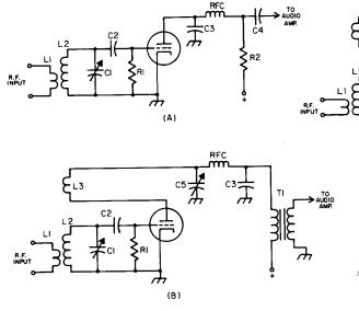
Fig. 5-7—(A) Triode grid-leak detector combines diode detection with triode amplification. Although shown here with resistive plate load,  $R_2$ , an audio choke coil or transformer could be used.
