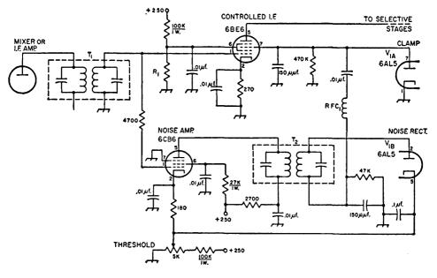
Fig. 5-21—Practical circuit diagram of an i.f. noise blanker. For best results the silencer should be used ahead of the high-selectivity portion of the receiver. T<sub>1</sub>—Interstage i.f. transformer
