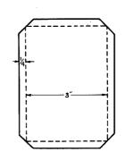
Fig. 16-30—Principal dimensions of the box, partitions and cover for the 432-Mc. amplifier. Material is 1/32-inch sheet brass, silver plated. Flat plates should be cut as shown then bent up along broken lines. Where precise bending cannot be done it is recommended that the cover be bent up to fit after the box is made. Hole sizes should be checked with available parts. Those shown are as follows:
