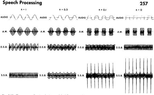
Fig. 9-10—The same audio signal gives widely-different envelope patterns, depending upon the type of transmitter. Various audio waveforms are shown in the top line; the resulting envelopes for 100 percent a.m., doublesideband suppressed carrier, and single-sideband suppressed carrier are shown below. The various audio waveforms are obtained by substituting values shown for n in sin<sup>n</sup> a.
