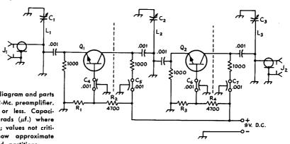
Fig. 16-28—Schematic diagram and parts information for the 432-Mc. preamplifier. Resistors are ½-watt or less. Capacitances are in microfarads (μf.) where shown on the diagram; values not critical. Broken lines show approximate positions of shield partitions.
