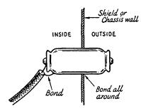
Fig. 23-12—The best method of using the "Hypass" type feed-through capacitor. Capacitances of 0.01 to 0.1  $\mu$ f. are satisfactory. Capacitors of this type are useful for high-current circuits, such as filament and 115-volt leads, as a substitute for the r.f. choke shown in Fig. 23-10, in cases where additional lead filtering is needed.
