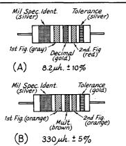
Fig. 20-7—Color coding for tubular encapsulated r.f. chokes. At A, an example of the coding for an 8.2-uh. choke is given. At B, the color bands for a 330-uh. inductor are illustrated.
