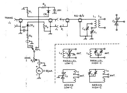
Fig. 13-18—Circuit diagram of the wide-range coupler. Capacitor  $C_8$  connects to  $L_2$  in several ways through use of clip leads. Similarly, the transmission line may be connected either to the outside of the inductor  $L_2$ (parallel tuning) or to the inside (series tuning).
