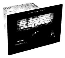
Fig. 6-46—The FET v.f.o. The panel is ½-inch aluminum, 7 by 10 inches. (Designed and built by G. D. Hanchett, W2YM.)
