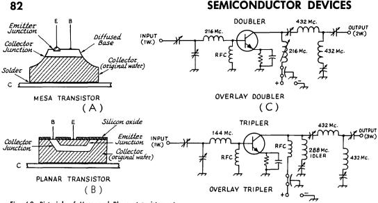
Fig. 4-9—Pictorials of Mesa and Planar transistors at A and B. At C and D, Overlay transistor frequency multipliers—a doubler and a tripler.
