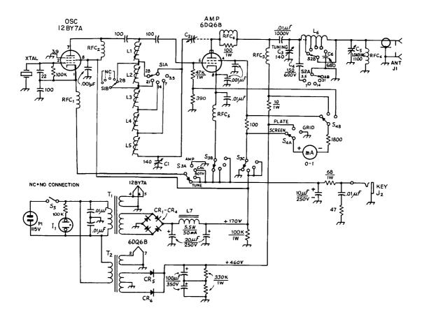
Fig. 6-42—Circuit diagram of the five-band 50 watter. Unless indicated otherwise, capacitances are in pf. and resistances are in ohms, ½-watt. Capacitors marked with polarity are electrolytic; capacitors with decimal value of μf. are disc ceramic.
