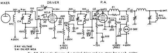
Fig. 9-9—Schematic diagram of a typical driver and p.a. stage for a s.s.b. exciter. Neutralization and parasitic-suppression circuits have been included.
