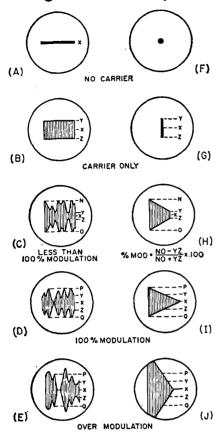
Fig. 11-3—Wave-envelope and trapezoidal patterns representing different conditions of modulation.
