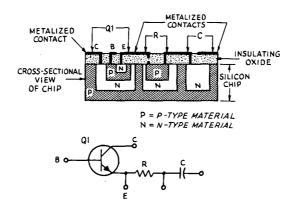
Fig. 4-26—Pictorial and schematic illustrations of a simple IC device.
