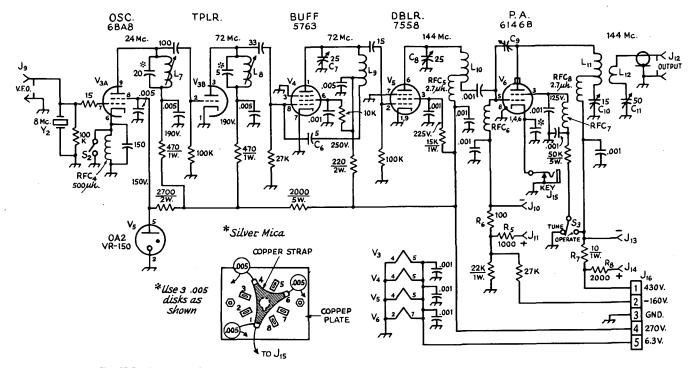
Fig. 17-7—The circuit of the 2-meter r.f section. Fixed-value capacitors are disc ceramic unless stated otherwise. Resistors are ½ watt composition unless noted differently.
