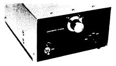
Fig. 5-44—Outside view of the three-band converter. The peaking control is at the top center, the band switch at the lower right, and the on-off switch and panel lamp are at the lower left. A home-made cabinet encloses the equipment, and the panel is painted gray to set off the white decal labels.
