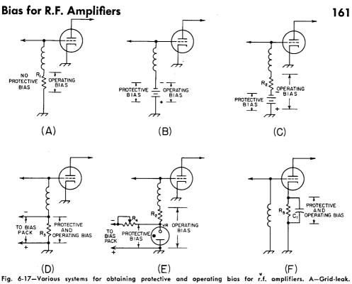
Fig. 6-17—Various systems for obtaining protective and operating bias for r.f. amplifiers. A—Grid-leak. B—Battery. C—Combination battery and grid leak. D—Grid leak and adjusted-voltage bias pack. E—Combination grid leak and voltage-regulated pack. F—Cathode bias.
