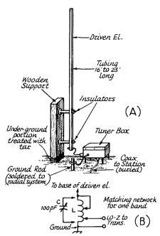
Fig. 14-26—Details for constructing a multiband vertical. A treated piece of  $2 \times 4$ -inch wood can be set in the ground and used as a support for the driven element. A weatherproof metal box houses the tuning network, and is located near the base of the vertical. A ground rod connects to the buried radials, and is also placed near the base of the antenna. At B, a schematic diagram of the tuning network required for
