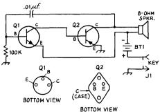
Fig. 1-2-Schematic diagram of the code oscillator. Resistance is in ohms. K = 1000. The 0.01-uf. capacitor is disk ceramic. BT1 is a 1.5-volt size-D flashlight cell. J<sub>1</sub> is a phono connector. Q<sub>1</sub> is an RCA 40309 (a 2N2102 is suitable also). Q2 is an RCA 2N2869/2N301. (An RCA 40022 is suitable, also). The cases of Q1 and Q<sub>2</sub> should be insulated from the chassis.
