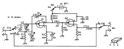
Fig. 5-42—Circuit diagram of the FET preselector. Resistances are in ohms; resistors are ½ watt. Fixed capacitors are disk ceramic. Circuit component designations not listed below are for etched circuit-board placement reference in QST.
