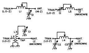
Fig. 13-11E—Networks for matching a lo-Z transmitter output to random-length end-fed wire antennas.
