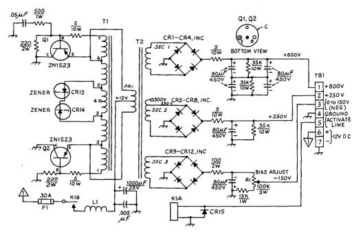
Fig. 12-41—Schematic diagram of the power supply. Polarized capacitors are electrolytic, others are paper or mica. Resistance is in ohms. K = 1000.
