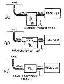
Fig. 5-29—Examples of series- and parallel-tuned single-frequency traps (installed) are shown at A and B. At C, FL1 represents the band-rejection filter described in the text. If possible, the filter used should be bolted to the chassis or case of the receiver. The receiver should have a good earth ground connected to it.
