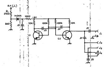
Fig. 6-45—Circuit diagram of the r.f.-powered keying monitor. Point marked "RF" connects to ungrounded lead of  $J_1$  (Fig. 6-42). This circuit can be used with any transmitter, simply by selecting an input resistor,  $R_1$ , that gives about —6 volts at the point shown.
