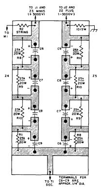
Fig. 12-36—Layouts for the circuit boards used at  $Z_2$  through  $Z_5$ . To assure good insulating properties highquality glass-epoxy board should be used.
