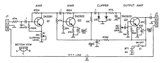
Fig. 8-19—Circuit diagram of the speech-amplifier/clipper. Capacitances are in pf. unless noted differently; capacitors with polarity indicated are electrolytic; 0.1-μf. capacitors are paper (Sprague 4PS-P10); 0.02-μf. capacitor is disk ceramic. Fixed resistors are ½-watt; resistances are in ohms (K = 1000).
