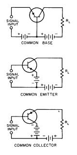
Fig. 4-12—Basic transistor amplifier circuits.  $R_L$ , the load resistance, may be an actual resistor or the primary of a transformer. The input signal may be supplied from a transformer secondary or by resistance-capacitance coupling. In any case it is to be understood that a d.c. path must exist between the base and emitter.
