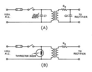
Fig. 12-29—Methods of suppressing line transients.
