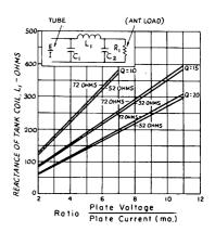
Fig. 6-14—Reactance of tank coil, L<sub>1</sub>, as a function of plate voltage and current, for pi networks.
