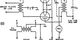
Fig. 8-5—Amplitude-modulator circuit diagrams. Tubes and circuit considerations are discussed in the text.
