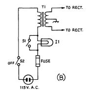
Fig. 12-28—The circuit at A shows how a 115-volt a.c. relay and a series dropping resistor,  $R_a$ , can provide surge protection while C charges. A simplified, manually-operated surge-protection system is shown at B. A switch and a light bulb provide protection to the rectifiers as C charges.
