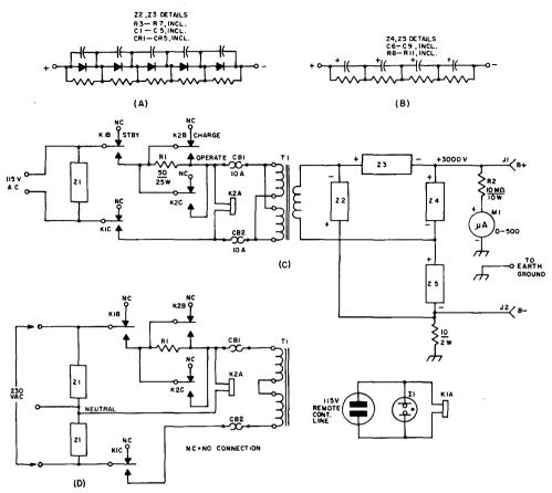
Fig. 12-37—Schematic diagram of the 3000-volt power supply. Capacitor used in assemblies Z<sub>2</sub> and Z<sub>3</sub> are 1000volt disk ceramic. The resistors in the two assemblies are ½-watt composition. Polarized capacitors are electrolytic.
