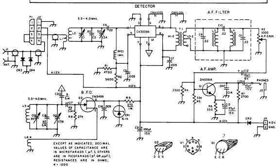
Fig. 5-49—Schematic diagram of the main portion of the Mark I. Capacitors with polarity marking are electrolytic. Other fixed capacitors are disk ceramic unless marked S.M. (silver mica). C<sub>0</sub>, C<sub>10</sub>, and C<sub>11</sub> are dipped polyester types. Fixed resistors are ½-watt composition unless noted otherwise. Component numbers not listed below are for identification purposes on the circuit board.
