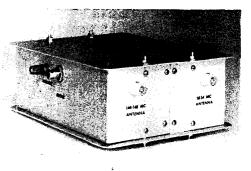
Fig. 16-7—The twin vhf converters are housed in a homemade aluminum box which has removable top and bottom covers for easy access to the circuit boards. Each converter has its own input and output jacks so that simultaneous operation is possible.
