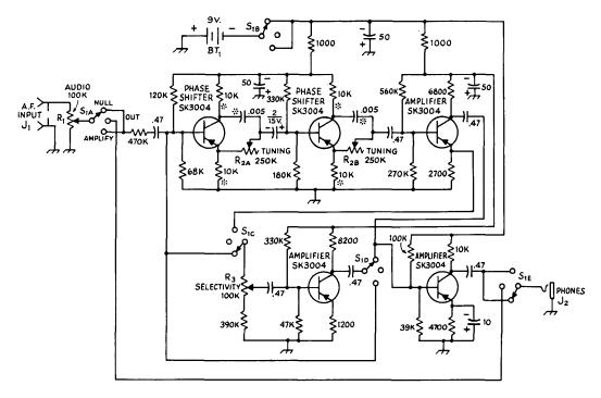
Fig. 5-36—Schematic diagram of Selectoject. Capacitors are rated 10 volts or better; those marked with polarity are electrolytic; capacitances are in microfarads ( $\mu$ f.) Unless specified otherwise, resistors are ½-watt, 10 per cent tolerance, resistances are in ohms. Resistors and capacitors marked with asterisk are matched as closely as possible.
