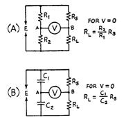
Fig. 21-46—Basic bridge circuits. (A) Resistance bridge;
