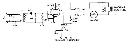
Fig. 10-4—Circuit diagram of the simple converter. The 100,000 ohm resistor is ½-watt composition, and the 0.02-μf. capacitor may be ceramic or Mylar type.
