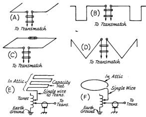
Fig. 14-40—Various configurations for small indoor antennas. A discussion of installation and tuning methods is covered in the text.
