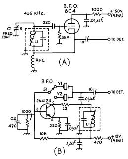
Fig. 5-16—B.f.o. circuits which are suitable for use with a.m. or product detectors of the type shown earlier. In the circuit at A,  $C_1$  varies the oscillator frequency above or below the i.f. to permit upper- or lower-sideband reception. *RFC* places the cathode above r.f. ground to provide feedback. A tap near the cold end of  $L_1$  could be used in place of the r.f. choke.
