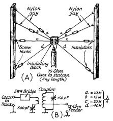
Fig. 14-18—Illustration of a multiband coax-fed antenna. Wooden support poles are recommended so that they will not interfere with the radiation pattern of the antenna. At B, a representative diagram of a coaxto-coax coupler that will reduce harmonic radiation from the system. It should be installed in the operating room, near the transmitter, and adjusted for a 1:1 SWR.
