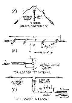
Fig. 14-28—Illustrations of three vertically-polarized short antennas for use on 1.8 to 2 MHz. They arc described in the text.
