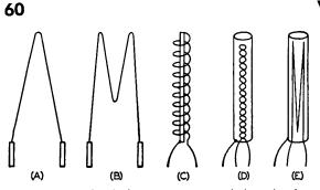
Fig. 3-2—Types of cathode construction. Directly heated cathodes or "filaments" are shown at A, B, and C. The inverted V filament is used in small receiving tubes, the M in both receiving and transmitting tubes. The spiral filament is a transmittingtube type. The indirectly-heated cathodes at D and E show two types of heater construction, one a twisted loop and the other bunched heater wires. Both types tend to cancel the magnetic
