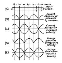
Fig. 13-2—Standing waves of voltage and current along short-circuited transmission line.
