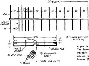
A folded-dipole driven element is employed and is designed to provide a feedpoint impedance of approximately 200 ohms. A 4:1 balun is used to step the impedance down to 50 ohms, unbalanced, so that coaxial feed line can be used. A 1:1 match can be secured by using a universal matching stub in the same fashion as described for the 2-meter Yagi.
