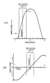
Fig. 5-35—F.m. or p.m. detection characteristics. A— "Slope detection," using the sloping side of the receiver's selectivity curve to convert f.m. or p.m. to a.m. for subsequent rectification. B—Typical discriminator characteristic. The straight portion of this curve between the two peaks is the useful region. The peaks should always lie outside the pass band of the receiver's selectivity curve. RFC<sub>1</sub>—High reactance at i.f.  $V_1$ —Sharp-cutoff pentode.  $V_2$ —Dual diode (6AL5).
