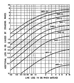
Fig. 13-9—Effect of standing-wove radio on line loss. The ordinates give the additional loss in decibels for the loss, under perfectly matched conditions, shown on horizontal scale.
