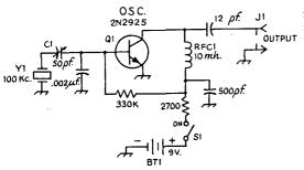
Fig. 21-11—Circuit of the 100-Kc. frequency standard. Resistances are in ohms. Resistors are ½ watt. K-1000. BT<sub>1</sub>—9-volt transistor radio battery.
