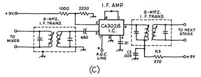
Fig. 5-15—Examples of typical i.f. amplifiers. A vacuum-tube circuit is given at A; B shows a bipolar transistor i.f. amplifier which has been neutralized; C illustrates how an integrated circuit can be used as a high-gain i.f. stage. All three circuits are shown with a.g.c. provisions. R<sub>1</sub> through R<sub>3</sub>, and C<sub>1</sub> through C<sub>3</sub> in all circuits serve as r.f. decoupling networks to prevent instability from interstage power-lead coupling.
