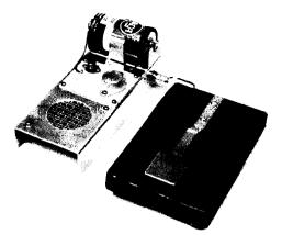
View of the code-practice set. The speaker mounts under the chassis and is protected by a piece of aluminum screening. Ordinary window screen will work here. The circuit board is mounted over a cut-out area in the chassis. Allow a ¼-inch overlap on all sides of the circuit board for mounting purposes. Four 4-40 bolts hold the board in place. The battery holder is a Keystone No. 175.
