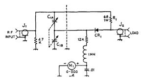
Fig. 21-57—Circuit of the impedance bridge. Resistors are composition, ½ watt except as noted. Fixed capacitors are ceramic.
