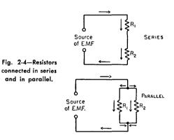
variety of ways. The two fundamental methods of connecting resistances are shown in Fig. 2-4. In the upper drawing, the current flows from the source of e.m.f. (in the direction shown by the arrow, let us say) down through the first resistance,  $R_1$ , then through the second,  $R_2$ , and then back to the source. These resistors are connected in **series**. The current everywhere in the circuit has the same value.
