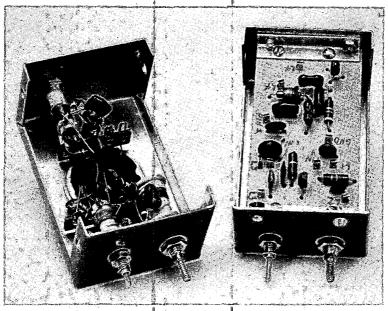
Fig. 5-50—Photo of two of the plug-in converters showing how point-to-point wiring compares to etchedcircuit construction. The converters are built in 31/4 imes 1% imes 2½-inch Miniboxes. The three slug-tuned coils mount on the ends of the boxes. In the circuitboard version, the coils are below the board.
