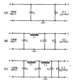
Fig. 12-5.—Capacitive-input filter circuits. A—Simple capacitive. B—Single-section. C—Double-section.
