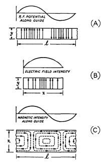
Fig. 2-63—Field distribution in a rectangular waveguide. The  $TE_{1,0}$  mode of propagation is depicted.
