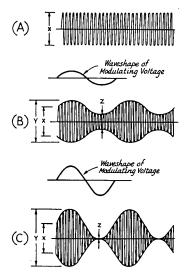
Fig. 8-20—Graphical representation of (A) r.f. output unmodulated, (B) modulated 50%, (C) modulated 100%. The modulation envelope is shown by the thin outline on the modulated wave.
