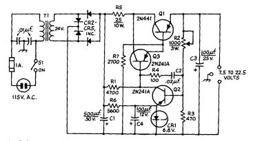
Fig. 12-25—Circuit of the improved regulator. Resistance is in ohms. Fixed-value resistors are ½-watt composition unless otherwise noted. Polarized capacitors are electrolytic. CR<sub>1</sub> is a 1N754 Zener diode, or equal. CR<sub>2</sub>-CR<sub>5</sub>, incl., are 1N191s or equiv. T<sub>1</sub> is a 24-volt, 1-ampere transformer.
