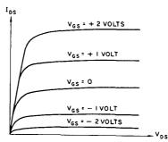
Fig. 4-22—Typical IGFET characteristic curves.
