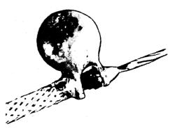
Fig. 23-9—Proper method of bypassing the end of a shielded lead using disk ceramic capacitor. The 0.001- $\mu$ f, size should be used for 1600 volts or less; 500  $\mu\mu$ f, at higher voltages. The leads are wrapped around the inner and outer conductors and soldered, so that the lead length is negligible. This photograph is about four times actual size.
