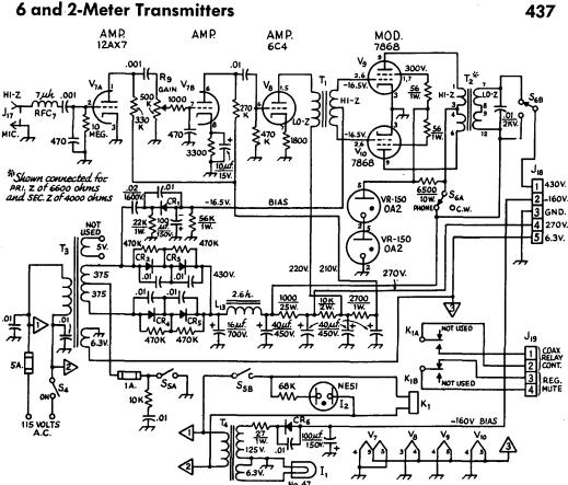
Fig. 17-8—Schematic diagram of the power supply and 30-watt modulator. Capacitors are disc ceramic. Those bearing polarity marking are electrolytic. Resistors are ½ watt composition unless noted otherwise.
