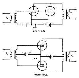
Fig. 3-12—Parallel and push-pull a.f. amplifier circuits.
