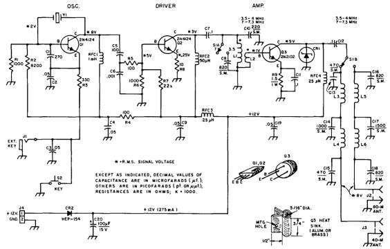
Fig. 6-36—Schematic diagram of the QRP transmitter. Except as specified, fixed-value capacitors are low-voltage disk ceramic; polarized capacitors are electrolytic; SM = silver mica. Resistors are ½-watt composition. Voltages marked with an asterisk are rms rf (see text). Component identifiers not appearing in the parts list are for identification purposes on the etched-circuit board layout.
