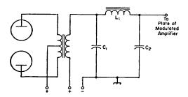
Fig. 8-11—Splatter-suppression filter for use at high level.
