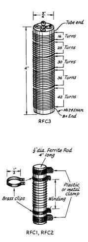
Fig. 6-63—Details for winding the plate choke, RFC<sub>8</sub>. Sketch also shows how RFC<sub>1</sub> and RFC<sub>2</sub> are assembled.
