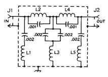
Fig. 5-28—Capacitance is in  $\mu$ f. Capacitors are disk or tubular ceramic.
