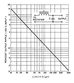
Fig. 12-12—Graph showing combinations of inductance and capacitance that may be used to reduce 120-Hz. rîpple with a single-section choke-input filter.
