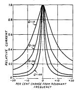
Fig. 2-39—Current in series-resonant circuits having different Qs. In this graph the current at resonance is assumed to be the same in all cases. The lower the Q, the more slowly the current decreases as the applied
