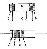
Fig. 20-6—Color coding of fixed composition resistors. The color code is given in Table 20-111. The colored areas have the following significance:
