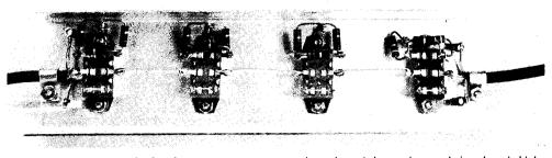
Fig. 5-31—Resistor networks for the attenuator are mounted on the switches and grounded to lugs held by the switches. Note that outer conductor of coaxial cable is fanned out and grounded either side of switch.
