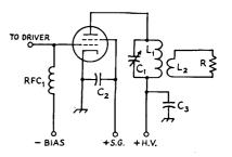
Fig. 6-10-Inductive-link output coupling circuits.
