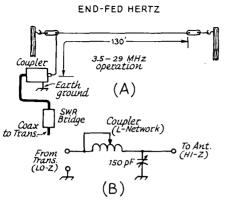
Fig. 14-22—Diagram of an end-fed Hertz. It is cut for the lowest desired operating frequency (½ wavelength), and is operated on its harmonic frequencies on the remaining bands above. An L-network is used to match it to 50- or 75-ohm unbalanced transmitter terminals. At B, schematic representation of an L-network tuner. The value of L and C is adjusted until a 1:1 match is obtained.
