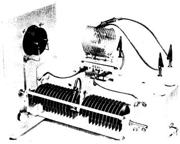
Fig. 13-19—The coupler is built on a 13 X 5 X 3-inch aluminum chassis. The front panel is 8 X  $10\frac{1}{2}$  inches. Split-stator C<sub>3</sub> is supported on 1-inch ceramic cone insulators, and the four alligator clips that take the transmission line are mounted on  $1\frac{1}{2}$ -inch cone insulators. Note clip lead connected to split-stator capacitor rotor connection: this can be connected to lug on chassis or to one side of L<sub>2</sub>.
