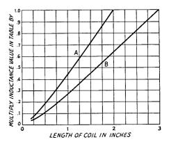
Fig. 2-15—Factor to be applied to the inductance of coils listed in the table below, as a function of coil length. Use curve A for coils marked A, curve B for coils marked R
