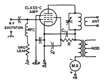
Fig. 8-25—Plate and screen modulation of a Class C r.f. amplifier using a screen-grid tube. The plate r.f. bypass capacitor, C<sub>1</sub>, should have reasonably high reactance at all audio frequencies; a value of 0.001 to 0.005  $\mu$ f. is generally satisfactory. The screen bypass, C<sub>2</sub>, should not exceed 0.002  $\mu$ f. in the usual case.
