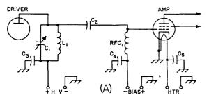
Fig. 6-21—Capacitive-coupled amplifiers. A—Simple capacitive coupling. B—Pi-section coupling.
