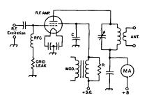
Fig. 8-28—Screen-grid modulation of beam tetrode. Capacitor C is an r.f. bypass capacitor and should have high reactance at audio frequencies. A value of 0.002  $\mu$ f. is satisfactory. The grid leak can have the same value that is used for c.w. operation of the tube.
