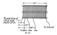
Fig. 22-5—Drawing of  $L_1$  and associated taps.  $L_1$ is 44 turns of No. 24, 32 turns per inch, 1 inch diameter (Miniductor 3016, Air Dux 832T). To solder the tap leads, indent each turn adjacent to the tap point. This will allow soldering room.
