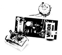
Fig. 5-41—At the left, on the circuit board, is the input coil combination  $L_1$  and  $L_2$ . At the lower left is the mounting bracket for the two modified compression trimmers,  $C_1$  and  $C_2$ . Just to the right of the coil assembly is  $C_3$ .
