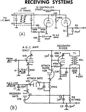
Fig. 5-18—Delayed automatic gain-control circuit using two diodes (A); B shows audio "hang" a.g.c. developed by W1DX. If manual control of gain is in i.f. and r.f. cathode circuits, point "A" is connected to chassis ground. If a negative supply is available, manual gain control can be negative bias applied between point "A" and ground.
