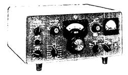
The 32S-3 operates in SSB or CW modes with 175 watts PEP input from 3.4 to 5.0 MHz and from 6.5 to 30.0 MHz. Supplied crystals cover the 80-, 40-, 20-, and 15-meter bands, and 200 kHz of the 10-meter amateur band, with provision for two more crystals. Features include mechanical filter sideband generation, permeability-tuned VFO and crystal-controlled HF oscillator.
