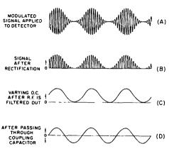
Fig. 5-3—Diagrams showing the detection process.
