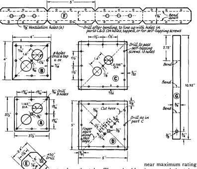
Fig. 17-36—Principal sheetmetal parts of the 1296-Mc. amplifier: top plate of the bypass capacitor, A; its bottom plate and top cover of the plate cavity, B; top plate of the cathode assembly, C; and two-piece bottom cover, D. The long strip, F, is the side walls of the cathode assembly, and G is the side walls of the plate cavity, both before bending into their square shape.
