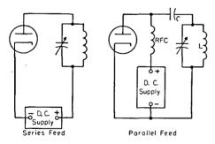
Fig. 2-57—Illustrating series and parallel feed.
