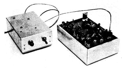
model when a signal-frequency resonance developed in the circuit board, causing an oscillation problem. Looking at the layout drawing of the circuit board pick out the 12-volt bus that runs from near the middle of the board horizontally to the right, before dropping vertically into the lower half. This should be severed below the letter "A" on the sketch. The 100-ohm  $R_2$ is bridged across the gap.
