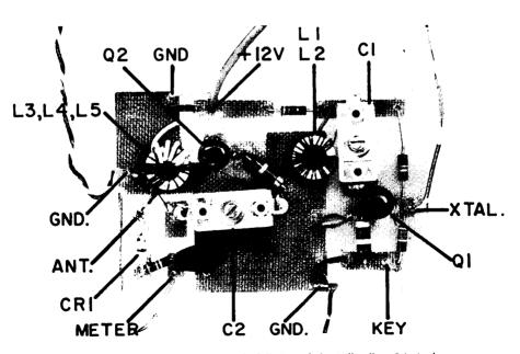
Fig. 19-48-Plan-view photograph, full size, of the Milligallon. Principal components are identified in this view as an aid to assembly; ones not labeled can easily be recognized by referring to Fig. 19-49. The dark areas are copper backing on the opposite side of the translucent circuit board and correspond (reversed left to right) to the layout shown in Fig. 19-51. (Designed and built by W7ZOI.)
