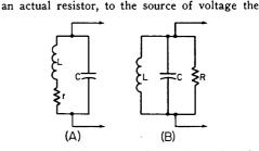
Fig. 2-41—Series and parallel equivalents when the two circuits are resonant. The series resistance, r, in A is replaced in B by the equivalent parallel resistance  $(R \equiv X_{\rm C}^2/r \equiv X_{\rm L}^2/r) \text{ and vice versa.}$
