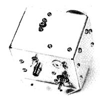
Fig. 6-51—View of the back side of the v.f.o. A phono connector is used as an output jack. A feedthrough capacitor is used as a B-plus connector, and is located just above the output jack. L<sub>1</sub> is mounted to the right of J<sub>1</sub>, just below trimmer capacitor C<sub>6</sub>. Trimmer capacitor  $C_7$  is accessible from the top of the case.
