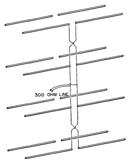
Fig. 18-11—Schematic of a 16-element collinear array. An adjustable matching stub, Fig. 18-2, can be attached at the feed point if precise matching is desired. Reflector-to-director spacing is 0.2 wavelength.
