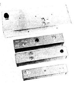
Fig. 23-24—High-Q strip-line filters for 50 Mc. (top), 220, 144 and 420 Mc. Those for the two highest bands are half-wave line circuits. All use standard chassis.
