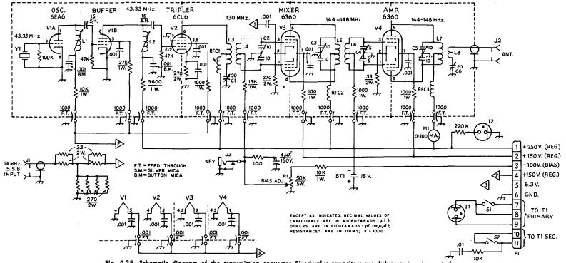
Fig. 9-35—Schematic diagram of the transmitting converter. Fixed-value capacitors are disk ceramic unless noted.
