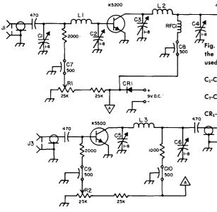
Fig. 16-25—Circuit diagram and parts information for the preamplifier stages. The upper portion should be used for a signal stage. Capacitor values are given in pf.
