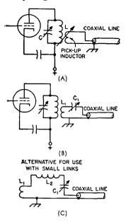
Fig. 6-11—With flat transmission lines, power transfer is obtained with looser coupling if the line input is tuned to resonance.  $C_1$  and  $L_1$  should resonate at the operating frequency. See table for maximum usable value of  $C_1$ . If circuit does not resonate with maximum  $C_1$  or less, inductance of  $L_1$  must be increased, or added in series at  $L_2$ .
