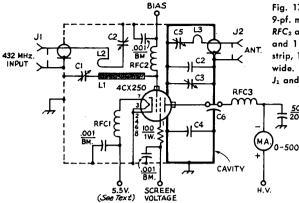
Fig. 17-30—Schematic of the amplifier.  $C_1$  and  $C_2$  are 9-pf. miniature variables (Johnson 160-104). RFC<sub>1</sub> and RFC<sub>2</sub> are each 8 turns of No. 16 enam., ½ inch diameter and 1 inch long. RFC<sub>3</sub> is a 1.4-uh. choke.  $L_1$  is a brass strip, 1/16 inch thick, 3-7/8 inches long, and 1¼ inches wide.  $L_2$  is a loop of No. 12 wire, 6 inches overall.  $J_1$  and  $J_2$  are type-N chassis connectors. B.M. == button mica.
