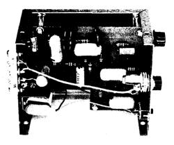
Fig. 8-18—Inside view showing the etched circuit board. The clipper diodes are near the upper edge of the board in this view.  $Q_3$  is at the left,  $Q_2$  is at the right, and  $Q_1$  is below  $Q_2$  with a paper capacitor in between.
