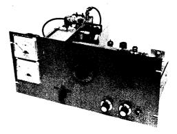
Fig. 17-9—The 220-MHz transmitter is set up for rack mounting on 8¾-inch panel. Meters at the left can be switched to read driver plate, amplifier screen and amplifier plate currents, and amplifier plate voltage.
