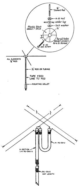
likely to shatter in cold weather. The elements can be fashioned from 1/2-inch diameter aluminum rods, but brass is more durable and is better able to withstand stress. Brass brazing rod is available from most automotive parts houses, or from welding shops, and is excellent material for turnstile elements. No. 10 copper weld wire also works well and is virtually indestructible.
