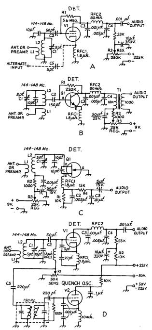
transistor such as a 2N3932. Q<sub>1</sub> at C should be a hightransconductance junction FET designed for v.h.f. use. The sensitivity of these detectors, at the frequency indicated, is such that a 30-percent modulated 0.5-uv. signal should be perfectly discernible when the output from the detectors is fed into a conventional audio channel. Capacitance is in pf. except decimal-value capacitances which are in  $\mu$ f. Polarized capacitors are
