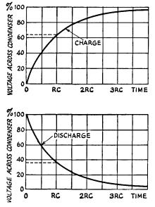
Fig. 2-20—How the voltage across a capacitor rises, with time, when charged through a resistor. The lower curve shows the way in which the voltage decreases across the capacitor terminals on discharging through the same resistor.
