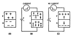
Fig. 4-1—A p-n junction (A) and its behavior when conducting (B) and non-conducting (C).
