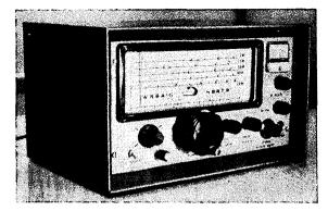
Fig. 5-58—Front view of the HB-70 receiver. An Eddystone tuning dial is used on this model. An S meter is visible at the upper right, but is not connected into the circuit. Various methods for employing an S meter are shown earlier in the chapter. They can
