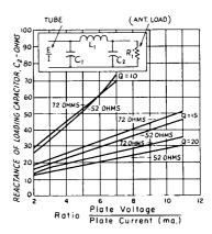
Fig. 6-15—Reactance of loading capacitor, C<sub>2</sub>, as a function of plate voltage and current, for pi networks.
