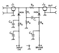
Fig. 21-47—Bridge circuit for s.w.r. measurements. This circuit is intended for use with a d.c. voltmeter, range 5 to 10 volts, having a resistance of 10,000 ohms
