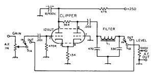
Fig. 8-9—Circuit of a typical vacuum-tube speech clipper.
