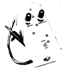
Fig. 9-22—The completed VOX unit. It goes between the microphone and the transmitter. The miniature knobs are Johnson Collet type 116-603.
