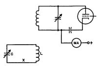
Fig. 21-9—Absorption frequency meter and a typical application. The meter consists simply of a calibrated resonant circuit LC. When coupled to an amplifier or oscillator the tube plate current will rise when the frequency meter is tuned to resonance. A flashlight lamp may be connected in series at X to give a visual indication, but it decreases the selectivity of the instrument and makes it necessary to use rather close coupling to the circuit being measured.
