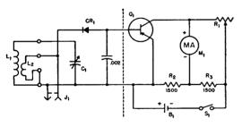
Fig. 21-45—Transistor d.c. amplifier applied to the wavemeter of Fig. 21-10 to increase sensitivity. Components not listed below are the same as in Fig. 21-10. B<sub>1</sub>—Small flashlight cell.
