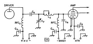
C1-Driver plate tank capacitor-see text and Fig. 6-9 for capacitance, Fig. 6-33 for voltage rating. C2-Coupling capacitor-50 to 150 pf. mica, as necessary for desired coupling. Voltage rating sum of driver plate and amplifier biasing voltages, plus safety factor.
