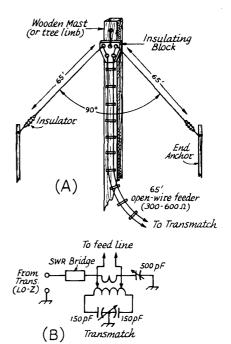
Fig. 14-14—Details for an Inverted-V antenna (sometimes called a "drooping doublet"). At A, a wooden mast supports the antenna at its center. Open wire feeders permit the antenna to be used for multiband operation. If this is done, a Transmatch of the type shown at B should be used to tune the system to resonance, and to match the feeder to the transmitter and receiver.
