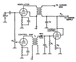
Fig. 8-29—Circuit for carrier control with screen modulation. A small triode such as the 6C4 can be used as the control amplifier and a 6Y6G is suitable as a carrier-control tube.  $T_1$  is an interstage audio transformer having a 1-to-1 or larger turns ratio.  $R_4$ is a 0.5-megohm volume control and also serves as the grid resistor for the modulator. A germanium crystal may be used as the rectifier. Other values are discussed in the text.
