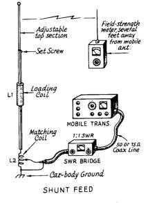
Fig. 19-9—A mobile antenna using shunt-feed matching. Overall antenna resonance is determined by the combination of  $L_1$  and  $L_2$ . Antenna resonance is set by pruning the turns of  $L_1$ , or adjusting the top section of the whip, while observing the field-strength meter or SWR bridge. Then, adjust the tap on  $L_2$  for lowest SWR.
