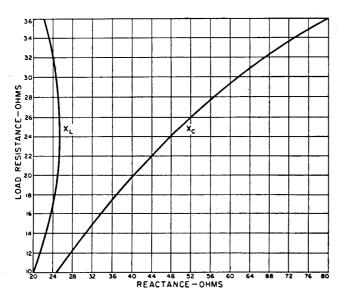
Fig. 19-12—Curves showing inductive and capacitive reactances required to match a 50-ohm coax line to a variety of antenna resistances.
