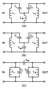
Fig. 2-46-Three methods of circuit coupling.
