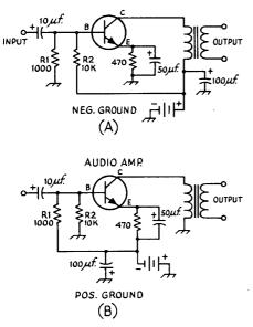
Fig. 4-14—Changing the circuit polarity.
