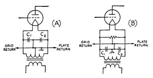
Fig. 3-18—Filament center-tapping methods for use with directly heated tubes.
