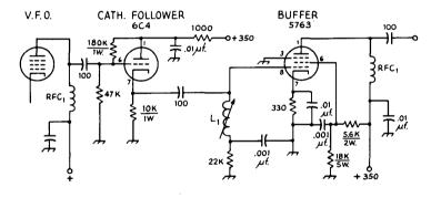
Fig. 6-6—Circuit of an isolating amplifier for use between v.f.o. and first tunable stage. Unless otherwise specified, all capacitances are in picofarads, all resistors are ½ watt. L<sub>1</sub>, for the 3.5-Mc. band, consists of 100-140 μh. adjustable inductor. RFC<sub>1</sub> is 100 μh. All capacitors are disk ceramic.
