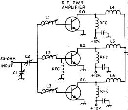
Fig. 4-16-Current-equalization method.
