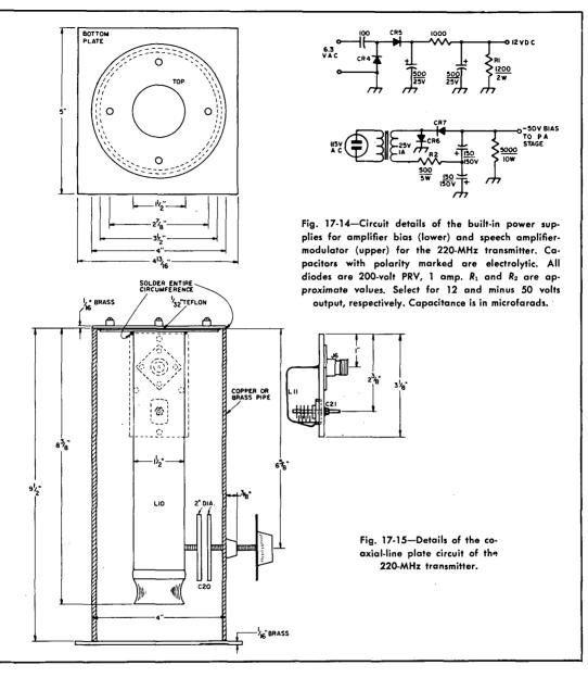
the exciter. Procedure here is like that for any similar lineup of tubes, but the 2E26 must be adjusted for optimum results when working into a 52-ohm load. Once an output of 10 to 12 watts is obtained in this way, leave the tuning of the 2E26 and preceding stages alone thereafter.
