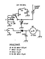
Fig. 19-32—A band-switched field-strength meter for tuning up the hf-band mobile antenna. It should be assembled in a metal box. In use, it should be placed several feet from the antenna under test.  $C_1$  is tuned for a peak meter reading at the operating frequency. It can be detuned for varying the sensitivity.
