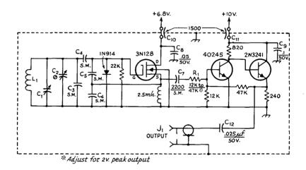
Fig. 6-47—Circuit diagram of the variable-frequency oscillator and buffer. Except as indicated, capacitances are in pf. ( $\mu\mu$ f.). Resistances are in ohms (K = 1000); resistors are ½-watt composition.
