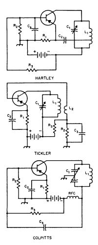
Fig. 4-17—Typical transistor oscillator circuits. Component values are discussed in the text.
