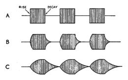
Fig. 7-1—Typical oscilloscope displays of a code transmitter. The rectangular-shaped dots or dashes (A) have serious key clicks extending many kc. either side of the transmitter frequency. Using proper shaping circuits increases the rise and decay times to give signals with the envelope form of B. This signal would have practically no key clicks. Carrying the shaping process too far, as in C, results in a signal that is too "soft" and is not quite as easy to copy as B.
