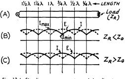
Fig. 13-4—Standing waves on a transmission line terminated in a resistive load.
