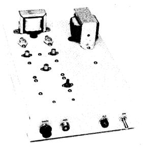
Fig. 8-12—Top view of the modulator chassis. The audio section is mounted along the left side of the chassis.  $T_2$  is mounted at the left rear. The power supply is located at the right rear of the chassis with the core of  $T_8$  mounted at right angles to that of  $T_2$  to avoid hum pick-up.
