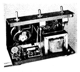
Fig. 21-30—Power supply for the noise generators is housed in a 7-inch wide sloping-panel cabinet (Bud AC-1613). Switches, from left to right, are (referring to Fig. 21-25) S<sub>8</sub>, S<sub>1</sub> and S<sub>2</sub>.
