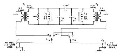
Fig. 5-40—Schematic of the audio filter. Capacitors are paper. The 560-ohm resistor is a ½-watt composition unit, and need not be included in the circuit. It was added experimentally to prevent "ringing," a condition that will not occur under normal circumstances.
