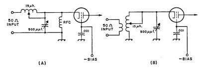
Fig. 6-28 shows two methods of coupling a grounded-grid amplifier to the 50-ohm output of an existing transmitter. At A an L network is used, while a conventional link-coupled tank is shown at B. The values shown will be approximately correct for most triode amplifiers operating at 3.5 Mc. Values should be cut in half each time frequency is doubled, i.e., 250 pF and 7.5  $\mu$ h. for 7 Mc., etc.
