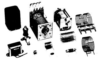
Inductors for power and radio frequencies. The two iron-core coils at the left are "chokes" for power-supply filters. The mounted air-core coils at the top center are adjustable inductors for transmitting tank circuits. The "pie-wound" coils at the left and in the foreground are radio-frequency choke coils. The remaining coils are typical of inductors used in r.f. tuned circuits, the larger sizes being used principally for transmitters.
