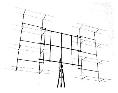
Fig. 18-12—Two 16element collinear arrays spaced 1% wavelength apart and fed in phase.
