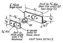
Fig. 19-43—Details of the homemade heat sink for  $Q_2$ . The assembly is mounted on insulating washers or rubber grommets to prevent a short circuit from collector to chassis. The hole in the angle stock is just large enough to permit  $Q_2$  to fit snugly. A thin layer of silicone grease will help transfer heat from case of  $Q_2$  to the heat sink.
