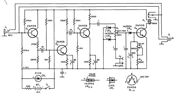
Fig. 9-23—Circuit diagram of the VOX unit. Capacitances are in μf.; resistances are in ohms; K = 1000. Resistors are ½-watt. Capacitors with polarity marking are electrolytic.
