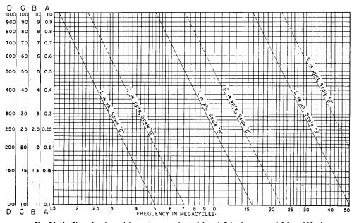
Fig. 21-41—Chart for determining unknown values of L and C in the range of 0.1 to 100 μh. and 2 to 1000 μμf., using standards of 100 μμf. and 5 μh.
