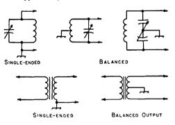
Fig. 2-59—Single-ended and balanced circuits.
