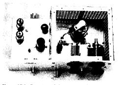
Figure 17-1—Top view of the 6-meter r.f. deck. The VR tubes are at the upper left,  $V_1$  is to the right of them, and the tuning knob for  $C_1$  is just above  $V_1$ . The 61468 p.a. and its plate tank are enclosed in the shielded area at the right.
