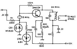
Fig. 8-33—Schematic of a transistor oscillator whose frequency is "pulled" by means of a variable-capacitance diode to obtain f.m.  $R_1$  is an r.f. isolating resistor.  $CR_1$  is a small Varactor diode. In some circuits a high-frequency small-signal silicon diode (or v.h.f. silicon transistor) is used for this same purpose.  $CR_2$  is a Zener diode.
