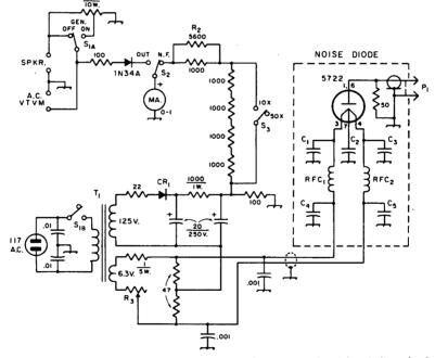
Fig. 21-28—Circuit diagram of the diode noise generators and power supply. Unless indicated otherwise, resistances are in ohms, resistors are ½-watt, capacitances are in μf.
