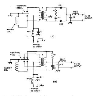
Fig. 19-25—Basic types of vibrator power supplies. A-Nansynchronous. B—Synchronous.
