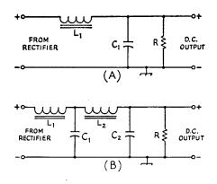
Fig. 12-10—Choke-input filter circuits. A—Single-section. B—Double-section.
