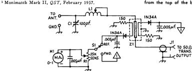
Fig. 13-21—Schematic of the tuner.  $C_1$  is an E. F. Johnson 154-14 variable.  $L_1$  is an Air Dux (Illumitronics) 2007A inductor consisting of 24 turns of No.-12 wire. It is 2½ inches in diameter and is 3¼ inches long. S1 is a s.p.d.t. wafer switch.  $R_1$  is a 25,000-ohm linear-taper carbon control.  $Z_1$  is a Monimatch-type s.w.r. bridge (see text). J<sub>1</sub> is an SO-239-type coax connector.
