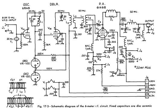
Fig. 17-3—Schematic diagram of the 6-meter r.f. circuit. Fixed capacitors are disc ceramic unless otherwise noted. Resistors are ½ watt composition unless specified differently.
