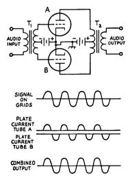
Fig. 3-13-Class B amplifier operation.
