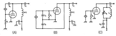
Fig. 6-2—Simple crystal oscillator circuits. A—Pierce. B—Equivalent of circuit A. C—Simple triode oscillator. C1 is a plate blocking capacitor, C2 an output coupling capacitor, and C3 a plate bypass. C4 and C5 are discussed in the text. C6 and L1 should tune to the crystal fundamental frequency. R1 is the grid leak.
