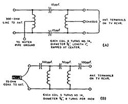
Fig. 23-29—High-pass filters for installation at the TV receiver antenna terminals. A—balanced filter for 300ohm line, B—for 75-ohm coaxial line. Important: Do not use a direct ground on the chassis of a transformerless receiver. Ground through a 0.001-μf, mica capacitor.
