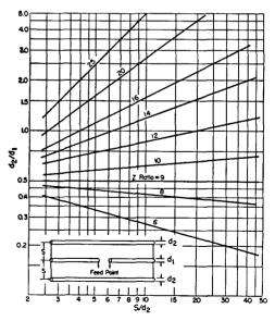
Fig. 14-37—Impedance transformation ratio, three-conductor folded dipole. The dimensions  $d_1$ ,  $d_2$  and s are shown on the inset drawing. Curves show the ratio of the impedance (resistive) seen by the transmission line to the radiation resistance of the resonant antenna system.
