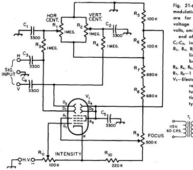
Fig. 21-63-Oscilloscope circuit for modulation monitoring. Constants are for 1500- to 2500-volt highvoltage supply. For 1000 to 1500 volts, omit R<sub>8</sub> and connect the bottom
