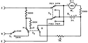
Fig. 21-43—Circuit diagrams of the transistor tester. Resistors are  $\frac{1}{2}$  watt. B<sub>1</sub>—Two C cells connected in series M<sub>1</sub>—O-1 milliameter (Lafayette 99 C 5052) S<sub>1</sub>, S<sub>2</sub>, S<sub>3</sub>—D.p.d.t. miniature slide switch
