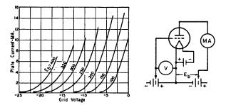
Fig. 3-6—Grid-voltage-vs.-plate-current curves at various fixed values of plate voltage (E<sub>b</sub>) for a typical small triode. Characteristic curves of this type can be taken by varying the battery voltages in the circuit at the right.
