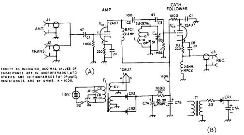
Fig. 22-4—Circuit diagram of the t.r. switch. Unless otherwise specified, resistors are ½ watt; decimal value fixed capacitors are disk ceramic, others are mica with the exception of C<sub>1</sub>, which is electrolytic. B—method of using a half-wave transformer for T<sub>1</sub>. Circuit designations not listed below are for text reference.
