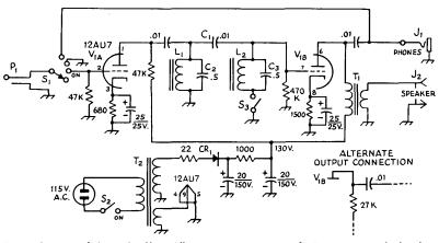
Fig. 5-38—Circuit diagram of the audio filter. All capacitances are in μf. Capacitors marked wth polarity are electrolytic. Resistances are in ohms; all resistors are ½-watt.
