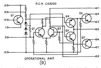
Fig. 4-27—At A, a representative circuit for a typical differential IC. An Operational Amplifier IC is illustrated at B, also in representative form.
