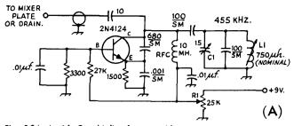
Fig. 5-24—An i.f. Q-multiplier for use with a bipolar transistor (A). At B, a tube-type r.f. Q-multiplier which can be used at the first stage of the receiver. The antenna coil is used for feedback to V<sub>1</sub>, which then introduces "negative resistance" to L<sub>2</sub>.
