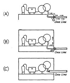
Fig. 23-19—Right (B) and wrong (A and C) ways to connect a coaxial line to the transmitter. In A or C, harmonic energy coupled by stray capacitance to the outside of the cable will flow without hindrance to the antenna system. In B the energy cannot leave the shield and can flow out only through, not over, the cable.
