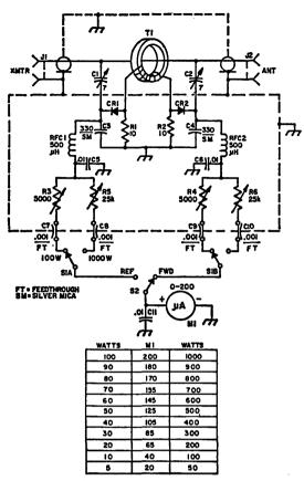
Fig. 21-53—Schematic diagram of the power wattmeter. A calibration scale for  $M_1$  is shown. Fixedvalue resistors are ½-watt composition. Fixed-value capacitors are disk ceramic unless otherwise noted. Decimal-value capacitances are in  $\mu$ F. Others are pF. Resistance is in ohms; k = 1000.
