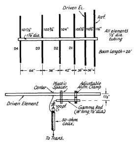
Fig. 18-5—Dimensions for the 50-Mc. array.  $C_1$  should be mounted in a weatherproof box, as near to the gamma rod as possible. The shield braid of the coax cable is grounded to the center of the driven element.
