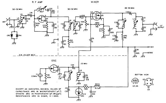
Fig. 16-9—Circuit diagram of the 6-meter converter. Resistors are ½-watt composition. Capacitors are disk ceramic unless specified differently. Numbered components not appearing in the parts list were so identified for circuit-board layout purposes.
