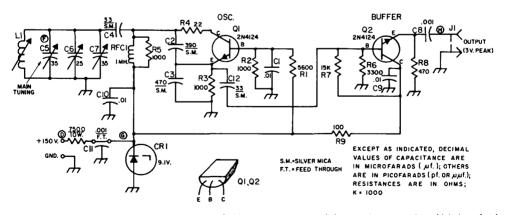
Fig. 6-52—Schematic diagram of the v.f.o. Fixed-value capacitors are disk ceramic except C11 which is a feedthrough type. Resistors are 1/2-watt composition unless noted otherwise. All parts carry numbers for identification purposes on the circuit-board template. Significant parts are listed below.
