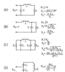
Fig. 2-52—Impedance-matching networks adaptable to amateur work. (A) L network for transforming to a lower value of resistance. (B) L network for transforming to a higher resistance value. (C) Pi network. R1 is the larger of the two resistors; Q is defined as R<sub>1</sub>/X<sub>C1</sub>. (D) Tapped tuned circuit used in some receiver applications. The impedance of the tuned circuit is transformed
