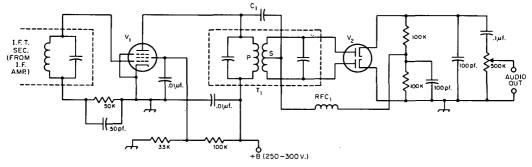
Fig. 5-34—Limiter-discriminator circuit.
