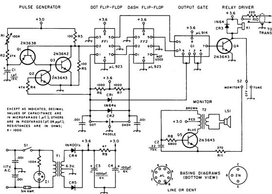
Fig. 7-10—Schematic of the Micro-TO keyer. Capacitances are in  $\mu$ f., polarity indicates electrolytic, others are ceramic. Resistances are in ohms (K = 1000); resistors are ½-watt. Component designations not listed below are for identification in board layout.
