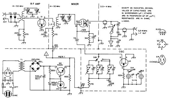
Fig. 5-45—Diagram of the converter. Fixed-value capacitors are disk ceramic or mica. Polarized capacitors are electrolytic. Resistors are ½-watt composition. F.J. denotes feed-through capacitors.
