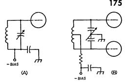
Fig. 6-34—The voltage rating of the grid tank capacitor in A should be equal to the biasing voltage plus about 20 per cent of the plate voltage.
