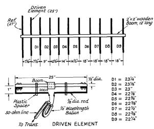
Fig. 18-9—Construction data for a high-performance 220-Mc. Yagi. Parasitic elements are made from ½-inch diameter aluminum rod. Balun precautions of Fig. 18-8 should be followed.
