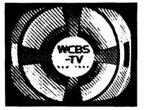
Fig. 23-5—"Cross-hatching," caused by the beat between the picture carrier and an interfering signal inside the TV channel.
