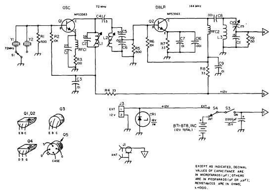
Fig. 19-36—Schematic of the 2-meter transceiver. Fixed-value capacitors are disk ceramic except those with polarity marking, which are electrolytic. Resistors are ½-watt composition. Component numbering is for identification of parts on the circuit-board templates. Significant parts are listed below in the usual manner.
