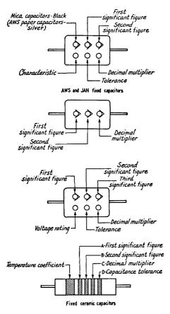
Fig. 20-5—Color coding of fixed mica, molded paper and tubular ceramic capacitors. The color code for mica and molded paper capacitors is given in Table 20-111. Table 20-1V gives the color code for tubular ceramic capacitors.
