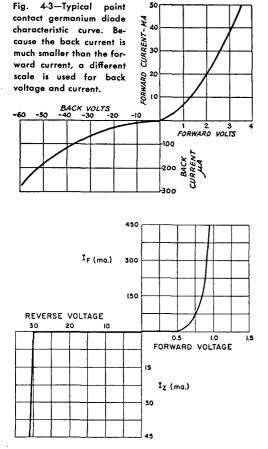
Fig. 4-4—Typical characteristic of a zener diode. In this example, the voltage drop is substantially constant at 30 volts in the (normally) reverse direction. Compare with Fig. 4-3. A diode with this characteristic would be called a "30-volt zener diode."
