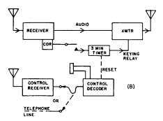
Fig. 10-7 Simple repeaters. The system at A is for local control. Remote control is shown at B.
