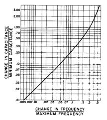
Fig. 5-9—Minimum circuit capacitance required in the circuit of Fig. 5-8A as a function of the capacitance change and the frequency change. Note that maximum
