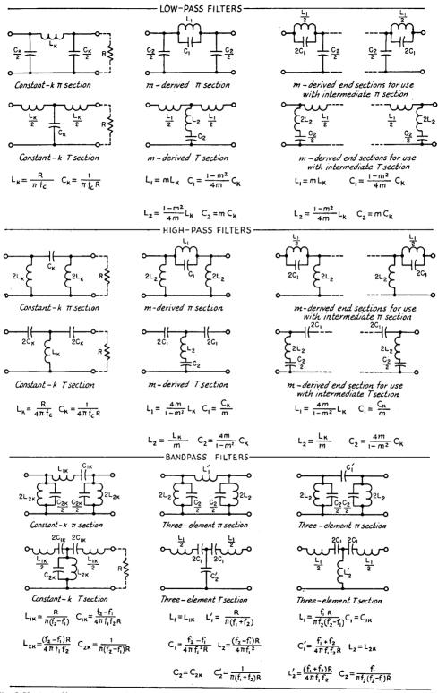
Fig. 2-53—Basic filter sections and design formulas. In the above formulas R is in ohms, C in farads, L in henrys, and f in cycles per second.
