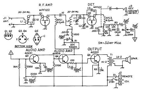
Fig. 19-56—Schematic diagram of the receiver. Unless otherwise noted, all resistors are ½-watt. Resistance is in ohms. K = 1000. Capacitors are disk ceramic unless otherwise indicated. Capacitors with polarity marks are electrolytic. Capacitance is in pF. Dashed lines indicate an optional circuit which is discussed in the text.
