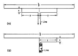
Fig. 14-38—The "T" match and "gamma" match.
