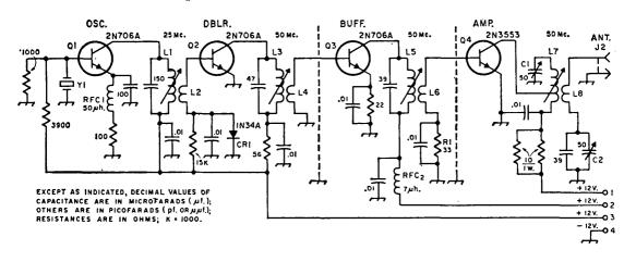
Fig. 17-16A—Schematic of the four-transistor rf strip. Decimal-value capacitors are 50-volt disk ceramics. Resistors are ½-watt composition unless noted otherwise.
