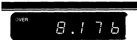
Fig. 6-12 — A 5-digit readout using light-emitting diodes.
