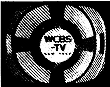
Fig. 16-7 — "Cross-hatching," caused by the beat between the picture carrier and an interfering signal inside the TV channel.
