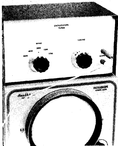
Fig. 13-29 — An oscilloscope adaptor permits monitoring of the output rf envelope from an hf transmitter. Any shop-type oscilloscope may be used.
