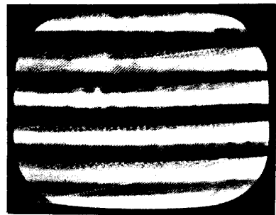
Fig. 16-8 — "Sound bars" or "modulation bars" accompanying amplitude modulation of an interfering signal. In this case the interfering carrier is strong enough to destroy the picture, but in mild cases the picture is visible through the horizontal bars. Sound bars may accompany modulation even though the unmodulated carrier gives no visible cross-hatching.
