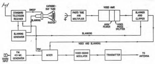
Fig. 15B-1 - Block diagram of the television system used by W2BK, formerly W2LNP. (From  $QST_{\rm s}$  June, 1950.)
