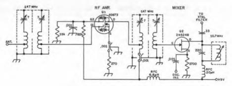
Fig. 9-6 - Schematic diagram of the Johnson 504 front-end circuit.
