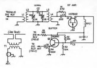
Fig. 1 — Schematic diagram of the rf amplifier and preselector. In this and succeeding diagrams, component designations not mentioned in the captions are for text and layout references only. Unless otherwise noted, resistors are 1/4- or 1/2-watt composition and capacitors are disk ceramic.
