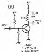
Fig. 6-31 — Metering circuits for (A) tubes and (B) transistors. To measure current, connect a meter at the point shown in series with the lead. For voltage measurements, connect the meter from the point indicated to the common or ground connection.
