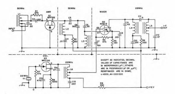
Fig. 2 — Schematic diagram of the six-meter converter. All resistors are 1/4-watt composition. C2, C8, C10 and C15 are .001 $\mu$ F disk ceramic, C4 is .01- $\mu$ F disk ceramic. All other capacitors are dipped mica.
