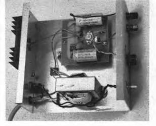
The manufacturer recommends a low-inductance connection between the case of the HEP C4069R and ground. No evidence of instability was noted with this circuit.
