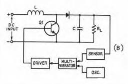
Fig. 5-26 — At A, the fundamental circuit of a flyback switching regulator, and at B, the elements of a practical circuit.
