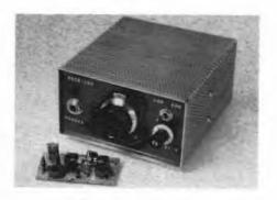
The major compromise was the elimination of age and multiband coverage. There is ample room inside the cabinet of this receiver to accommodate one or two small converters for reception of bands other than 40 meters. This main frame is designed for 7- to 7.175-MHz coverage.
