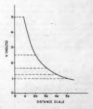
Fig. 1B — Variation of potential with distance f the charged sphere of Fig. 1A.
