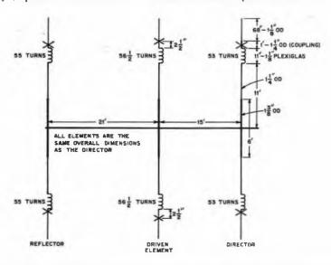
Fig. 5 — Mechanical details and dimensions for the 40-meter Yagi. Each of the elements uses the same dimensions; the difference is only the number of turns on the inductors and the placement of the capacitance hats. See the text for more details.
