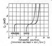
Fig. 4-8 — Curves showing the comparison in characteristics between a 1N21G point-contect diode and a Hewlett-Packard HPA2350 hot-carrier diode
