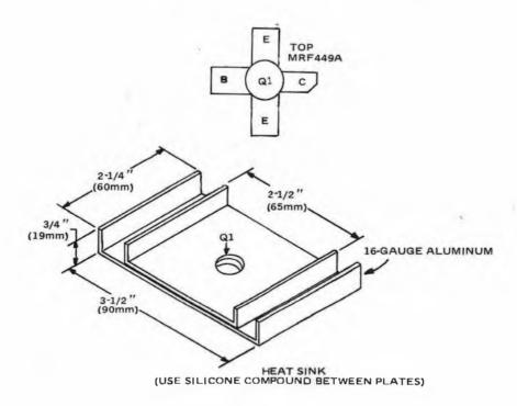
Fig. 2 — Scale layout of the pc board. Heat-sink dimensions are given in English and metric. The heat sink is held to the double-clad pc board by means of the transistor stud and two 4-40 screws and nuts. A substantially larger heat sink should be used if the amplifier is revised for 30 watts of output.
