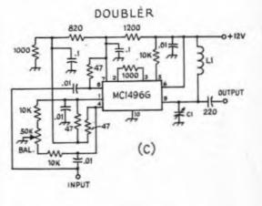
Fig. 6-14 — Frequency-multiplier circuits.
