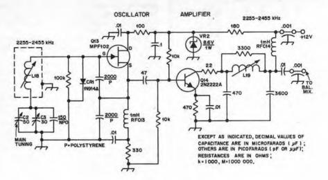
Fig. 2 — Circuit diagram of the local oscillator. Capacitors are disk ceramic unless specified differently. Resistors are 1/2-W composition. Entire assembly is enclosed in a shield box made from pc-board sections.
