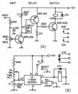
Fig. 14-31 — (A) COR circuit for repeater use. R2 sets the length of time that K1 will stay closed after the input voltage dissappears. K1 may be any relay with a 12-volt coil, although the long-life reed type is preferred. CR1 is a silicon diode. (B) Timer circuit using a Signetics NE555. R1, C1 sets the timers range. C1 should be a low-leakage type capacitor. S1, S2 could have their contacts paralleled by the receiver COR for automatic START and RESET controlled by an incoming signal.
