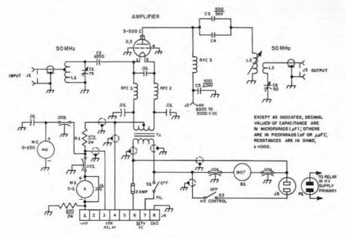
Schematic diagram information for the 50-MHz grounded-grid ampli-
