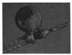
Fig. 16-7 — Proper mathod of bypassing the end of a shielded lead using disk ceramic capacitor. The .001- $\mu$ F size should be used for 1600 volts or less; 500 pF at higher voltages. The leads are wrapped around the inner and outer conductors and soldered, so that the lead length is negligible. This photograph is about four times actual size.
