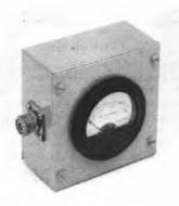
Fig. 17-10 — Rf ammeter mounted in a Minibox, with connectors for placing the meter in series with a coaxial line. A bakelite-case meter should be used to minimize shunt capacitance (which introduces error) although a metal-case meter can be used if mounted on bakelite sheet with a large cut-out in the case around the rim. The meter can be used for rf power measurements (P = ½R) when connected between a transmitter and a nonreactive load of known resistance.
