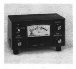
The phone patch unit is built into a homemade aluminum enclosure measuring 3 X 3 X 6 inches. A coating of spray-on enamel, rubber feet, and wet-transfer decal labels plus shiny knobs give the unit a professional appearance.
