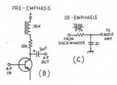
Fig. 14-6 — (A) The phase-shifter type of phase modulator. (B) Pre-emphasis and (C) de-emphasis circuits.
