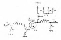
Fig. 1 - Schematic diagram of the 220-MHz amplifier.
