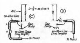
Fig. 10-23 — At A and B, an illustration of how a quarter-wavelength vertical antenna can be mounted on a car roof. The whip section should be soldered into the cap portion of the Millen connector, then screwed to the base socket. This handy arrangement permits removing the antenna when desired. Epoxy cement should be used at the two mounting screws to prevent moisture from entering the car. Diagrams C and D are discussed in the text.
