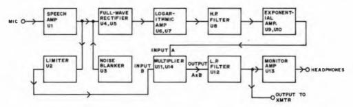
Fig. 2 - Block diagram for the processor.
