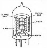
Fig. 3-16 — Representative arrangement of elements in a screen-grid tetrode, with part of plate and screen cut away. This is "single-ended" construction with a button base, typical of miniature receiving tubes. To reduce capacitance between control grid and plate the leads from these elements are brought out at opposite sides; actual tubes probably would have additional shielding between these leads.
