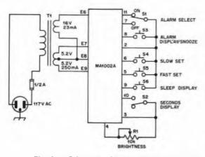
Fig. 1 — Schematic diagram of the clock. T1 is discussed in the text. S1 and S2 are spot miniature toggle switches. S3 through S6 are momentary switches that are normally open. R1 is a miniature linear-taper potentiometer.
