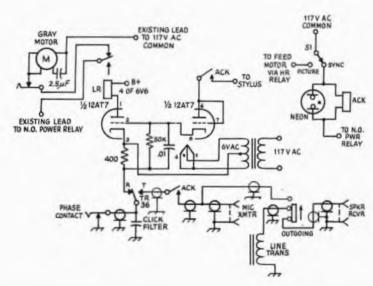
Fig. 3 — Circuit modification for sending or receiving sync information before picture scan begins. These modifications were originally described by W7QCV in QST for May, 1972.
