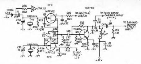
Fig. 5 — Carrier oscillator board. C30, C33 — Miniature pc-mount air variable
