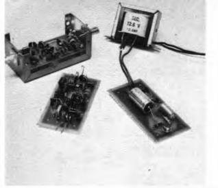
Fig. 1 — Completed six- and two-meter converters (left and center) with power supply.
