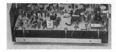
respective tuned circuits. For simplicity s sake only two tuned circuits are used ahead of the mixer, which uses a dual-gate MOSFET. The combination of FETs Q1 and Q2 assures low IMD and provides good immunity to overloading. Output from the mixer is supplied to FL1. This is a four-pole 10.7-MHz i-f filter which is fed from a 900-ohm tap point on tuned circuit C9-C10-L3.
