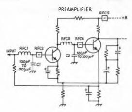
Fig. 16-25 — Typical circuit of a solid-state preamplifier.
