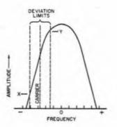
Fig. 14-9 — Fm detector characteristics. Slope detection, using the sloping side of the receivers selectivity curve to convert fm to a-m for subsequent detection.
