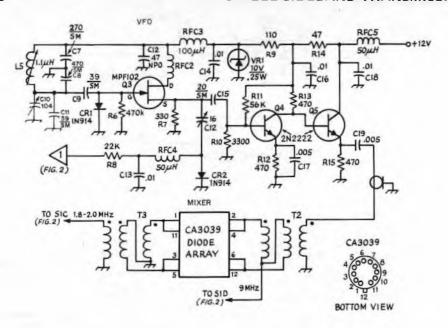
Fig. 3 — Schematic diagram of LO and mixer module, If greater bandspread is desired, a smaller value capacitor could be substituted for C10 with C11 increased by an appropriate amount to set the low-frequency end of the tuning range to 10.8 MHz.
