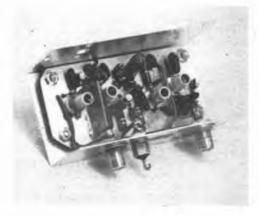
WWV converter as nested in the chassis. The shield shown in the photograph was found to be unnecessary since stray coupling between the input and output of the rf amplifier proved not to be a problem.
