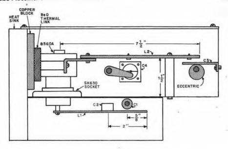
Fig. 2 — Cutaway drawing from the side of the grid and plate compartments. The plate line may be made of two pieces, as shown here, or of one single piece of aluminum strip. C4 is shown from the end-on view. The arm that moves C4 and the eccentric that moves C3 are fastened to their insulated shafts by epoxy cement. Small Teflon buttons prevent accidental shorts between the capacitors and the plate line.
