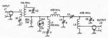
Fig. 1 - Schematic for the varactor tripler.
