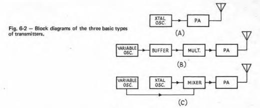
made the heterodyne exciter of Fig. 6-2C increasingly popular, in spite of the slightly more complex circuitry required.
