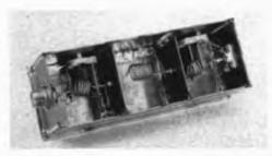
Pc board serves as an enclosure for this ellipticfunction filter.
