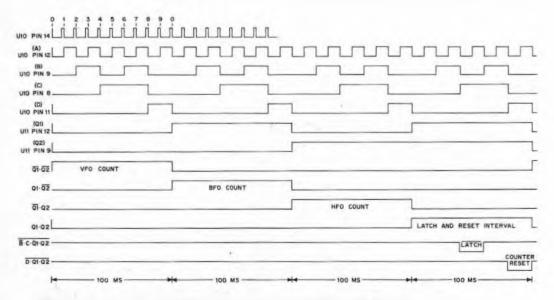
Fig. 11 - Chart showing waveforms associated with a standard count sequence,
