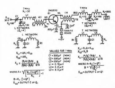
Example: An amplifier stage must deliver 10 watts to a known resistive load. The dc voltage from collector to emitter is 13.6.  $R_L$  is
