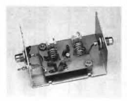
Fig. 14-44 — The 2-meter preamp, may be mounted in a small Minibox or connected directly inside an fm receiver,
