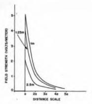
Fig. 1C — Variation of field strength with distance around a sphere charged to 5 volts for spheres of different radii.
