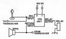
Fig. 3 — Typical connections to the VOX unit.
