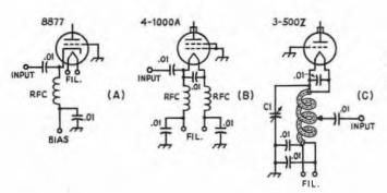
Fig. 6-21 — Input circuits for triode or triode-connected power tubes operated grounded grid.
