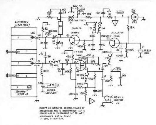
Fig. 2 - Schematic diagram of the 1296-MHz converter with oscillator and multiplier sections included, Dimensions for the filter and mixer assembly are given in Fig. 1.
