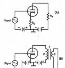
Fig. 3-14 — Simple circuits for producing feedback.
