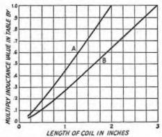
Fig. 2-15 — Factor to be applied to the inductance of coils listed in the table below, as a function of coil length. Use curve A for colls marked A, and curve B for colls marked B.
