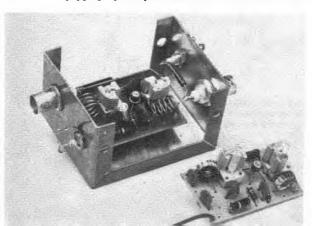
Two versions of the preamplifier. The one in the box is for 2-meter use. Toroids are used in the six-meter version (right) and in the ten-meter preamplifier (not shown). Input is at the right on both units. The extra rf choke and feedthrough capacitor on the right end of the Minibox are for decoupling a crystal-current metering circuit that is part of a 2304-MHz mixer.
