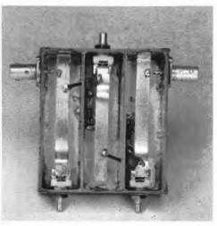
Fig. 14-46 — The 440-MHz preamplifier is constructed in a 3 X 3 1/2 X 1-inch box made of double-sided circuit board. All abutting edges are soldered to complete the enclosure. Two 3 X 15/16-inch shields separate the tuned lines.
