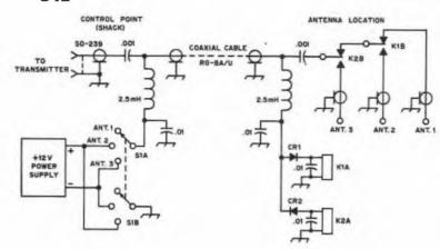
Fig. 23-1 - A remote antenna switching system using low voltage relays handles three different antennas. The coaxial cable is used as the control line. CR1 and CR2 can be any low voltage silicon diodes 1N4001 (Motorola equiv.). K1 and K2 can be any 12-V dc relays with suitable contact ratings (Potter and Brumfield KA5DG or equiv.). The rotary switch should have at least two sections and three positions.
