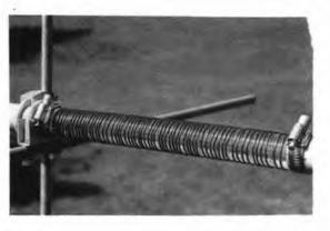
Fig. 4 — Each loading coil is wound on Plexiglas rod. The capacitance hats for the parasitic elements are mounted next to the coil, asshown here. The hose clamps compress the tubing against the Plexiglas rod. Each capacitance hat consists of two sections of tubing and associated muffler clamps.
