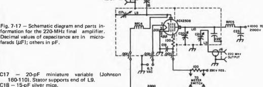
formation for the 220-MHz final amplifier. Decimal values of capacitance are in microfarads (UF); others in pF.
