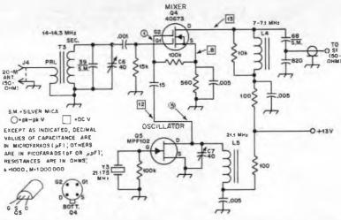
Fig. 3 — Schematic diagram of the 20-meter converter. Fixed-value capacitors are disk ceramic unless noted otherwise. Resistors are 1/4- or 1/2-W composition. Rough pc template and layout available for 25d and an s.a.s.e.
