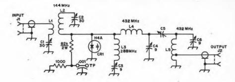
Fig. 3 - Schematic diagram of the varactor tripler.
