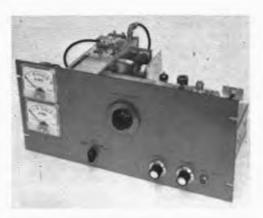
Fig. 7-13 — The 220-MHz transmitter is set up for rack mounting on 8 3/4-inch panel. Meters at the left can be switched to read driver plate, amplifier screen and amplifier plate currents, and amplifier plate voltage.
