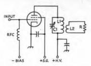
Fig. 6-25 — Inductive-link output coupling circuits.
