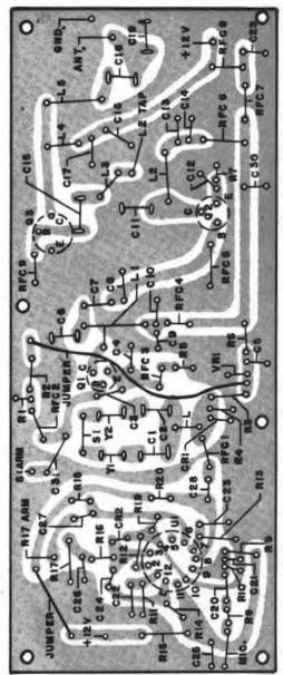
Fig. 2 — Template and parts layout for the transmitter drawn to full scale. Foil-side view.
