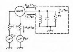
Fig. 1 — The I-f port of a double-balanced mixer is matched at fLO-frf and reactive at fLO+frf. In this configuration conversion loss, rf compression and desensitization levels can vary  $\pm 3$  dB while harmonic modulation and third-order IMO products can vary  $\pm 20$  dB.
