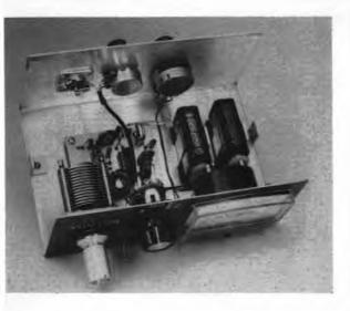
Inside view of the field strength meter. Most of the components are mounted on a circuit board.
