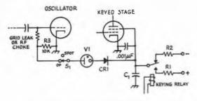
Fig. 11-8 - VR-tube differential keying in an
