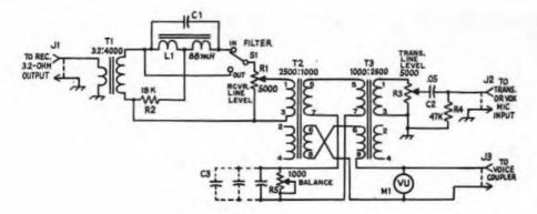
Fig. 1 — Schematic diagram of the phone-patch circuit. Resistances are in ohms, k=1000. Fixed resistors may be 1/2 watt, 10 percent tolerance. Capacitance is in microferads. Components not listed below are identified for text reference.
