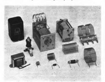
Inductors for power and radio frequencies. The two iron-core coils at the left are "chokes" for power-supply filters. The mounted air-core coils at the top center are adjustable inductors for transmitting tank circuits. The "piewound" coils at the left and in the foreground are radio-frequency choke coils. The remaining coils are typical of inductors used in rf tuned circuits, the larger sizes being used principally for transmitters.
