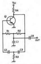
Fig. 17-23 — Twin-T audio oscillator circuit, Representative values for R1-R2 and C1 range from 18k  $\Omega$  and .05  $\mu\text{F}$  for 750 Hz to 15k  $\Omega$  and .02  $\mu\text{F}$  for 1800 Hz. For the same frequency range, R3 and C2-C3 vary from 1800 ohms and .02  $\mu\text{F}$  to 1500 ohms and .01  $\mu\text{F}$ . R4 should be approximately 3300 ohms, C4, the output coupling capacitor, can be .05  $\mu\text{F}$  for high-impedance loads.
