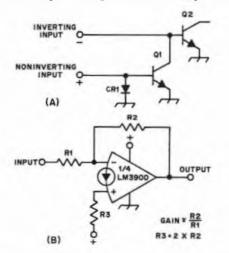
Fig. 1 — (A) Simplified input circuit for a Norton operational amplifier such as used in the National Semiconductor LM3900. (B) Design equations for an audio amplifier using the LM3900.
