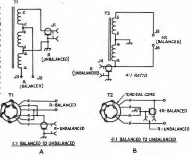
Low-loss high-frequency ferrite core material is used for T1 and T2.<sup>1,3</sup> The cores are made from Q-2 material and cost approximately \$5.50 in single-lot quantity. They are 0.5 inches thick, have an OD of 2.4 inches, and the ID is 1.4 inches. The permeability rating of the cores is 40. A packaged one-kilowatt balun kit, with winding instructions for 1:1 or 4:1 impedance transformation ratios, is available, but uses a core of slightly different dimensions.<sup>2</sup>
