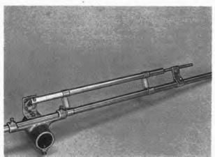
Fig. 22-9 - A hand-made coaxial gamma match for 50-MHz arrays. A 1/4-inch rod or tube 14 inches or longer slides inside a 1/2-inch sleeve that is connected to the coaxial fitting above the boom, The rod slides on plastic sleeves inside the larger section. Separation is maintained with two ceramic pillars mounted with wraparound clips. Both the coaxial capacitor and the sliding clip between rod and element are adfor minimum reflected iusted power in the coaxial line.
