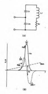
Fig. 9 — A capacitively coupled resonator is shown at (A). See text for explanation of figure shown at (B).
