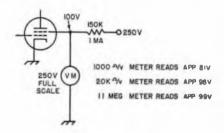
Fig. 17-3 — Effect of voltmeter resistance on accuracy of readings. It is assumed that the donesistance of the screen circuit is constant at 100 kilohms. The actual current and voltage without the voltmeter connected are 1 mA and 100 volts. The voltmeter readings will differ because the different types of meters draw different amounts of current through the 150-kilohm resistor.
