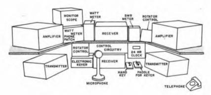
This neatly arranged station belongs to W@TDR in Missouri. The equipment is mounted in a home-made console placed on top of a desk. All controls are easily reachable. A telephone is conveniently located to the right of the operating position. Directly in front of the operator, above the lower receiver, is the control panel which handles antenna and station component switching. This layout is ideal for the right-handed operator.
