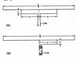
Fig. 20-13 - The "T" match and "gamma" match.
