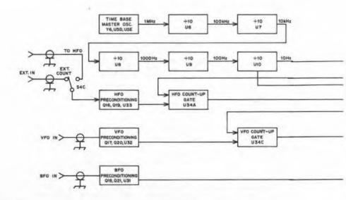
Fig. 9 - Simplified block diagram of the receiver frequency display.
