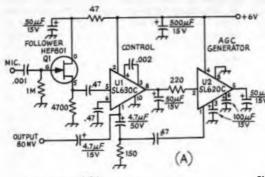
Fig. 13-18 — Typical solid-state compressor circuit.
