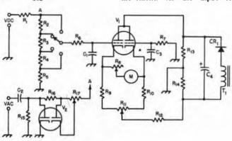
Fig. 17-8 - Vacuum-tube voltmeter circuit.
