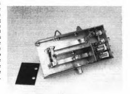
The varactor tripler is assembled in a box made from double-sided pc board.
