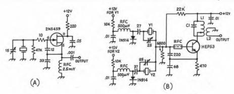
Fig. 6-5 — Two practical crystal-oscillator designs. (A) For low-power output applications such as a conversion oscillator or BFO, (B) an example of diode switching of crystals. The rf choke on the base lead of the transistor is a ferrite bead which prevents whi parasitic oscillation.
