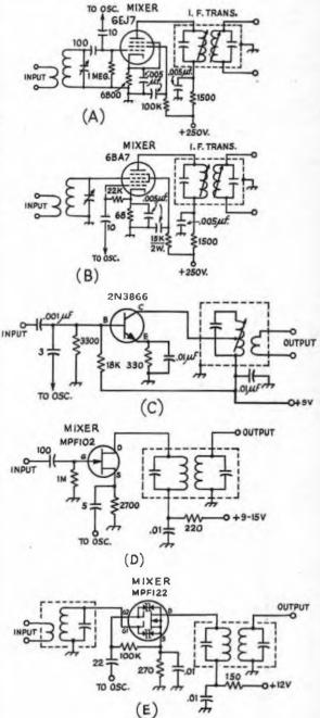
Fig. 8-15 — Typical single-ended mixer circuits.
