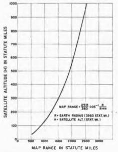
Fig. 15E-1 — Satellite altitude above earth versus ground station map range (statute miles).
