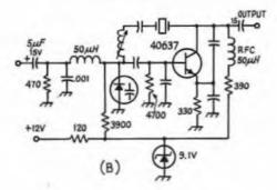
Fig. 14-5 — Reactance modulators using (A) a high-transconductance MOSFET and (B) a varactor diode.
