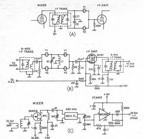
Fig. 8-25 — A half-lattice bandpass filter at A; B shows two half-lattice filters in cascade; C shows a mechanical filter.
