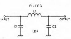
(D) Pi-section output filter, C1 and C2 are 39-pF mica capacitors (Elmenco 6ED390J03 or equiv.), and L1 consists of 2 turns of No. 18 tinned wire, 1/4 inch ID, 0.2 inch long (approximately 44 nH).
