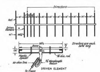
Fig. 22-12 — High-performance long Yagi for 144 MHz, from experimental work by W2NLY and W6QKI. Dimensions are for maximum gain between 144 and 145 MHz.
