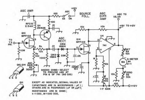
Fig. 5 - Schematic diagram of the ago system. Capacitors are disk ceramic except when polarity is indicated, which signifies electrolytic. Fixed-value resistors are 1/2-W composition. This module is not enclosed in a shield compartment.
