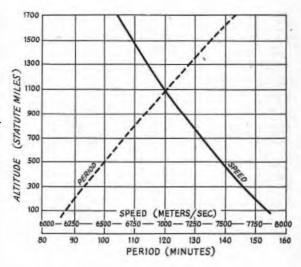
Fig. 15E-4 — Satellite attitude versus its period (time for one revolution) and speed.
