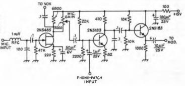
Fig. 13-12 — Typical phase-inverter circuits for transistor amplifier applications.
