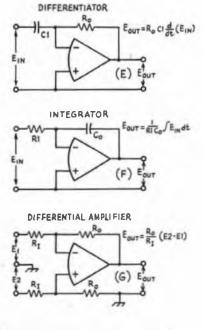
Fig. 4-33 — Basic op-amp circuits.
