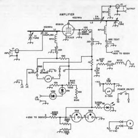
Fig. 1 — Schematic diagram of the 432-MHz amplifier.
