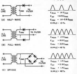
Fig. 5-8 — Fundamental rectifier circuits. A — Half-wave ( $E_{PRV} = 1.4~E_{RMS}$  with resistive load, = 2.8  $E_{RMS}$  with capacitor-input filter). B — Full-wave. C — Full-wave bridge. Output voltage values do not include rectifier voltage drops.
