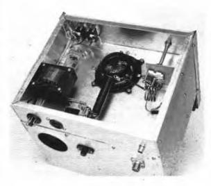
Fig. 7-29 — With the bottom cover removed, a fook into the chassis from the rear shows the input circuit, L1,C1, right, the bifilar filament chokes, foreground, filament transformer and control switches. Opening in the rear wall is for air intake.
