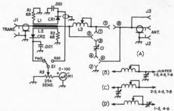
Fig. 21-33 — Circuit diagram of the L-network Transmatch. The eight banans jacks are E. F. Johnson type 108-900, and three dual banana plugs are required, E. F. Johnson type 108-200. C1 — Variable capacitor, 350 pF (E. F. Johnson
