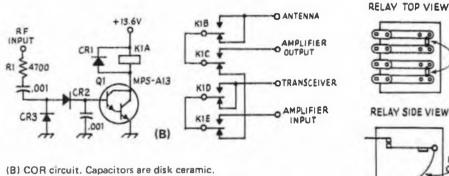
The COR relay is modified by removing the connecting wires from all four wiper arms and adding two shorting bars, as shown. Only the stationary-contact connections are used.
