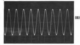
Fig. 14-13 — (A) Input wave form to a limiter stage shows a-m and noise. (B) The same signal, after passing through two limiter stages, is devoid of a-m components.
