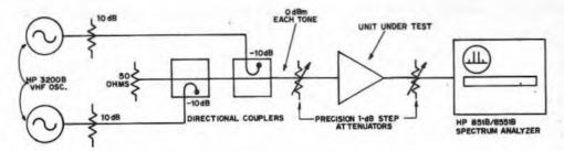
Fig. 6-A test setup used to measure IMD. The first attenuator adjusts the input level to the unit under test. The second one provides a means of staying within the linear range or the spectrum analyzer.
