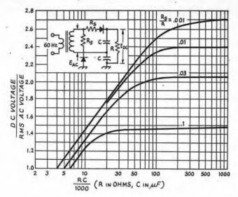
Fig. 5-18 - Dc output voltages from a full-wave voltage-doubling circuit as a function of the filter capacitances and load resistance. For the ratio R<sub>s</sub>/R and for the RC product, resistances are in ohms and capacitance is in microfarads. Equal resistance values for Rs and equal capacitance values for C are assumed.
