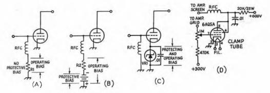
Fig. 6-18 — (A-C) Various systems for obtaining protective and operating bias. (D) Screen clamper circuit for protecting power tetrodes.
