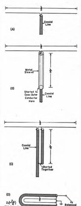
Fig. 20-14 — Radiator with coaxial feed (A) and methods of preventing unbalanced currents from flowing on the outside of the transmission line (B and C). The half-wave phasing section shown at D is used for coupling between an unbalanced and a balanced circuit when a 4-to-1 impedance ratio is desired or can be accepted.
