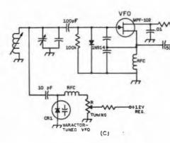
Fig. 4-6 — Varactor frequency multipliers are shown at A and B. In practice the tuned circuits and impedance-matching techniques are somewhat more complex than those shown in these representative circuits. At C, a varactor diode is used to vary the frequency of a typical JFET VFO. As the dc voltage is changed by control R, the junction capacitance of CR1 changes to shift the resonant frequency of the tuned circuit.
