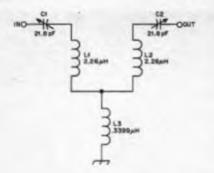
Fig. 3 — Schematic diagram of the "Citation Eliminator." Component values shown are theoretical computed inductances and capacitances for a bandpass filter resonant at 21.14 MHz with a bandwidth of 4.5 MHz.
