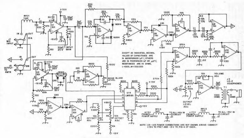
Fig. 3 — Circuit diagram for the speech processor. CR1, CR2 — pair of matched silicon diodes (see text).
