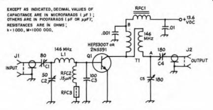
Fig. 14-55 - Circuit diagram of the 25-watt amplifier. Capacitors are disk ceramic unless otherwise noted.
