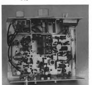
Fig. 2 — Inside view of the receiver. Most of the components are mounted on a 4- X 6-inch printed-circuit board. The rf amplifier and product detector components are grouped together at the upper left corner of the board, while the audio channel occupies the left foreground. The VFO main-tuning capacitor, C24, is centered in the cabinet, and is positioned directly over the VFO. The S-meter amplifier circuitry is visible at the right.
