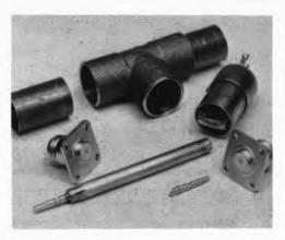
Fig. 22-24 — Major components of the line sampler. The brass T and two end sections are at the back of the picture. A completed probe assembly is at the right. The N connectors have their center pins removed. The pins are shown with one inserted in the left end of the inner conductor and the other lying in the right foreground.
