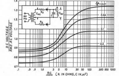
Fig. 5-5 - Dc output voltages from a full-wave rectifier circuit as a function of the filter capacitance and load resistance. includes transformer winding resistance and rectifier forward resistance. For the ratio R<sub>s</sub>/R, both resistances are in ohms; for the RC product, R is in ohms and C is in µF.
