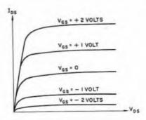
Fig. 4-218-Typical MOSFET characteristic curves.
