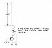
Fig. 10-20 — Diagram of 5/8-wavelength 220 MHz mobile antenna.
