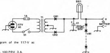
Fig. 1 — Schematic diagram of the 117-V ac charger.
