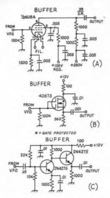
Fig. 6-7 — Isolating stages to be used between a VFO and the following amplifier or mixer stage.
