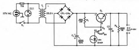
Fig. 5-23 — Schematic diagram of the power supply. Capacitances are in  $\mu$ F; capacitors marked with a polarity are electrolytic. Resistances are in ohms; R1 and R2 are composition.
