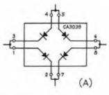
Fig. 13-5 — Additional balanced-modulator circuits in which integrated circuits are used.
