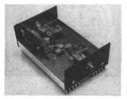
lamp should illuminate to slightly more than normal brilliance. Power output into a 50-ohm load should be between 1-1/2 and 2 watts Current drain will be between 200 and 250 mA, speech amplifier included.
