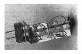
Inside view of the variable inductor antenna coupler. A shield is placed between the two inductors. Care must be taken to assure that moving wires attached to the inductors have a minimum of stress placed on them during dial rotation.
