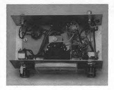
The layout of the phone-patch components is not critical. The two hybrid-network transformers are visible to the right of center, and in the upper left corner of the circuit board the receiver matching transformer may be seen. Two damping capacitors added during modification of the Calectro DI-930A meter are visible atop the meter case; two more are hidden beneath the meter.
