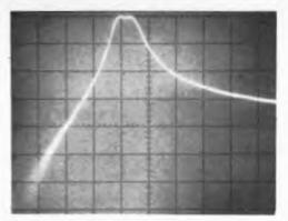
Fig. 4 — Response of the "Citation Eliminator." Attenuation and frequency scale 10 dB/div. (vertical) and 5 MHz/div. (horizontal).
