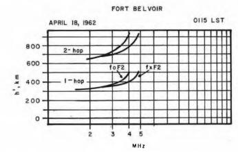
19-4 F-laver Fig. ionogram taken at night during magnetically quiet conditions. The traces show the breaking up into ordinary and extraordinary waves. Because it required twice the travel time, the double-hop return appears as having come from twice the height ρf single-hop,
