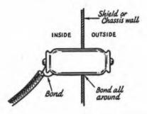
Fig. 16-10 - The best method of using the "Hypass" type feed-through capacitor, Capacitances of .01 to 0.1 µF are satisfactory, Capacitors of this type are useful for high-current circuits, such as filament and 117-volt leads, as a substitute for the rf choke shown in Fig. 16-8, in cases where additional lead filtering is needed.
