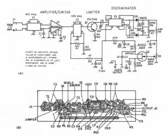
Fig. 14-24 — (A) Diagram of the 455-kHz narrow-band adapter. Resistors are 1/4- or 1/2-watt composition and capacitors are disk ceramic, except those with polarity marked, which are electrolytic. Components with reference numbers that are not listed below are noted for circuit-board location.
