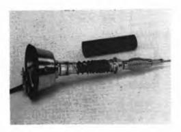
Fig. 1 — The new coil is tapped two turns from the base end, it may be necessary to file the coil ends so that the assembly will fit in the phenolic covering.
