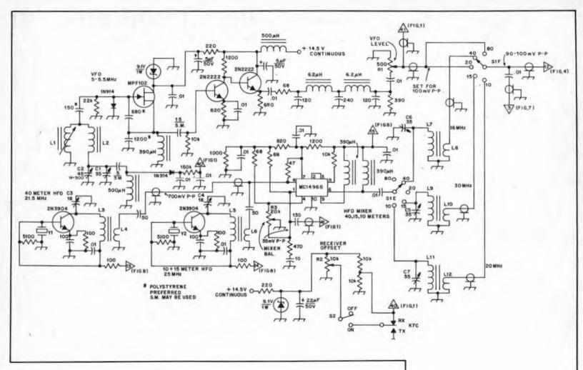
Fig. 1 — Circuit diagram for the transceiver VFO, HFO, and mixer.
