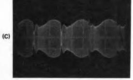
Fig. 8-22 — The delay and lengthening of a noise pulse when passed through a 2-kHz wide amplifier with good skirt selectivity (4 kHz at -60 dB). (B) a 3.75-MHz carrier modulated 30 percent, interfered with by noise pulses. The noise pulses were originally 1000 times the amplitude of the signal; they have been reduced (and lengthened) by overload in the i-f. The i-f bandwidth is 5 kHz. Sweep speed = 1 millisecond/cm. (C) Same as B but with a noise blanker on.
