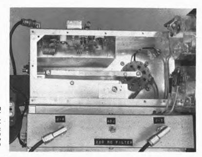
Fig. 7-21 — Looking into the amplifier grid compartment. The varector tripler is in the upper left portion. Below the compartment is the 220-MHz strip-line filter.
