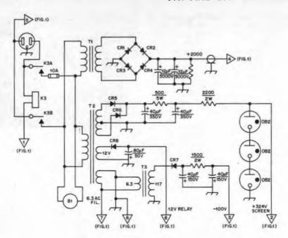
Fig. 2 — Power supply for the amplifier.
