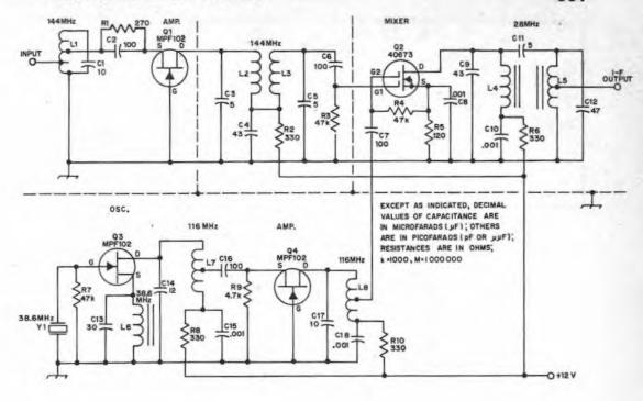
Fig. 3 — Schematic diagram of the two-meter converter. All resistors are 1/4-watt composition. C8, C10, C15 and C18 are .001- $\mu$ F disk ceramic, All other capacitors are dipped mica units,
