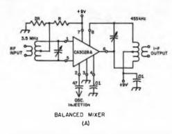
Fig. 4-25 — Some typical circuit applications for a differential amplifier IC. The internal circuit of the CA3028A IC is given in Fig. 4-24 at A.
