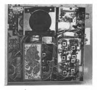
In this particular model transceiver, room was available to mount the converter in an inverted position just below the speaker. A small bracket is fastened under one of the bolts that also holds a transformer to the bottom sidewall. Cables are routed along with existing wiring harnesses and tied in place. The 28-MHz input connector is fastened to the rear apron of the equipment.
