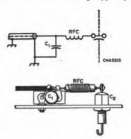
Fig. 16-9 — Additional lead filtering for harmonics or other spurious frequencies in the high whf TV band (174-216 MHz).
