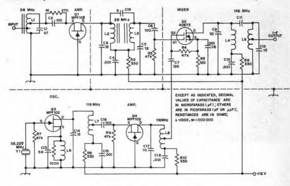
Fig. 1 — The schematic diagram of the "Rochester" converter as modified for up-conversion.
