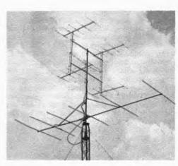
Fig. 22-7 — Antennas for two bands on a single support. Four 5-element Yagis for 144 MHz, top, have one-wavelength spacing each way. The 50-MHz Yagi is set up to make optimum use of 6 elements on a 20-foot boom.
