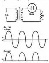
Fig. 3-4 — Rectification in a diode. Current flows only when the plate is positive with respect to the cathode, so that only half-cycles of current flow through the load resistor, R.
