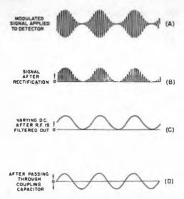
Fig. 8-5 - Diagrams showing the detection process.
