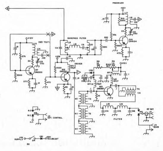
Fig. 2 — Schematic diagram of the 80- or 20-meter low-power ssb/cw transmitter. Capacitors with polarity marked are electrolytic. Fixed-value capacitors are ceramic unless otherwise noted. Resistors are 1/2-watt composition unless marked otherwise. Numbered parts not appearing below are so identified for pc-board layout purposes only.
