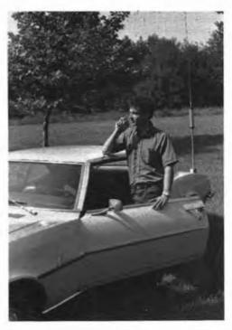
Fig. 10-7 — Here a mobile station is used as a porteble/emergency station. As such, it can be connected to a full-size stationary antenna for maximum effectiveness. The engine should be noise-suppressed, and should be kept running during operation of the station to assure full battery power, (WA3EQK operating.)
