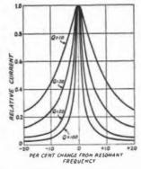
Fig. 2-39 — Current in series-resonant circuits having different Qs. In this graph the current at resonance is assumed to be the same in all cases. The lower the Qs, the more slowly the current decreases as the applied frequency is moved away from resonance.
