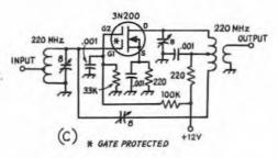
Fig. 9-1 — Typical grounded-source of amplifiers. The dual-gate MOSFET,A, is useful below 500 MHz. The junction FET,B, and neutralized MOSFET,C, work well on all vhf bands. Except where given, component values depend on frequency.
