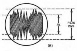
Fig. 13-17 — (A) Typical ssb voice-modulated signal might have an envelope of the general nature shown, where the ri amplitude (current or voltage) is plotted as a function of time, which increases to the right horizontally. (B) Envelope pattern after speech processing to increase the average level of power output.
