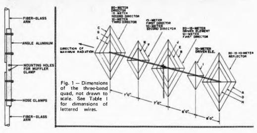
Fig. 2 — Details of one of two assemblies for a spreader frame. The two assemblies are jointed to form an x with a muffler clamp mounted at the position shown.
