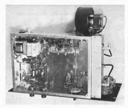
Fig. 7-20 - Looking underneath chassis of the 220-MHz transmitter, we see the speech amplifierclipper at the lower left, the exciter circuits across the top, power supply components at the upper left, and meter switching, lower right.
