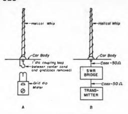
Fig. 10-13 — The resonant frequency of the antenna can be checked (A) with a grid-dip meter or (B) by finding the frequency at which minimum feed-line SWR occurs. The latter method is more accurate at high frequencies because it eliminates the effect of the coupling loop required in A.
