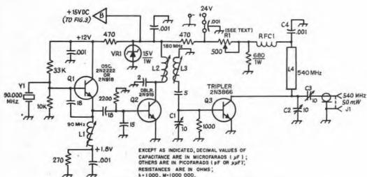
Fig. 4 — Schematic diagram of the oscillator and multiplier for the 2304-MHz converter. As explained in the text and shown in the photographs, a fixed-value resistor may be substituted for R1 after the value that provides proper performance has been found.
