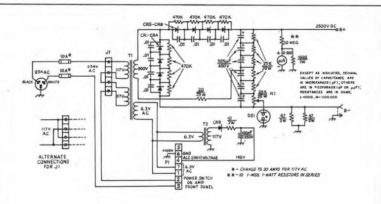
Fig. 2 — Circuit diagram for the power supply. The power transformer is available from Harmond; type no. 101165. CR1 through CR9 are 2.5 A, 1000 PRV; see Fig. 1 for suitable part number. T2 is Stancor part number P-8190 and is
