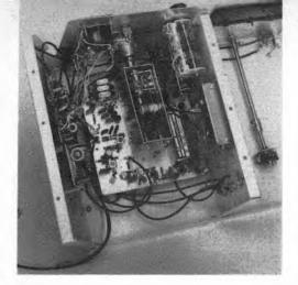
View of the receiver compartment prior to installation of the converter boards,
