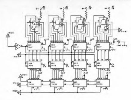
Fig. 10 - Circuit diagram for the display unit. ,
