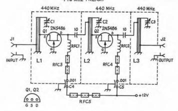
Schematic diagram of the uhf Fig. 14-47 preamplifier. Capacitors are disk ceramic unless otherwise noted.
