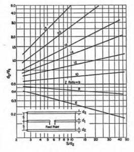
Fig. 20-12 — Impedance transformation ratio, three-conductor folded dipole. The dimensions d1, d2 and s are shown on the inset drawing. Curves show the ratio of the impedance (resistive) seen by the transmission line to the radiation resistance of the resonant entenna system.
