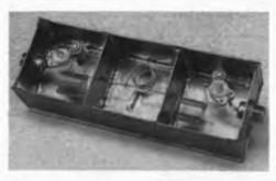
A similar construction using pc board is shown for the "Citation Eliminator." Approximate dimensions are 2 X 2-3/4 X 2-3/4 (HWD). A top cover with hole for capacitor adjustment should be soldered on after filter is initially aligned. Power rating is suitable for transmitters in 75-watt input class.
