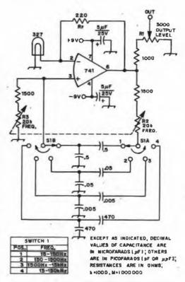
Fig. 1 — A simple audio oscillator that provides a selectable frequency range. R2 and R3 control the frequency and R1 varies the output level.
