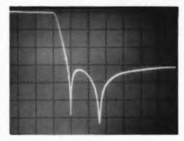
Fig. 2 — Response curve of the filter shown in Fig. 1. Vertical scale represents 10 dB/div. and horizontal scale is 10 MHz/div.
