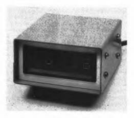
four LEDs as indicators. The normal display indicates the time in hours and minutes. Using the external switches it is possible to call up the seconds display, alarm time, and sleep time. The module used for this clock (MA1002A) is a 12-hour format that contains the clock/radio feature. There are two outputs available for controlling external devices. Each output (sleep or alarm) is a positive current source that can turn on an npn transistor for control purposes.
