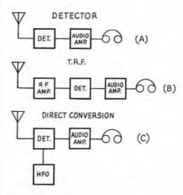
Fig. 8-3 - Block diagrams of three simple receivers.
