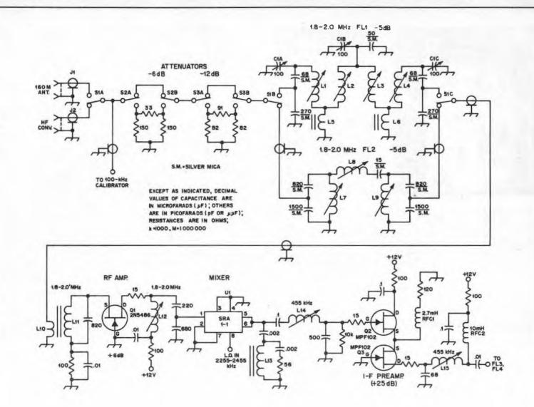
Q1, Q2, Q3 – Motorola JFET. RFC1 – 2.7-mH miniature choke (J. W. Miller Three-pole, two-position phenolic wafer S2, S3 — Two-pole, double-throw miniature toggle. U1 — Mini-Circuits Labs. SRA-1-1 doubly balanced - Mini-Circuits Labs. SRA-1-1 doubly balanced L15 — 1.3 to 3.0 mH, slug-tuned inductor (J. W. Miller 9059). RFC2 - 10-mH miniature choke (J. W. Miller diode mixer, (2913 Quentin Rd., Brooklyn, NY - 120 to 280 µH, slug-tuned inductor (J. W. 70F273A1). 70F102A1). switch. 1 S1
