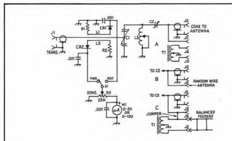
Fig. 20-22 — Circuit diagram of the Transmatch. The .001- $\mu$ F capacitors used are disk ceramic.
