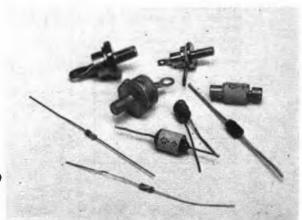
Typical silicon and germanium diodes of the present era. The larger units are designed to handle high current.
