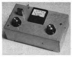
Fig. 17-56 — The deviation meter is constructed in a Calectro aluminum box. A four-position switch is at the lower right. The crystal plugs in on the left, with the frequency adjusting trimmer just below. A short whip or pickup wire can be plugged into the phono connector that is mounted on the back wall of the box.
