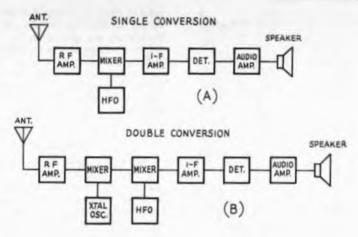
Fig. 8-12 — Block diagrams of a (A) single- and (B) double-conversion superheterodyne receiver.
