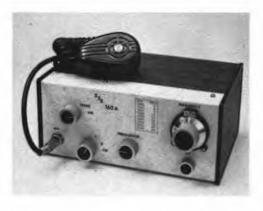
This ssb transceiver is suitable for QRP operation from batteries or as a main frame for fixed-station use. Its circuitry is simple enough to permit easy duplication (or substitution of components where necessary) by proficient builders with only limited experience in solid-state design.
