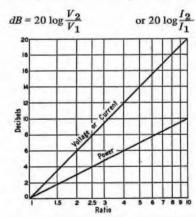
Fig. 2-36 - Decibel chart for power, voltage and current ratios for power ratios of 1:1 and 10:1. In determining decibels for current or voltage ratios the currents (or voltages) being compared must be referred to the same value of impedance.
