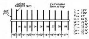
Fig. 22-13 — 11-element Yagi for 220 MHz. Dimensions are for maximum gain in the lower 2 MHz of the band. Recommended feed method is a delta match, with universal stub and balun. Delta sides should be about 3 inches, tapped 2 inches either side of the element midpoint.
