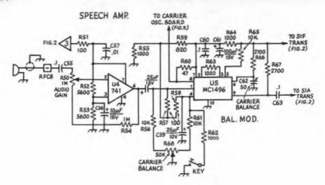
Fig. 7 – Schematic diagram of the speech amplifier and the balanced modulator boards.
