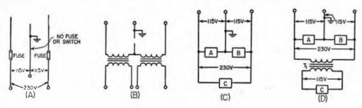
Fig. 5-1 — Three-wire power-line circuits. A — Normal 3-wire-line termination. No fuse should be used in the grounded (neutral) line. B — Showing that a switch in the neutral does not remove voltage from either side of the line. C — Connections for both 115- and 230-volt transformers. D — Operating a 115-volt plate transformer from the 230-volt line to avoid light blinking. T1 is a 2-to-1 step-down transformer.
