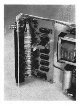
The use of a bezel and a single pc board allows very compact packaging in this counter. Leads that interconnect between the bezel and the circuit board have been made extra long. This excess length is tucked under the bezel and allows the pc board to be removed and worked on while still connected to the counter.
