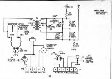
Fig. 1 — Circuit diagram for the 8877 two-kilowatt amplifier. Component designations not listed below are for text reference only.
