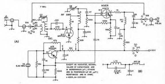
optimization of circuit values for each band of interest. The system used in this receiver calls for switching of only de and 50-ohm circuitry. Lowimpedance switching eliminates problems caused by long switch leads. Switching at high-impedance points, which is the usual technique in multiband receivers, can impair the quality of the tuned circuits and makes isolation of critical circuits more difficult.
