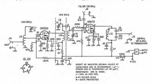
Fig. 7-10 — Diagram of the converter section. Resistors are 1/4-watt composition and capacitors are disk ceramic, except as noted otherwise.
