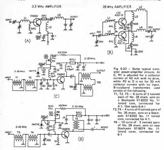
power-output curves of the transistors used, changing from 25 dB at 2 MHz to 13 dB at 30 MHz. IMD is typically 30 dB or more down with either circuit.
