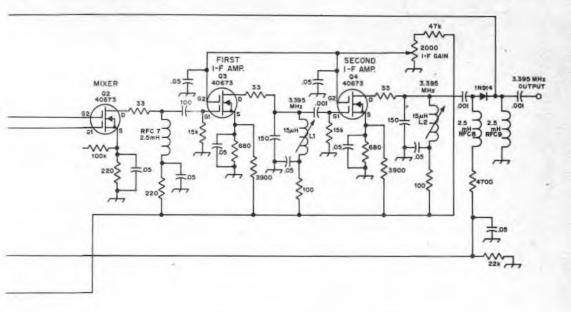
Fig. 1 — Circuit diagram for the Band-Pass Tuner. All resistors are 1/2-watt composition. FL1 and FL2 are Collins types. RFC's are from Millen. All capacitors are disc ceramic. The output of the Pass-Band Tuner should be connected in the receiver at a point before the receiver i-f filter system. The i-f control should be adjusted to give suitable gain when the unit is placed in operation as outlined in the text.
