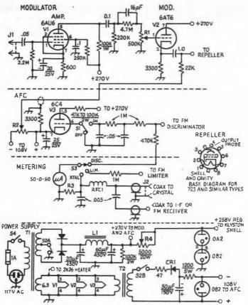
Fig. 3-25 — Schematic diagram and parts information for a power supply and control unit suitable for amateur microwave transceivers. Unless otherwise specified, capacitor values are in μF and resistors are 1/2-watt composition.
