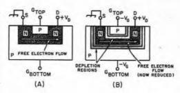
Fig. 4-20 — Operation of the JFET under applied bias. A depletion region (light shading) is formed, compressing the channel and increasing its resistance to current flow.
