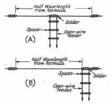
Fig. 21-12 — The half-wave antennas can be fed at the center or at one end with open-wire feeders. The length of the antennas can be computed from Equation 21-8 or Fig. 21-4.
