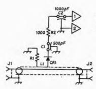
Fig. 22-25 — Circuit diagram for the line sampler. C1 — 500-pF feedthrough capacitor, solder-in type. C2 — 1000-pF feedthrough capacitor, threaded type.
