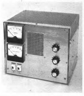
Fig. 7-27 — Table-top 50-MHz amplifier of grounded-grid design, only 10 X 12 inches in size. Grid and plate current are monitored simultaneously. Knobs at the right are for input tuning, bottom, amplifier loading, center, and plate tuning, top.
