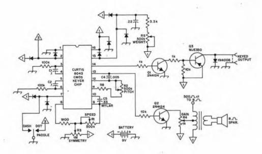
Fig. 1 — Circuit diagram for the keyer. All diodes are 1N4006 or equiv. All potentiometers are linear taper and resistors are 1/2 or 1/4 watt.
