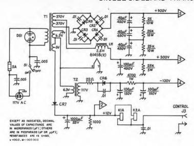
Fig. 2- Diagram of the power-supply section. Resistors are 1/2-watt composition. Capacitors are disk ceramic, except those with polarity marked which are electrolytic. CR2-CR5, incl. - Silicon, 1000 PRV, 1 A.
