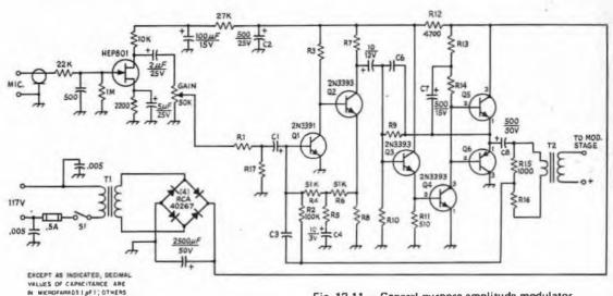
Fig. 12-11 — General-purpose amplitude modulator for 3 to 20 watts of audio power. Capacitors with polarity indicated are electrolytic, See Table 12-I for parts not listed below.
