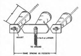
Fig. 23-3 — A simple lightning arrester made from three stand-off or feedthrough insulators and sections of a 1/8 × 1/2-inch brass or copper strap. It should be installed in the open-wire or Twin-Lead line at the point where it is nearest the ground outside the house. The heavy ground lead should be as short and direct as possible. Gap setting should be minimum for transmitter power.
