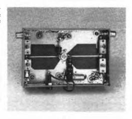
Completed amplifier. Phone plugs were used for this first model. In actual use better vhf connectors should be installed.
