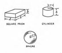
Fig. 2-64 - Forms of cavity resonators.
