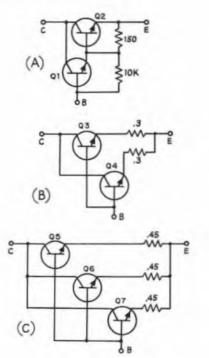
Fig. 5-25 — At A, a Darlington-connected pair for use as the pass element in a series-regulating circuit. At B and C, the method of connecting two or more transistors in parallel for high current output. Resistances are in ohms. The circuit at A may be used for load currents from 100 mA to 5 A, at B for currents from 6 to 10 A, and at C for currents from 9 to 15 A.
