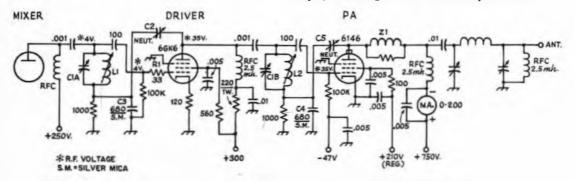
Fig. 13-16 — Schematic diagram of a typical driver and final stage for ssb exciter. Neutralization and parasitic-suppression circuits have been included.
