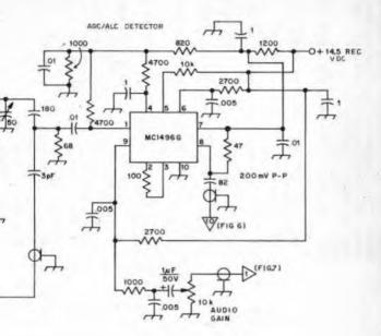
EXCEPT AS INDICATED, DECIMAL VALUES OF CAPACITANCE ARE IN MICROFARADS (JF); OTHERS ARE IN PICOFARADS (JF); RESISTANCES ARE IN OHMS; b=1000, M=1000,000
