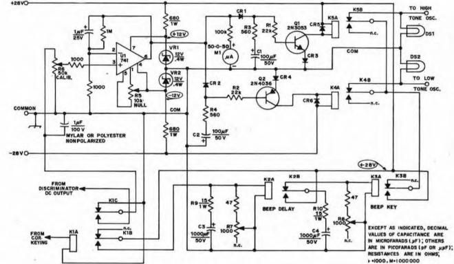
output of the 741 with K1 R5, NULL point of K4 or control, Fig. 1 — The schematic diagram of the tone-beep keyer. A dual 28-V K5 is adjusted by deenergized. for zero dc volts supply is used in this system, but there should be no difficulty in revising values to make use of lower voltages. The charging current of C1 through C4 is limited to a safe value by means of the series resistor in each case. If the meter is omitted, tip jacks should be provided to aid in adjusting the circuit.
