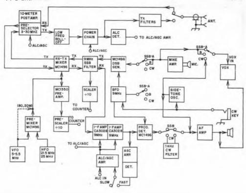
Block diagram for the K1ZJH transceiver. The counter circuit is not included.
