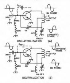
Fig. 4-11 — Transit-time effects (in combination with base-collector capacitance Cbc) can cause the positive-feedback condition shown at A. Normally, the phase of the collector signal of an amplifier is the inverse of the base signal. Positive feedback can be corrected by using unilateralization, feeding an equal amount of opposite-phase signal back to the base through Uc. Neutralization is shown at B, and deals with negative feedback, as can be seen by the phase relationships shown.
