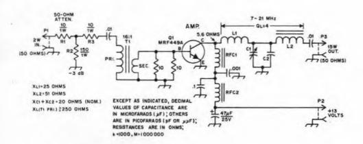
Fig. 1 — Schematic diagram of the 15-watt amplifier. Fixed-value capacitors are disk caramic unless otherwise noted. Resistors are 1/2-watt composition unless specified differently. The 47-μF capacitor can be electrolytic or tantalum.
