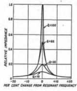
Fig. 2-42 — Relative impedance of parallel-resonant circuits with different Qs. These curves are similar to those in Fig. 2-39 for current in a series-resonant circuit. The effect of Q on impedance is most marked near the resonant frequency.
