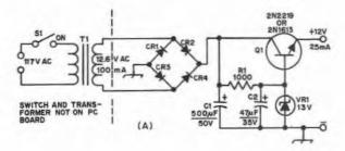
Fig. 7 — Schematic diagram and parts-placement guide for the power supply to the converters. The transformer is mounted external to the board. Pc board size is identical to the one used for the converters.
