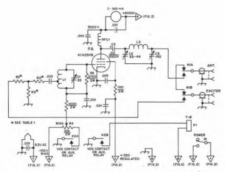
Fig. 1 — Schematic diagram of the amplifier. Unless otherwise specified, capacitors are disk ceramic and resistors are carbon composition.
