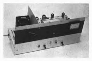
Fig. 7-7 — Panel view of the 2-meter transverter. This version is patterned after a transmitting converter design by K9UIF. The on-off switches for ac and dc sections of the power supply are mounted on the front panel of the unit as are the pllot lamps and plate meter for the PA stage. The tuning controls for the various stages are accessible from the top of the chassis.
