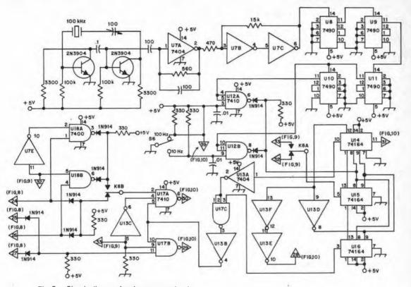
Fig. 9 - Circuit diagram for the counter circuits.
