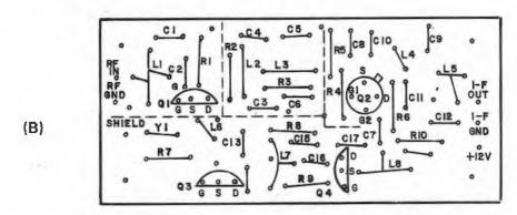
Fig. 4 — Parts-placement guide for the six-meter converter, A, and the two-meter converter, B. View is from the foil side of the board. Dashed lines show the location of shields that are soldered to short pieces of wire which project through holes in the pc board. The shields may be fabricated from sheet brass or copper, or scraps of copper-clad board material.
