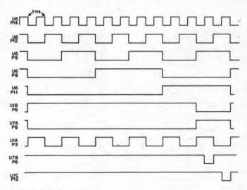
Fig. 2 - Timing diagram of the counter.
