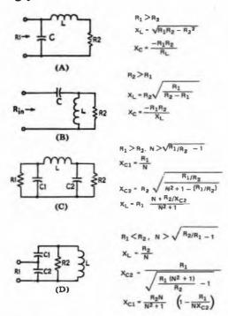
Fig. 14 — Four matching networks that can be used to couple a source and load with different resistance values. (Although networks are drawn with R1 appearing as the source resistance, all can be applied with R2 at the source end.)
