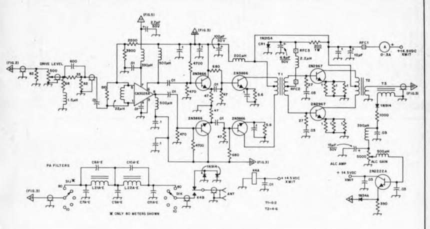
Fig. 3 — Circuit diagram for the transmitter power chain. See Table I for capacitor values.
