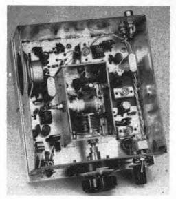
Interior view of the receiver. The front end is at the lower right. The leads of U1 are bent to align with an 8-pin dual-in-line IC socket. The rim of the speaker is tack-soldered to the pc-board side wall at two points. The 20-meter converter mounts on the rear wall inside the receiver (upper left corner).
