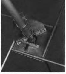
Fig. 21-27 — The ground-plane antenna partially assembled (left) and completely assembled, ready for installation (right). Both views are looking down on the base plate, which is in an inverted position in these photos. In the view at the right may be seen an added bracket which supports a coaxial chassis connector, type SO-239, and the shunt inductor. A right-engle connector is used at the chassis connector to avoid a bend in the coax, which is secured to the mast during installation.
