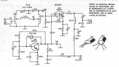
Fig. 8 — Schematic diagram of the 80-mater converter, Capacitors are disc ceramic, Resistors can be 1/4- or 1/2-watt composition types.
