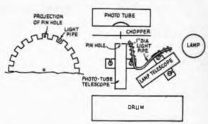
Fig. 2 — Addition of a fiber-optics light pipe for transmission of positive pictures.
