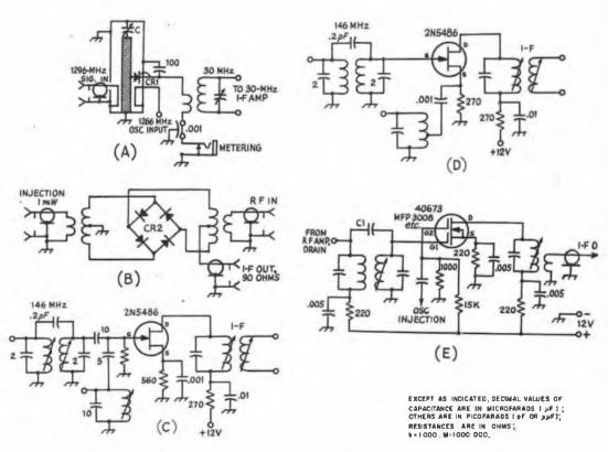
Fig. 9-8 — Whf and uhf mixer circuits. A diode mixer for 1296 MHz, with a coaxial circuit for the signal frequency, is shown in A. CR1 is a uhf diode, such as the 1N21 series. A balanced mixer, as in B, gives improved rejection of the signal and injection frequencies. If hot-carrier diodes are used for CR2, sorting for matched characteristics is eliminated. Gate and source injection of a JFET mixer are shown at C and D, respectively.
