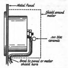
Fig. 16-11 - Meter shielding and bypassing. It is essential to shield the meter mounting hole since the meter will carry of through it to be radiated. Suitable shields can be made from 2 1/2- or 3-inch diameter metal cans or small metal chassis boxes.
