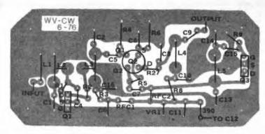
Fig. 2 — Etching pattern and parts-placement guide for the converter circuit board. 1/2-watt resistors were used throughout, but 1/4-watt resistors may also be used if preferred.
