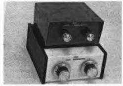
Fig. 22-21 — These 6- and 2-mater Transmatches may be used with powers up to 500 watts. They can be employed with either balanced or unbalanced feeders.
