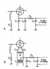
Fig. 11-3 — The basic cathode (A) and center-tap (3) keying circuits. In either case C1 is the rf return to ground, shunted by a larger capacitor, C2, for shaping. Voltage ratings at least equal to the cutoff voltage of the tube are required. T1 is the normal filament transformer, C1 and C3 can be about .01 µF.
