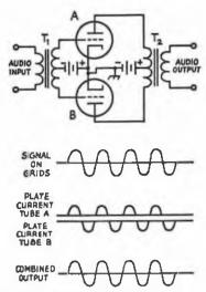
Fig. 3-13 — Class B amplifier operation.
