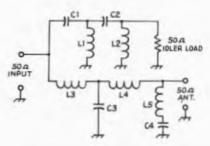
Fig. 1 — Schematic diagram of the absorptive filter. The pc board used is MIL-P-13949D, FL-GT-.062 in, C-2/2-11017, Class 1, Grade A. Polychem Bud Division. Capacitance between copper surfaces is 10-pF per square inch. Values are as follows for a design cutoff frequency of 40 MHz and rejection peak in Channel 2:
