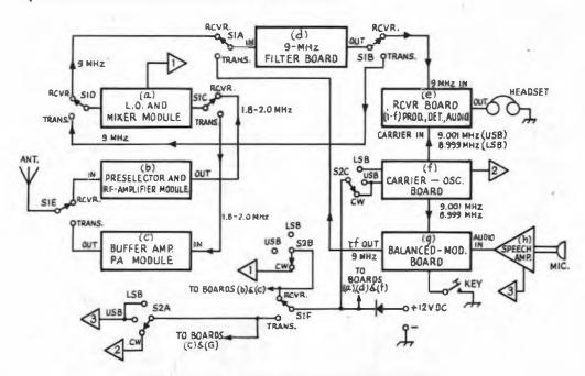
Fig. 2 - Block diagram & switching logic of the transceiver,
