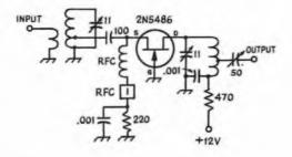
Fig. 9-2 — Grounded-gate FET preamplifier tends to have lower gain and broader frequency response than other amplifiers described.
