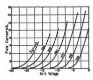
Fig. 3-6 — Grid-voltage-vs.-plate-current curves at various fixed values of plate voltage  $(E_{\rm b})$  for a typical small triode. Characteristic curves of this type can be taken by varying the battery voltages in the circuit at the right.
