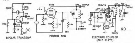
Fig. 6-4 — Crystal-oscillator circuits that are designed to deliver power. L1/C1 resonate at the crystal frequency, or a multiple thereof if the second, third, or fourth harmonic is the desired output frequency.
