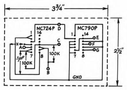
Fig. 17-32 -Wiring plan for the circuit board, component side. Dimensions for placement of parts are exact. X – jumper, Other letters indicate external connection points, corresponding to similarly lettered connections in Fig. 17-30.
