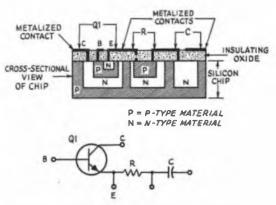
Fig. 4-23 — Pictorial and schematic illustrations of a simple IC device.
