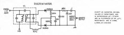
Fig. 14-16 — Typical frequency-discriminator circuit used for fm detection. T1 is a Miller 12-C45.
