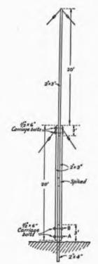
Fig. 2 — A simple and sturdy most for heights in the vicinity of 40 feet, pivoted at the base for easy erection. The height can be extended to 50 feet or more by using 2 X 4s instead of 2 X
