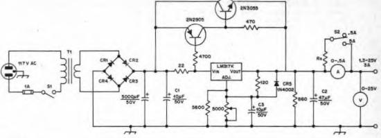
Fig. 2 — Schematic diagram of the complete power supply. All resistors are 1/2 watt composition. C1 through C3 are solid tantalum capacitors. T1 and CR1 through CR4 are discussed in the text. R1 is a panel-mounted linear-taper potentiometer. S1 and
