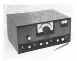
signal levels during on-the-air experiments with other stations (antennas, amplifiers and such). Also, FL2, a fixed-tuned 1.8- to 2-MHz bandpass filter, need not be included if the operator is willing to repeak the three-pole tracking filter (FL1) when tuning about in the band. The fixed-tuned filter is useful when the down convergers are in use.
