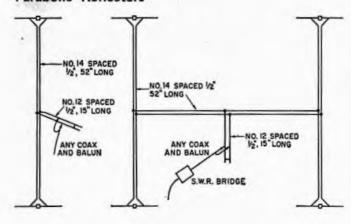
Fig. 22-15 — Phasing methods for using two or four 11-element Yagis for 432 MHz, with 2-wavelength spacing. Universal-stub match permits use of any type of transmission line.
