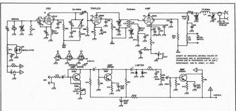
Fig. 7-15 — Schematic diagram and parts information for the W1QWJ 220-MHz exciter and frequency modulator. Capacitors with polarity marked are electrolytic. Components not specified below are marked for text reference purposes. C1 through C5 are dipped mice or silver mice.
