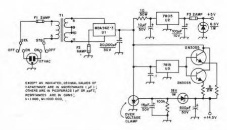
Fig. 11 — Circuit diagram for the transceiver power supply. U2 and U3 are manufactured by Fairchild. VR1 is a General Electric type C35B. U1 is from Motorola. T1 is a Stancor RT-204.
