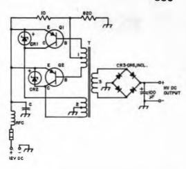
Fig. 10-26 — Typical dc-to-dc converter. Ratings for CR3-CR6, and the 100-μF filter capacitor can be selected from data in the power-supply chapter.
