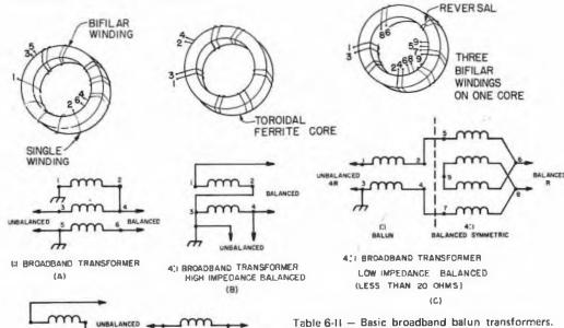
BALANCED \_ Bifilar windings are six to ten turns, depending on the ferrite-core permeability. A suitable ferrite material is Q1 with a permeability of 125. Very small size cores (1/4-to 3/4-inch OD) may be used for receiving and low-power applications. For full-power applications a 2-1/2-inch OD Q1 core with 1/2-inch cross section wound with No. 14 UNBALANCED LIPHASE REVERSING AUTO-TRANSFORMER TRANSFORMER Formex copper wire, seven turns per winding, is (E) (G) recommended
