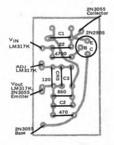
Fig. 3 — Template for pc board. View from the foil side.
