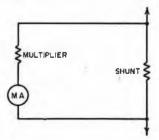
Fig. 17-4 — Voltmeter method of measuring current. This method permits using relatively large values of resistance in the shunt, standard values of fixed resistors frequently being usable. If the multiplier resistance is 20 (or more) times the shunt resistance, the error in assuming that all the current flows through the shunt will not be of consequence in most practical applications.
