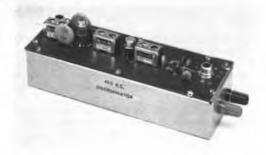
Fig. 14-23 — The solid-state fm adapter is constructed on a 6 X 2-inch atched-circuit board, mounted on a homemade chassis.
