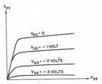
Fig. 4-21A-Typical JFET characteristic curves.
