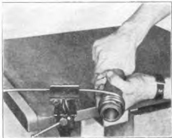
WINDING A COPPER-TUBING INDUCTANCE
