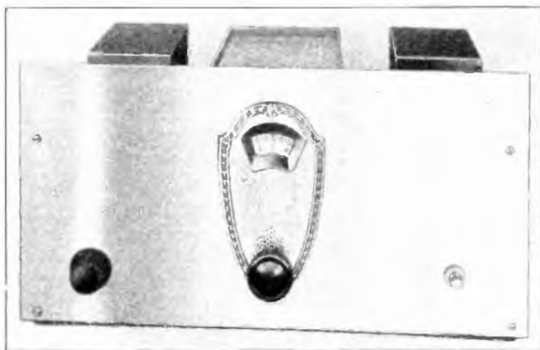
PANEL VIEW OF THE THREE-TUBE A. C. RECEIVER
