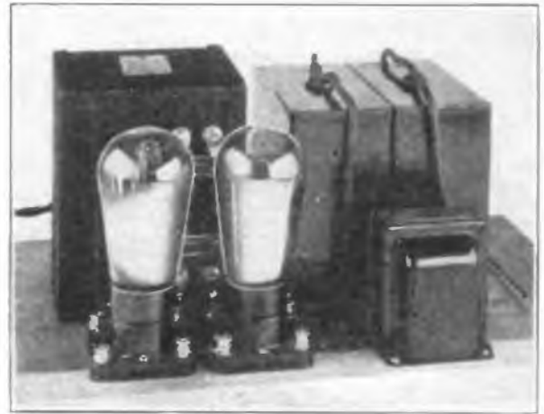
COMPLETE POWER SUPPLY
