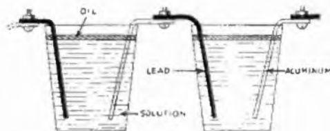
TYPICAL CHEMICAL RECTIFIER CELLS
