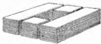
ANOTHER METHOD OF BUILDING A CORE FOR A CHOKO COIL
