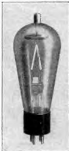
A TYPICAL HOT-CATHODE MERCURY-VAPOR RECTIFIER TUBE
