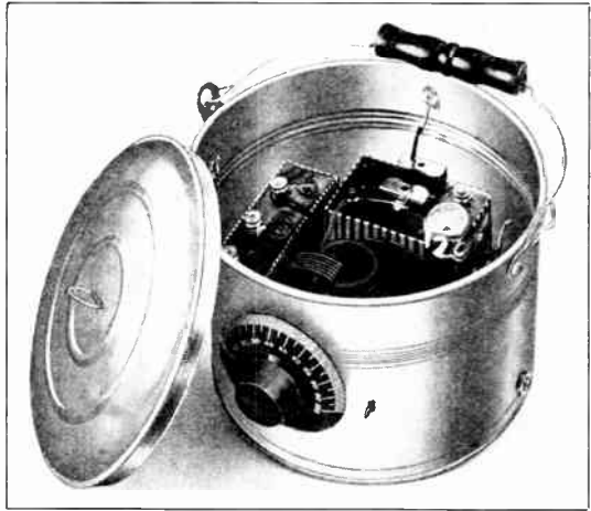
THE MONITOR-BOX USED TO CHECK THE CHARACTER OF THE SIGNAL
