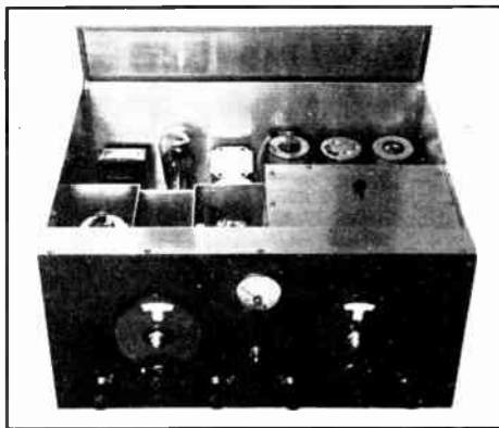
FIG. 531 — A TYPICAL SINGLE-SIGNAL TYPE SUPERHETERODYNE CUSTOM BUILT BY HENDRICKS & HARVEY
