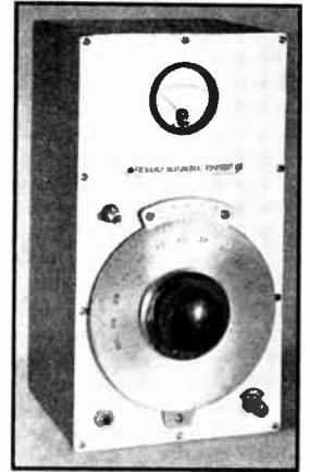
FIG. 66. — A PANEL VIEW OF THE ELECTRON-COUPLED FREQUENCY METER
