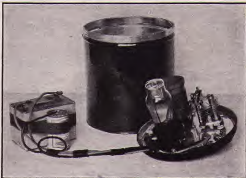
FIG. 601 — AN INEXPENSIVE MONITOR BUILT IN A CRACKER TIN The simple construction shown above is typical. The monitor, despite its simplicity and low cost, is an indispensable piece of station equipment.
