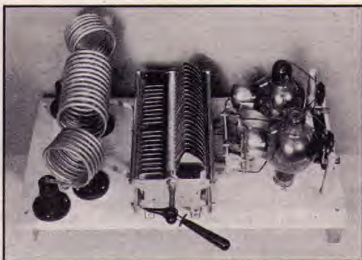
FIG. 729 — A TYPICAL EXAMPLE OF THE USE OF 852 TUBES IN A PUSH-PULL AMPLIFIER
