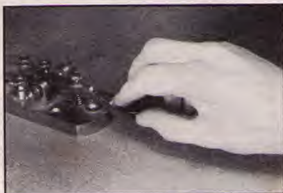
ILLUSTRATING THE CORRECT POSITION OF THE HAND AND FINGERS FOR THE OPERATION OF A TELEGRAPH KEY
