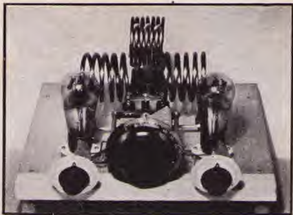
FIG. 708 — A PUSH-PULL OSCILLATOR
