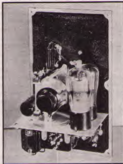
FIG. 608 — AN INTERIOR VIEW OF THE TWO-TUBE E. C. FREQUENCY-METER-MONITOR
