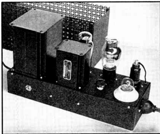
Fig. 1206—Power-supply for the 10-watt amplifier. A voltage-regulator is incorporated for all speech-amplifier tubes except the 2A3's.
