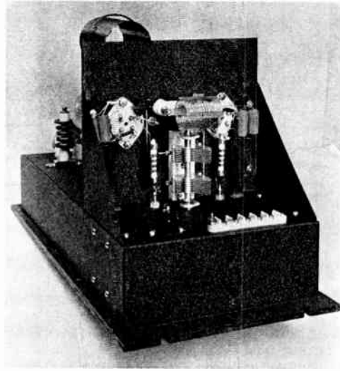
Fig. 1036 — The grid-circuit components of the 450-watt amplifier are mounted on this side of the partition which is braced by standard 5-in. triangular brackets. The tank condenser is mounted by means of a screw in the hole which remains when the shield between the stators is removed. The ceramic terminal strip is for all external connections except for positive high voltage for which a special safety terminal is provided. A large clearance hole should be cut in the chassis for the condenser shaft. The shaft should come at the center line of the chassis.
