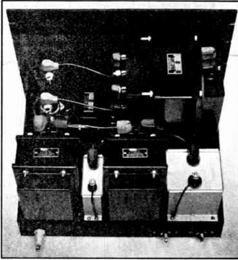
Fig. 1126 — This unit delivers 2025 and 2480 volts at full-load current of 450 ma. with a ripple of 0.5% and regulation of 19%. Voltages are selected by taps on the secondary. All exposed high-voltage terminals are covered with Sprague rubber safety terminal caps and the tube plate terminals with moulded caps. The rectifier tubes are spaced away from the plate transformer to avoid induction troubles. The panel is 14 in. by 19 in., and the chassis 13 in. by 17 in. by 2 in. The exposed high-voltage terminal should be covered with a rubber-tubing sleeve.
