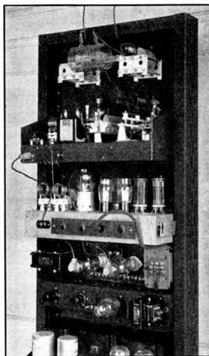
Fig. 1313 — Rear view of 150-watt phone transmitter showing antenna coupler, r.f. final amplifier, exciter, modulator and speech amplifier.
