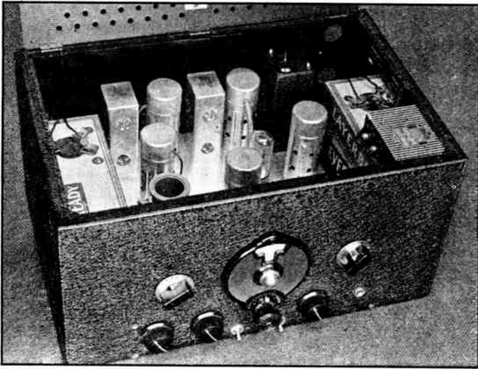
Fig. 822 — A 6-tube dry-battery superhet receiver. Self-contained, it can be used in any location where line power is not available.
