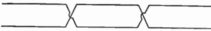
Fig. 1008 — Method of transposing a two-wire open transmission line to preserve balance to ground and nearby objects.
