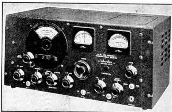
◆ Fig. 1120 — The Hallicrafter S-27 u.h.f. receiver can be used for either a.m. or f.m. reception. The scale at the left indicates the frequency — the center scale is a vernier reading for accurate logging of signals. ◆
