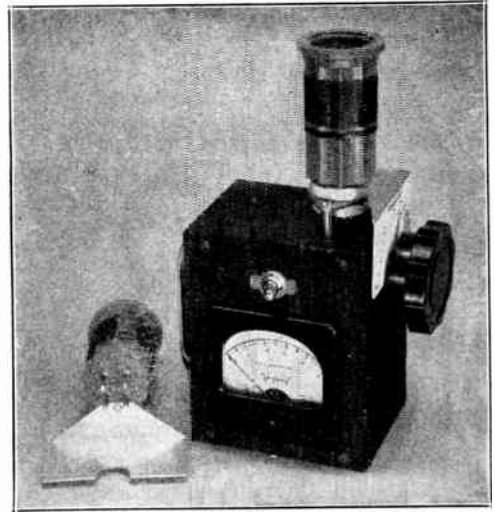
Fig. 1202 — A sensitive absorption frequency meter with a crystal detector-rectifier and d.c. milliammeter indicating circuit. Individual calibration charts mounted on each coil form make the meter direct-reading. A toggle switch connects a 10-ma. shunt across the 0-1 ma. meter; the 10-ma. range is used for preliminary readings, to avoid burning out meter or crystal. The meter gives indications several feet from a low-power oscillator.
