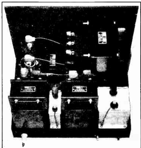
Fig. 1342 — This power-supply unit delivers 2025 or 2480 volts at full-load current of 450 ma., with ripple of 0.5 per cent and regulation of 19 per cent. Voltages are selected by taps on the secondary. All exposed high-voltage terminals are covered with Sprague rubber safety caps and the tube plate terminals with moulded caps. The rectifier tubes are placed away from the plate transformer to avoid induction troubles. The panel is 14 × 19 inches and the chassis 13 × 17 × 2 inches. The exposed high-voltage terminal should be covered with a rubber-tubing sleeve. The circuit is shown in Fig. 1343.
