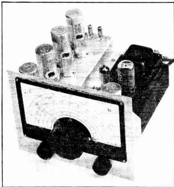
Fig. 1221 — A 28-Mc. converter that uses fixed-tuned r.f. stages and thus eliminates the ganging problem. The knob at left is for the "send-receive" switch, and the right-hand knob is for gain control.
